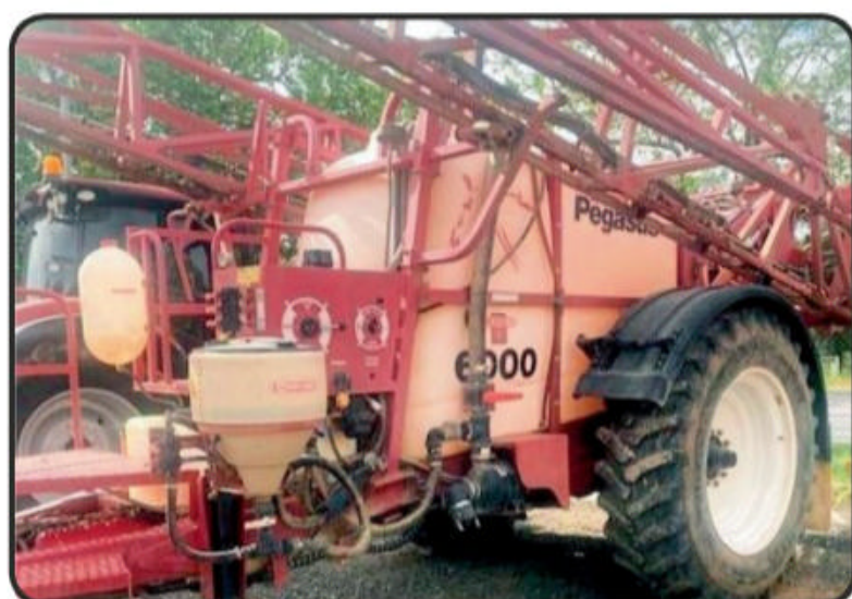
CROPLANDS PEGASUS 6000 trailed boom sprayer, 6000L main tank, 36M boom, 7 sections, BA7000 rate controller, 3 inch hydraulic drive fill pump, left and right fence nozzles. TA1154542. $33,000
