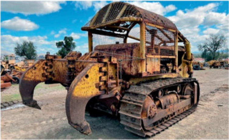
ALLIS CHALMERS HD16DC Just in for dismantling, swivel tyne pacific rippers, near new late style undercarriage all round, Allis 16,000 engine, final drives rebuilt, bull tilt blade, all parts available, Phone Brendan or Pete on 02 6762 4466. S173. TA1153539. POA
