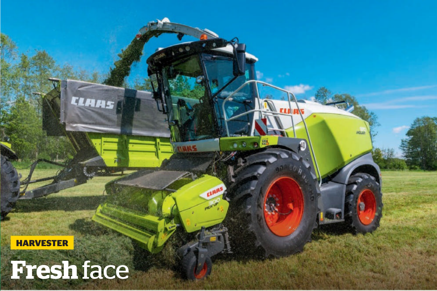
The speeds of the pick-up reel and intake auger match to the prevailing conditions with Claas's new optional hydraulic drive system.
