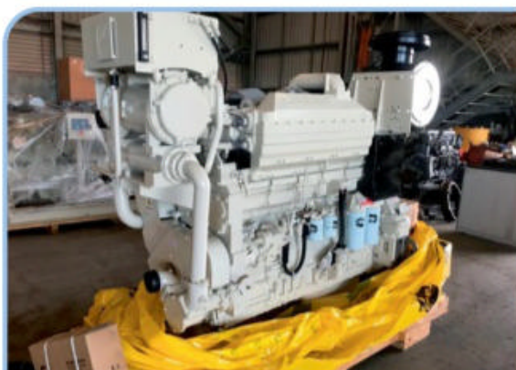
NEW CUMMINS KTA19-M500 500HP HEAT EXCHANGER COOLED
