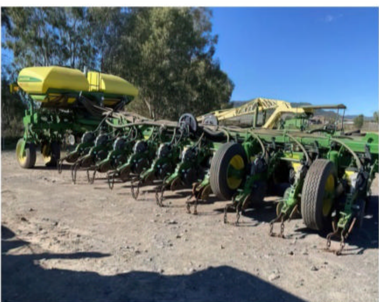
2013 John Deere 1770NT CCS Planter, 60ft, 24 rows on 30 inch spacings, seedstar 2 less monitor, command row clutches, tapered teeth, pneumatic down force, walking guage wheels, aari rate transmission.
