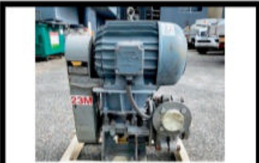
WARMAN PUMP 2X1 1/2 TYPE M slurry pump with 7.5kW 3 phase motor. Over under belt driven 7.5kW 3 phase. Pump has new impeller, casing liner & gland seals. This unit is fitted to a steel base plate with 4x lifting lugs and forklift tine slots. Has incorporated motor starter and 6m three phase power cable with 4 Pin 20 AMP male plug top, N/A. VIC. DIY1153153. 0418 331 405. $3,300
