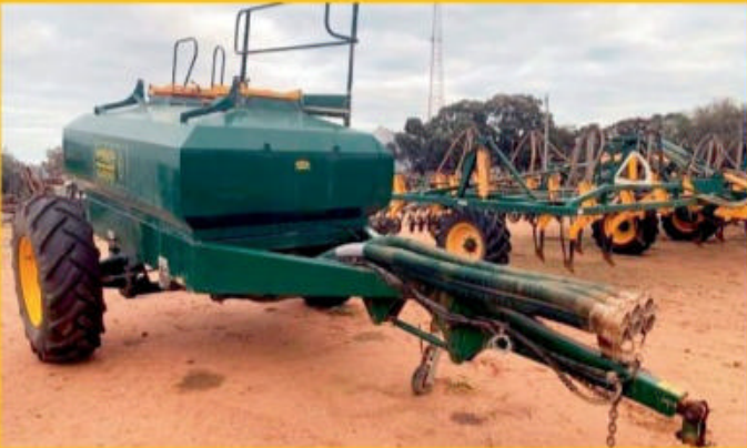
SIMPLICITY 6000TR2 2008, 6000 litre, 2 bin trailed cart, HD hydraulic motor. AS1585. TA1140730. $71,500
