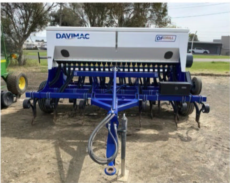
2018 Davimac DF Drill Trailing drill, 24 run on 6 inch spacing, double shoot, direct drill points, 11.5/80.15.3 implement tyres, rear platform, new points with machine but not fitted. Machine presents 9/10.
