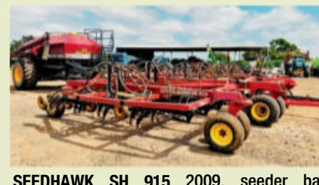
SEEDHAWK SH 915 2009, seeder bar SH915, 35ft sowing widthm 40 openers @ 10" spacing, 9mtr working width, unit in good condition, older bar but current model layout. HC2233. TA1126589. $99,000
