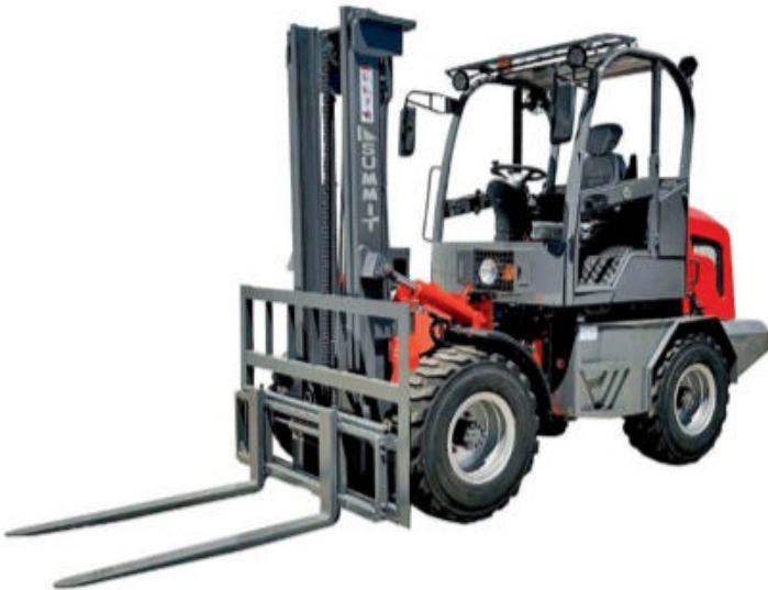
SUMMIT H20 2 ton 4WD Rough Terrain 50HP diesel engine, constant 4WD, 2000kg capacity, 3300kg operating weight, 2 speed power shift, 2 stage 3.5 meter mast with side shift. S14. TA1101875. $29,500 Inc GST
