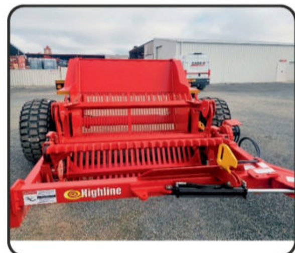
HIGHLINE NT78 2022, new 2022 rockpicker, hydraulic drive, 2mt picking width, 2.5CMT bucket. TA1140043. POA
