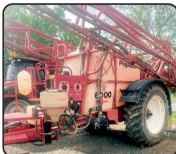
CROPLANDS PEGASUS 6000 trailed boom sprayer, 6000L main tank, 36M boom, 7 sections, BA7000 rate controller, 3 inch hydraulic drive ifil pump, left land right fence nozzles. TA1154542. $33,000
