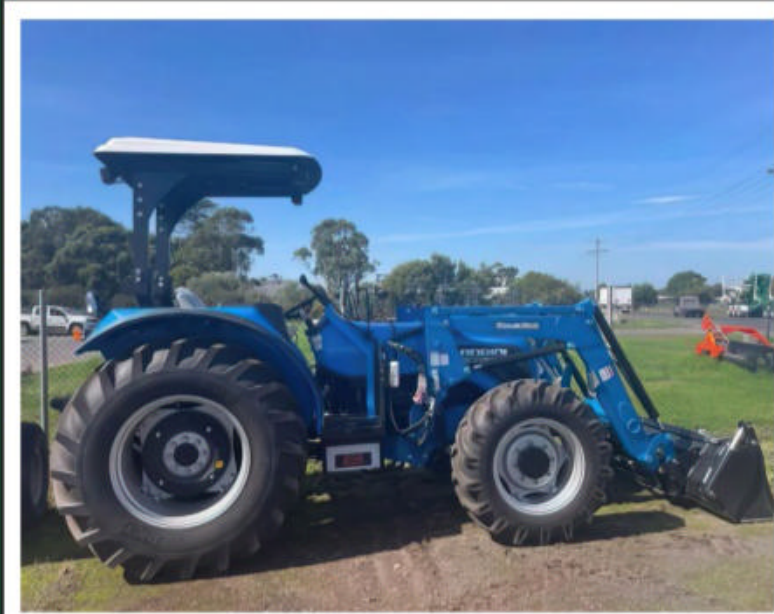
Landini Discovery 75 Comes standard with 4 cylinder 4100 turbo charged diesel engine, large 78 litre fuel tank.
