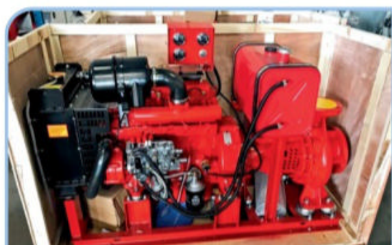
BRAND NEW 4" DIESEL, POWERED WATER PUMP MODEL WP100Y, 4 CYLINDER DIESEL, 80M3 /HR 20M HEAD
