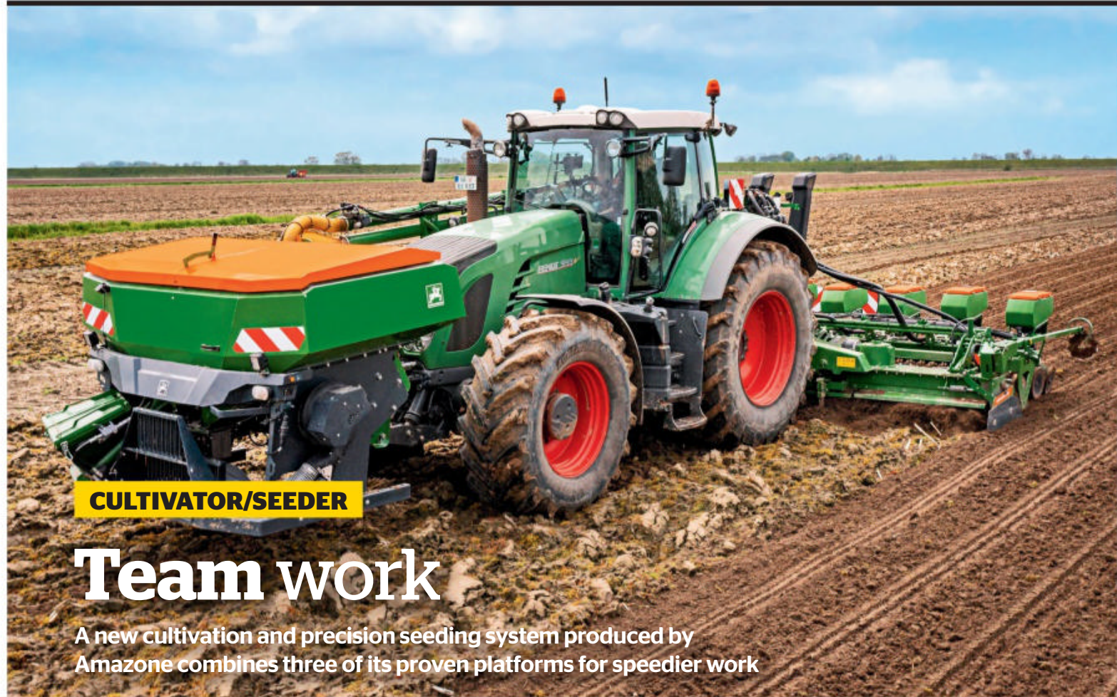
Amazone's new Precea 6000-2AFCC fitted with a 2200 litre FTender front-mounted hopper
