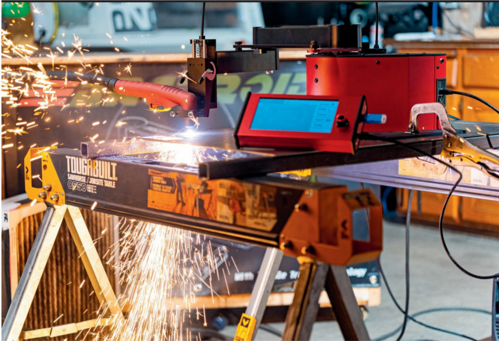
The ArcDroid CNC portable plasma robot boasts Simple Trace technology that make it ideal for onsite structural work, agricultural repairs and vehicle restoration.
