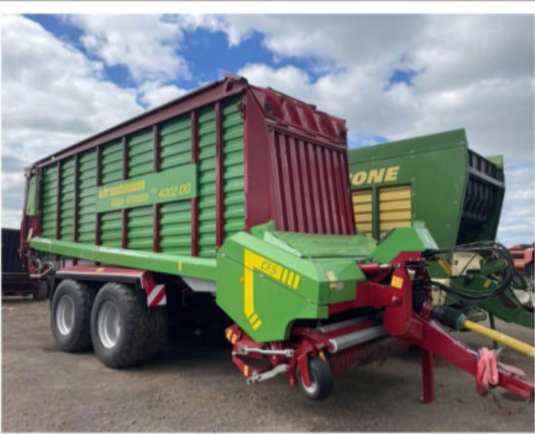
2019 Strautmann Giga Vitesse 4002 Cutting length of 35 mmr knife change without use of tools knife bar can be hydraulically swivelled out.
