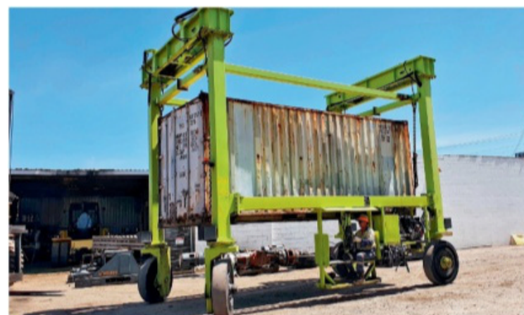
ISOLOADER 21 load unload and travel with 27t 20' and 40' containers. New Kohler diesel - Low cost container handler. R3621. TA1061595.
