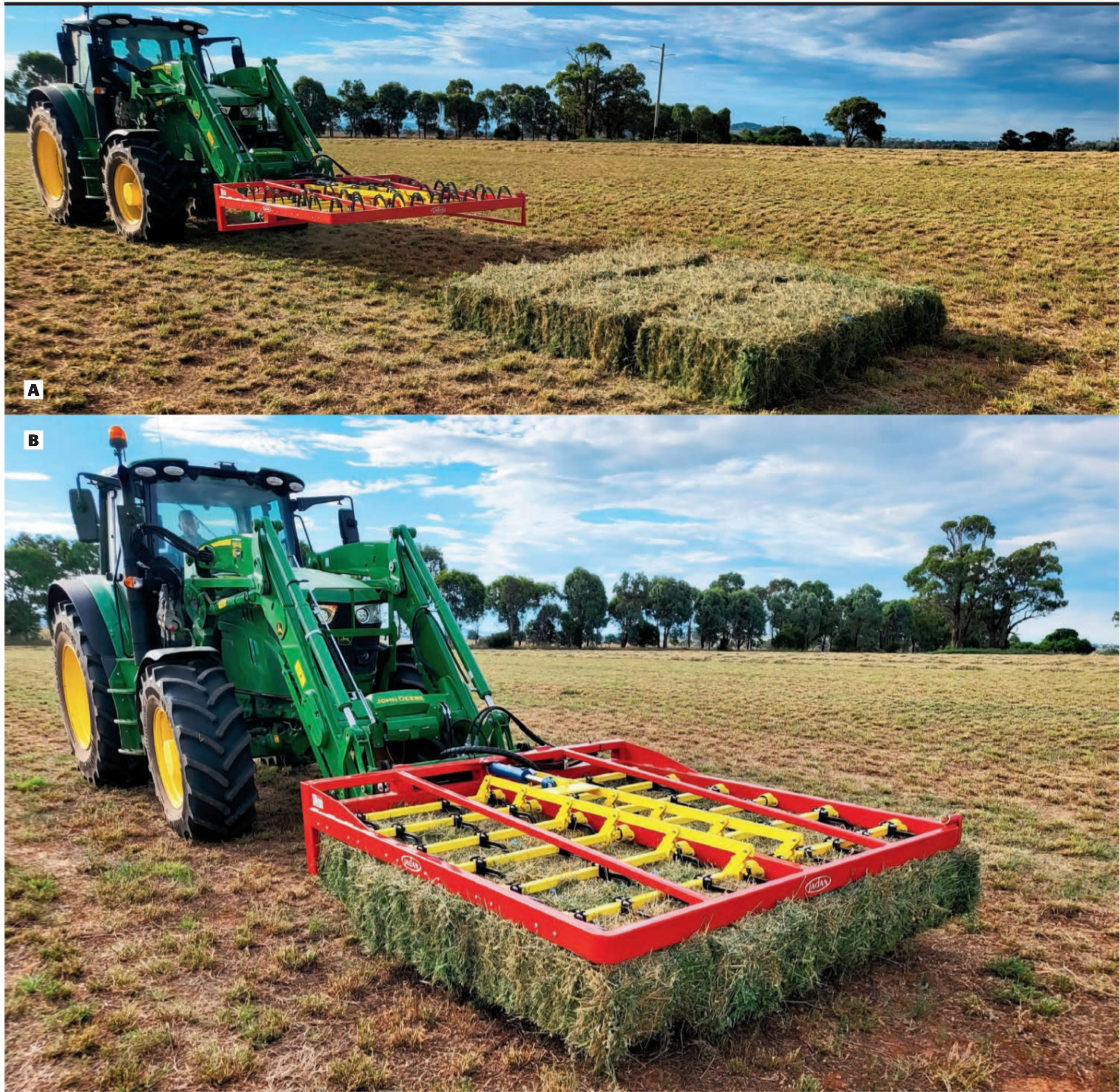
A An upgraded head design means a stronger frame B The new lower clearance grab has been designed for tight spaces
