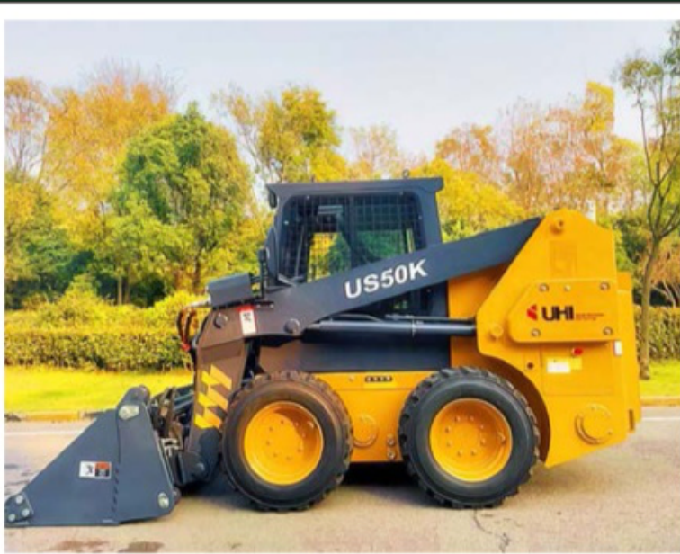
Uhi U550K 68 HP, EUROS, 900KG loading capacity, 4in1 bucket. Yanmar engine.
