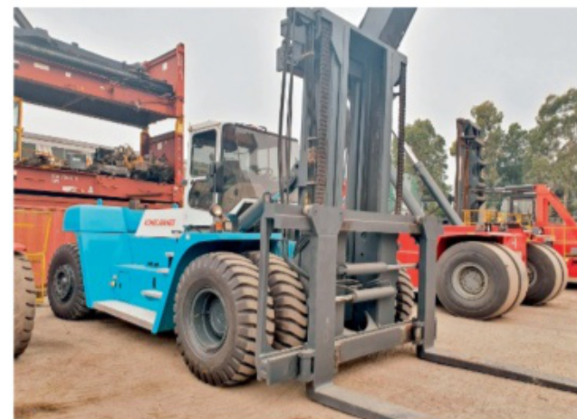
KONECRANES SMV SL32-1200B 2011, rated 32,000kg at 1200mm load centre 1 can stack highcube 20' containers 2 high and can transport without need to dismantle. R3376. TA1038152.
