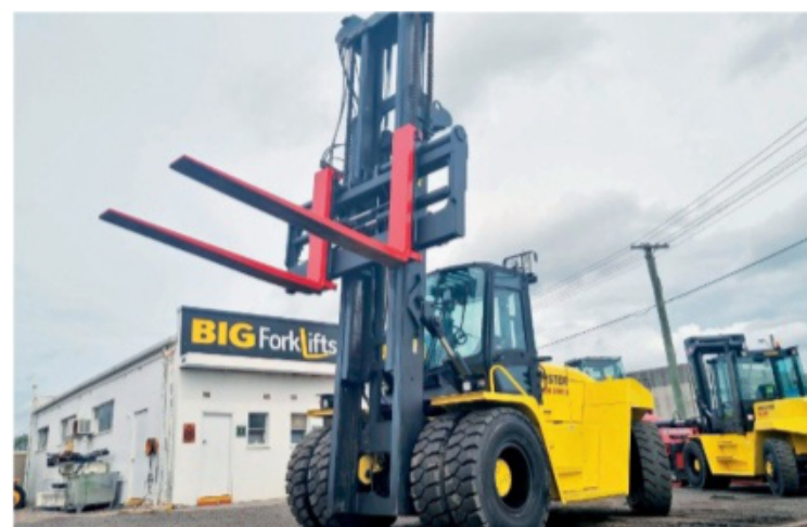
HYSTER H18.00XM-12 with fork positioning sideshift carriage, 2440mm long forks, Cummins engine, fully enclosed air conditioned cab. R3632. TA1124211.
