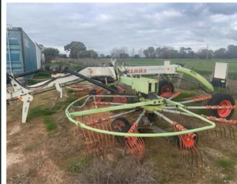
Claas liner 2600 Class twin rotor rake with hydraulic width adjustment.
