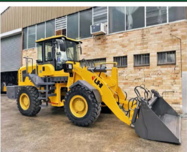
UHI UWL350 New wheel loader, 6 cyl cummins, auto trans, 3500kg load rated.
