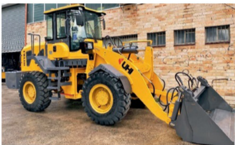
UHI UWL350 3.5T loading capacity, 150HP Cummins engine, free 4in1 bucket and fork attachment. S25. TA1132093. $69,990
