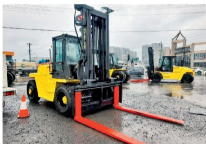
HYSTER H12.00XL sideshift and 8' forks, serated 8,100kg at 1200mm load centre able to stack highcube 20' container 2 high. Easy Mast on delivery. Perkins diesel. R3664. TA1124218.
