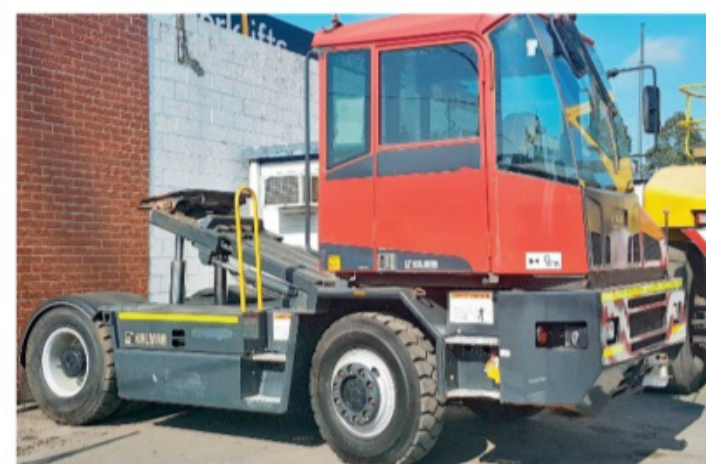
KALMAR TR618I 2014, ideal for trailers to from RoRo or Barge. 32,000kg at 5th wheel, boom has 1000mm lift height. Fwd and Rev Driver controls. Volvo diesel and Dana Trans with SISU drive and steer axles. R3552. TA899444.
