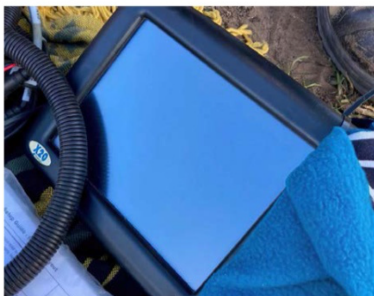
Topcon X20 Electric steering wheel, Nav controller with receiver and modem for full RTK.
