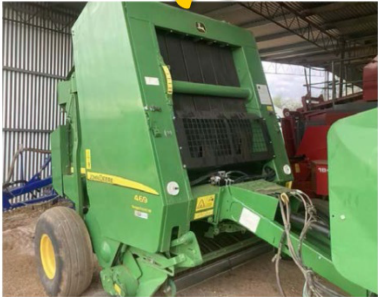
2016 John Deere 469 Silage Special Round baler, 19879 bales, 6 x 4 with coveredge surface wrap, bale push bar, hi flotation tyres and variable core valve. Located Albury.
