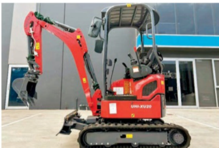
UHI XU20 Top brand quality, 1900kg operation weight, 15.8hp Kubota diesel engine, swing boom, expandable track, free 4 attachments. S10. TA1090064. $32,000
