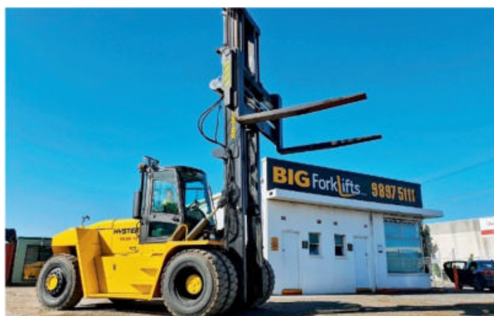
HYSTER H18.00XM-12 2008, 18,000kg highcube 20' containers 3 high with 2440 forks + fork positioning sideshift. Option 14,000kg with ELME 558 Sidelift for 20' and 40' highcube. R3282. TA511086.
