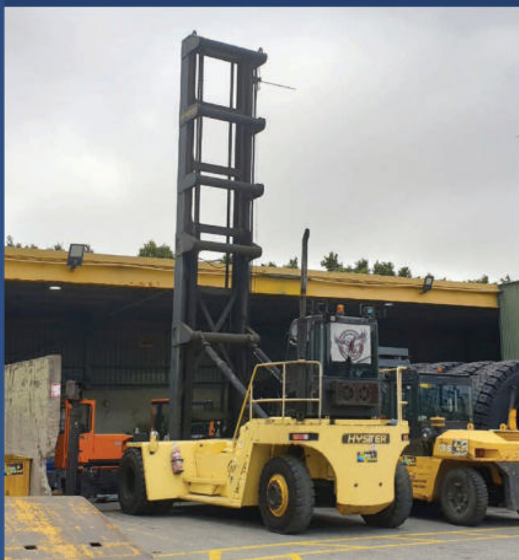
HYSTER H22.00XM-12EC LIFTING CAPACITY: 9000KG, CUMMINS / QSB6.7, LOAD CNTR OF GRAV: 1219 MM
