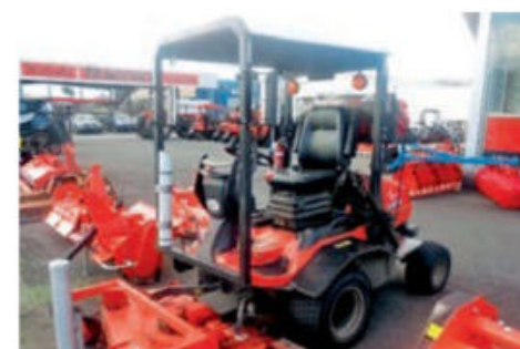
KUBOTA F3690 REAR DISCHARGE 60" rear discharge deck Comfort air seat 4 post roof 2 range hydrostatic. S613. TA1131269. $17,990
