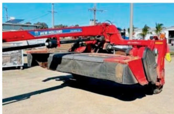
NEW HOLLAND 313 MOWER CONDITIONER Rubber roller mower conditioner, 4 meter cut. 3 meter chevron rollers, center pull, three point linkage 1000rpm pto. At our Echuca dealership. S494. TA1102279. $37,400
