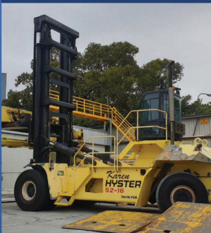
HYSTER H52.00XM MAXIMUM LIFT: 52000KG, DIESEL, MAX LIFT: 9755CM, 20 40 SPREADER
