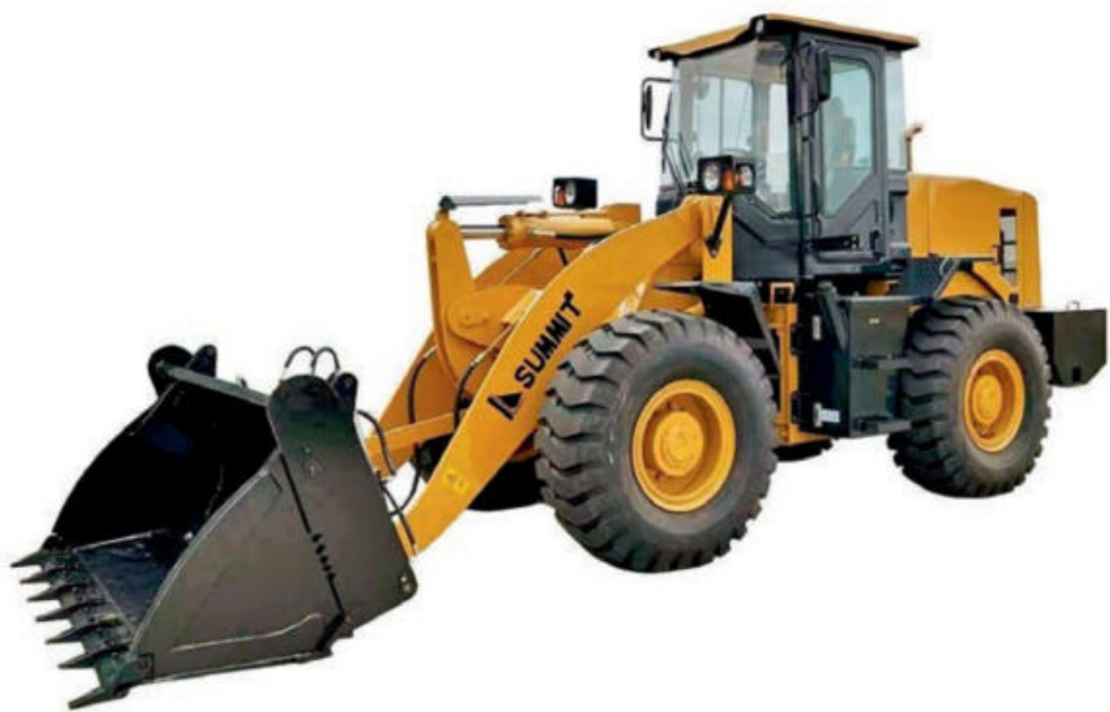
SUMMIT 946 11T WHEEL LOADER WITH 180HP CUMMINS & 4 SPEED ZF 4000kg capacity 11000 kg operating weight 180HP genuine Cummins engine 4 speed genuine ZF gearbox Wet disc bracke axles Comes with GP bucket, pallet forks. S17. TA1120591. $91,190 Inc GST
