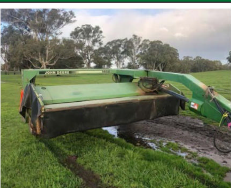
John Deere 1460 Mower conditioner - 3m, rubber on rubber condition rollers, hydraulic swing, side pull.
