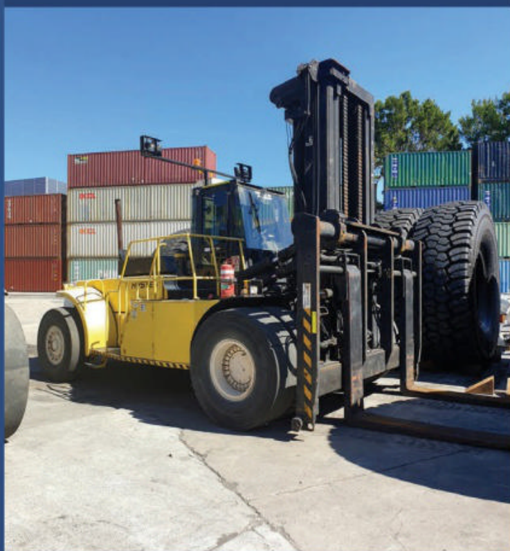
HYSTER H32.00F WEIGHT KG: 43KG, LIFT 32,000KG @ 1,200MM, CUMMINS 6CTA TURBO DIESEL
