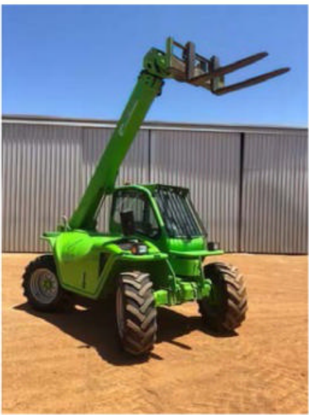
2012 Merlo P34.7 Plus 100Hp Deutz engine, pallet forks & 1.0 cubic meter general purpose bucket, 40km/h 2 speed hydrostatic transmission, 3.4t on lift capacity 7meter boom, 405/70-24 Mitas tyres 60%.
