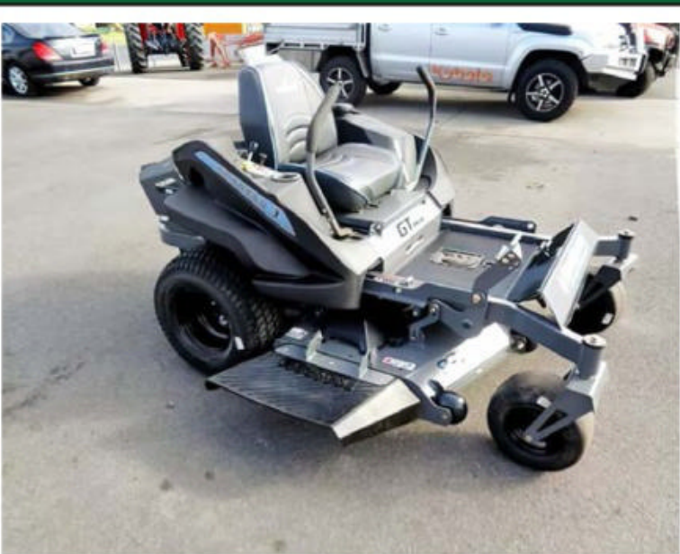
Bushranger Spartan RZ 48" Kawasaki FR691 premium and commercial grade engine. Engine guard. 13.6 kph top speed. 18.9 litres fuel capacity.
