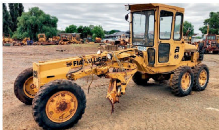
FIAT M65 Just in for dismantling, 10 Moldboard, D262 engine, rear ripper, very tidy all round, all parts available. Phone Brendan 02 6762 4466. S168. TA1123569.
