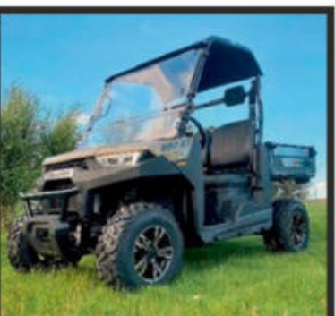
CROSSFIRE 400GT 23 HP engine with electronic fuel injection and liquid cooling capacity is 352cc, automatic CVT shaft driven transmission, on demand 4WD, .. NSW. DIY1130342. 02 8783 8411. $10,999
