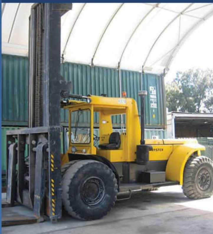
HYSTER H520B WEIGHT: 45,330KG, LIFT CAPACITY 23,500KG @ 1,220, ALLISON 3 SPEED
