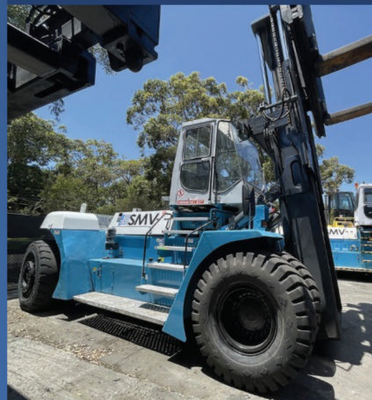
SMV 32-1200A COG: 32 T, CENTRE OF GRAVITY 1200 MM, WEIGHT: 41.3 T, ENGINE: SCANIA
