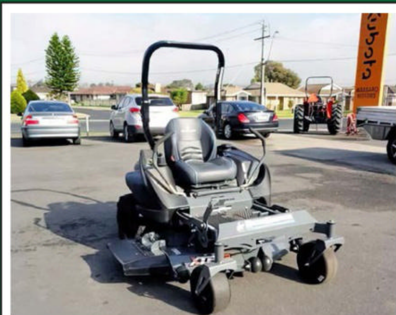
Bushranger Spartan RZHD 48" Kawasaki FR691V premium and commercial grade V-Twin engine. Engine guard. 14.48 kph Top speed. 18.9 litres fuel capacity.
