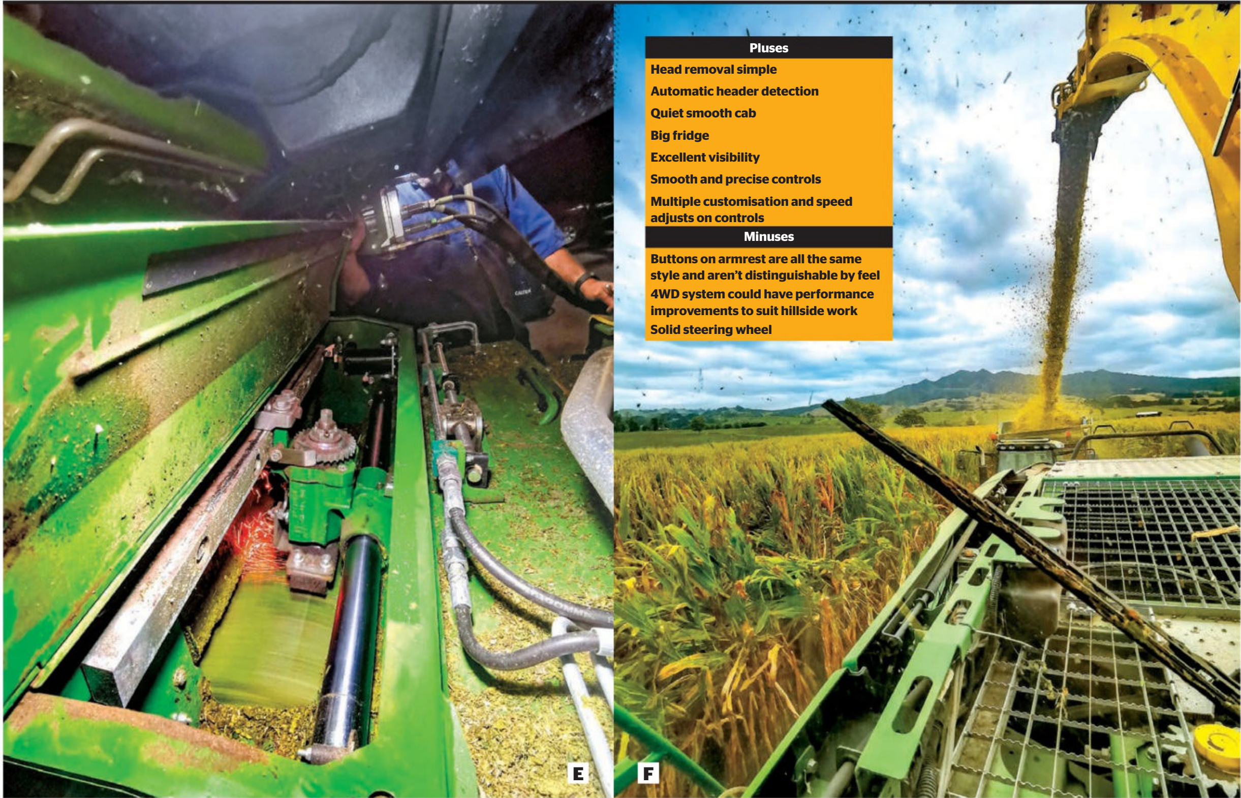
E Automatic knife sharpener in action. A light (under the cab) provides illumination for after-dark inspections
