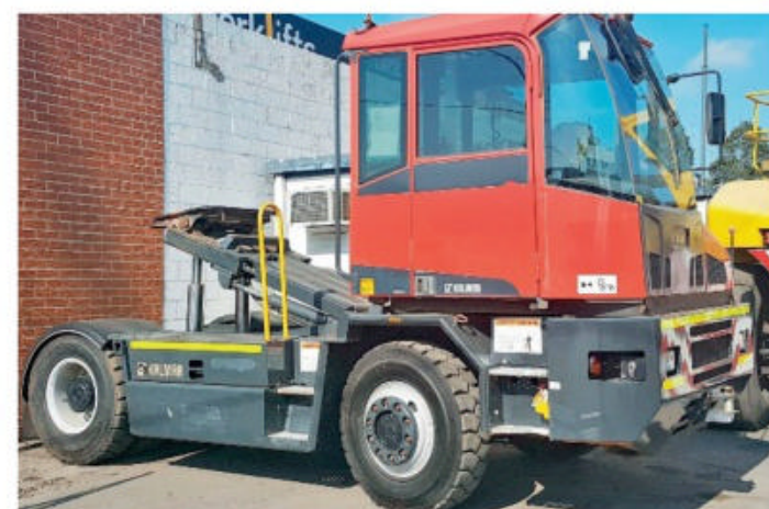
KALMAR TR618I 2014, ideal for trailers to from RoRo or Barge. 32,000kg at 5th wheel, boom has 1000mm lift height. Fwd and Rev Driver controls. Volvo diesel and Dana Trans with SISU drive and steer axles. R3552. TA899444. POA
