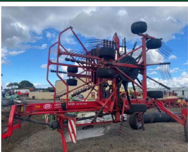
Lely Hibiscus 915 CD Vario Pull type twin rotor rake. Twin rotors, cam track, tandem-axle wheel, steering device, hydraulic systems.
