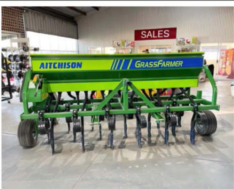
Aitchison 3018C Overall width - 3320mm (10'11"). Overall height - 1550mm (5'0"). Overall length - 2250mm (7'5"). Weight empty - 920kg.
