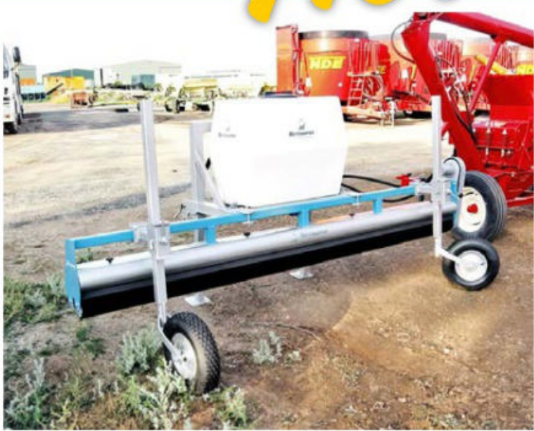
Rotowiper FU600 New trailing or tractor mount Rotowiper Weedwipers. 1.8 - 4.5 metre trailing, 2.9 - 9 metre tractor mount units. Use less chemical. Suitable for windy conditions.
