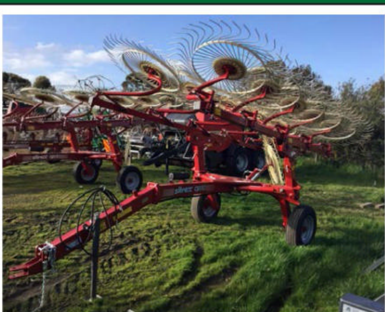
Sitrex QR10 Carted V style wheel rake. Compact, manoeuvrable and stable both in working position and transport.
