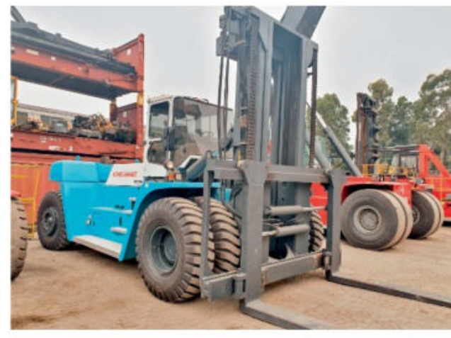
KONECRANES SMV SL32-1200B 2011, rated 32,000kg at 1200mm load centre 1 can stack highcube 20' containers 2 high and can transport without need to dismantle. R3376. TA1038152. POA For Sale or Hire Ph: 1800688788
