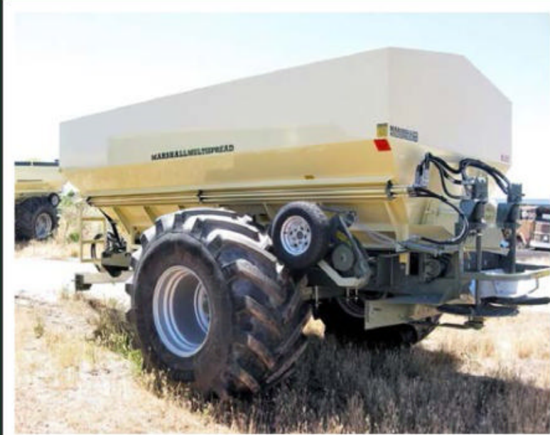
Marshall 814T New 14 tonne trailing spreader with hydraulic twin spinners, 825mm wide chain & belt 4-speed conveyor, 750/65R26 tyres.
