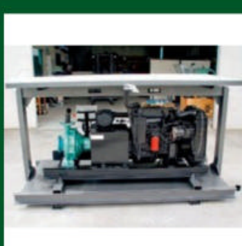
SOUTHERN CROSS 100X65-315 PUMP SET with Nissan QD32 (65hp), skid fuel tank, oil-temp, hi/lo timer watchdog and fork lift roof. Vel67912. TA11060. $13,750
