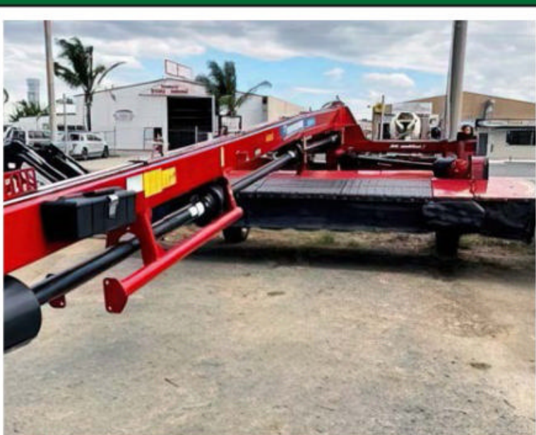
New Holland 316 Steel Roller Mower Conditioner, 5 meter cut, Ex demo machine, done little work, steel rollers, ready to go. At our Echuca Dealership.
