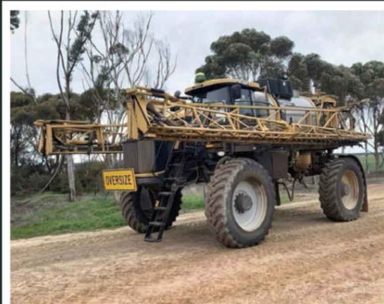
2015 Rogator R 1300B SP sprayer. 120' boom @ 20" spacings. Raven Viper Pro 4 triple X nozzle bodies. 60L scud tank, 800L fresh water tank, 6000L solution tank.
