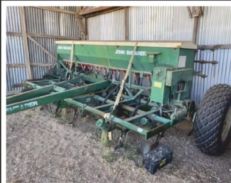
John Shearer John Shearer 24 run seed drill raised seed box, direct drill points 4 rank finger tyne harrow.
