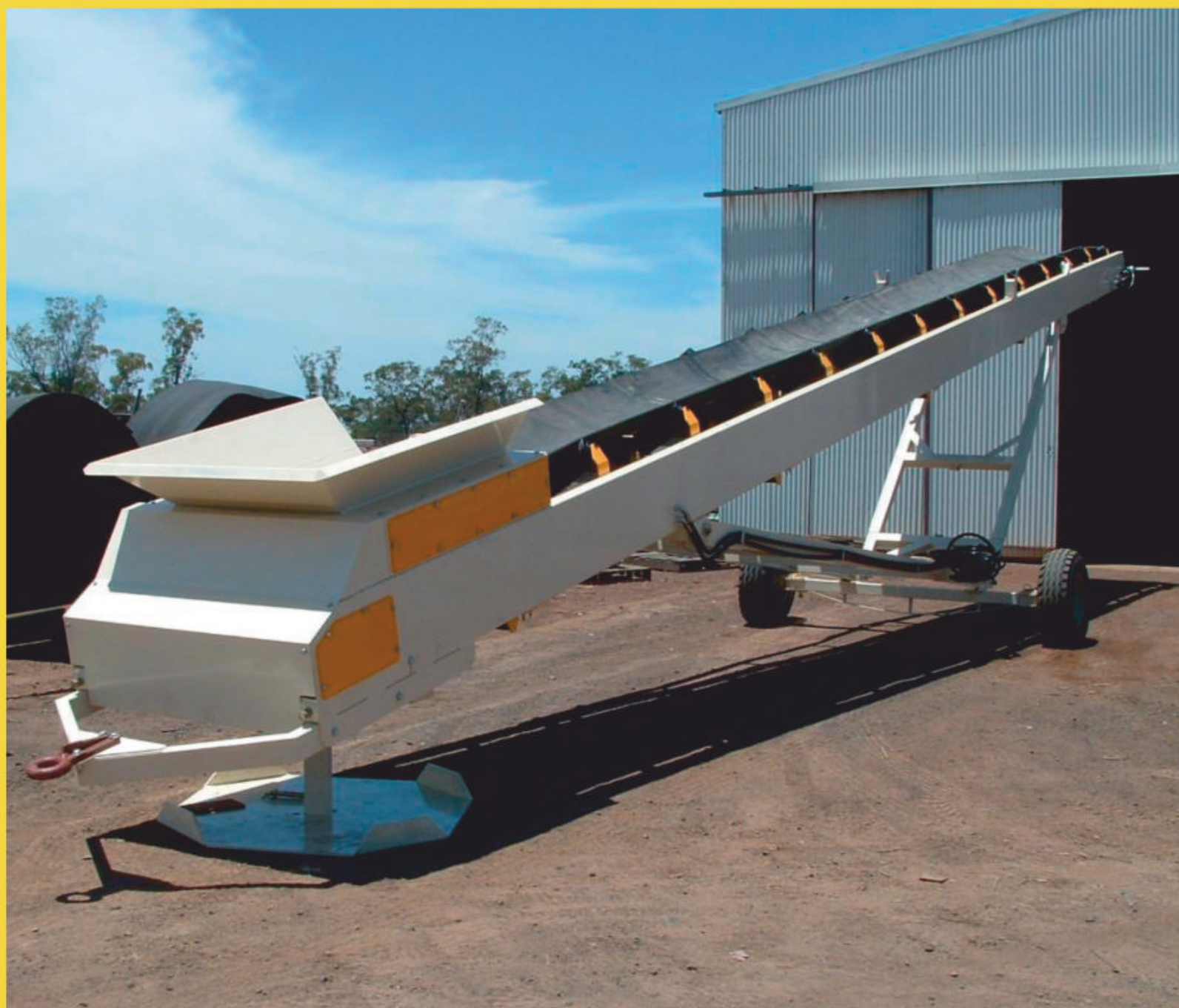
THOMAS RADIAL STACKER 15m x 900mm wide hydraulic drive hydraulic raise & lower. TRS15MX900. TA114185. Quoted to Customer Spec POA
