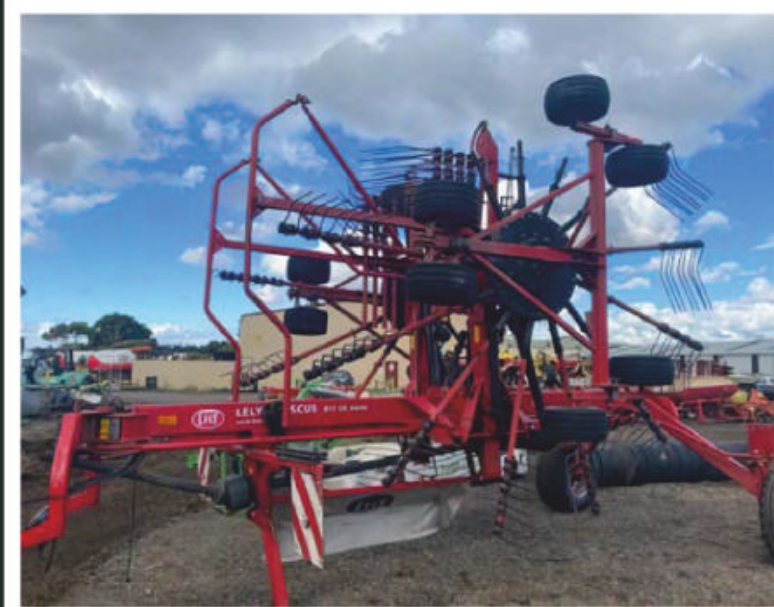
Lely Hibiscus 915 CD Vario Pull type twin rotor rake. Twin rotors, cam track, tandem-axle wheel, steering device, hydraulic systems.
