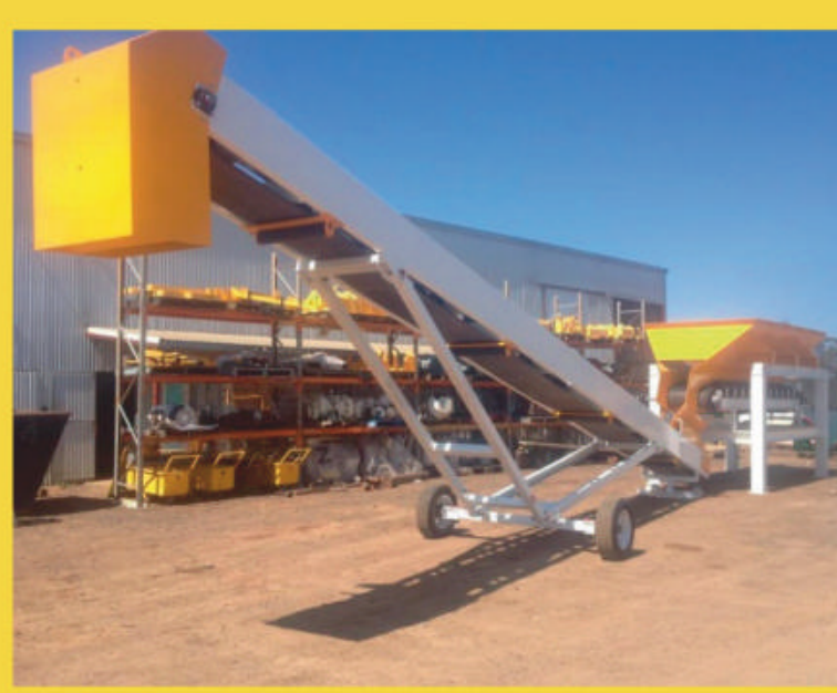
THOMAS PRE COATING PLANT 1 x 6 cubic metre Hopper with 750 wide Feed Conveyor. 12 metre x 600 wide Radial Stacker. Electrical Cabinet on stand, fitted with all necessary starting equipment. THPCP2014. TADPLin77608. Quoted to Customer Spec POA
