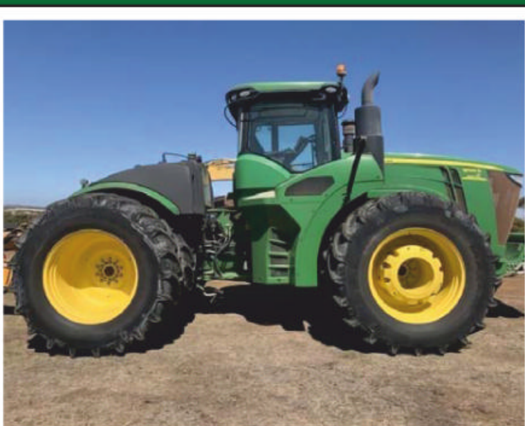
2020 John Deere 9520R e18 transmission, 18 F/6 R speeds with efficiency manager, 4600 CommandCenter with extended monitor, CommandCenter premium activation 3.0, 4600 processor.
