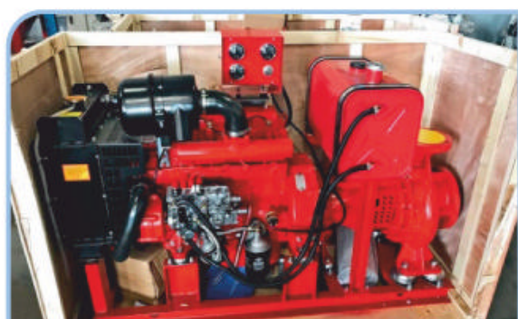
BRAND NEW 4" DIESEL, POWERED WATER PUMP MODEL WP100Y, 4 CYLINDER DIESEL, 80M3 /HR 20M HEAD
