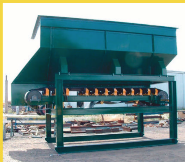
THOMAS FEED HOPPER 20 CUBIC METER with 900mm wide, feed conveyor TH20900. TA122049. Quoted to Customer Spec POA
