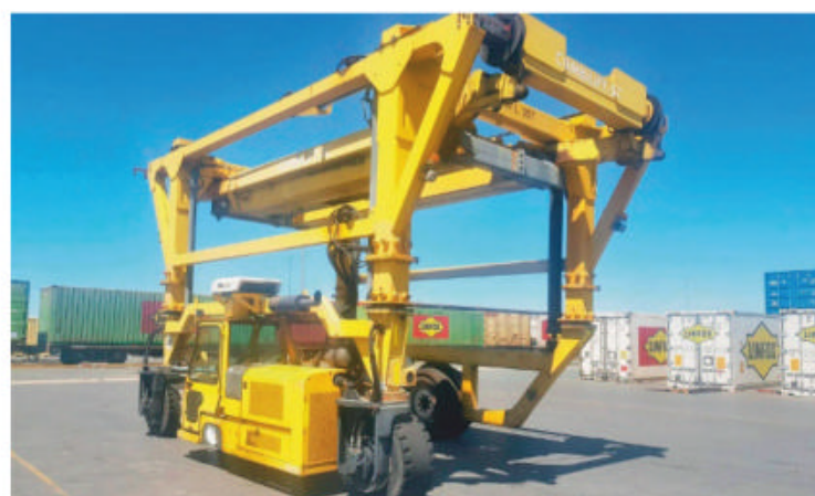
COMBILIFT SC3T 2013, 35,000kg capacity 2 high highcube container. 20-40 spreader controlled from within the cab. Low ground pressure when fully loaded. R3665. TA1113072.
