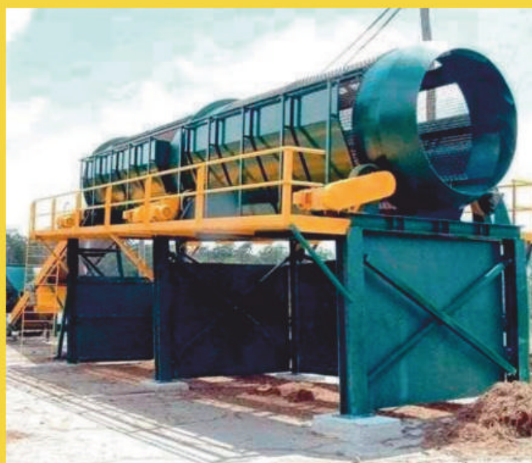
THOMAS DOUBLE TROMMEL 2 barrel screening trommel with 8m 3 feed hopper complete with 1,500mm feed belt - trommel feed conveyor 12m x 1,200mm. 77635. TADPLin77635. Quoted to Customer Spec POA
