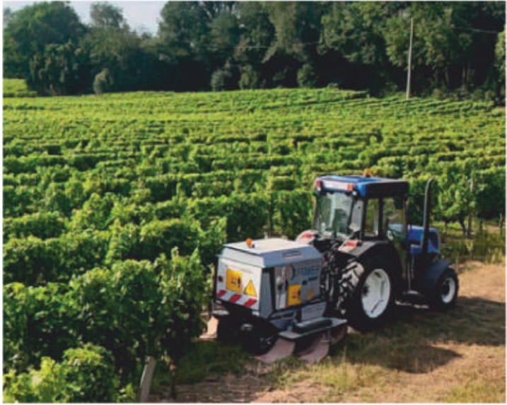
⬆ The Zasso Electroherb weed electrocution machine
