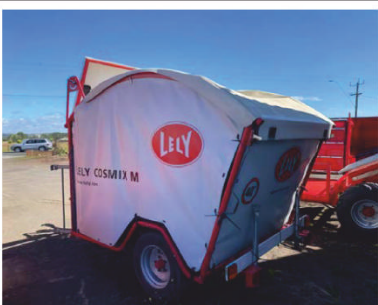
Lely Cosmix M A one-tonne hopper on a trailer that can be towed to wherever the calves are and left in the paddock.
