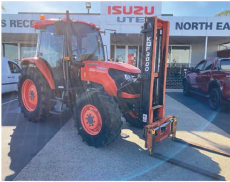
2010 Kubota M8540 4424 hrs. KBF3000 forklift attachment. Engine 85.5 HP 4x4 MFWD 4WD. Transmission: Hydraulic-Shuttle 18 x 18. Creeper - low - high gearing.
