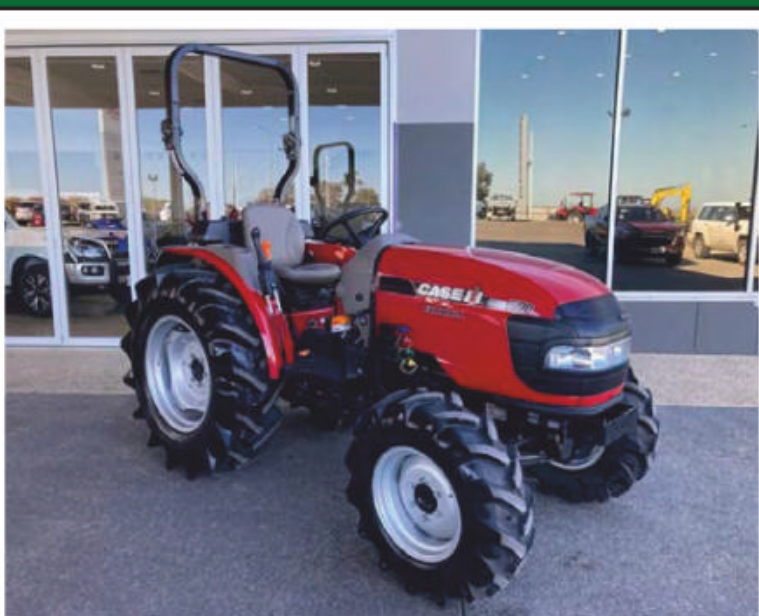
2021 Case IH Farmall 50 B 2.5 litre 4 cylinder diesel engine 50hp. 3 point linkage 1252kg capacity. Mechanical transmission.
