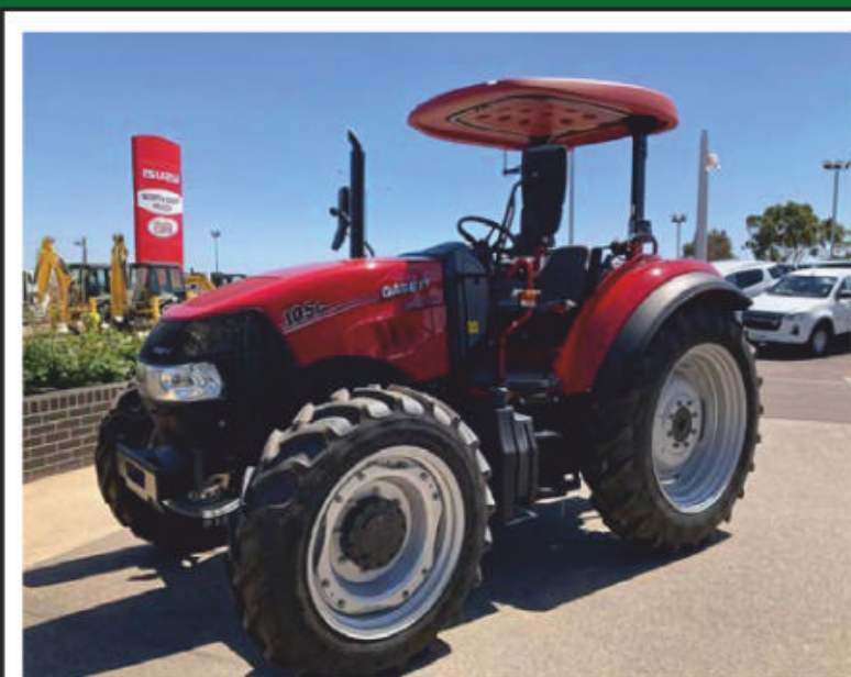
2020 Case IH Farmall 105C 3.4L FPT engine 107 HP. PTO 91 HP. 24 x 24 power shuttle Hi Lo transmission. hydraulic main pump flow 64LPM. Rear remotes x 2.
