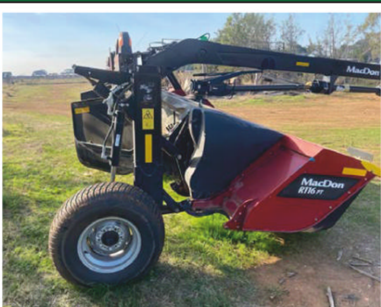
2017 Macdon R116 2017 Macdon R116 mower conditioner PTO pull type rubber rollers, tidy new blades.
