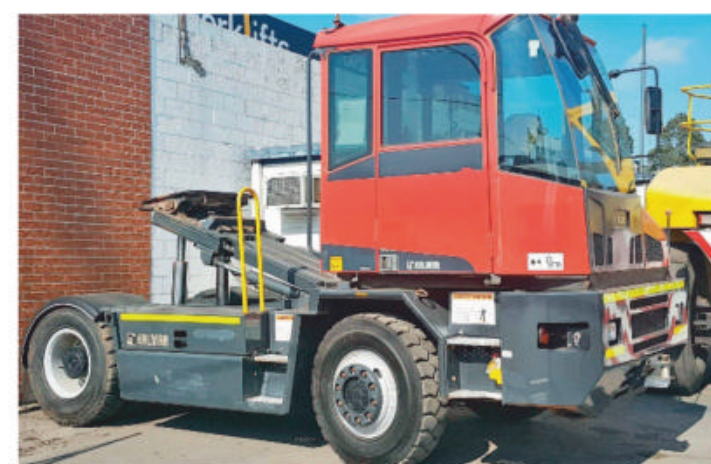
KALMAR TR618I 2014, ideal for trailers to from RoRo or Barge. 32,000kg at 5th wheel, boom has 1000mm lift height. Fwd and Rev Driver controls. Volvo diesel and Dana Trans with SISU drive and steer axles. R3552. TA899444.
