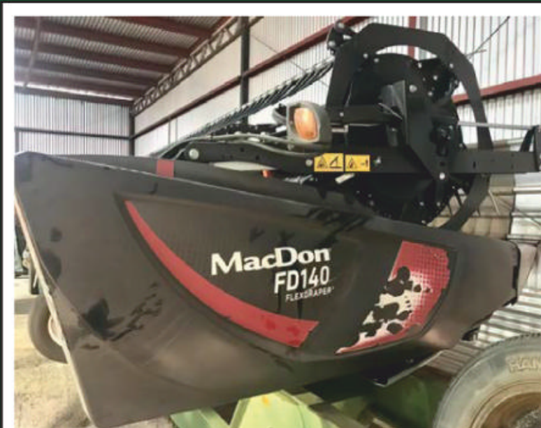
2018 Macdon FD140 Flex Draper 40 foot front, top x auger, it has new plastic pan. new SS feeder floor. New RTD chain. New knife for 21. New knife guards for 21.
