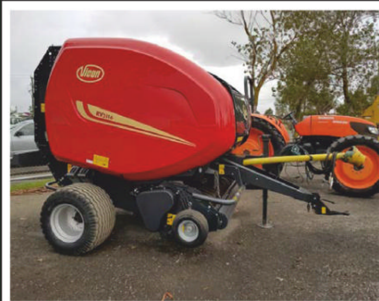
Vicon RV5116 Round Baler. Done 11,196 bales. New chain and drive sprockets. Full workshop service.
