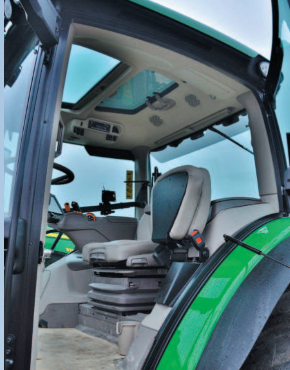
Above: Latest 6R range introduces a new low-profile cab roof and the option of either wide-opening full-frame doors (pictured) or the standard five-post cab frame with a B-pillar hinged nearside door
