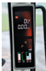
Above: Conventional steering console with integrated dials/gauges has been replaced by a corner post primary display unit mounted on the A-pillar (inset)
