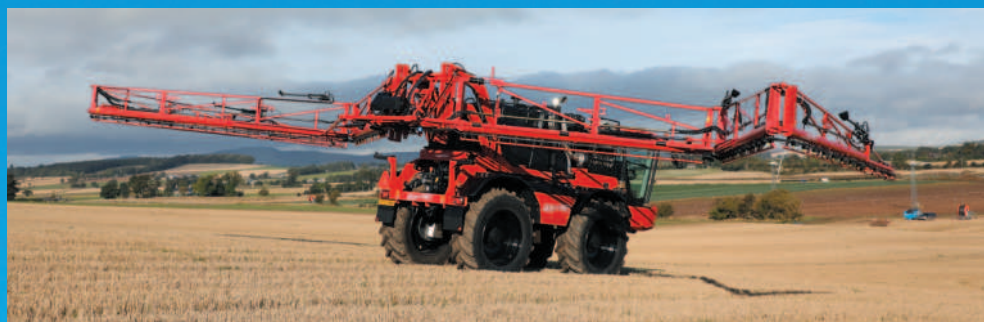
Above and below: With FastFoldPlus, the spray boom is folded and unfolded easier and faster. This 36m boom can be unfolded in 20 seconds
