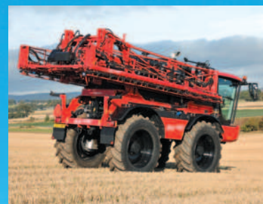
Above and below: With FastFoldPlus, the spray boom is folded and unfolded easier and faster. This 36m boom can be unfolded in 20 seconds
