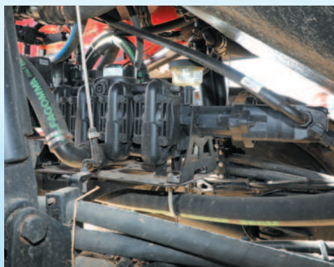
Above: GreenFlowPlus is a very compact pump system with short pipes and electrically operated valves
