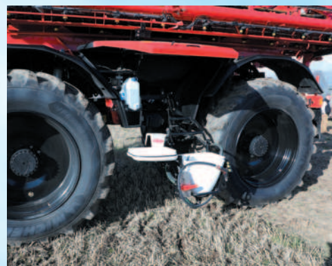
Above: GreenFlowPlus is a very compact pump system with short pipes and electrically operated valves
