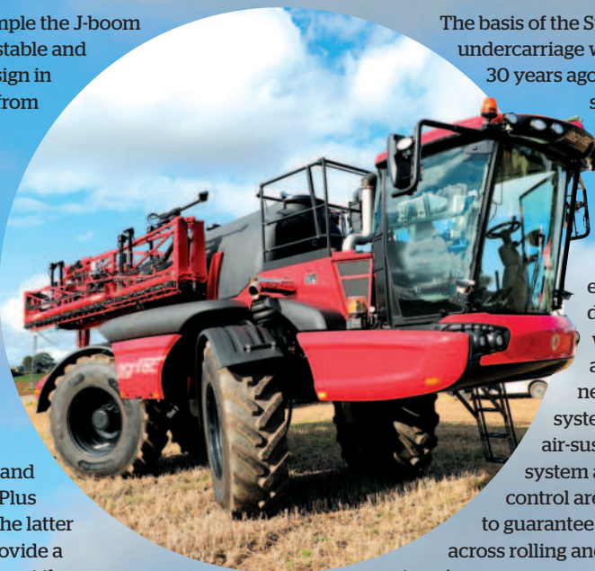
Above: Steering can be selected as four-wheel, two-wheel or crab
