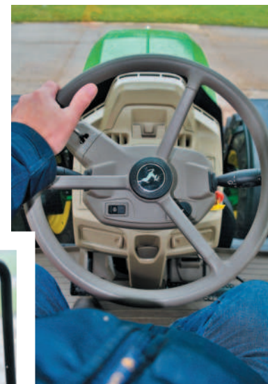
Above: Conventional steering console with integrated dials/gauges has been replaced by a corner post primary display unit mounted on the A-pillar (inset)
