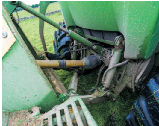
Above: The 'front linkage' features tilt and side-to-side movement
