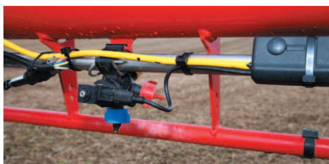
Top: Solenoid valves in pulse width modulation systems (above) turn the flow on/off up to 100 times a second, which alters flow to match variations in speed while pressure remains constant
