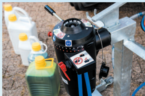
Above: Products can be added with this closed transfer system (CTS) without having to open containers
