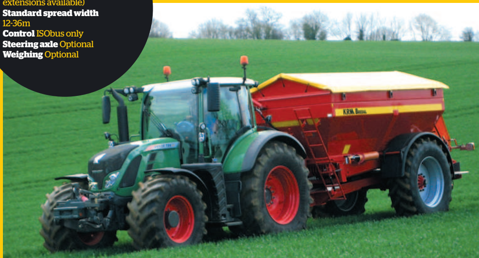
Left: Bredal spreaders use ISOBus for control but Muller screens can be fitted in tractors that aren't compatible
