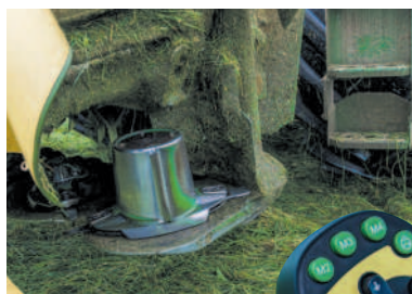
Right: The BiG M features the same SafeCut disc protection as the tractor-mounted machines
