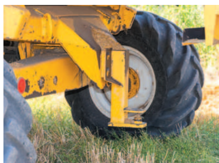
Above: A simple hydraulic quick coupler is used to connect and disconnect the 20ft (6.1m) header on the TX66
