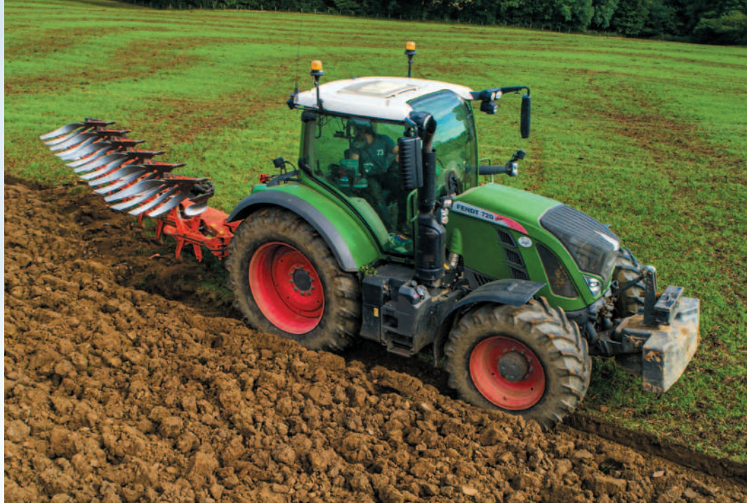
Above: After demonstrating with Rabe, Colin was sold on the idea of slatted mouldboards and has been running them since the early 1990s
