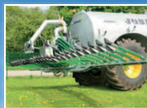
Integrated "anti-drip" lifting device (Twist system)
