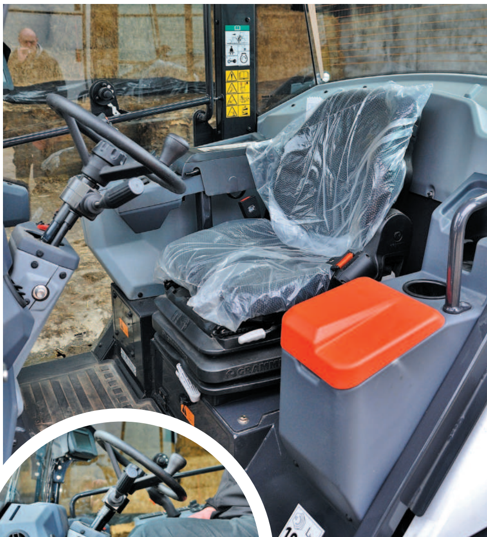
Above: Cab interior is thoughtfully laid out and features an air seat. Adjustable steering allows the driving position to be set for tall drivers (inset left) without compromising leg space
