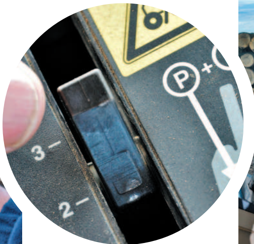
Left: The 7700 F-R shuttle lever integrates the powershift ratios in both directions. To prevent inadvertently engaging too high a gear when shuttling, adjustable stops were fitted (inset above)
