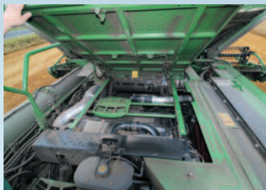
Right: John Deere X9 1100 is powered by a 700hp PowerTech PSS 13.6-litre engine
