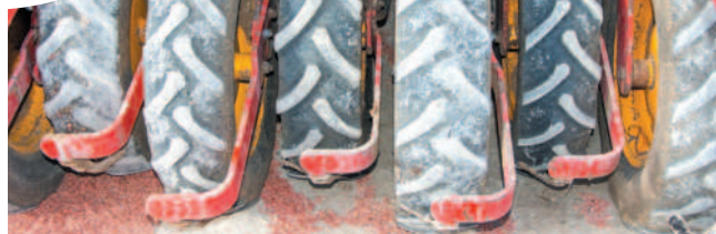
Above: Tim prefers the staggered press wheels on his 6m Rapid compared to the straight-line packer roll on the previous Rapid 400F
