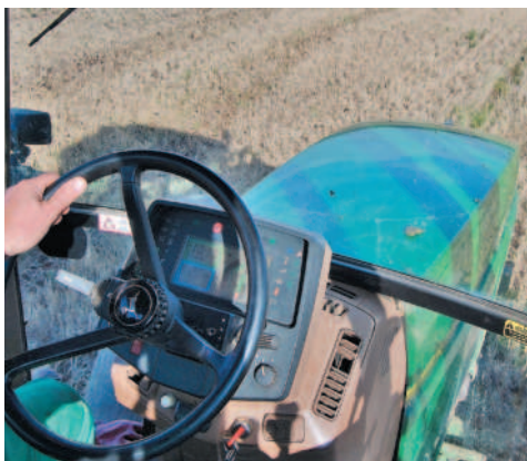
Right: At the time of its launch, the 7700's new two-door TechCenter cab was quieter and offered 40 per cent more interior room than the SoundGard 2 on previous ranges
