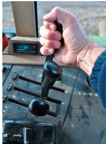
Above: Hydraulic levers are well placed and offer simple pull-a-lever operation. Electronic rear linkage control features dials to adjust lift height and response (inset left)
