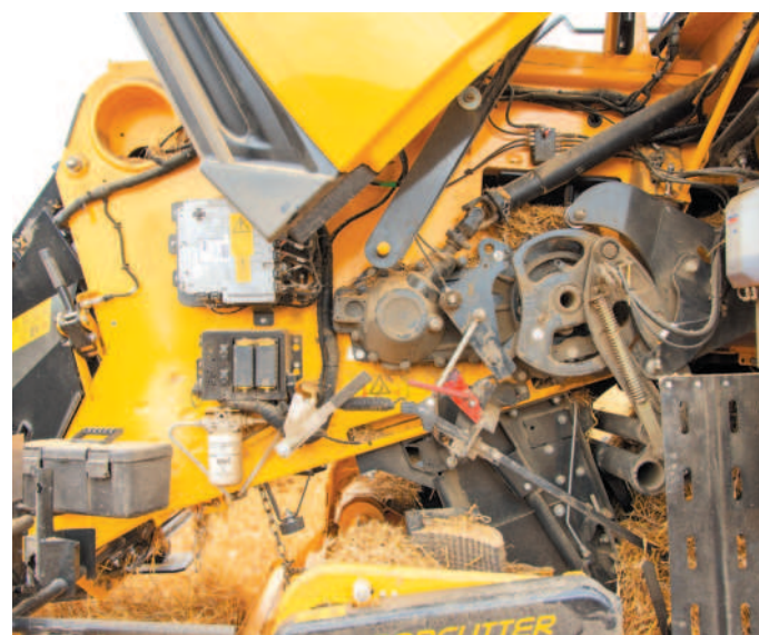
Above: The 1290HD comes with an improved pre-compression chamber with an updated six-tine stuffer fork
