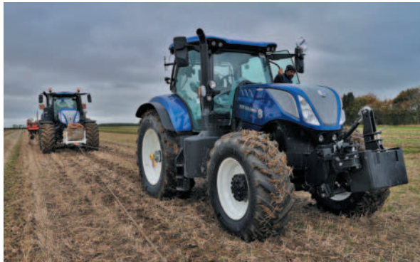
Above and top: Connected using a cable pulley system, which enabled the tractor with the most traction to pull ahead, the Axiobib 2 tractor surged ahead of the second tractor with Multibib tyres
