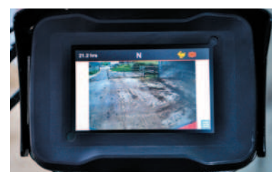
Above: LED screen settings are controlled using this pad with a scroll and selection buttons. Screen settings can identify vital operating statistics, machine performance or the integrated reversing camera
