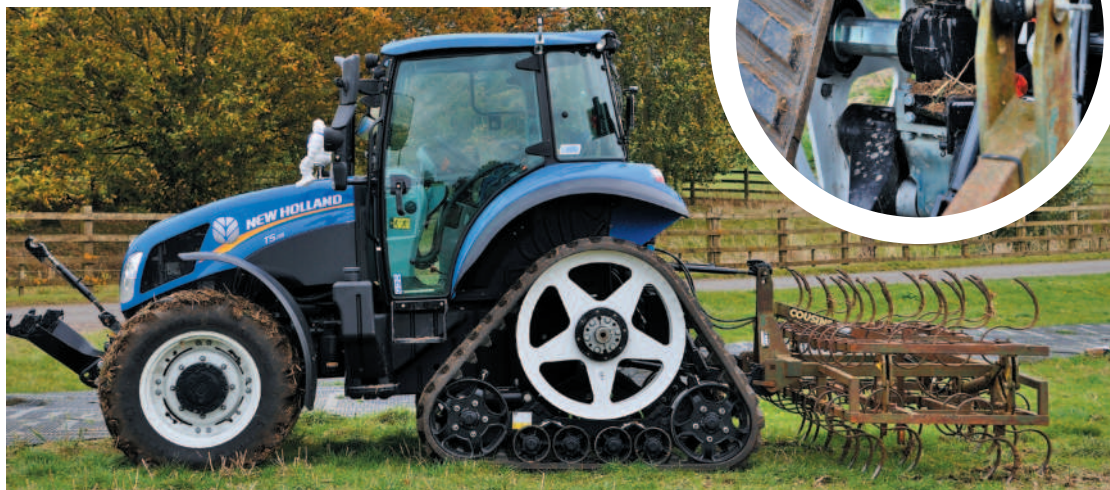
Left: Mounted on a conventional bar axle with the wheels removed (above left inset), the track unit on this T5.115 comes with an anti-rotation device that limits oscillation
