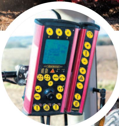
Right inset: Control station is used to monitor performance and alter seed rates on the move
