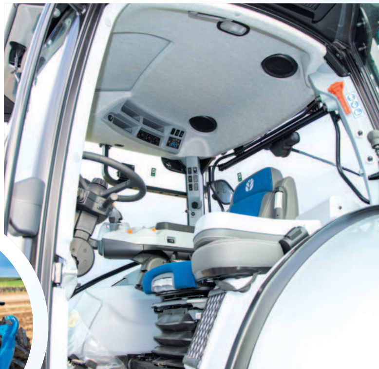
Left: The Dynamic Comfort fully suspended operator's seat features pneumatic lumbar support and two-stage heating
