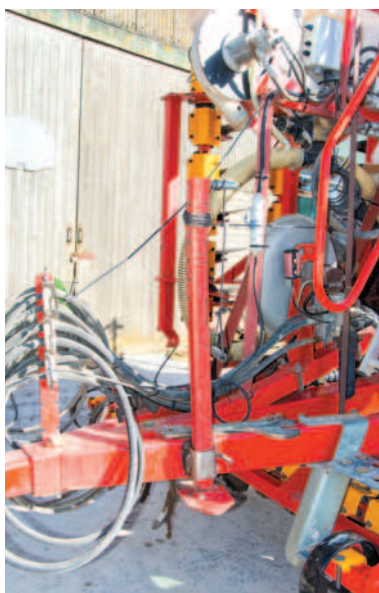
Left: Hydraulic connections are fed through a series of hooks mounted on a stanchion to keep things tidy
