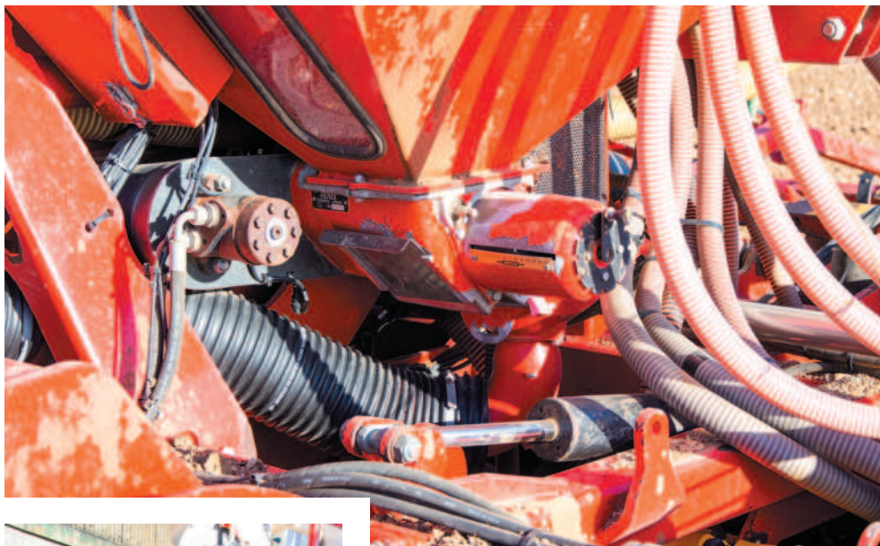
Left: Hydraulic connections are fed through a series of hooks mounted on a stanchion to keep things tidy
