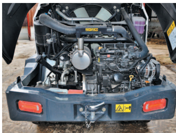
Below: Wide-opening engine cover reveals an engine bay designed for service access. All filters and check points are easily reached. Service intervals are 500 hours
