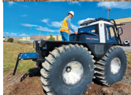
Top: A new pick-up version has a redesigned cab with a new front entry door and integrated step
