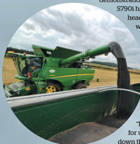
Above: It takes just over 90 seconds to unload the S790's 14,100-litre grain tank at 135 litres per second
