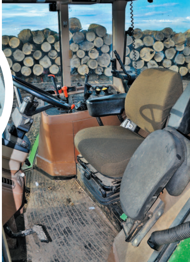
Left: The 7700 F-R shuttle lever integrates the powershift ratios in both directions. To prevent inadvertently engaging too high a gear when shuttling, adjustable stops were fitted (inset above)
