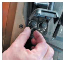
Above: Hydraulic levers are well placed and offer simple pull-a-lever operation. Electronic rear linkage control features dials to adjust lift height and response (inset left)
