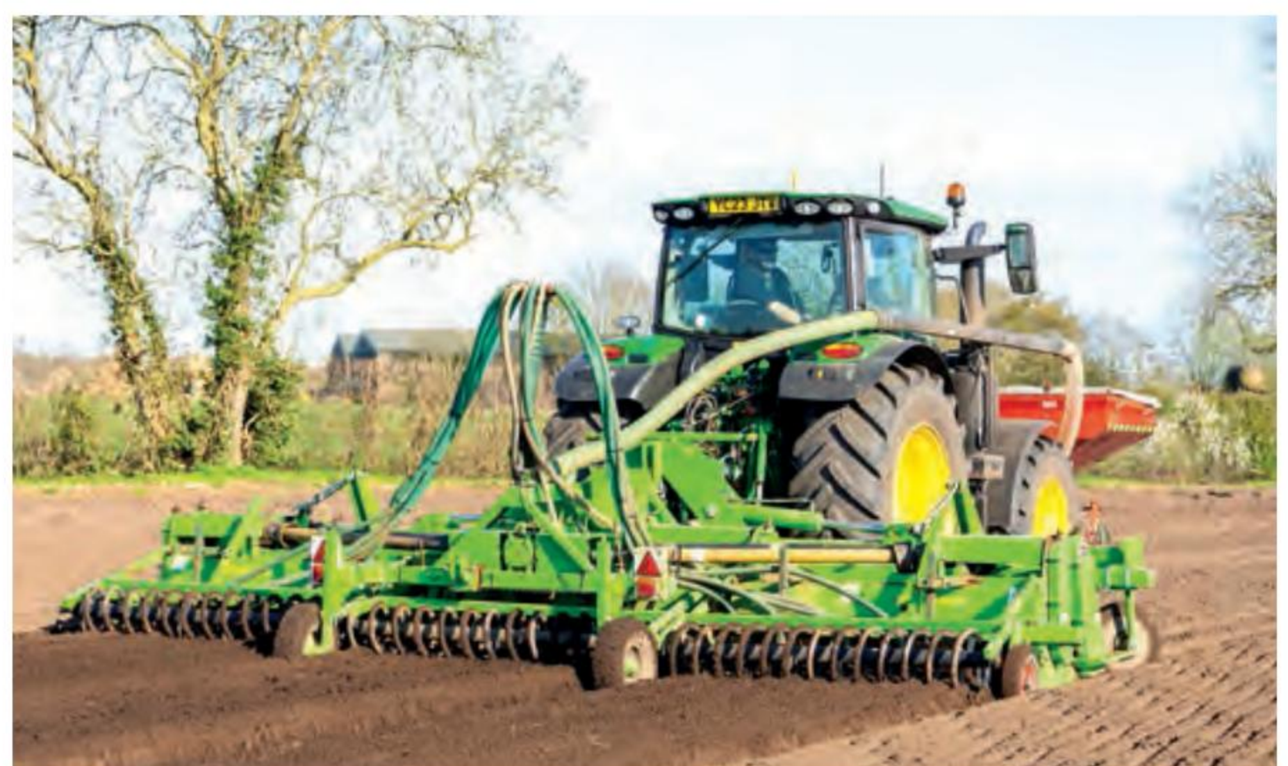
Above: The 6R 185’s category 3 rear linkage is capable of lifting up to 8100kg at the hook ends and has no issues lifting and powering this impressive Jones Engineering triple bed former
