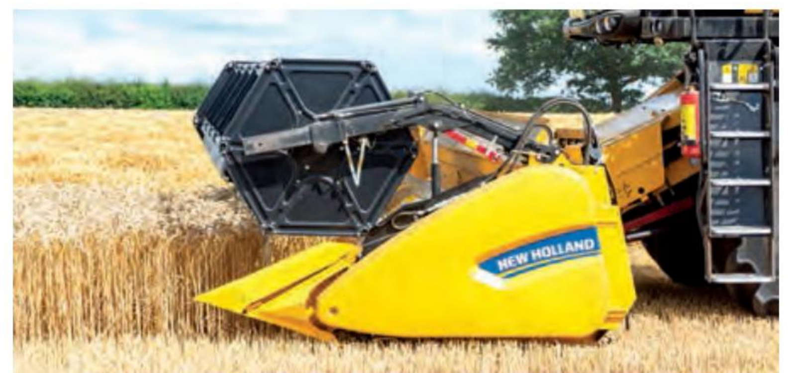
Above: The table of the VariFeed header can be extended forwards by up to 57.5cm to reduce losses in tinder-dry crops while New Holland's automated header height control system enables it to follow ground contours accurately
