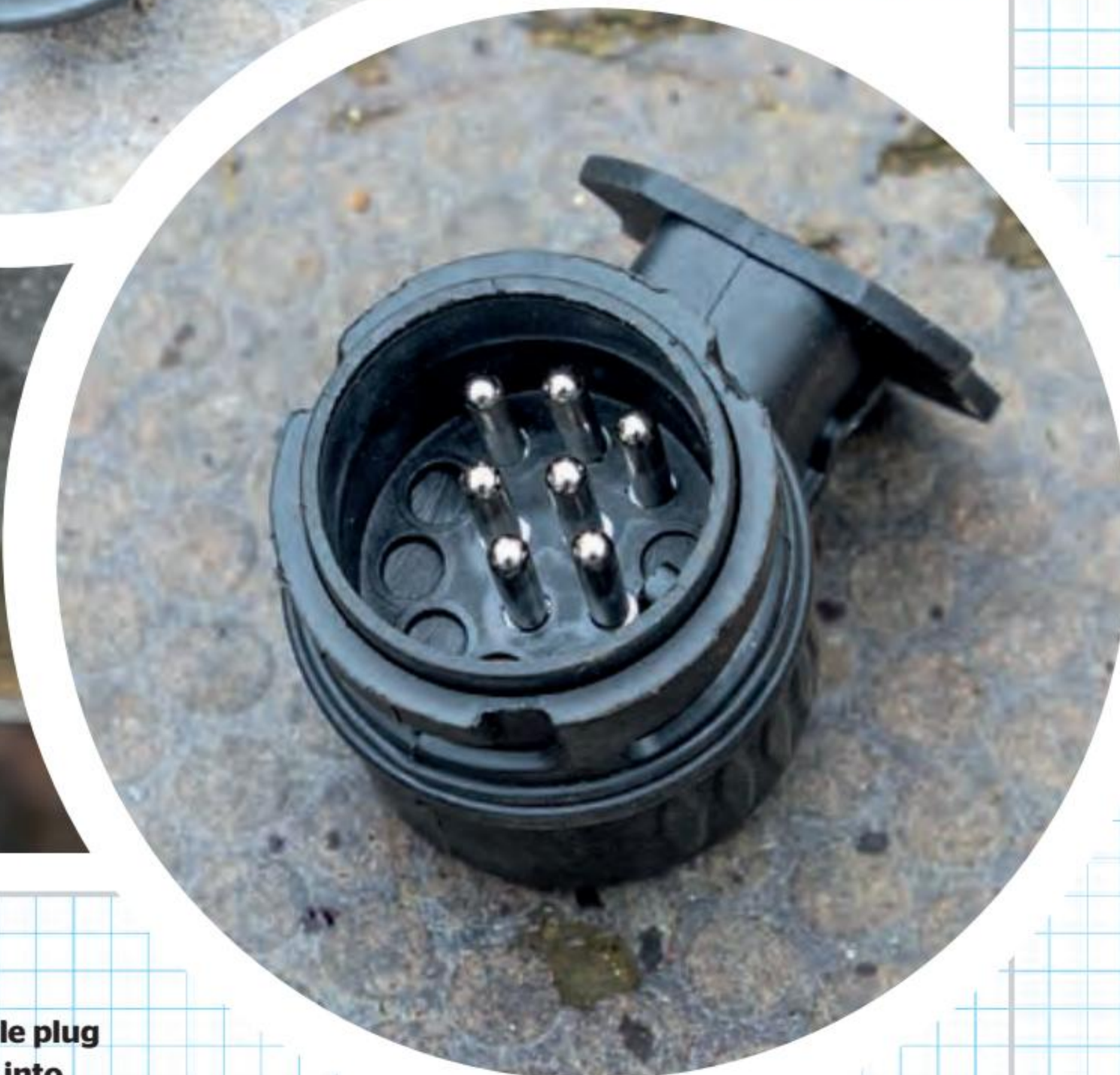
Above inset: A 13-to-7 pin adapter can be used to convert a modern towing vehicle equipped with 13-pin electrics into one that can create a 7-pin outlet to power an older trailer. Along with an earth, 7-pin supplies power for side lights, brake lights, number plate light, indicators and fog lamp
