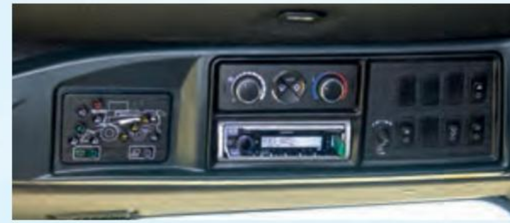
Left: The CX8.70's climate control centre situated above and to the right of the operator also includes the combine's lighting controls and a digital radio
