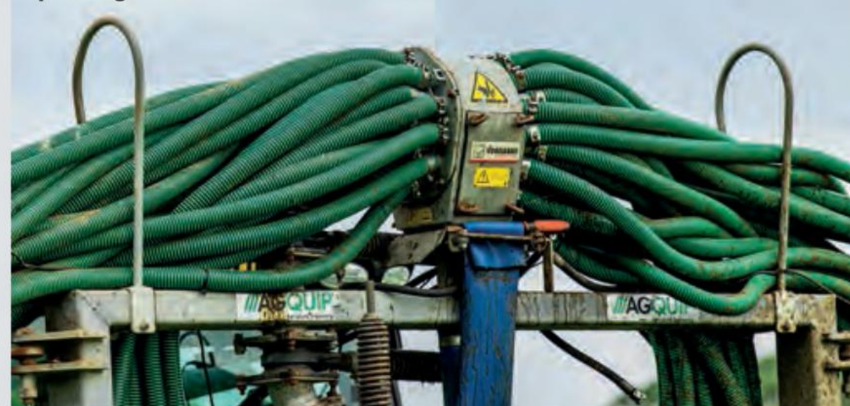
The 12m wide Agquip dribble bar is fitted with a Vogelsang macerator which is the last component before spreading
