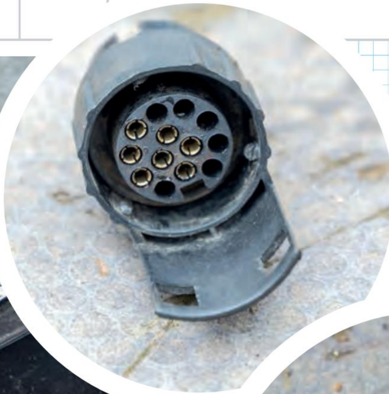
Left inset: A 13-pin to 7-pin trailer socket adapter can also be used to convert 13-pin trailer sockets to a 7-pin system, to suit older towing vehicles. Pin sockets are also numbered, making it easy to check the functionality of each connection
