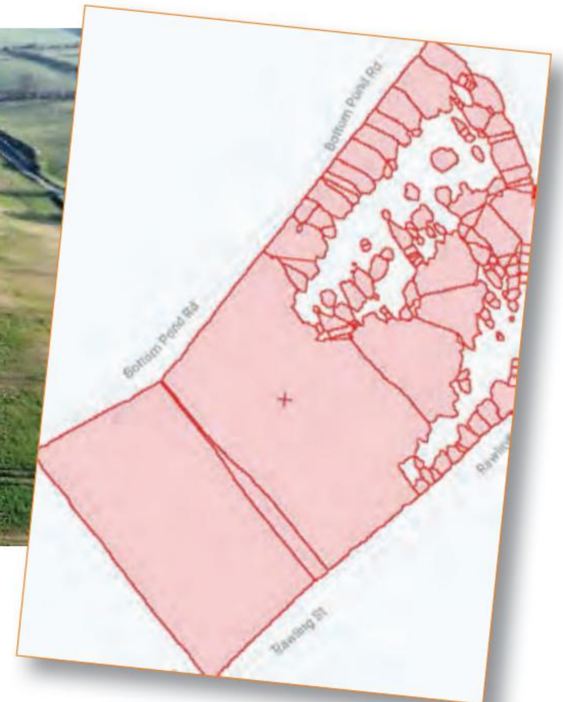
Above and right inset: As applied maps from Syngenta variable rate application trials in oilseed rape show, fungicide was applied to just 68% of the field and plant growth regulator to just 15%
