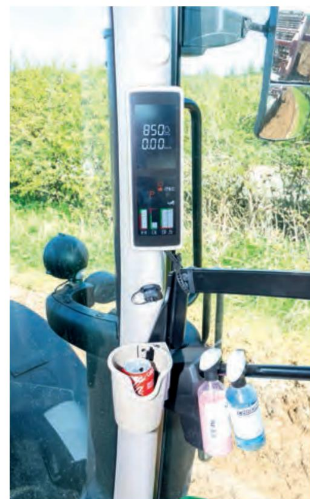
Right: John Deere's latest generation of 6R series tractors come equipped with this new A-pillar corner post display screen that clearly shows the tractor's fluid and fuel levels as well as engine rpm and ground speed
