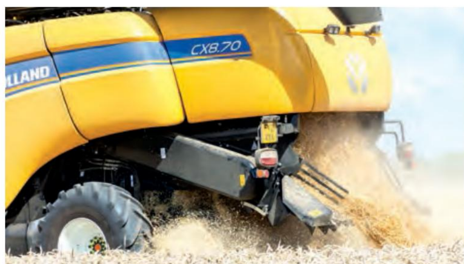
Above: Will says the CX8.70's threshing system that comprises four drums and six straw walkers produces an excellent straw swath in all of the cereal crops he grows
