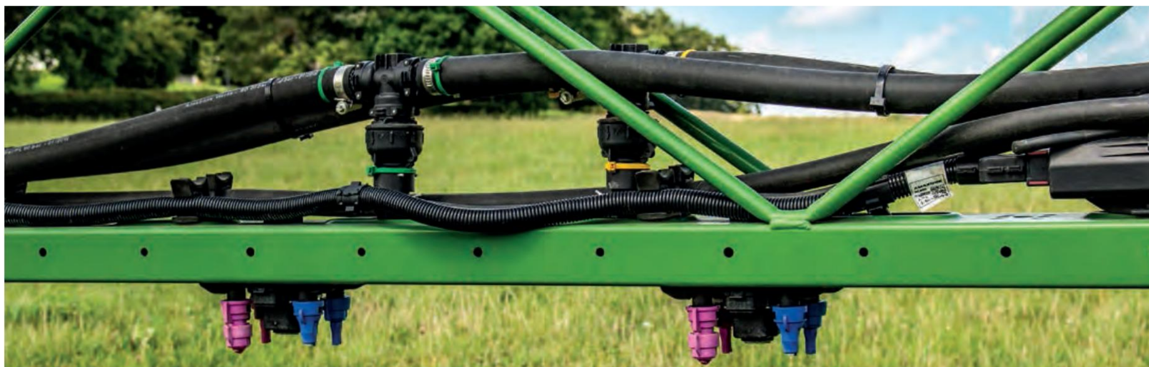
Above: Direct injection makes it possible to apply targeted treatments at the same time as applying another product, by using feeding liquid to the nozzles from another sprayline
