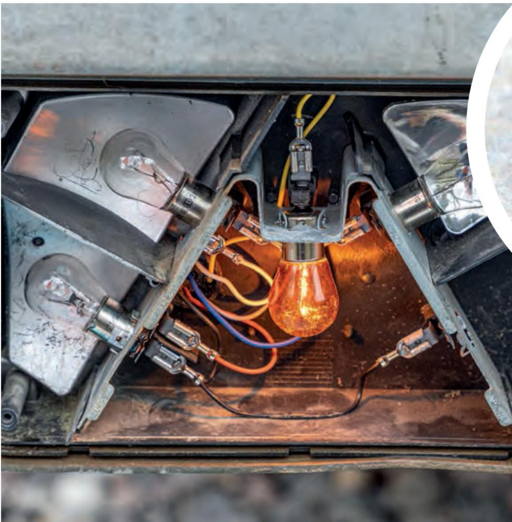
Above: With the lens removed and power turned on, check for power at the bulbs. If power is available at the bulb pins, but the light doesn't illuminate, it's likely to be a failed filament.
