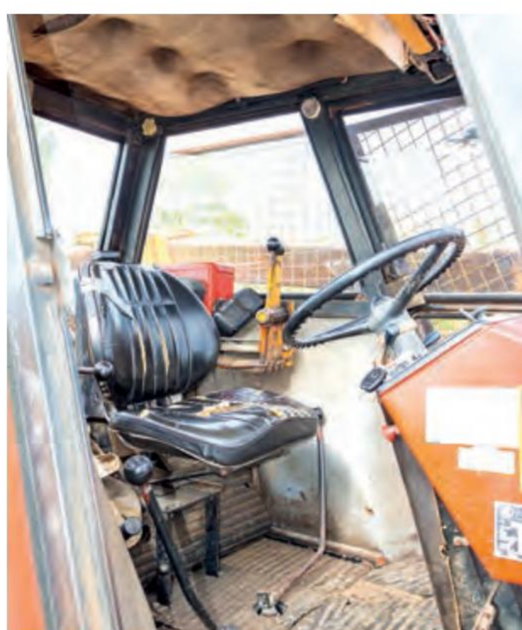
Above: The 1001's spacious flat-deck cab comes with a dash-mounted hand throttle, floor-mounted gear levers, heavy-duty interior cladding and roof insulation, and a sprung seat
