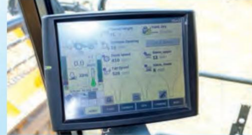
Left: The Harvest Suite Ultra cab is equipped with the 26.4cm-wide Intelliview touch-screen terminal that's capable of monitoring all major functions and is used to set up operating parameters
