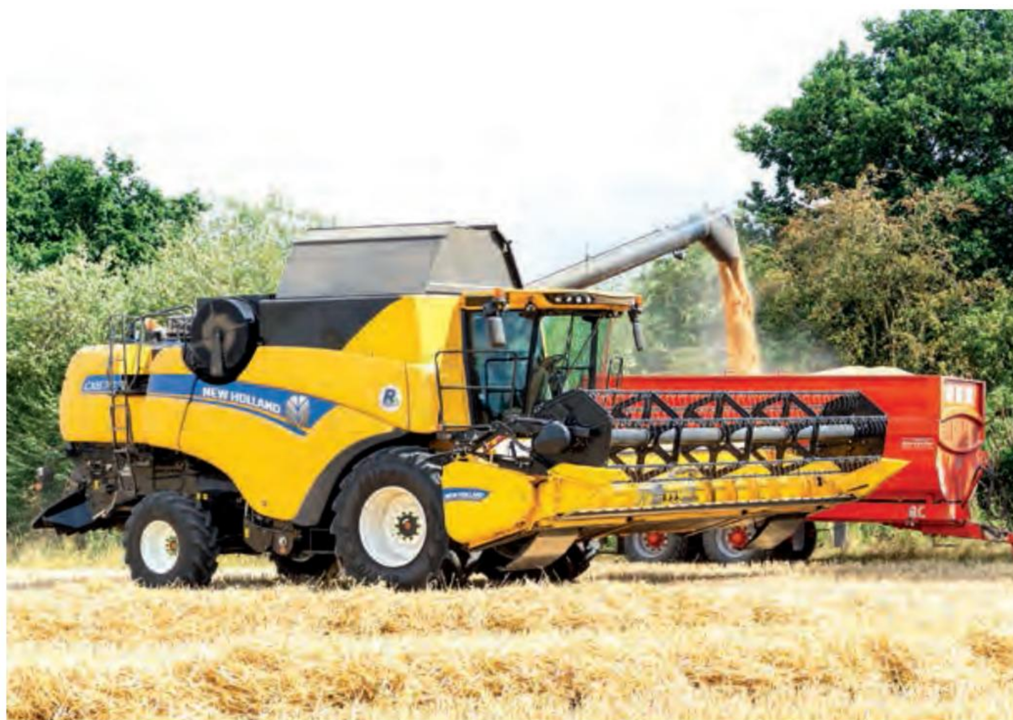
Above: The CX8.70's 11500-litre grain tank is emptied into trailers waiting on the headland at a rate of 125 litres per second
