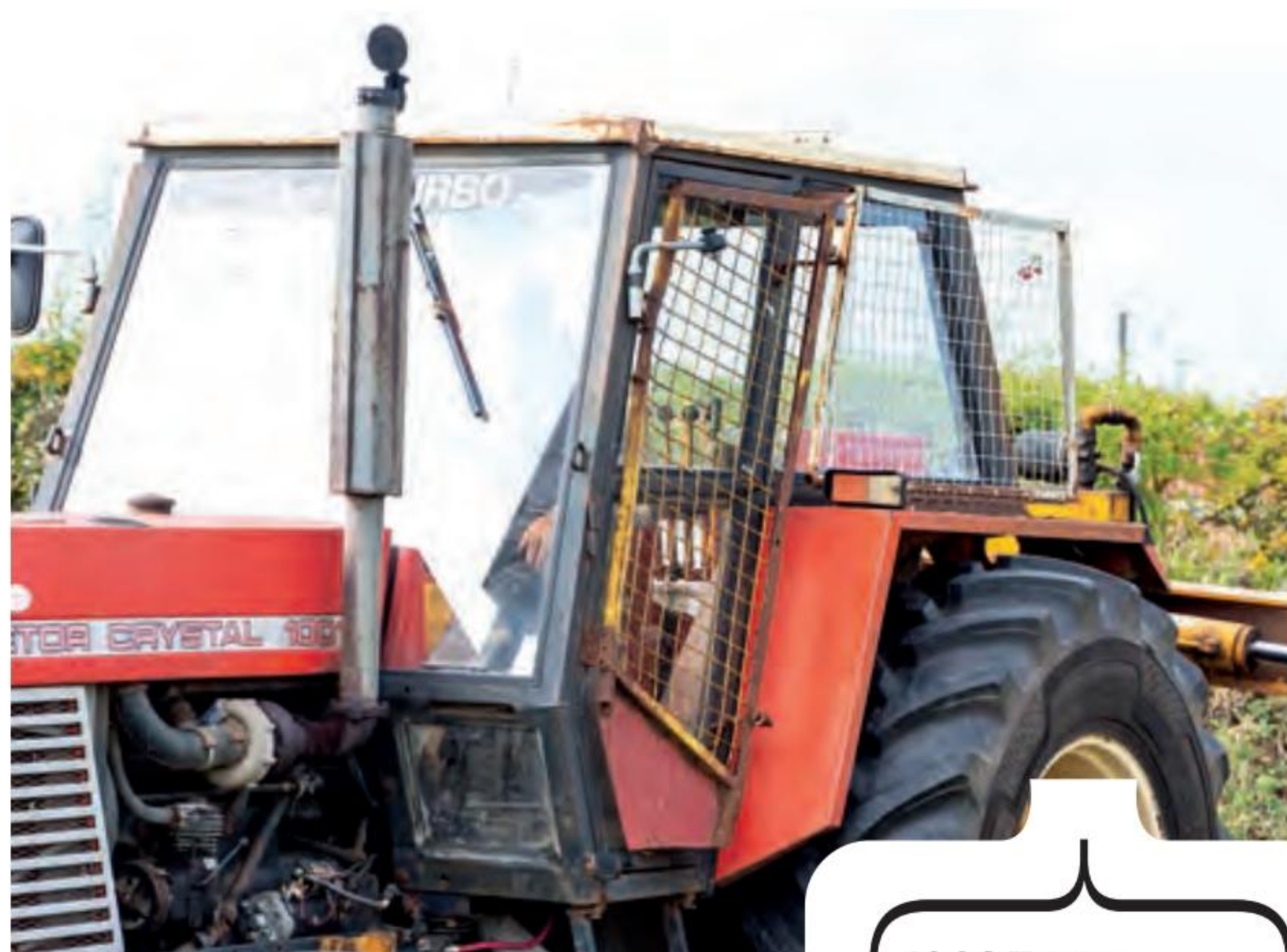
Left: A previous owner fitted the 1001's huge cab with these guards to stop branches and debris from overgrown hedges breaking the glass
