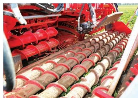
Above: The rollerbed uses seven 100mm-diameter rollers
