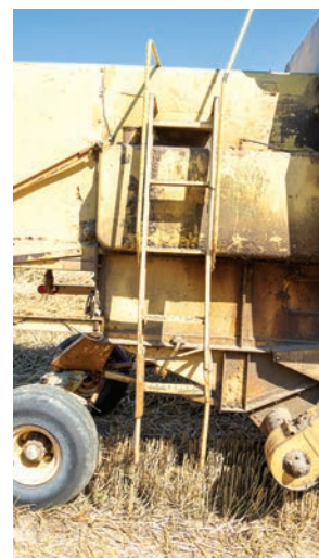
Above: Access to the engine bay and grain tank is aided by a ladder in front of the 250-litre diesel tank
