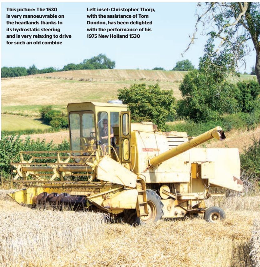
Left: This 1530 rides on Dunlop 8.50-12 tyres on its rear axle and a pair of Goodyear Torque Grip 18.4-26 tyres up front
