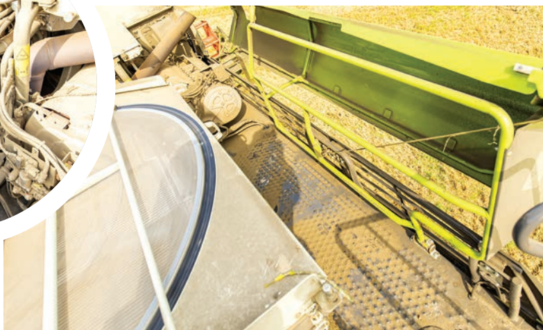
Above: Access platforms make getting to key parts of the 5300 safe and easy. The engine bay has one panel for maintenance checks (above left inset)
