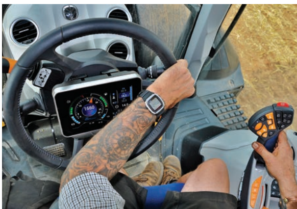
Above: CentreView display in the steering wheel (left) is bright and functional but can be hard to read and is often obscured by the driver's arm. If you don't opt for this you get a more traditional InfoView screen fixed to the steering column behind the wheel
