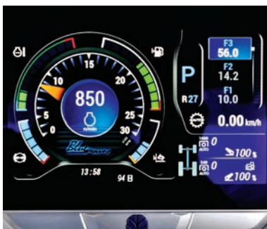
Above: CentreView display in the steering wheel (left) is bright and functional but can be hard to read and is often obscured by the driver's arm. If you don't opt for this you get a more traditional InfoView screen fixed to the steering column behind the wheel
