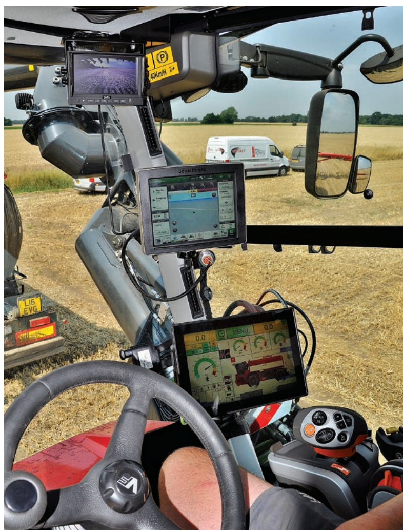
Above: The Quad 550 comes prepared for an NIR sensor. It's the only machine of its type to integrate John Deere Harvest Lab NIR technology into the terminal screen
