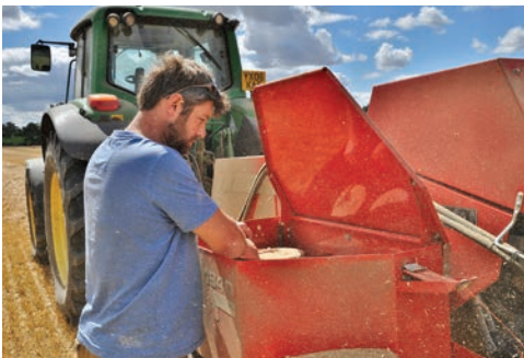
Below and below right: The 1840 features two twine boxes, which together hold five bales of twine each (inset). Baling at an average of 500-550 bales an hour, the baler has enough twine capacity to last five to six hours
