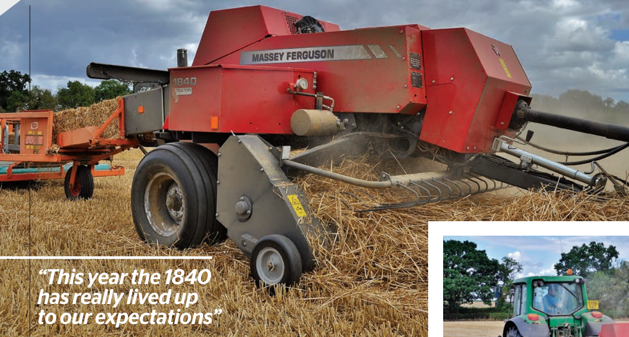
Left: The 1840 baler introduced a new pick-up/auger design, additional twine storage, an adjustable drawbar and an Optiform extended length bale chamber
