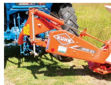
Above: A sturdy hydraulic ram is used to fold up the GMD 24, which also features an articulation point to work on slopes
