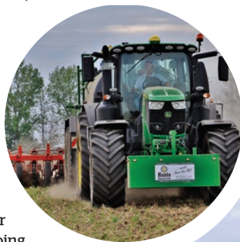
Bottom: New software for strip tillage manure application requires both the tractor (below inset) and tanker to be equipped with Starfire receivers
