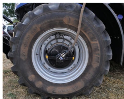
This picture and above inset: Central tyre inflation system allows pressures to be controlled via the terminal. All T7 HDs can be ordered CTIS ready. A higher capacity compressor can also be specified
