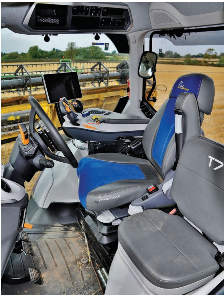
This picture and above inset: Central tyre inflation system allows pressures to be controlled via the terminal. All T7 HDs can be ordered CTIS ready. A higher capacity compressor can also be specified
