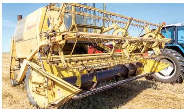
Below: The 1530 is equipped with a 3.65m (12ft) header, which worked very well this summer
