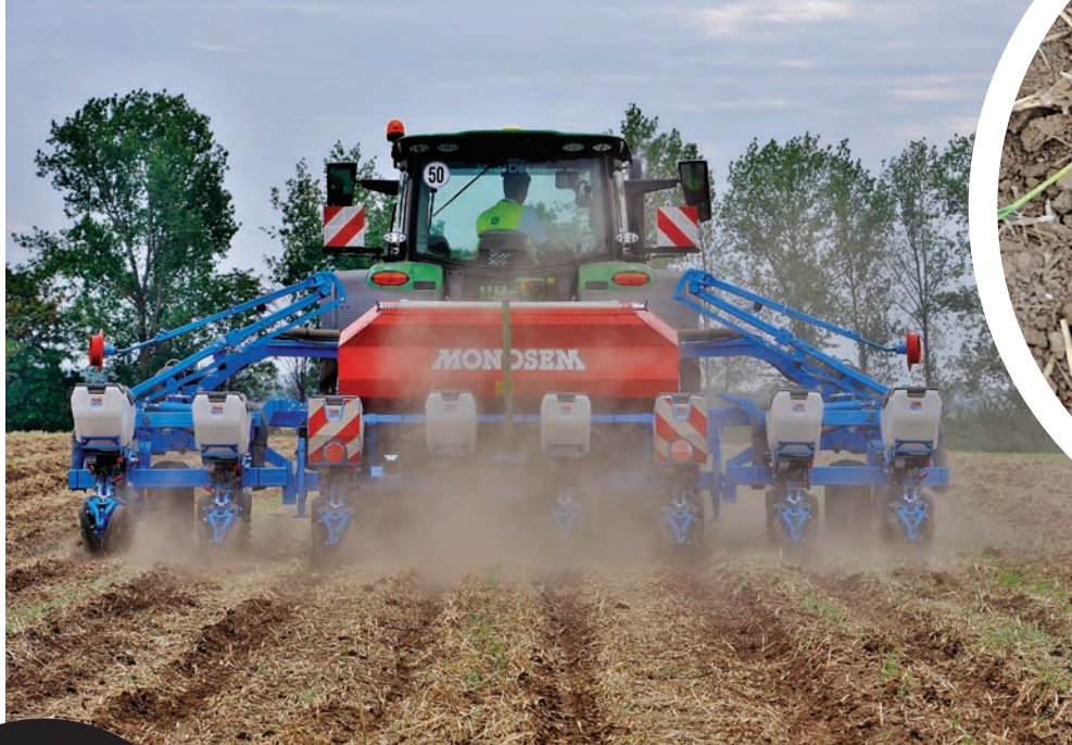
Left: GPS data from a tanker is used to control a precision seed drill. The seed is placed directly above the slurry belt (above inset) and the exact position of every seed planted is recorded
