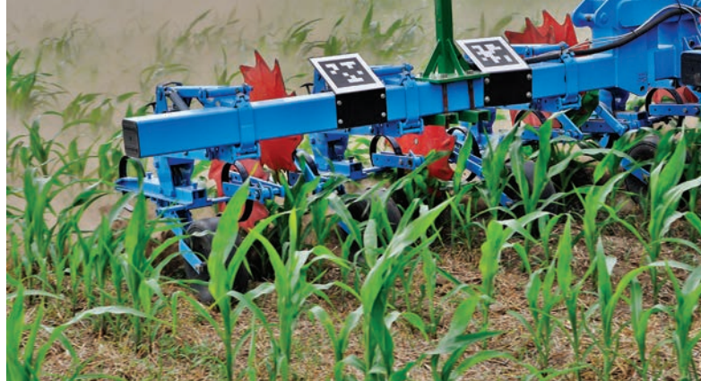
Above: Mechanical weed control uses data gathered by the AutoPath system on the seed drill to guide a hoe or cultivator
