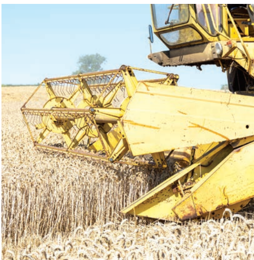
Above: The header is equipped with a 107cm-diameter reel fitted with 120-degree curved tines
