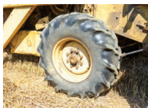
Left: This 1530 rides on Dunlop 8.50-12 tyres on its rear axle and a pair of Goodyear Torque Grip 18.4-26 tyres up front
