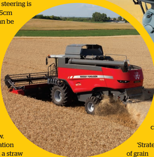
Above inset: The grain tank is 9000 litres on the MF 7370, or 8600 with ParaLevel option
