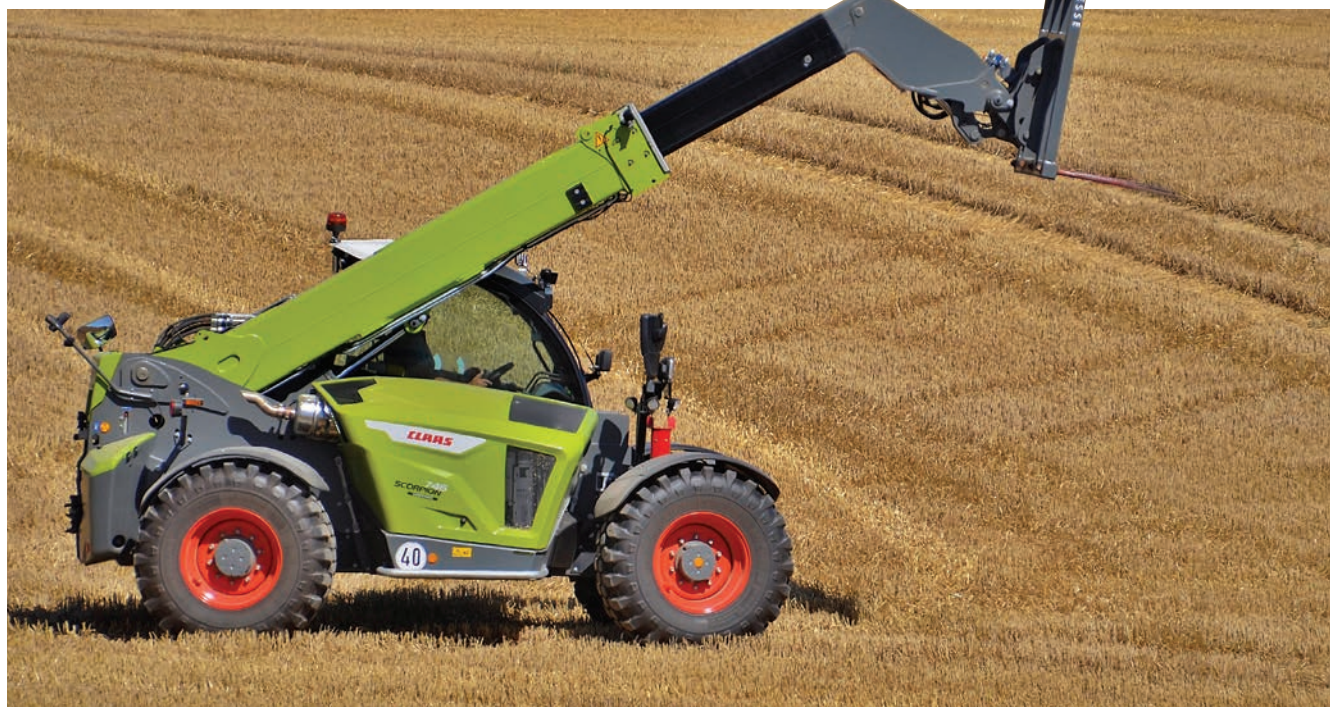
Below: Scorpion 732, 736, 741 and 746 models will get a more powerful Liebherr-optimised 3.6-litre Deutz engine, a revised cab with improved air conditioning and regenerative hydraulics
