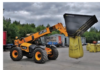
Above: The flow of barley from this pre-production bucket yielded approximately 500kg in 30 seconds
