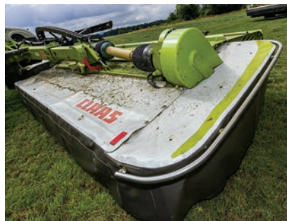
Below: In transport the 1100 will fold to well under 4m in height, but the three-point hitch has to be lowered
