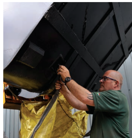
Above: Hooks on the base of the bucket hold bags in place and allow them to be moved away once filled
