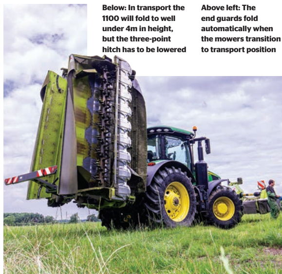
Above: Even the inner guards are automatic when folding, which prevents them hitting the floor
