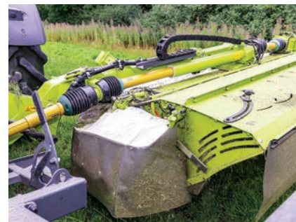
Above left: The end guards fold automatically when the mowers transition to transport position
