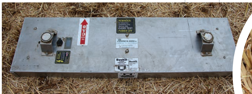
Above: The red drop pan sits inside the magnetic cover, which keeps the pan free of debris and grains until it is released
