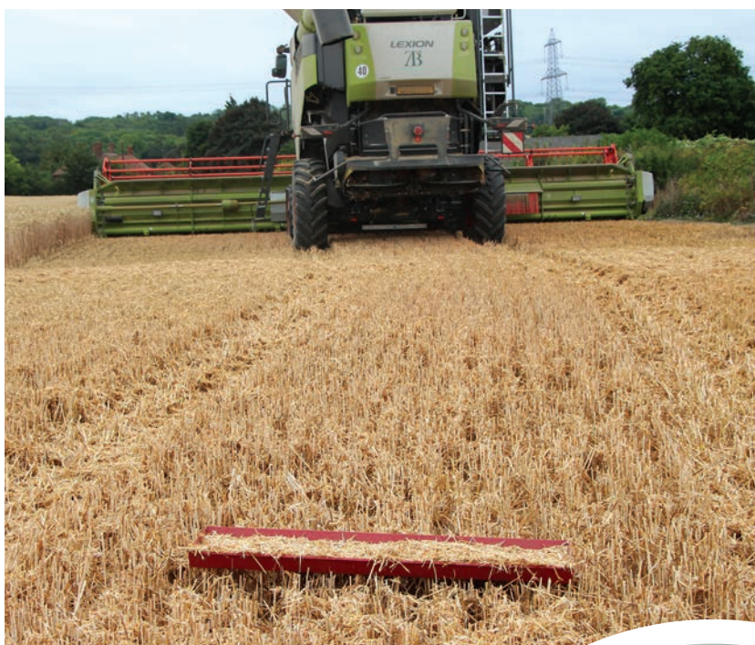
Above: The red drop pan sits inside the magnetic cover, which keeps the pan free of debris and grains until it is released
