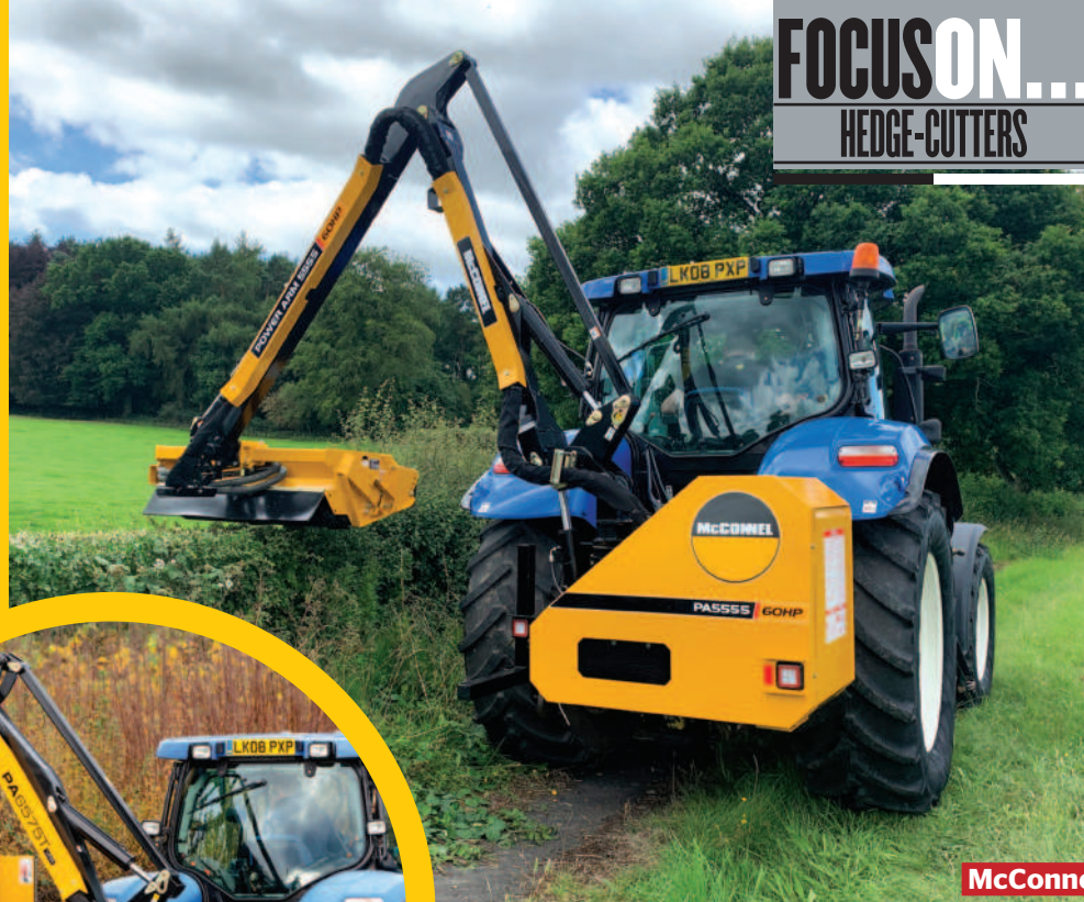
Left inset: The 6575 is mid-range in McConnell's 65 series. Reach is 6.5m with a telescopic arm
