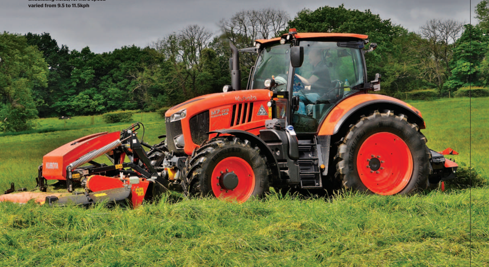
Mowing first-cut silage in Lancashire and dropping 6.4m of damp grass on undulating fields, forward speed varied from 9.5 to 11.5kph
