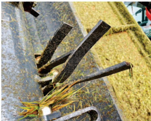
Above: The front mower was a new N-model featuring optional nylon conditioner tines. The rear unit was a T-model with steel conditioner tines. Note the single lever conditioner adjustment (left)
