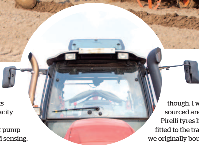
Left inset: Like many tractors indigenous to mainland Europe, the Iron's cab features an opening front screen and large sunroof
