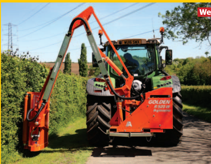
Above: 90hp is the minimum for a tractor hosting the R520, which weighs 1.1t
