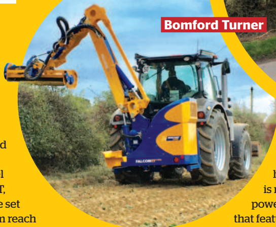
Above inset: The Falcon is the flagship in Bomford's VFA range; the forward arm improves visibility
