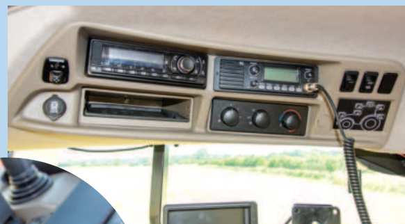
Above: A digital radio, CB, lighting, heating and air-conditioning controls are integrated into the roof console
