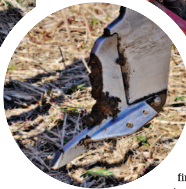
Above inset: The LDS tines and points lift and shatter simultaneously, with very little surface disturbance
