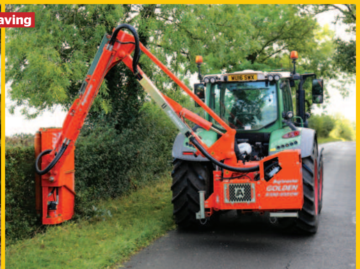
Above: The 6.5m telescopic arm of the Agrimaster R650T uses a three-belt head drive
