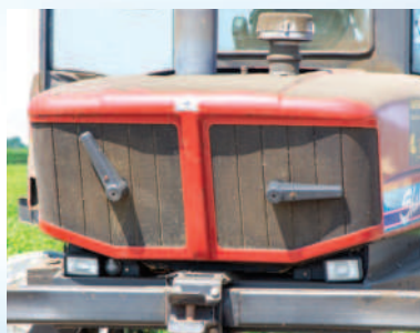
Left: The Advantage features an improved one-piece hinged engine cover, while all of Colin's swathers use rotary air intake cleaners
