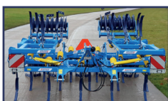
2023 FARMET Phantom 4.7m stubble cultivator, auto-reset tines at 215mm spacing, steel ring packer, tungsten points, in stock, enquire for demo
