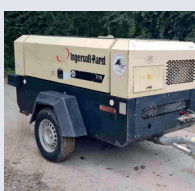
Ingersoll Rand 7/71 3790 hrs, 260cfm @ 7 bars, 4 outlets, Daumot DPF exhaust system. Choice from £7000
