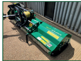
NEW SPEARHEAD SNIPER 270 NOW £5,950 WAS £6,250 2.70m cutting width, RH hammer flails, 10mm - 30mm cutting height, Rear Mounted, Hyd side shift.
