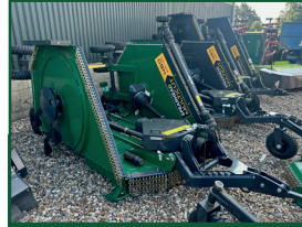
NEW SPEARHEAD MULTICUT 480 ECOLINE £20,500 4.6m cutting width, 3 rotor, 3 blades per rotor, 25mm - 400mm cutting height, hyd fold, standard wheels, standard axles, Alamo 250hp / 165hp gearboxes, standard towing eye, 6 spline PTO shaft, 1000 rpm, flat deck, 7 year gearbox warranty.
