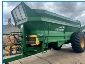
2010 BUNNING LOWLANDER 150 HD TVA £21,500 Widebody twin vertical augers, Flared sides, Greedy boards to make a 175, Hydraulic slurry door, Rear drawbar and connections, Sprung drawbar, Wide angle PTO, Road lights and beacons, 710/70R38 tyres
