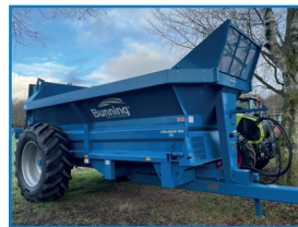
NEW BUNNING LOWLANDER 105 TVA MK4 £29,950 13.2m 3 10.5 tonne spreader, twin vert shrd augers 10mm Boron heat-treated steel, rubber protected, Grade 80 16mm floor chains with high tensile box slats, fully welded body, 14t axle hyd brakes, Walterscheid w/a PTO shaft, DA hyd slurry door, 580/70R38, T60 driveline, Flared sides to sheet height.
