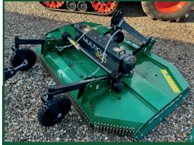
NEW SPEARHEAD MULTICUT 300 £9,500 2.84m cutting width, 2 timed rotors, floating headstock, 2 blades per rotor, 6 spline 1000 rpm PTO, 7 year gearbox warranty, 10mm - 350mm cutting height, 2 wheels.
