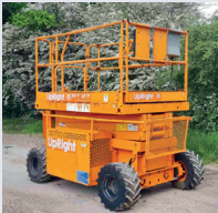
Upright 66907-001 4 person scissor lift, 4WD, 3cyl Kubota diesel eng 10.2 metre max platform height, extending deck & POA
