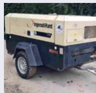
Ingersol Rand 7/71 3790 hrs, 260cfm @ 7 bars, 4 outlets, Daumot DPF exhaust system. Choice from £7000
