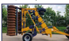
2014 TWB 6m 9 leg trailed subsoiler working tines, shouldered packers
