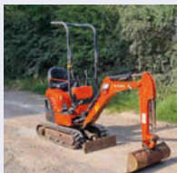
Kubota U10-3, 2017 micro-digger, expanding tracks 1825hrs, piped, offset, c/w 3 buckets GWO £11250
