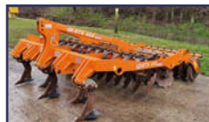
2009 SIMBA DTX 3m cultivator 5 subsoiler legs, Pro-active discs, 600mm DD lite
