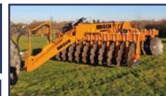
BROCK Deep Disc 4m heavy disc harrow c/w 36" disc blades to suit land reclamation, deep tillage or soil stabilisation projects, see video
