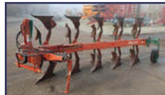
2007 KV LD85-200 5f hi-clearance plough, hyd ftr furrow, man vari-width, no.8's
