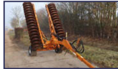
2004 SIMBA 8.2m DD Single Press, telescopic drawbar, width can be reduced
