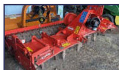
2014 KUHN HR 3004D 3m powerharrow, Q-fit tines, Maxipacker, due in
