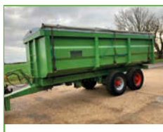
RICHARD WESTERN 14T GRAIN TRAILER Commercial axles with air and hyd brakes, roll over sheet .....£10000
