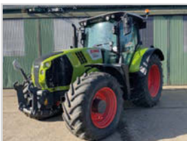
2019 CLAAS ARION 650 £POA 50 Kph, 189 HP, AdBlue Engine, 3,000 hrs, 540/65 R30 Fronts, 650/65 R42 Rears, 4 Spools, Front suspension, Front Linkage, GPS steering, A/C, Isobus, Air brakes, Electric Hyd, PU Hitch, Power Beyond, Cab Suspension
