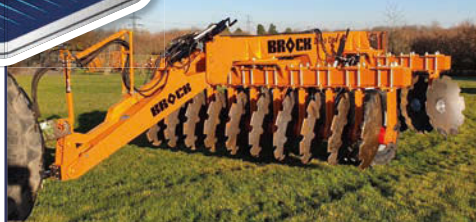
BROCK Deep Disc 4m heavy disc harrow c/w 36" disc blades to suit land reclamation, deep tillage or soil stabilisation projects, see video
