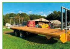
STAINES 27FT BALE TRAILER 20T commercial axles, air and hydraulic brakes ..... £8500
