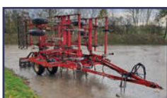
KONGSKILDE VibroTill 2800 6m primary/secondary springtine, 16cm tine spacing
