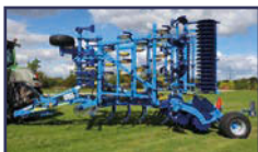
2022 FARMET Classic 6.5m stubble cultivator, hyd paddles, 4 rows of auto-reset tines at 200mm spacing, steel ring packer, in stock, enquire for demo
