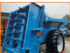
NEW BUNNING LOWLANDER 150 TVA MK4 IN STOCK 16 cu/m, 650/65R38 178A8, 16mm floor chains, Double acting hydr guillotine slurry door with indicator, Widebody augers (T60) Large diameter bottom blades, w/a PTO shaft 6 & 21 spline, Flare to standard sheet height, Weight cell ready with sprung drawbar 18T, Dual air/hyd brakes no ABS.
