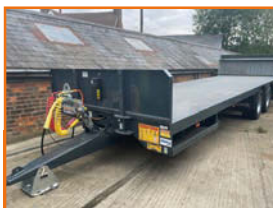
NEW RICHARD WESTERN BTTA16/28HS £15,995 Flat-bed trailer, mono leaf springs, 2.0m axle track, 2ft headboard, LED lights, Sprung drawbar, Air & hydraulic brakes with LSV for Air brakes, Hyd Load Sensing Valve
