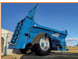
NEW BUNNING 105 TVA MK4 £29,950 13.2m 3 10.5 tonne spreader, twinvert shred augers, 10mm Boron heat-treated steel, rubber protected, 16mm floor chains with high tensile box slats, fully welded body, 14t axle hyd brakes, DA hyd slurry door
