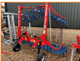
NEW OLICO GRASS HARROW £4,995 6m working width, 7mm tines, 4x flexing beds, 3m transport width, 32 tines/m in 6 rows, 10 angle settings.
