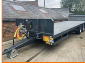
NEW RICHARD WESTERN BT16/28HS £15,995 Flat-bed trailer, mono leaf springs, 2.0m axle track, 2ft headboard, LED lights, Sprung drawbar, Air & hydraulic brakes with LSV for Air brakes, Hyd Load Sensing Valve
