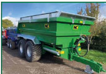
NC 20/22t Dump Trailers, Sprung D-bar & Magic Tailgate, Greedy Boards
