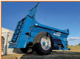
NEW BUNNING 105 TVA MK4 £29,950 13.2m 3 10.5 tonne spreader, twinvert shred augers, 10mm Boron heat-treated steel, rubber protected, 16mm floor chains with high tensile box slats, fully welded body, 14t axle hyd brakes, DA hydr slurry door
