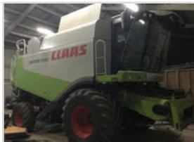
2007 CLAAS LEXION 530 POA 6m VARIO Header, 30 kph, 2650 / 1750 hrs, 800/65 R32 Fronts, 500/70 R24 Rears, RH V knife, Yield/Q Meter, Straw Chopper, Chaff Spreader, Reversing Camera, 5 walker, 3D hillside sieves, Chaff Spreader, CEBIS
