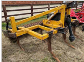
MCCONNEL SHAKERATOR £4,750 7 legs, Toothed packer, Shaker works ok, very tidy machine, 3.5m working width
