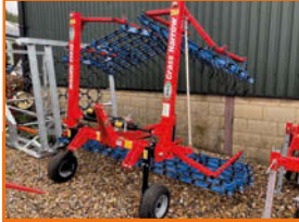
NEW OPICO GRASS HARROW £4,995 6m working width, 7mm tines, 4x flexing beds, 3m transport width, 32 tines/m in 6 rows, 10 angle settings.
