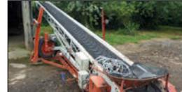
Straight Elevator with 60mm belt and Tracking wheels to slew from side to side. Plus powered drive 7.50 - 16 drive wheels. Small circular hopper and end chute. **Very Good Condition** ☎ Shaun 07850 978188
