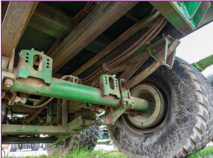
Prior to the introduction of the Extra models, leaf springs and hydraulic brakes were fitted as standard. Although this running gear is tough, the leaf springs can snap, particularly on units run at speed across tramlines or rough terrain. There is a great deal to check on all models so allow at least a couple of hours to look over a non-prepared buy.
