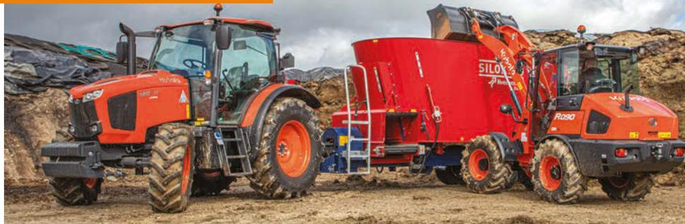
DPF cleaning intervals are 8,000 hours for the 6.1 litre engine, and up to 6,000 hours for the smaller 3.8 litre engine, again contributing to reduced operating costs. The engine oil change requirement is every 500 hours, on all M6-001 Utility models.
