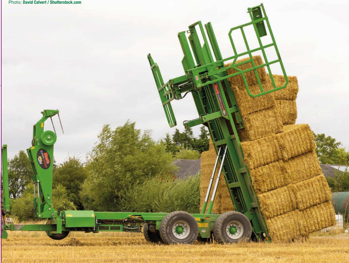
A straw hungry harvest always proves a great time for those with access to a bale chaser. These self-loading units collecting, carting and stacking bales without the need for a handler. Here we look at the established Heath SuperChaser models and outline what to consider when looking for a used example.
