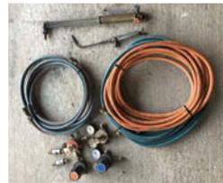
**£60.** Two separate Welding and cutting torches c/w 2x Flashback Arrestors for cutting torch, 2 X pairs of tubing and pressure regulators for Oxygen and Propane/Acetylene. No gas bottles. Cash on collection TEL: 07817 801287, West Sussex
