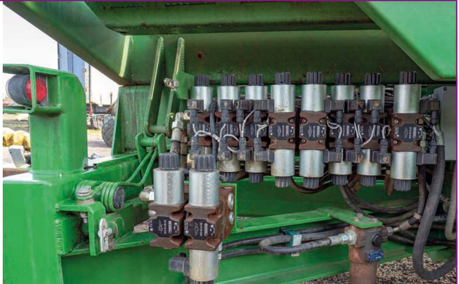
Located under a cover at the front of the chaser, the bank of solenoids that co-ordinate the various hydraulic functions will either work or not. The only way to check is to connect up a tractor and run through a collection and stack sequence.
