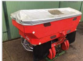
**2008 KUHN AXIS 30.1 QUANTRON-E £3,295** Electric shutoff, 3000kg rated, Headland Limiter, Wide fill hopper extension, LED road lights, Forward speed related spreading, Electric shutoff - new actuators fitted two seasons ago, 24m spreading vanes - New VXR vanes last season - very good, no pitting, Folding hopper cover - small tear on front LH corner
