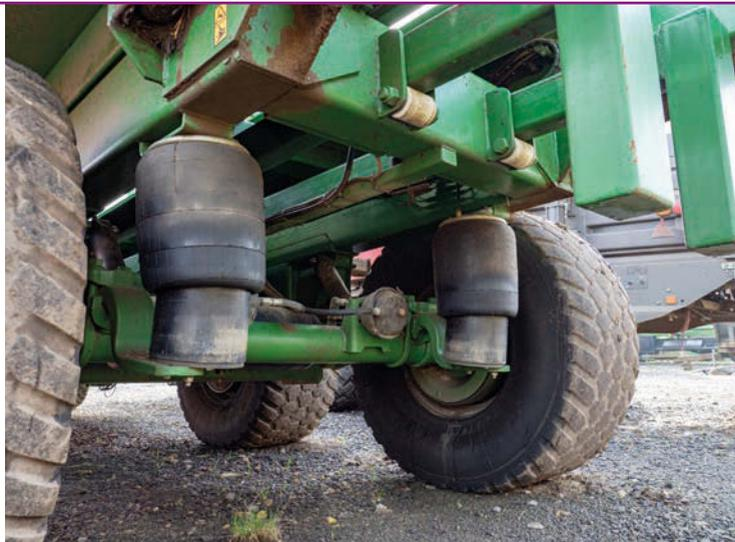
Air suspension makes a big difference to the ride of the chaser, with the system pretty much becoming a default fit for all Extra models from 2012. More recent models are likely to have ABS for the air brakes, ideal where fast road travel is part of the work cycle.
