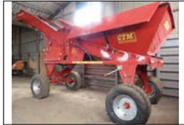
High Capacity beet cleaner loader fitted pre cleaner web in the middle. 3 Cylinder Deutz electric start engine drives the machine hydraulically and folds the elevator up and the hopper sides down as required for side loading. 40mm Rod links in base of hopper. 42mm Continental unloading web. Only done 160 hours work **Excellent Condition** ☎ Shaun 07850 978188
