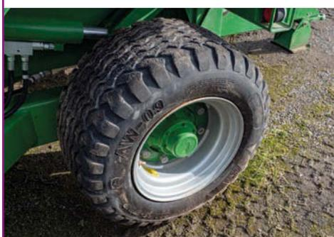
The small jockey wheel fitted to the front offside of all Extra models can take a real hammering, so check the tyre and rim. Most later models will be foam filled to resist punctures. Check the wheel rim and nuts. These must, like all wheel nuts, be checked for tightness as part of daily maintenance checks.
