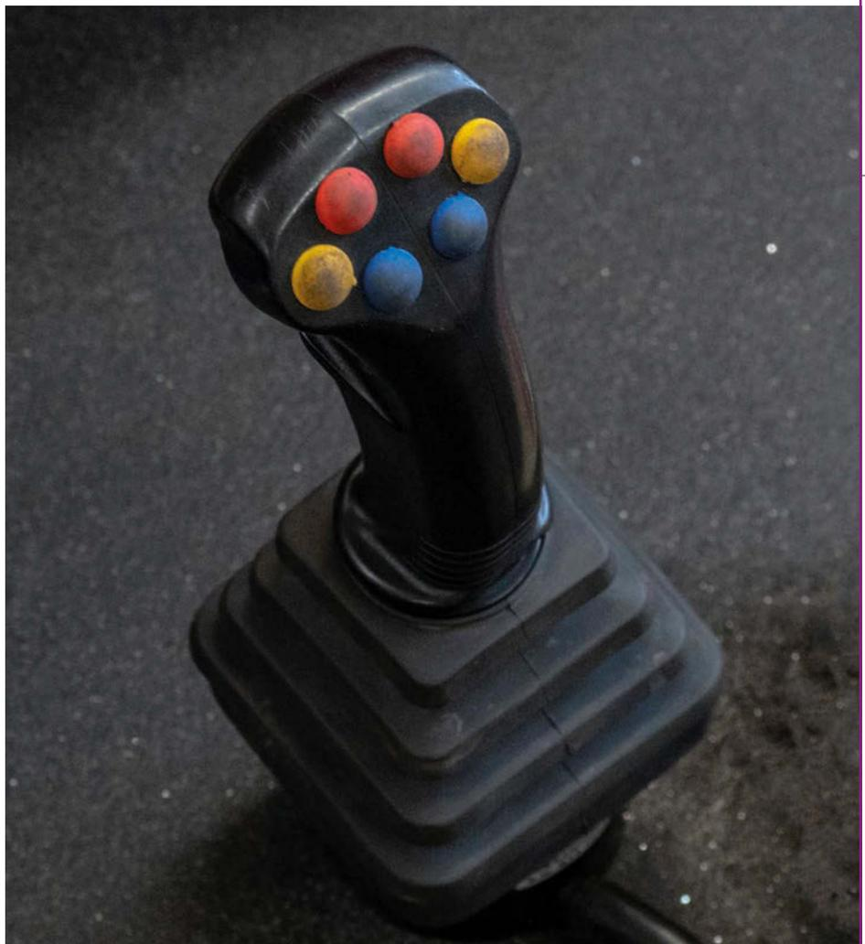
Colour coding helps identify the various button functions, a chart easing familiarisation of which does what. Although simple, it takes practice to seamlessly master operating a SuperChaser.
