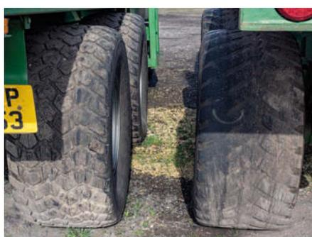
It is unlikely that there are many chasers running around on super single tyres now, radials offering greater floatation and holding up better at higher transport speeds. Pronounced shoulder wear is typical of units employed on fast road work (right).
