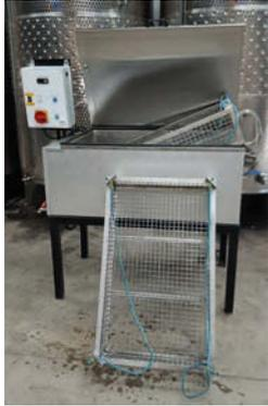
**POA.** 2 Vigo batch pasteurisers on stands and with 3 cages for lifting product in and out. Fully programmable for temperature and time, thermostatically controlled. 3 phase. 100 x 750ml. bottles capacity each. Very good condition. Less than half the new price
