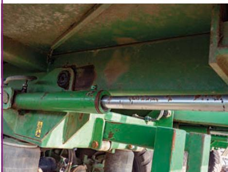
Some areas of concern are easy to spot, such as corrosion on a ram. Less easy to detect is wear in the pivot points. There are a number of grease points on all models and each needs a meticulous grease routine. As some can get overlooked, look for clear signs of recent greasing.
