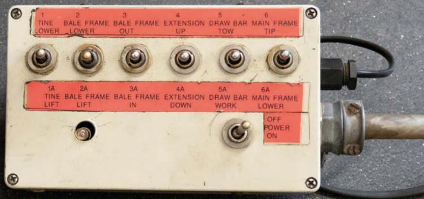
Original switchbox electronic controller may look dated but it is easy to use once you become familiar with what switch starts a particular action. Operators familiar with a SuperChaser can collect a load of bales in as little as five minutes, offloading the same as a stack in under a minute.
