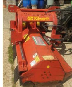
**£2,150 +VAT.** MTL200 flail mower, hydraulic side sift, front/rear mounted, some welds, reasonable life left in the flails. Video of it running up, side shift and working on request.
