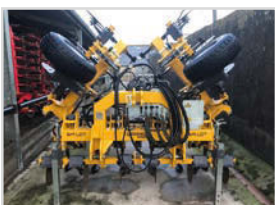
2020 GRANGE MACHINERY GM 6M LDT £31,750 Low Disturbance Toolbar, Hydraulic auto reset legs, Clevis hitch (HD CAT 3), Hydraulic front cutting discs, Free flow return extension, ISOBUS extension cable, Automatic wing folding, 7 pin socket, 6m
