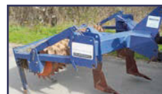
TIM HOWARD 3 Leg Subsoiler, rear tooth packer, shearin leg protection
