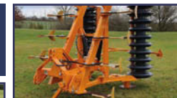
2021 BROCK Sub-V 4m 7 leg folding subsoiler, 571mm leg spacing, 700mm steel ring packer, swivelling scrapers, shearbolts, Cat 3/4 linkage, in stock
