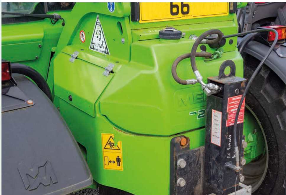
The 100 litre capacity fuel tank on the P32.6 is located at the rear of the handler, the pictured pick-up hitch providing useful protection should the machine get reversed into something. The battery lives at the front of the cab and is easily accessible.
