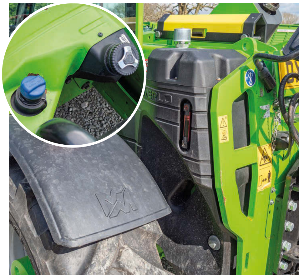
On the TF33.7, fuel is carried in an 80 litre capacity tank at the front nearside, along with a separate 15 litre Ad-Blue tank. The latter should not be allowed to run dry, a low-level warning light in the cab illuminating typically when the minimum level of 5 litres is reached. It is important to ensure the tank is filled with quality Ad-Blue and kept clean. Relocated to the rear, the TF33.7 hydraulic oil tank has a sight level and holds 85 litres. The guard protection should prevent reversing mishaps damaging the tank, but still check.
