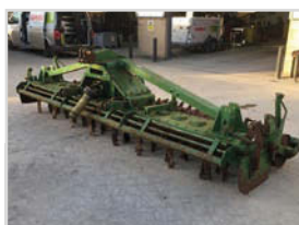
1990 DOWDESWELL POWER HARROW £2,985 4m power harrow, Rear packer roller, HD frame, Straight machine, Hinged side deflectors
