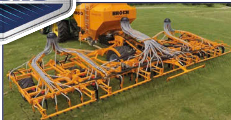
BROCK Campaign tine drill, 4 rows of coulters, 150mm row spacing, tungsten points, pre-em, Artemis control, available in 6m – 13.35m widths, see video
