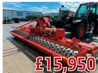
£15,950 41079847 KVERNELAND NG-H 101 F30, 6mtr hyd folding power harrow, rear packer with hyd depth control, 2015
