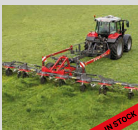
MF TD1028 X TRC TEDDER Hook tines 10.2M Working width 8 Rotors 7 Tine arms per rotor POA
