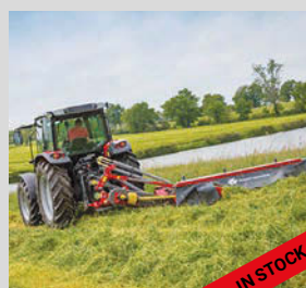
MF DM246 DISC MOWER 2.4m Working width 6 Mower discs Rear mounted POA
