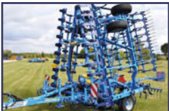
2020 FARMET Verso 8m/9m springtine, tungsten points, track eradicators, front & rear levellers, 5 rows of tines, rear harrows, in stock
