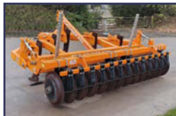
2012 SIMBA Flatliner 3.5m 5 leg subsolter, Pro-lift legs, DD packer
