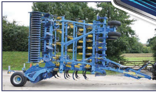
2021 FARMET Classic 8.5m stubble cultivator, front levelling paddles, 190mm tine spacing, levelling discs, steel ring packer, 330-495 hp, in stock
