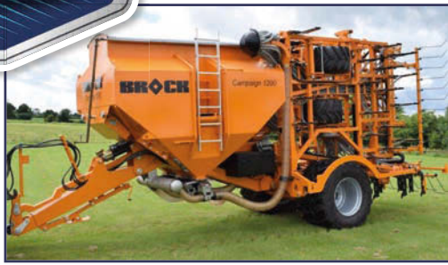
BROCK Campaign tine drill, 4 rows of coulters, 150mm row spacing, tungsten points, pre-em, Artemis control, available in 6m - 13.35m widths, see video
