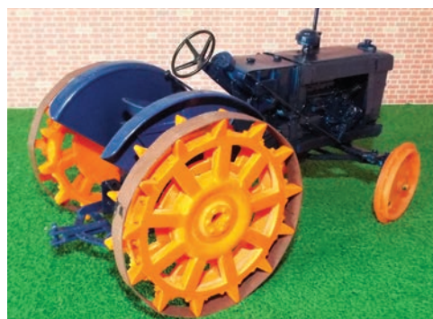
ABOVE: The final design for a governor to suit the OHV engine had yet to be undertaken so a Weybourn governor was adapted to fit the tractor. A considerable amount of work was still to be done at the front end of the engine, and as yet a diesel version had not been assembled.
