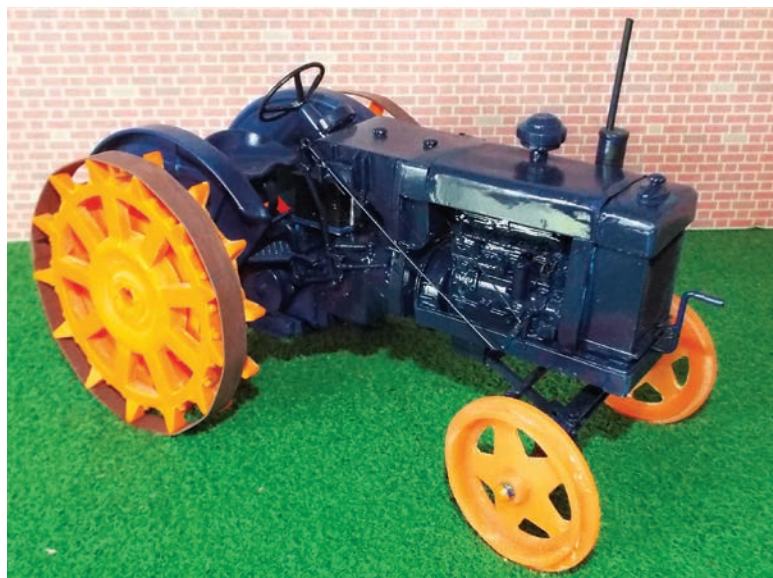
ABOVE: The final design for a governor to suit the OHV engine had yet to be undertaken so a Weybourn governor was adapted to fit the tractor. A considerable amount of work was still to be done at the front end of the engine, and as yet a diesel version had not been assembled.
