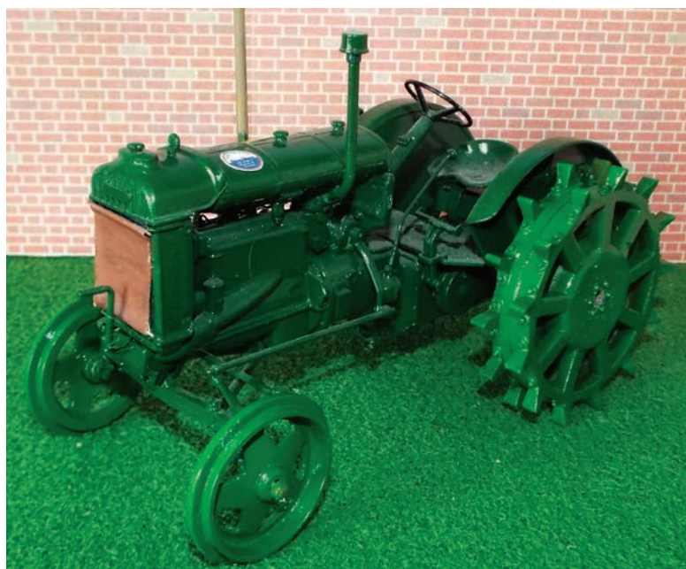
The final prototype built in 1944 was close to the production tractors apart from a few details. Shared parts between the N and E27N meant that from the dash forward the tractor was almost pure model N, apart from the front axle.
