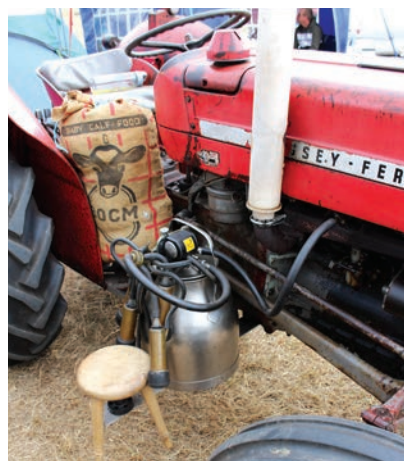
LEFT: A tap from the exhaust manifold allowed a small milking machine to be operated in the field from the 135.
