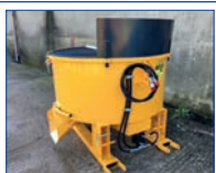
NEW HYDRAULIC PAN MIXER, 850LTR / 3/4M CUBE, 3POINT LINKAGE AND PALLET FORK MOUNTED .....£2,600
