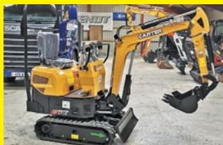
NEW CARTER CT10, 1 ton micro digger, 180° slew, manual QH, 3 buckets.
