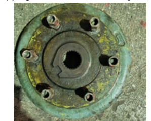
Brake drum for Bautz 300 tractor , this brake drum is also a drive. Email: p.gibbons126@gmail.com. [LAW122]
