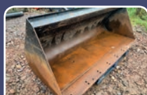
USED Strickland Bucket , Heavy Duty, 2.24m (7ft4) wide, approx 1m 3 capacity, very strong & well made bucket, perfect for stone, rubble etc. Holes for digging teeth. JCB Q-fit brackets .....£1,495
