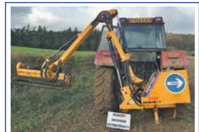
1999 Bomford B458 hedge trimmer, good working order, 1.3m head with boot flails, cable controls ..... £3,600
