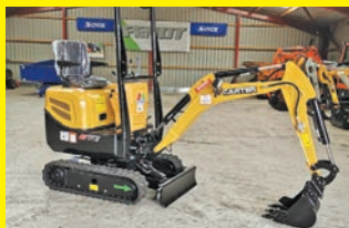
NEW CARTER CT12, 1.2 ton, 3 cyl Yanmar engine, expanding tracks, expanding blade, QH.
