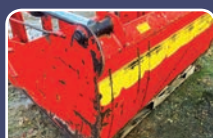
USED Conor 150 Shear Grab , 1.5m wide, approx 0.85m 3 capacity, 12 tines (all tight & straight), twin ram, good cutting edge, hydraulic hoses, in good condition but with some welding. Trima No 5 brackets .....£1,095
