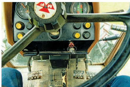
Above: During his 1985 test drive, Terry found the foot throttle, positioned only just right of centre beneath the steering wheel, wasn't the most comfortable or natural to use. However, longer-term users say it is something you get used to.
