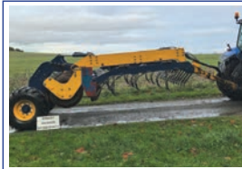
2003 TWB Terminator 3 metre trailed cultivator, very good condition, heavy duty spring tines, hydraulic shatter boards and 800 mm packer roller ..... £POA
