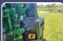
NEW Quicke Q-Bloq counterweights , 600kg to 1,800kg, additional 600kg add on available, 3 point linkage mounted, very sleek and stylish weight blocks. Choice of sizes & colours in stock.....£POA
