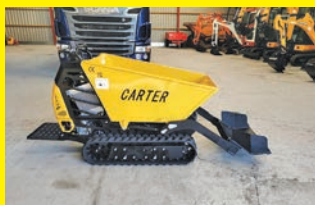
NEW CARTER MINI DUMPER, 500KG payload, 760mm wide, front power loader.
