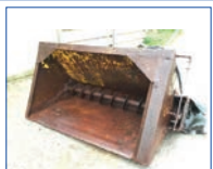
FEEDER BUCKET 6FT HYDRAULIC DRIVE BOBCAT BRACKETS OR EURO BRACKETS GWO .....£750
