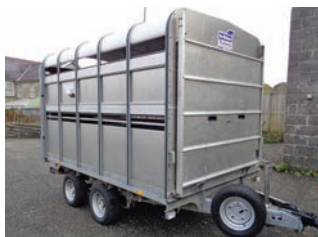
Ifor Williams DP120G-10 livestock trailer , length, ten-foot, gross weight, 3,500kg, standard ramp, twin axle, deep chassis, large cross-division gate, removable container, lockable drawbar coupling, tyres: 195/60R12C, spare wheel (brand new). £3,500 + VAT. Tel: 07855 356468. Carmarthenshire. [ABW78]
