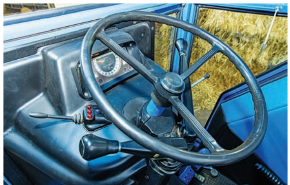
Above: Replacement dashboard shrouds for this Lambourn cab are no longer available, so the damaged original had to be skilfully repaired.
