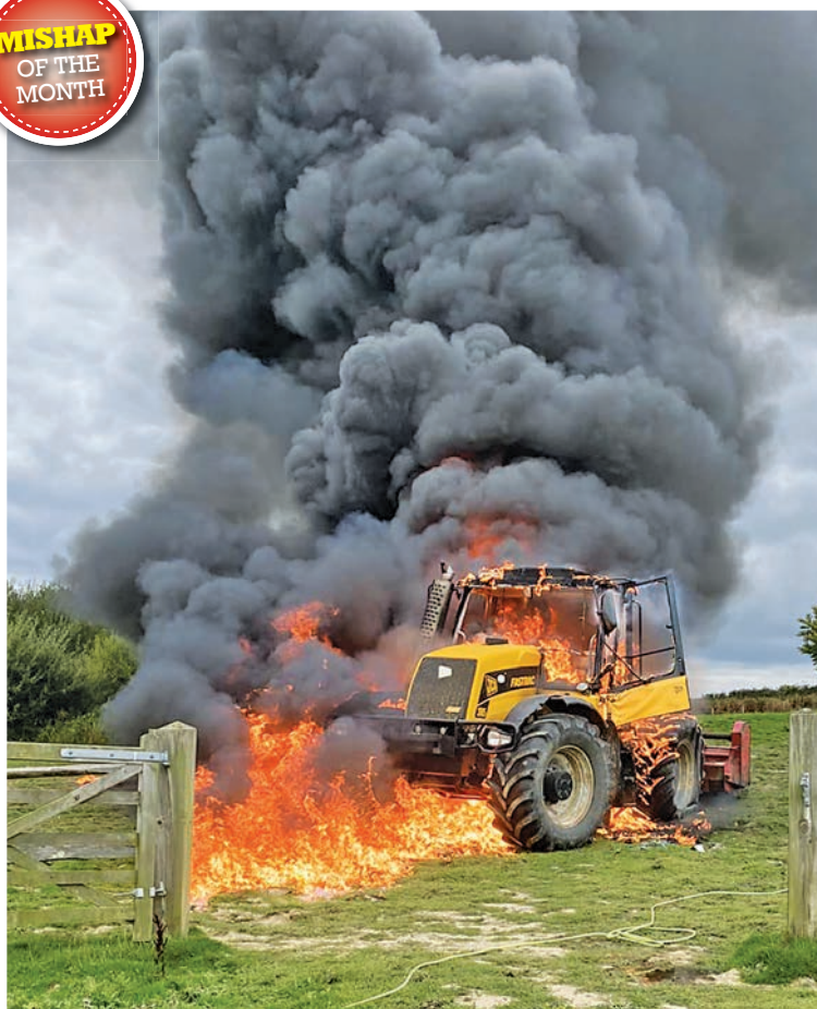
Lloyd Baker had worked hard to buy this JCB Fastrac 3185 and it was his pride and joy. Understandably, he was left devastated after an electrical fault, that nemesis of all older JCB Fastracs, caused this catastrophic fire.
