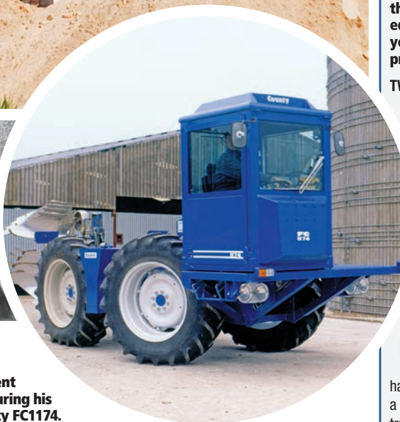
Above right: The County 1174FC, launched in late 1977, represented a significant departure from the ageing 1004FC it replaced, both in terms of its appearance and features. As well as a new modular cab with plug-in electrical and hydraulic services, the 1174FC also had fuel tanks between the wheels and a greater load capacity. This early 1174FC, probably a pre-production machine, appeared in early marketing material.
