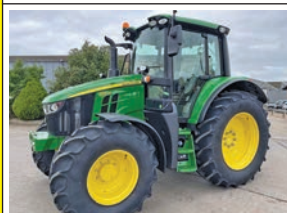
JOHN DEERE 6120M 5/2022, 500 HOURS, 24X24 AUTO QUAD, ECO-SHIFT, 40K, CAB + FRONT SUSP, 3 SPOOLS, AIR CON, AIR SEAT, 114 LT HYDRAULIC PUMP, HI-LIFT.
