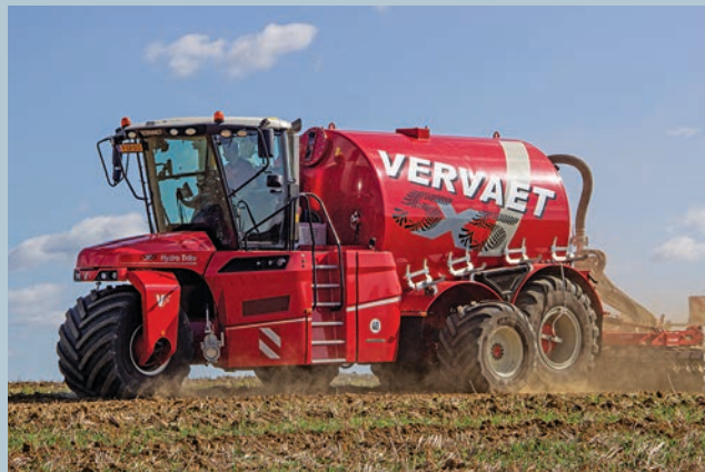
Above: Recent product updates have included the introduction of a more advanced variable transmission and the option of five-wheel drive for the XL version of the Hydro Trike.
