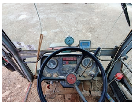
Left: What no bonnet. Sitting in an MF 600 Series cab and looking out across a blank space where the engine and bonnet would normally be is a strange sensation. The engine on this forward control Knight conversion is behind the cab.
