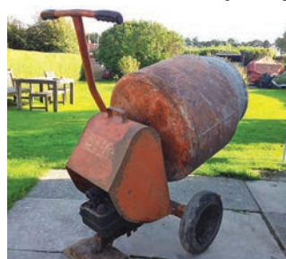
Belle petrol mixer, from 1973, original, strong-made early style with metal engine shroud, Briggs 3hp engine, looked after machine, needs carb priming from cold otherwise good running condition, with a stand. £90 collection only. Tel: 01253 836653. Preston. [LAW50]
