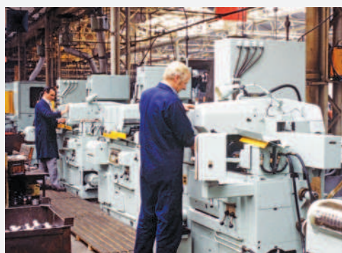
Left: More American investment in the form of what were, at the time (1970s), state-of-the-art gear cutting machine tools.
