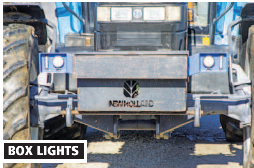
Left: Alec originally made this weight box for a New Holland TM140. The newly-added blue brackets house a set of flashing strobes and LEDs.
