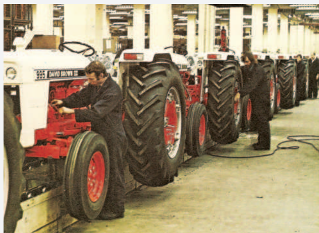
Above: David Brown 9 Series tractors near the end of the main assembly line in R Block. The fitment of PAVT rear wheels, flat fenders and high nose cone lighting suggests they were destined for export, possibly to the USA.
