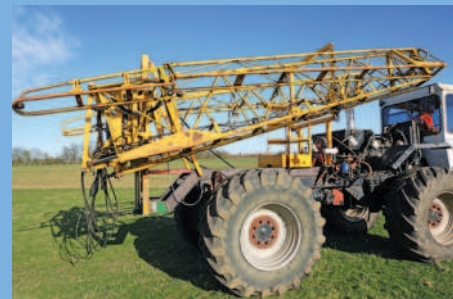
Above: Dave has fabricated a substantial demount frame for the applicator. The adapted mast, booms, boom-rests and platform came from a donor Chafer E-series trailed sprayer.
