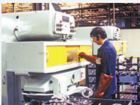
Left: Gears being wet cut. Cutting oil was fed onto the cutting head to minimise wear and tooth distortion, hence the splash screen and operator's rubber gloves.
