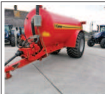
Conor 2500 tanker, with Dodo pump to supply umbilical system, 2016
