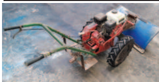
Mayfield 5.5hp petrol Detroit engine, two wheeled garden tractor, currently with snow plough / yard scraper attachment including snow chains and balast boxes, good runner, regularly used for paddock mowing (mower attachment not included in this sale) new tyres and recent oil change, there are 3 forward and 1 reverse gear they all work although the linkage is slack, the clutch sticks a bit but again it's very useable, Could be used "as is" or restored for showing. £350. Tel: 07971 360 145. Cheshire. [HT19W25R]
