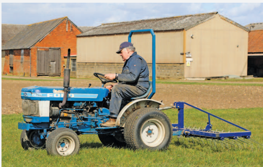
The 16hp Ford 1210 was the smallest member of the Series 10 family. Richard Carr's example, fitted with a replacement Perkins engine, is useful for mowing field margins.
