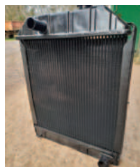
Ford 5000, genuine Fo MoCo radiator , been just re-cored, reconditioned, tested and ready to fit. £225 + VAT. Tel: 07870 559146. Ludlow. [DEW63R]
