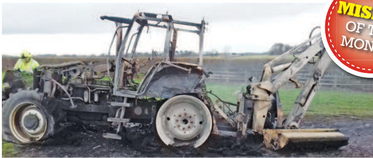
Back in 2017, an electrical fault in the dashboard of Angus Dods' Case IH Maxxum MXM140 caused a fire that completely destroyed not only the tractor, but also the McConnell hedge cutter attached to its linkage. Talk about a double whammy.
