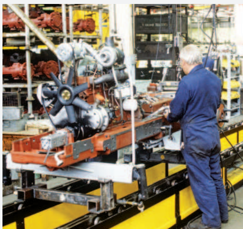
Above: This photograph was taken at the west end of the upper line in R block. Note the Plessey front-mounted tandem pump, a rarely specified optional extra which doubled the flow via an operator actuated combining valve.
