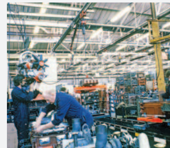
Above: A view of the upper line in R Block. Note the fitment of the Plessey power steering pump. This task was always done by two weekly rotating personnel from Engine Rectification Shop 109 at Meltham Mills. Photos courtesy of Stuart Gibbard.
