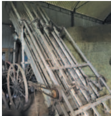
Bamford hay loader, barn stored and in working order, to follow behind wagon and pick up loose hay, driven by land wheels, winner of the RASE Silver Medal in 1919. £Offers. Tel: 07889 896872. Hereford. [EFW80]
