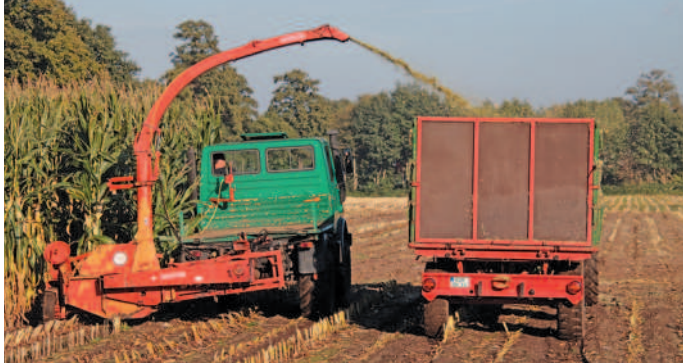
Above: A 100hp Mercedes-Benz Unimog 1000 from 1980 working with a two-row Kemper semi-mounted forage harvester attached to its three-point linkage.
