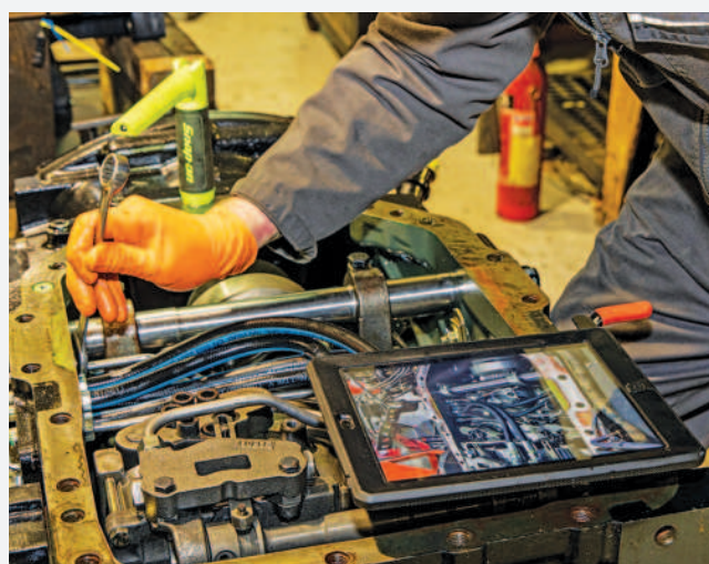
Technician Dan Smith double-checking the connections for the AGCO ML180 Vario unit after it has been loaded into the JCB casting for testing.
