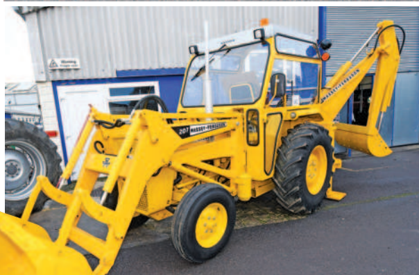
Above: Adding a splash of bright yellow to the predominantly red and grey display was D. Scurlock's 1969 MF 2203 industrial tractor equipped with a Winsam cab, MF 207 loader and MF 220 backhoe.
