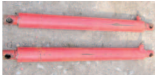
Loader rams , used single acting, 33.25 inch between centres closed, 3 inch OD. £180, buyer to collect. Tel: 01889 500303 or 07850 525693. Staffs. [CDW51R]
