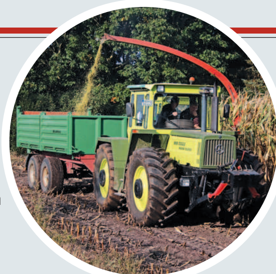
Above: This 156hp MB-trac 1600 turbo was busy carting the harvested maize crop with a 10t twin-axle tipping trailer.
