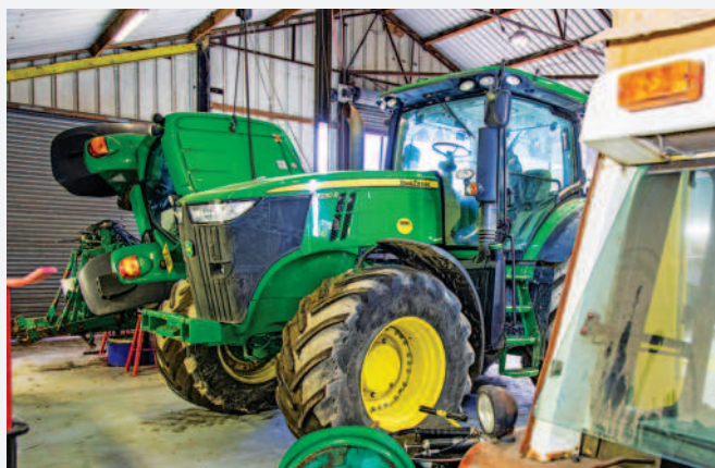
The source of a transmission rumble at 1500rpm in this John Deere 7230R was being investigated by the Swinnerton Machinery team.
