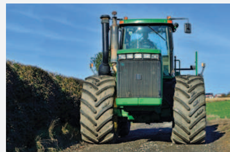
Jonty's decision to equip his John Deere 9400 with 900/50R42 wide singles has made it much easier to use on the road compared to its previous dual-wheel set-up.
