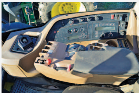
Main controls on the John Deere 9400 are conveniently located on the right-hand CommandArm and console. The throttle, the lever for the 12-speed powershift, and the linkage and spool valve controls are all in the armrest.
