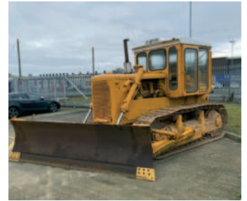
Caterpillar D6 Bulldozer with 3m Blade
