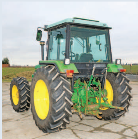
Above: Some rust on the nearside mudguard is probably this tractor's worst feature. The paintwork on the back end has fared remarkably well, but the cab roof has faded in the sun.
