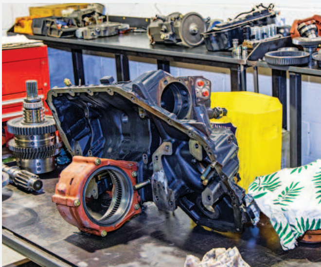
A Steyr CVT tractor from the early 2000s is something of a rarity in the Swinnerton Machinery workshop as they are normally a very reliable unit. This one was suffering from a long working life.
