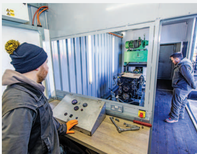
The ML180 Vario transmission performed as expected during the test, with nothing but a few oil splashes to see. Dan Smith, left, is standing by the remote engine and clutch controls.
