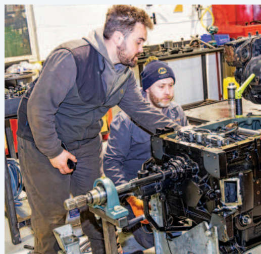
Tom Swinnerton, left, helps technician Dan Smith to prepare the AGCO ML180 transmission for its run in the test cell.
