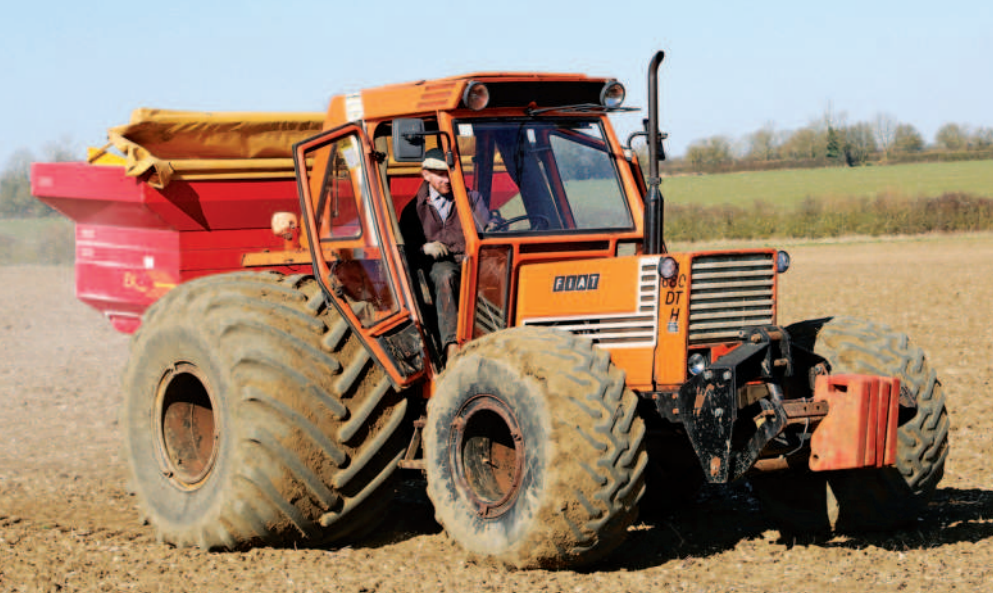
Above: This T-registered Fiat 680 DTH was the first to arrive at Radwinter Park Farm and has done the most hours (5634). It makes an impressive sight when shod on these low ground pressure 66x43.00-25NHS Goodyear Terra-Tires, which barely leave a mark on the surface.
