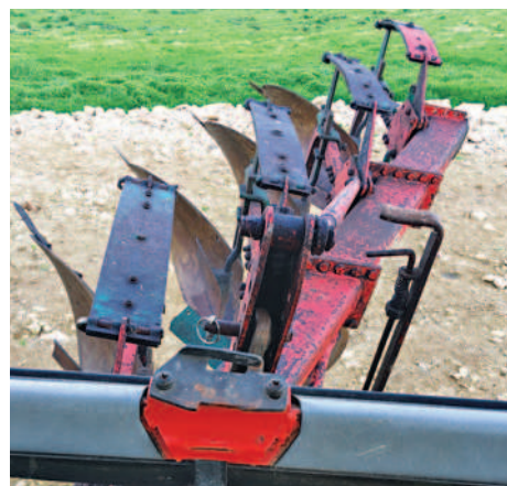
Above right: This Kverneland four-furrow auto-reset plough, a recent purchase, is period-correct for the age of the tractor. Right: A set of taller 38in rear wheels, aimed at reducing the generous tyre-to-mudguard gap, are on this owner's wish list.
