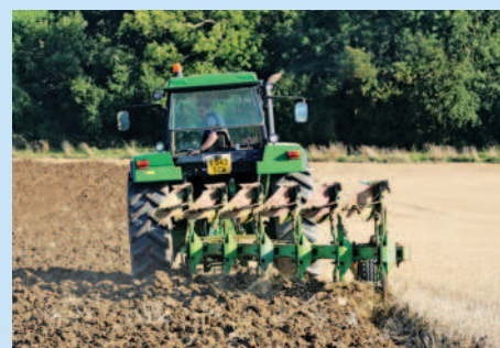
Above: Once set-up to suit the tractor, the Dowdeswell plough worked well, with its UCN bodies inverting the medium-to-heavy soil nicely and producing a level finish.
