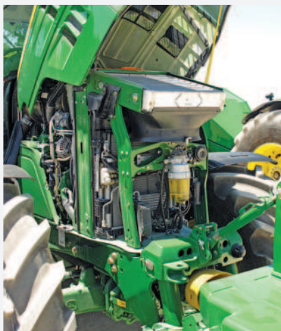
Above: The cooling pack on a modern John Deere 6R Series tractor, circa 2011. Modern cooling systems incorporate separate radiators/coolers for the engine, intercooler, hydraulic and transmission oil and air conditioning (condenser).
