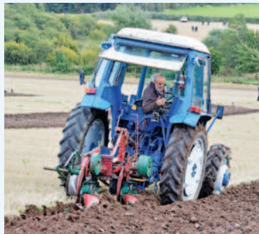
Bill Tonkin's four-wheel drive Ford 4600 is unusual in having a centre-drive Kramer front axle. The Devon ploughman was competing in the plough-off in the Conventional class.
