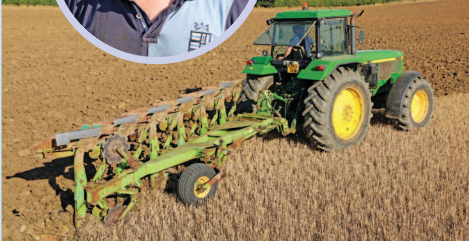
Above: Jon bought his Dowdeswell 120 Series MA plough this September. It was set to a 12in furrow width, but Jon had adjusted this to 14in before starting work.
