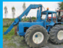
COUNTY 1164 c/w crane
