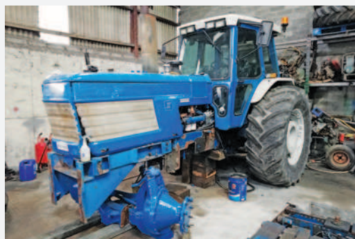
Above: Prior to the front axle from the donor County 1454 being fitted, the chassis of the Ford TW-35 was strengthened. Inch-thick steel plate was used to make a new frame to hold the front cross-member. This frame also houses a look-alike diesel tank.
