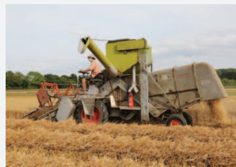
Above: This 1964 Claas Europa, the smallest self-propelled combine in Charles' collection, has been retro-fitted with a grain tank from a later machine.
