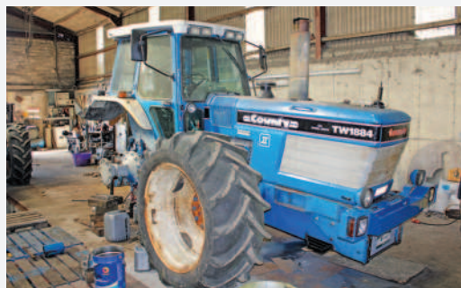
Above: The front linkage arms and rams, etc were removed, but the frame was retained and strengthened using inch-thick steel plate. Note how the tractor has already gained its non-standard but stylish bonnet decals. This wheel fitment was temporary.
