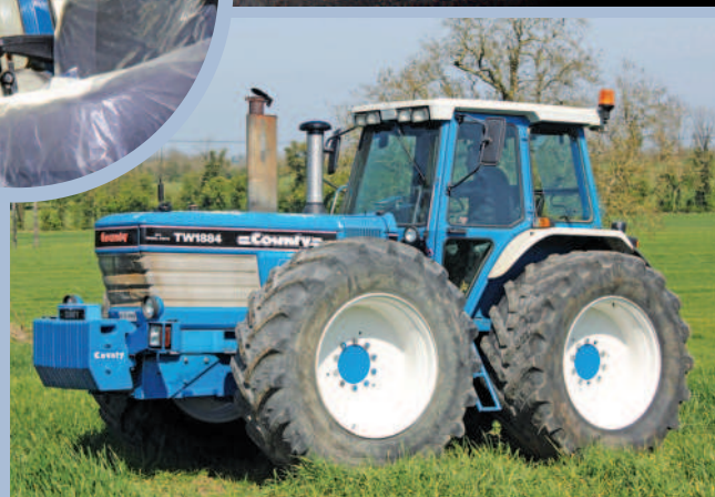
Above: Non-standard mods include the fitment of an extended stainless steel air cleaner stack, a bonnet-mounted CB aerial, additional work lights and a flashing beacon.
