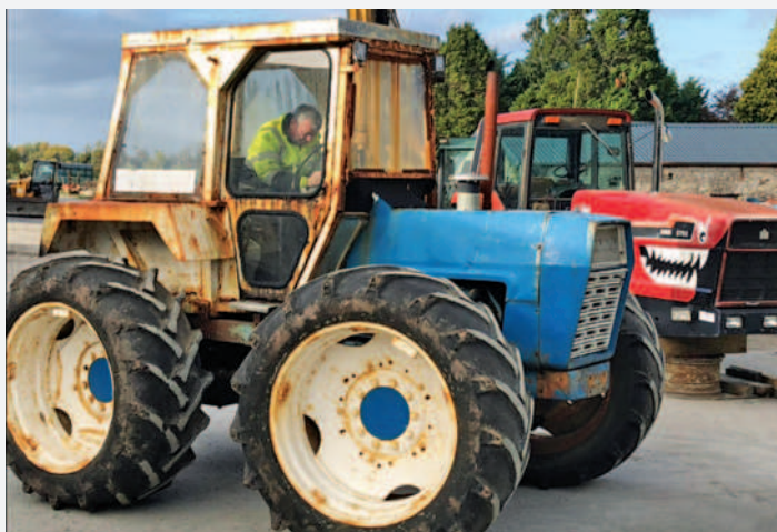
Above: A donor County 1454 was found in Co. Mayo in the West of Ireland. Its cab was rough, but crucially it had all of the essential four-wheel drive parts required to transform Pat's Ford TW-35 into a replica of a County 1884.
