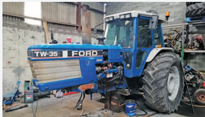
Above: One of the first jobs in the workshop was to remove the front axle from the Ford TW-35 in the workshop. As the owner of Overseas Plant Sales, a construction equipment retail business, Pat and his team are used to working on heavy machines.
