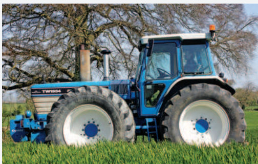
Above: During an initial trial fitment of the front axle, it was found that the gap between the front and rear wheels was insufficient, to the point where the tyres almost touched. Mounting the front axle further forward on the chassis overcame this problem.
