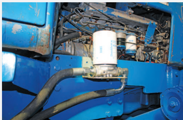
Top: The Ford TW-35's hydraulic oil filter was obstructing the path of the offside four-wheel drive shaft, so it had to be removed and relocated. It now sits neatly on a new bracket on the main chassis frame, above. It is much easier to access now.
