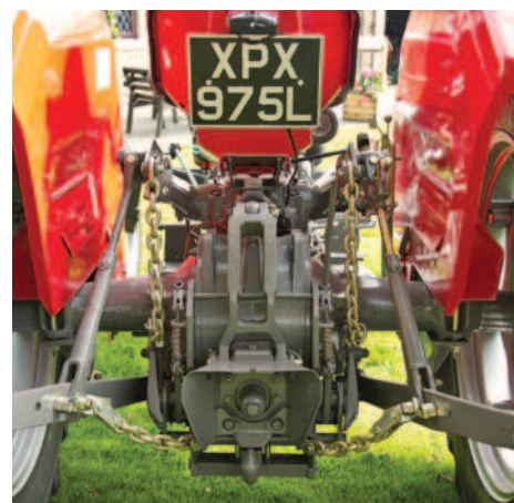
Above right: Genuine Massey Ferguson enamel paint has been used throughout to recreate a sympathetic ex-factory paint finish. Right: Trevor, always a stickler for detail, has fitted the correct MF 148 PTO guard, which differs slightly to the MF 135.
