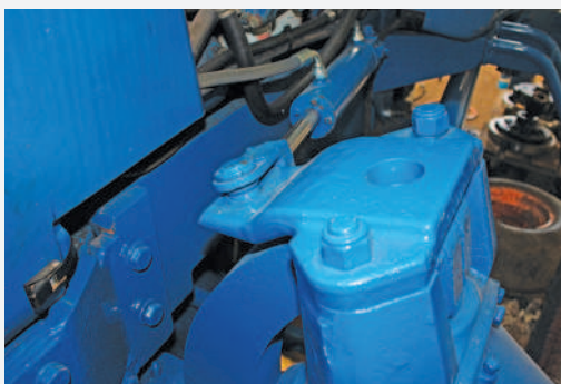
Above: A section of the Ford TW-35's nearside bonnet side panel had to be cut out to provide sufficient clearance for the power steering ram. This tinwork adaptation was also carried out by County engineers on the original 1884.
