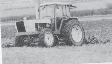
Six cylinders up front, not enough furrows behind. FTD's Chieftain tractor makes light work of three furrows ploughing 10in deep.
