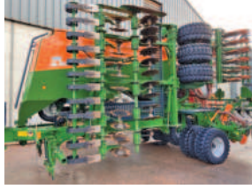
AMAZONE CIRRUS 6003-2 DRILL 2017, 6M, RADAR, LEVELLING BOARD, 2 ROWS OF ROTEC PRO MATRIXEM DISCS, TRAMLINE KIT, PRE EMERGENCE MARKERS, TRACK ERADICATORS.
