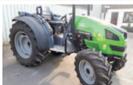
Deutz-Fahr 3050, 51 hp, 12F x 12R gears, 44 x 18 -20 rears tyres, 31 x 13.5 -15 front tyres. £24,732
