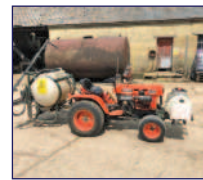
Kubota B4200 4wd , c/w sprayer set up, excellent condition, electric rate control.
