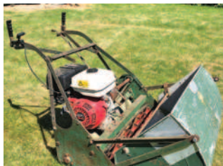
Vintage Atco cylinder mower, 34" cut, new Honda 9hp engine fitted, ideal for cricket pitch etc. Tel: 07802 453554. East Yorkshire. [JW56R]
