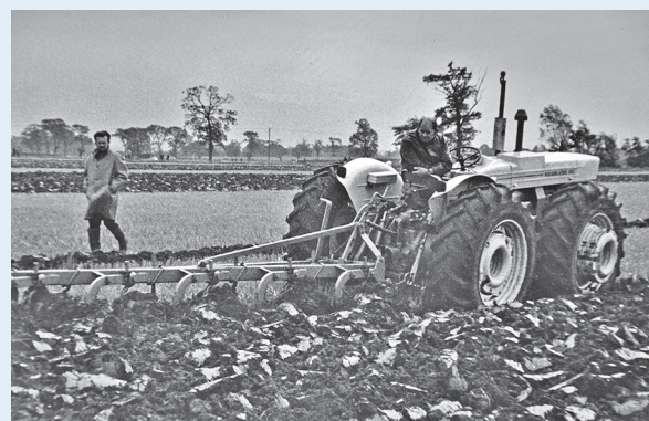
Above: Keeping a close eye on the ploughing during a 1968 demo. The equal-wheel Roadless 115 that Arthur was using with a five-furrow conventional plough at this event was new on the scene, having made its debut at the 1968 Royal Show.
