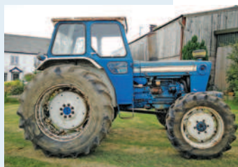
Ford 7000 has been converted to four-wheel drive with a Schindler axle.
