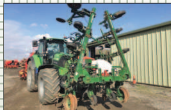
Garford robo-crop front mounted hoe for raised bed with camera and colour screen .....POA
