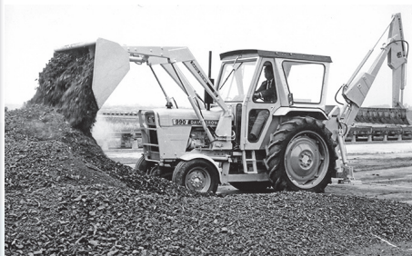
Above: A David Brown 990 Highway model equipped for industrial work with a David Brown front loader and a Ditcher-Digger-Loader attachment acting as a backhoe.
