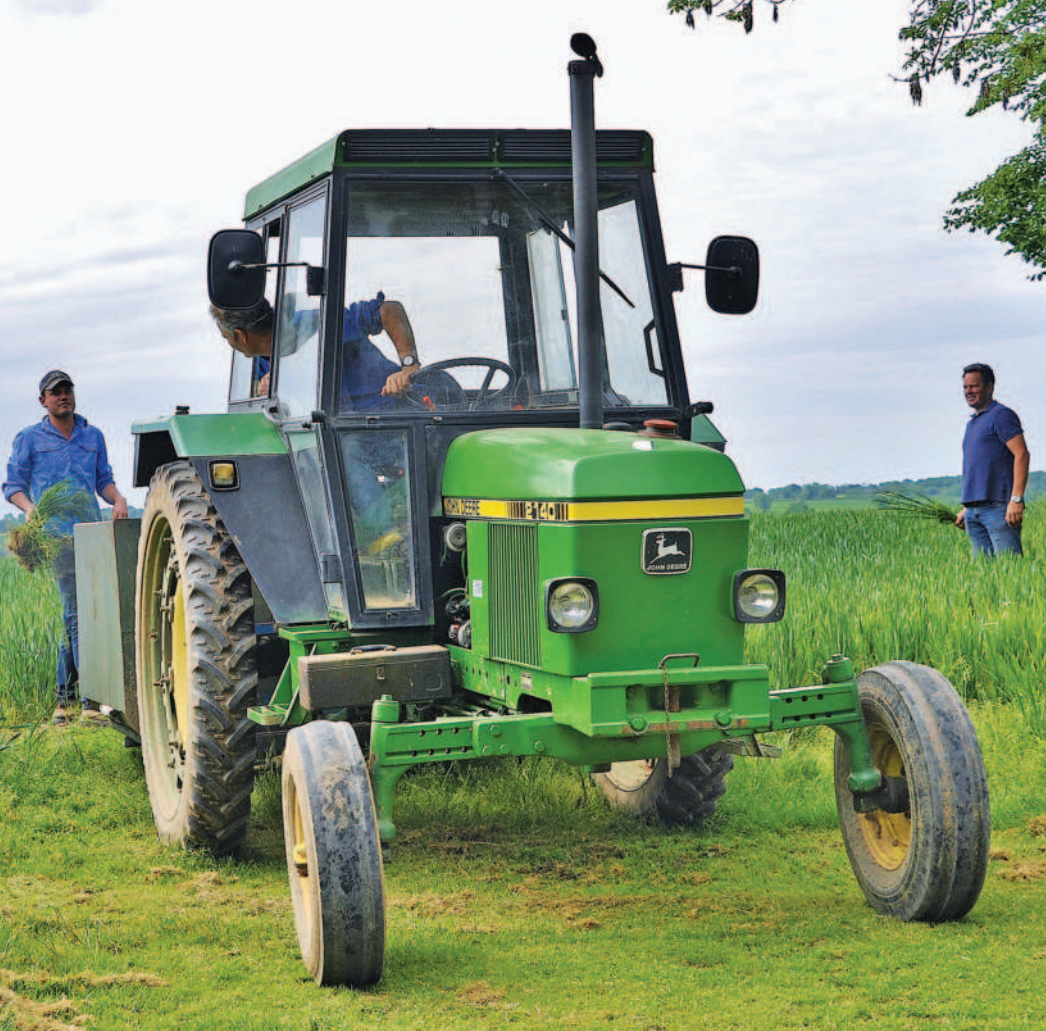
Left: Purchased new by the Hibbert family in 1980, this very clean John Deere 2140 is equipped with the Sekura OPU cab that was a feature of the early 40 Series tractors, circa 1979-1981. It has clocked 16,000 hours.
