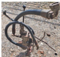
Auxiliary service spool valve , for 100 Series Massey Ferguson tractors with Multipower, single lever, foot plate mounted, can be piped to combine flow from main hydraulic pump and Multipower pump for increased flow. £250 ono. Tel: 07970 919666. Totnes. [HIW17]
