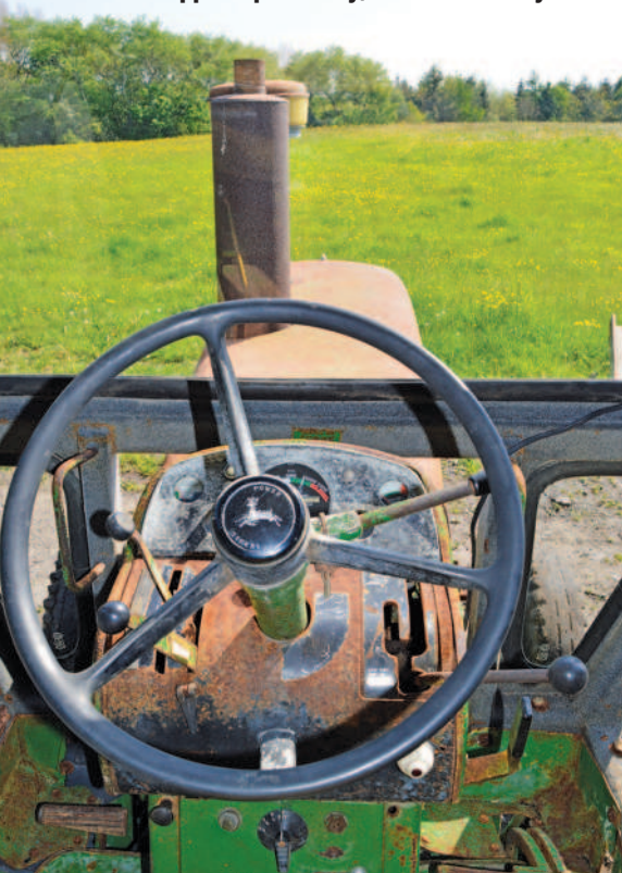
A driver's view from the cab of GKK 570D. Although the bonnet and instrument fascia appear quite rusty, the metal is very solid.
