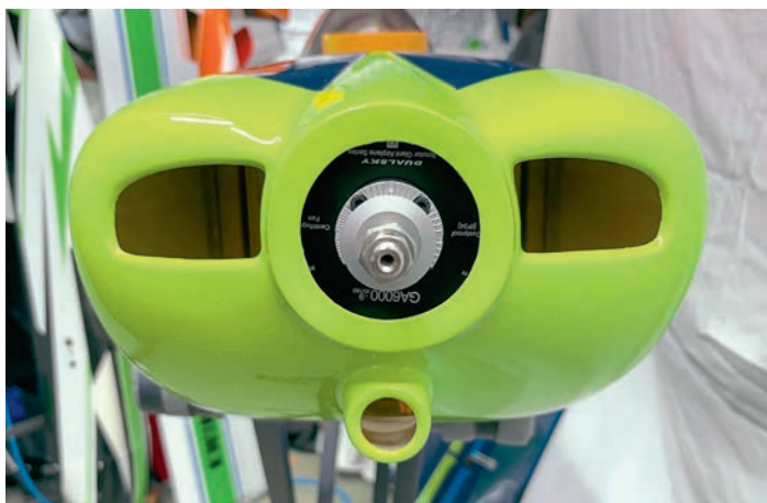
Offsetting the mounts keeps the motor neatly lined up with the front opening of the cowl, although a small amount of parallax suggests otherwise in this picture.
