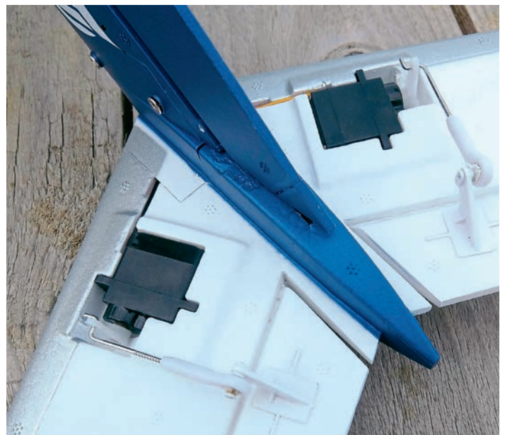
Elevator servos in detail. Take care to not trap any of the wires when nipping up the screws that hold the horizontal stab.
