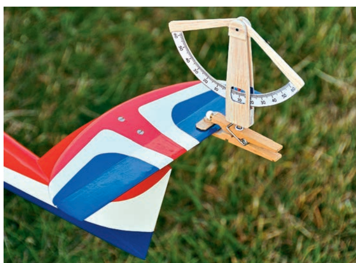
Now with up elevator, showing a deflection of 9^\circ up.
