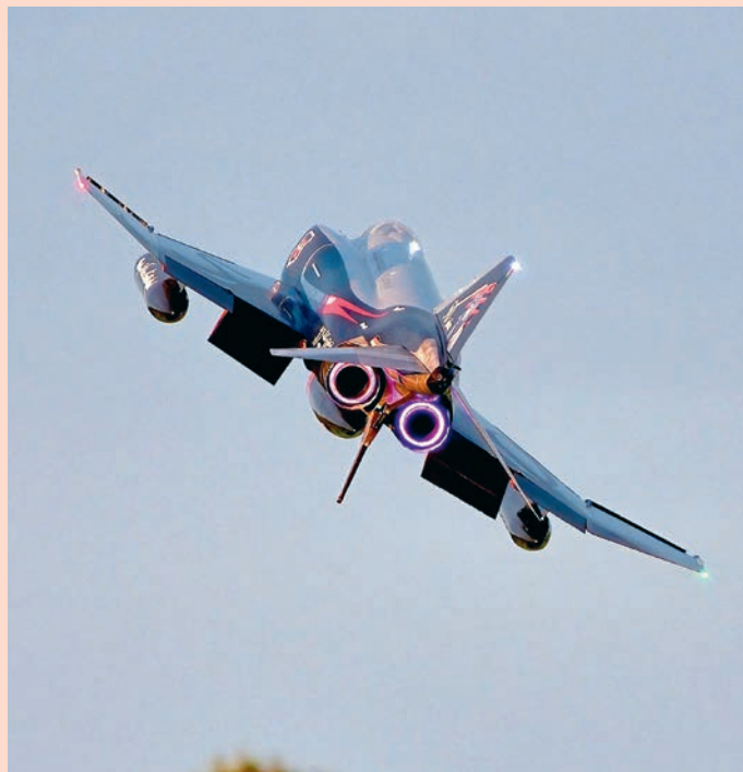
Max Chrubasik of CARF Models knows how to put on a display! Here is his 1:4.5 scale, 2.65 metre span F-4 Phantom in 'Red Baron' livery. The model houses two KingTech K-235 turbines, each supplied by its own 5.5 litre fuel tank.
