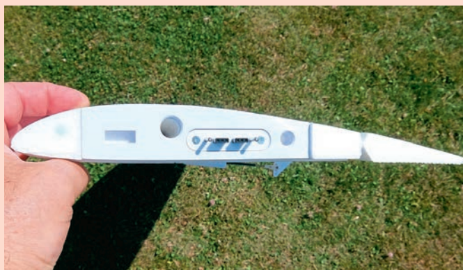
Wing root and wing seat in detail showing the plug-in servo connectors and metal latch at the front.
