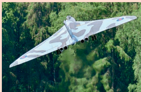
Steve Kilbon gives a scale perspective to his immense 1/6th scale Avro Vulcan bomber. All wood construction with a pair of Jet Italia Lion 220N turbines providing the thrust.
