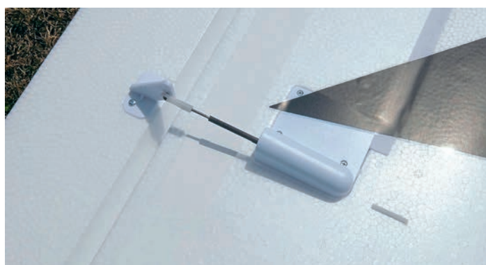
All wing servos are neatly covered by screw down covers.
