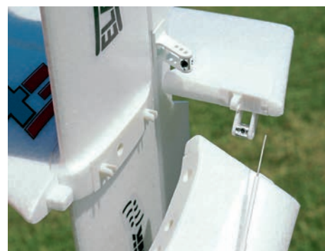
...although these grub screws aren't the best way of reconnecting control surfaces.
