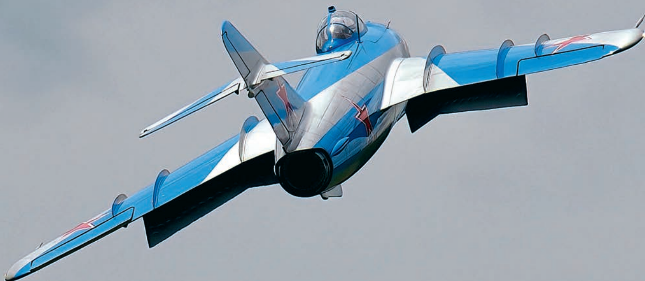
CARF Models MiG-17 climbing out after a dirty pass. 2.65 m span, 1:3.7 scale, typically powered by a 220 to 240N size turbine.
