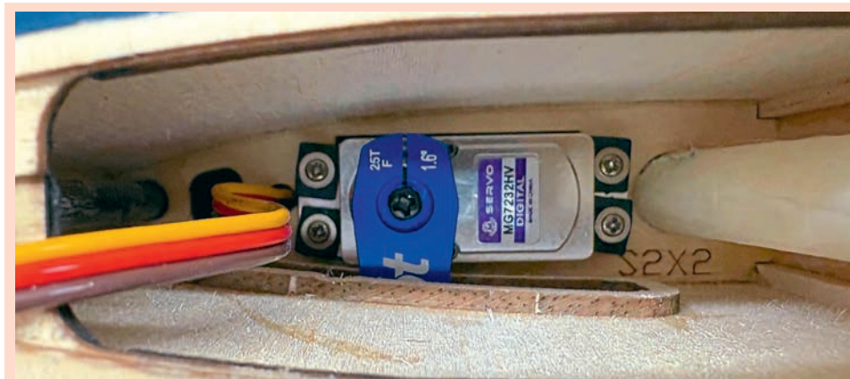
One of the elevator servos buried inside a tailplane half. It's easier to fit without a servo arm already in place.
