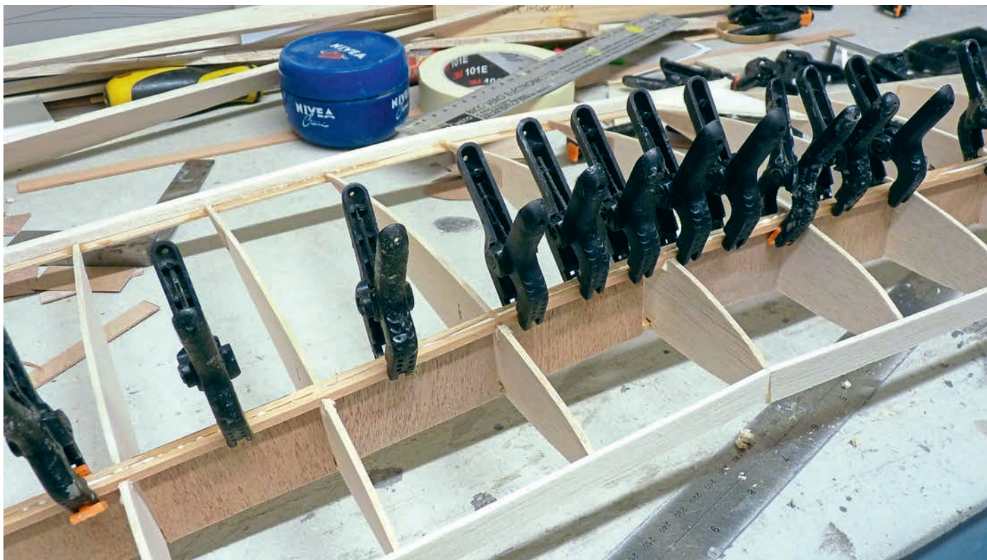
Adding the secondary sub spar.
