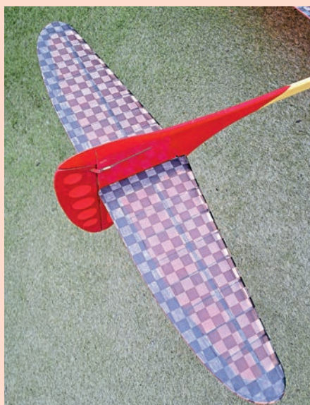
Finished Thermic 100 tail feathers look just-so, despite being laid over old tissue remnants already on the structure.
