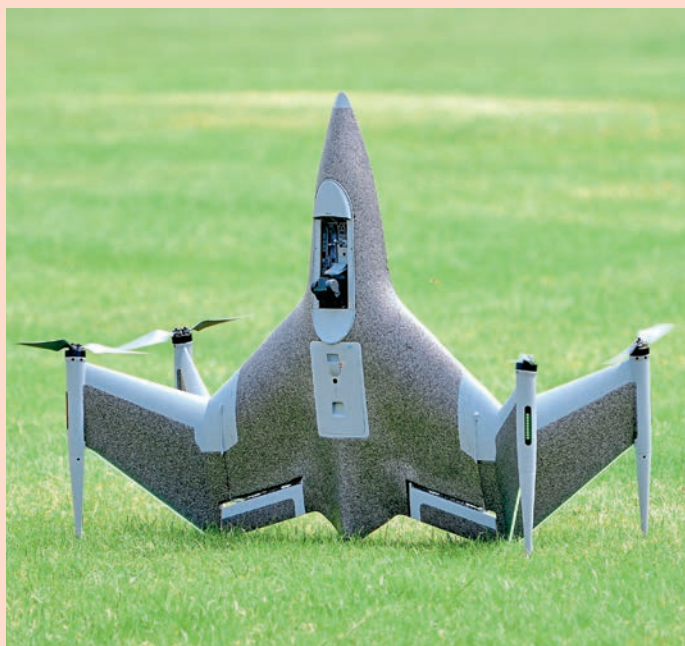
Fly Wing's X-Wing Fighter is an interesting concept. It takes off like a traditional drone...
