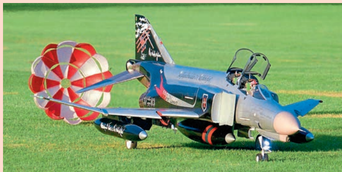
Max Chrubasik of CARF Models knows how to put on a display! Here is his 1:4.5 scale, 2.65 metre span F-4 Phantom in 'Red Baron' livery. The model houses two KingTech K-235 turbines, each supplied by its own 5.5 litre fuel tank.
