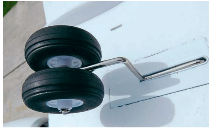
The undercarriage clips in and can be removed for belly landings in longer grass, as can the nose-leg. Power scale soaring, anyone?
