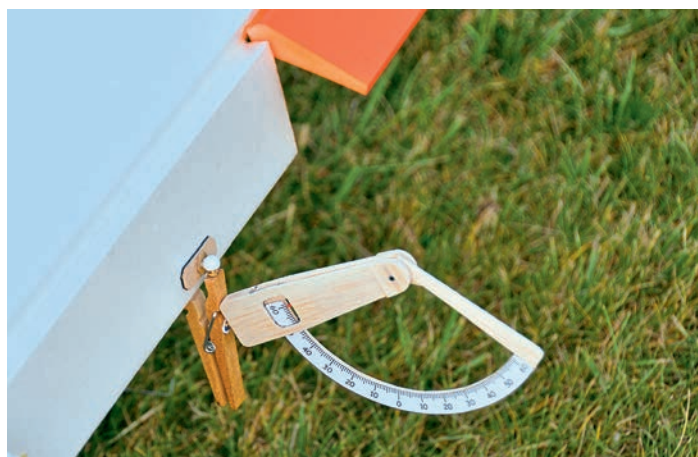
...the 60^\circ shown on the gauge at full down flap means the desired 70^\circ deflection has been achieved! ( 10^\circ + 60^\circ )
