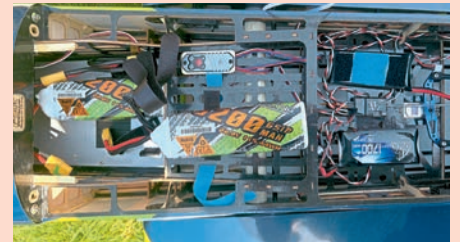
Moving the packs around to achieve the correct CG resulted in one 6S LiPo up front with the other strapped on the middle tray immediately behind. The two R/C packs now straddle the receiver at the rear.
