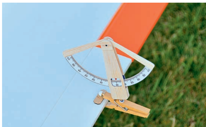
If angles of more than 60^\circ are required (for flaps, say) pre-load the Throw Gauge with the additional degrees required. My Bush Cub requires 70^\circ down flap deflection so I have pre-loaded the gauge with 10^\circ and...
