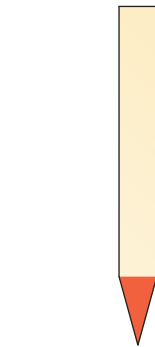
SPACER/POINTER FROM 3.2mm SHEET (PAINT POINT RED)
