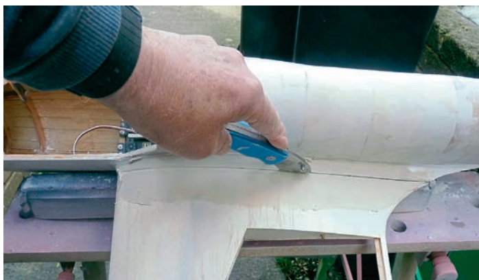
Separating the wings whilst the filler is at the 'cheesy' state.
