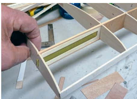
View of the brass joiner box in the wing.
