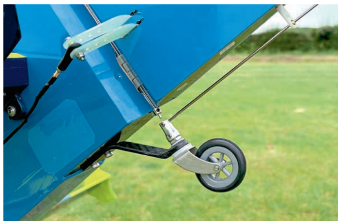
A few interesting details in this pic, including the full-length rudder pin secured with a collet and the neat steerable tailwheel. Note the use of a cut down ball-link to connect the rudder to the wheel-post via a piece of wire.
