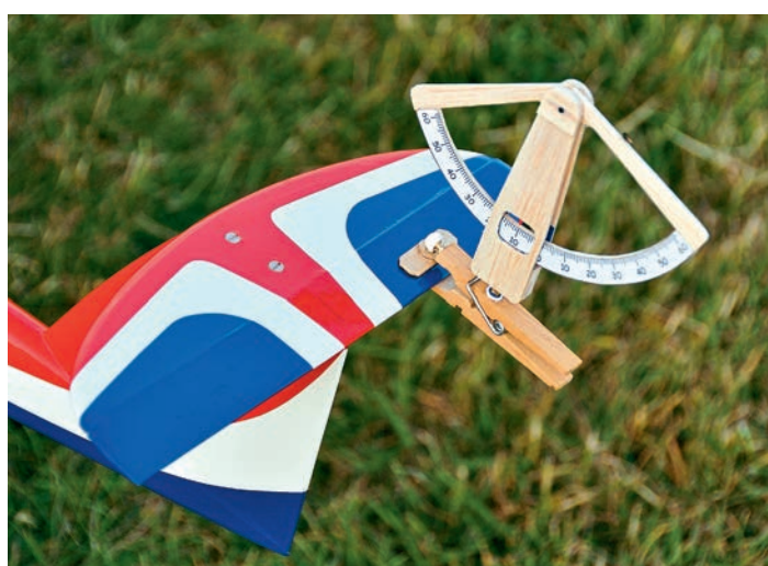
Here down elevator has been applied showing a deflection of 10^\circ down.
