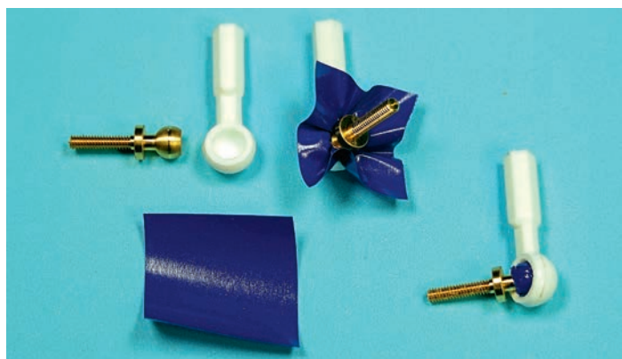
Friction of the ball and socket joint for the pendulum frame is increased by trapping a piece of covering in the joint and trimming away the excess.
