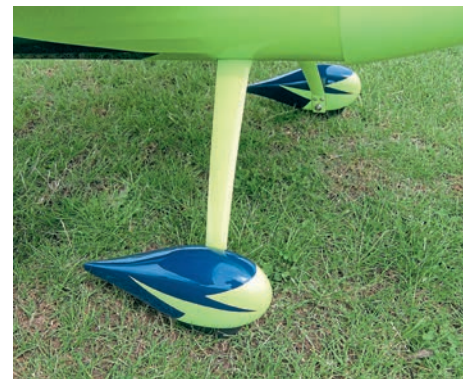
Wheels are enclosed in a pair of smart moulded spats.
