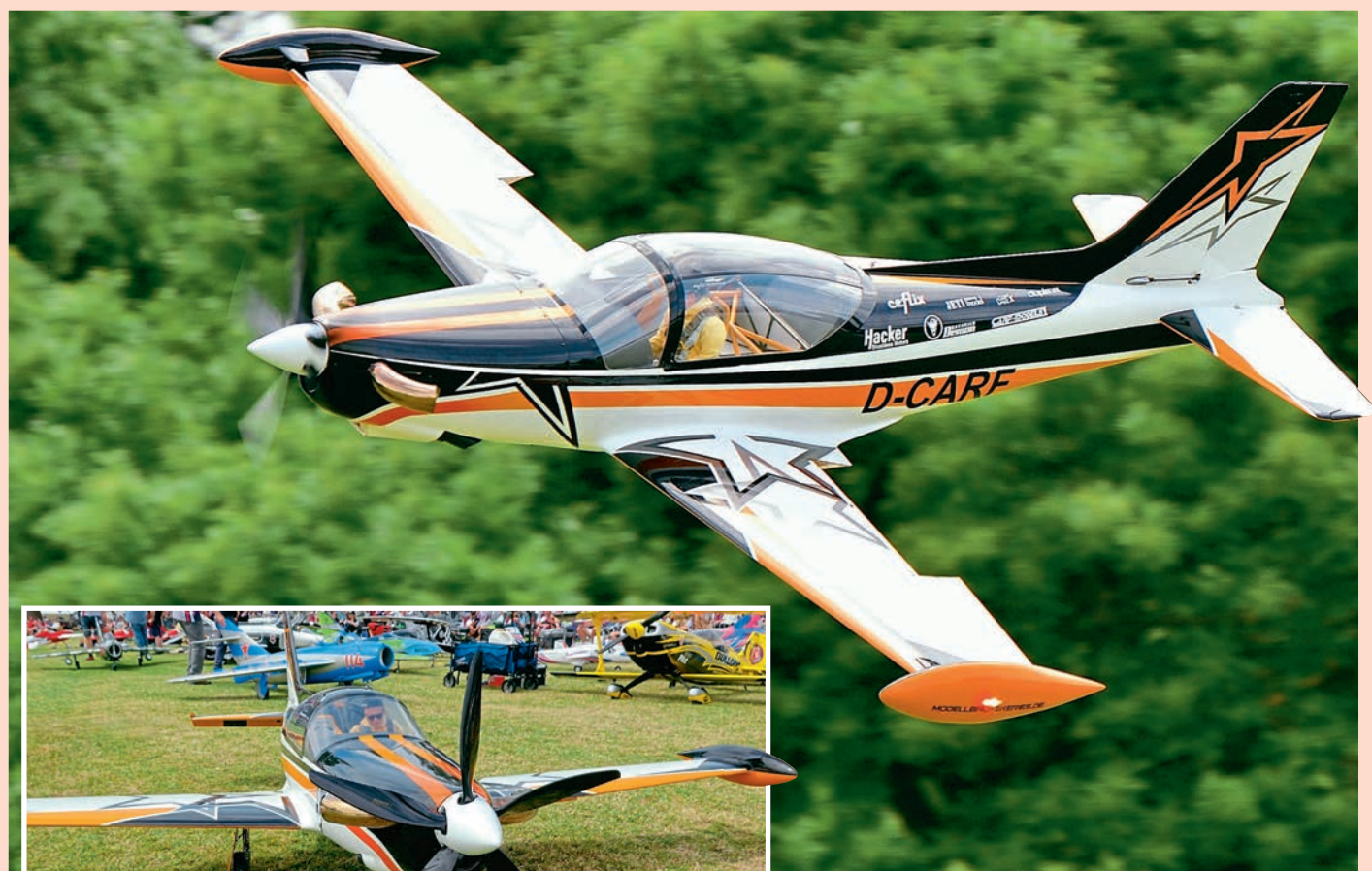
CARF Models also displayed their 2.83 m span, 1:2.9 scale SIAI Marchetti SF-260 powered by a JetCat SPT-5 Turboprop and a beautiful Falcon five-bladed carbon prop.
