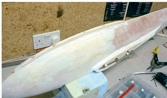
Adding hardwood dowel pieces to accept screws for the aileron servo horn.
