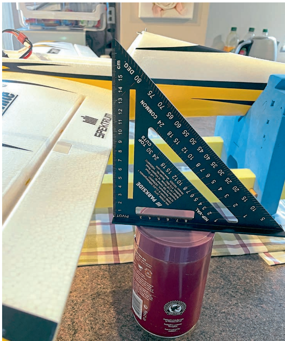
Hip-Val in use checking the aileron movements of the recently reviewed E-flite Sportix. Vertical measurements show up well whilst the T-beam base provides a flat support, raised to a suitable level on top of a can of coffee!
