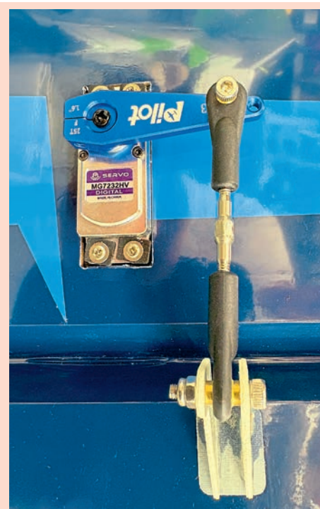
Chunky turnbuckle style pushrods are used to connect the ailerons and elevators to their servos. Short one on the wings and longer ones at the tail.
