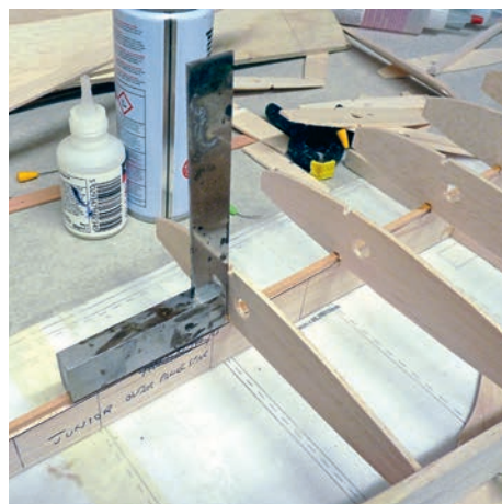
Ribs are set at 90 degrees to whichever part of the spar they are being attached to.
