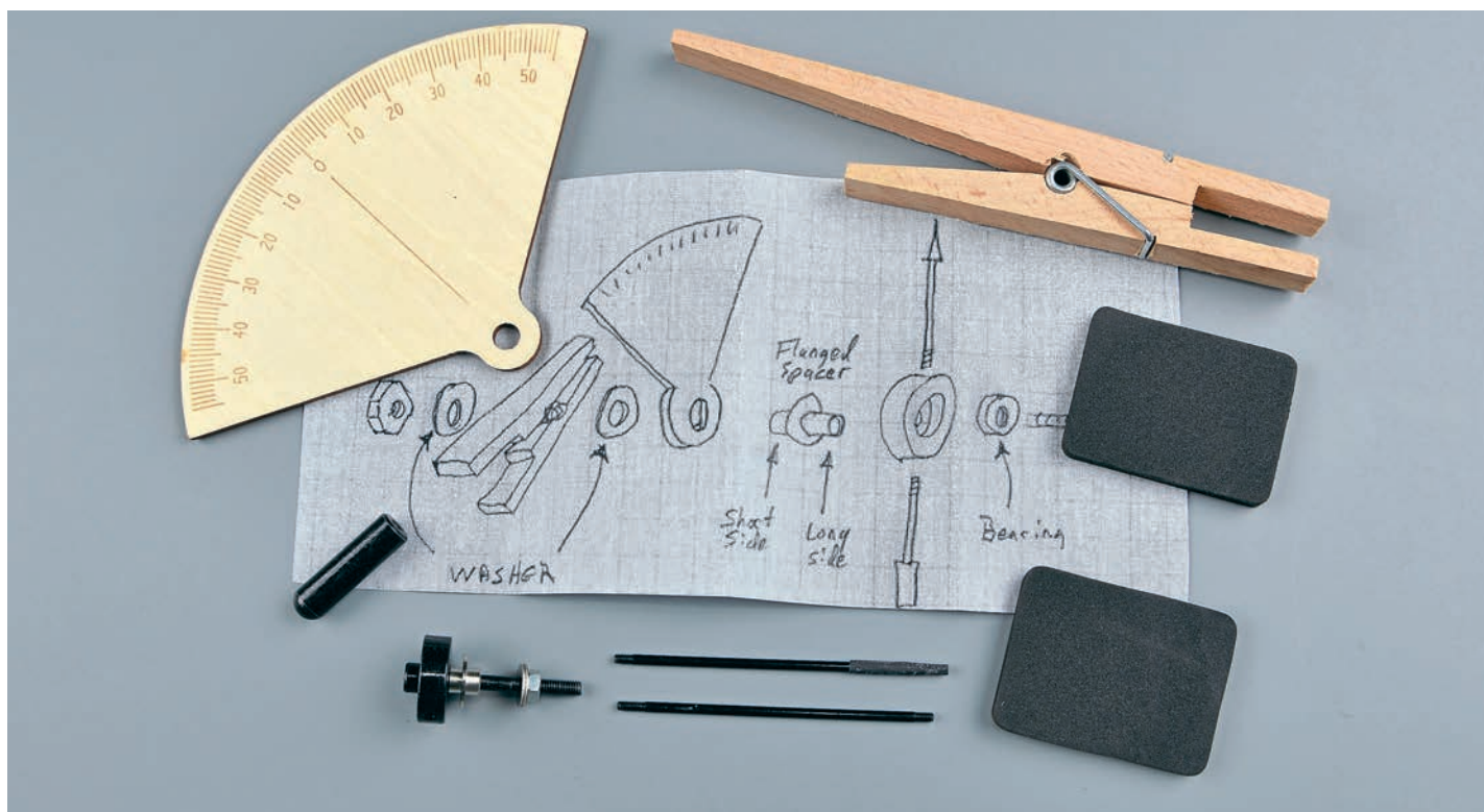
Build it yourself pendulum gauge purchased via eBay but similar in style to Mike Freeman's DIY version shown on page 18.
