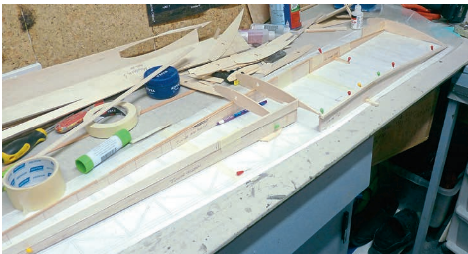
First stage of wing construction with the gull jigs.
