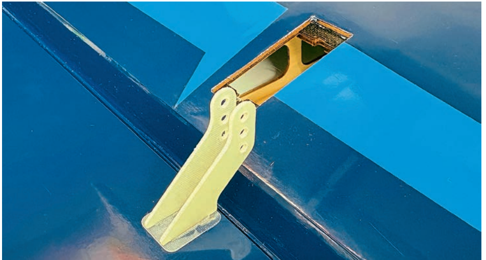
First order of business is to glue in the epoxy glass control horns, a pair on each surface. Don't forget to fit the flat plate before doing so, easily overlooked.
