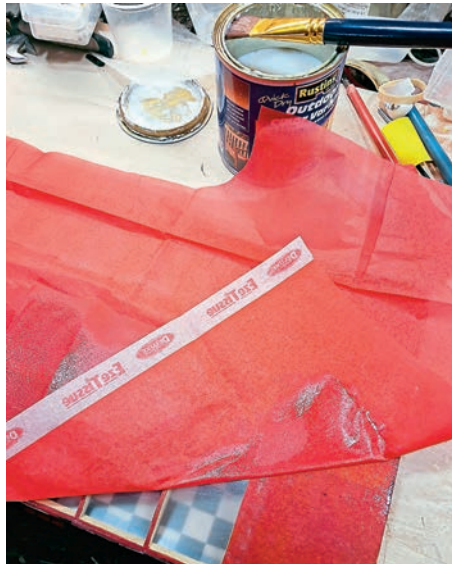
Acrylic doping the Eze-Tissue onto the Doculam covered Thermic wing. Very easy to do if you take things steadily.
