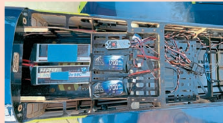
The original battery placements with two 6S 5000 LiPos on the forward tray and twin LiFe R/C packs on the middle tray behind. Far too nose heavy!
