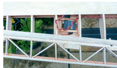
View of an aileron servo and linkage.
