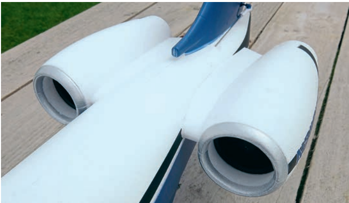
Twin 40 mm, 12-bladed fan units are hidden in the nacelles, powered by two 1413-5000kV motors. The 20A ESCs can provide reverse thrust, with the set up fully explained in the comprehensive manual.
