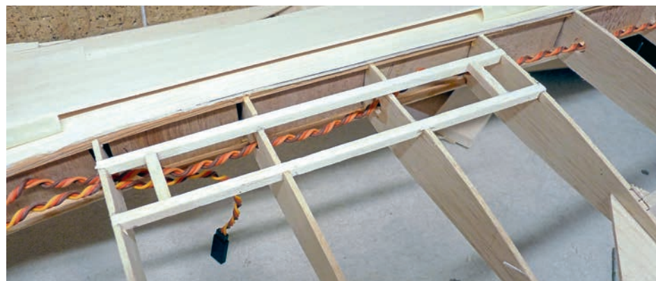
Dropping in the support spars for the spoiler.
