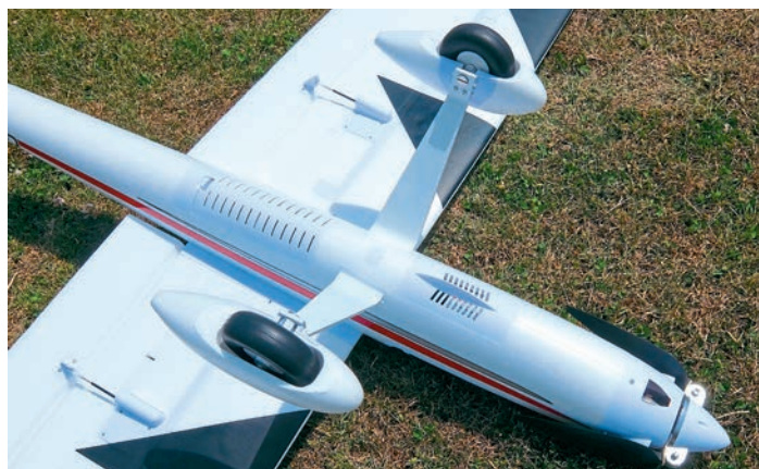
Undercarriage legs and wheels take just a few seconds to fit.
