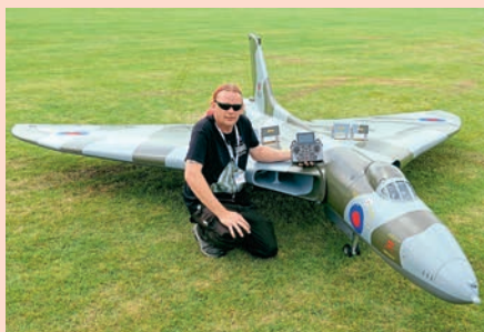
Steve Kilbon gives a scale perspective to his immense 1/6th scale Avro Vulcan bomber. All wood construction with a pair of Jet Italia Lion 220N turbines providing the thrust.
