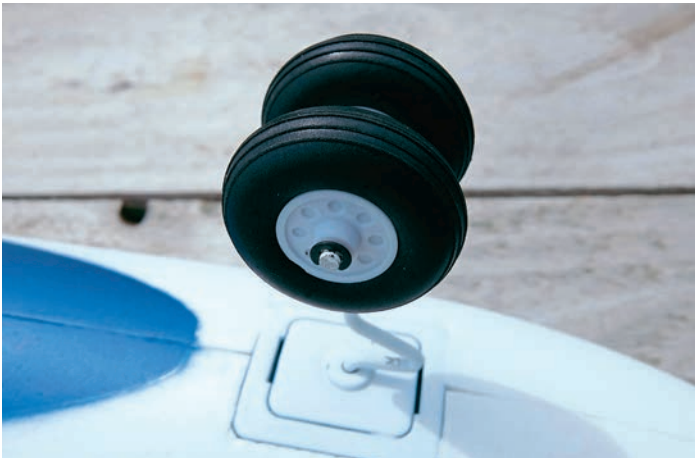
Twin wheel steerable nose-leg is connected to the rudder servo.
