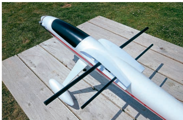
Wing panels are supported on a pair of sturdy joiner tubes.
