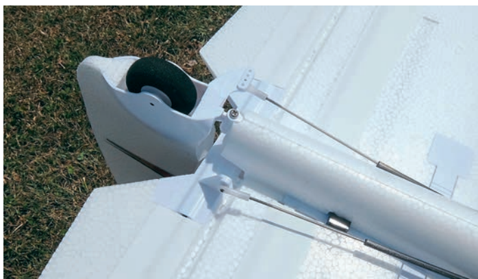
Close up on the narrow gauge pushrods and small ball-links at the rear. We will glue the rods and links together once flight testing is finished to prevent them from pulling apart. Note the connector for the optional LED night light set.
