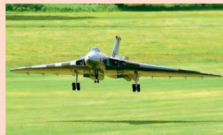
Steve Kilbon gives a scale perspective to his immense 1/6th scale Avro Vulcan bomber. All wood construction with a pair of Jet Italia Lion 220N turbines providing the thrust.
