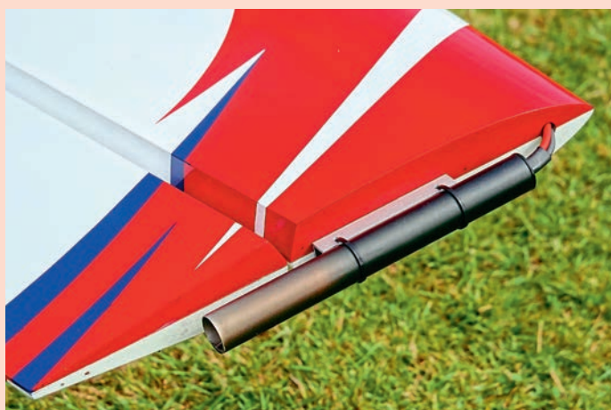
Gunter Zielke's CARF Extra 330LX is powered by a Hacker Q100/8 electric motor, 30 x 12 prop and a 14S 7000 mAh LiPo pack. As such it has no exhaust to generate smoke, so Gunter invented his own smoke system called 'Smoke-EL' which uses standard smoke oil and switchable heater tubes on the wingtips, running off the flight battery, to generate smoke.
