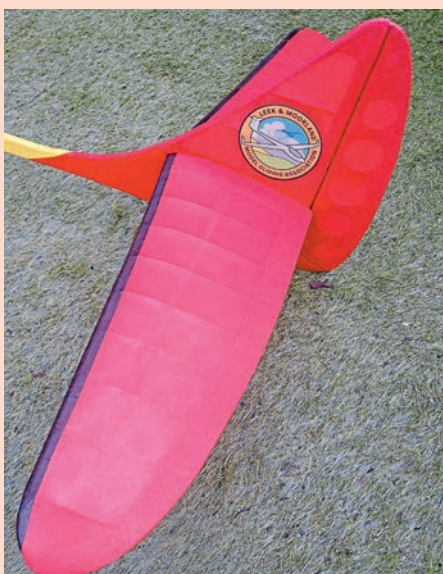
Finished Thermic 100 tail feathers look just-so, despite being laid over old tissue remnants already on the structure.
