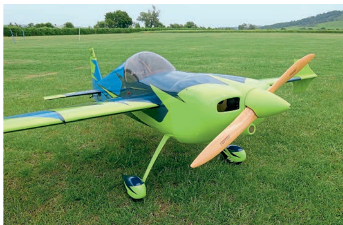
Just to underline the point, note how well the spinner is aligned with the cowl in this shot.
