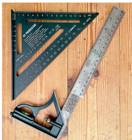
Hip-Val square next to my father's well-used combination square. Although the original measurements are indistinct, they show up well on the modern 'see through' plastic ruler.
