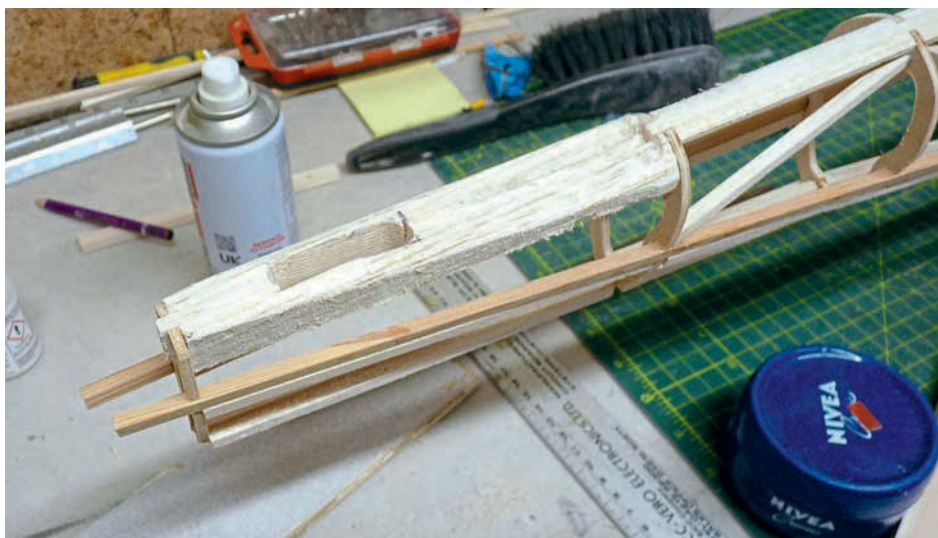
Finalising the tailplane mount before sheeting.
