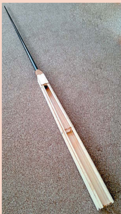
The fuselage is a simple balsa pod with a tapering carbon fibre tail boom. A tapering balsa sandwich gives a neat finish to the boom/fuselage joint.
