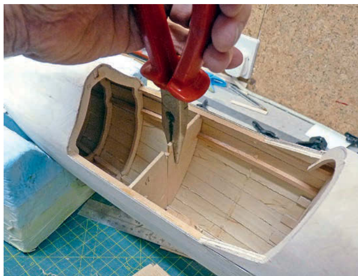
It's time to remove the temporary formers before glassing the interior.
