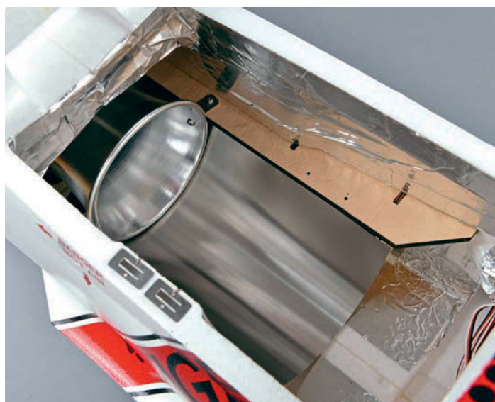
Turbine mount is surrounded by lots of heat reflective material. Note the bell-mouth entry to the jet pipe.
