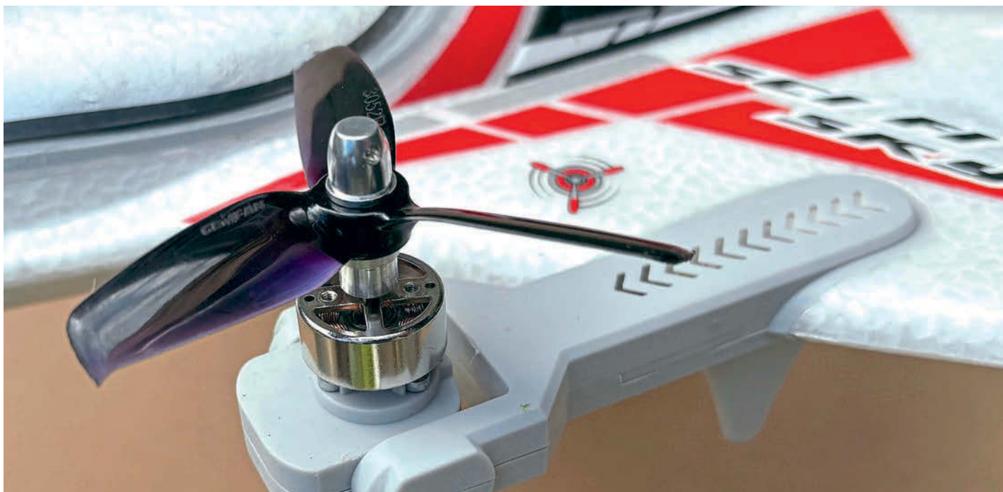
Three-blade prop and hidden motor tilt system.
