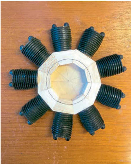
Jeff also made a complete 9-cylinder dummy radial for his SBD Dauntless using the same moulding kit.
