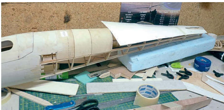
Rear turtle decking is formed from separate sheets to accommodate the compound curve.
