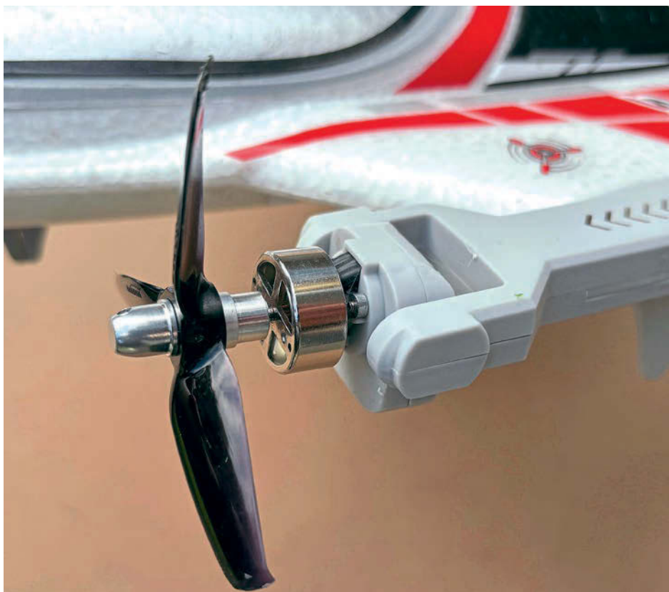
Vertical hovering position, which is also used in aircraft mode.
