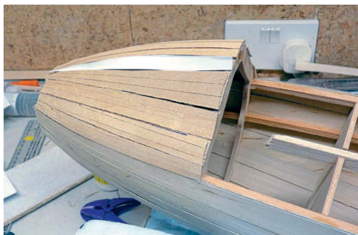
Finalising the planking at the front.
