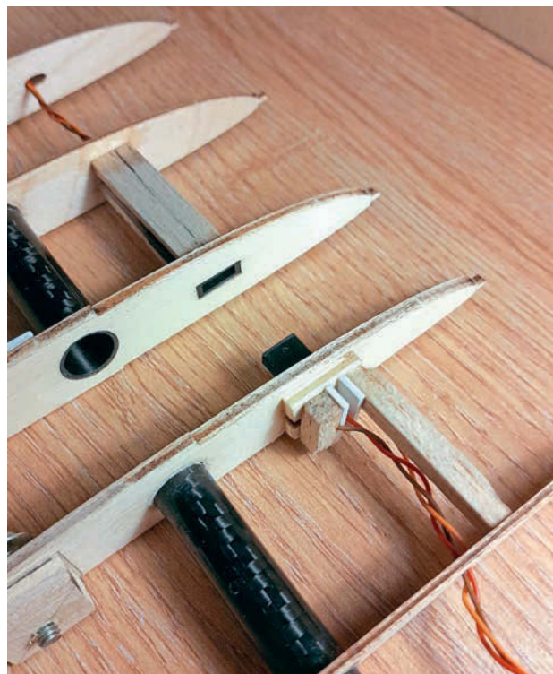
Servo wire connections between wing sections were made by crimping standard connectors and gluing them into the end ribs, having programmed the exact cut-out sizes in devWing.
