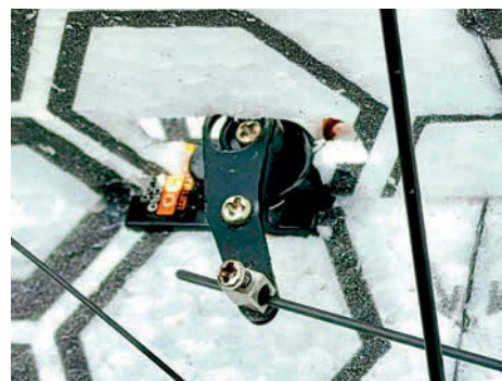
John also fitted the aileron servo earlier than shown in the instructions.
