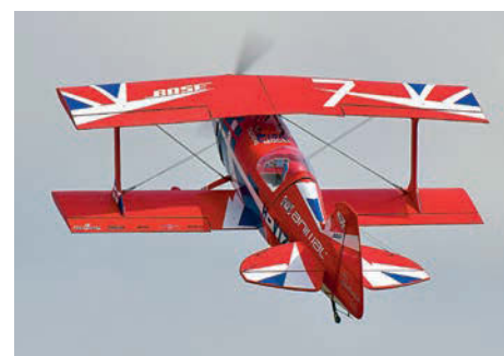
Keith Barnes' Skip Models Pitts Challenger climbs out powered by a DLE 120 cc twin engine plus 28 x 10 Falcon prop.
