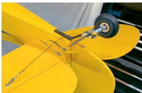
Tailwheel assembly with its scale leaf-spring is a nice piece of engineering.
