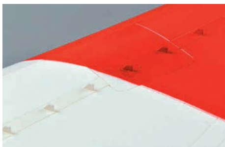
Upper wing surfaces are lined with a row of small turbulators. Whilst not unusual on foam ARTF models these are in fact scale details from the full-size.
