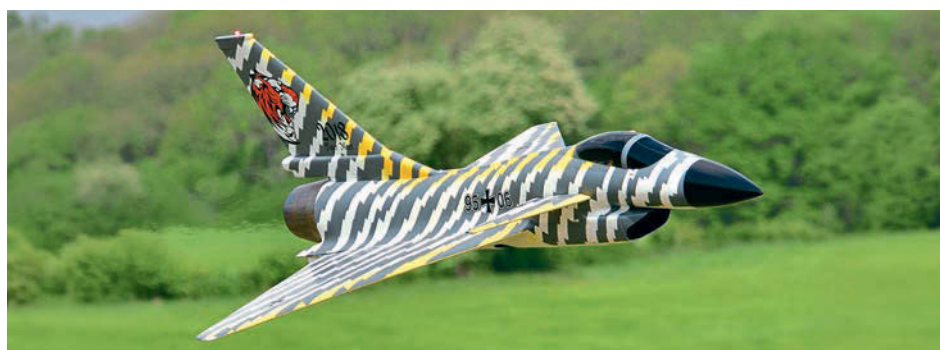
Neil Garnett's CARF J-10 looked fabulous on a high-speed beat along the strip. Powered by a Jets Munt M222NG turbine the 1.5 m span and 2.6 m long model has a flying weight of 15 kg, 5 kg of which is fuel.
