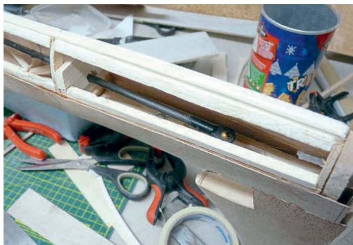
Underside view of the elevator pushrod with its ball-link connector.
