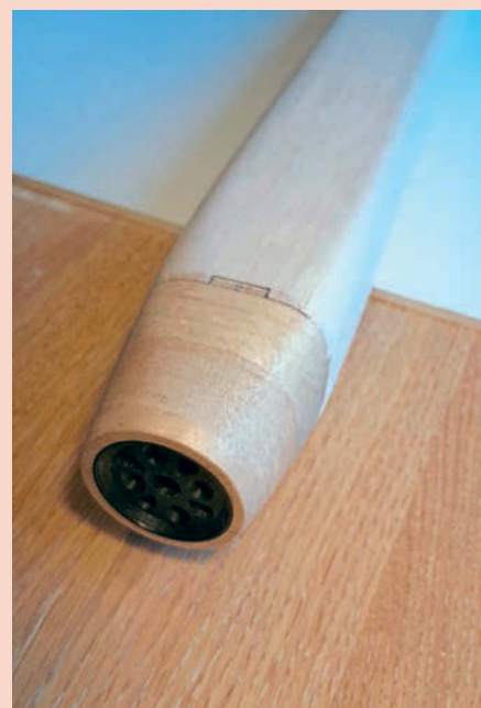
The fuselage is a simple balsa pod with a tapering carbon fibre tail boom. A tapering balsa sandwich gives a neat finish to the boom/fuselage joint.
