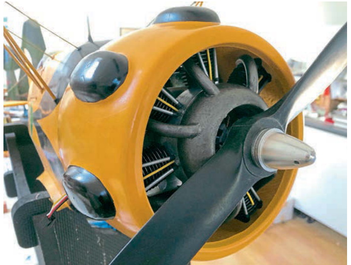
With the Jungmeister's cowl fitted the dummy radial really looks the part.
