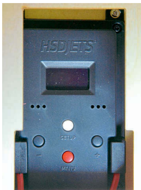
Easy access is provided to the buttons of the multi-function flight controller. I will be using a Futaba S-Bus receiver so setting up is almost 'Plug N Play'.
