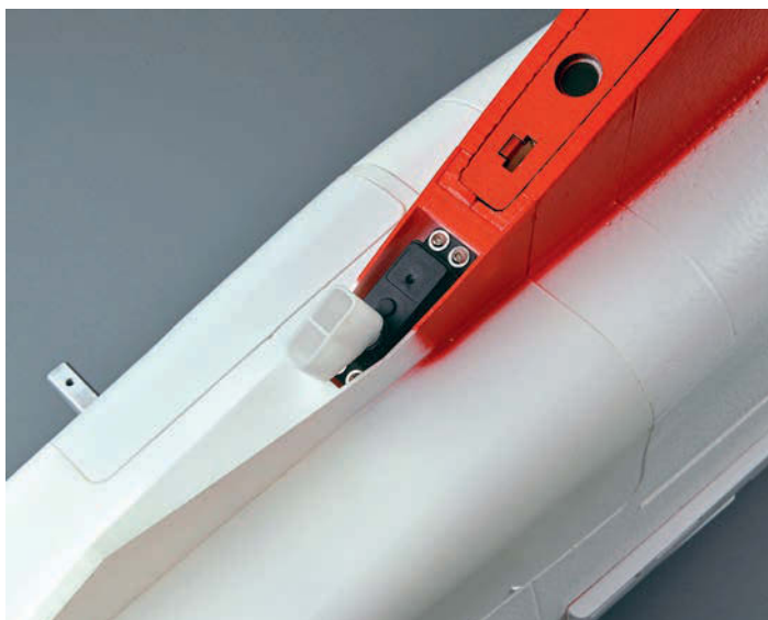
Rudder servo is fitted with an unusually shaped oblong control horn that slots into the fin assembly.
