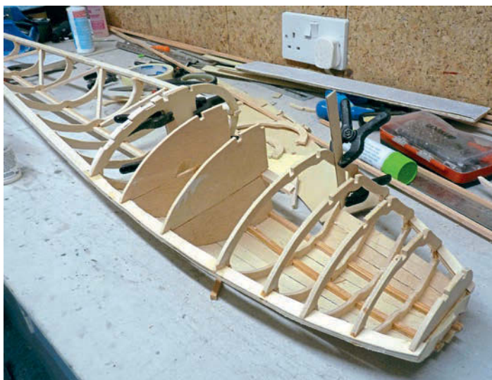
Adding formers to the other side of the fuselage.
