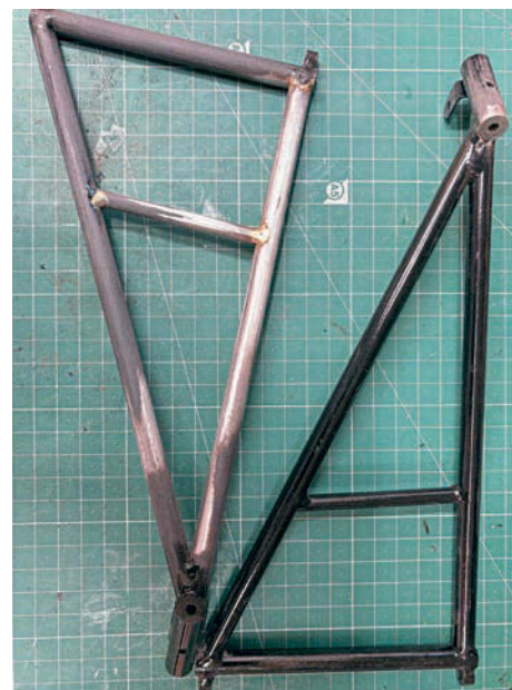
Tubular undercarriage parts are sprayed gloss black. Unfortunately, one set had gone rusty whilst in its unforeseen period of storage so needed a respray.
