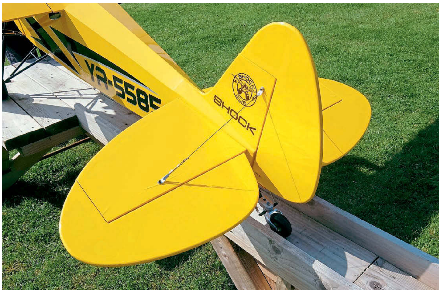
Tailplane rigging wires are structural so should not be left off.
