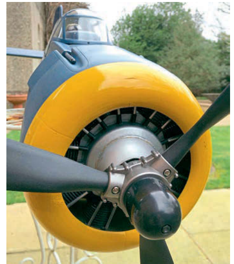
With the radial fully cowled and fitted with a dummy variable pitch 3-bladed prop, Jeff's Dauntless nears completion.
