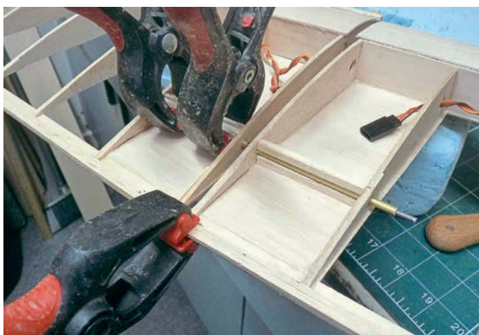
Lining up the outer wing panel accurately.
