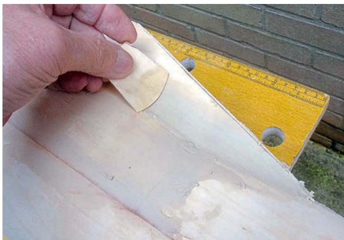
Smoothing the fuselage/pylon junction with a custom ply spreader.
