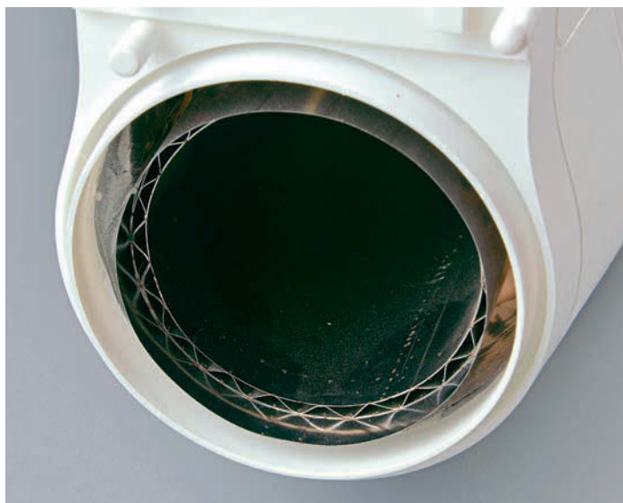
Jet pipe detail. Note the corrugations and the surrounding foil, all designed to help shield the foam from the turbine's hot gasses.
