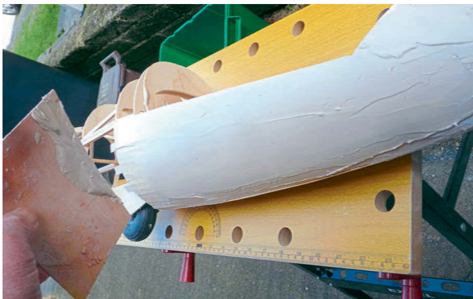
The 1/32" ply conforms well to the shape of the fuselage.
