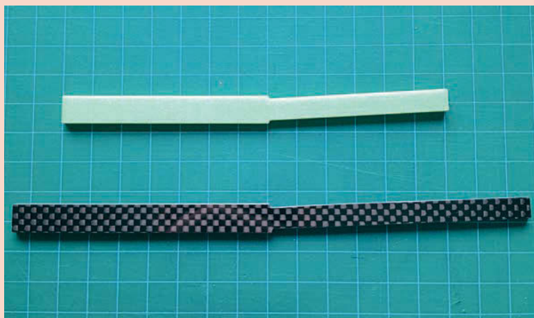
Once cut the carbon joiners were sandwiched between hard balsa to fit snugly inside the carbon wing tubes.
