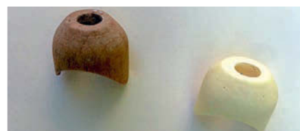
P-51 machine gun blister original made from wood alongside a resin copy.
