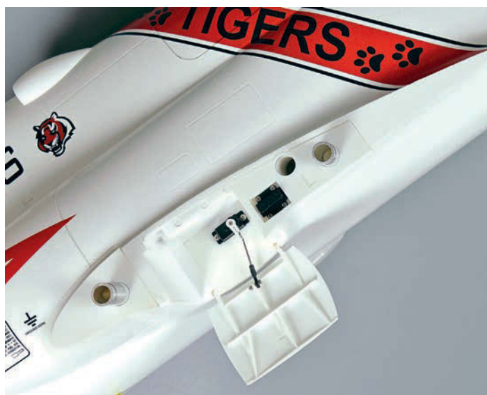
Fuselage wing root showing a sequenced gear door and servo.
