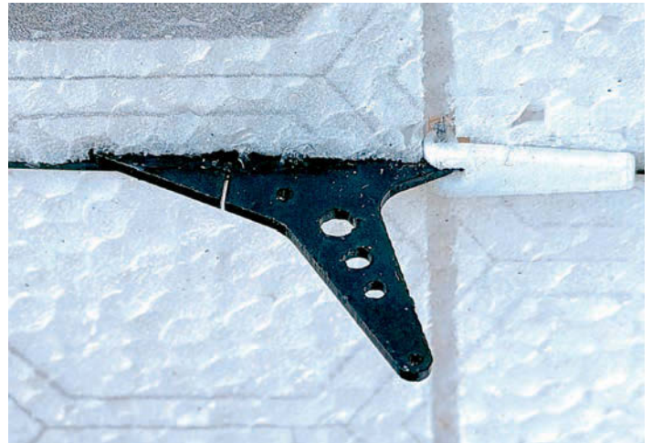
Closed loop control horn and hinge. The horn is quite large.
