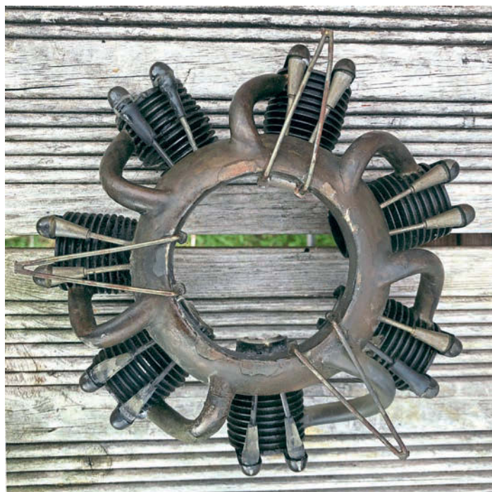
Front view of the dummy radial after the missing cylinders were fitted.
