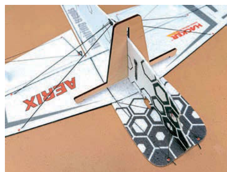
Wings, lower fuselage and tailplane are the first elements to be built. The ply jig helps when fitting all the CF rod bracing.
