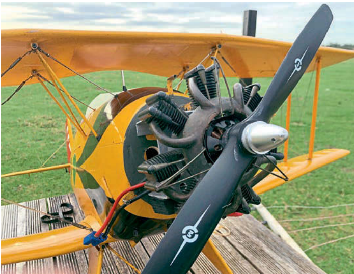
Siemens Radial test fitted to Jeff's Jungmeister.
