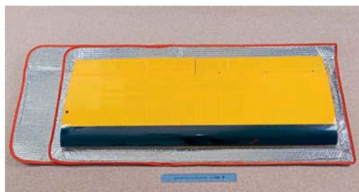
Protective padded wing bags are included in the kit. The struts can be folded against the undersides and fit easily alongside each wing panel.
