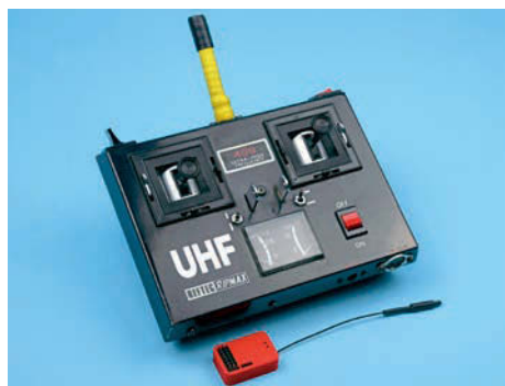
My 'new' old Reftec set is now working reliably with Tobe's modern UHFRF module, receiver and a Phil Green encoder.
