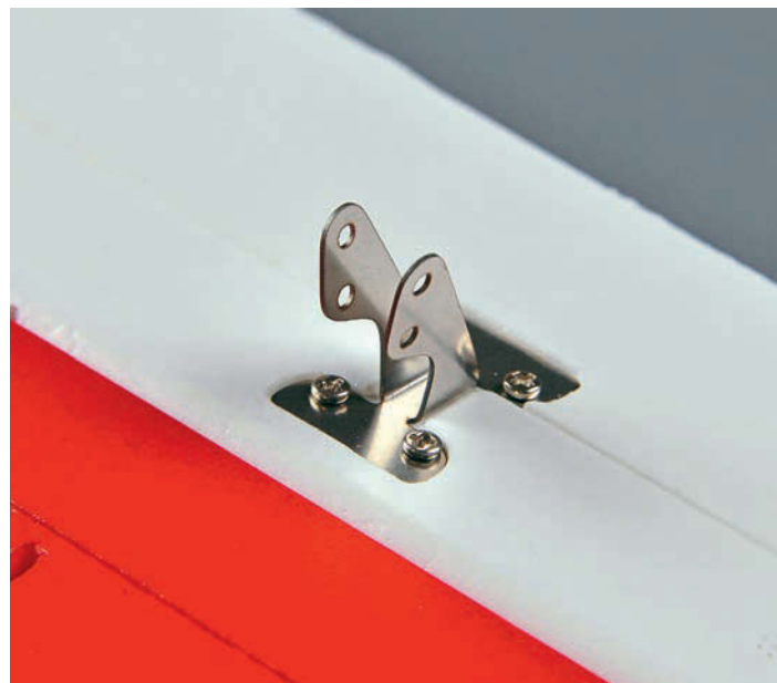
Ailerons have the security of folded metal horns, with the arms extending on each side of the pushrod's ball-link.
