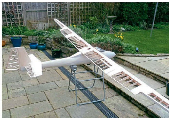
Getting towards the finish, the Skylark airframe awaits its ailerons.
