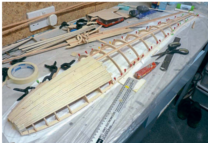
Once enough of the front planking has been added, plus the balsa diagonals at the rear, the half-shell can be removed from the board.
