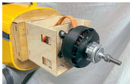
Shock Cub can be powered by a 35 to 55 cc glow or petrol engine, but we opted for 12S electric power using the additional motor box supplied to fit a Dualsky GA4000.7 motor.
