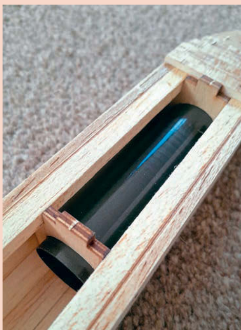
The fuselage is a simple balsa pod with a tapering carbon fibre tail boom. A tapering balsa sandwich gives a neat finish to the boom/fuselage joint.
