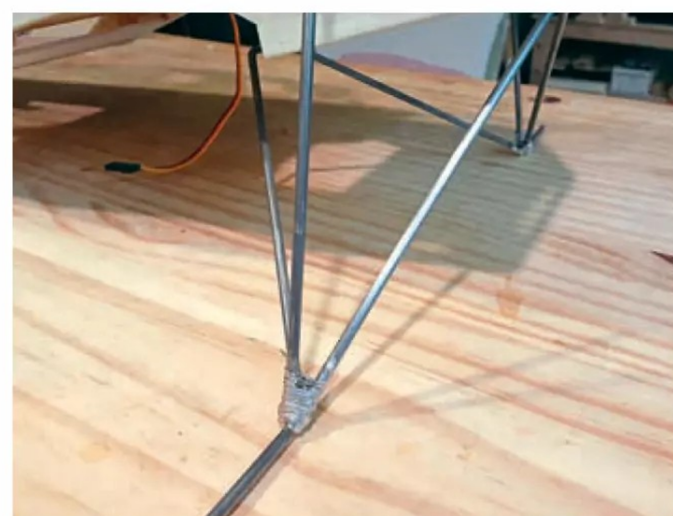
Undercarriage leg joints are bound with copper wire and soldered.
