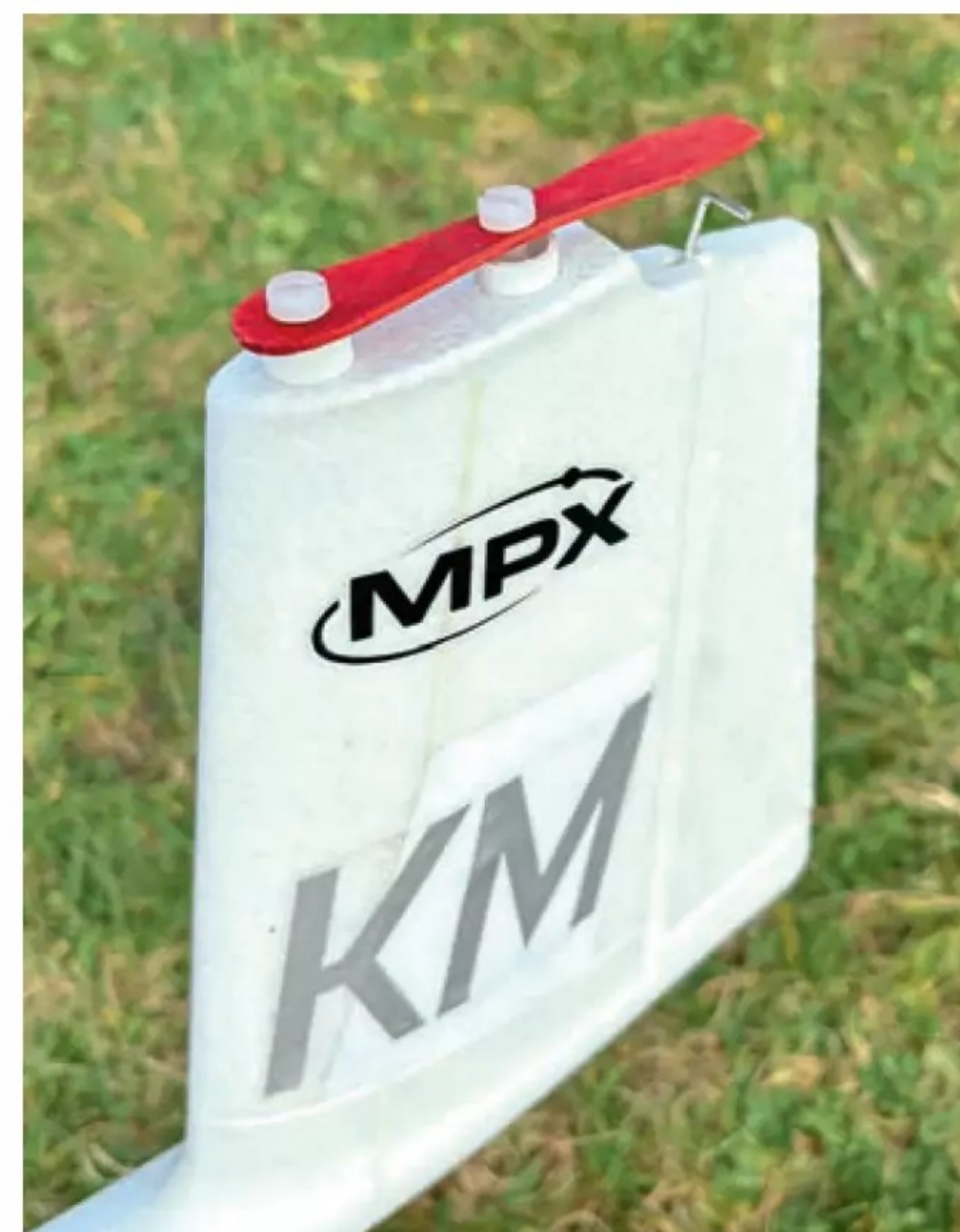
Eric's Heron/Lentus tail screwdriver retention system.
