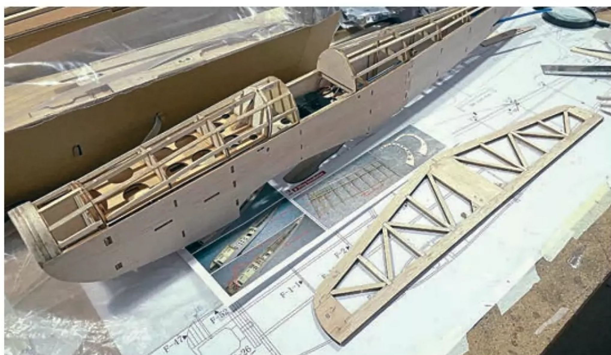
Chris swapped out the 2 mm square balsa stringers for 5 mm Paulownia alternatives. Still light but much stronger!
