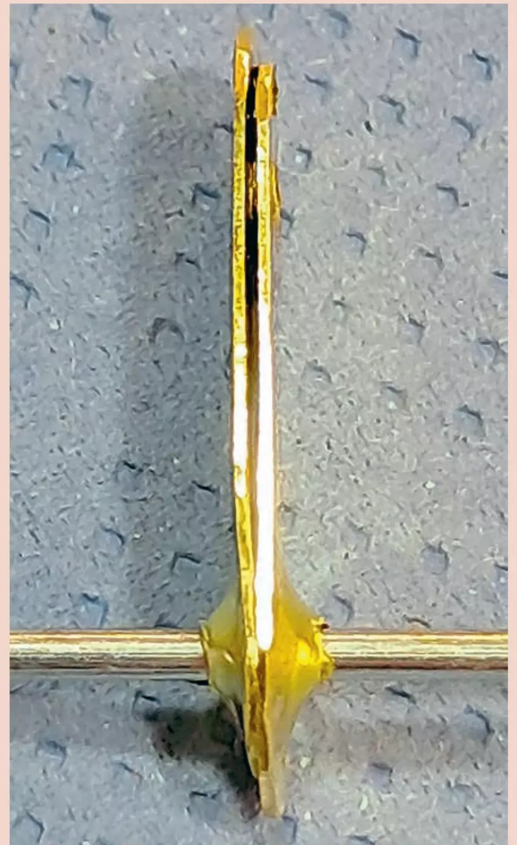
Doubled dimpled horns show how the simple modification of a flat plate gives much more soldering area/volume.
