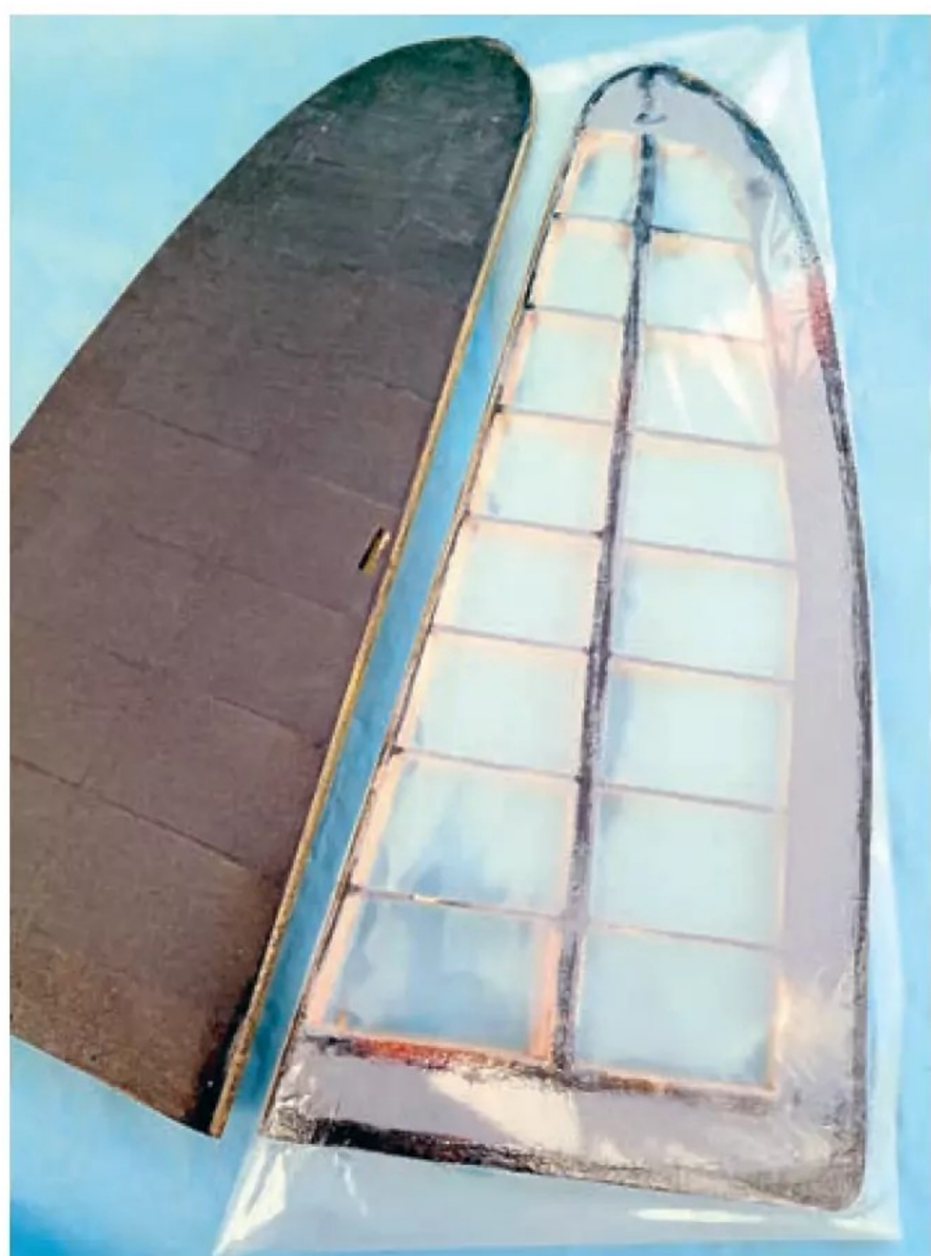
Thermic 100 tailplane halves. Original tissue covering on the left with replacement Doculam being prepared on the right.
