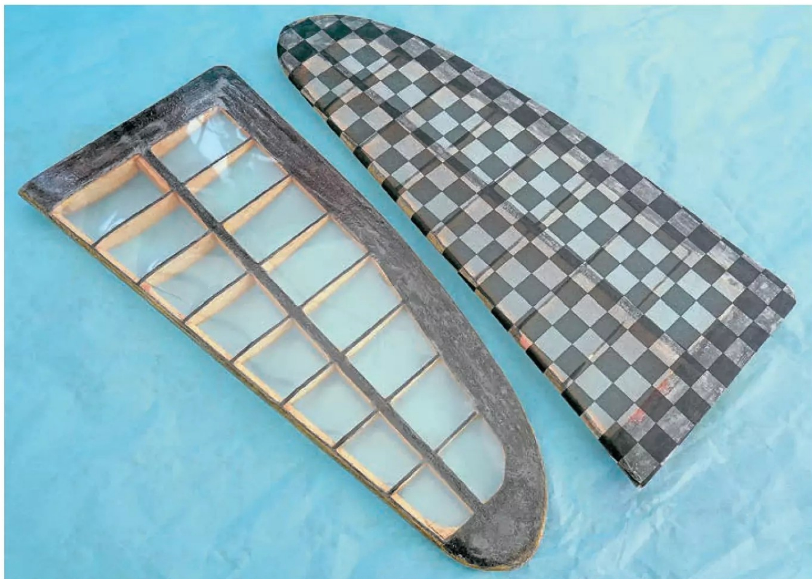
Finishing the Thermic 100 tailplane halves. Left shows the initial Doculam covering, whilst right shows the doped-on Eze-Tissue chequer disguising the old tissue remnants.
