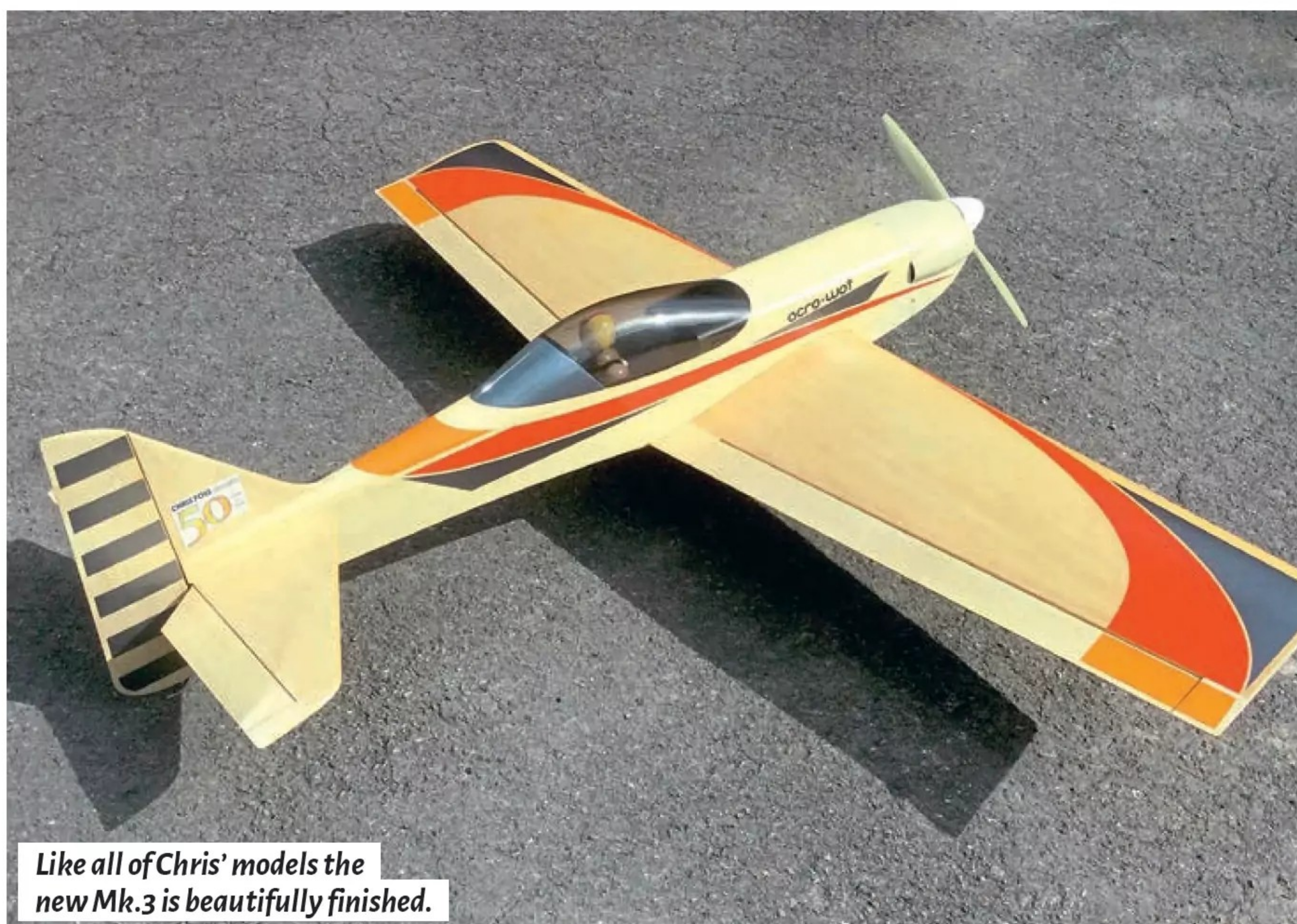
Note the flush cowl. The trim scheme is painted. All Acro Wot Mk.3 pictures are courtesy of Chris Foss.
