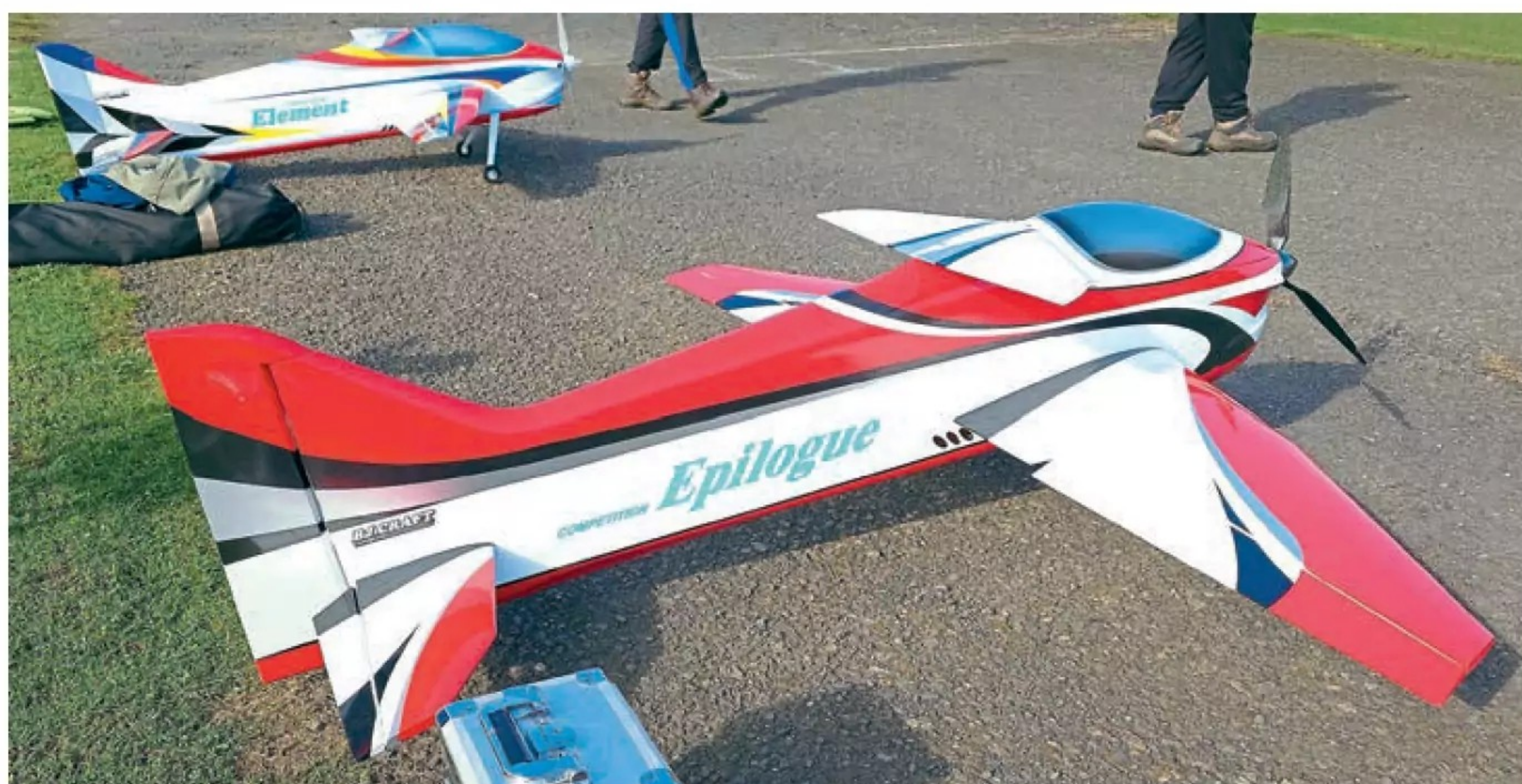
BJ Craft Epilogue belonging to Tom Laird. This lovely model continues to be very popular in F3A circles. Mono-prop drive using a Hacker Q80, D3 ESC and RS 3-2-3 three blade propeller.
