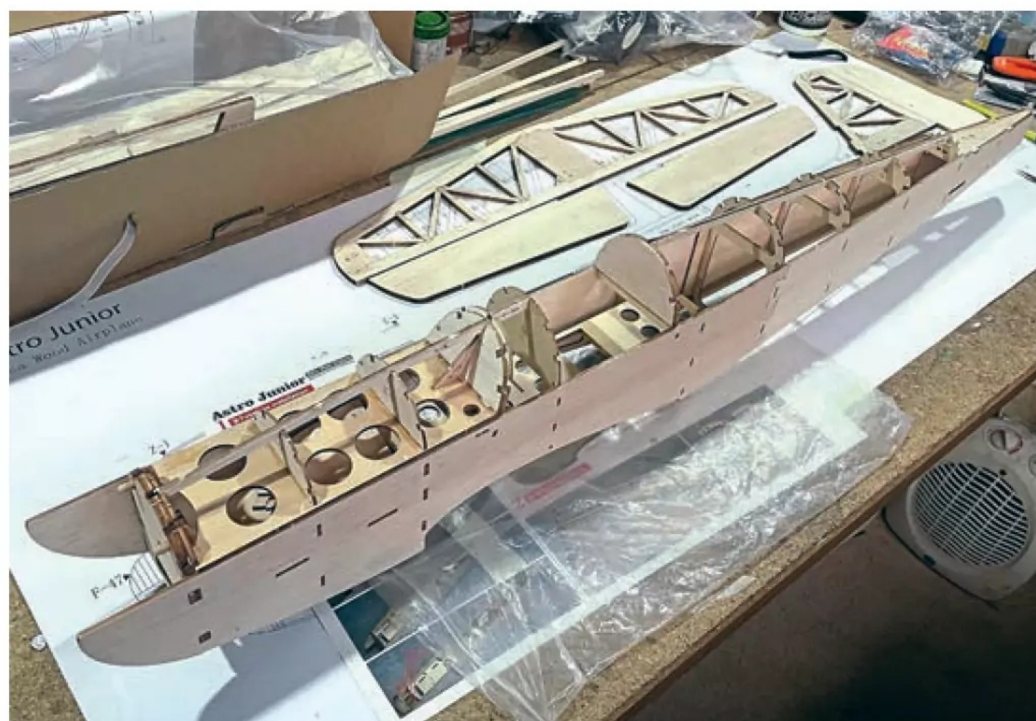
Fuselage boxed together and ready for the stringers.
