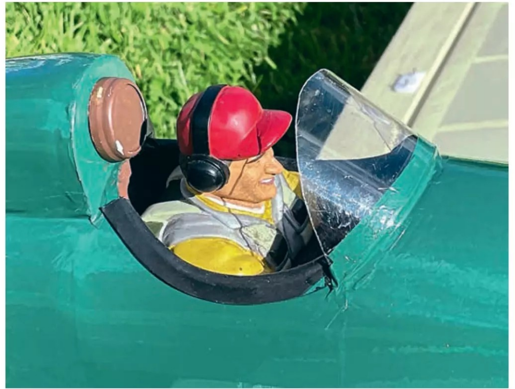
Chris sourced a pilot with a toothy grin and made a windscreen from a plastic bottle.
