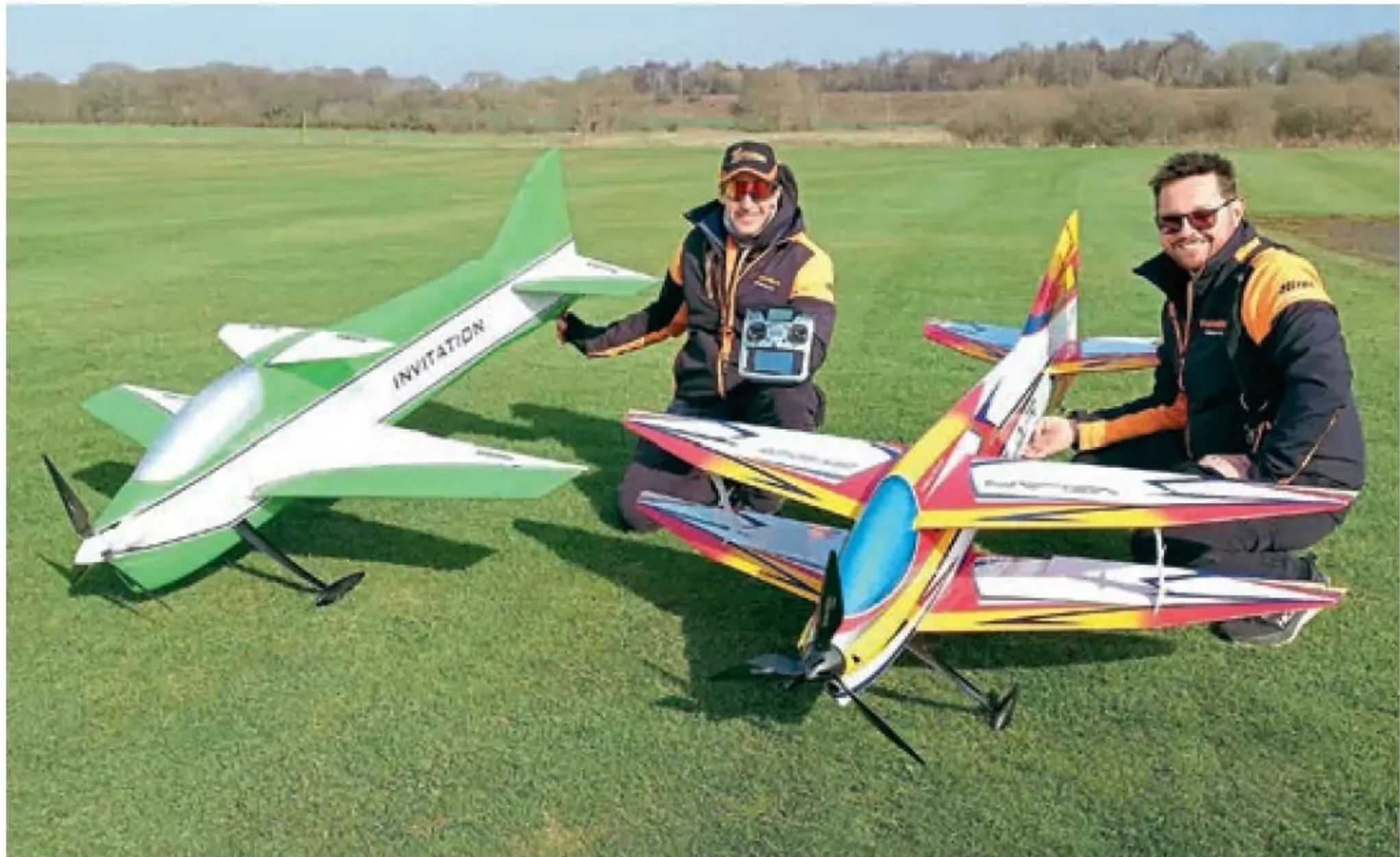
Dan Gallo with his BJ Craft Invitation in characteristic green! Propulsion by the ever-popular Hacker Q80 single drive motor. On the right, UK team pilot Malcolm Balfour with his Velar biplane. Plettenburg Advance single drive with RS3-2-3 three blade propeller.
