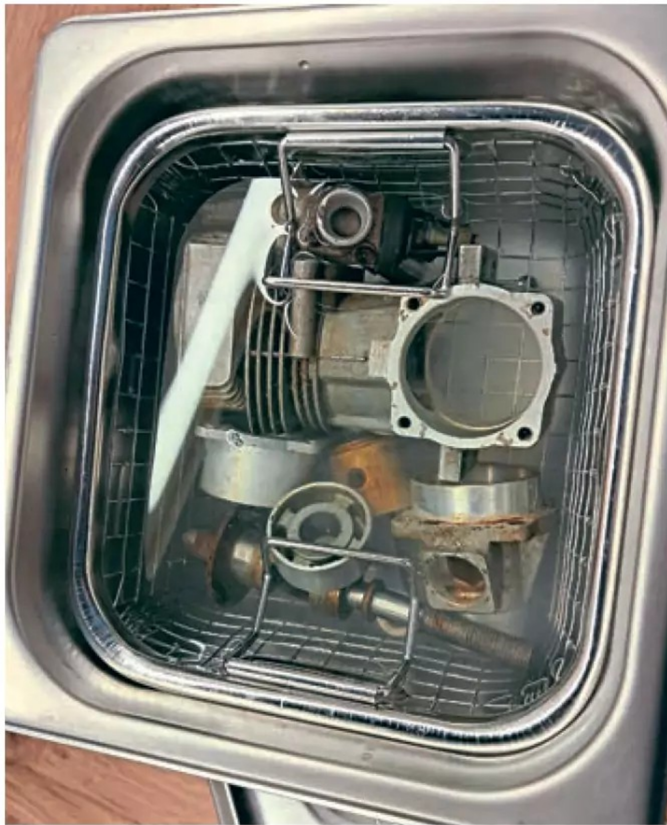
My ancient Super Tigre .61 gets the ultrasonic treatment. It shifted most of the grot but will need application of non-caustic oven cleaner to finish the job.
