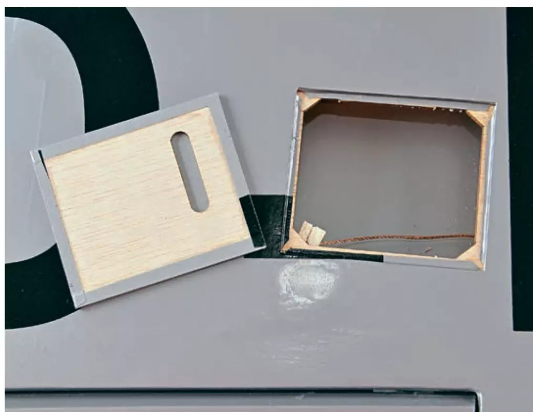
Aileron servos need to be mounted to the servo hatches before screwing them into position under each lower wing.
