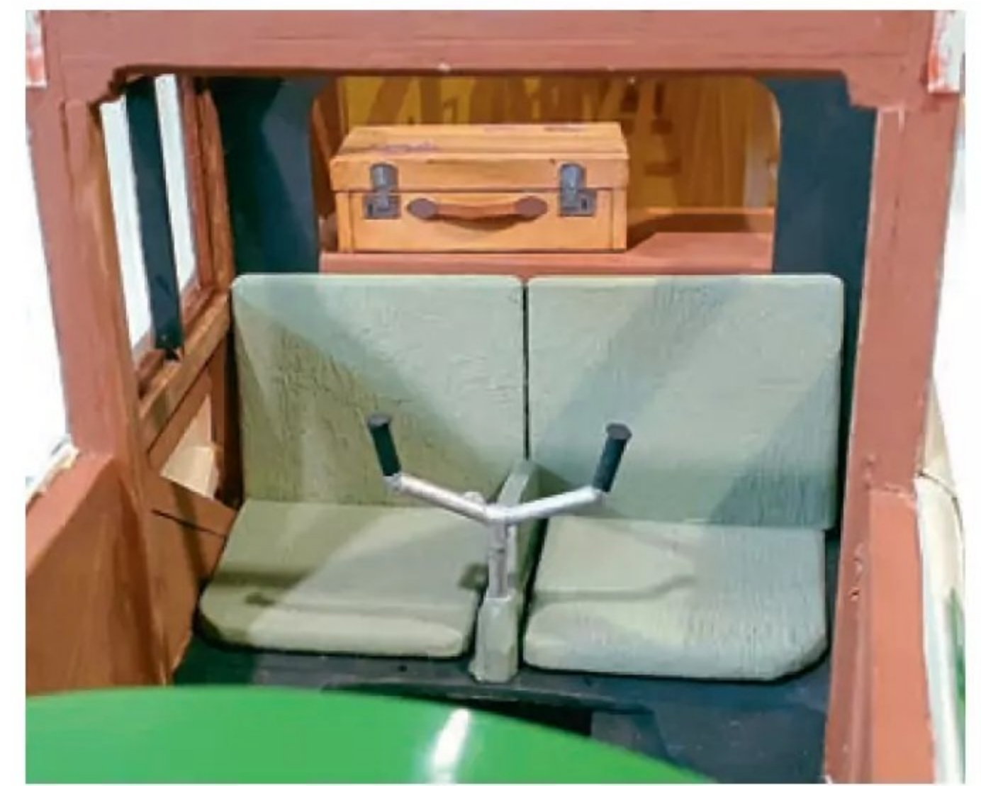
Seat pads and backs are from 6 mm foamboard covered with textured paper towel using thinned PVA glue to harden the surface and add a cloth-like texture. The case is a foam block covered with thin card.
