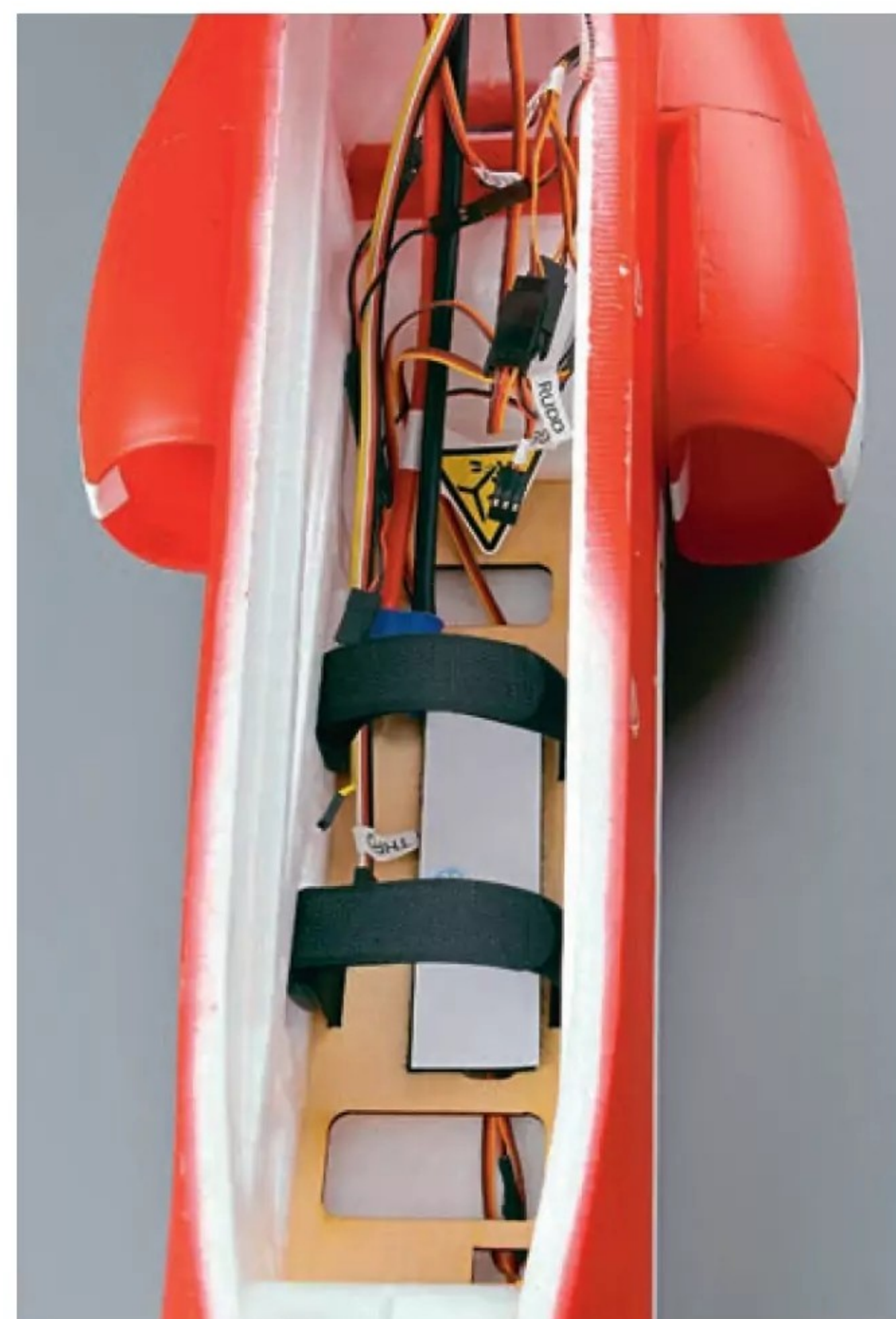
Inside the battery and radio bay. Fitting and connecting up the receiver should only take a few minutes. The battery tray uses strong hook & loop strips and straps to retain a 6S 4000 mAh LiPo.
