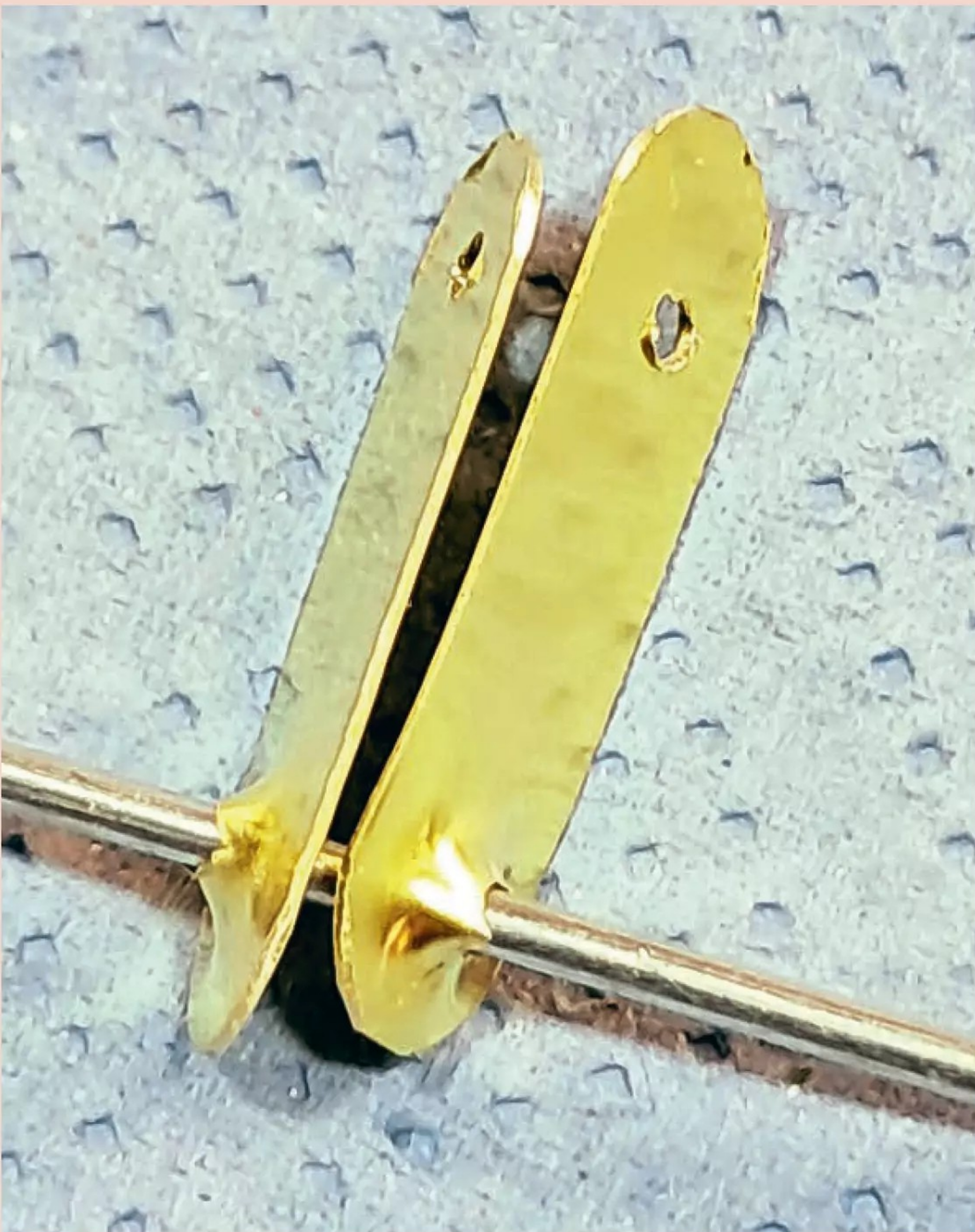
Doubled dimpled horns show how the simple modification of a flat plate gives much more soldering area/volume.
