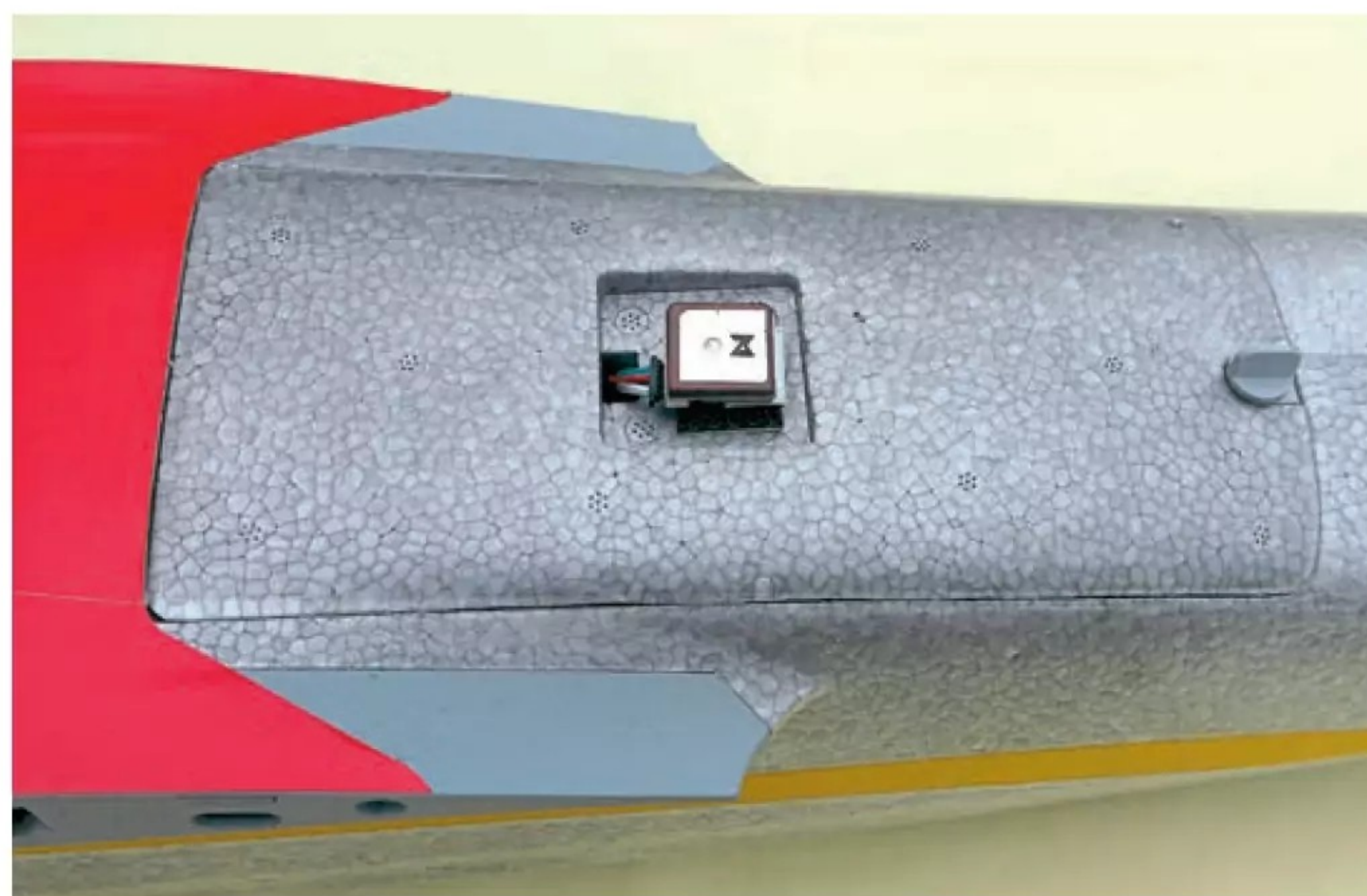
Rear hatch has a recess for fitting a GPS module.
