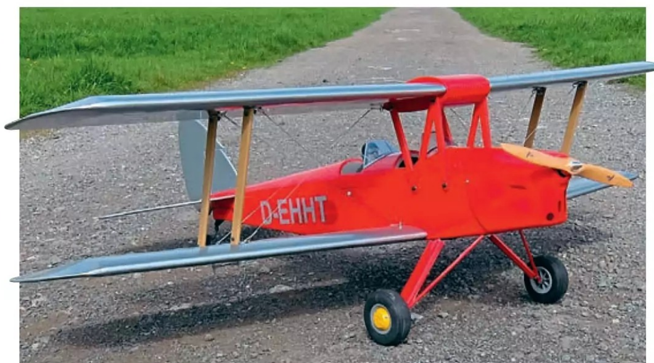
The rigging wires improve the strength of the wings.
