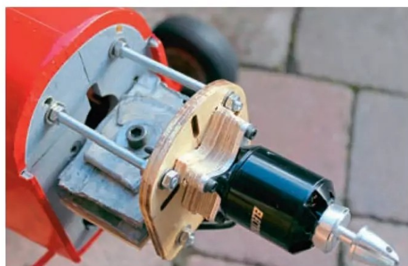
Motor mount showing the 10 mm packing piece needed to extend the firewall to prop driver distance. Note also the plates of lead bolted to the lower mounting bolts to achieve the recommended CG.
