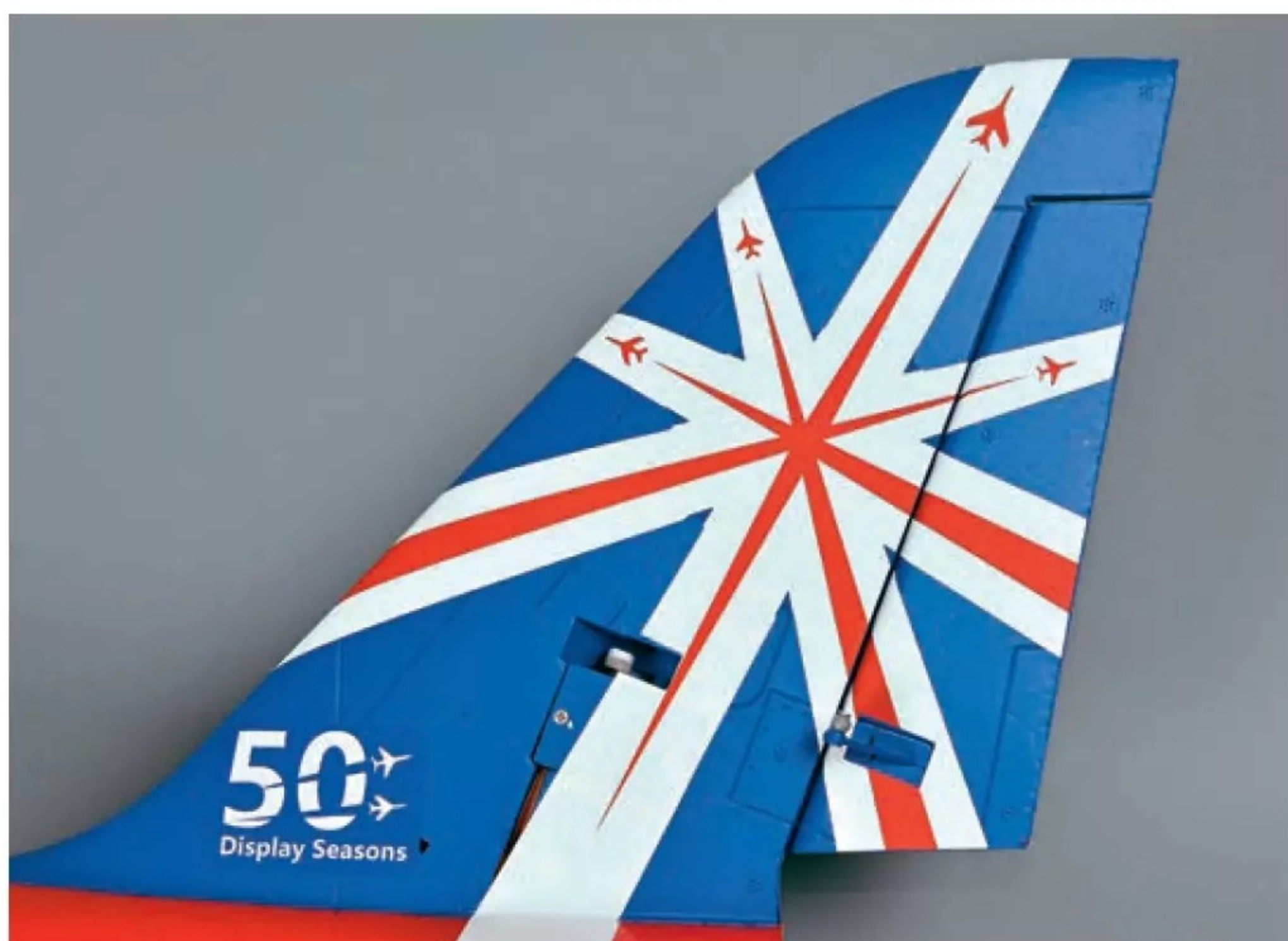
Like all the other control surfaces the rudder has its servo factory fitted close by and ready to connect with a short ball-link equipped pushrod.
