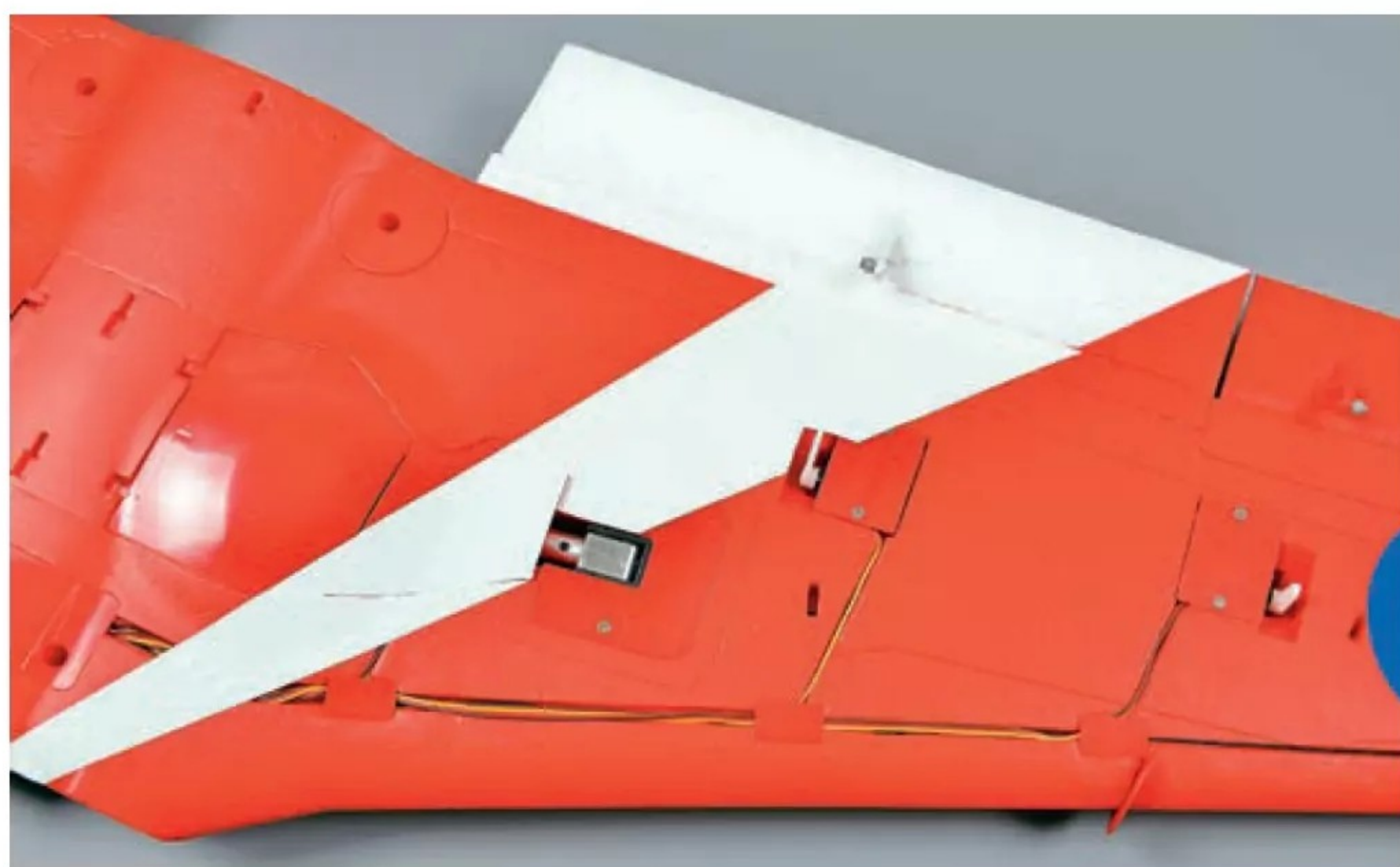
Under-wing detail showing one of the main retracts covered by its gear doors, and the aileron and flap servos, with all wiring neatly channelled close to the wing leading edge.
