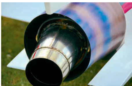
The vectored thrust nozzle on Enrico's J-10 is perfect at keeping the model 3D controlled in pitch and yaw planes but is not very effective in the roll plane.
