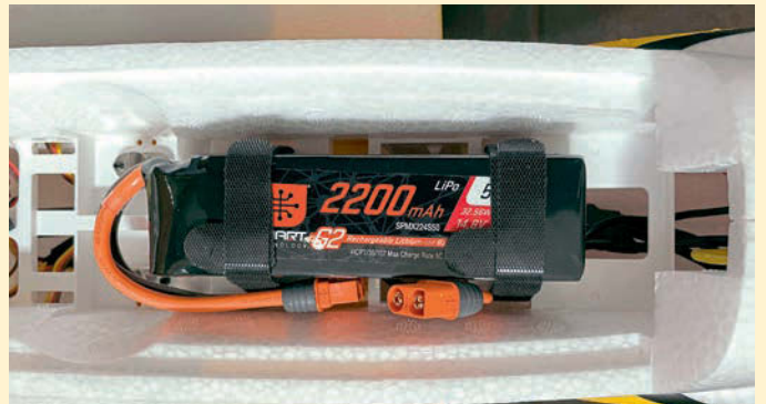
We fitted a Spektrum 2200 mAh 4S Smart LiPo so that we could use the telemetry functions provided by the AR631 six channel Rx and our Spektrum NX8+ Tx. But any 3S or 4S 2200 - 3200 mAh LiPo can be used if fitted with either an IC3 (orange) or EC3 (blue) connector.
