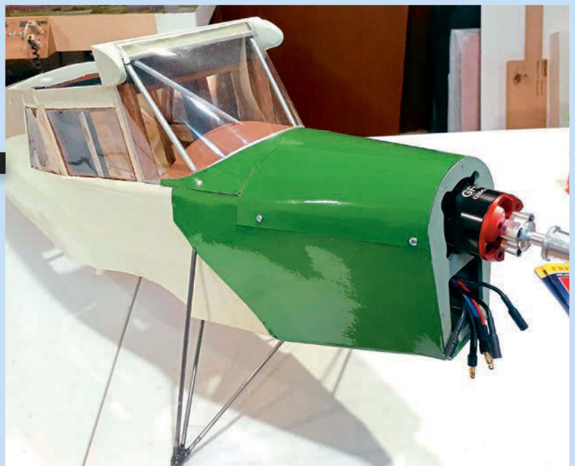
Views showing the windscreen being glued on with canopy glue and the cowl sections being shaped and fitted.
