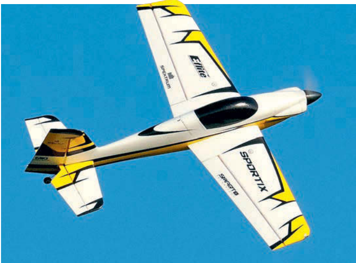
BNF Basic version is equipped with a Spektrum AR631+ receiver featuring AS3X+ stabilisation along with optional-use SAFE Select. We would recommend keeping AS3X+ always on.
