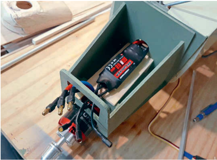
Bottom view of the motor and ESC in the motor mount structure.
