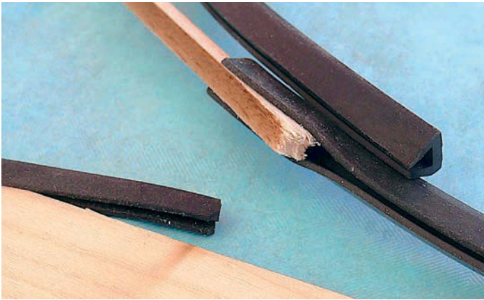
'U' section rubber edging. Narrow type on the left is perfect for cockpit coaming, with a wider version (right) perfect for slipping over wider wooden sections.
