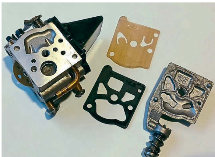
Pump side of the carb showing the pumping diaphragm and gasket.
