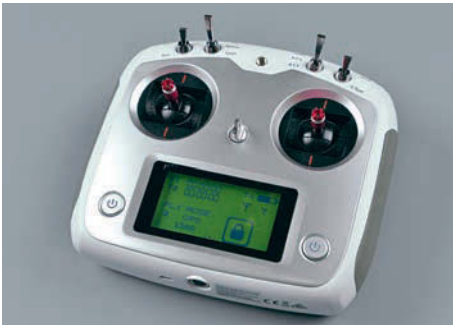
It comes with the same controller as used for the Bell 206 JetRanger but with ATT (Attitude) control replacing 3D mode. Much more appropriate for scale flying.
