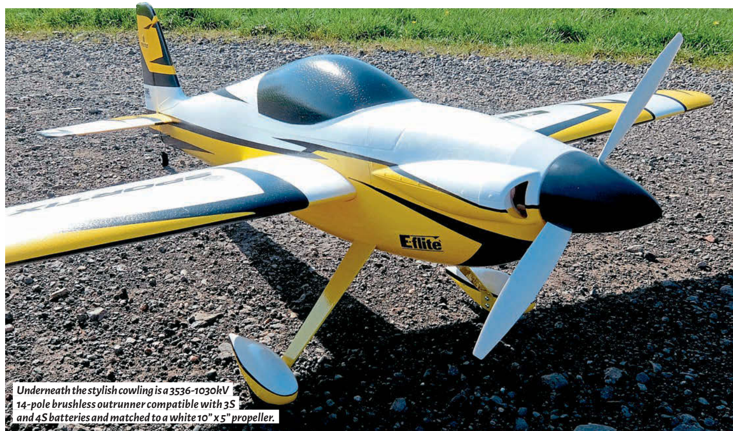
Aluminium landing gear comes factory fitted with wheels and spats. Any binding on the spats can be relieved by slackening the spat closure screws slightly.
