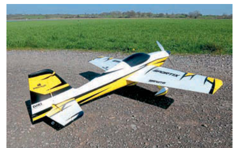
A large top mounted hatch provides easy access to the LiPo tray and the wing retainers.
