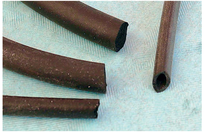
A few EPDM foam sections along with a foam tube. The tube can be carefully split lengthways to provide soft edging.
