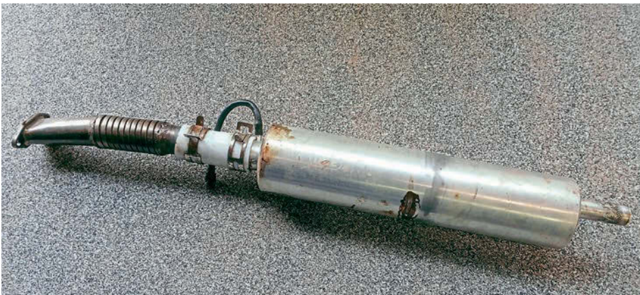
DLE canister muffler and header. This whole assembly comes in at 450 mm so is quite a hefty bit of kit. But a good muffler is needed for flying at normal club fields as the engine would be fairly noisy without it.
