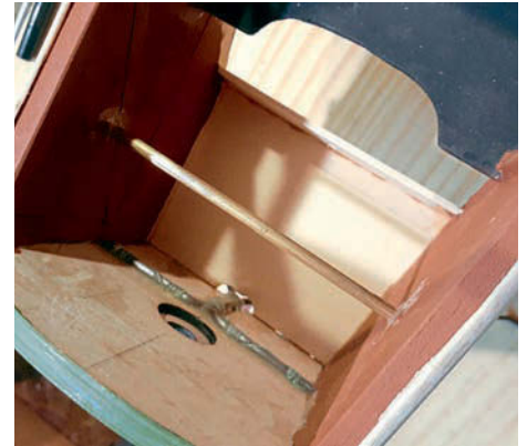
Undercarriage mounting tube is from brass tube sized to fit over the 3 mm or 1/8" U/C wire.
