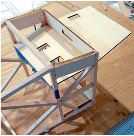
Floor structure and F3 align the rear fuselage sides.
