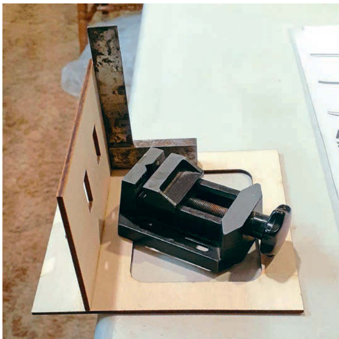
Floor and F3 being glued in place.
