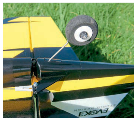
Tailwheel simply slots into place at the base of the large rudder.
