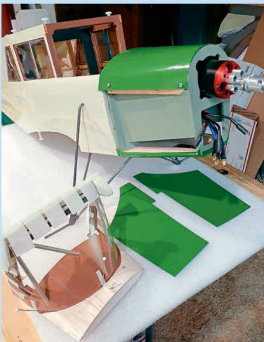
Views showing the windscreen being glued on with canopy glue and the cowl sections being shaped and fitted.
