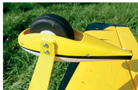
Aluminium landing gear comes factory fitted with wheels and spats. Any binding on the spats can be relieved by slackening the spat closure screws slightly.
