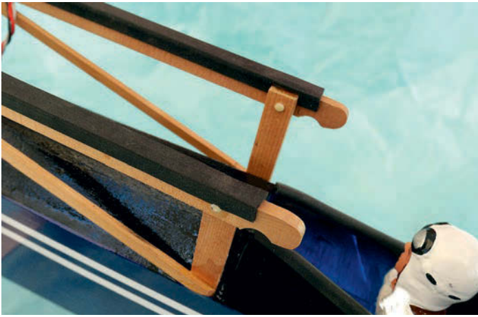
'U' section rubber edging was used to good effect on the 'Overture' wing rails. It stops the wing from wandering and chafing on the rails.
