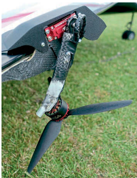
Here the thruster on Enrico's model is halfway between 'parked' and 'reverse' modes. The beefy Chaservo HV7010 servo was the only one Ralph and Enrico could find capable of coping with the immense torque generated from the set up!
