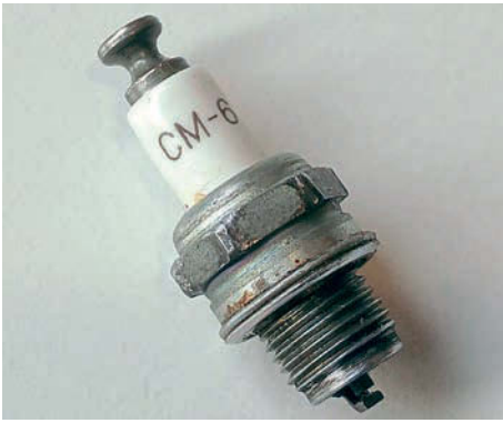
These spark plugs are cute. This is the one that was in the model when I brought it. A spark plug can tell you a lot about how your engine is running. A light tan or greyish color on the insulator tip would indicate efficient combustion and proper fuel mixture.
