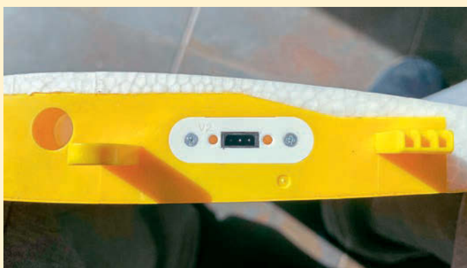
Two-piece wing has hands-free servo connections. Wing left, fuselage right.
