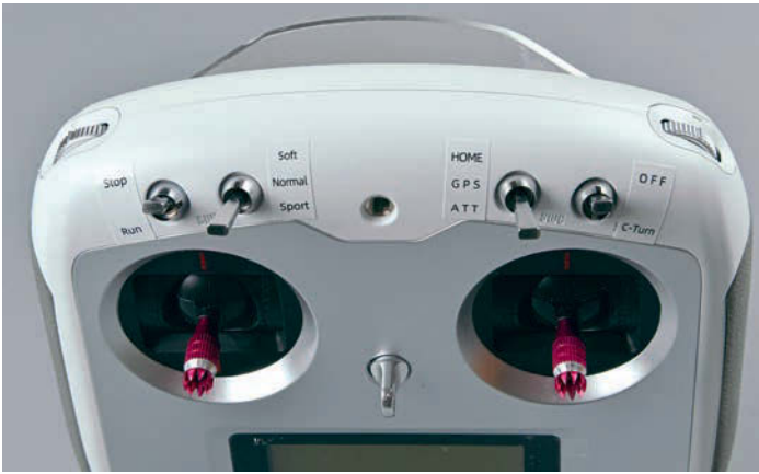
The last three shoulder switches on the ACE controller now access different functions to the H1 set used by our previous Bell 206. SW-B has three sensitivity settings instead of auto circle and figure of eight patterns whilst SW-C has an ATT setting in place of 3D mode. Finally, the unused SW-D now switches on C-Turn - but we won't be using it.
