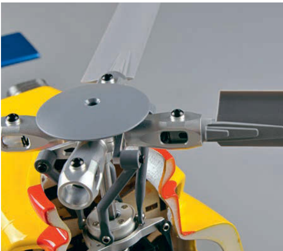
Each blade is inserted vertically, pushed in against a spring and then turned to lock them in place.
