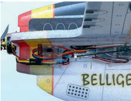
With the Rx and ESC on one side and the 2S 450 LiPo on the other.
