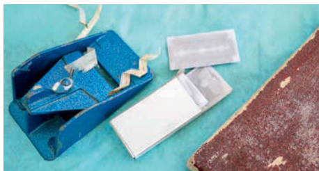
My poor battered razor plane saw hard use on the 'Overture' build. Regular blade replacement was demanded by the iron-hard wood.
