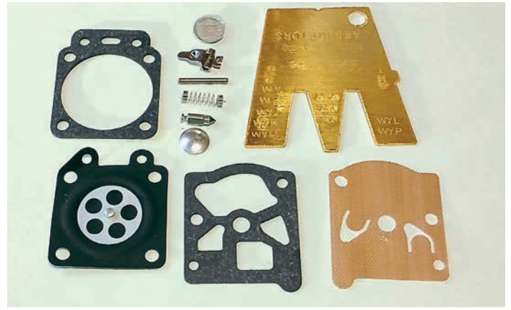
The parts needed to service the WT series carb on my DLE engine. The kit came with two of everything and parts for other carb types but finding the bits you need is straightforward.
