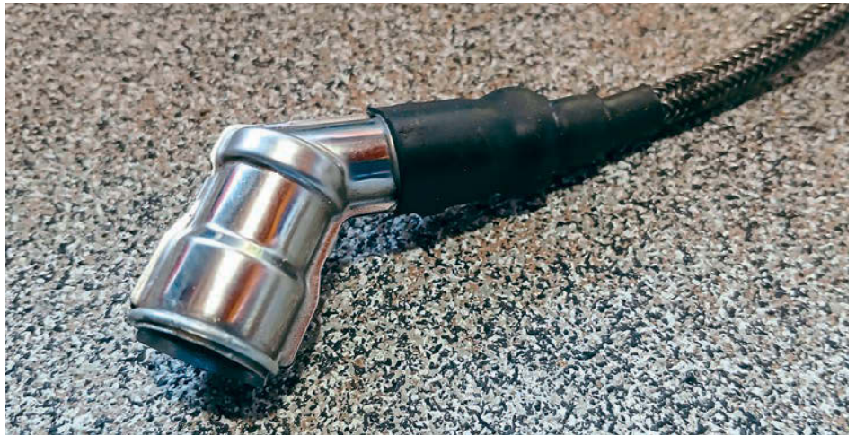
The spark-plug cap and insulator that I needed to change. It was simple to do and new parts were swiftly sent courtesy of Probuild.
