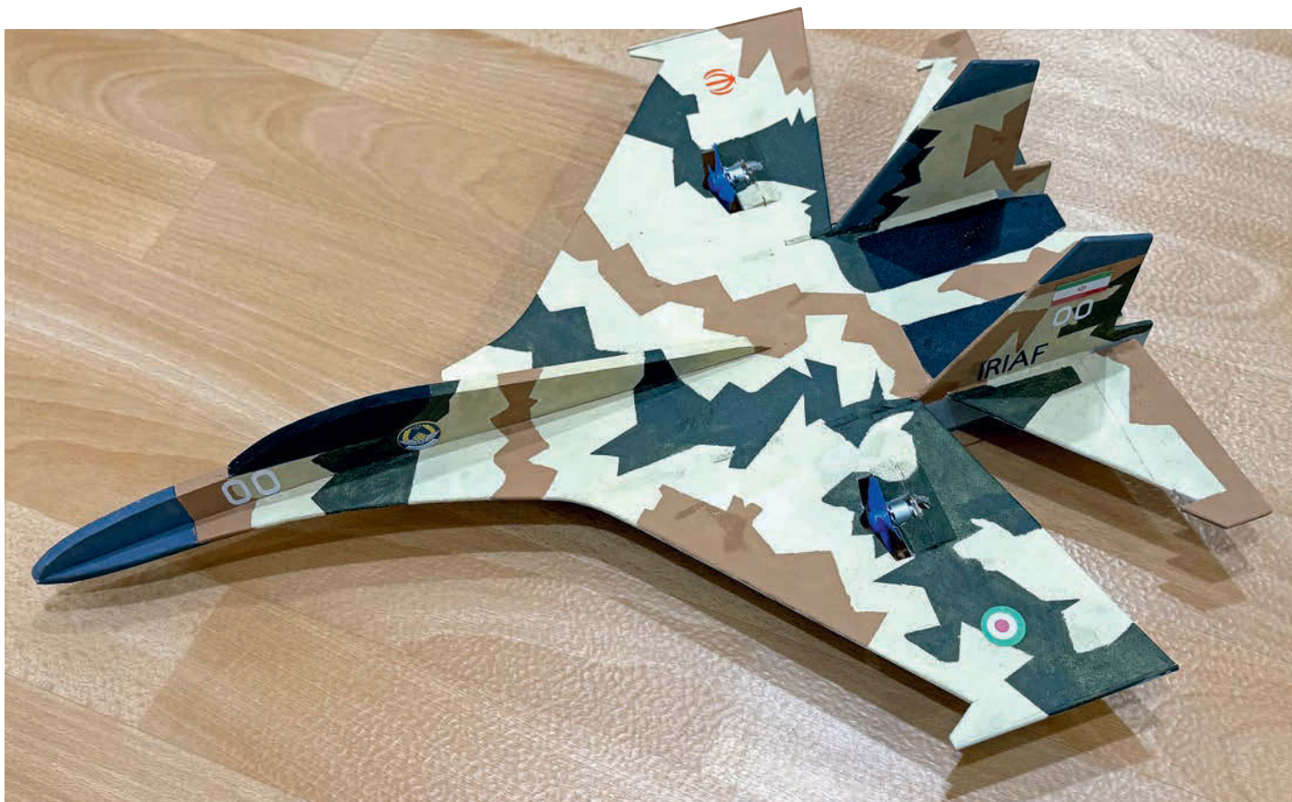
Su-27 uses two brushless units from a quad and flies brilliantly.
