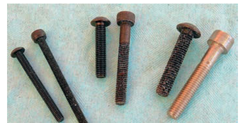
'Cap' and 'button' head screws/bolts. You can see the height saving of the button over the cap type. There's virtually no difference in strength.
