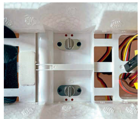
Quarter turn spring lock retainers make securing the wing panels a quick and easy task.
