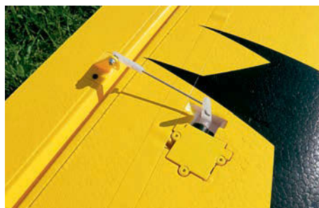
Four A347 Sub-Micro Digital 9g Metal Gear servos operate the flight controls via ball-link linkages. Aileron servo shown here.
