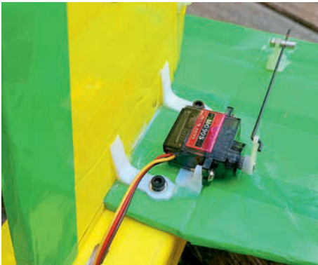
Tail assembly showing one side of the vertical stab mount and the elevator servo mounts.
