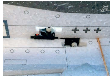
6g servos almost disappear in the 10 mm thick EPP.
