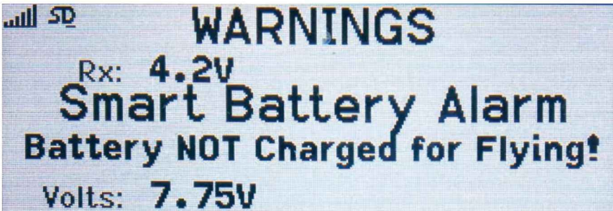
Many of Horizon's latest products have Smart Technology embedded within them. This warning came up automatically when a partially charged LiPo was plugged in to our latest review model.
