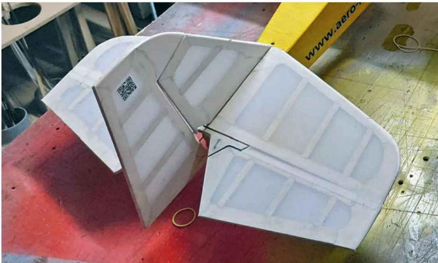
Tail parts are simple to build. Paper covering is supplied for this area.
