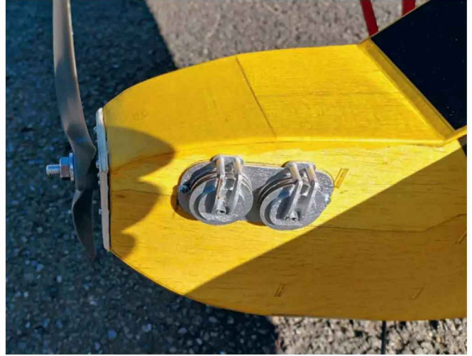
Best hold off adding the top nose sheeting until the ESC has been installed and connected to the motor. Bernd's home-made dummy engine pots add to the character of the model.
