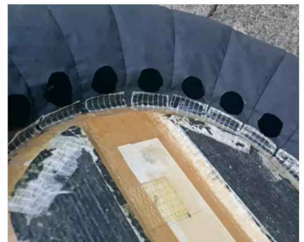
Under-skirt of Alan's F1 Racer showing the bleed holes that allow air to pass from the bag skirt into the plenum under the hovercraft. Cross-weave tape keeps the internal edge of the skirt in place.
