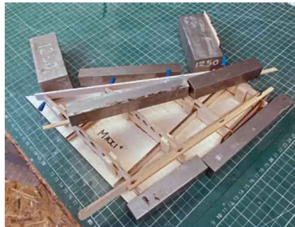
The fin was also built on a simple jig.
