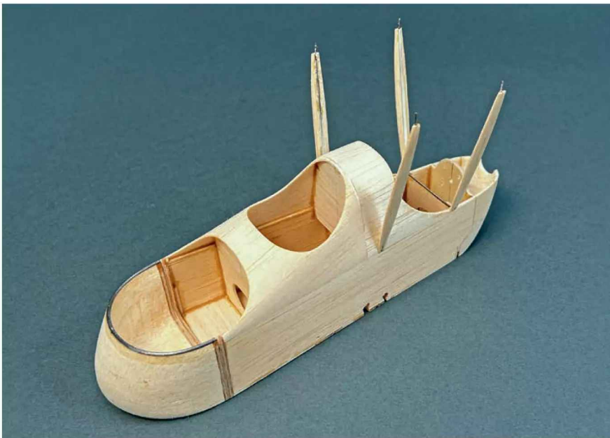
Completed front fuselage ready for covering.
