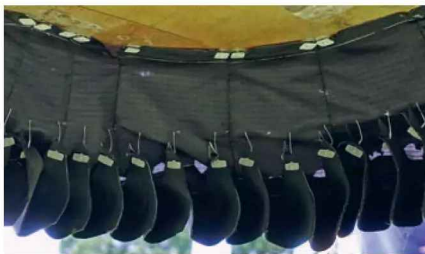
Some of the air bleed holes from the SR.N6 bag skirt into the fingers can be seen here, as well as the 'Quick Tags' used to stop the fingers from blowing out.
