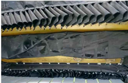
A look under the skirt of Tim Stevenson's SR.N6 hovercraft showing the combined bag and finger skirt sections. That keel down the centre inflates when the fan is running to create a baffle down the centre of the plenum to help reduce the loss of air if the hovercraft gets stuck.
