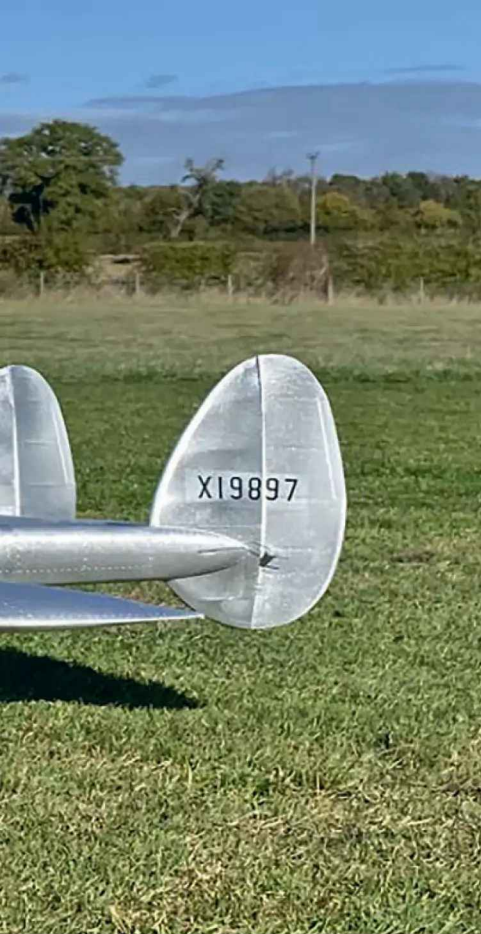
Most of the model uses normal PLA or PLA Tough. I used PLA Tough, with a few components printed using PLA LW (Light Weight). TPU was used for the tyres and flexible hinges.
