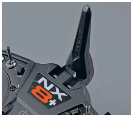
Antenna should be raised in flight to avoid pointing it directly at the model. There are several angles to choose from.
