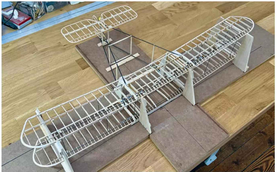
Test assembly using the fuselage and wing jigs to support the delicate airframe.
