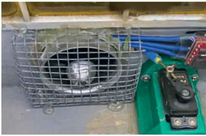
The EDF unit used for the PuffPort. The servo opens the door and an Arduino Nano Microcontroller sequences the fan to start up once the door is fully open.
