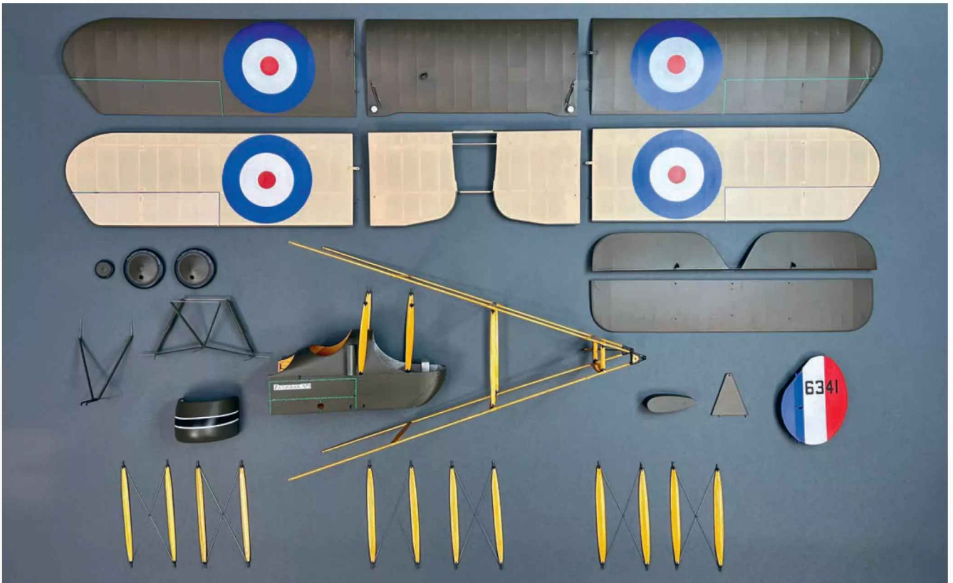
All parts are individually finished prior to final assembly of the FE2b. 6341 has a typical RFC colour scheme using Clear Doped Linen on the undersides and PC10 on the upper sides.
