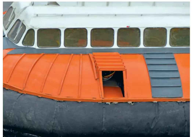
Close up of the left hand 'PuffPort' side thruster with the door open.
