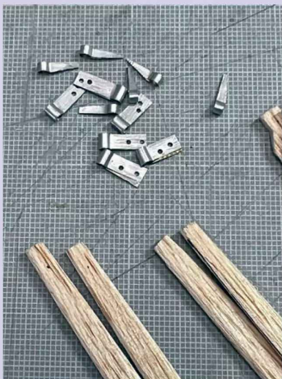
Strips of beer can sheet metal are used to attach the balsa struts to the carbon fibre tail boom tubes. The strips bend around the tubes and form strong mounts for the struts.
