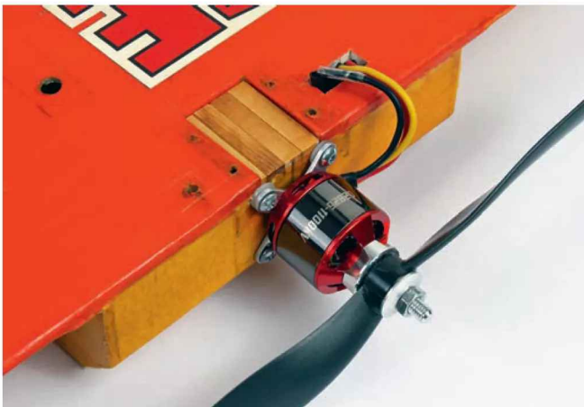
With the original PAW 1.49 diesel long gone I added an outrunner.
