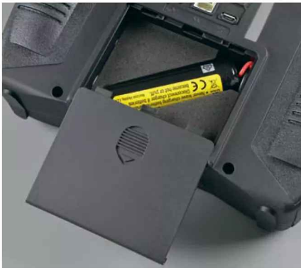
In the back of the Tx is a 3.7V 2200 mAh 1S Li-Ion battery.
