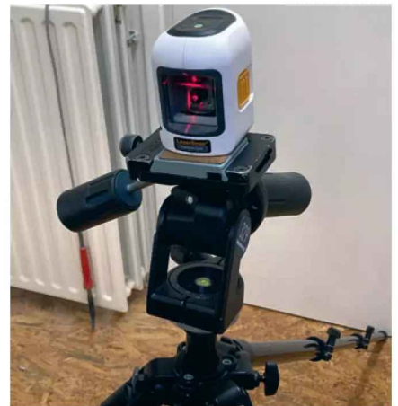
To ensure accurate positioning of the fin and stabiliser, both in relation to the fuselage and each other, I used a simple laser liner, placed on a tripod.
