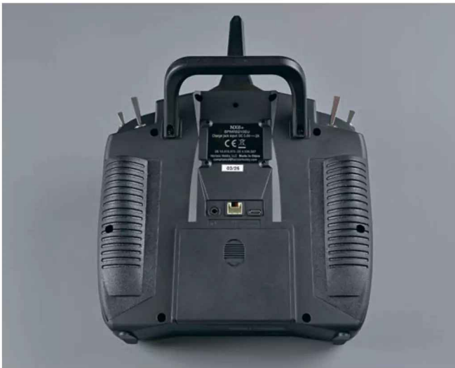
Back panel view. The area denoted by the CE label can be used to screw down a Crossfire module connected to the white serial port, but you'll need to power the module from a separate battery.
