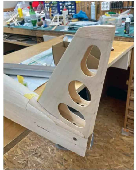
This is how it all looks once finished. The fuselage was designed to extend slightly, enabling it to be sanded flush after installing the fin.
