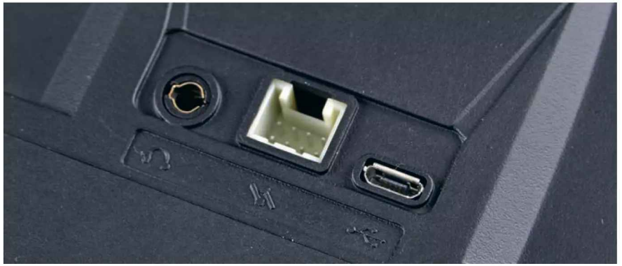
Connector area just above the battery bay showing the headphone port on the left, serial port in the middle and USB port to the right.
