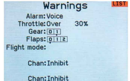
Warnings menu allows you to program voice, tone or vibration alerts for any channel or switch position.
