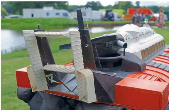
Look closely and you can see the bell-crank that controls the elevators. Tim uses a switch on his Tx to trim the elevators to adjust the pitch of the hovercraft in flight. It's surprisingly effective, especially in windy conditions.
