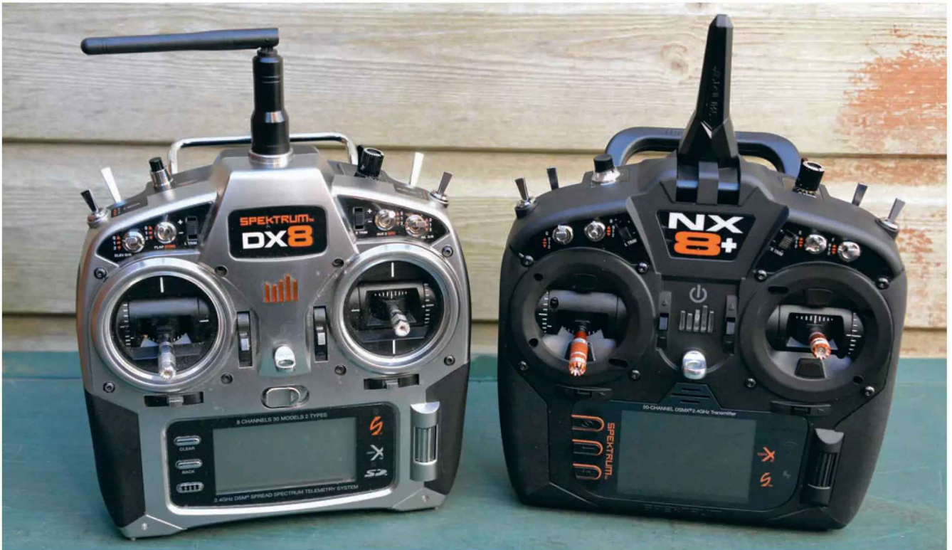
You can share model files from a DX transmitter to the NX8+, but you can't do it the other way around.
