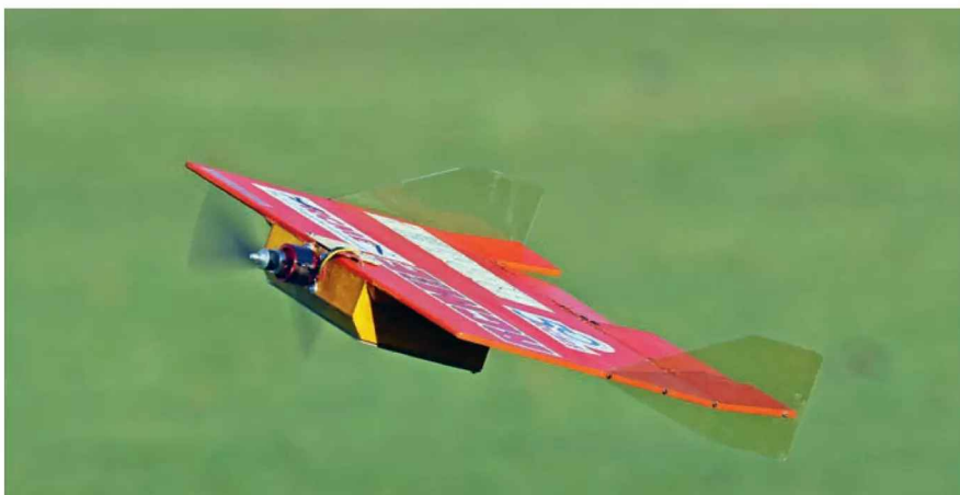
It seems to fly with a distinct nose up attitude, although the plan makes no mention of down thrust.
