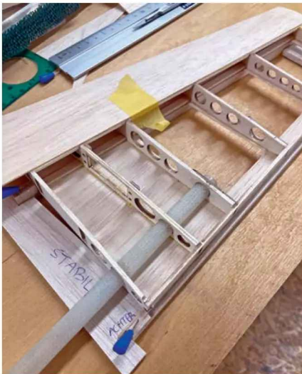
A look inside a stabiliser, using the second rib as an aperture to fit the elevator servo. Fiddly to install, but thankfully it is only required once.
