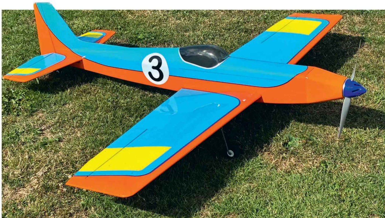
Much as I liked the 'Gulf' scheme it proved to have insufficient contrast so bright yellow patches were added later in lieu of the logos.
