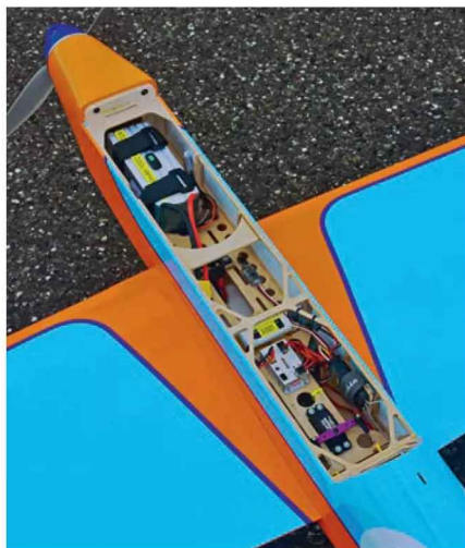
Plenty of room inside. With the battery located against the front former, there is no need for ballast. Removable hatch gives unrestricted access.
