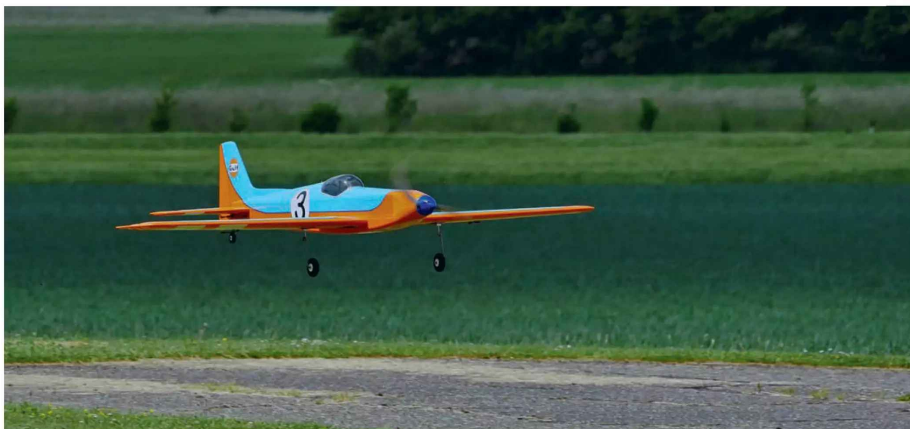
Coming in for landing. It takes time for the speed to bleed off as the model is so aerodynamically clean.
