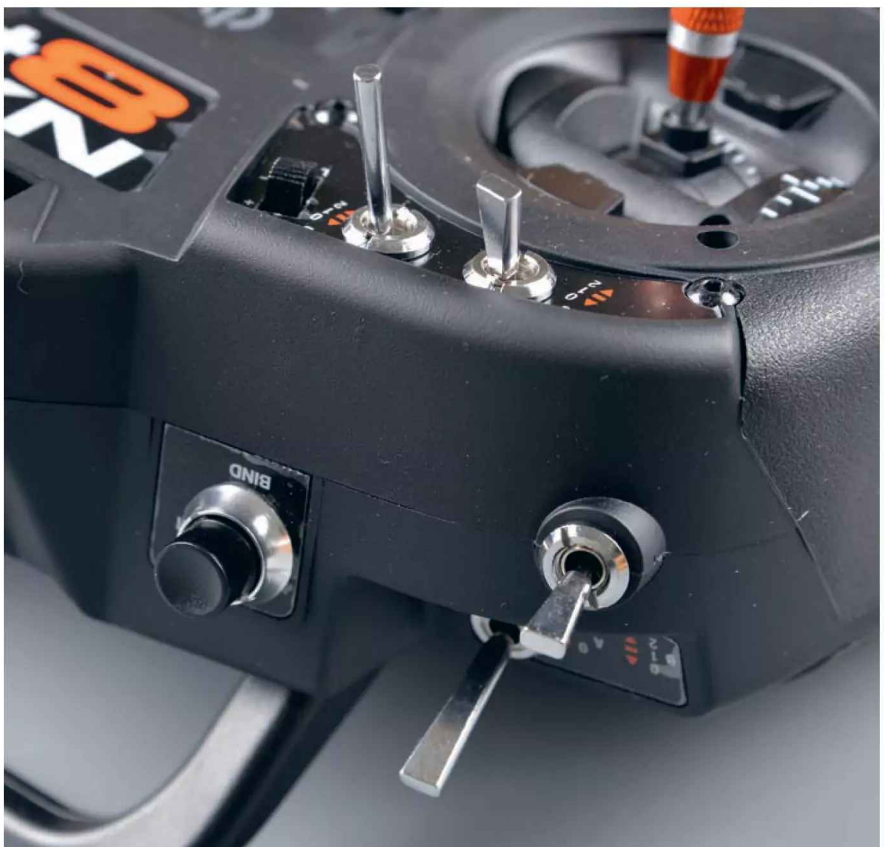
Top & above: NX8+ has the usual array of programmable shoulder switches, including a variable knob on the right and the Bind/Trainer button on the left.
