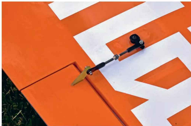
Savöx SB-2265MG+ aileron servos are placed upright and are recessed as deep into the wing as possible to minimise turbulence.
