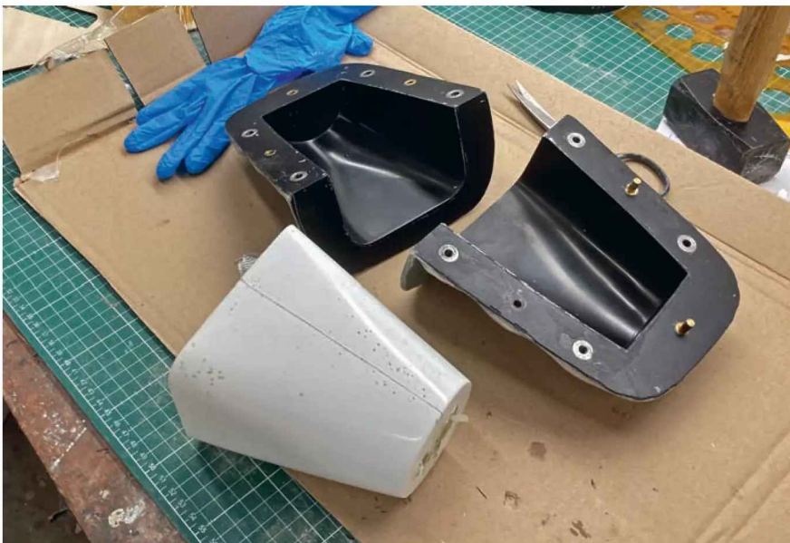
A project in itself, this shows the cowling and the two-part mould in which it was constructed.
