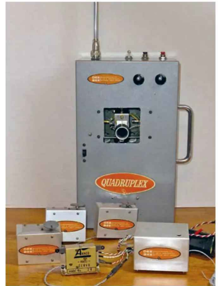
An example of the Dee Bee Quadruplex, another R/C system used by Maynard in some of his record-breaking flights.
