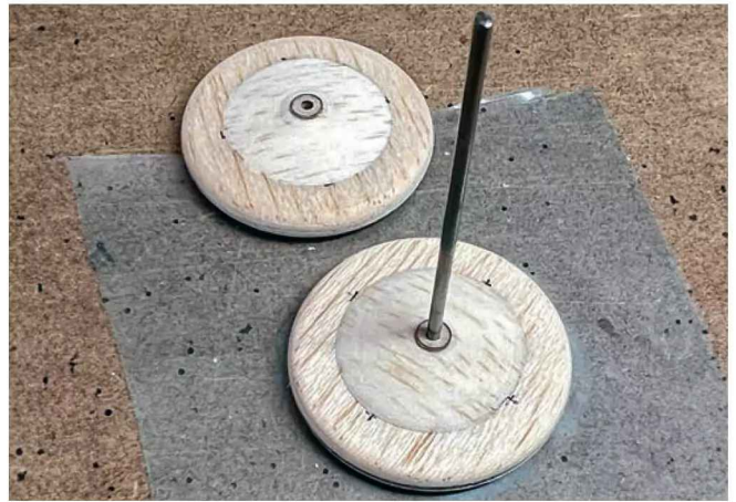
Hubs are made from 2 mm plastic tubes with 1 mm holes. The balsa blanks were turned using a mini drill.
