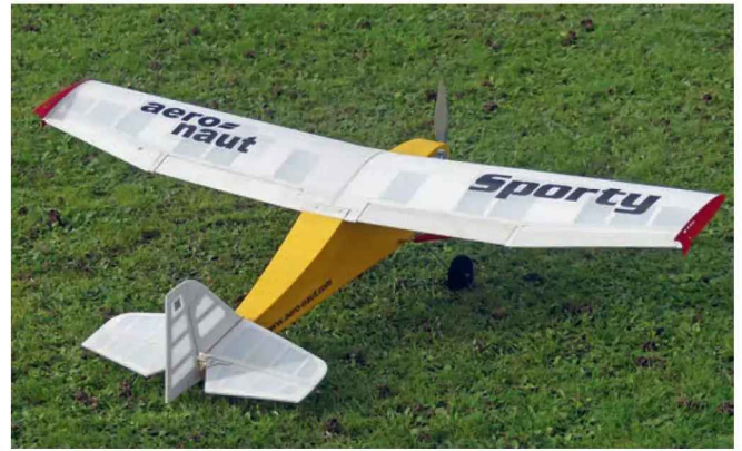
Sporty has generously sized control surfaces. The recommended movements result in an easy to fly model.
