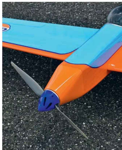
Intake of cooling air is solely provided through a 70 mm Kuza spinner. Airscrew is an APC-E14 x 10.
