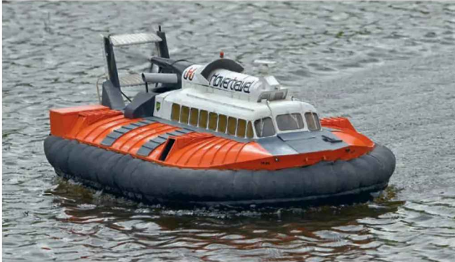
PuffPorts improve the manoeuvrability of Tim's SR.N6 immensely. Check out the wake as the hovercraft sideslips across the water.
