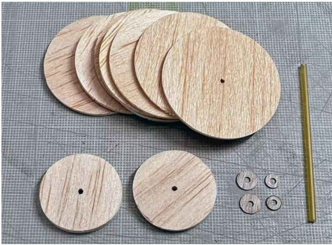
Wheels are laminated from 1.5 mm balsa discs.
