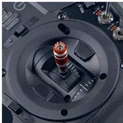
Stick length can be adjusted using the Allen key supplied. As a 'thumbs on top' flyer I found them most comfortable when wound fully down.
