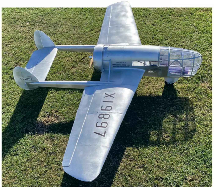
Most of the model uses normal PLA or PLA Tough. I used PLA Tough, with a few components printed using PLA LW (Light Weight). TPU was used for the tyres and flexible hinges.
