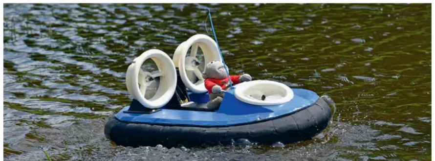
Differential speeds of the thrust motors make Alan's hovercraft very manoeuvrable.
