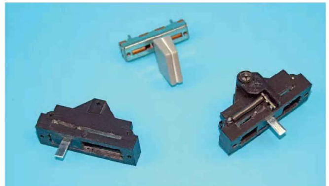
Tobe designed 3D printed housings for the slider pots to allow them to self-neutralise for rudder, aileron and elevator.
