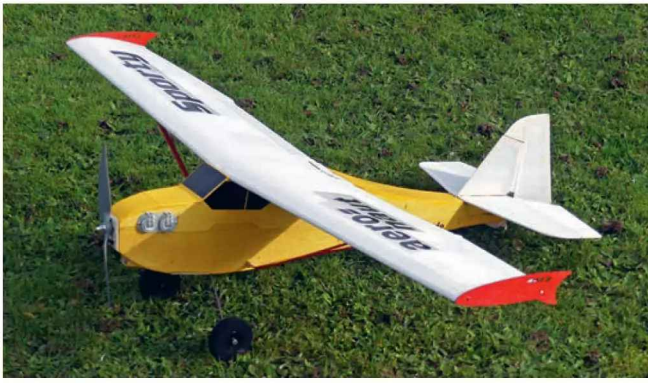
The fuselage was covered with yellow Jap tissue paper and painted with clear varnish. Bernd covered the wings and tail with ProfiCover2 film which is ironed on and looks just like silk.
