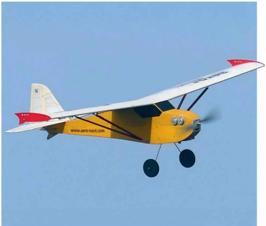
This easy to fly model can be equipped with optional flaps and a tow release for tugging up small gliders.
