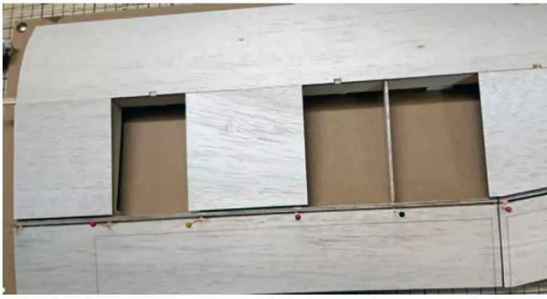
Wing sheeting almost complete, with the flaps and ailerons marked and ready for cutting out.
