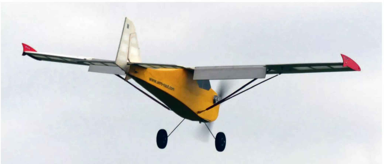
With full flap Sporty can be flown down the flightline at walking pace.
