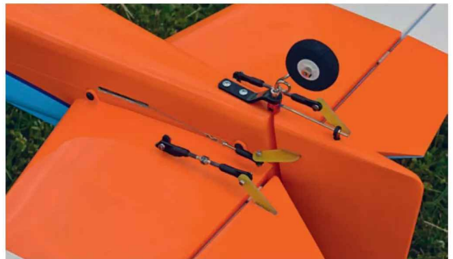
Lots going on at the rear. The tailwheel is a generic assembly for .60 to .90 size models. The rudder is actuated by pull-pull cables and each elevator half has its own servo to allow removal for transport and storage. Note the mounting lips on the root rib and the ball link for the tailwheel steering.
