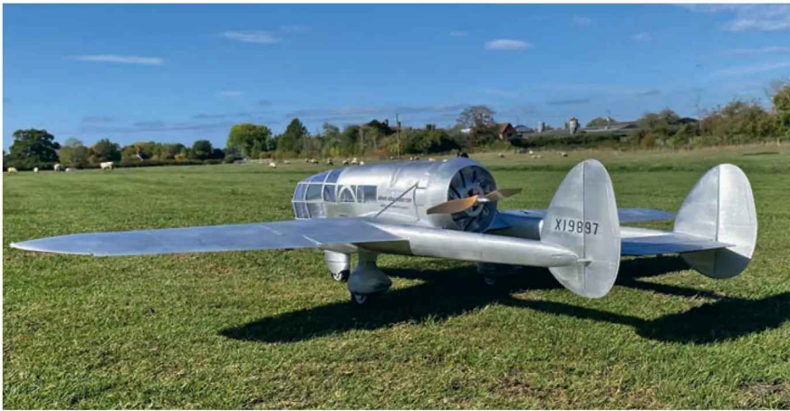
My Abrams P1 Explorer has had quite a few flights with no signs of any damage. But it did need the elevator cable beefing up.
