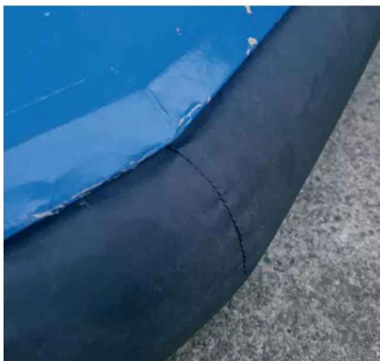
Close up of the skirt on Alan's F1 Racer. Double sided tape attaches it to the hull.
