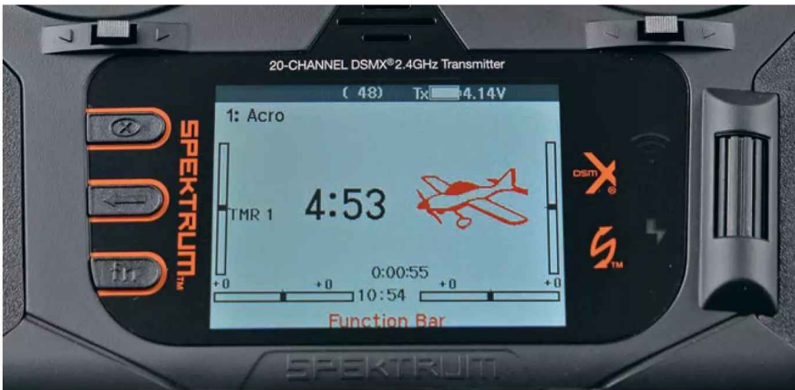
Navigation of menus shown on the 3.2" colour display are quickly made using the roller wheel on the right and the Clear, Back, and Function buttons on the left.
