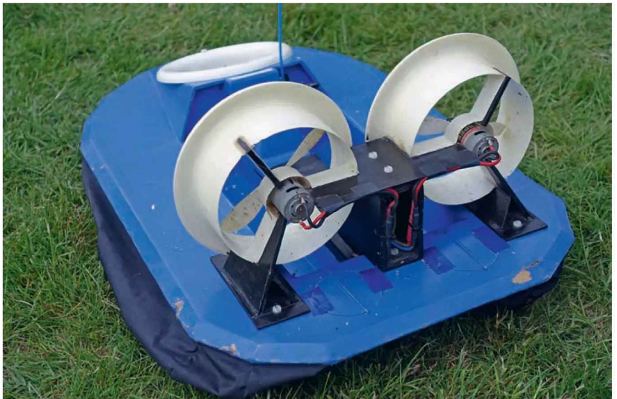
Alan's F1 Racer is 20 years old and still runs on the original Speed 400 motors and Gunther props. Cheap construction and simple controls make it terrific value for money.
