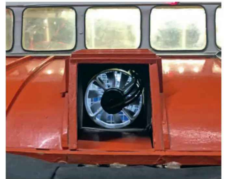
Looking down the PuffPort duct to the EDF unit.
