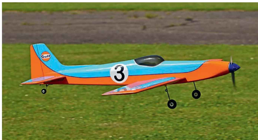
Mäxi+ uses a retractable taildragger undercarriage instead of the tricycle gear used on the original design.
