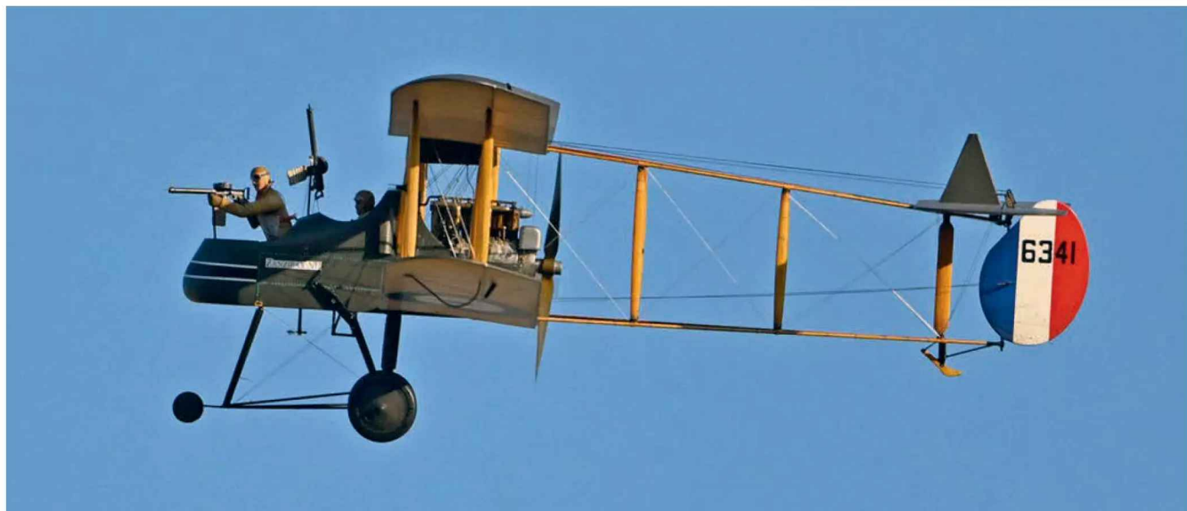
FE2b is tricky regarding the CG position because of the rear mounted motor. But the battery can be placed at the front. Consideration also needs to be made of the moment arm, i.e. the length of the nose in front of the CG and the length of the rear fuselage behind the CG, and the ratio between them.
