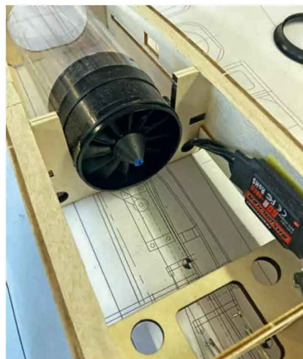
EDF unit and ESC fitted and tested for correct rotation.
