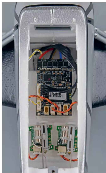
Inside view of the fuselage mounted avionics. Combined receiver and ESC at the top and two long throw linear servos for the rudder and elevator below. The black ribbon cable connects to the wing mounted distribution board.
