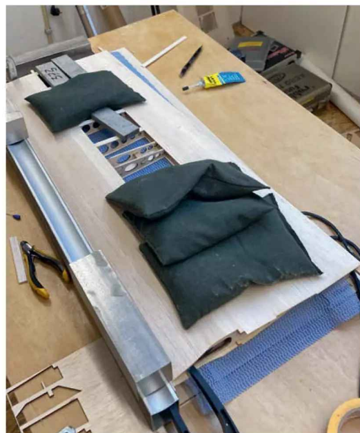
Placed in another jig, sheeting is applied with slow-drying PVA and left to dry for at least 24 hours whilst being weighed down with bags of sand.
