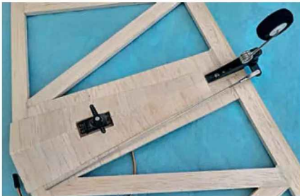
Under 'The Bigger Ship' tailplane showing the steerable tailwheel option. If the tailwheel turns in opposition to the rudder, I'll simply swap the pushrod from one servo arm to the other.
