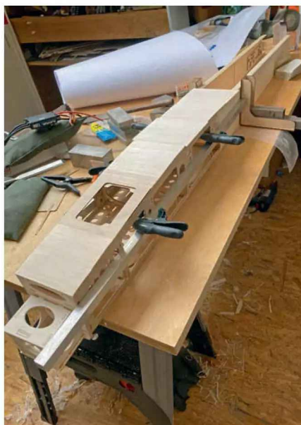
The front half of the fuselage is basically a square box. It is clamped tightly to the workbench and multiple aluminium sections are temporarily attached to ensure it remains straight during initial sheeting. Once the glue has dried the fuselage becomes so stiff that it is nearly impossible for it go banana shaped.
