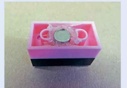
Standard square and rectangular bricks with magnets epoxied in place.
