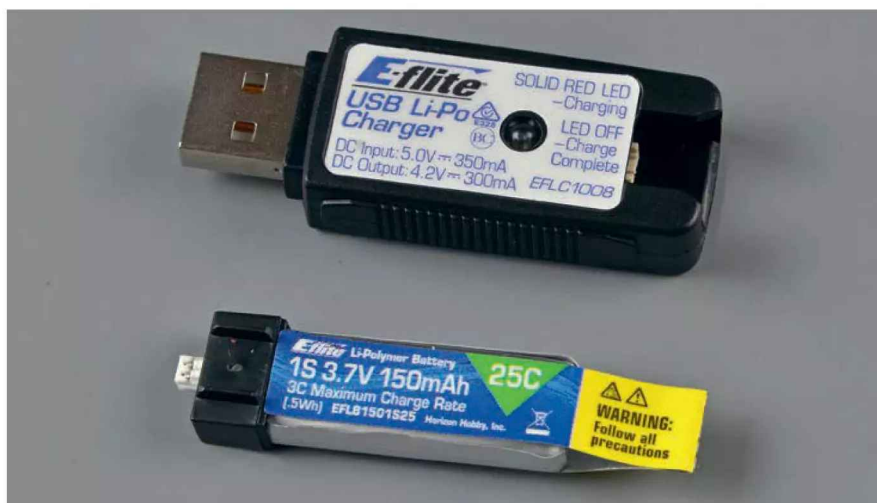
Night Vapor is supplied with a 150 mAh one-cell LiPo and matching USB charger.
