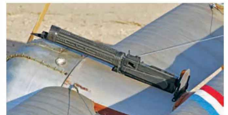
Vickers .303 machine gun was 3D printed by Luis Vazquez.
