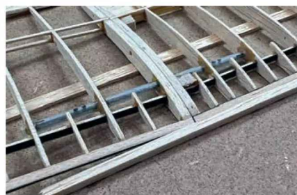
Dihedral joints are made using thin plastic tubes and one and two millimetre carbon fibre tubes.
