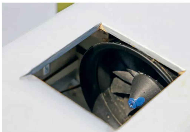
Underside air intake hole can be used to gain access to the swing-wing links.
