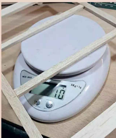
If you're going to do a test piece for new covering, document all the weights for later calculations.
