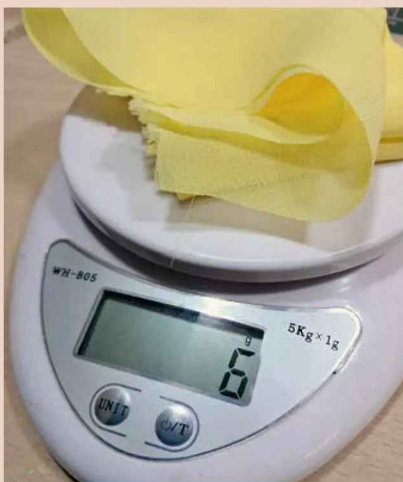
If you're going to do a test piece for new covering, document all the weights for later calculations.
