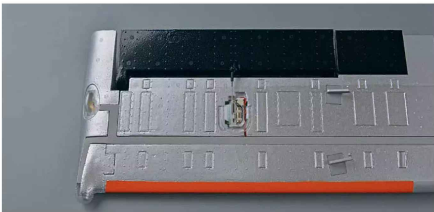
End of a wing panel showing one of the jumbo ailerons connected to its long throw linear servo. Note also the two small ball mounts to the right-hand side for connecting a V-strut.
