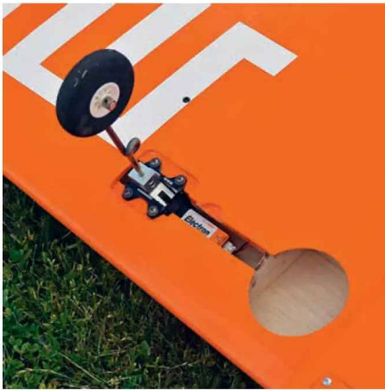
Electron ER-30 Classic retracts are used in the Mäxi+. The black dot in the 'M' of the Mäxi logo is the head of the M3 screw securing the wing joiner tube.
