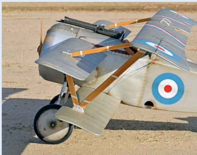
The Triplane's interplane struts were probably some of the most uncommon ever made. In the model they are made from Marupa, a closed grained tropical wood, with 1 mm steel plate laser cut fittings embedded in the ends.
