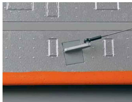
V-strut wing fixings are much easier. Simply pop on the ball links!
