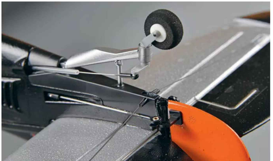
The steerable tail wheel closely resembles the full-size affair and is operated by a separate, thinner pushrod. Note the sturdier gauge wire used to operate the tail surfaces.
