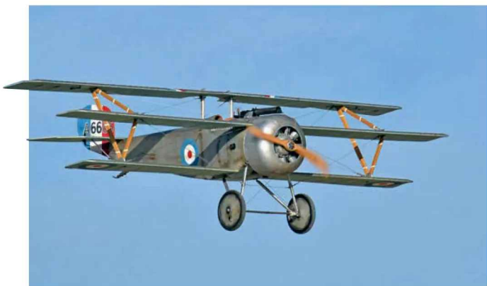
Mário's Triplane was covered in 'Antique' Oratex fabric, sprayed with automotive paint but without a base coat to save weight.
