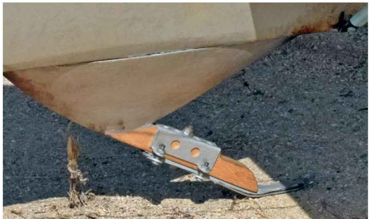
Tail skid is made from Marupa and steel plates, glued to a ply former and faired with balsa wood.
