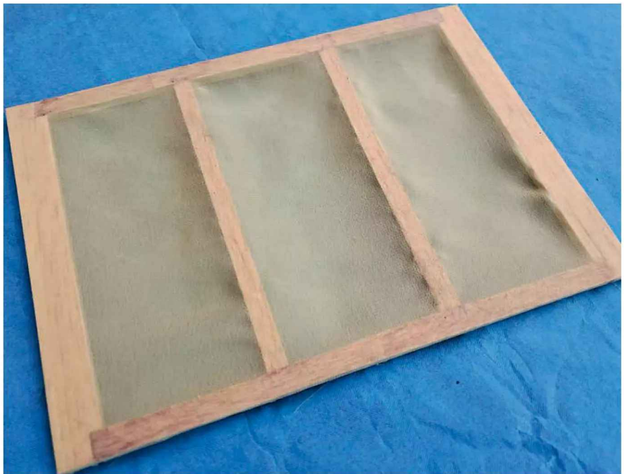
The test frame I made to check out polyester cloth as a covering material.
