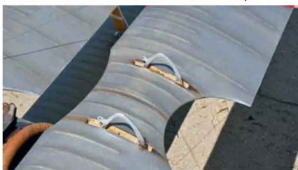
On the original the ailerons were actuated by centre section horns via torque tubes. In Mário's model they are moved by servos in the wing, but the ailerons are connected to the fake horns for a more realistic action.
