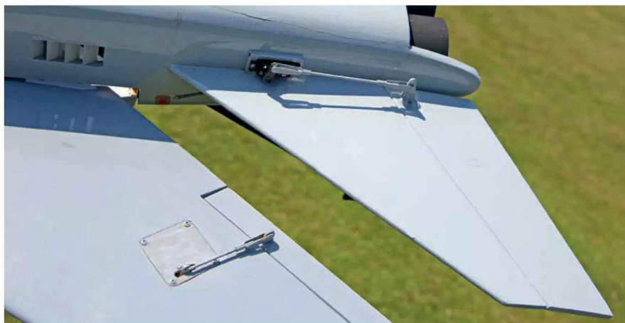
With the wings swept the short and direct aileron and elevator linkages can clearly be seen.
