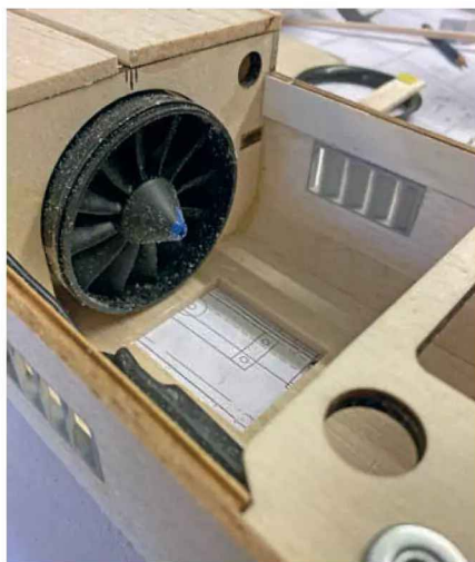
View of the critically sized air intakes, two on the sides and one at the bottom.
