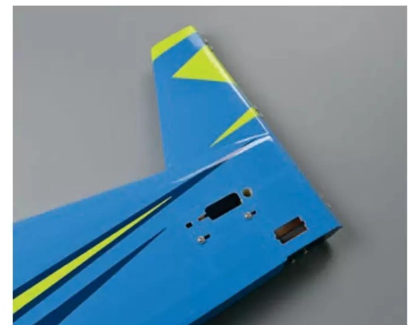
*Rear fuselage showing the tailplane mounting area and a slot for a rear mounted rudder servo. I might opt for a closed loop rudder servo mounted amidships instead.*
