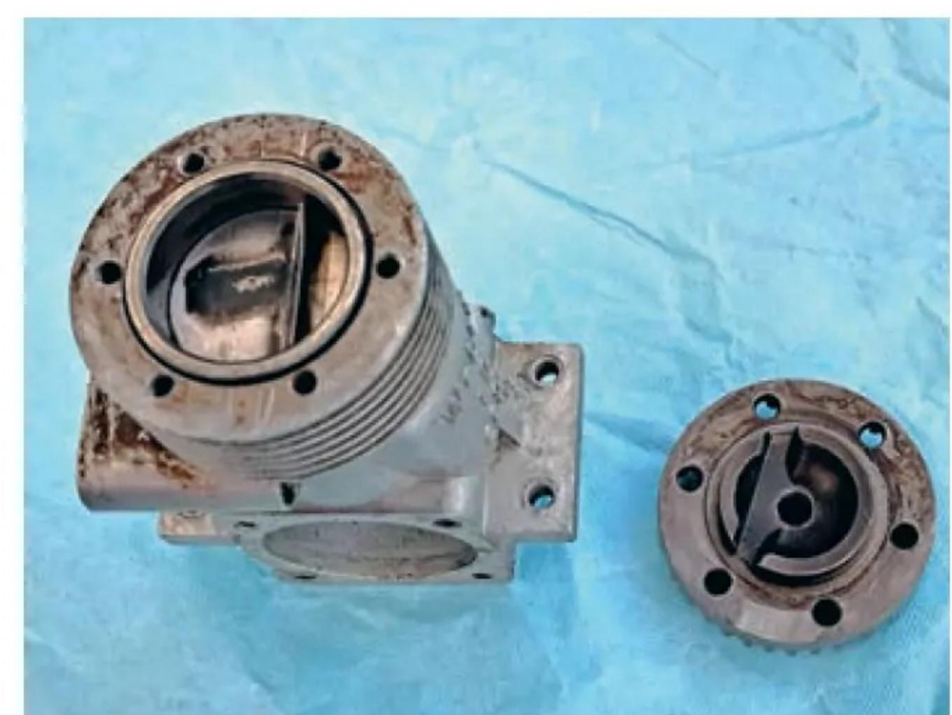
A bit of scrubbing needed! The Webra combustion chamber shows its burn pattern 'witness' marks writ in carbon.
