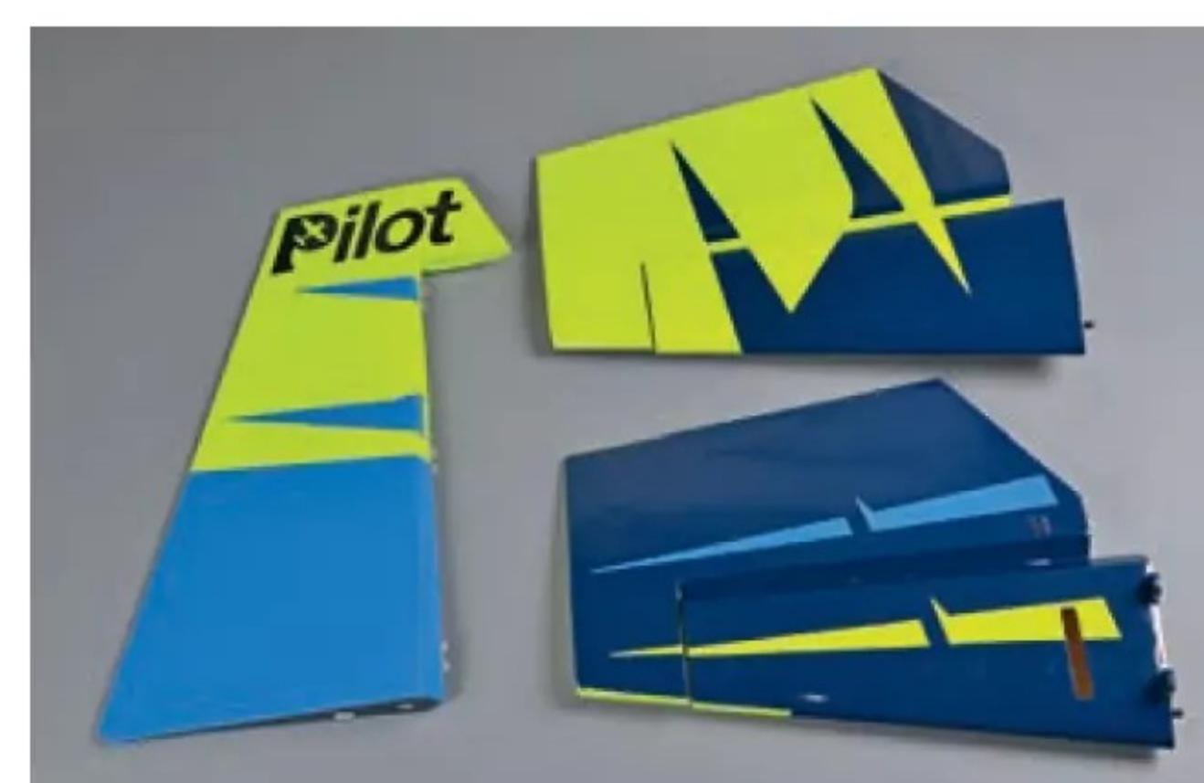
*Stabiliser halves and the rudder are removable for transit and storage but can be quickly reattached at the flying field.*
