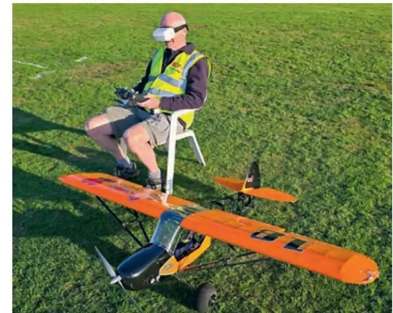
**Yours truly about to take an FPV joyride in Dom Mitchell's 1.9 m span Dancing Wings Savage Bobber bush plane fitted with a Walksnail GM3 3-axis gimballed FPV camera. I'm wearing Walksnail Avatar HD FPV goggles with integrated head tracking which drives the camera gimbal - amazing stuff! I'm just holding the Tx for the photo. Dom did the actual flying.**
