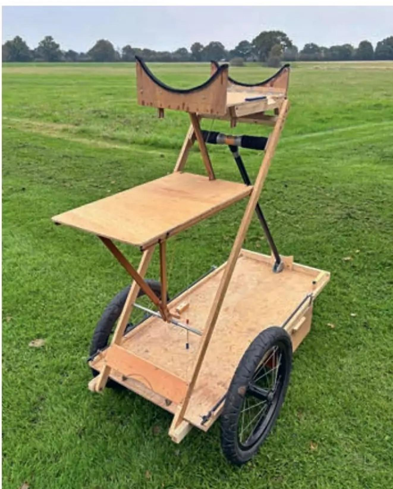
*The model rack unclips and a stand/shelf slides out from underneath.*
