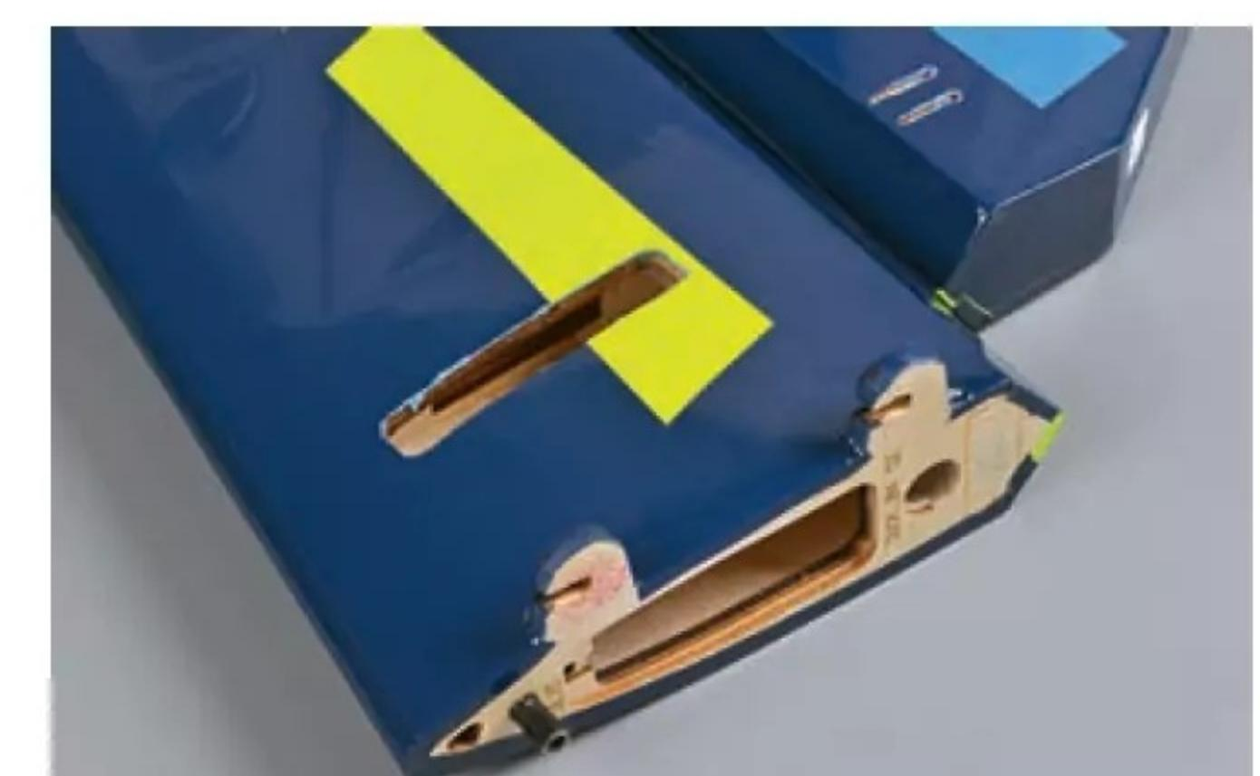
*Tailplane root showing slots for an elevator servo and dual control horns, as well as two hooks for quickly securing each stabiliser to the fuselage side.*
