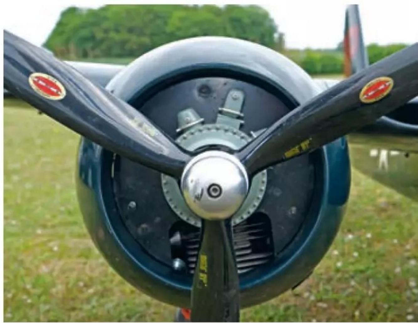
*Each of the two Zenoah ZG62 engines is fitted with a 20x10 three-blade Biela carbon prop. Note the Hamilton scale decals.*
