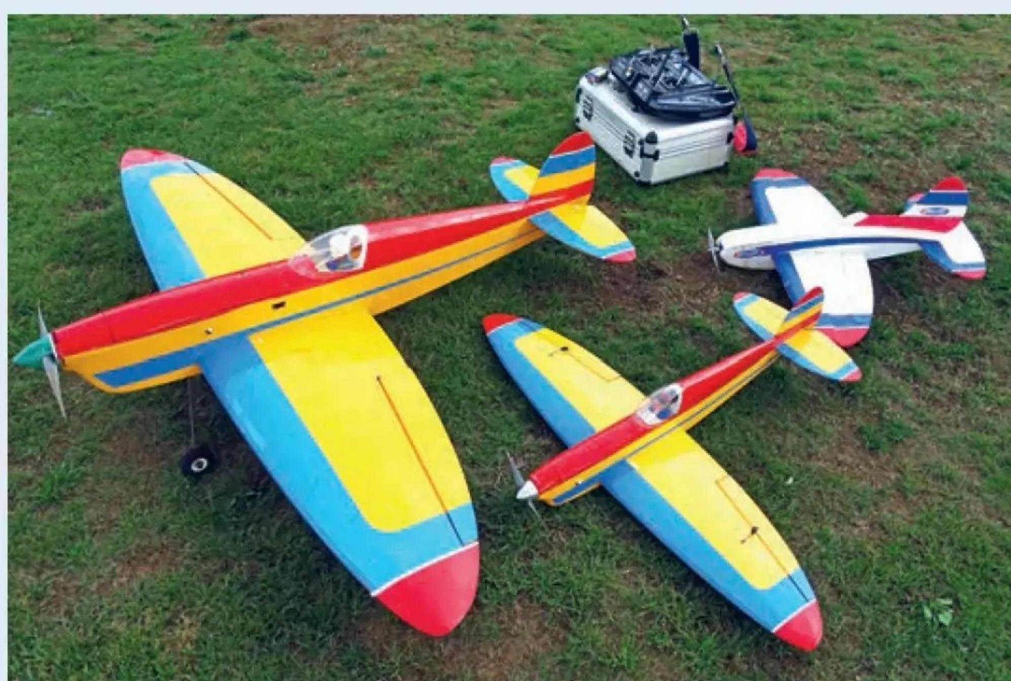
**Alan Haskell loves elliptical wings and brought along two of his own design models with trad balsa construction and film covering. The smaller one, Sprite, has a wingspan of 880 mm and flies with a 3S 1300 mAh LiPo and 2320 kV motor, either hand or dolly launched. The larger one is Big Elf with a wingspan of 1875 mm and a flying weight of 2315g, including a 5S 3700 mAh LiPo. Bringing up the rear is his foamboard 'Spitty'.**
