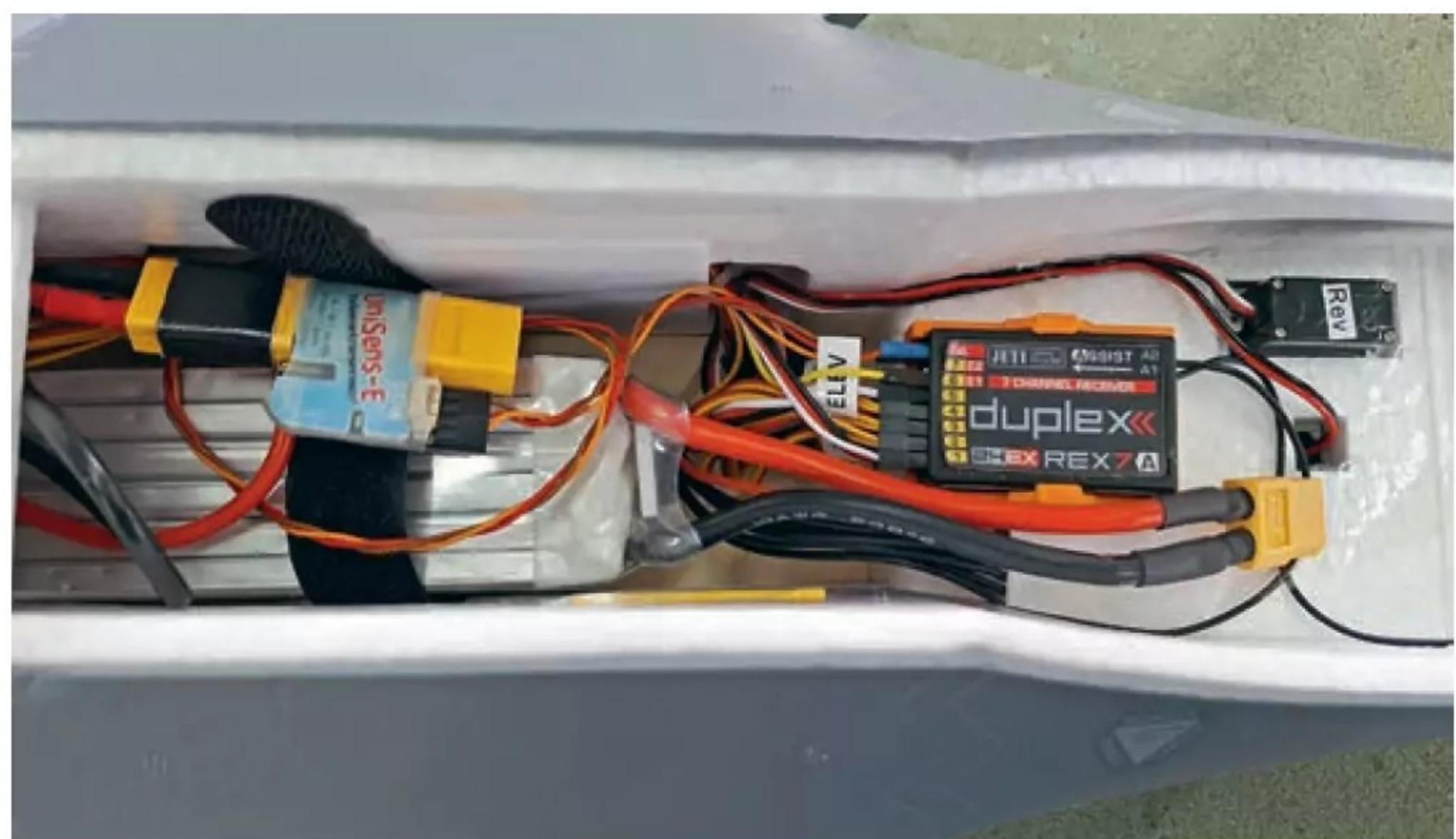
*There's plenty of room for the LiPo, receiver and telemetry sensor.*
