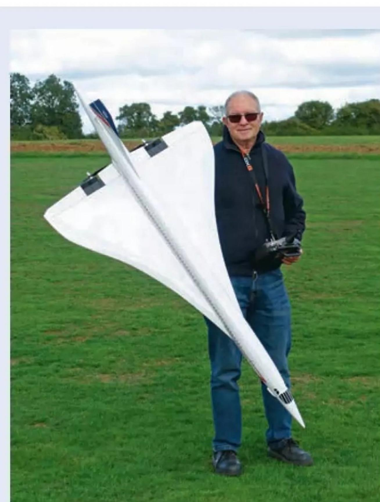
*John Given from the Chobham Common Club brought along this 32" span Concorde built from the Tony Nijhuis plan. Rather than fit EDFs, and with the help of George at 4-Max Models, John modified it to run off twin PO2834-1680 motors spinning 7x5 contra rotating props. John says there is ample power for hand launching and scale flying.*
