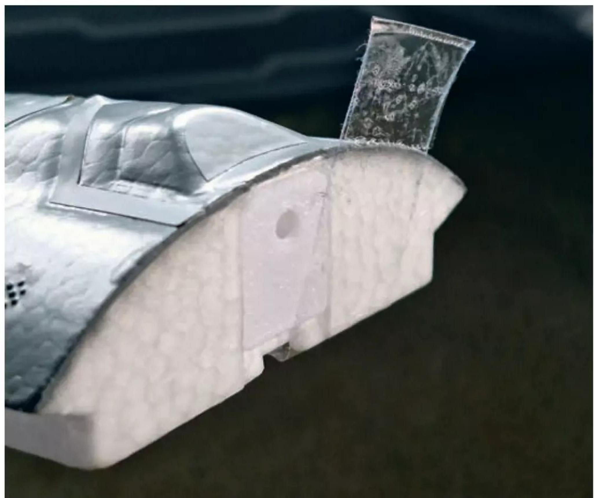
*...so I added a bit of clear tape as a handle to help remove the top hatch.*
