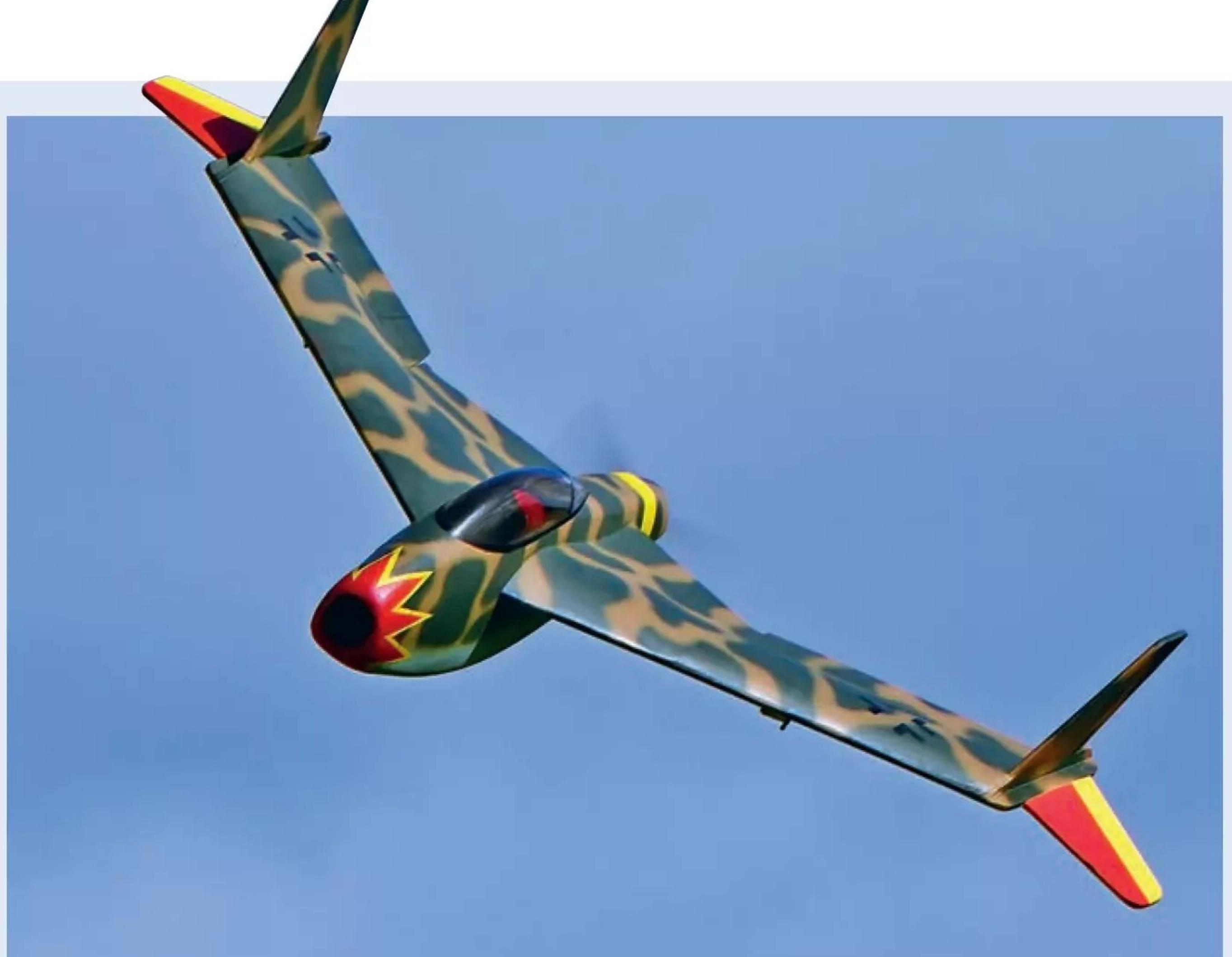
**Colin Low and his Blohm & Voss BV215 from the RCM&E free plan, February 2011. Built from Depron and balsa it spans 990 mm and is powered by a 4-Max Models Value Pack. A 3S 1800 mAh LiPo gives Colin around 20-minute flights, including plenty of vertical performance. That colourscheme was inspired by a giraffe!**
