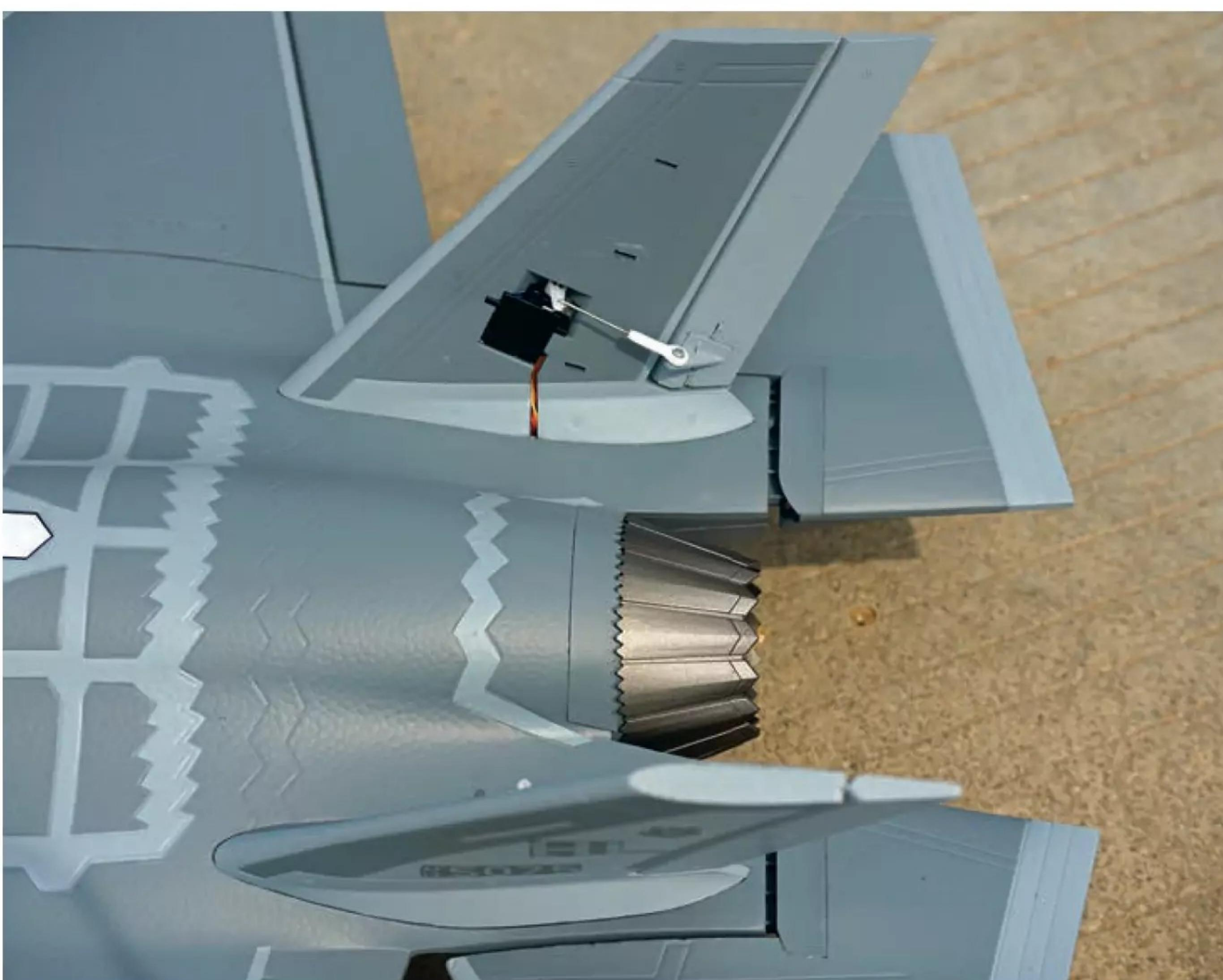
Twin fin and thrust tube details.
