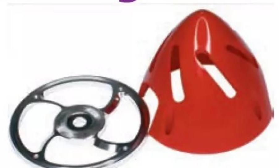
These ultra light weight spinners for electric motors are supplied with a specially cut aluminium backplate (like a propeller) which pulls cooling air through the nose of the spinner and then forces it out of the back and in to the motor, helping keep the motor cool even on a hot day.
