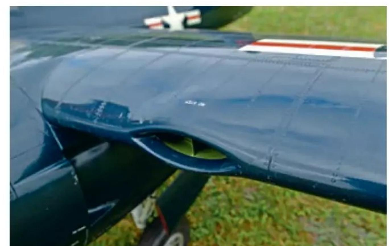
Inlets either side of the engines were ram air intakes for the elliptical air coolers fitted to full size aircraft.
