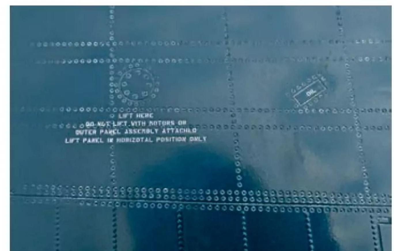
Close up on some of the neat rivet and panel details on one of the wing skins.
