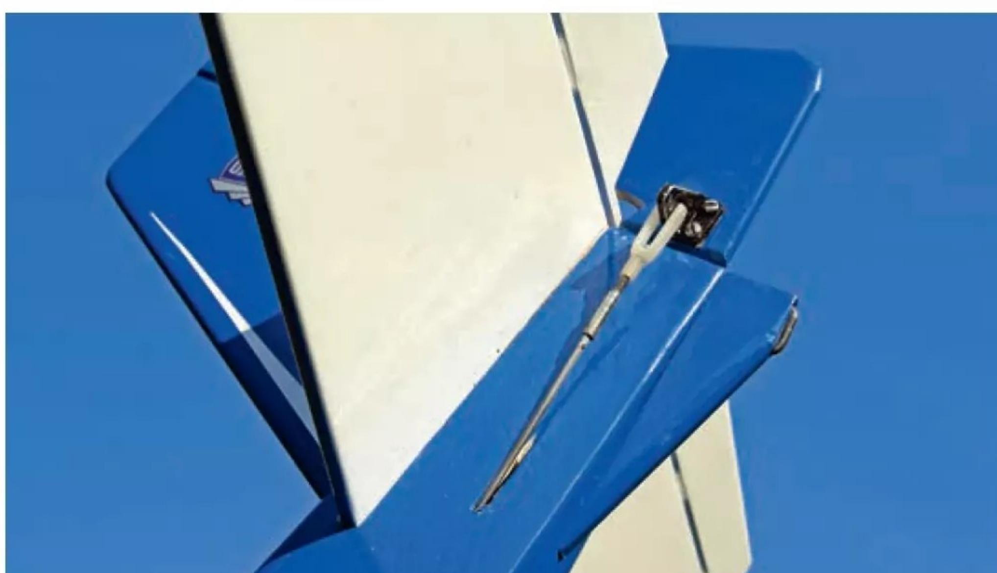
**Rudder pushrod required a small offset bending into the wire rod to achieve correct alignment.**
