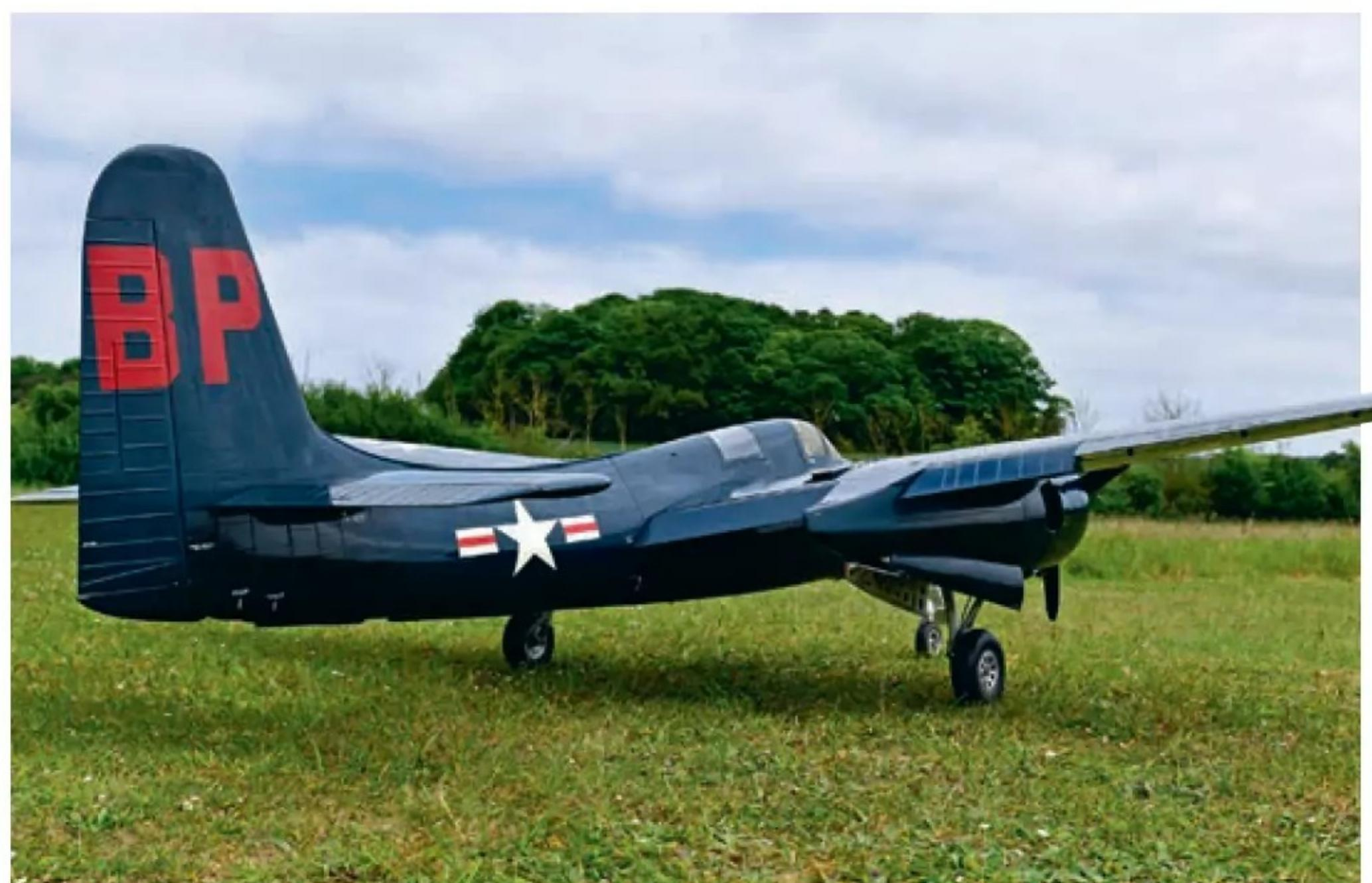
*The large fin and rudder can cause an easily controllable yaw in a crosswind but otherwise she flies straight and true.*
