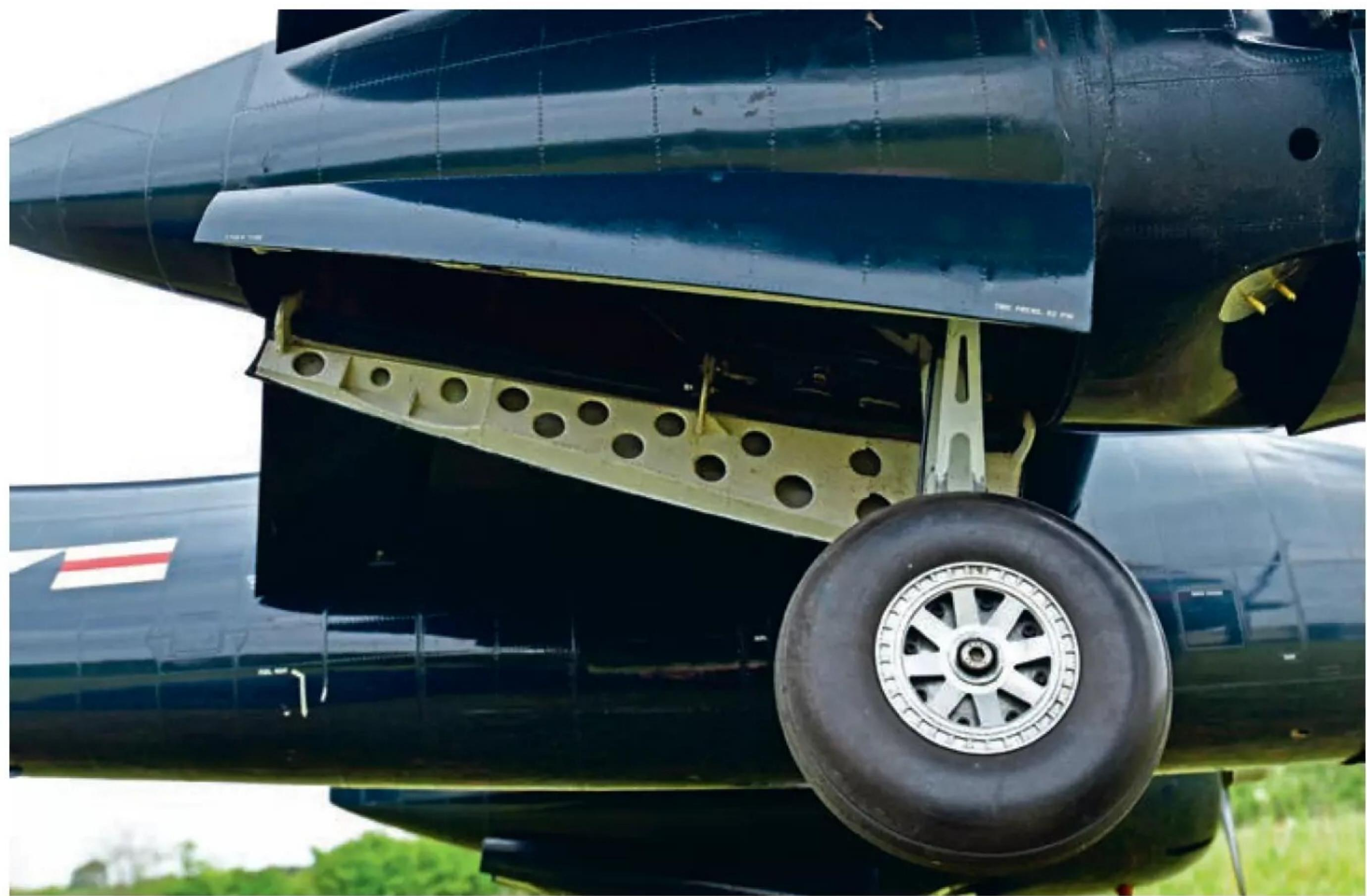
*Model raised off the ground to show one of the HAWE pneumatic retracts with its sequenced doors.*
