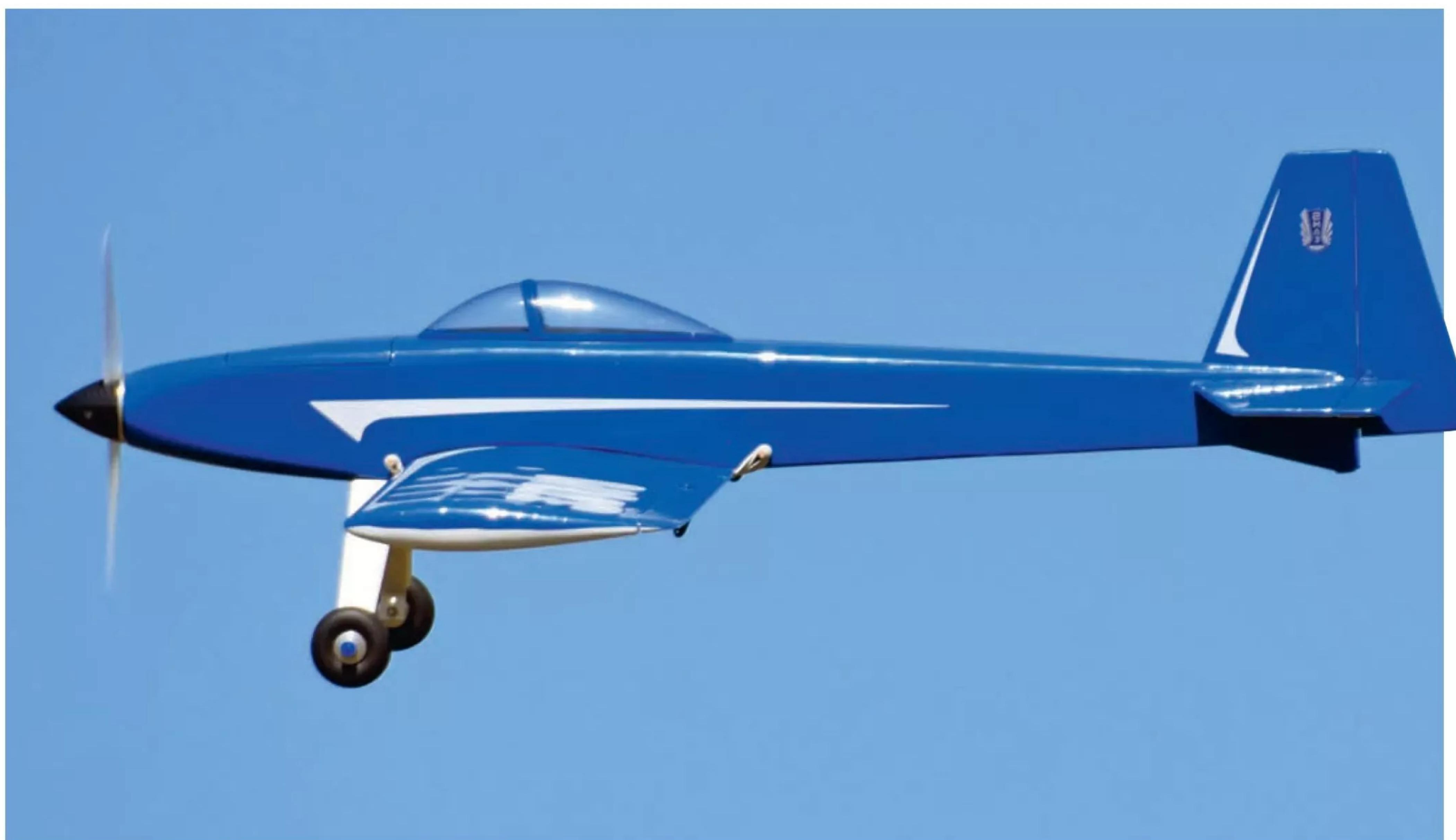
Just a touch of down was needed on the test flight, but it was expected as the CofG was slightly rearward of the indicated point.
