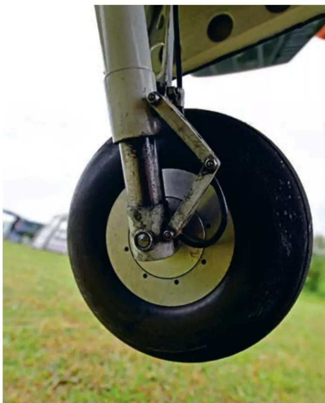
*The undercarriage is fitted with scale hubs, with pneumatic brakes on the main wheels.*
