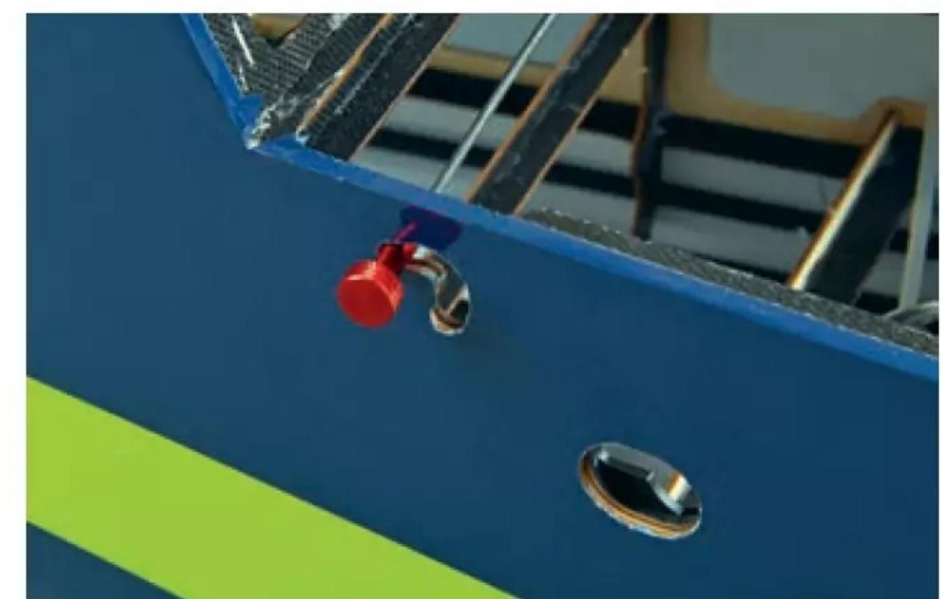
*...and a sprung wire rod at the back. The knurled button slots into a hook protruding down from each side of the canopy.*
