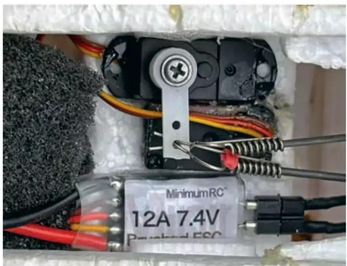
I fitted a larger servo arm on both the elevator and ailerons.
