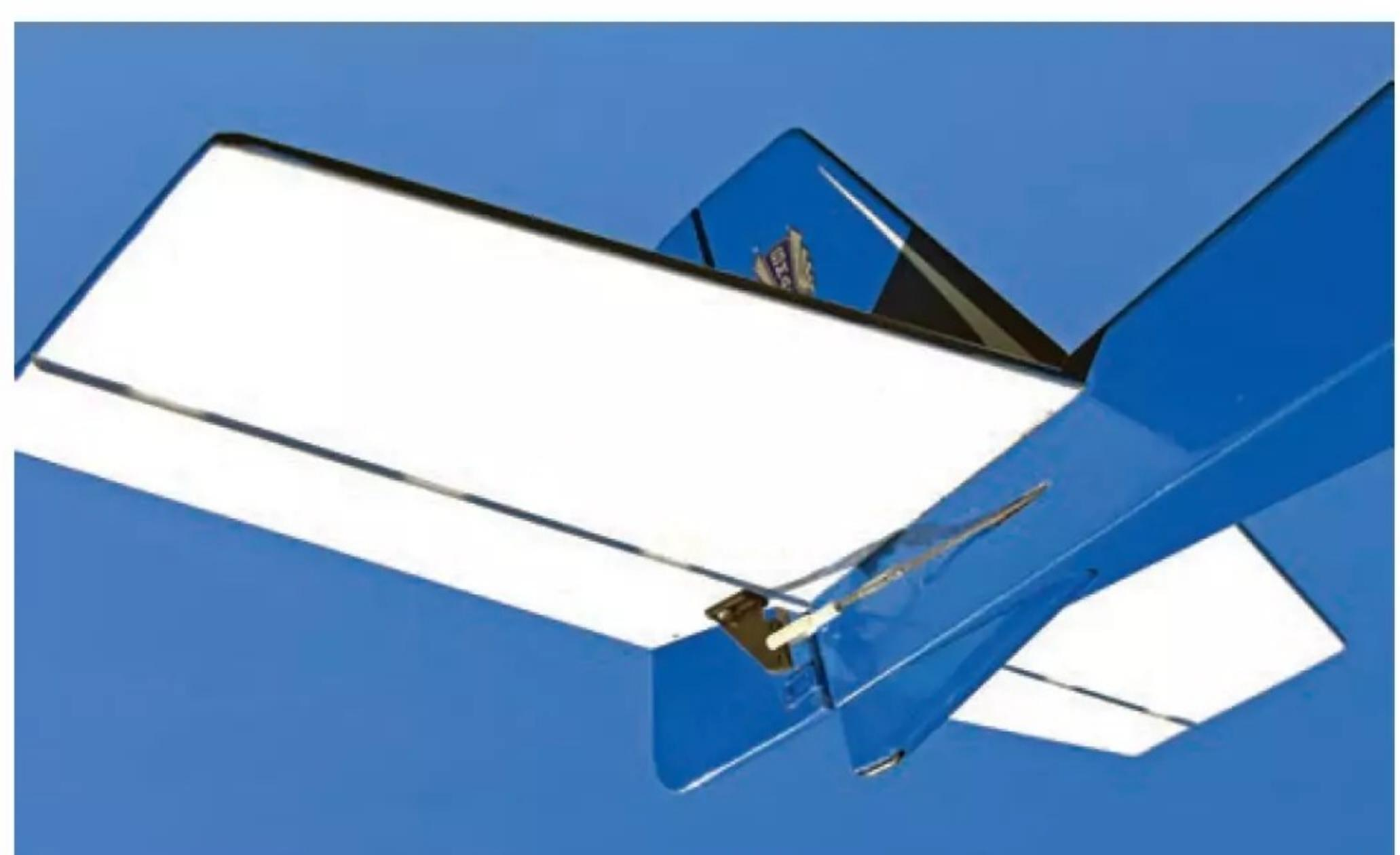
**Again, elevator connection is direct and friction free.**
