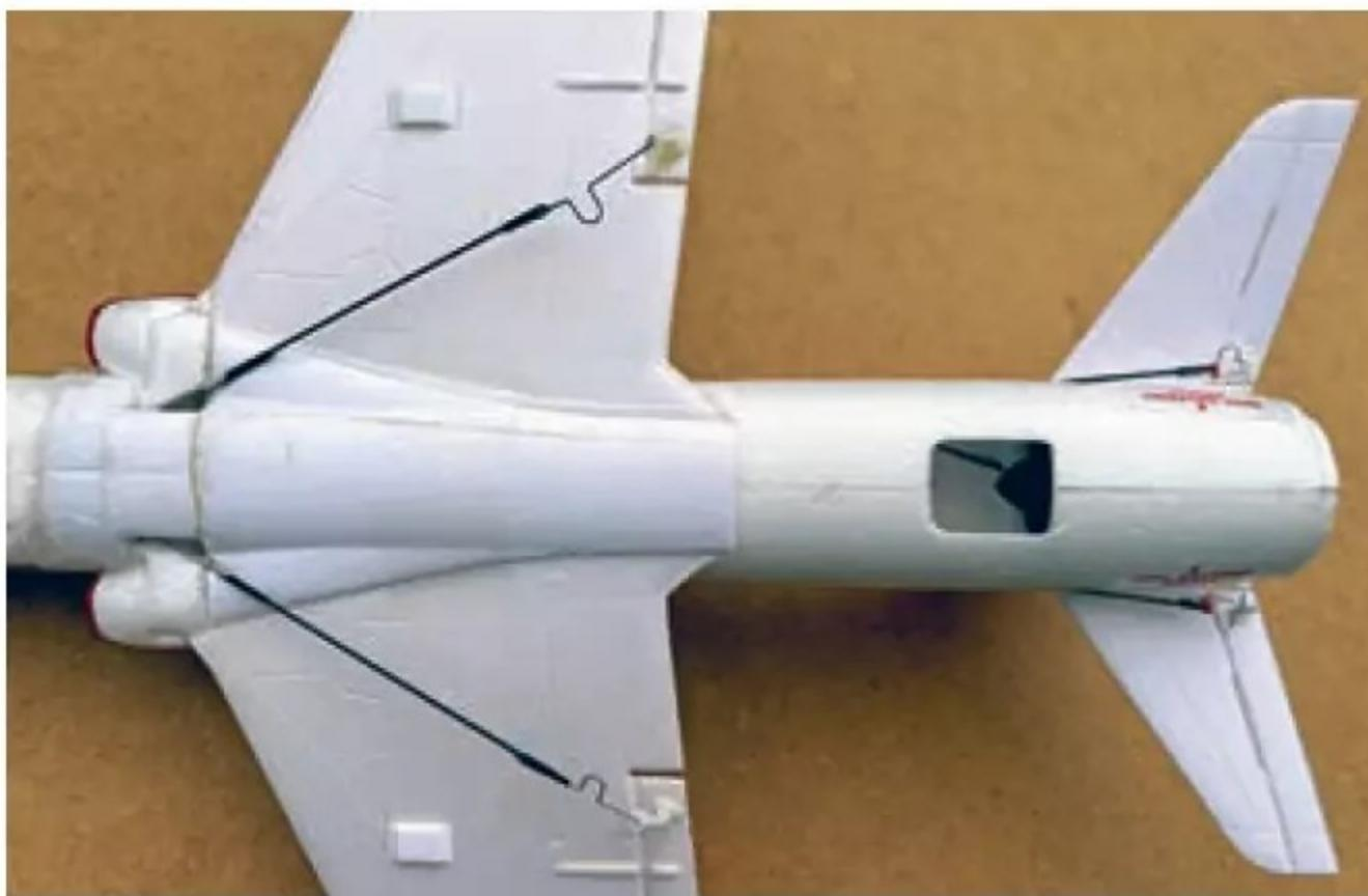
The model uses a small 'cheat intake' right in front of the EDF unit.
