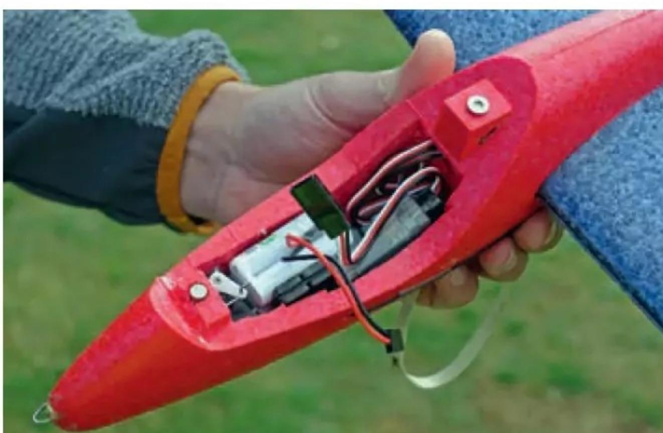
*Nick hollowed out the nose of the Lidl glider to accommodate the R/C gear. Note the simple 'disappearing pin' tow release in the nose.*
