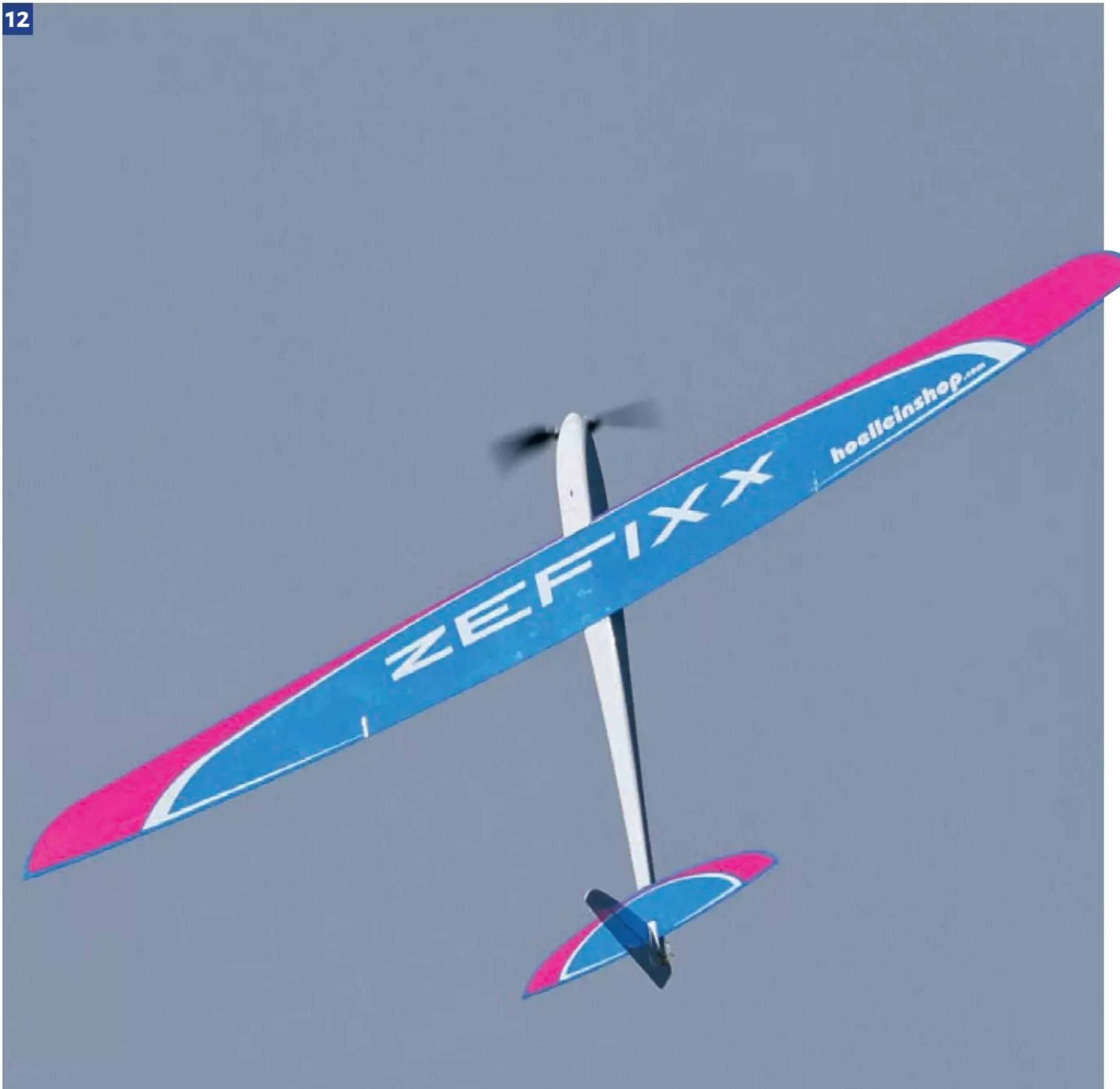
laser-cut kit, including an electronic retractable landing gear. Zefixx (pictured) is a mini hotliner with a one-piece plywood covered wing and a wingspan of 1.47 m controlled via ailerons, elevators and motor. Optionally, the model can also be fitted with a rudder.
