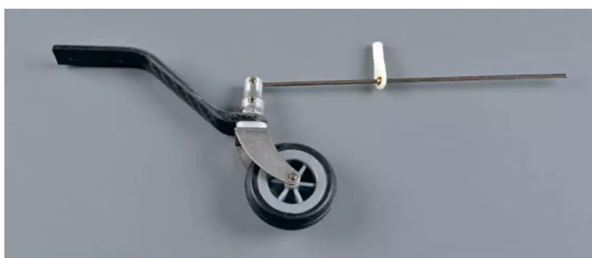
The steerable tailwheel was an area which stopped me in my tracks when building the Extra. The ball link is supplied separately so I didn't realise that it was meant to be slid onto the rod and fixed in a hole in the underside of the rudder. Easy when you know how but puzzling without any instructions!
