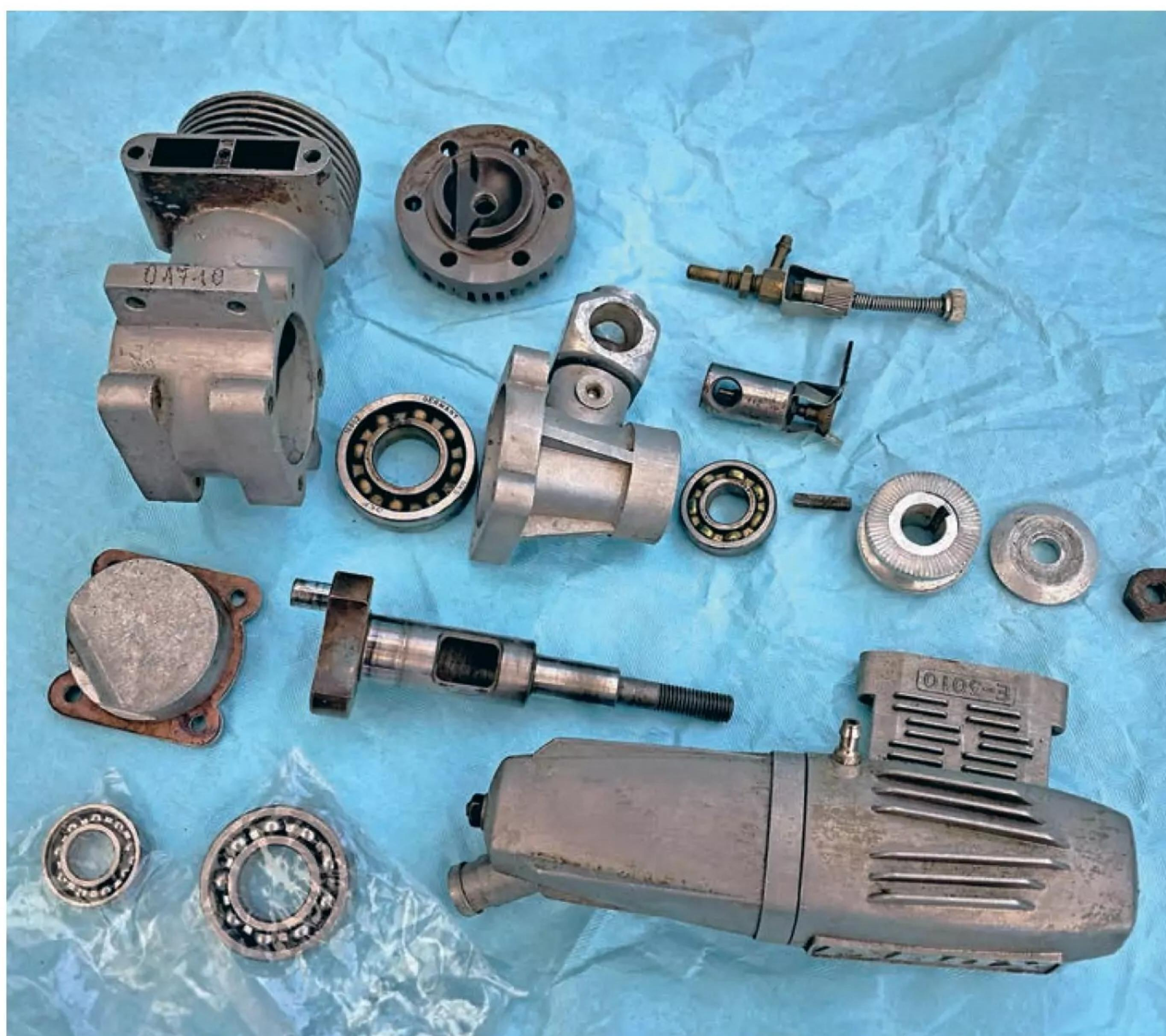
All good solid stuff here, the big Webra awaits its reassembly. The new bearings stayed sealed until the last moment before fitting.
