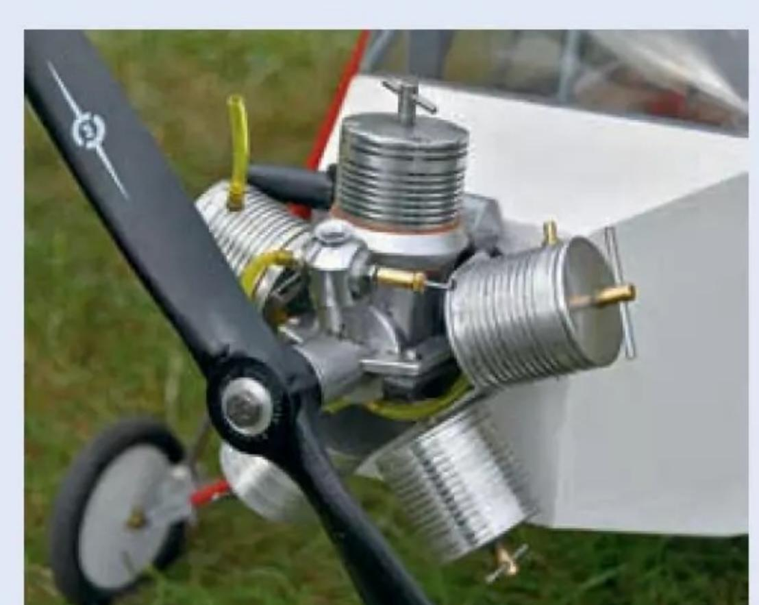
Close up of the larger R.17 five-cylinder engine. See text for details.
