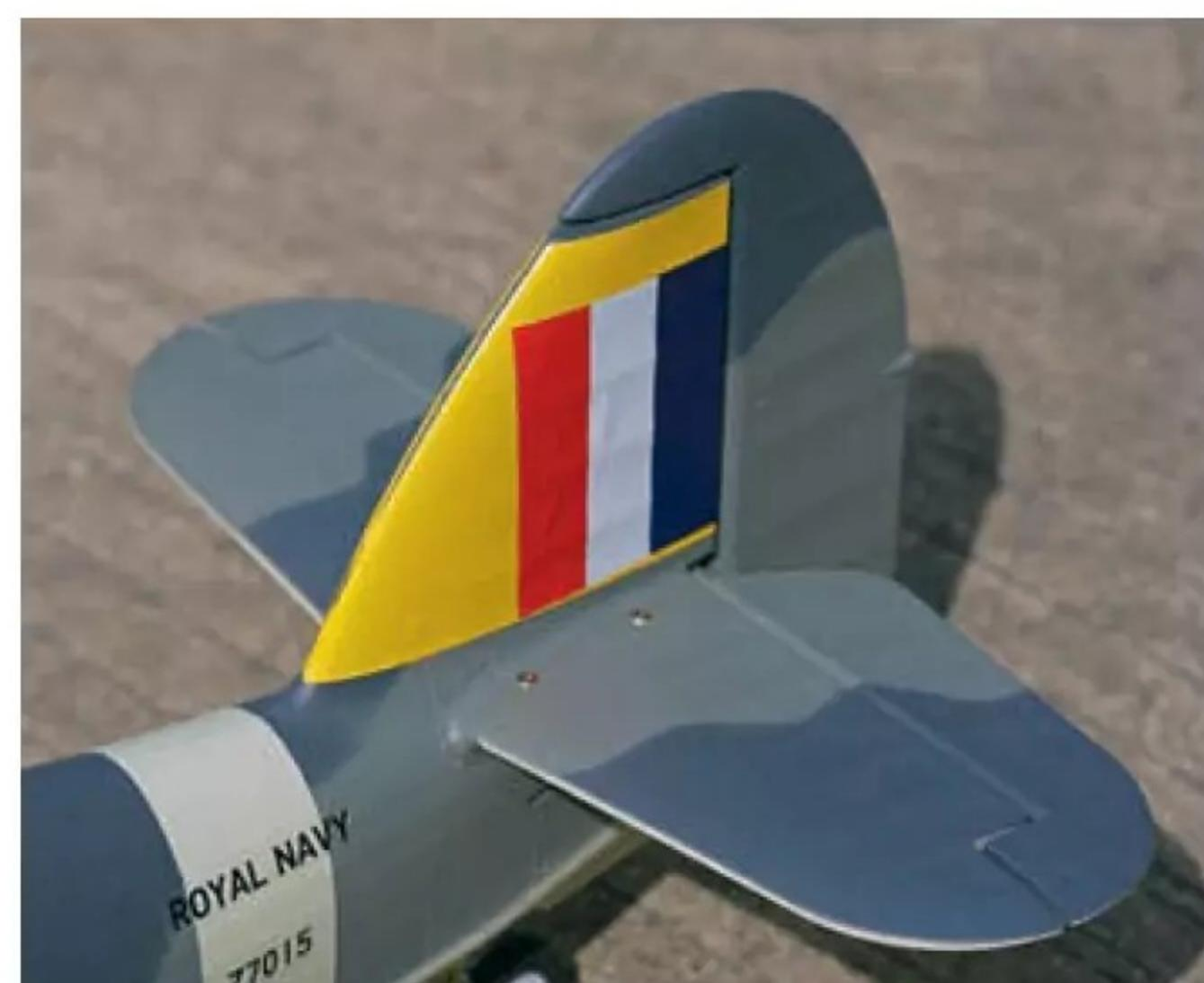
Assembly starts by sliding each stabiliser half into cuffs on either side of the fin and securing with short hex headed screws.
