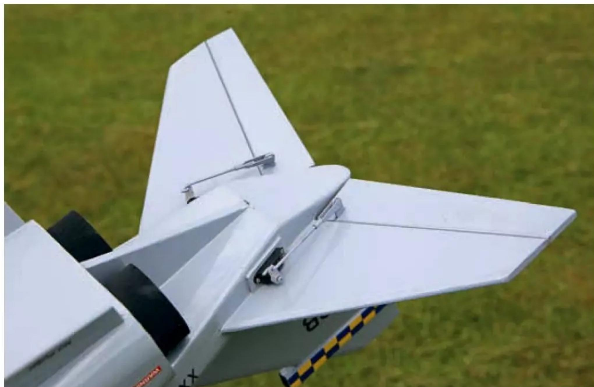
**Elevator linkages are commendably short. Note also the ply doublers to reinforce the servo openings.**
