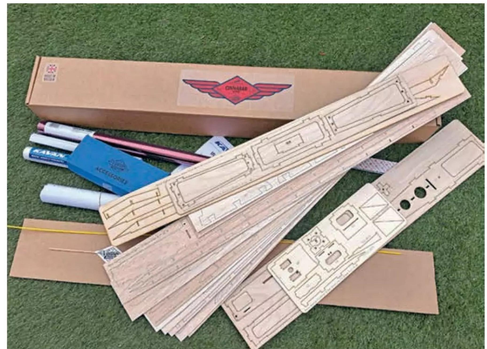
That's a well filled box! Cinnabar kit is very complete, right down to the two rolls of Kavan covering film.
