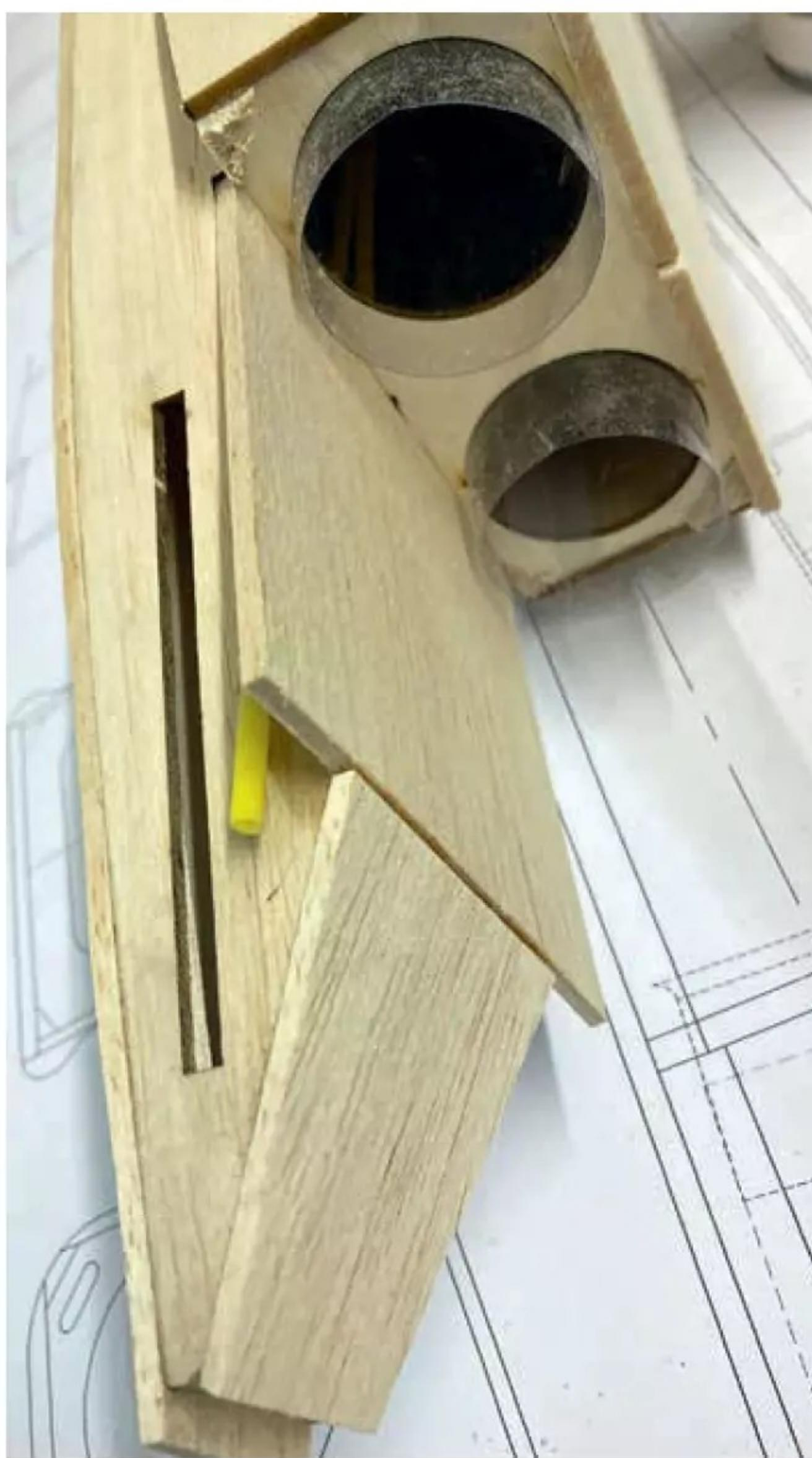
**Sheeting the rear end of the fuselage prior to shaping.**
