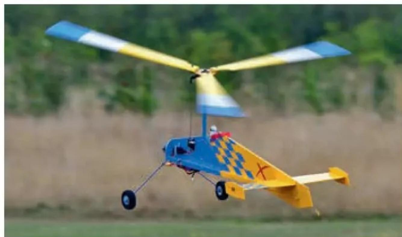
Rich Harris' prototype gyrocopter called 'Whippet X'. 1100 mm rotor, 4-Max PO-3535-1090 kV motor, 11x5.5 prop, 40A ESC and 3S 2200 mAh LiPo. Rich is experimenting with moment arms and tail areas. You just can't keep a good designer from trying new things!
