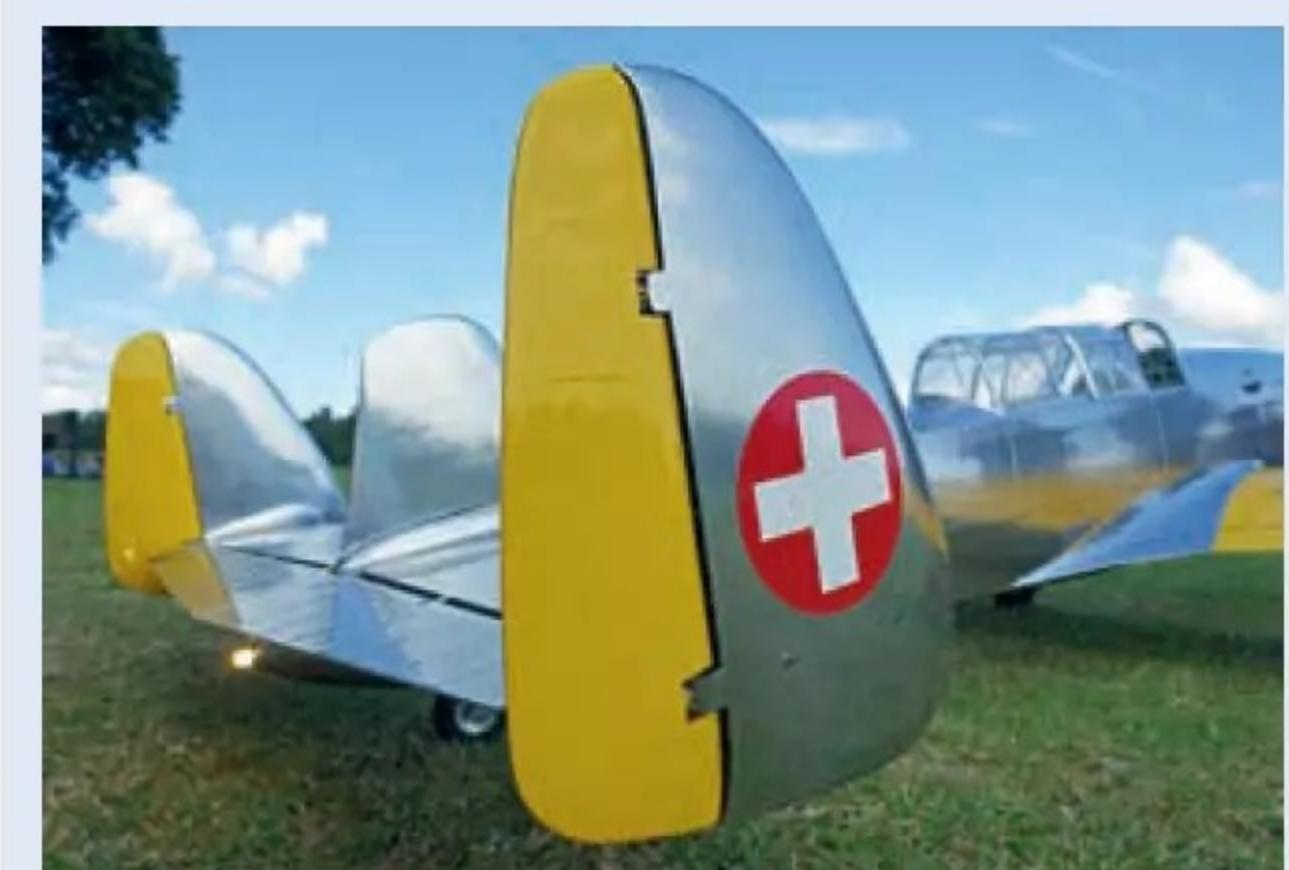
A central tail fin was added to the C-3603 airframe to compensate for the longer nose of the C-3605.
