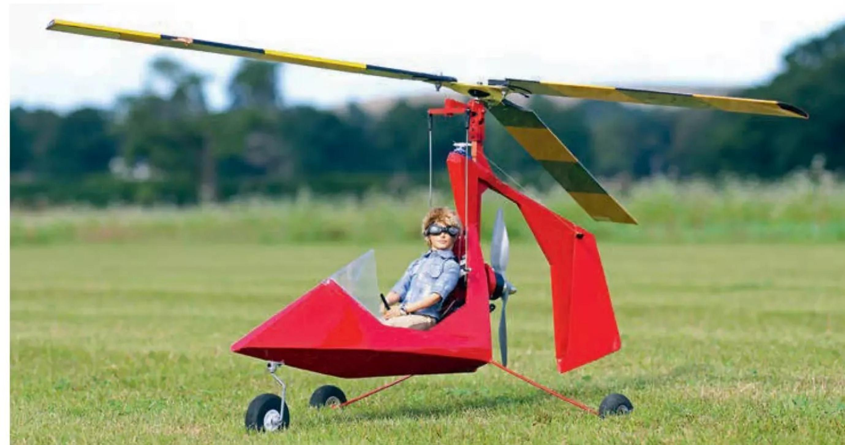
*My Elfpusher is another experimental model investigating the use of a top mounted tail boom. Not a single curve in sight!*
