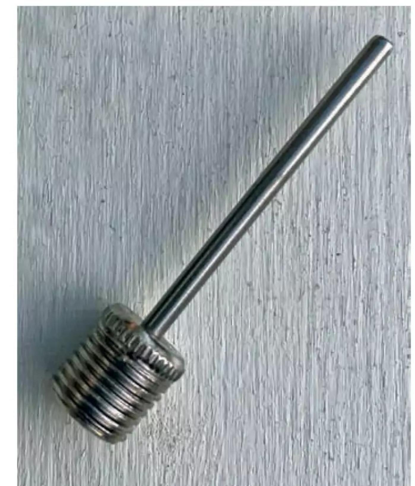
The kit comes with a tyre inflation nozzle which needs to be inserted into the valve to release some air.
