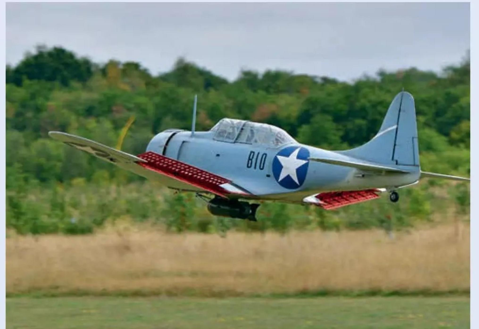
Split flaps on the Dauntless are actually dive brakes which pilots used to eliminate tail buffeting during dive bombing targets, most notably during the Battle of Midway in June 1942.
