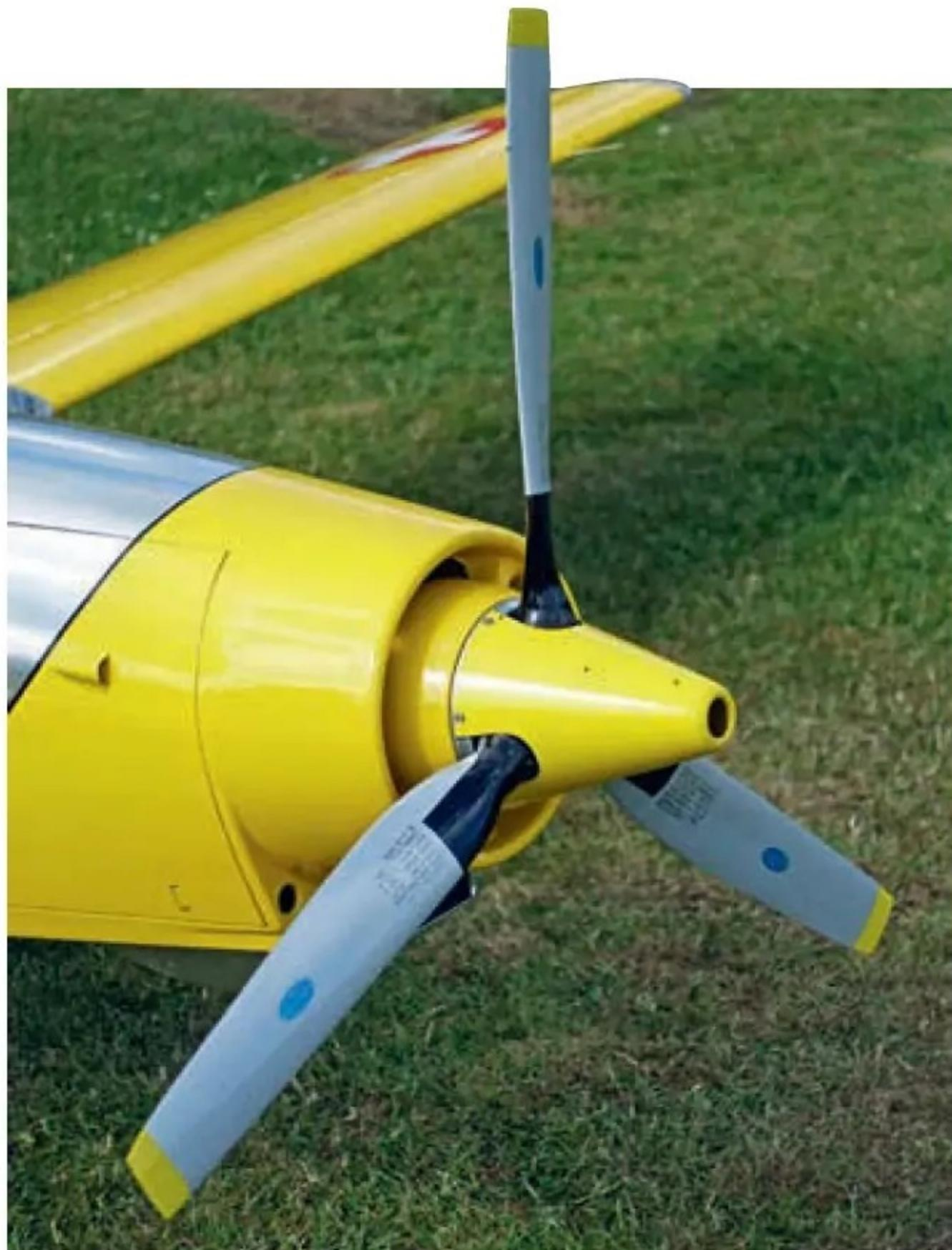
*The 32" diameter Ramoser 3-bladed varioPROP 32i has a variable pitch which, after flight testing, has been set at 17".*
