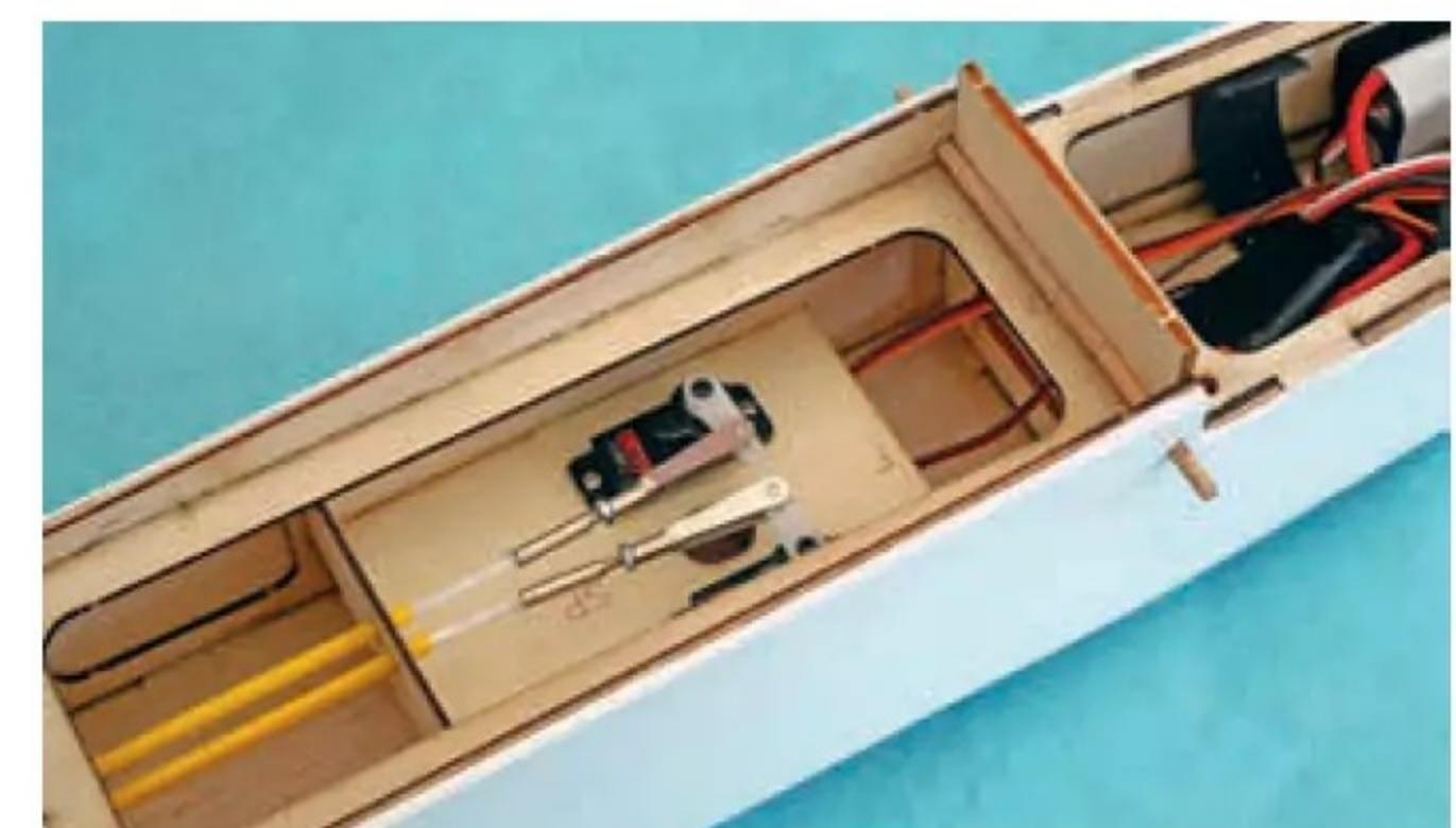
*Servos are simple to fit and access for adjustment. It makes finishing the model that much easier.*
