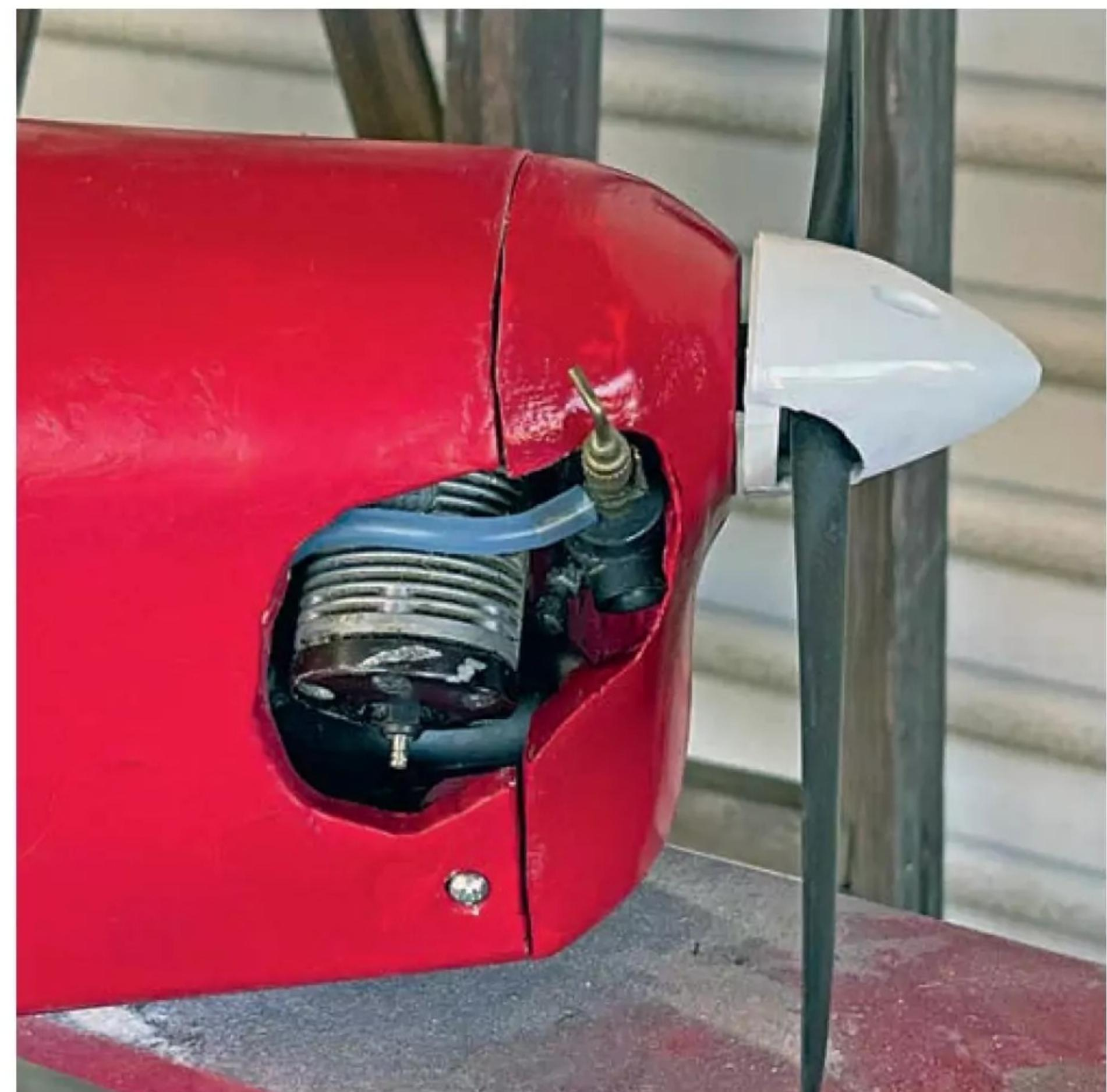
I solved the problem by replacing it with a 1.1/2" spinner. Hardly noticeable, but it fits the prop. Just.
