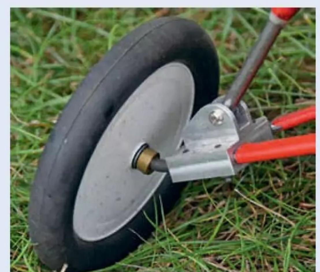
Tim model has functioning telescopic suspension using internal springs. He made the aluminium bracket on his recently acquired mini milling machine.
