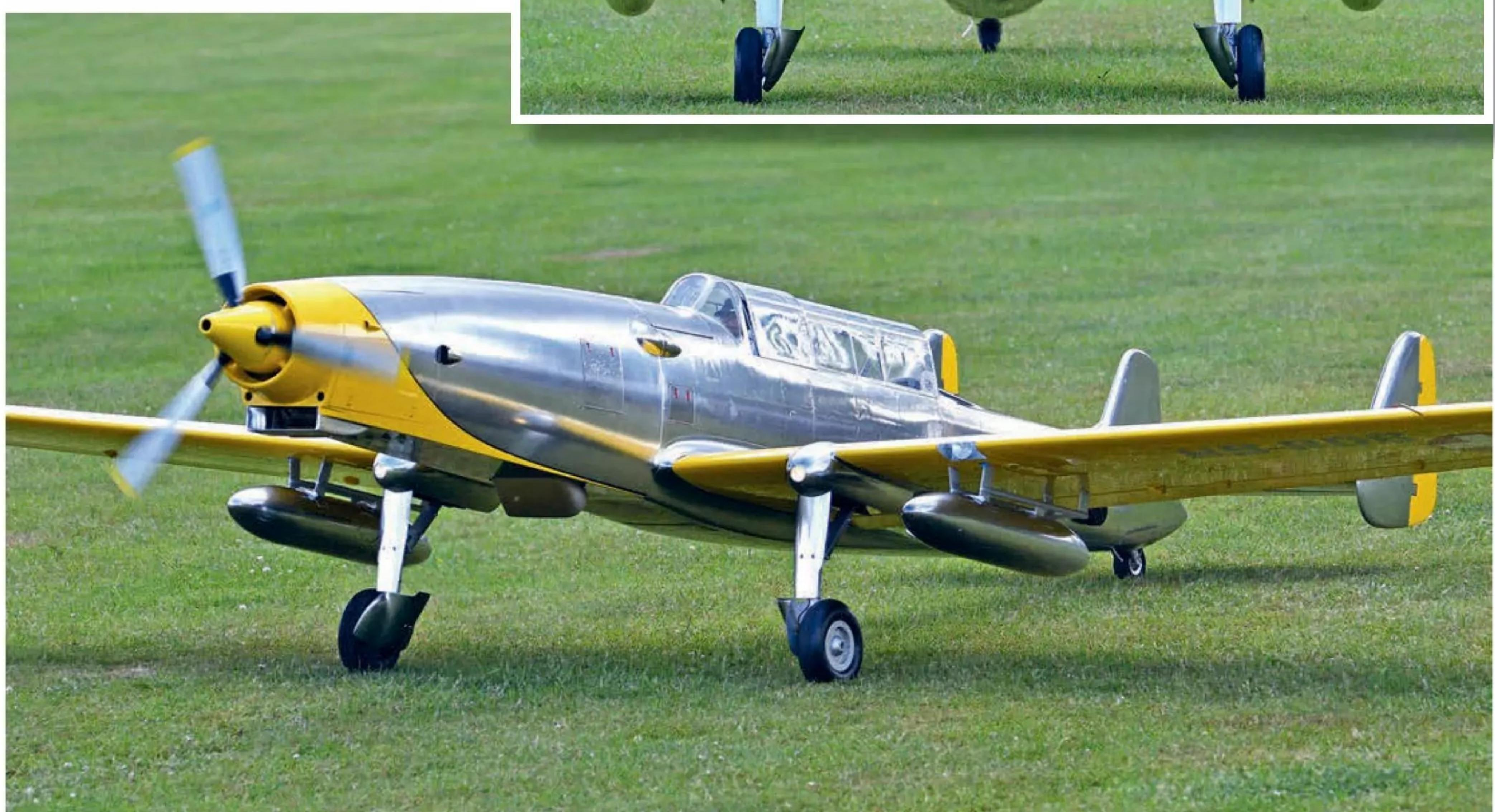
*Note the vertical joint line just in front of the wing LE. This is where the long fuselage splits in two for transportation.*
