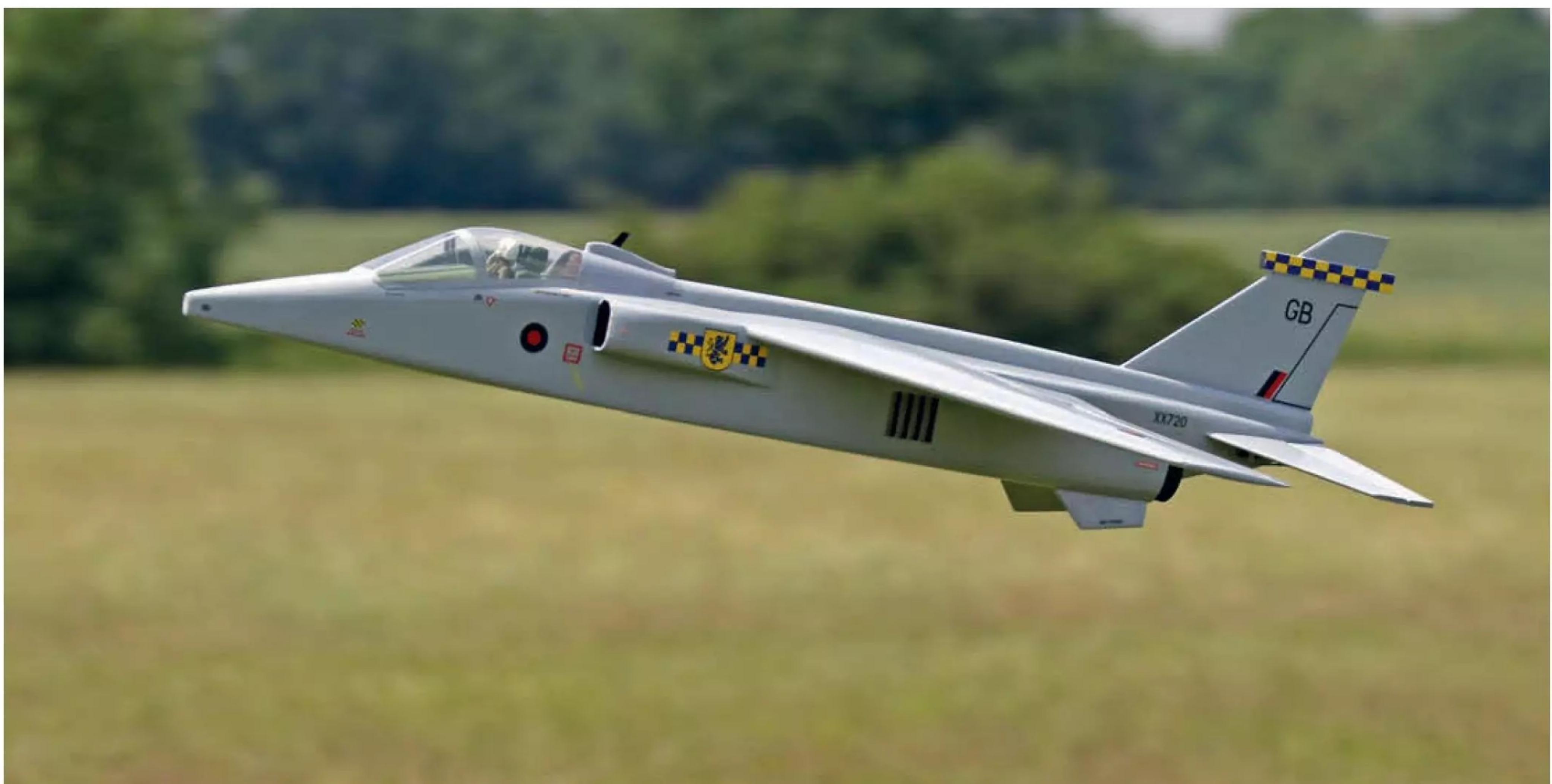
*The wing is effectively a delta with anhedral and as such the model will cope with a bit of high alpha.*
