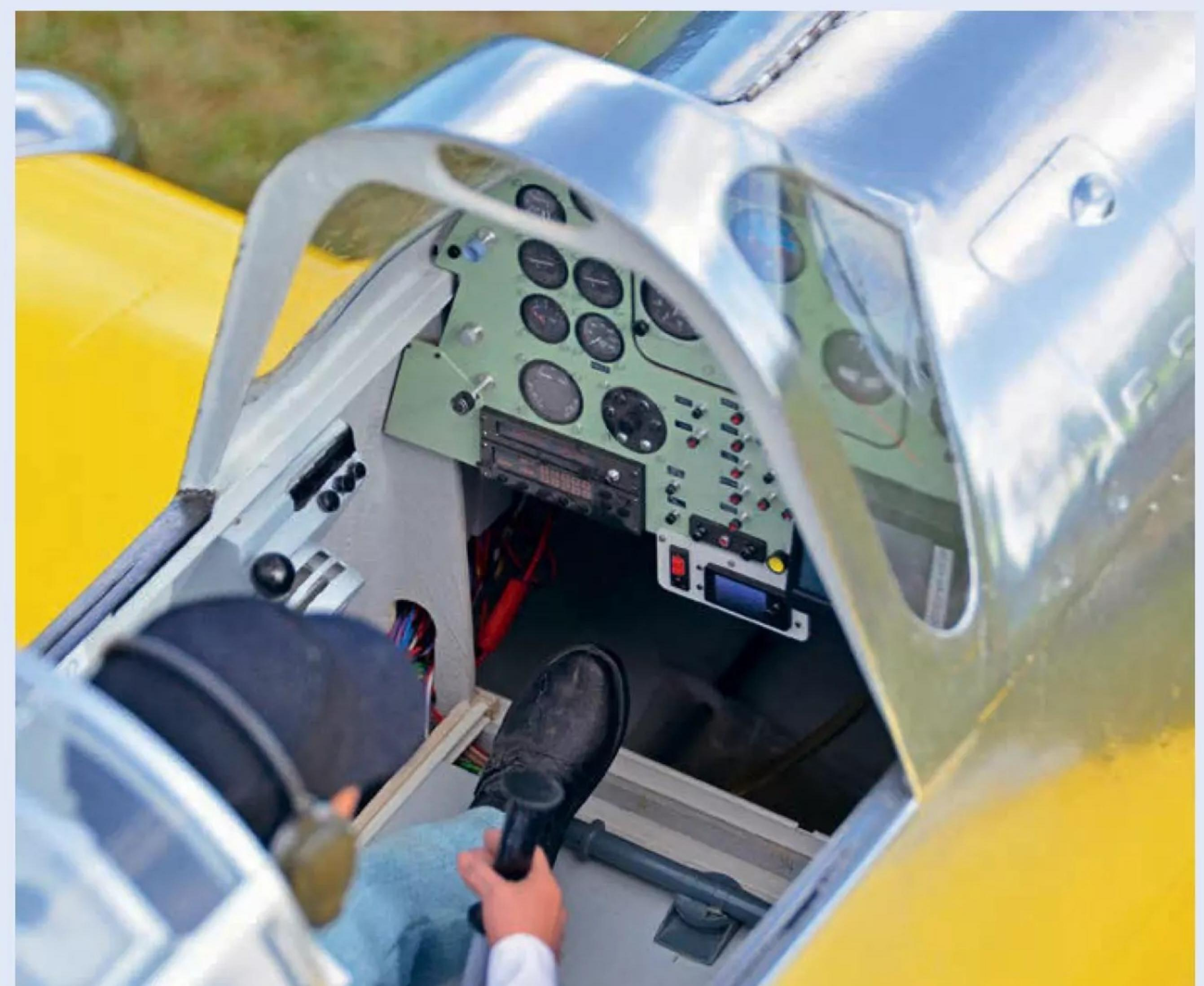
*The cockpit canopy is servo operated. At the flick of a switch it slides open to show some of the detailing Thomas has added to the model.*
