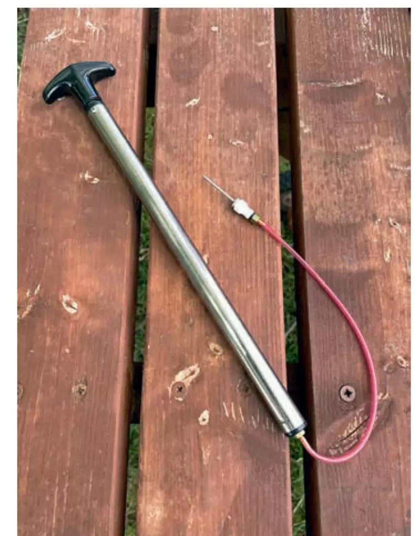
My old retract pump has found a new lease of life after being fitted with the air-wheel inflation nozzle.
