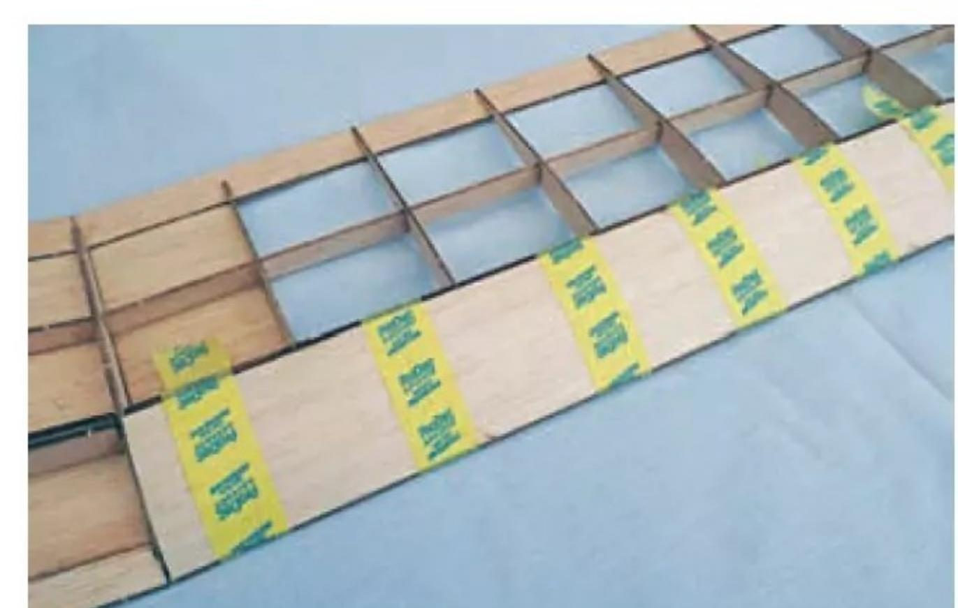
**Sheeting the wing is simply done using 'low-tack' tape to keep it all in place. Be absolutely sure to identify and fit the slightly angled wing root end of the sheet correctly.**
