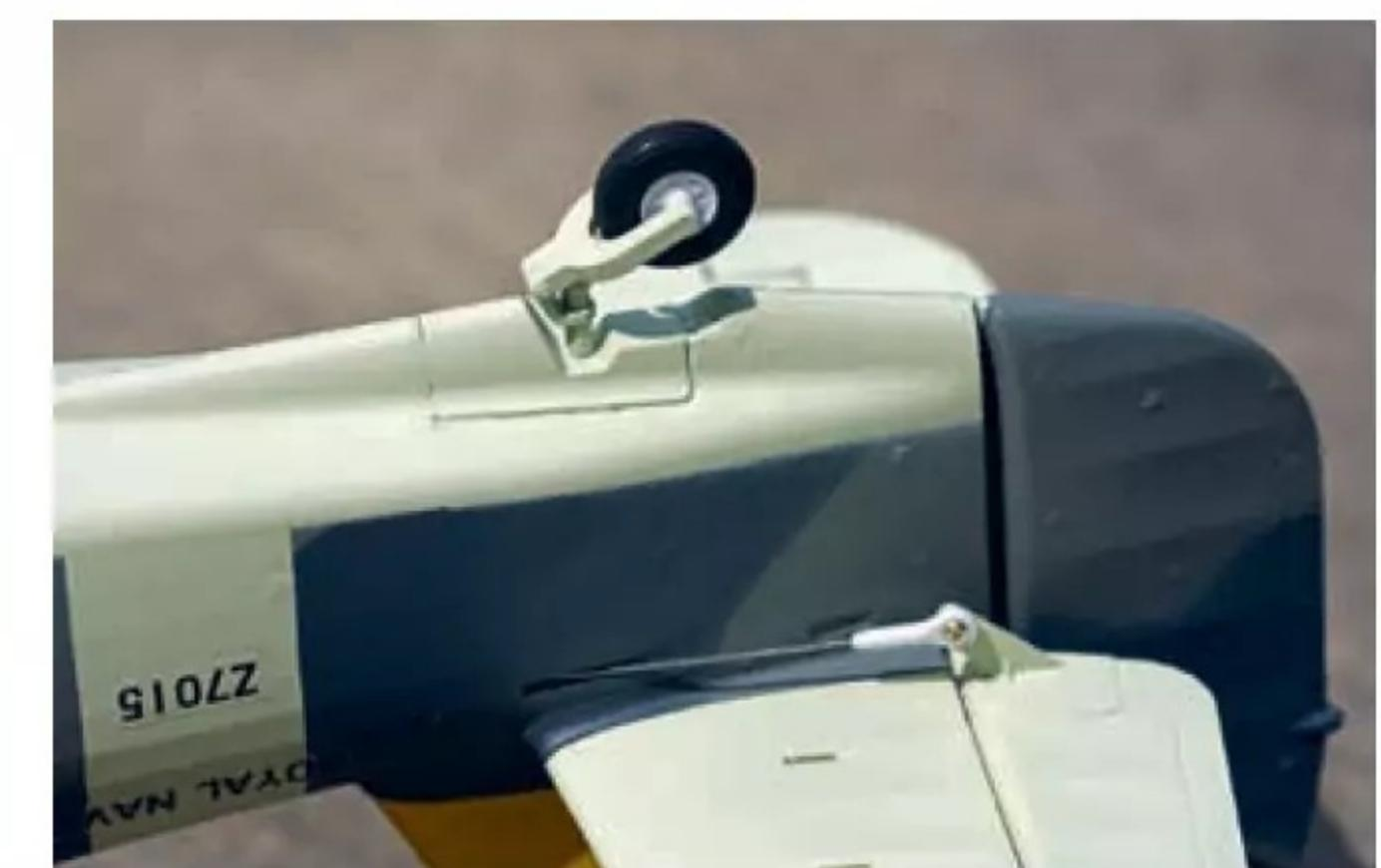
The scale effect continues at the back with a steerable yoke mounted tailwheel.
