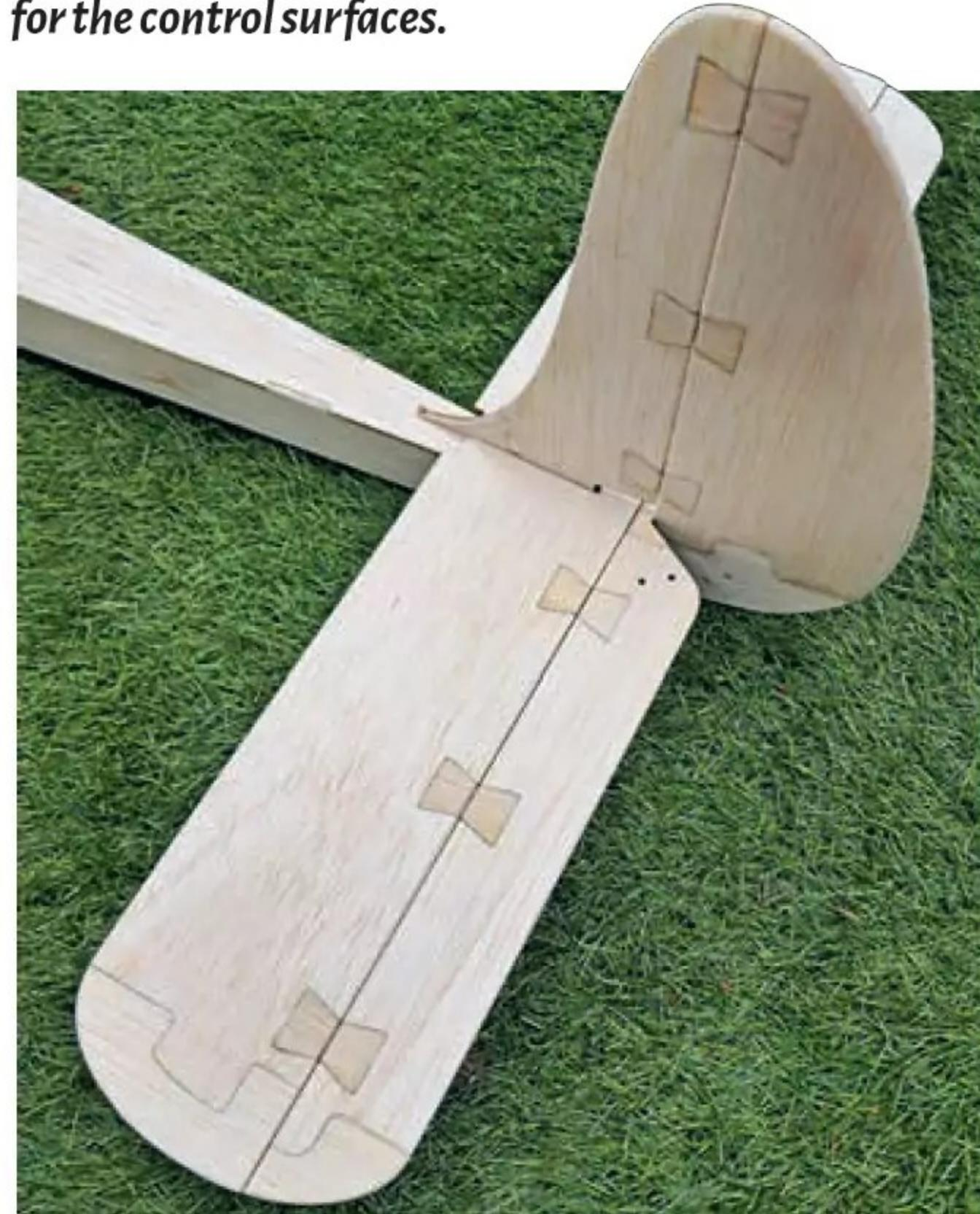
**Covered over hinge points are neat and tidy but be sure to sand all surfaces flat before covering.**
