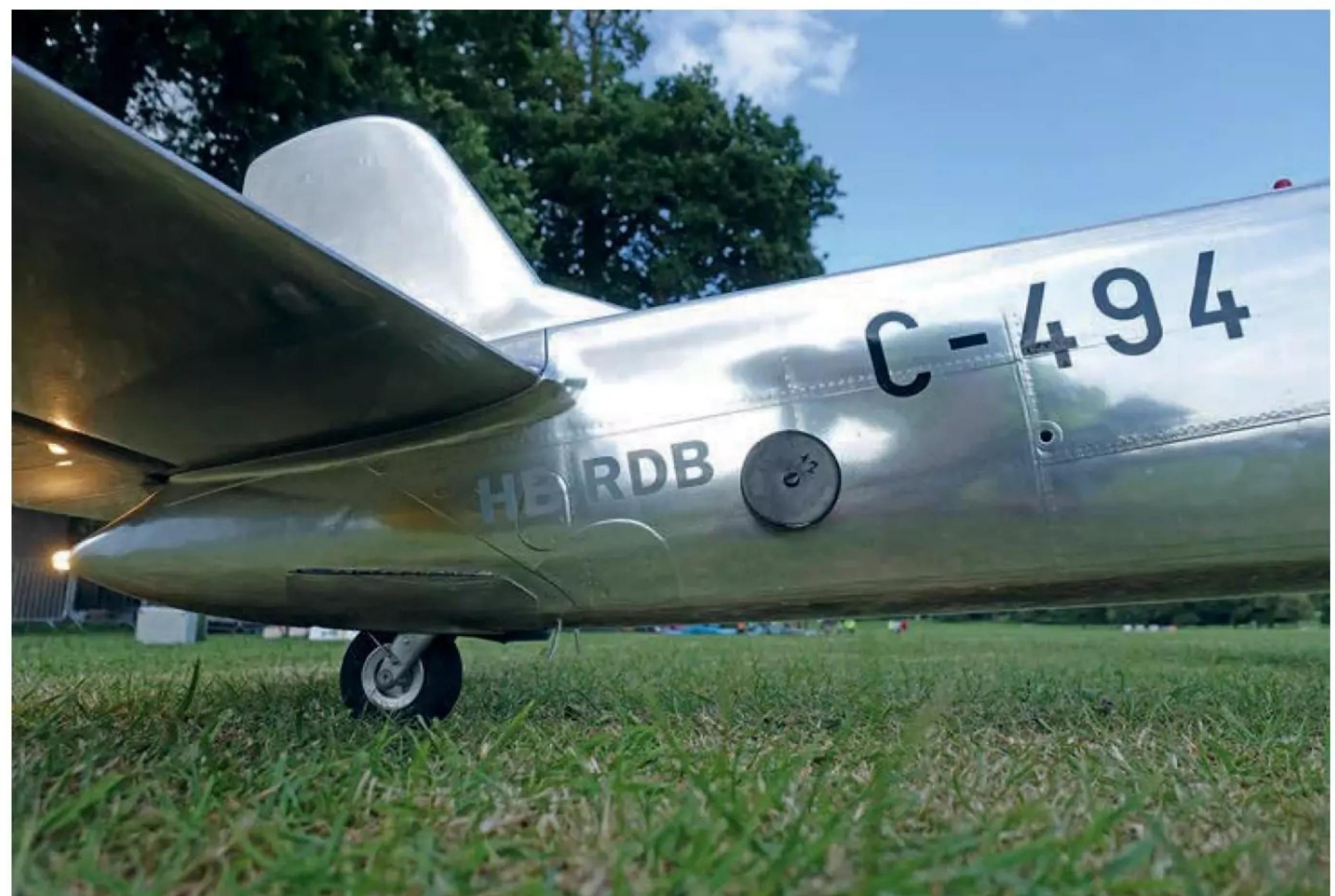
That curious black disc is ballast that the full-size needs when the rear machine gun or target towing winch are removed. Thomas took advantage of this feature to counterbalance the turbine engine in the model's long nose!
