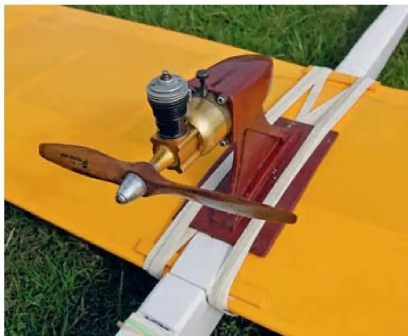
*I'm not looking for high performance, just enough to get my gliders to altitude. For that my favourite Pro-Synth glow fuel is fine. But for a high revving performance I would recommend using a fuel with castor oil as it has a higher flash point. I'm only using a 10% nitromethane content but with higher content fuels these little engines really can come alive.*
