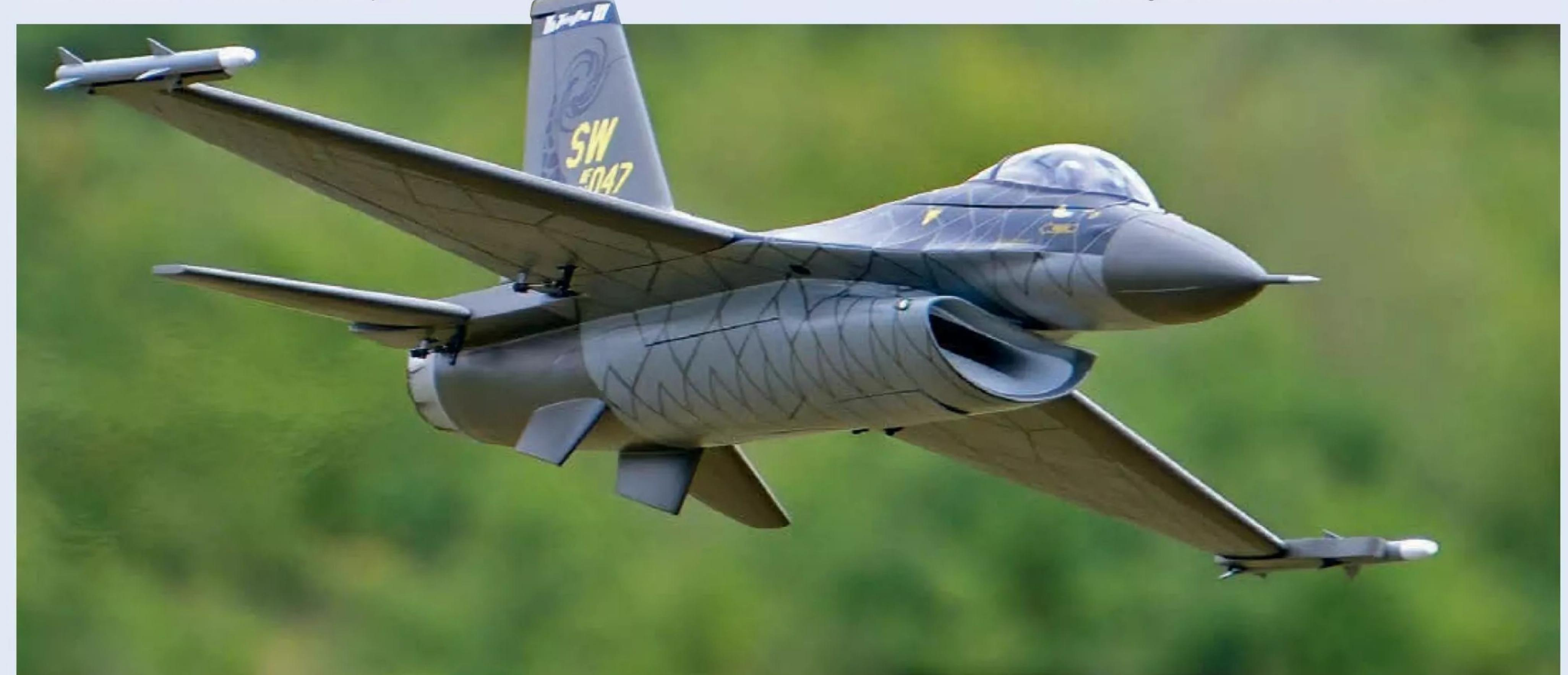
The underslung air intake meant that a lot of grass cuttings got sucked in during take-off but, thankfully, the KingTech K-86 turbine has a built in FOD screen for such eventualities!
