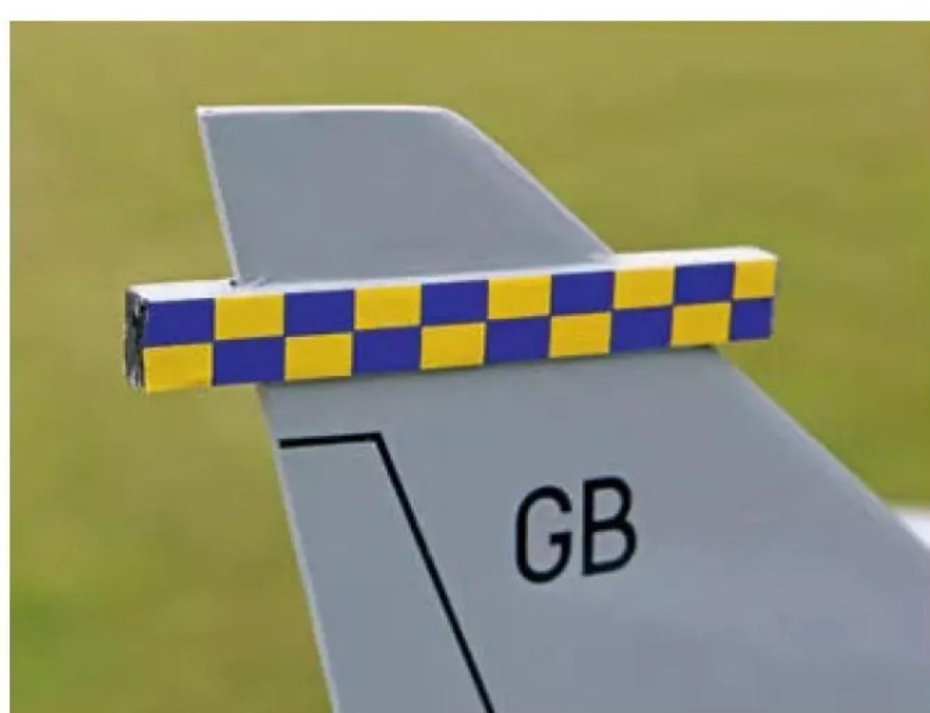
*Fin mounted Radar Warning Receiver housing is a distinctive feature of the Jaguar...*
