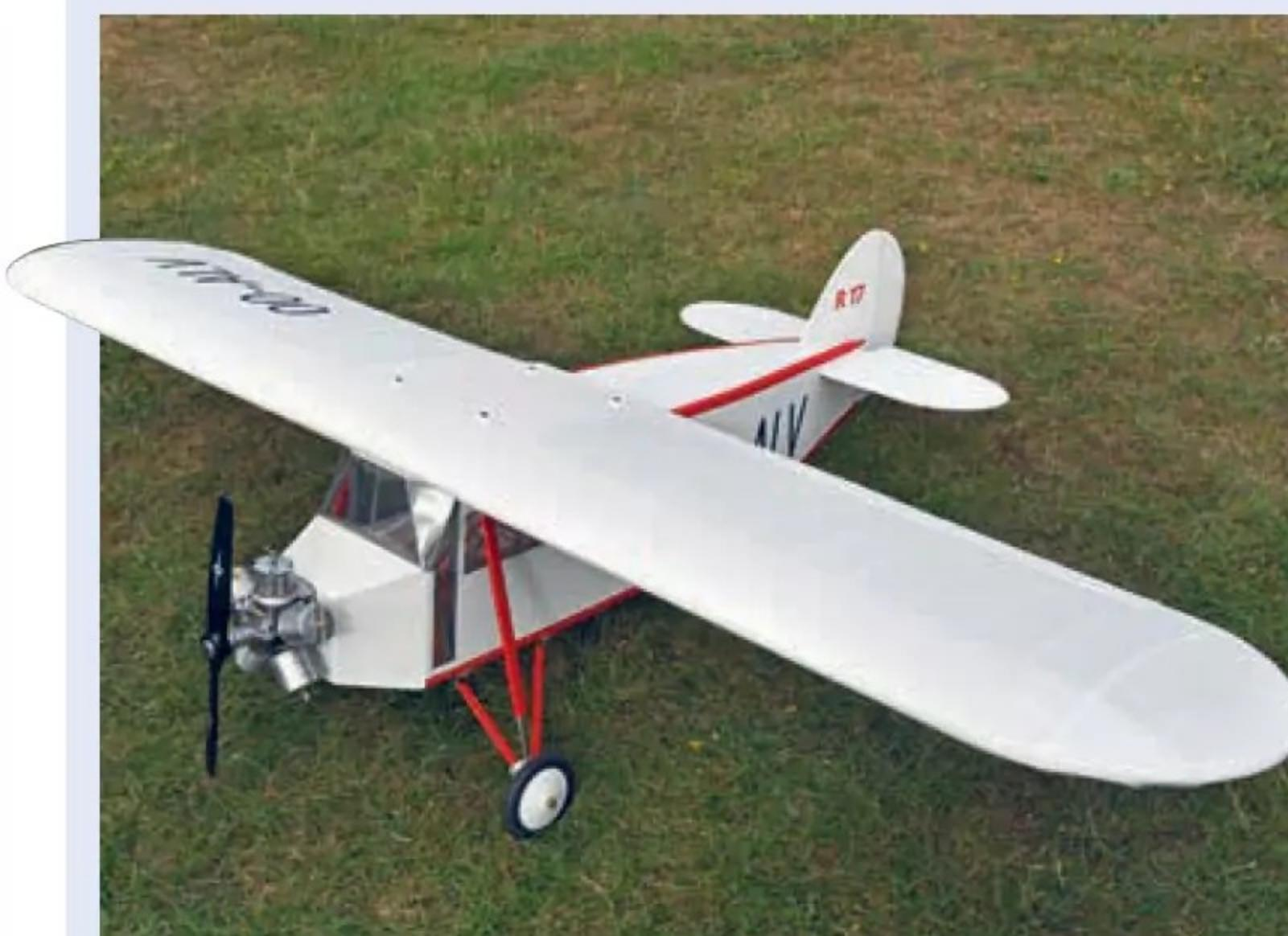
Tim's model of the Belgian designed Renard R.17 with novel, for the period, cantilever wings with no struts!
