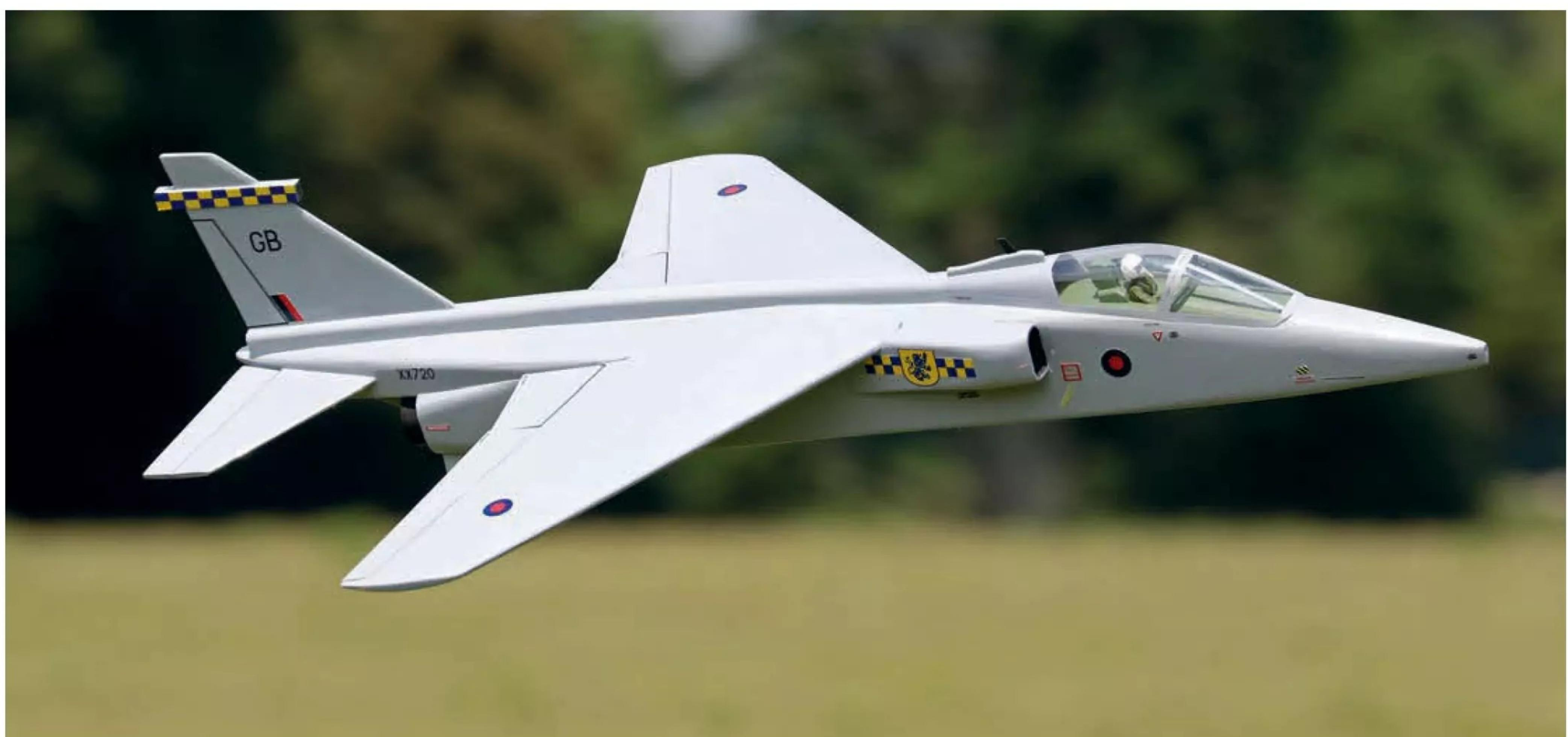
*The prototype was covered using light grey Oracover and painted parts were covered in corresponding Orapaint.*
