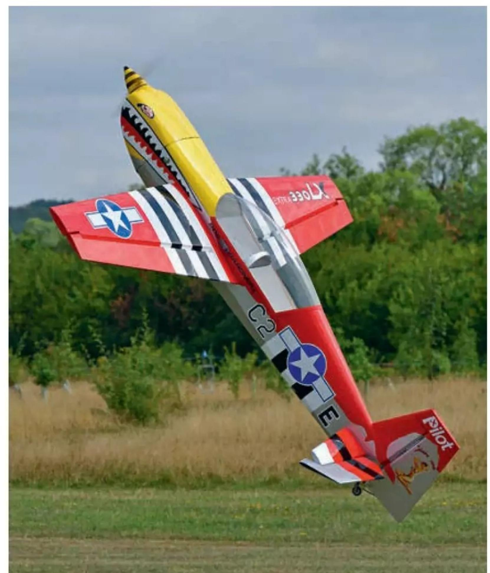
Rob Gardner's Pilot RC Extra 330. The DLE55 engine and 23x8 prop pulled it through the 3-D manoeuvres with ease. 89" span and PowerBox gear.
