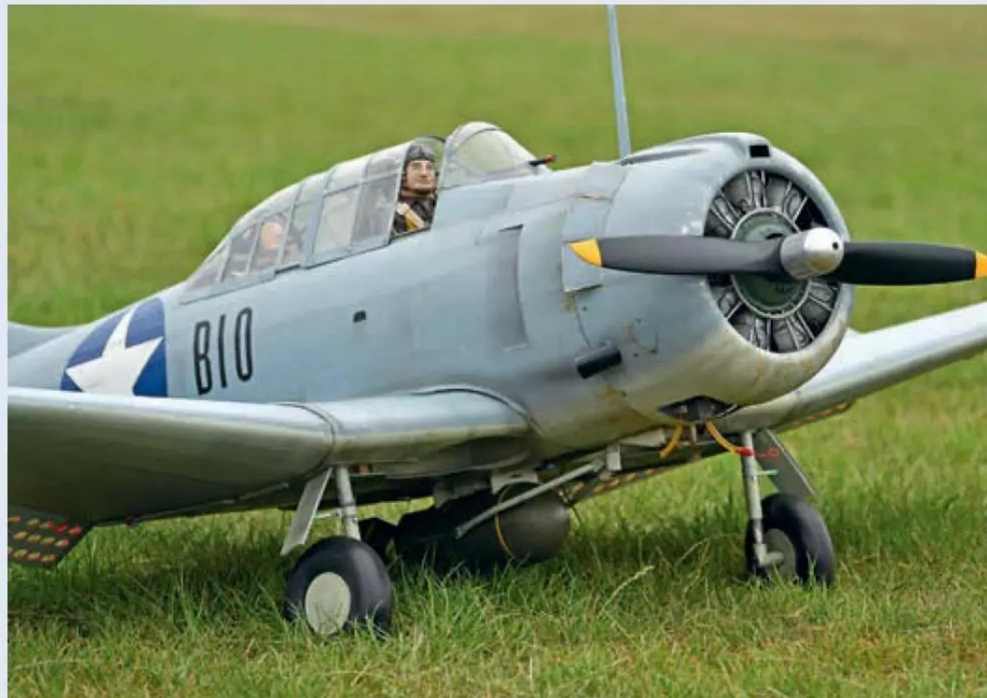
Close up of Adam's club-mate, Stewart Lunny's scale detailing and weathering on the Dauntless. The dummy 9-cylinder Curtiss Wright Cyclone radial hides the Zenoah 74cc Twin engine perfectly.
