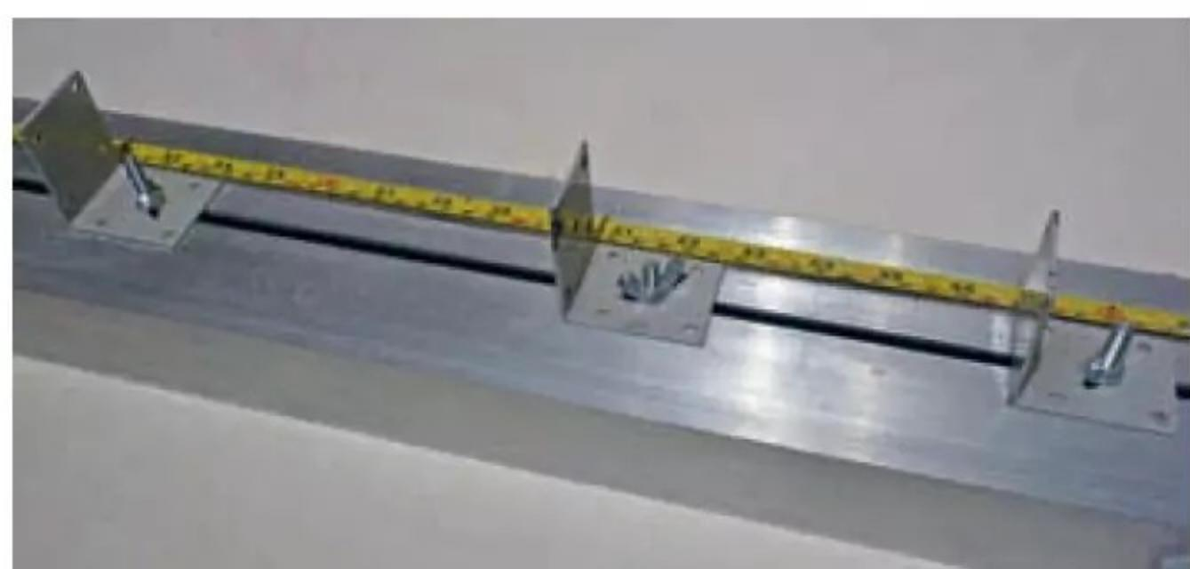
Butterfly nuts make for simple setting up. The fixed tape measure allows for accurate longitudinal alignment.
