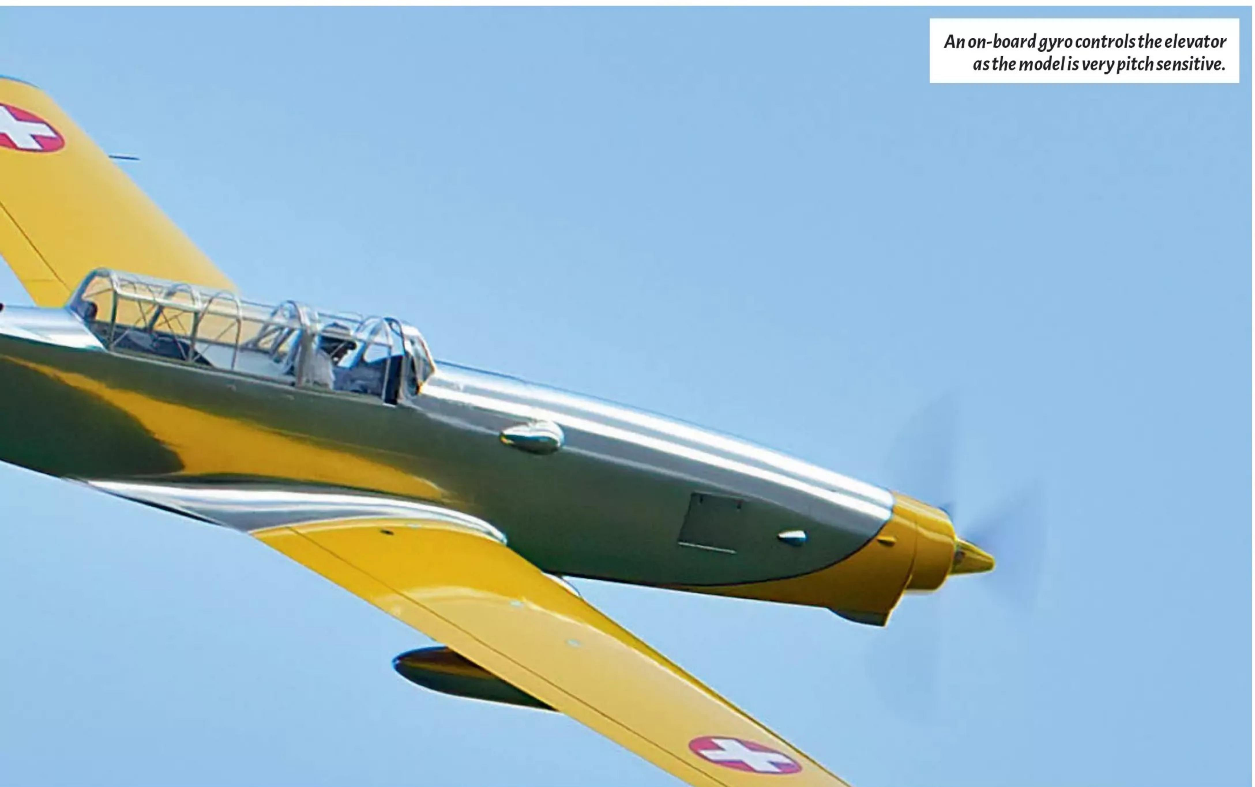
*An on-board gyro controls the elevator as the model is very pitch sensitive.*
