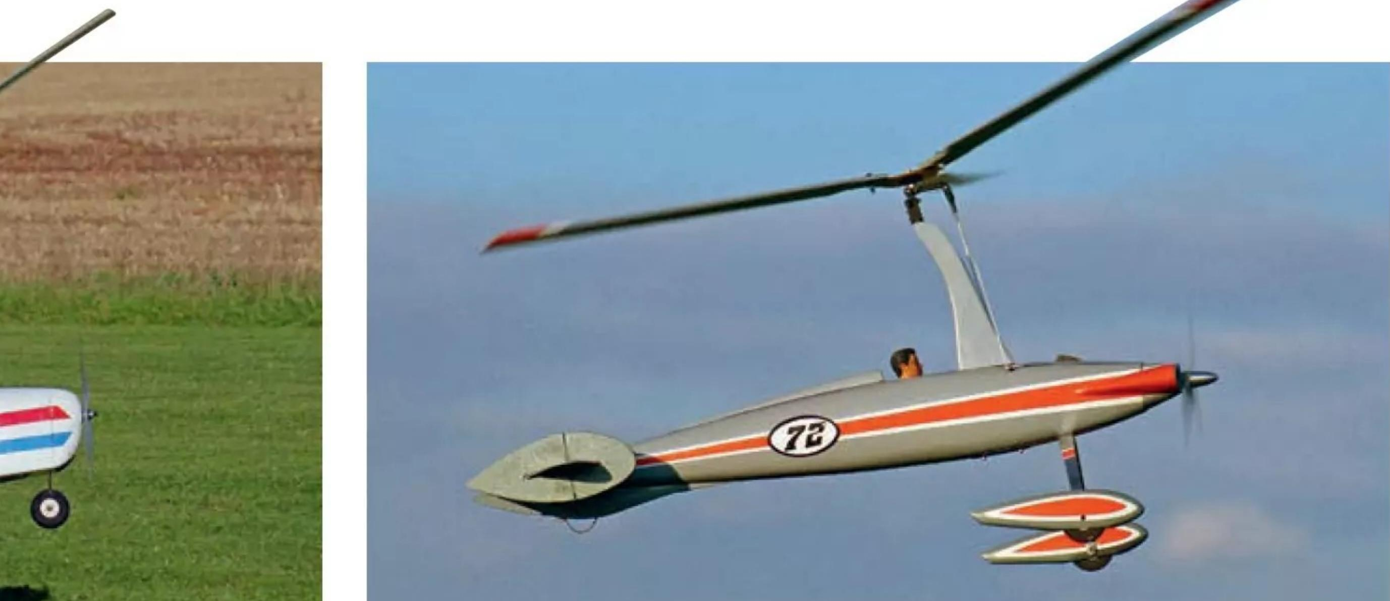
**The Twister** is one of my own, a sleek tractor still in its experimental stage. The sharp eyed will note the Depron fins, soon to be replaced with wooden units now that they are sized correctly.
