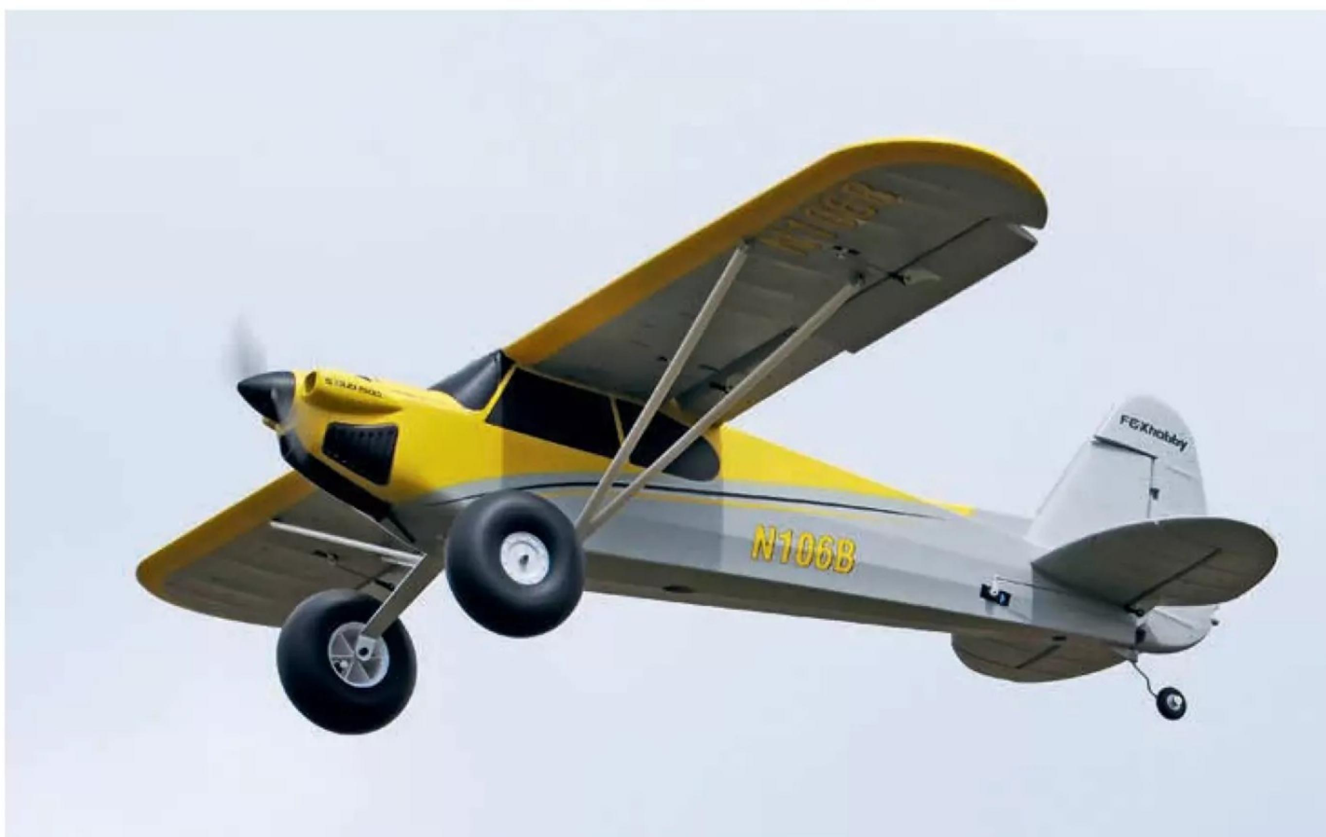
Minimise the bounce on S Cub landings by taking some air out of the chunky balloon tyres.
