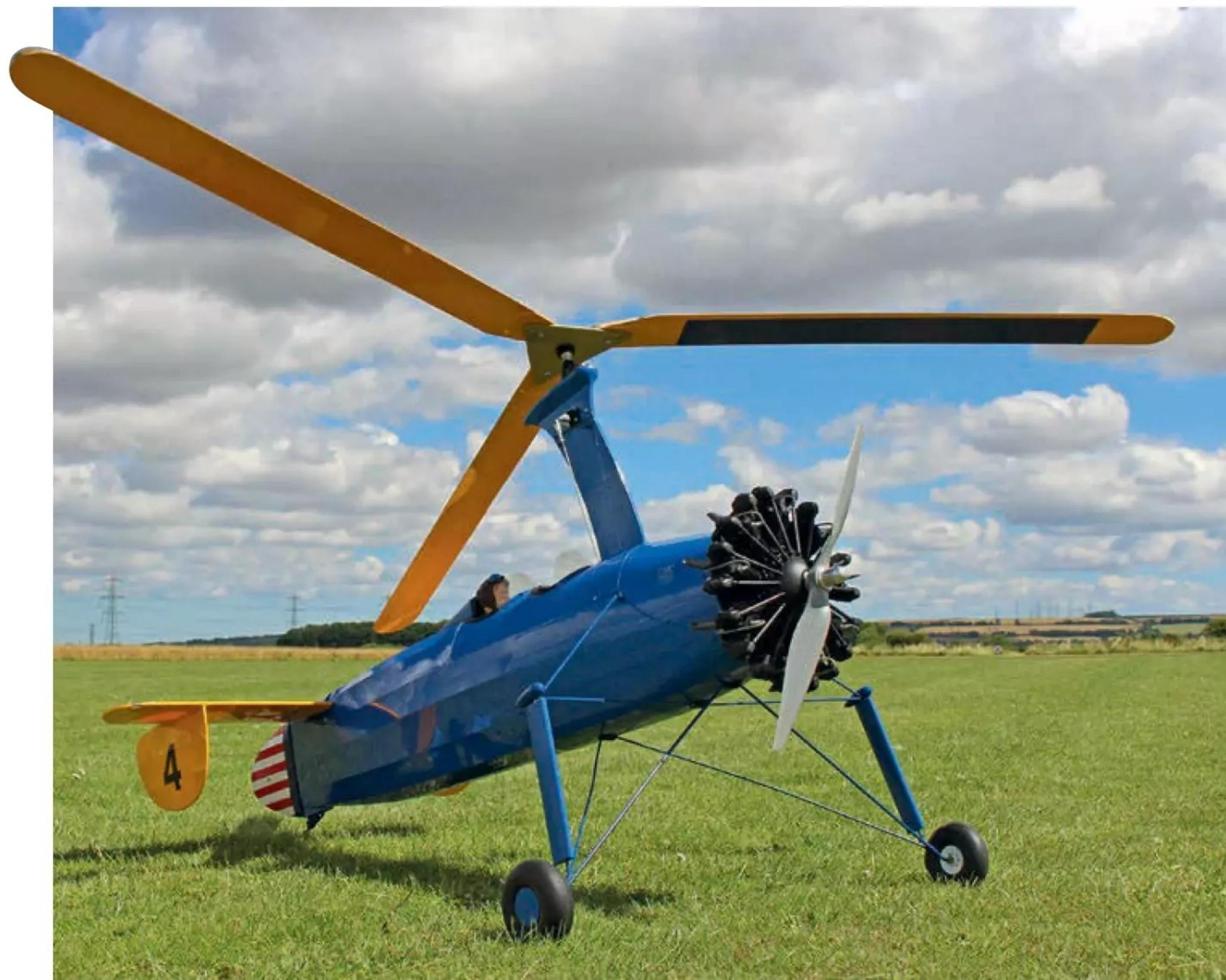
Back in the 1990s Autogyrros of Arizona produced a comprehensive kit of the 1930s Kellett. It featured a roll only head with and an all-moving tailplane. This well-presented model has been covered in the US Air Force training scheme. The dummy Jacobs radial finishes it off a treat.
