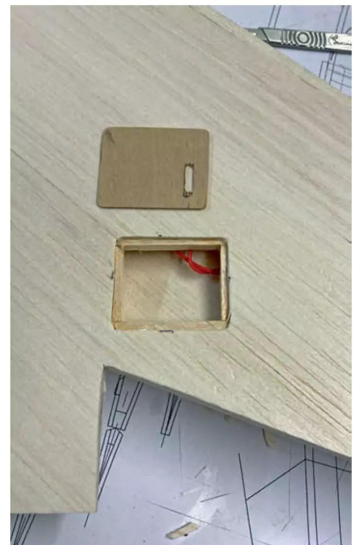
**Aileron servo hatch after being cut out from the wing sheeting.**
