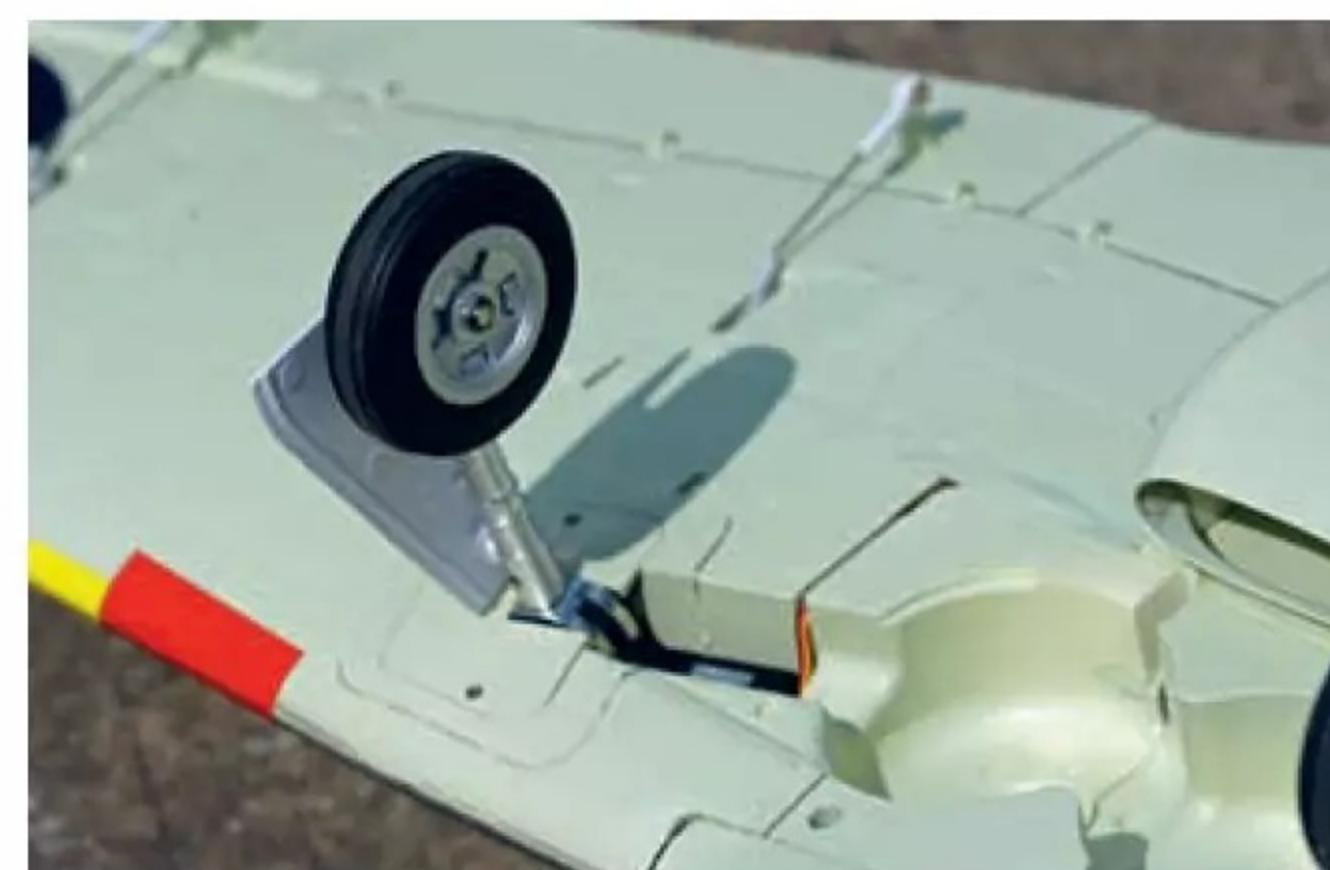
The Hurricane sports a nice pair of scale like wheels fitted to electric retracts.
