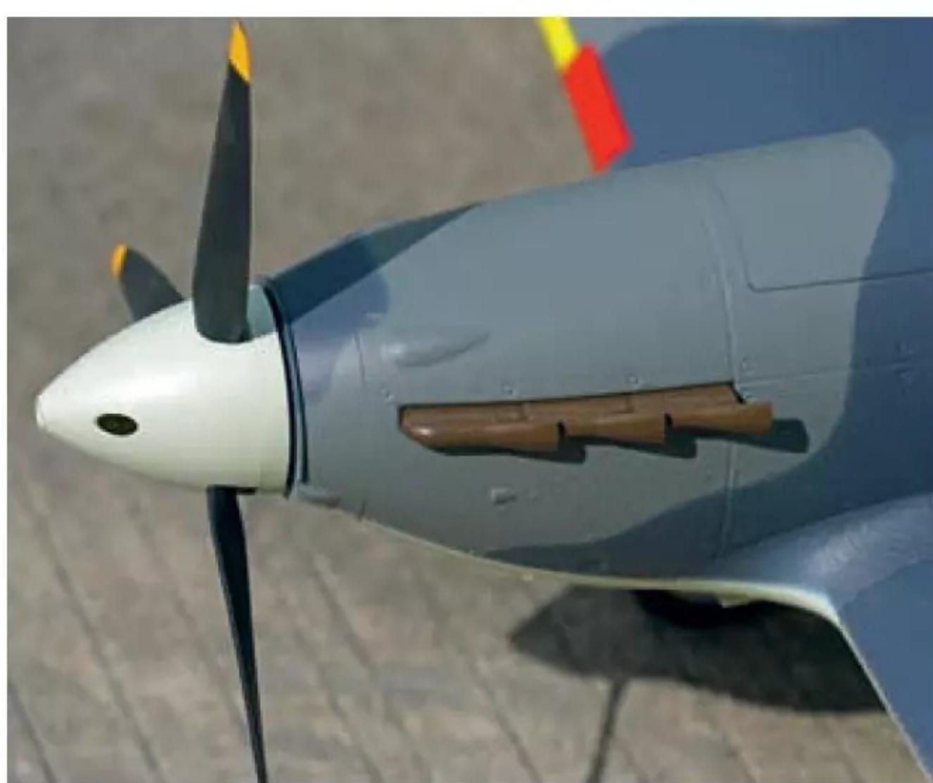
Close up on the neat three blade prop and spinner, just forward of the dummy Merlin exhausts.
