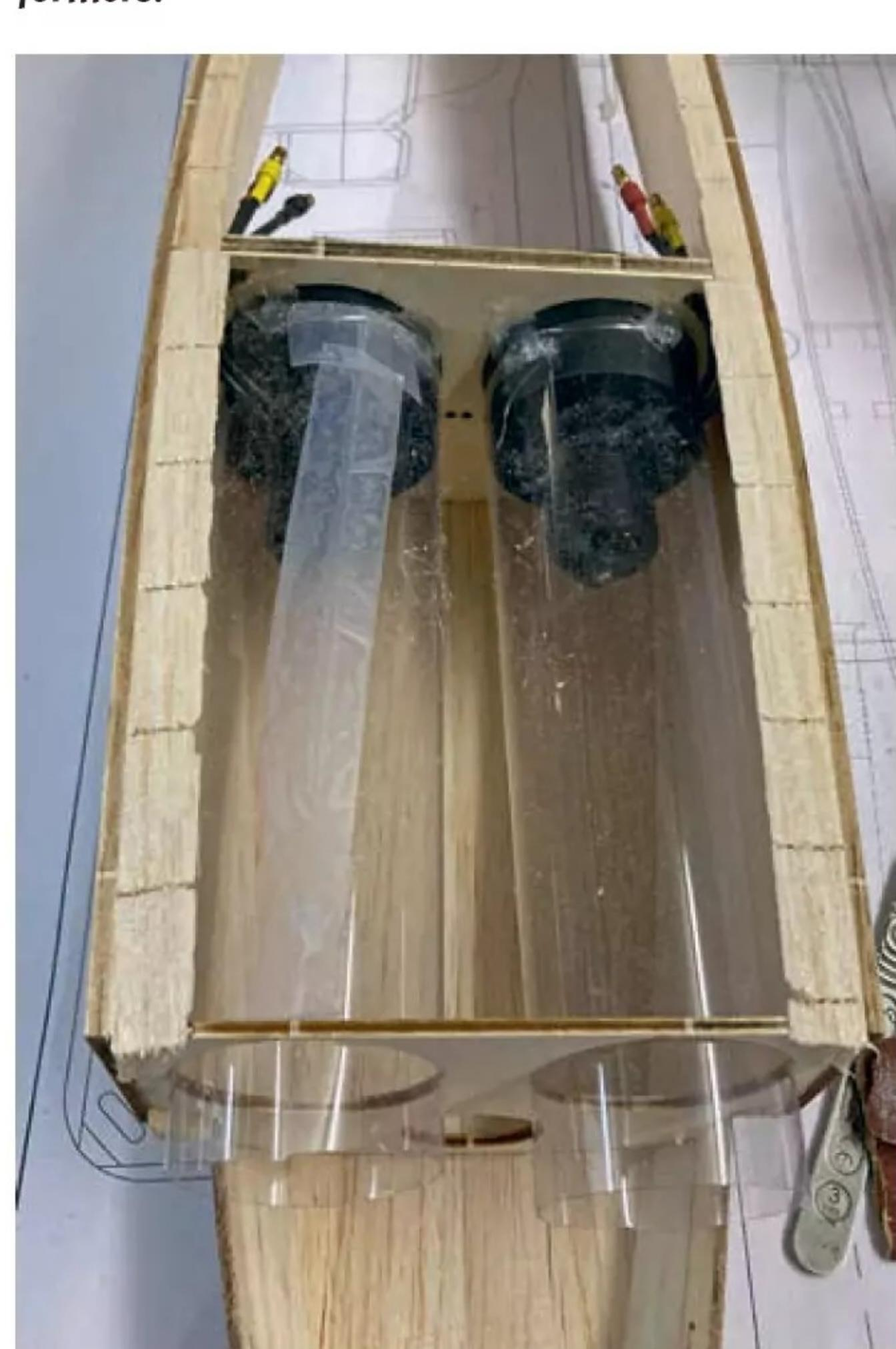
**Make up the thrust tubes using the template shown on the plan. Roll them around the fans and secure the overlaps with tape. Fix to the fans with blobs of hot glue.**
