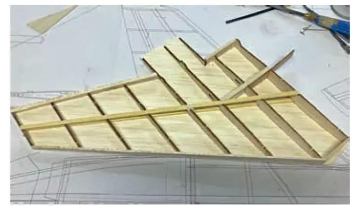
**Wings are of traditional built-up construction and are made over the plan.**
