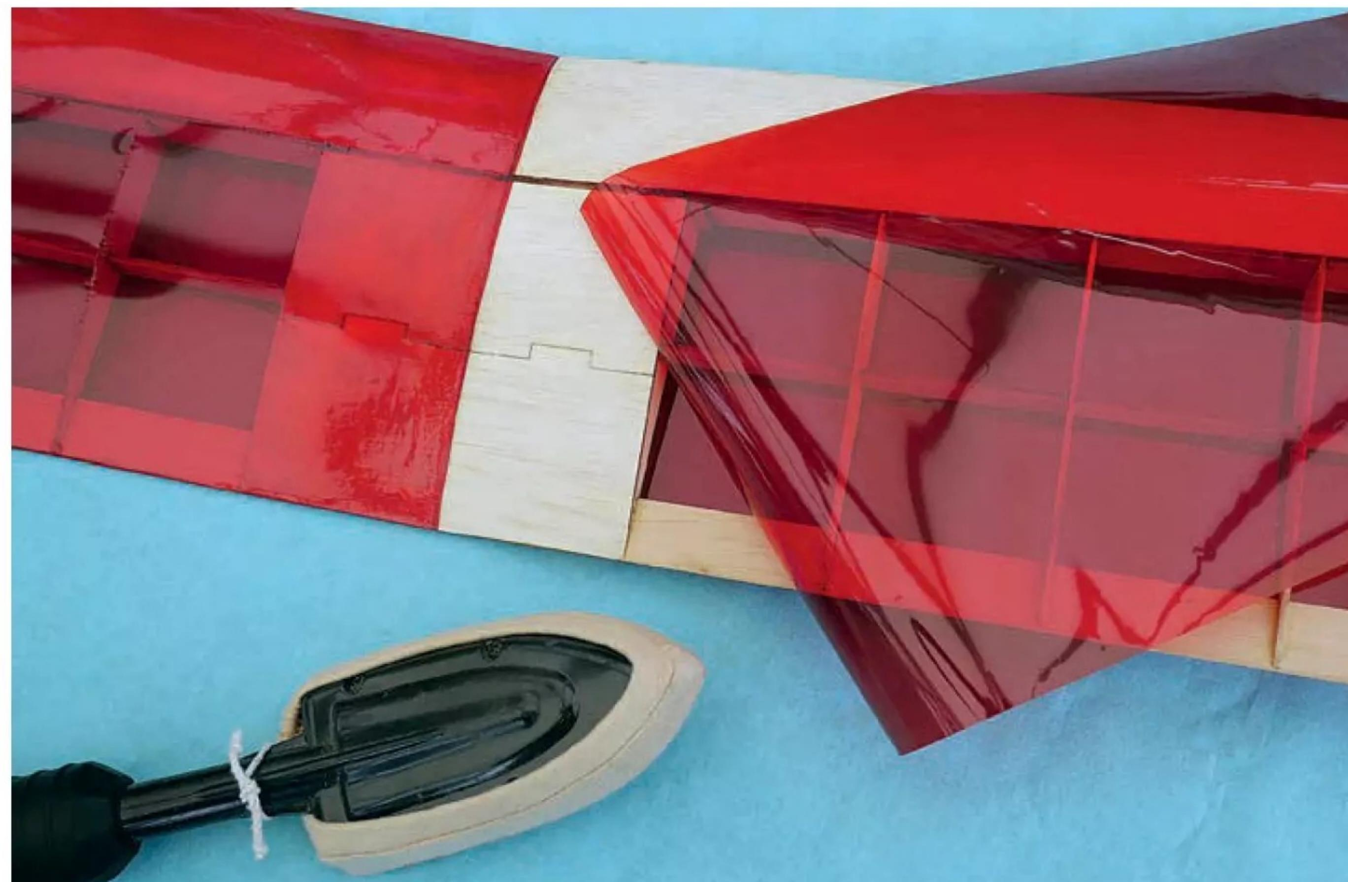
*Supplied Kavan covering film is easy to apply and tauten, but care must be taken not to inadvertently build in warps. A cotton 'sock' on the iron prevents scratching the film surface.*
