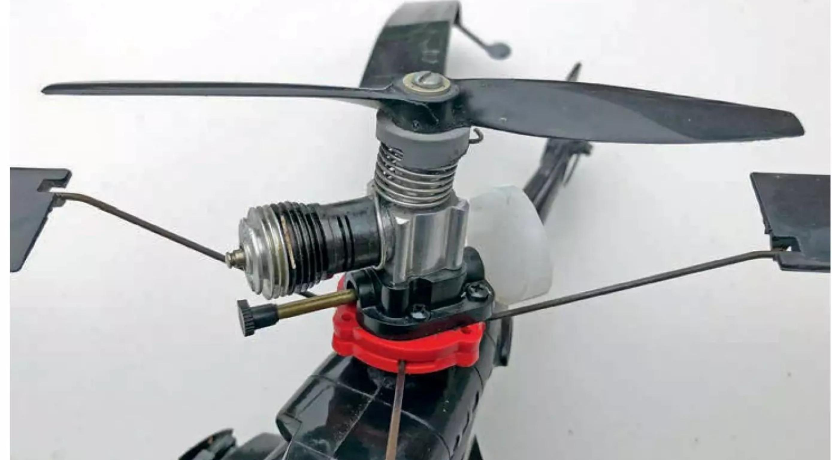
*Just behind the prop is the sprung SnapStarter fitted to the Airwolf's .049 engine.*
