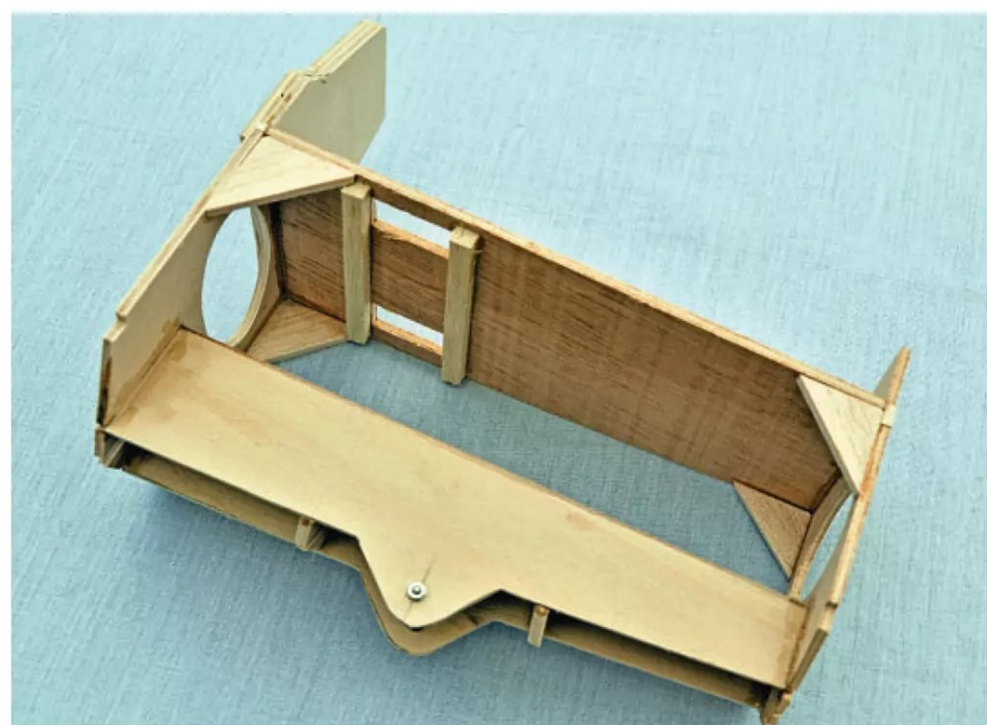
Assembled and glued, the central fuselage interior is ready to be built upon.
