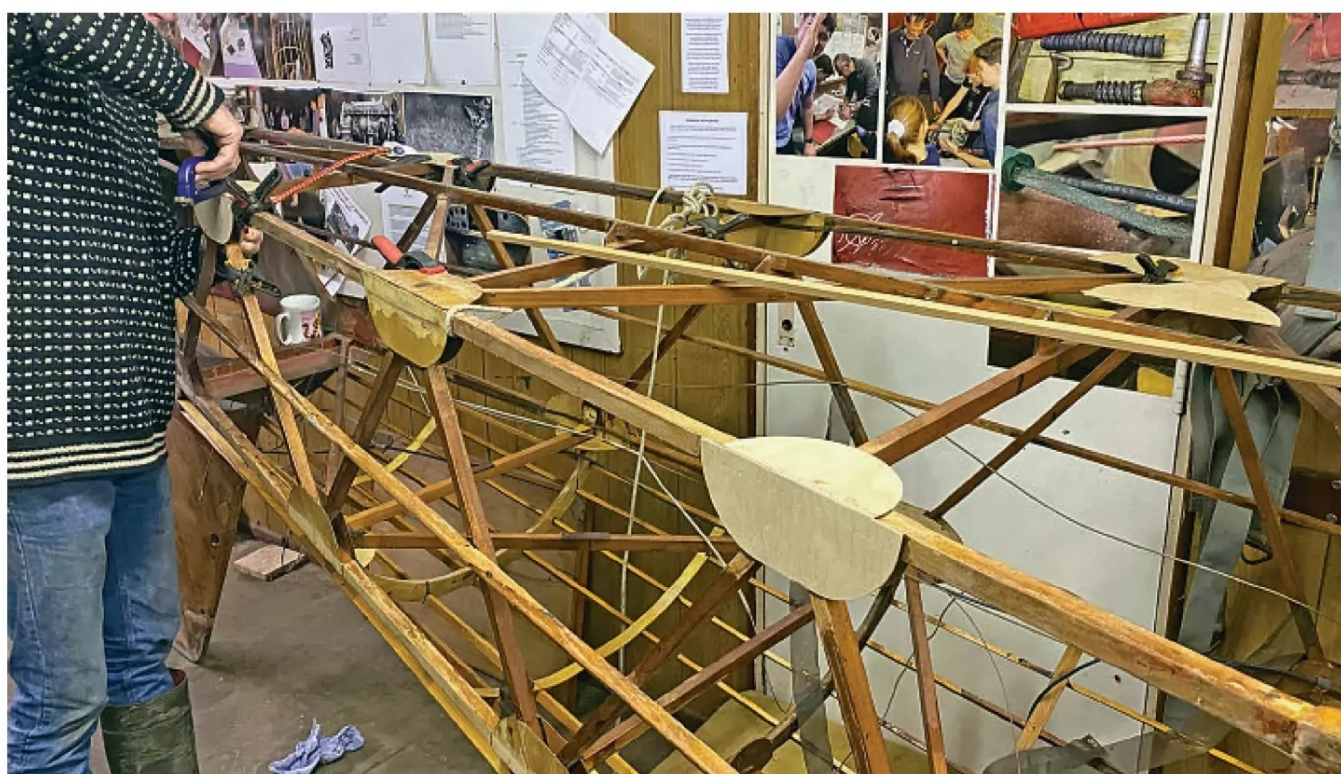
Replacement 'biscuit' joints, glued and stapled on the inverted fuselage of the full-size Linnet.
