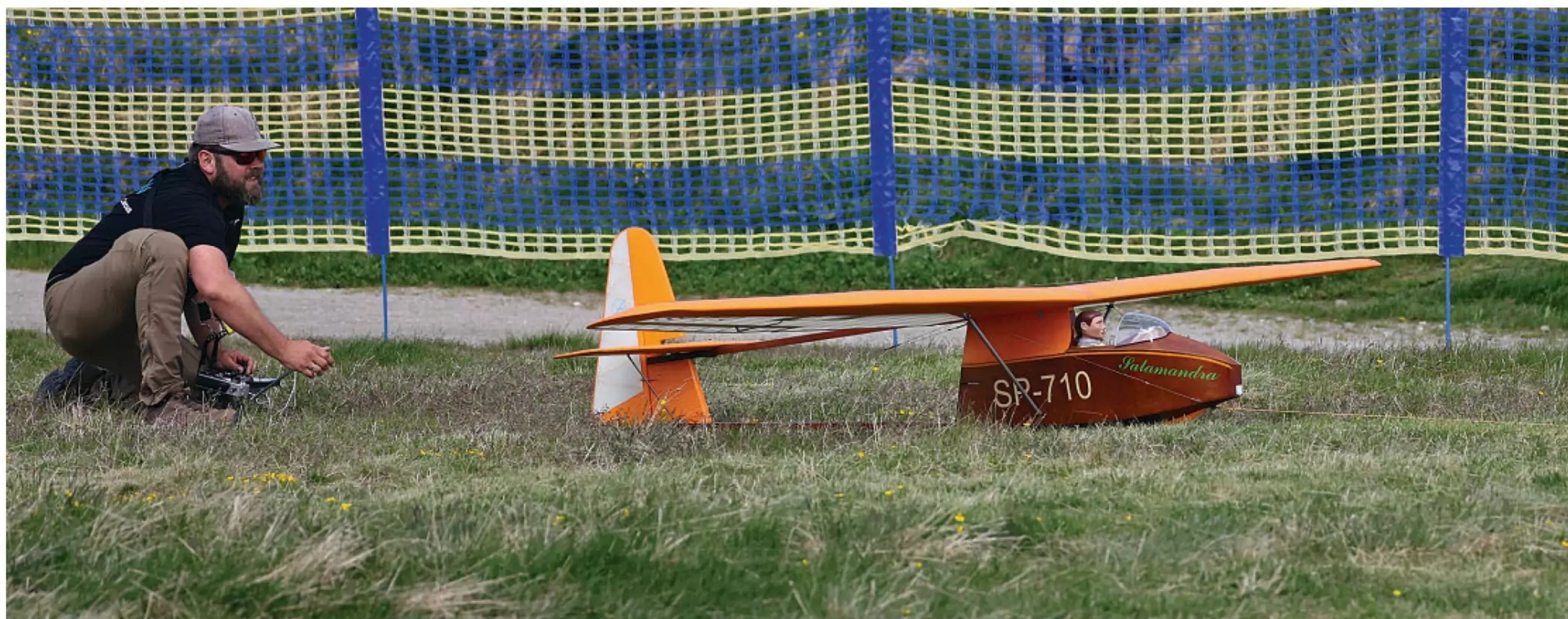
Josef Leng releases his IS-A Salamandra. His replica of the Polish training single-seater has a wingspan of 4.2 m and is made of plywood covered with Oratex.
