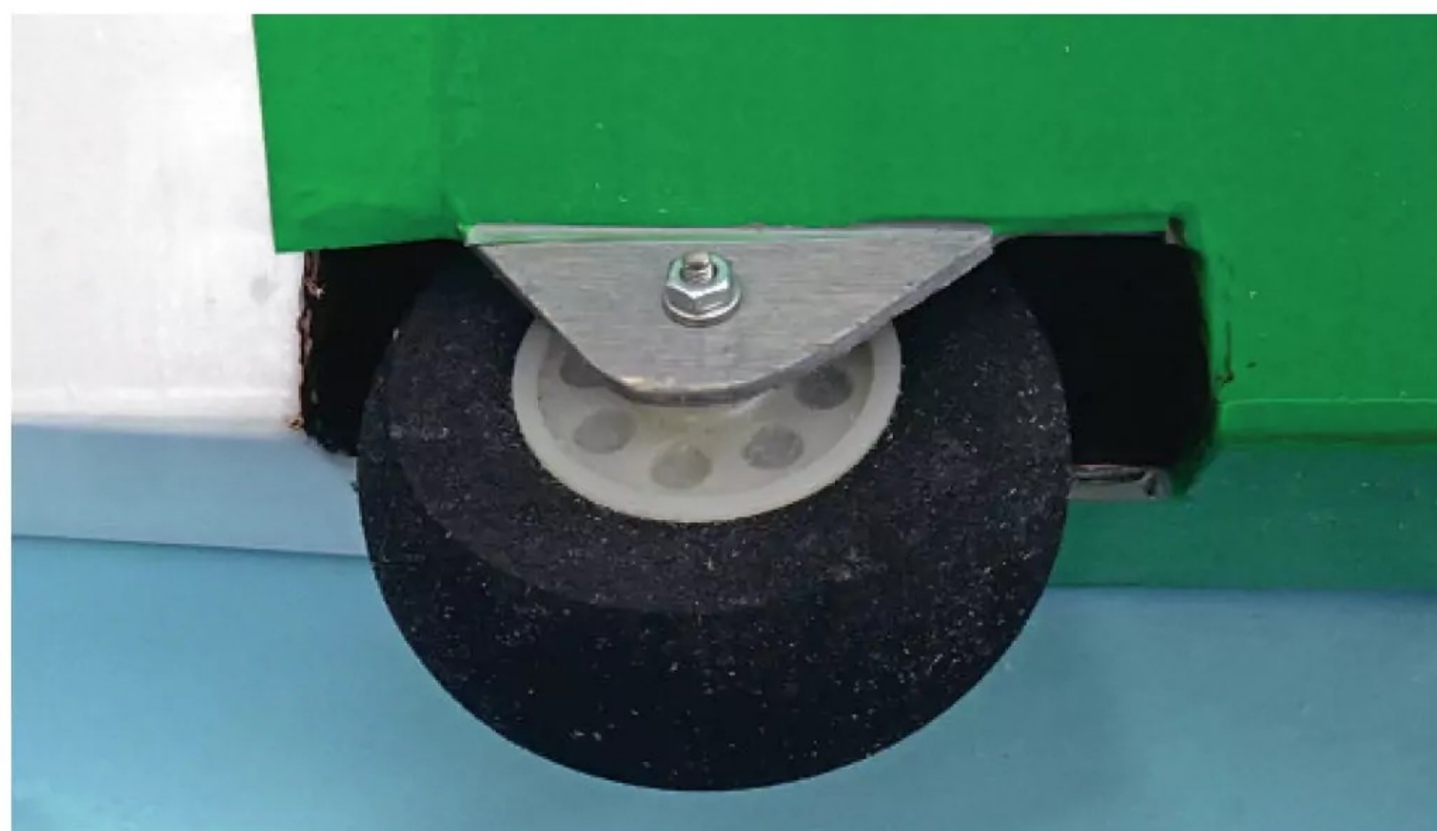
Landing wheel is very noticeable and shouldn't be omitted. Sleeving the wheel axle prevents 'pulling-in' of the plywood mounts.
