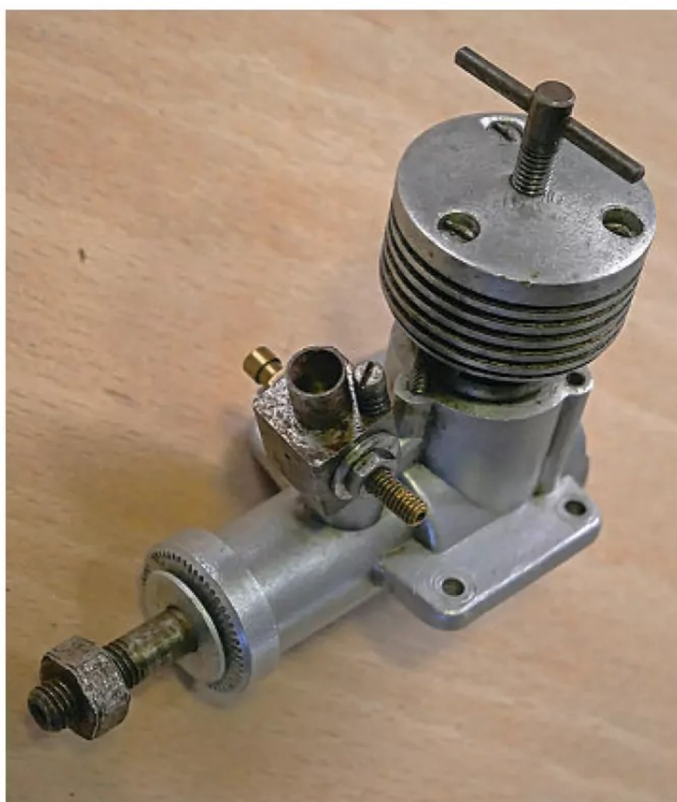
A handsome beast. The PAW 2.49 R/C, not me! A careful clean and rebuild has resulted in another thoroughly useful motor.
