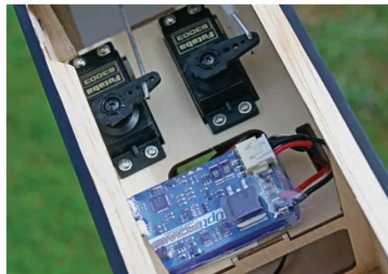
Optiguard is a 2S back-up solution that kicks in when it senses a voltage drop at the Rx.
