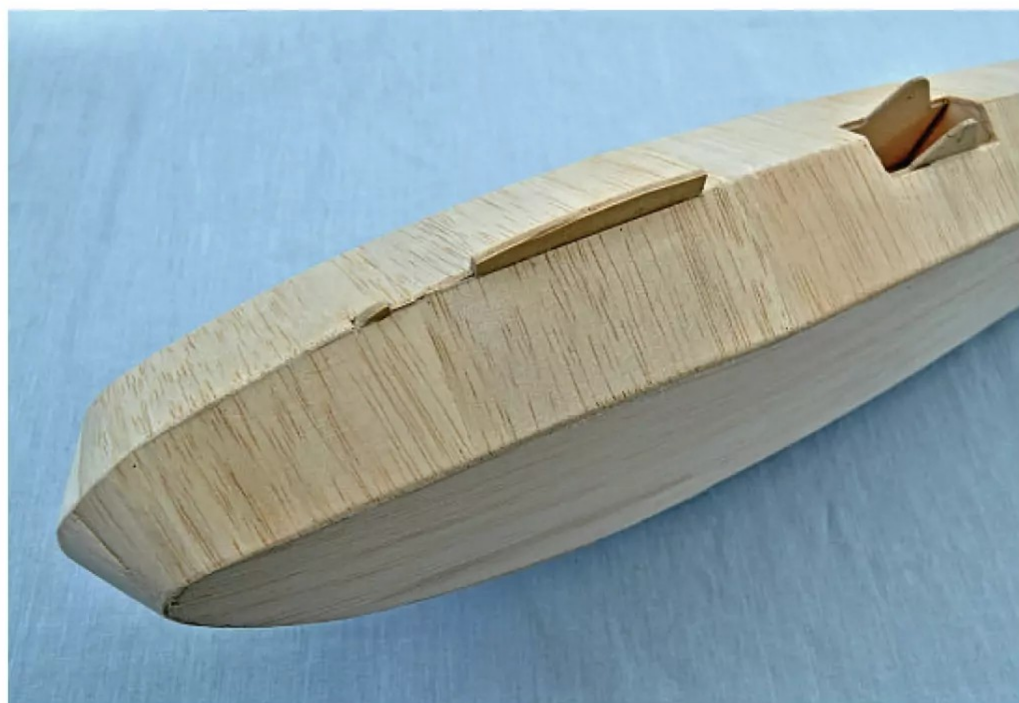
Nose underside is sheeted to give that distinctive shape.
