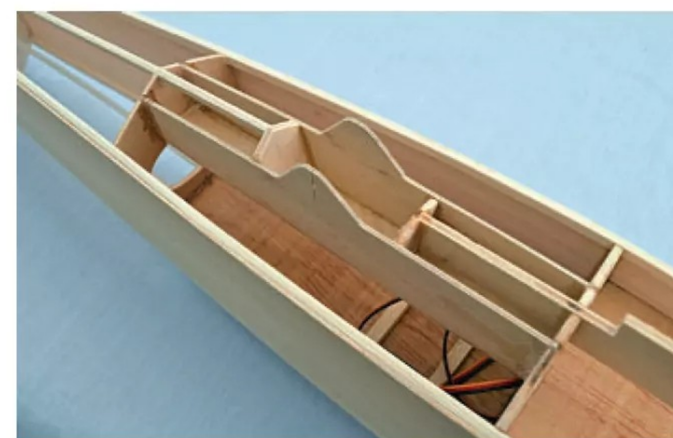
Wheel mount and skid form a simple yet strong central spine.
