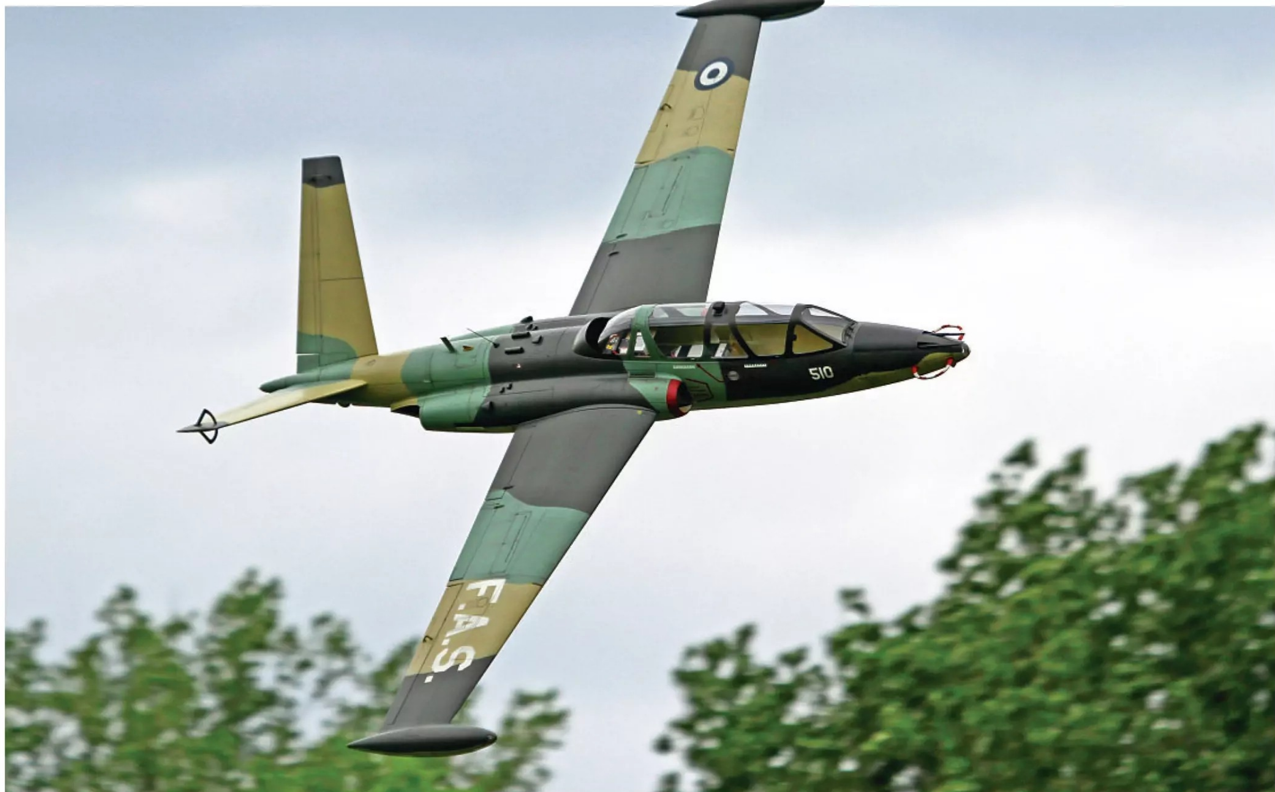
The Magister is painted in matt wall paint, protected by a thin layer of semi-matt yacht varnish. Decals are from paint masks with waterslide paper used for small signs.
