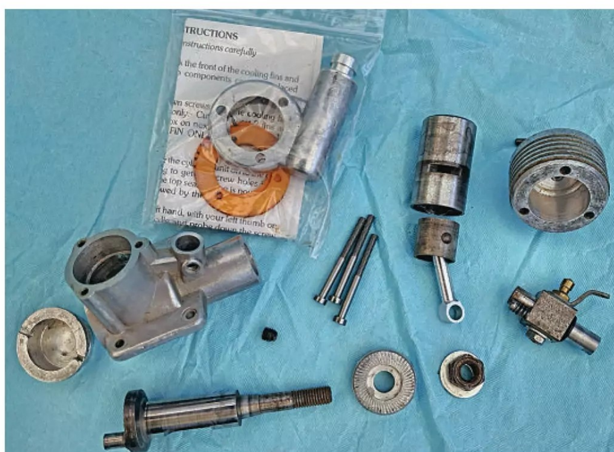
Parts from the gifted PAW 2.49 R/C engine cleaned of sully 'laquer' and ready for assembly. It's a tough and dependable motor, even after many years of misuse.
