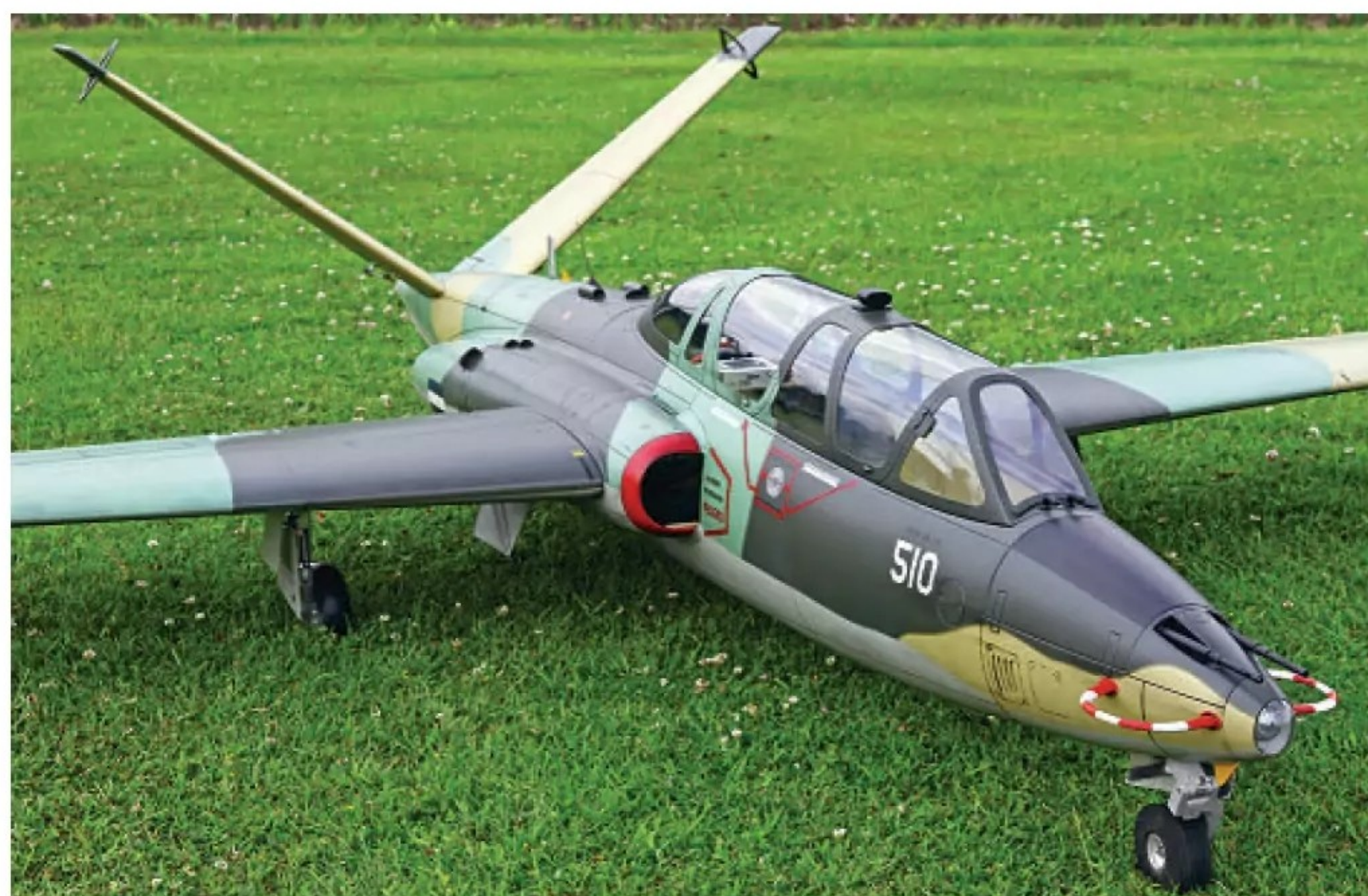
Dirk chose to make a fully moulded fuselage as he wanted it to be light.
