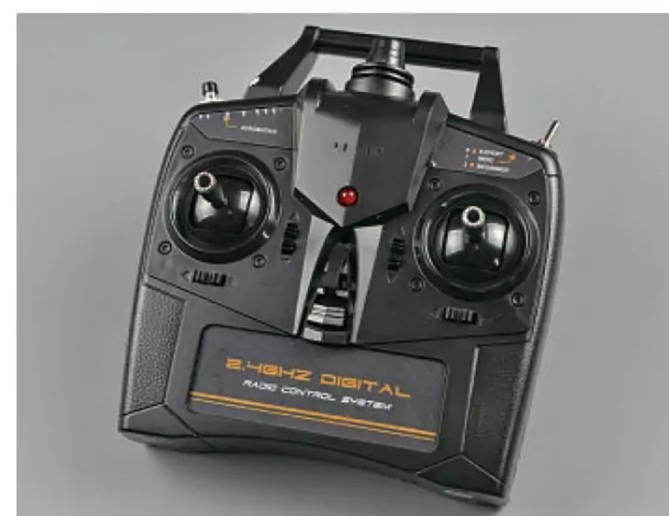
The basic transmitter supplied is set up to fly the Corsair and does the job perfectly well. Or you can use your own DSM or SBUS Tx by plugging in a suitably small receiver.
