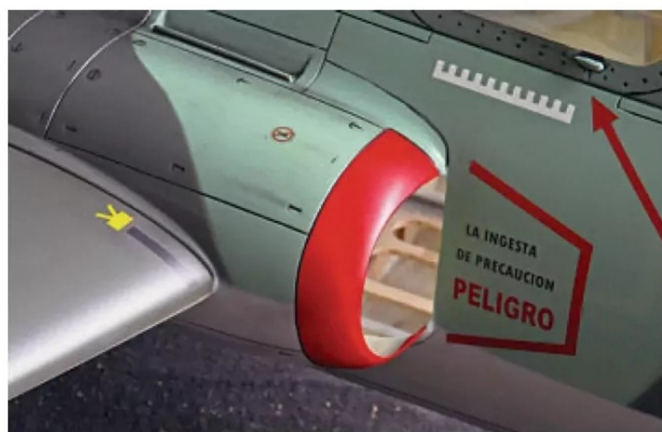
Jet intake giving a hint of the lightweight structure inside.
