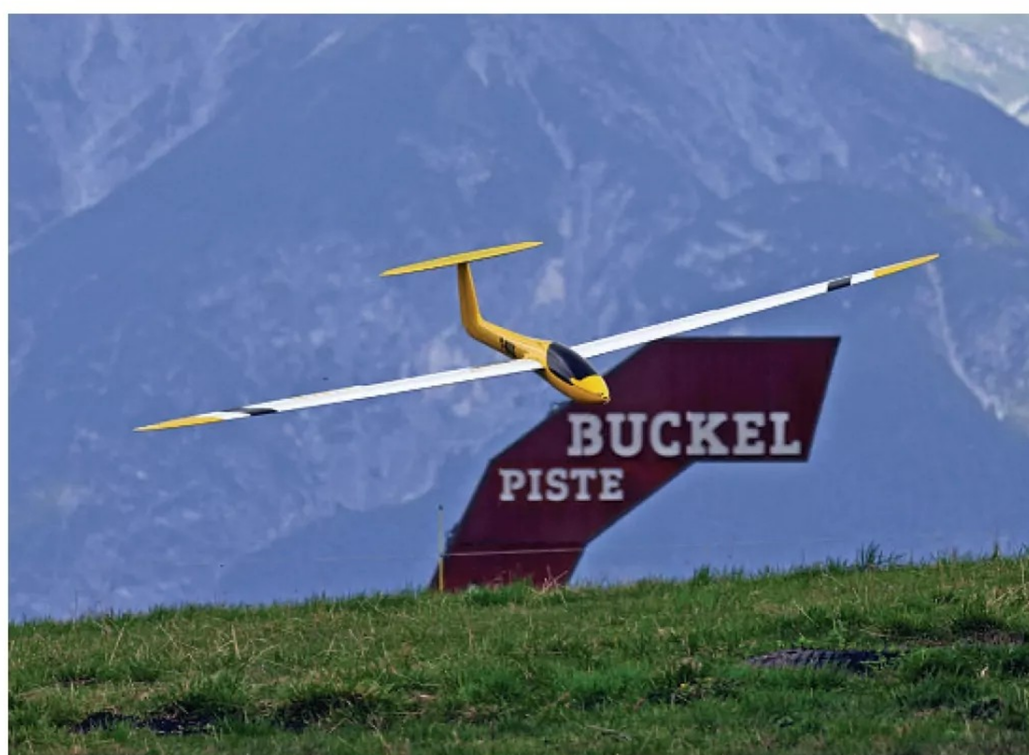
T-Max from Competition-Tools piloted by Rafael Schydlo. Wings come from the F3x Mamba series fitted to a scale-like, all-purpose fuselage. Offers performance of a competition model with a scale look.
