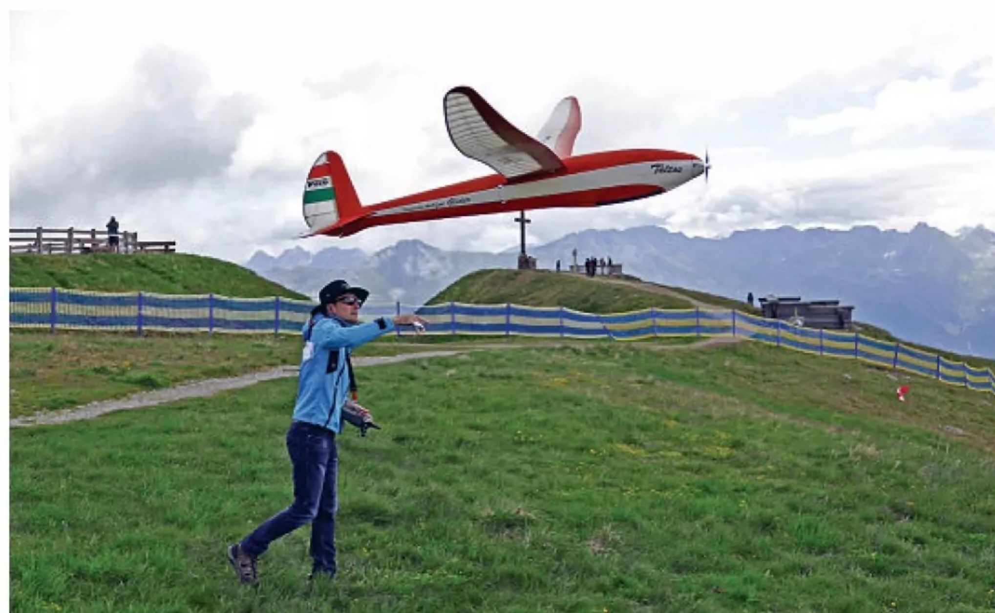
Stefan Nam launches his the Táltos 'Pegasus' (3.5 m wingspan) from Paco Scale Models in Hungary. The model is built to order. Assembly uses furniture clamps so the large glider can be transported and stored in a small box.
