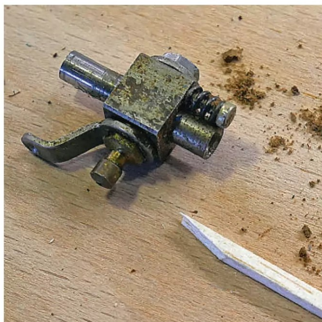
Post exhumation, the once-buried little PAW carburettor was cleared of local 'loam' before stripping and cleaning.
