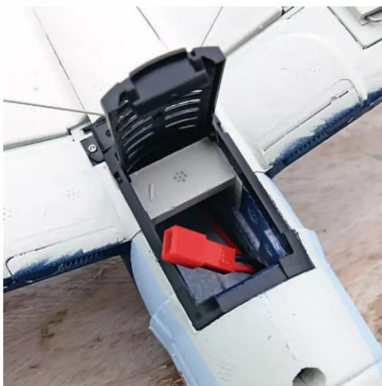
The little LiPo drops vertically inside the battery bay.
