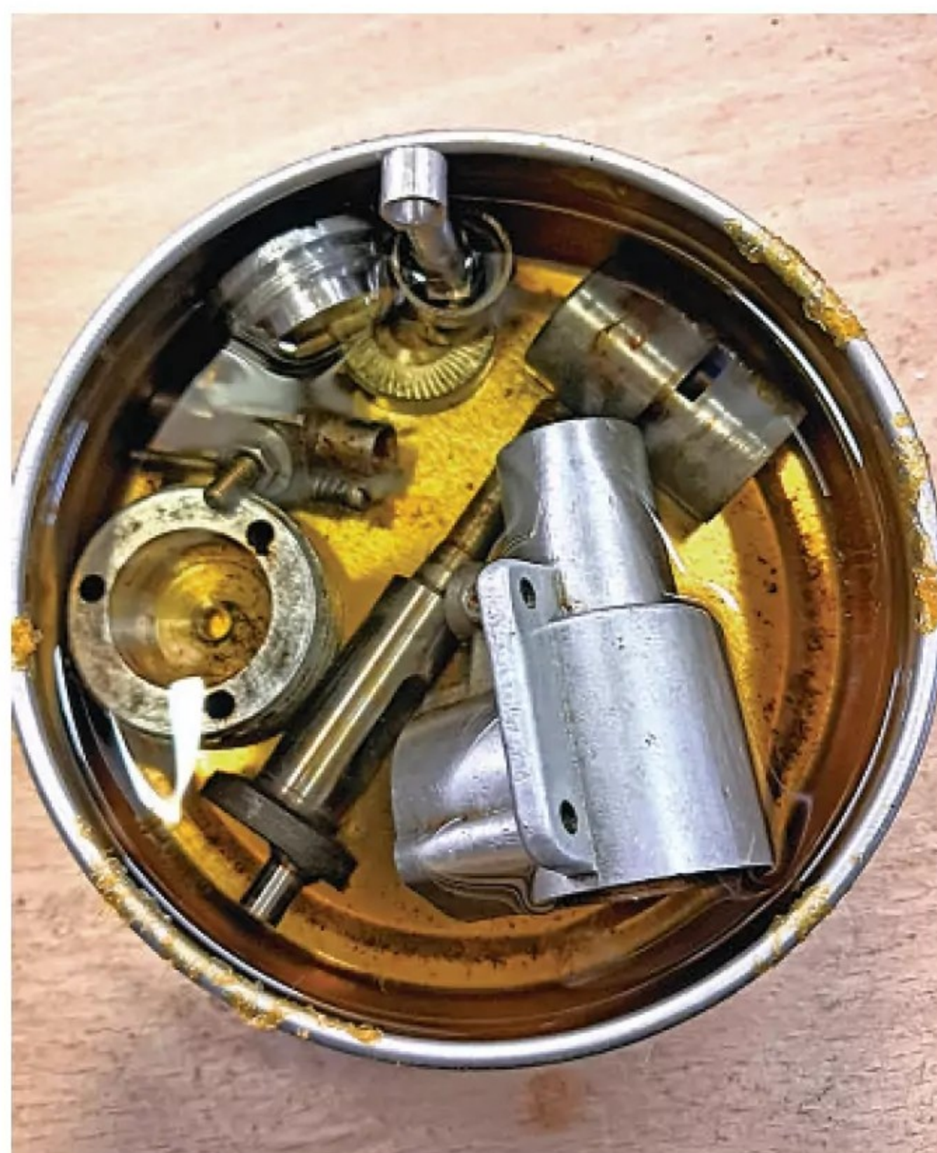
Once stripped and 'de-soiled' the little PAW motor parts were soaked in solvent to soften old burnt fuel 'laquer'.
