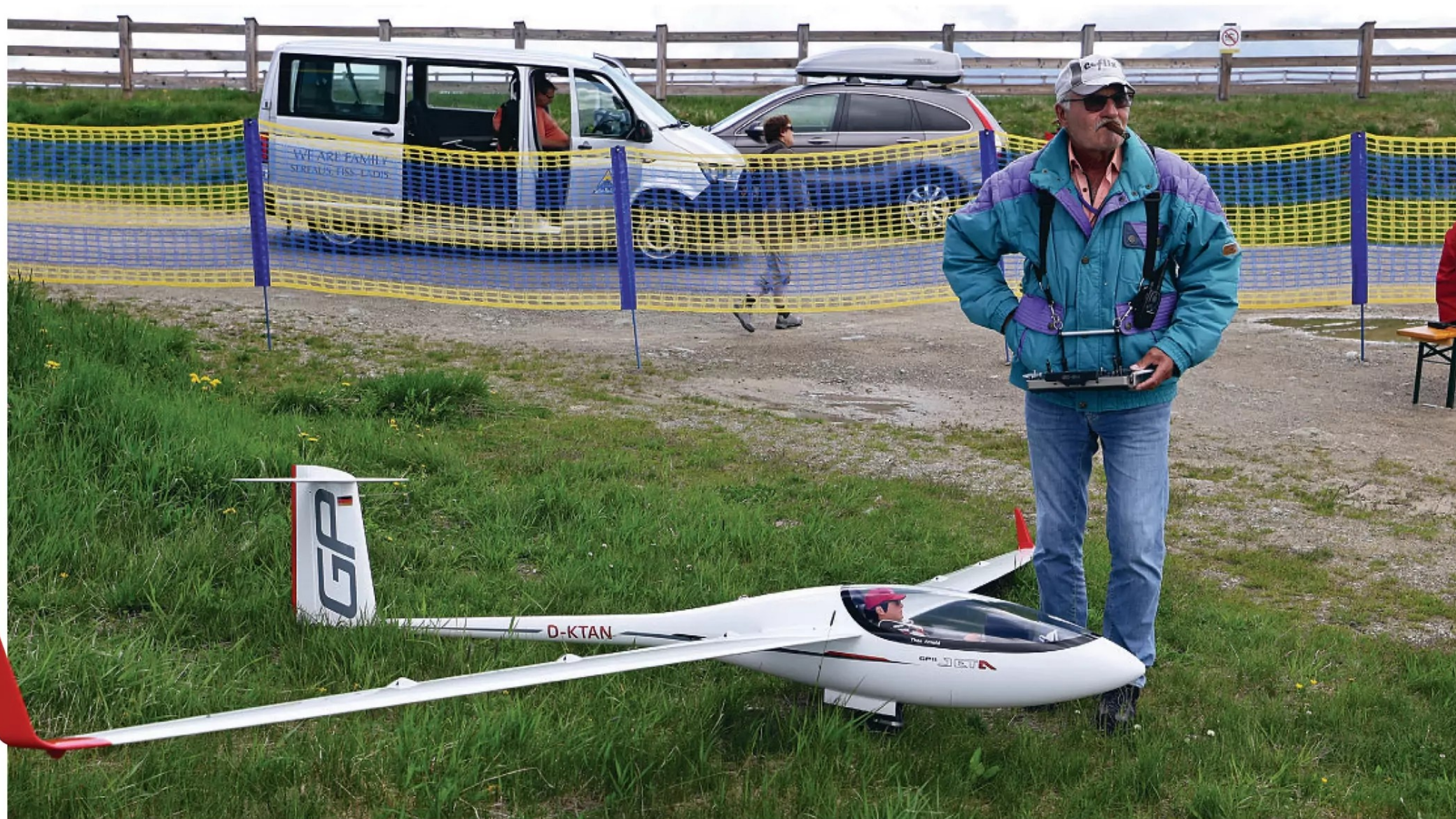
Theo Arnold with his new 1:2.5 scale GP15 from Ceflix (6.0 m wingspan, 2.57 m length). Theo's GP15 is powered by a KTW Orbis 20 x 13 self-launching system on 12S.
