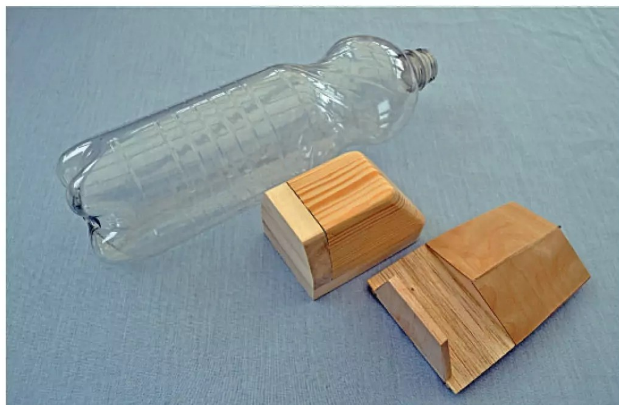
A canopy is heat shrunk over a shaped plug. Very easy if you are careful with a plastic bottle and heat gun.
