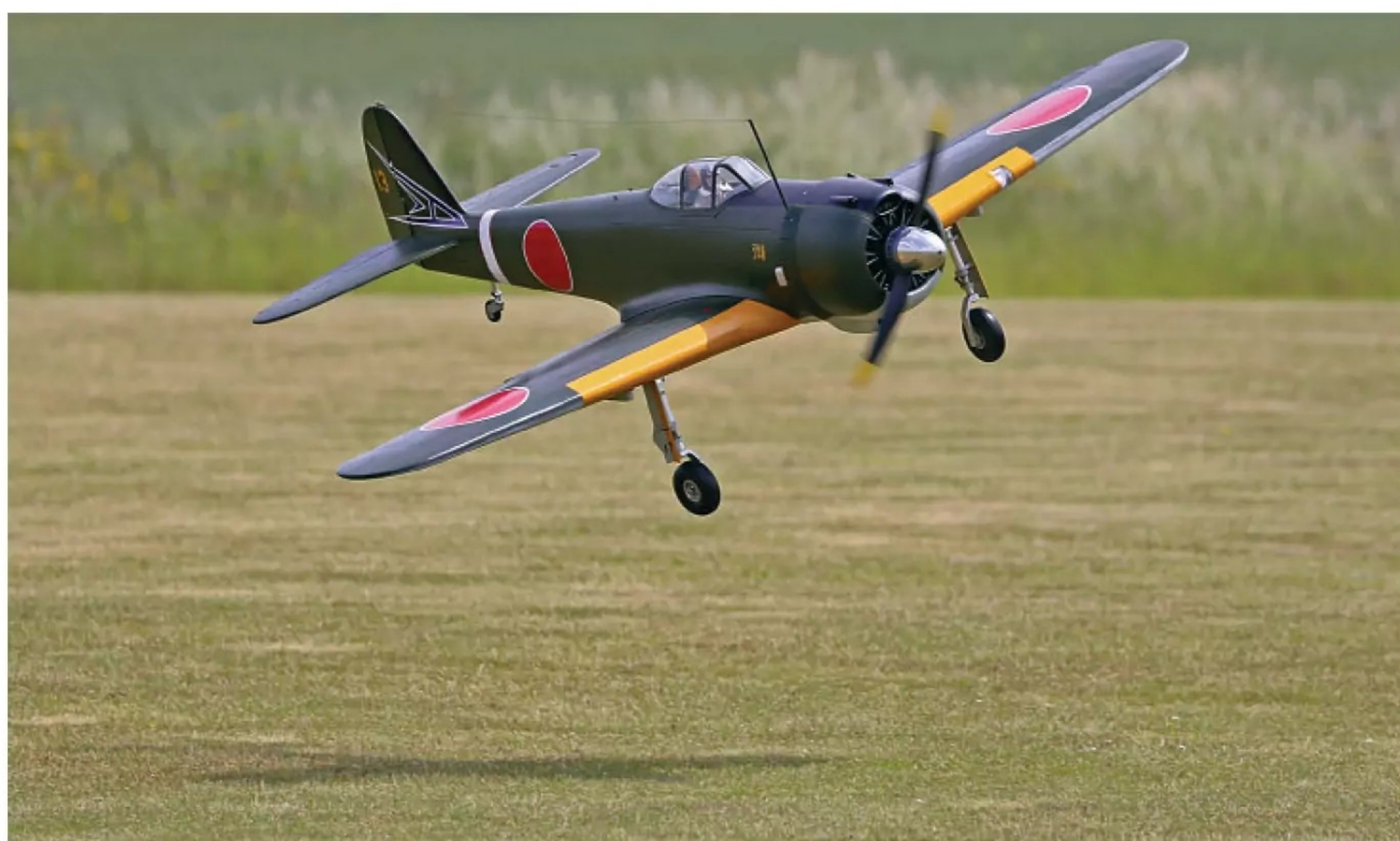
Nigel Nixon's Ki-43 Oscar is a beautifully re-worked and re-finished ARTF. It uses 12S power to spin a 24" x 12" prop.
