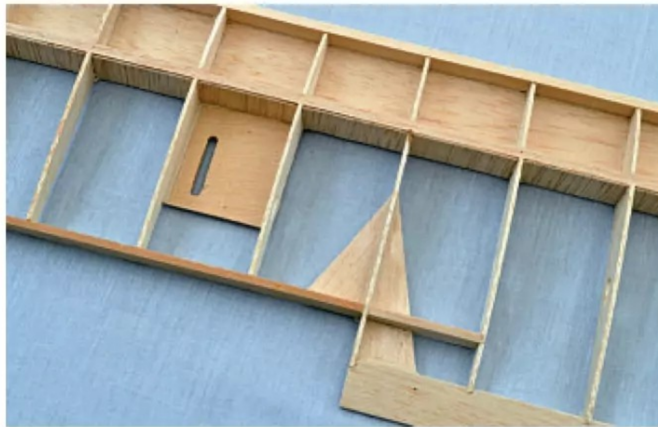
Simple wing structure before the top sheeting is fitted. Aileron servos and arms are tested and adjusted before gluing in place.
