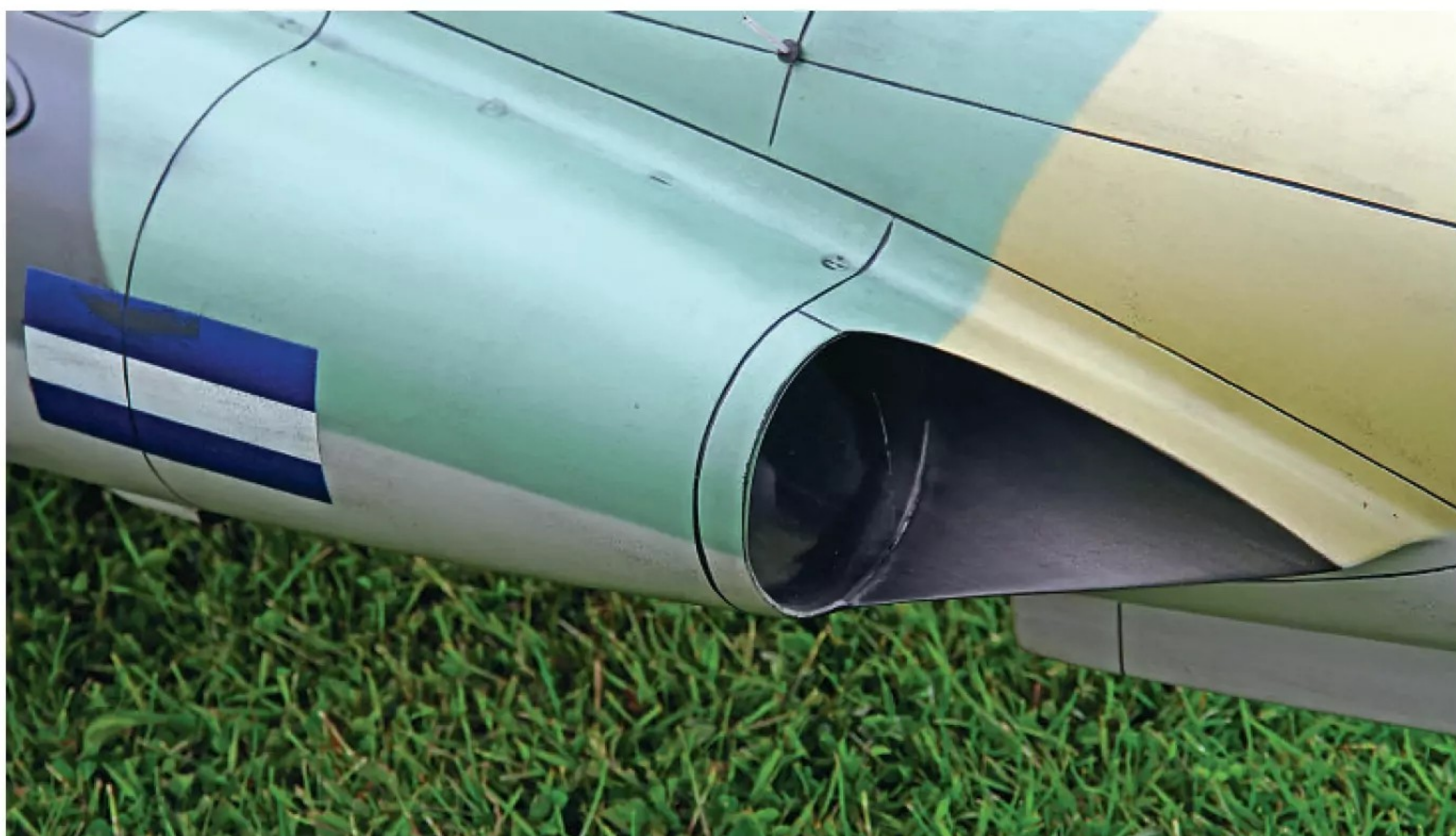
Thrust tube plug was 3D printed due to its complex geometry.
