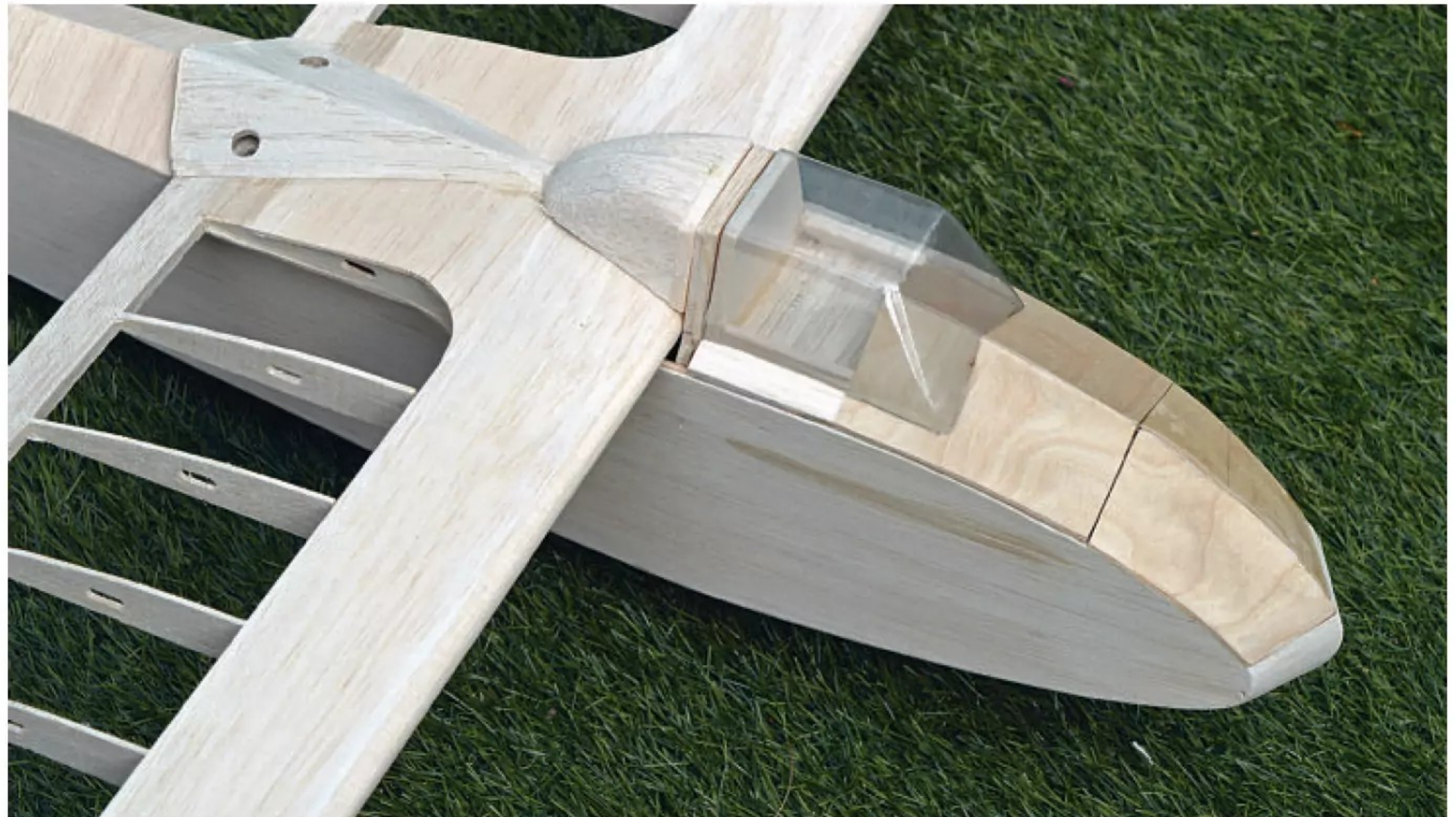
Here you can see the distinctive nose and wing fairings. Simple to achieve with a little work and care.
