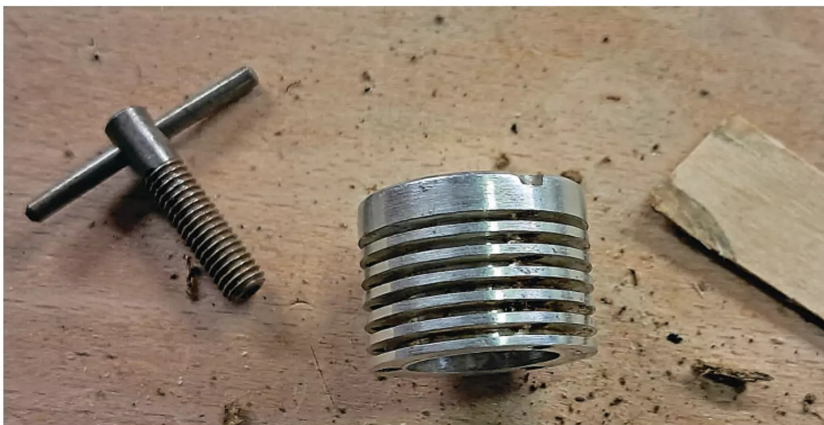
Don't poke and prod with a screwdriver, etc. Clear muck and soil from between cooling fans with a strip of thin plywood. It'll do the job without scratching or scoring.
