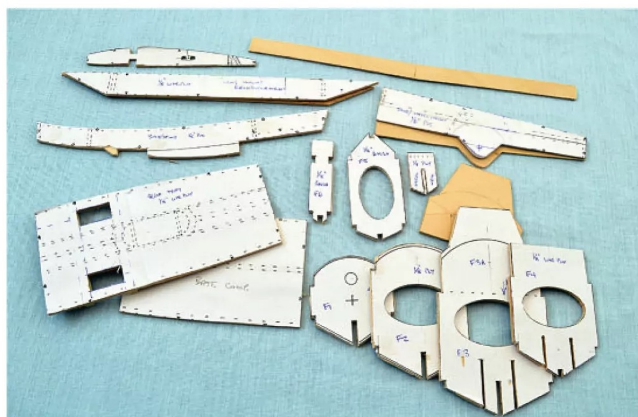
All the plywood parts. I glue stick photocopies of the parts onto the plywood as it's easier to keep the cutting/sanding accurate.
