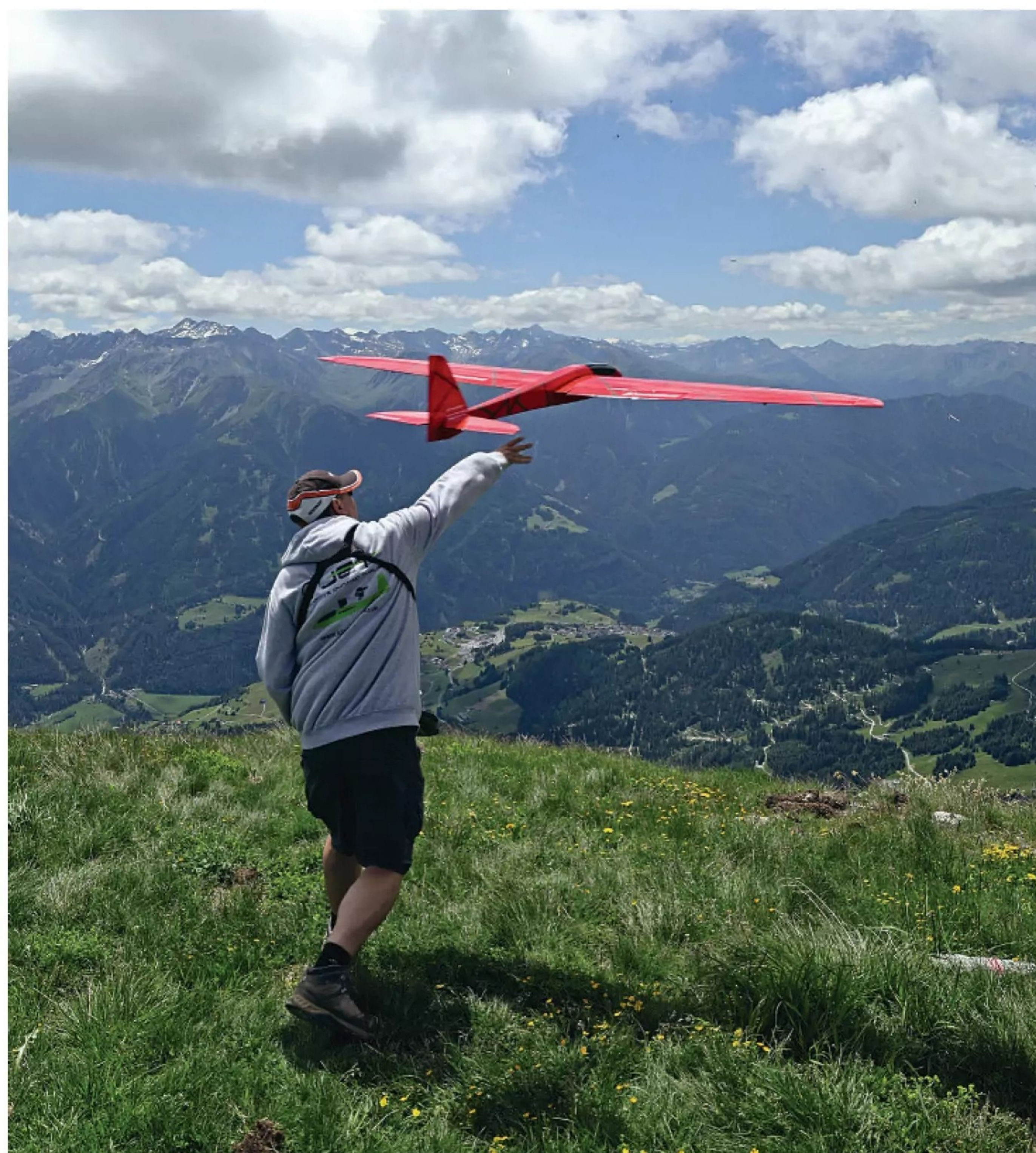
Steve Steff gets his Teufel safely away. Of wooden construction and fully aerobatic, it still flies well in thermals. Wingspan is approx. 2.2 m, with a modified MH 43 profile.
