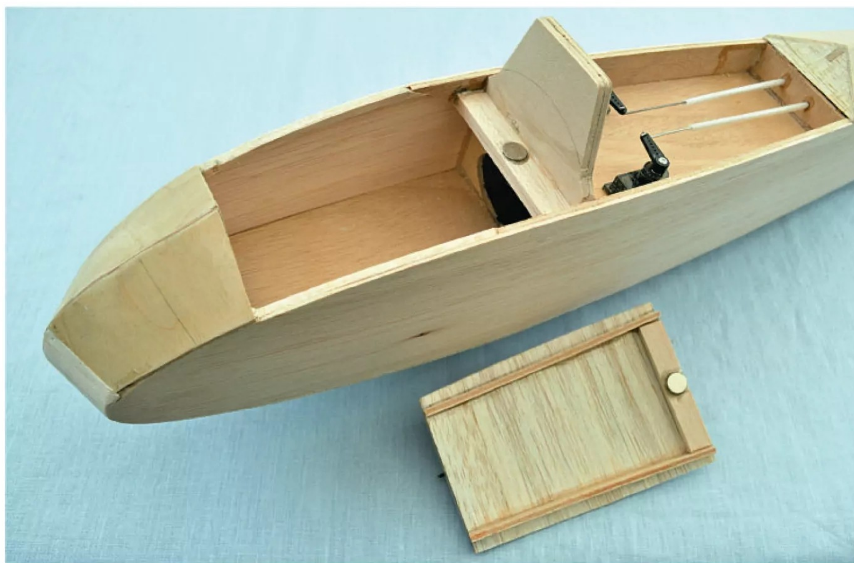
Lots of space for your radio gear and battery. The cockpit base is simply made from sheet and curved formers.
