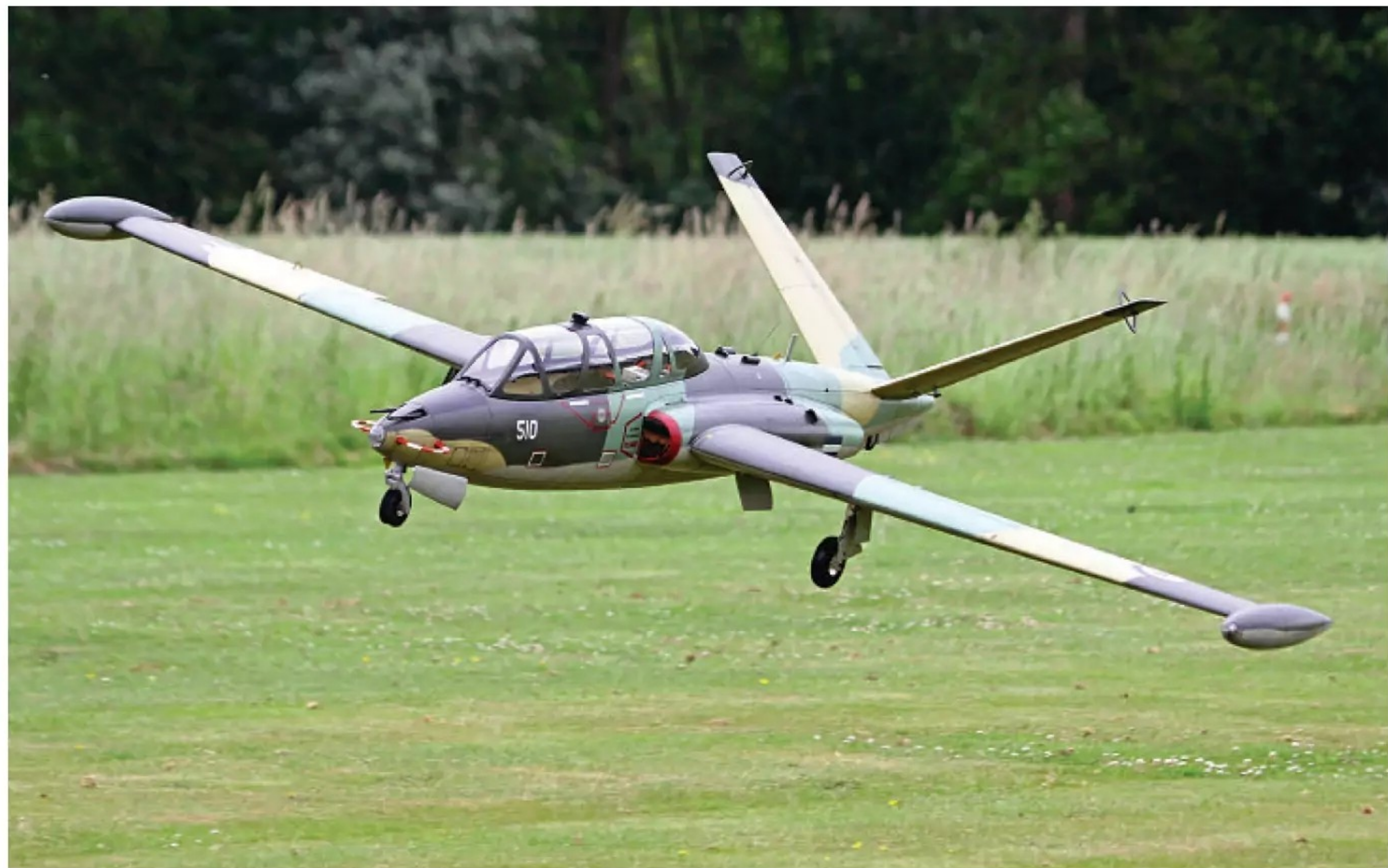
Using the flaps and speed-brakes are very helpful when landing, especially on short runways, otherwise the Magister keeps floating on!
