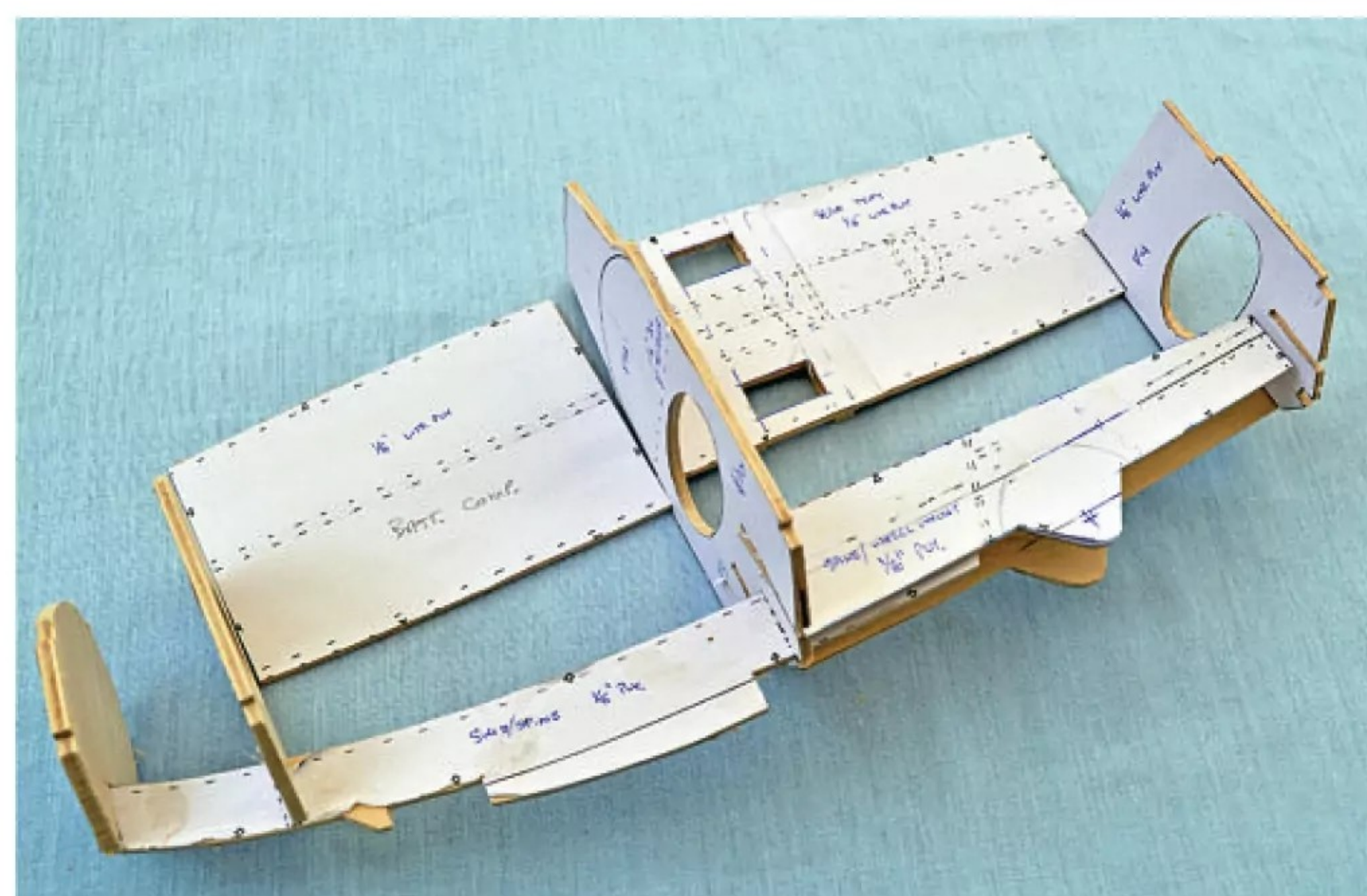
Fuselage formers are test assembled to prove accuracy.
