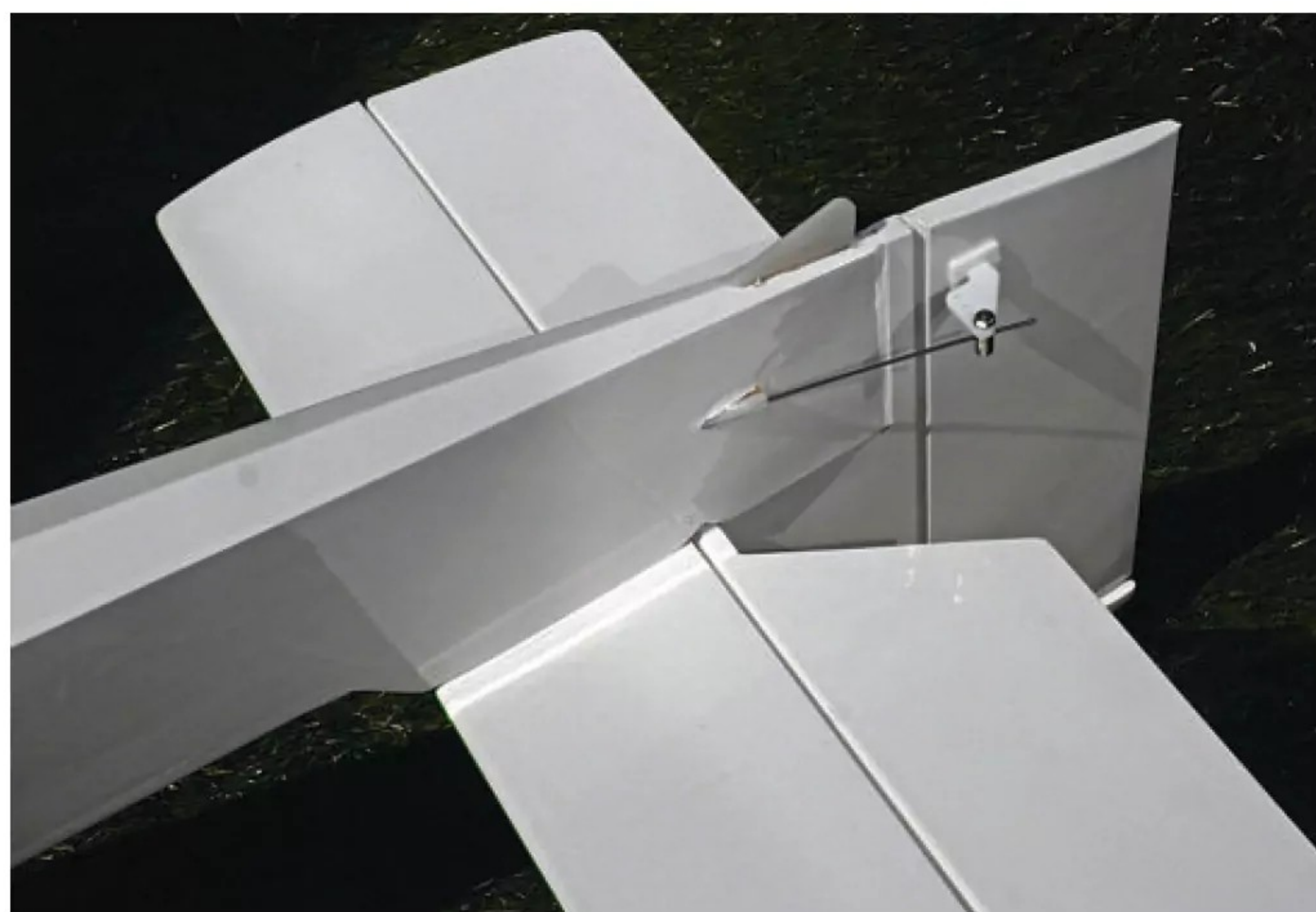
Rudder hook-up of the wire pushrod. Ditto for the elevator.
