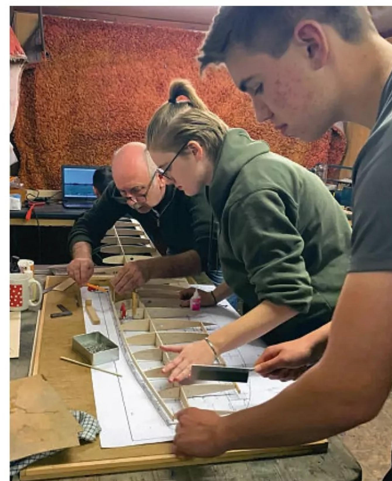
Laminated leading edge being fitted to the Stokesley model.
