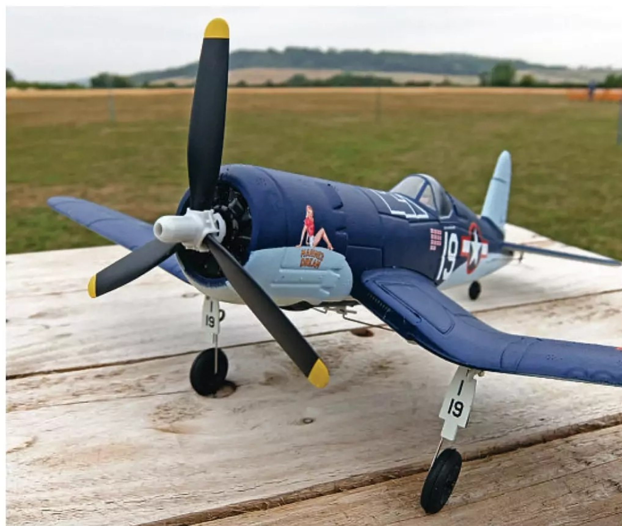
Behind the scale looking 3-blade prop is the clip-on prop saver. Removing the prop (and wheels) allows the model to be safely stored in its original box.
