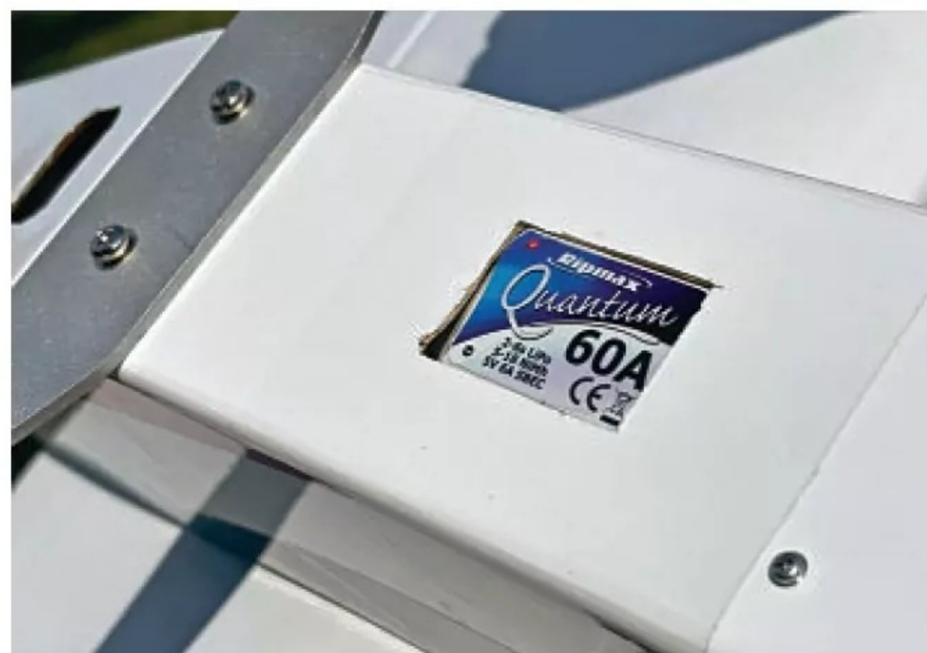
One solution is to cut an aperture in the fuselage underside.
