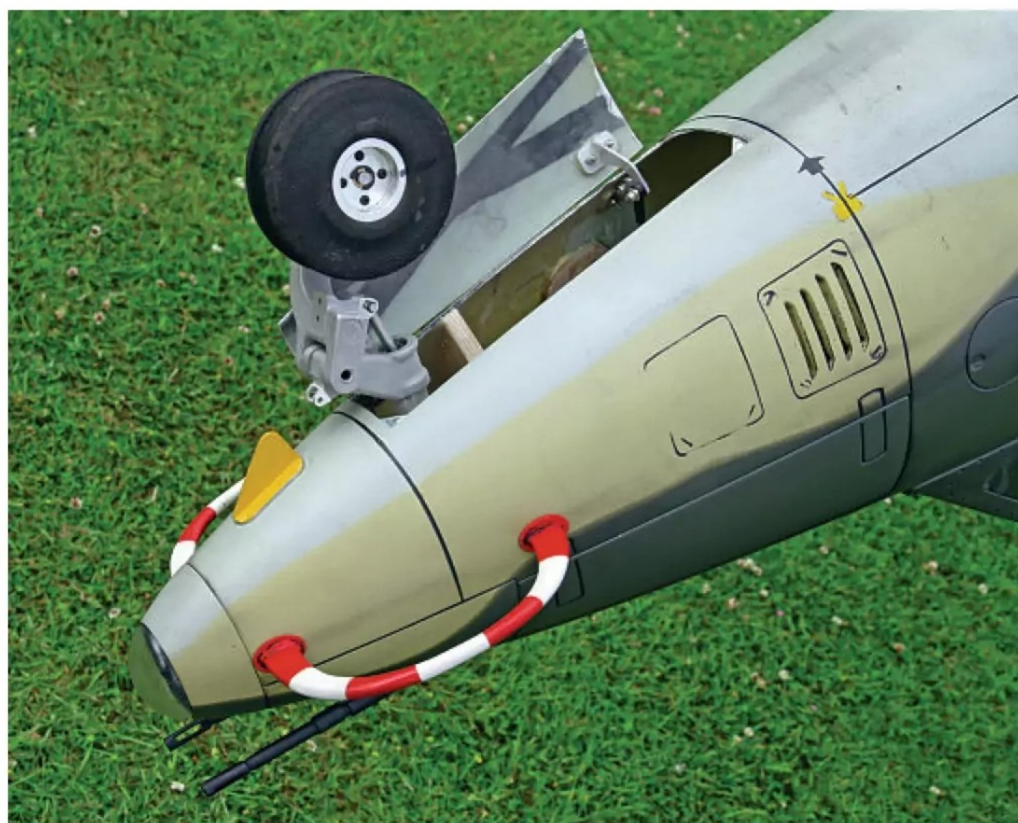
Nose gear strut and hub are Avonds Jet items, fitted with a homemade foam tyre to save weight.
