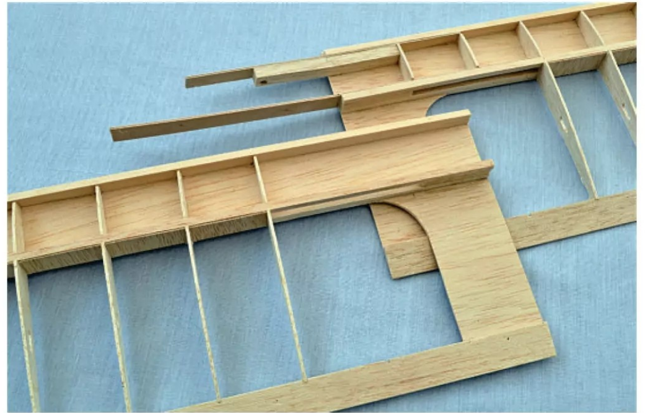
Ready for joining, the wing halves have the centre half-ribs added later.
