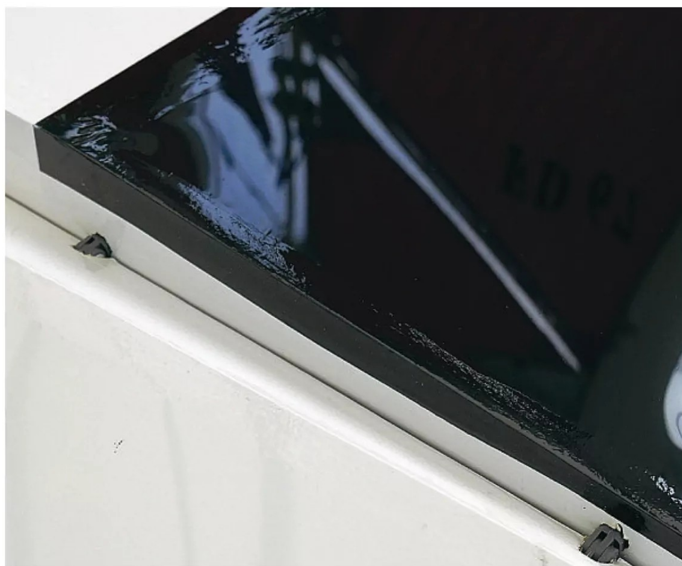
An aileron underside shows the tidy fit achieved by using a drilling jig.
