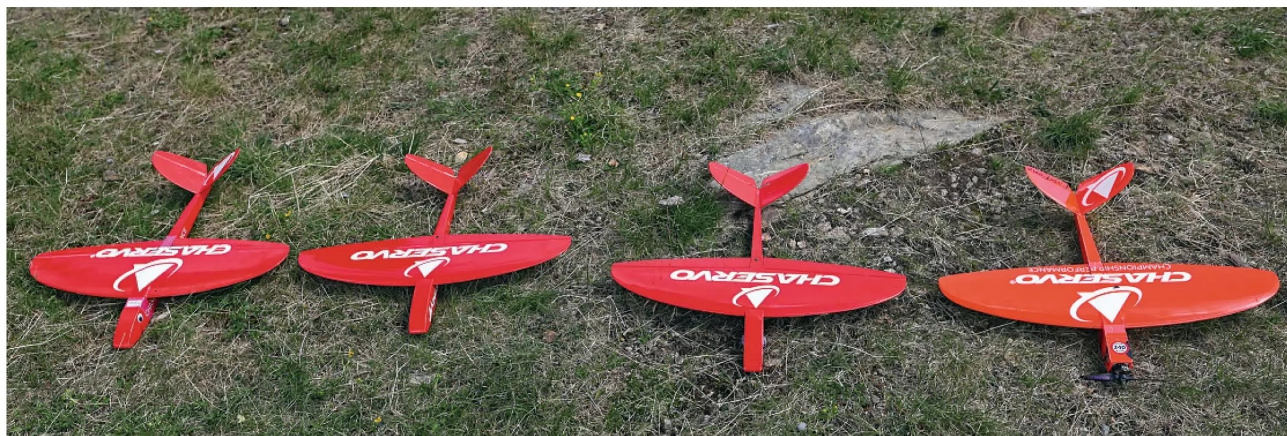
Brand new from CHAServo was the Firlefanx, now available as a ready-built RTF with 3 x DSO6 CHAServos. 50 cm wingspan, approx. 155 g take-off weight.
