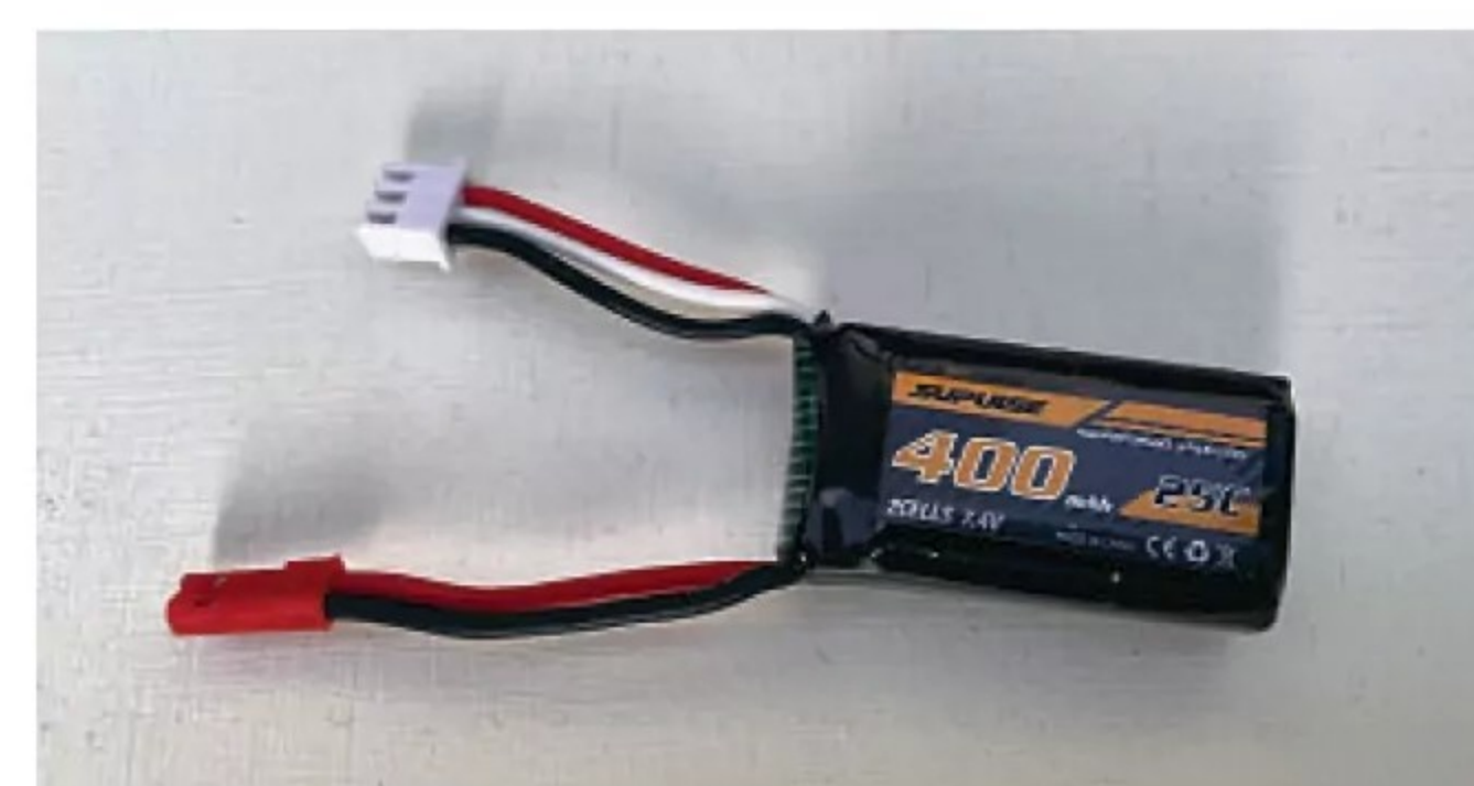
A USB charger is supplied with which to charge the 2S 400 mAh LiPo, but the JST lead and HX balance connector mean that it can also be used with a fast charger. You'll need a JST adapter lead to suit your charger.
