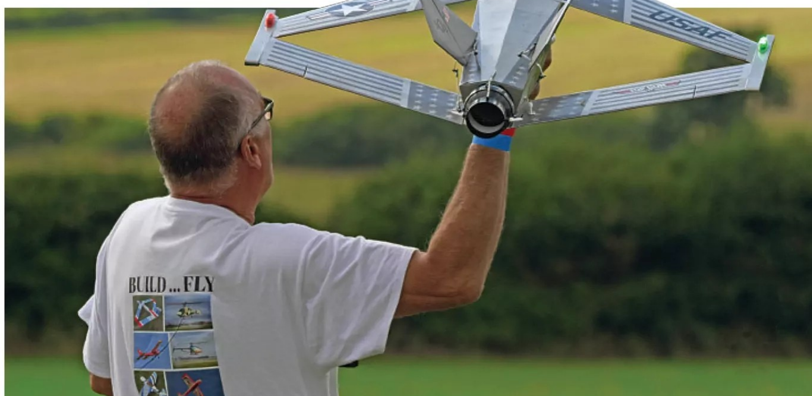
John Hutson launches his EDF Quark prototype powered by a 70 mm 4S Powerfun unit. Up to 4.5 minutes flight time, including vectored thrust.
