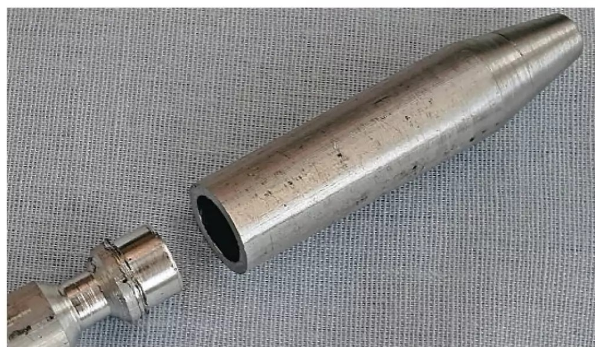
'Kingcat' silencer was made as a pressed together unit. Here the tail is fixed with the nose end to follow.
