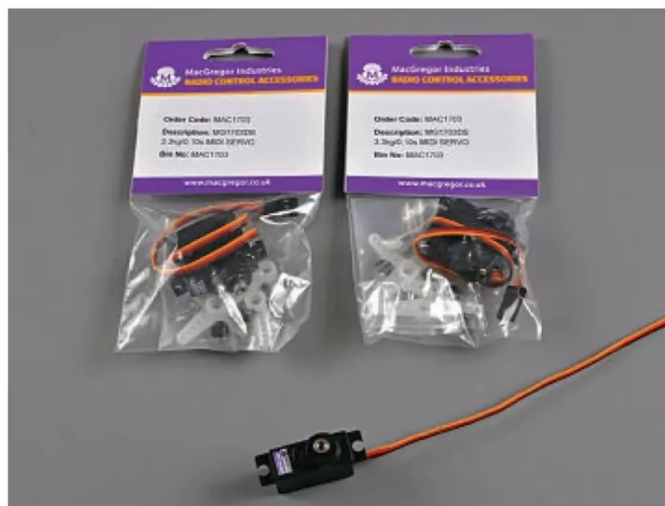
MacGregor MG1703DS midi servos were supplied to operate the ailerons.
