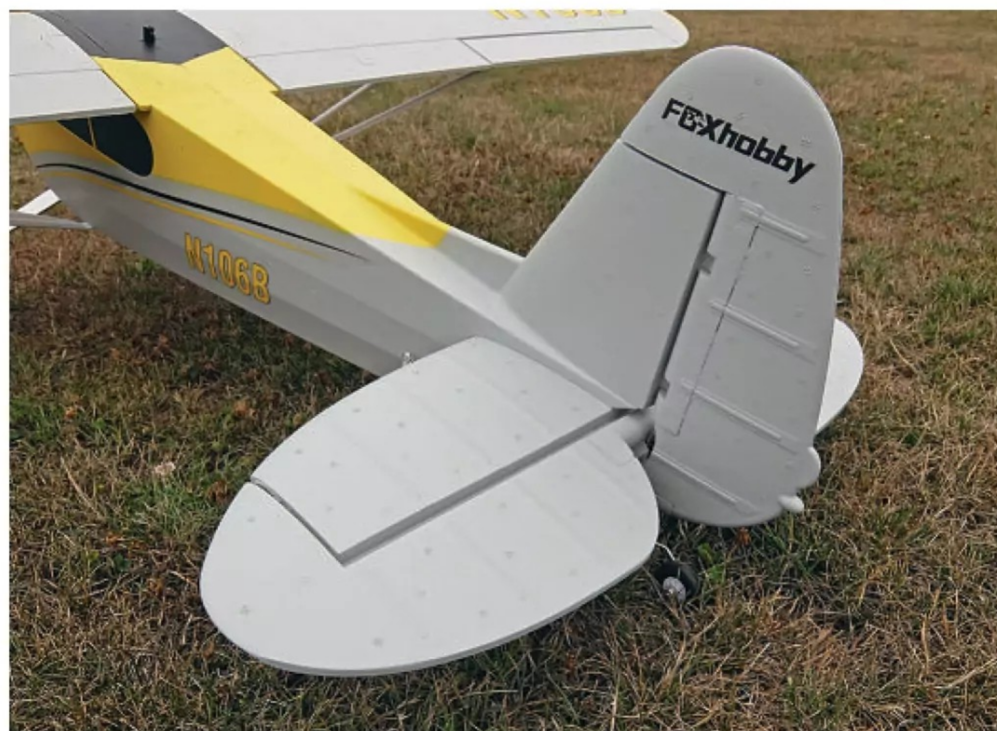
Tall rudder is simply clipped into place.
