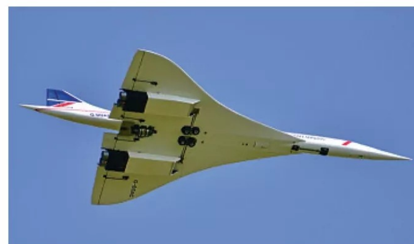
Underside view showing the single Wren 70N turbine nestled between the two flap servos. It looks rather small but powered the Concorde admirably!
