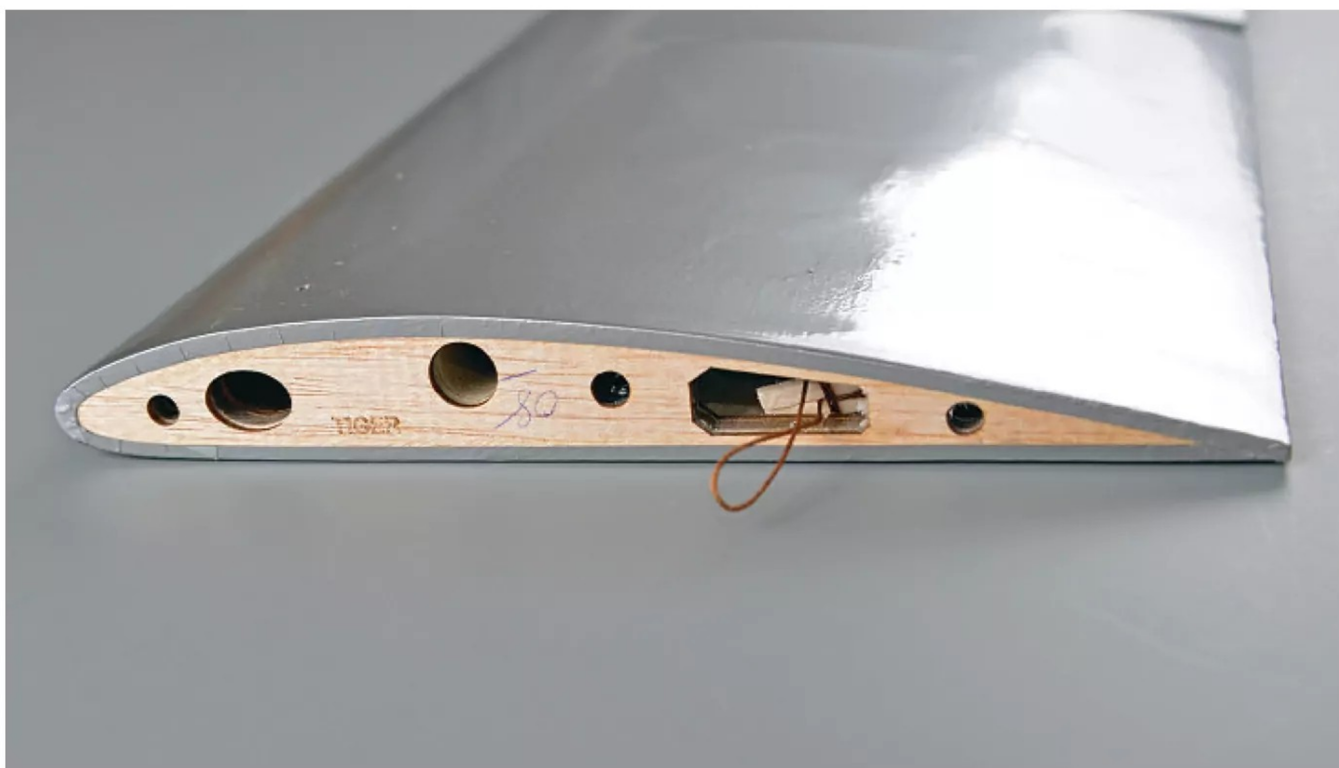
Lower wing root showing neat laser cutting and a repeat of the well-trimmed and folded over edges of the covering seen at the firewall.
