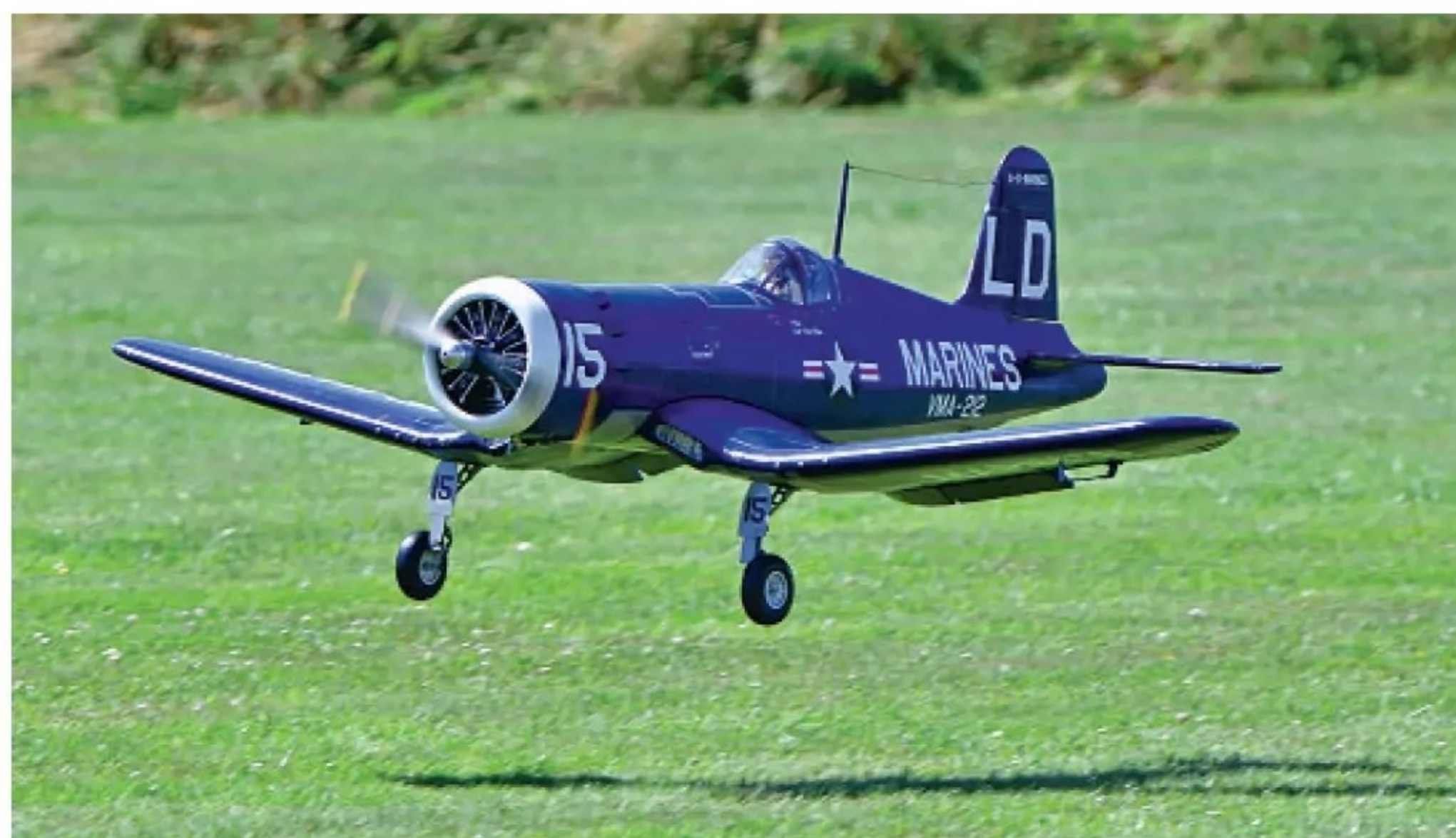
Jeff Fraser's 88" span, 1/5th scale Top Flite F4U Corsair is amply pulled along by its DLE55 engine and 22 x 10 prop.
