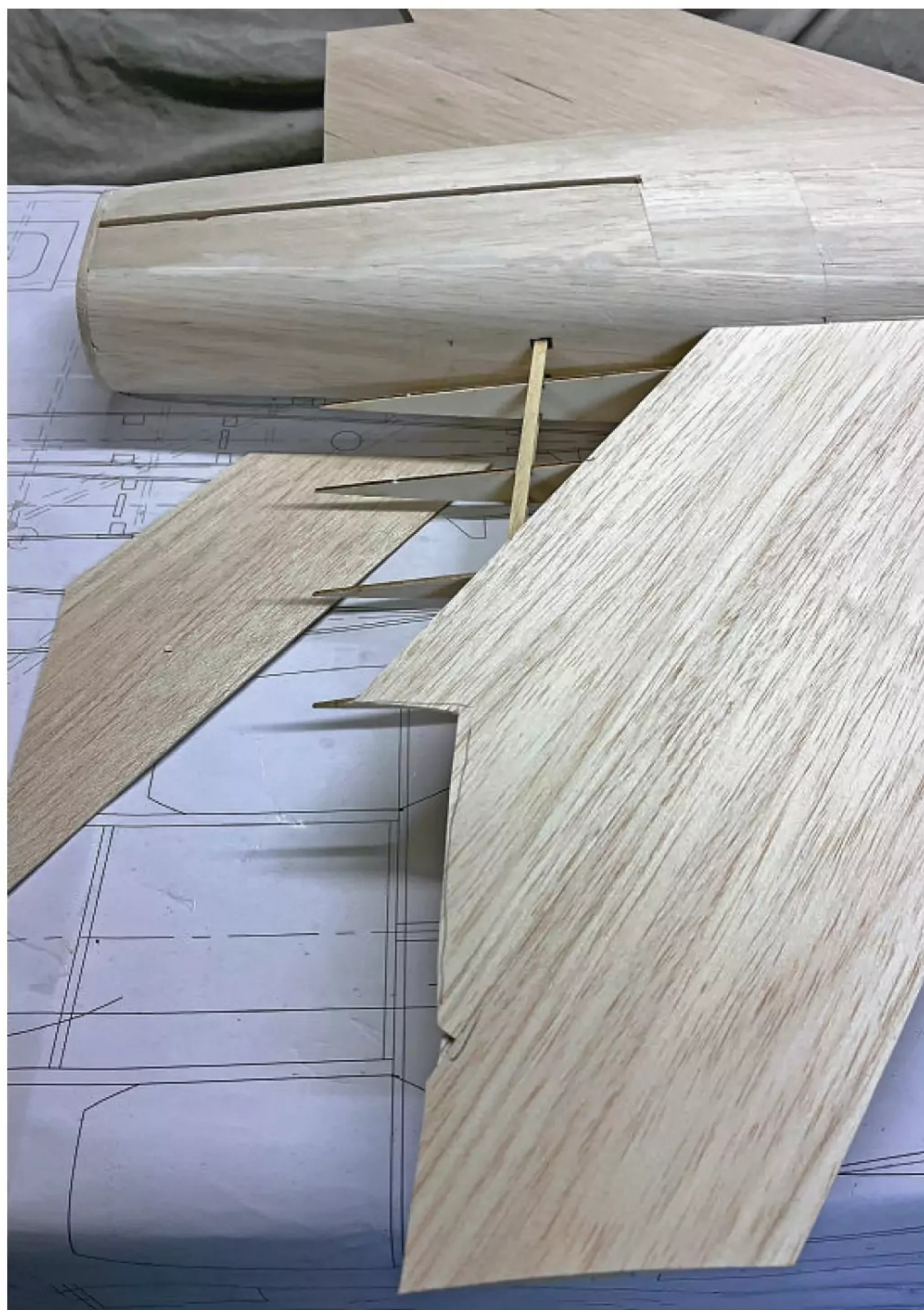
Using 1.5 mm balsa sheet the top of the wings from the leading edge back. Trim the sheeting to the finished wing perimeter.
