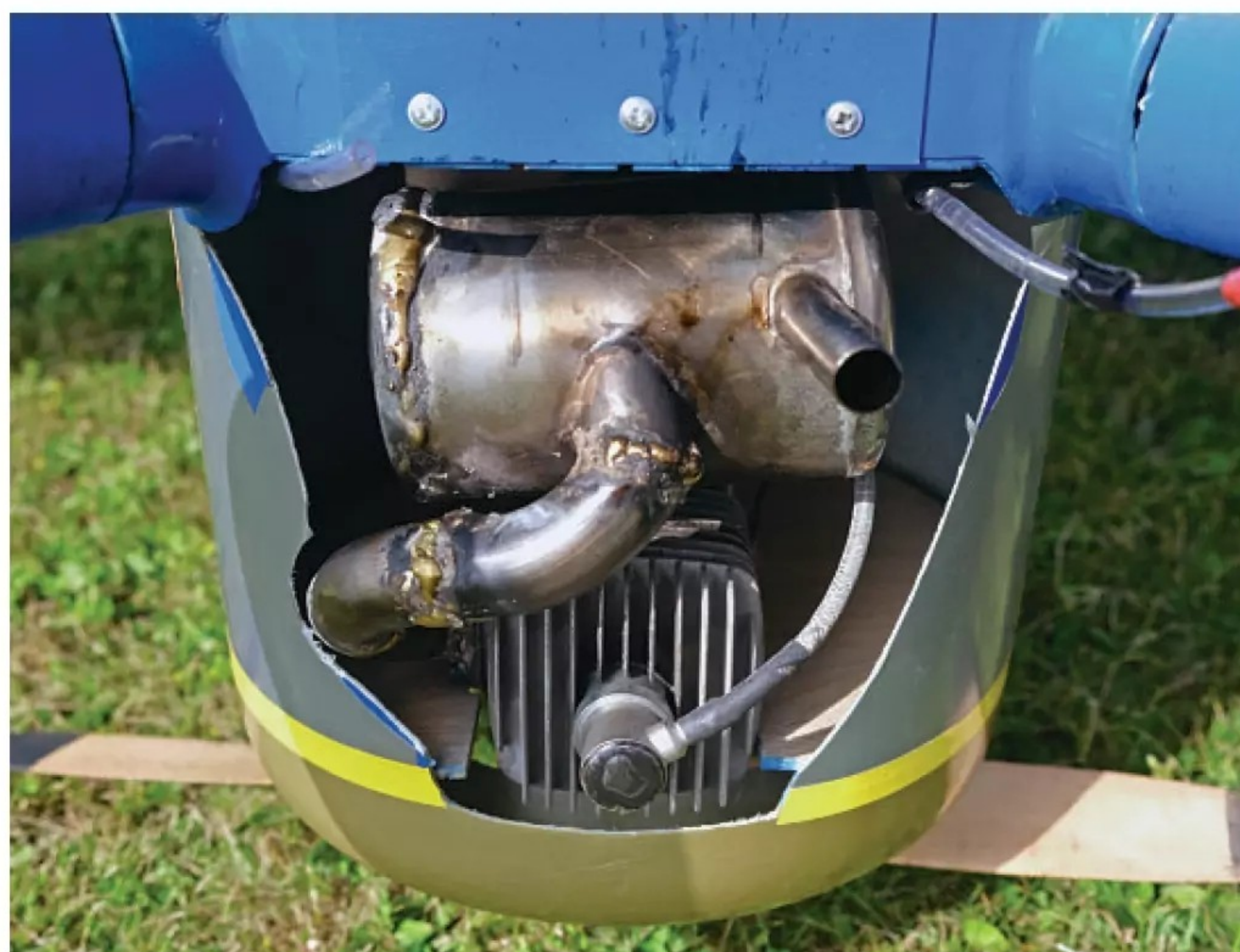
ZDZ 70 is silenced by a Zimmerman Zenoah 62 silencer modified by Colin using Krumscheid stainless exhaust bends and a ZDZ compatible exhaust flange.
