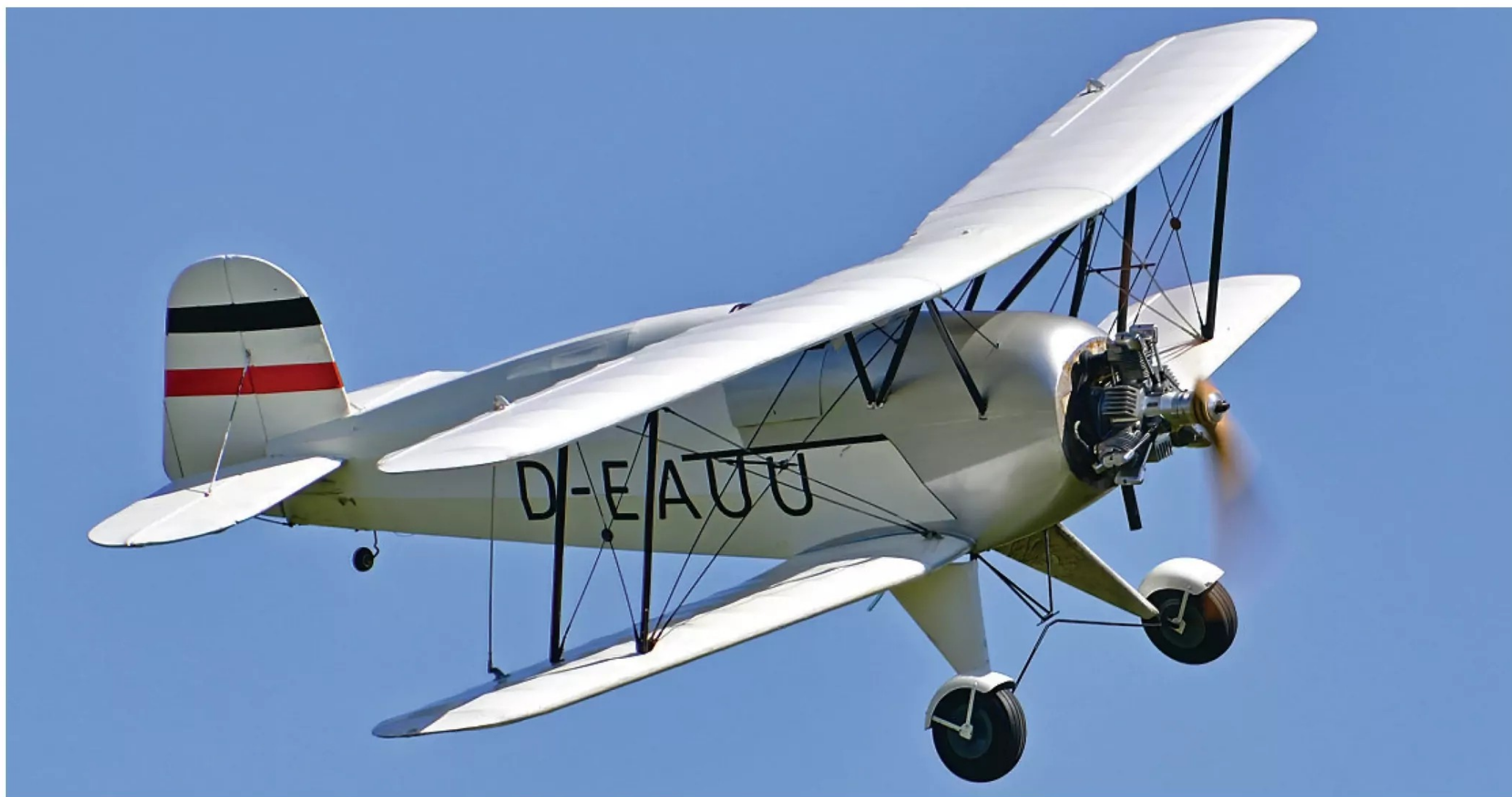
Father and son team Simon and Tom Wood brought several models to the show. Here's Tom's 86" span 1/3rd scale Jungmeister which was built from the Gary Allen kit and powered by a Saito FG-90R3.
