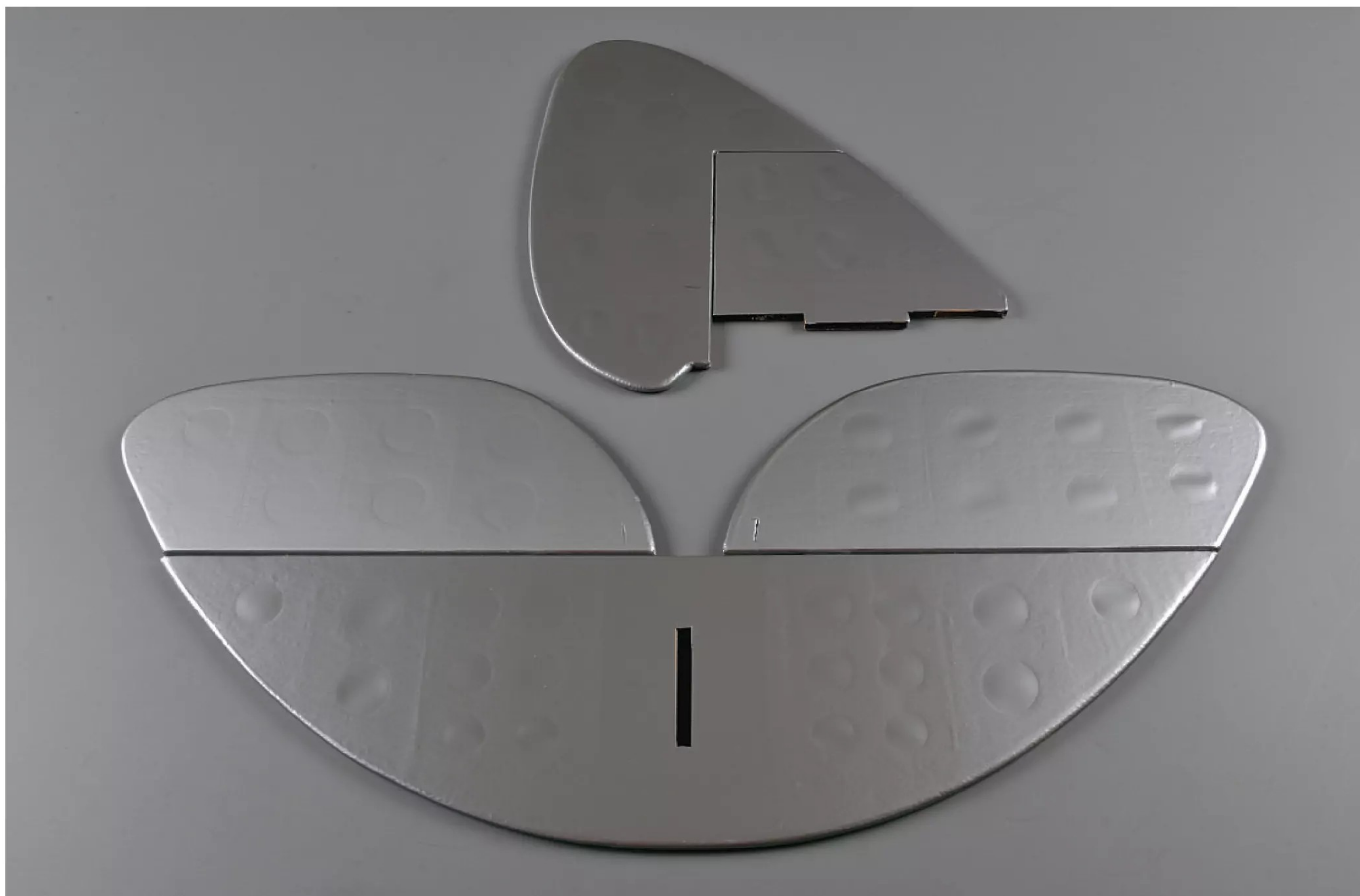
Distinctive Tiger Moth style tail feathers come fully sheeted but are lightened with many round holes.
