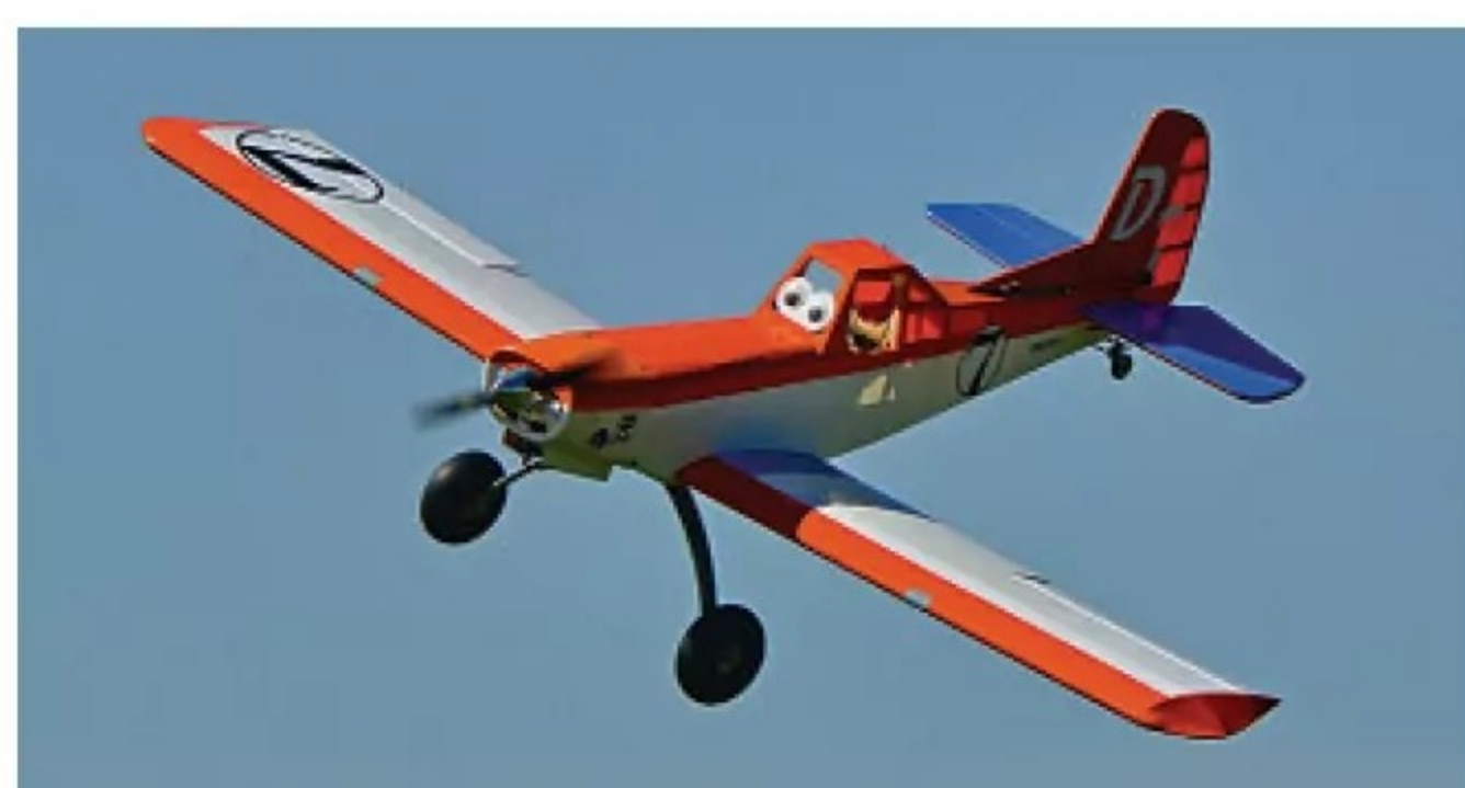
Kyle Millet flew his Farmyard in the 'Dusty Crophopper' colour scheme from the Planes film. 96-inch span and powered by a Zenoah 38 cc petrol engine.
