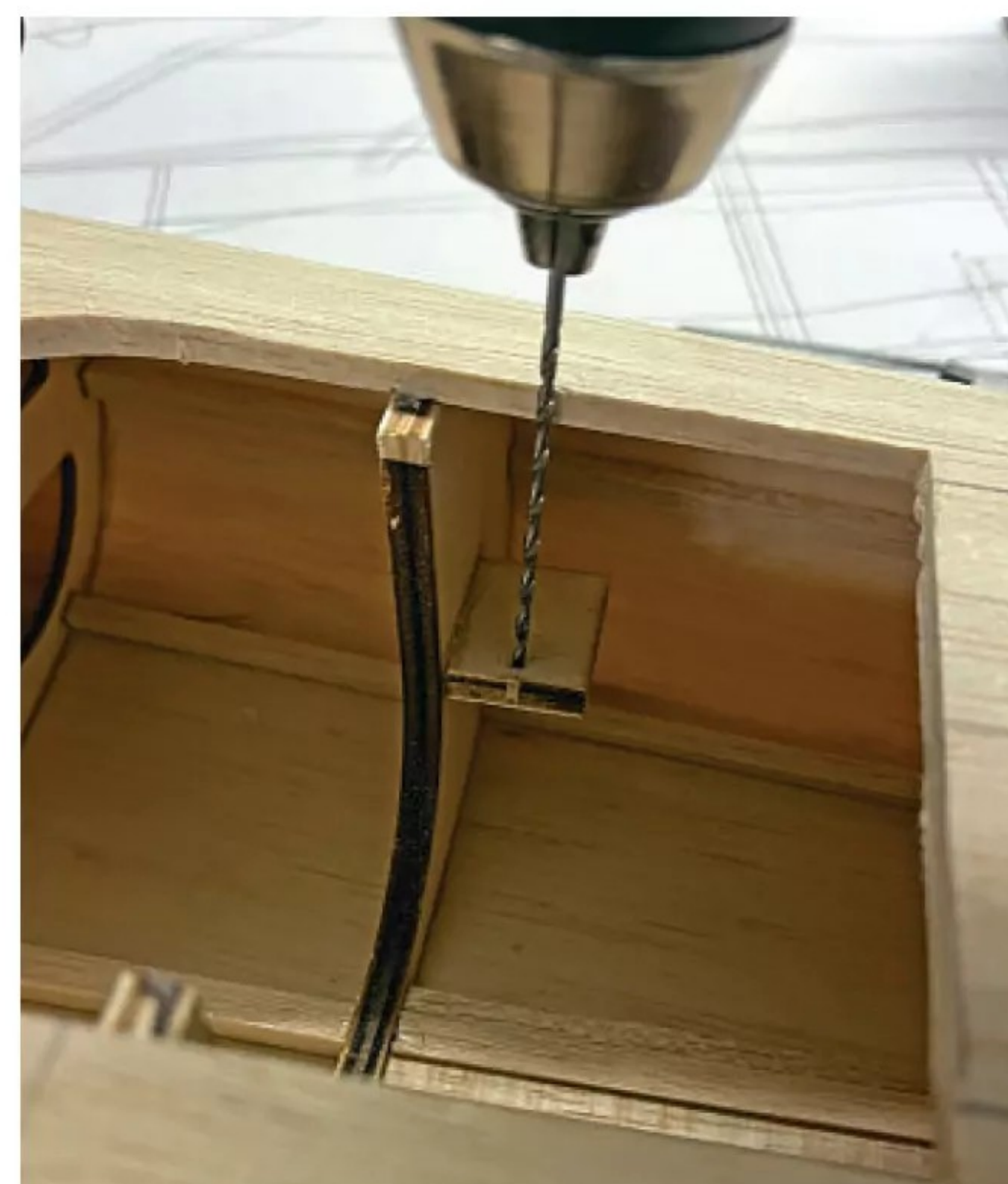
Drilling the fan mounting plates.
