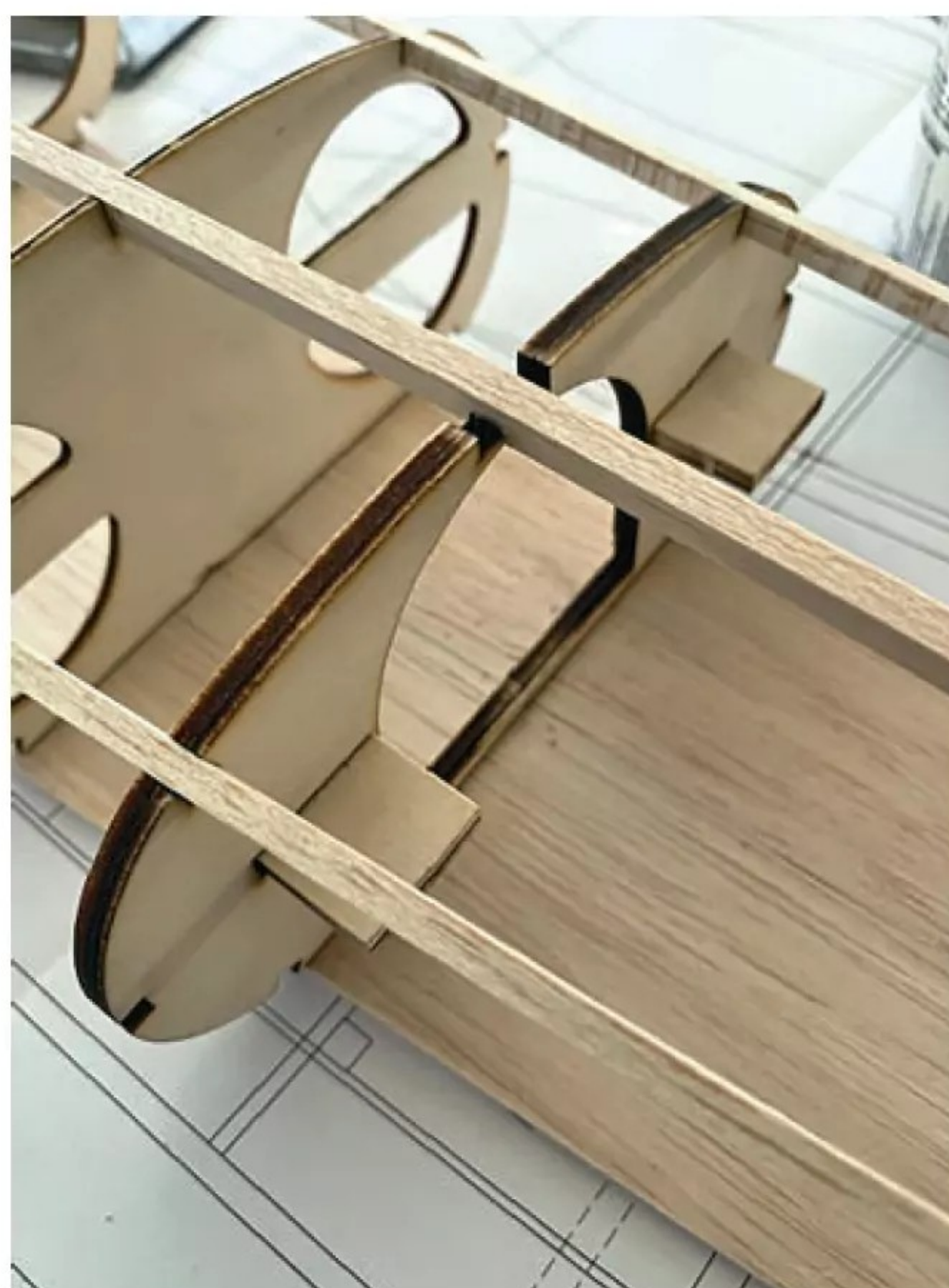
Glue into position the fan mounting plates FM1.
