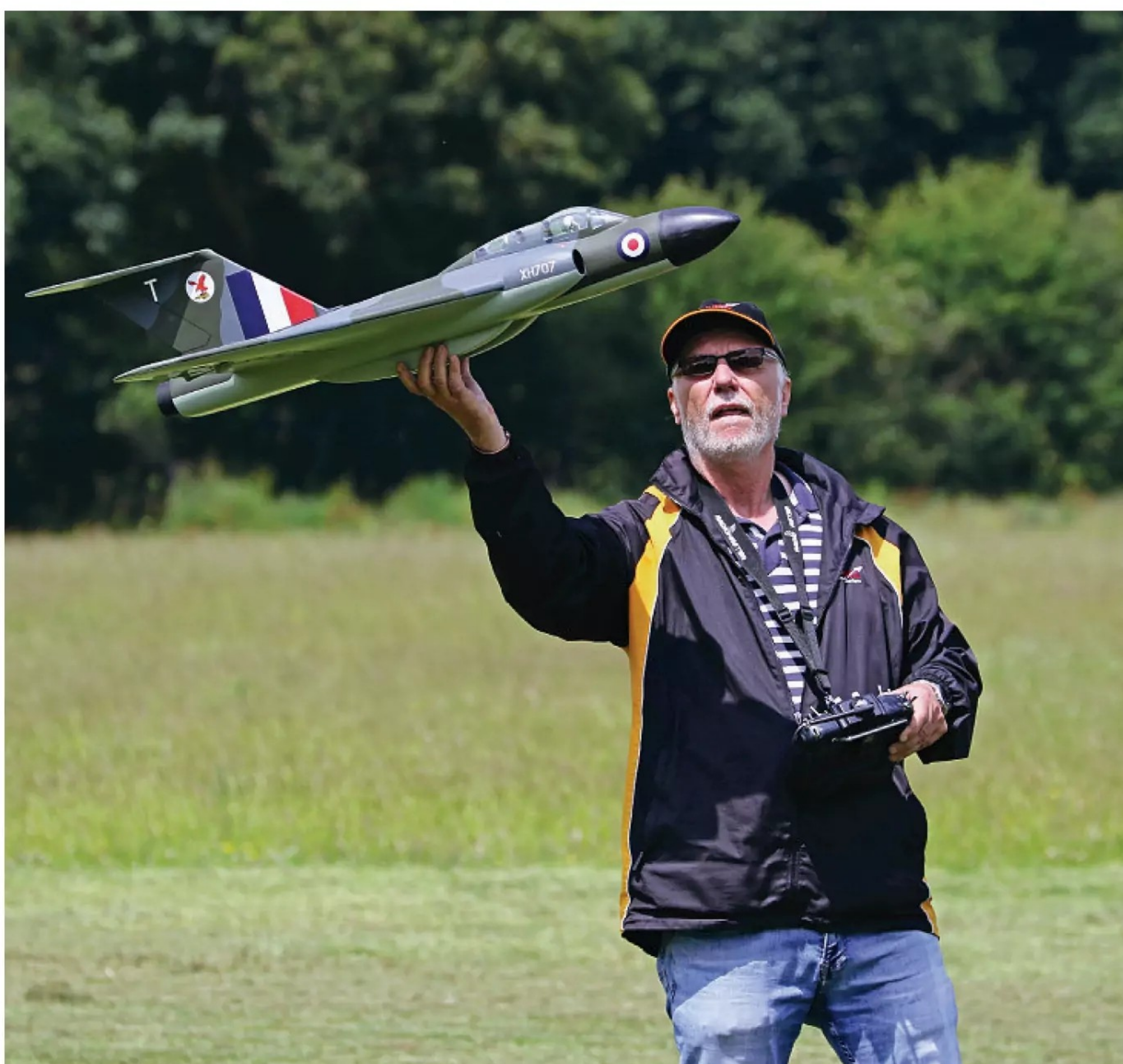
Two dummy under-pods allow for a good grip when hand launching.
