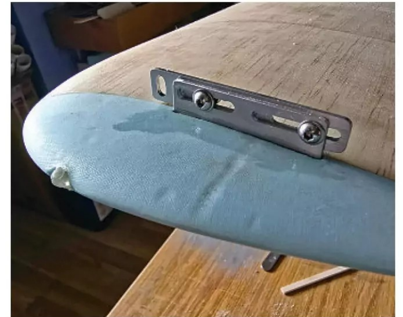
Using my mill, I made an adjustable lead-out guide. I run both lines through the one hole.
