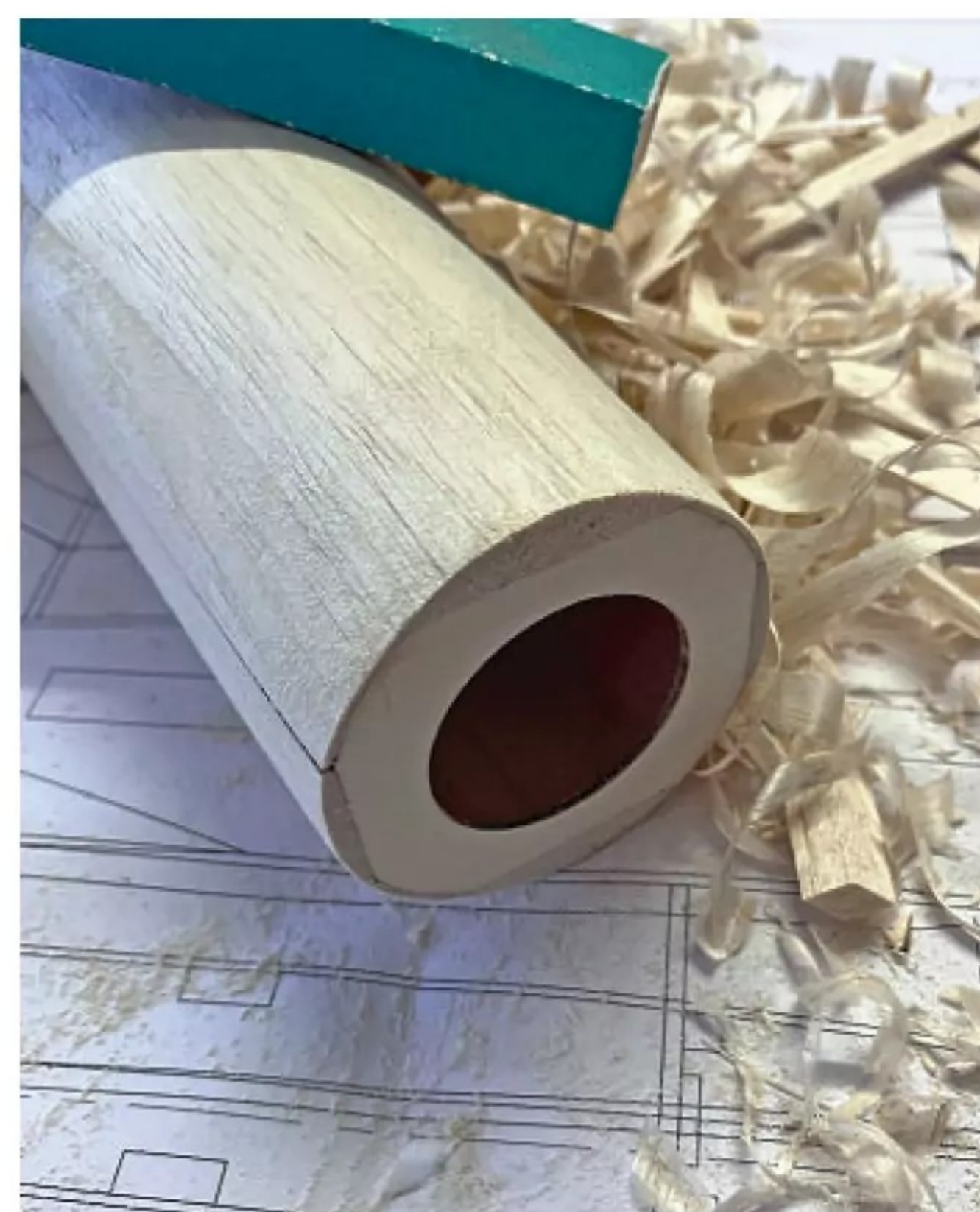
Plane and sand the top and bottom edges flush with the formers then add the top and bottom sheeting using 9.5 mm balsa. When dry shape the fuselage to a smooth, round radius.
