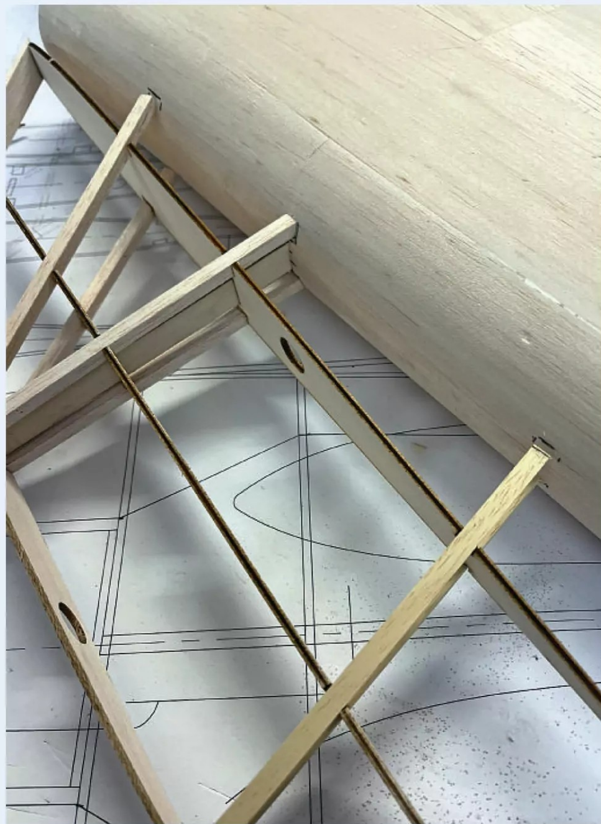
Where the spars touch the fuselage, mark and cut out the openings for these to pass through.
