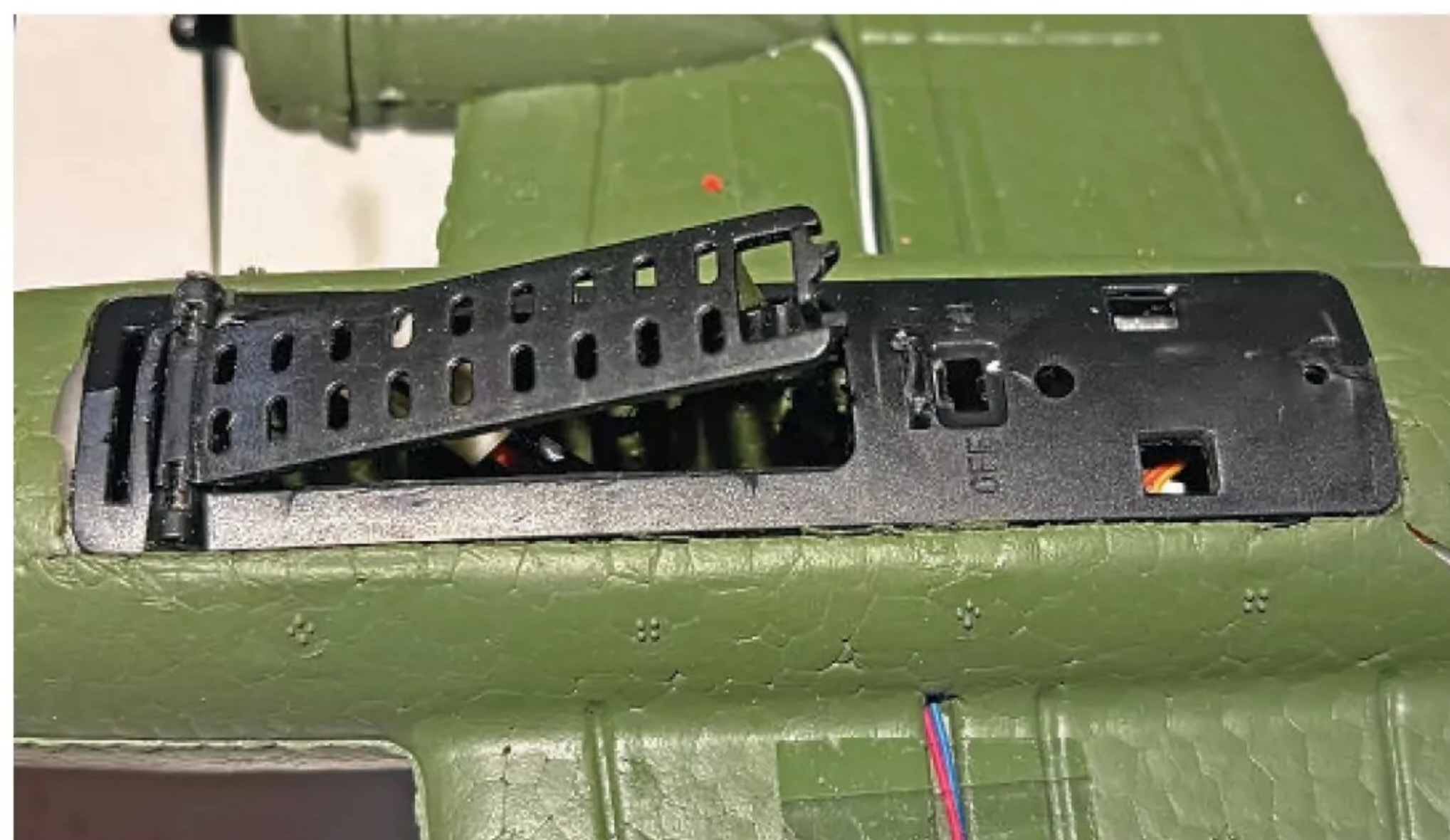
The replacement micro-Rx and original LiPo fit in with room to spare.
