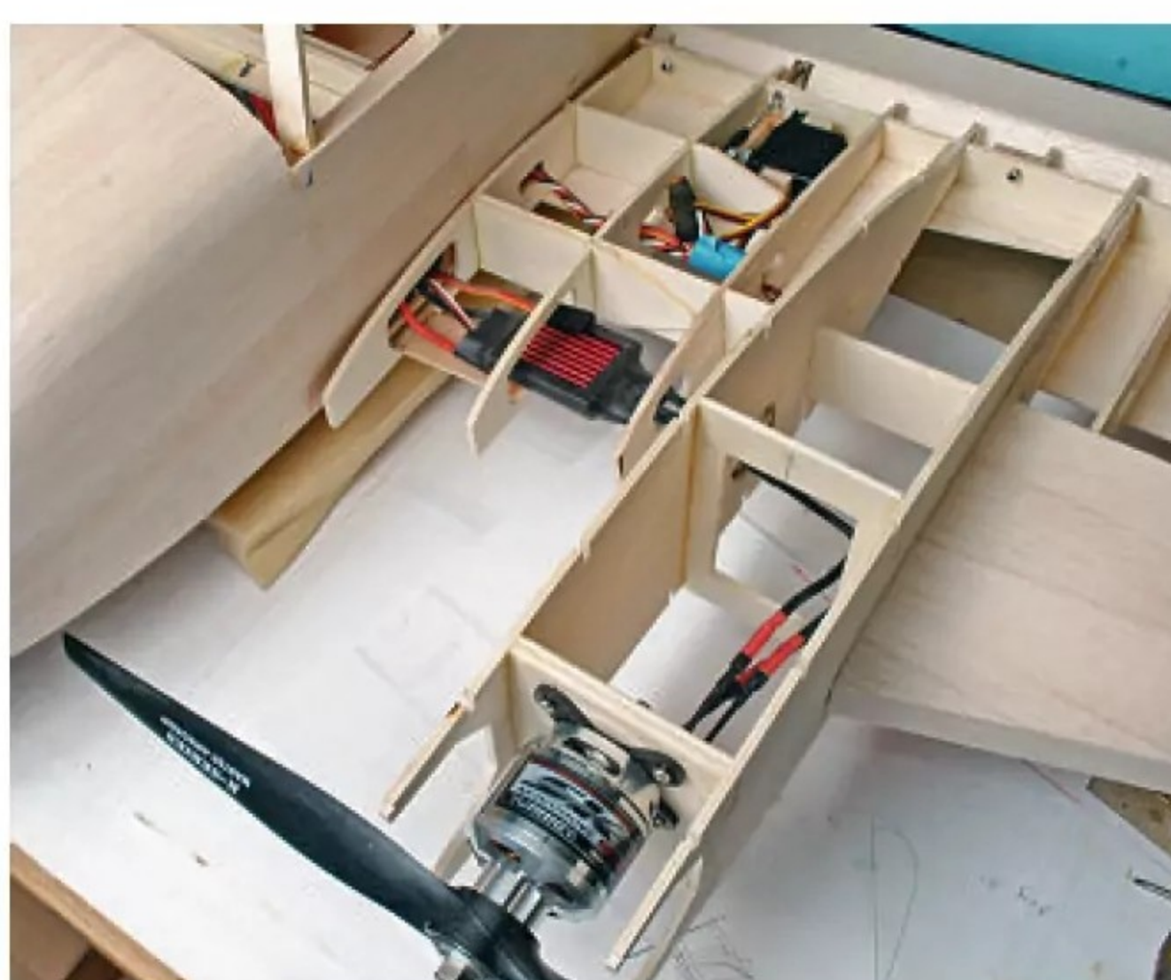
This picture shows one of the ESCs located in the leading edge. Also visible is the flap servo with internal linkages.
