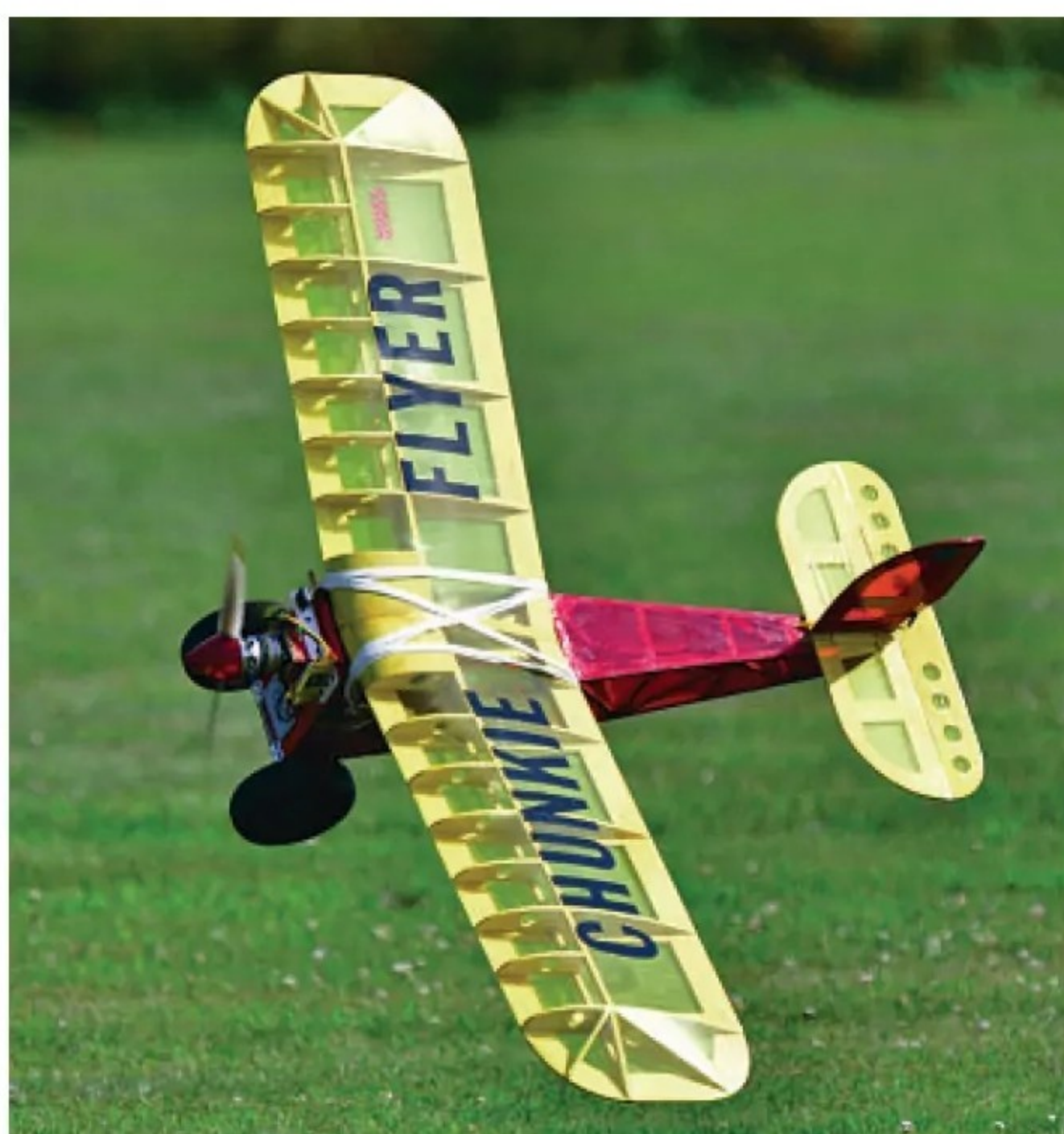
Simon Wood and his son's double sized Chunkie, the original of which is available from Sarik Hobbies (MW2939). 48" wingspan running off a brushless outrunner, 40A ESC and 3S 2200mAh LiPo.
