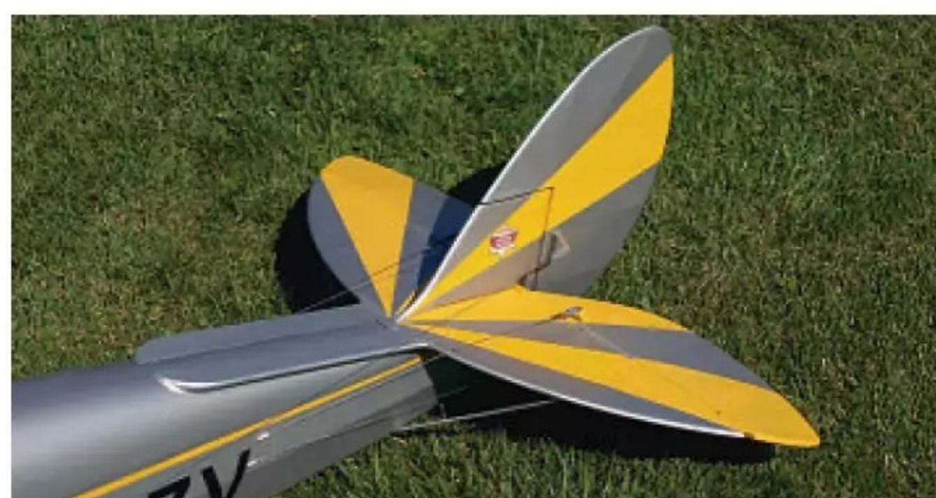
The Tiger Moth has three separate closed loop systems for the rudder and each elevator half. I bet that lot took some setting up!
