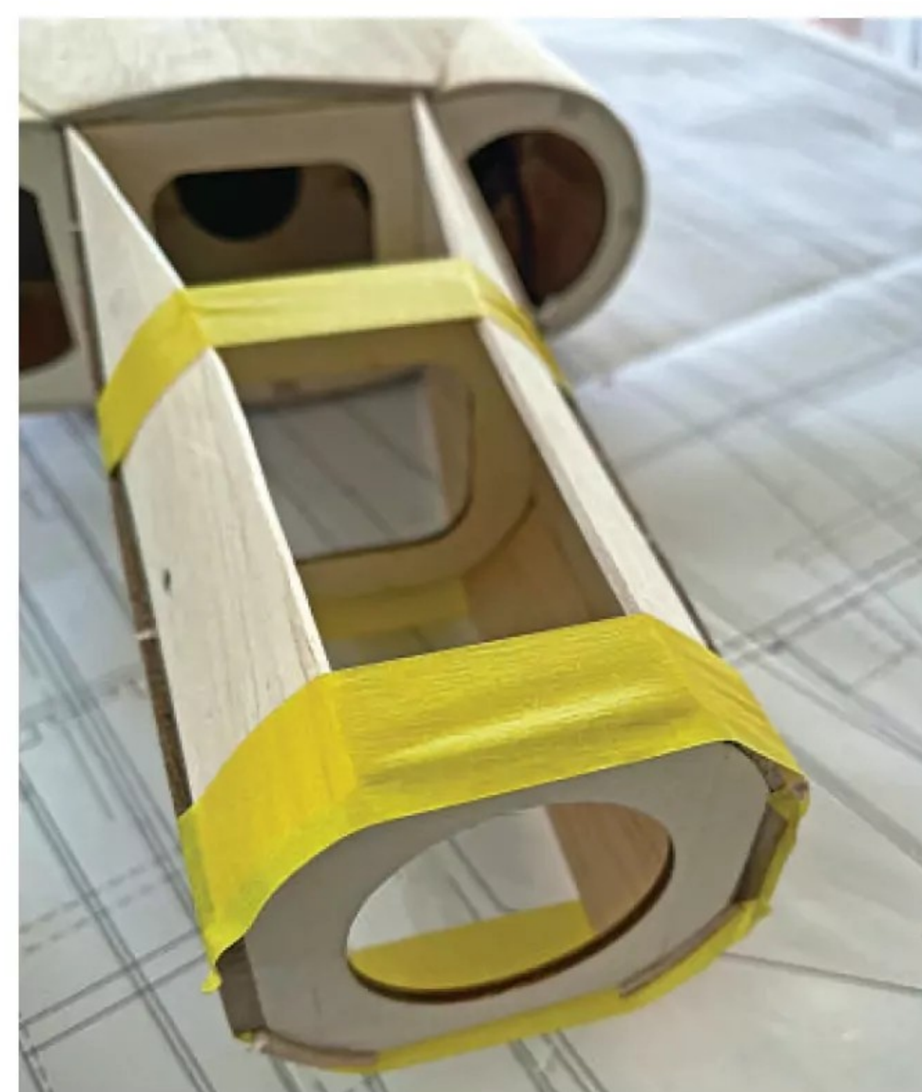
Four pieces of 2.4 mm sheeting form the sides of the front fuselage. Wet the outside surface of the sheet to assist in bending and glue into position.
