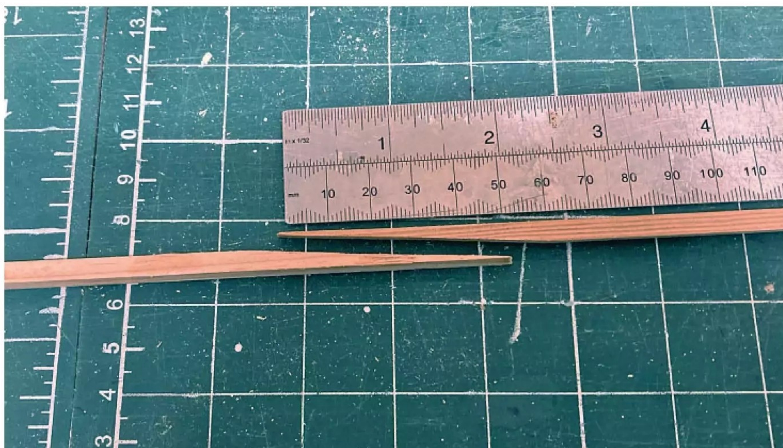
These 5 mm square spars show a join ratio of 10:1.
