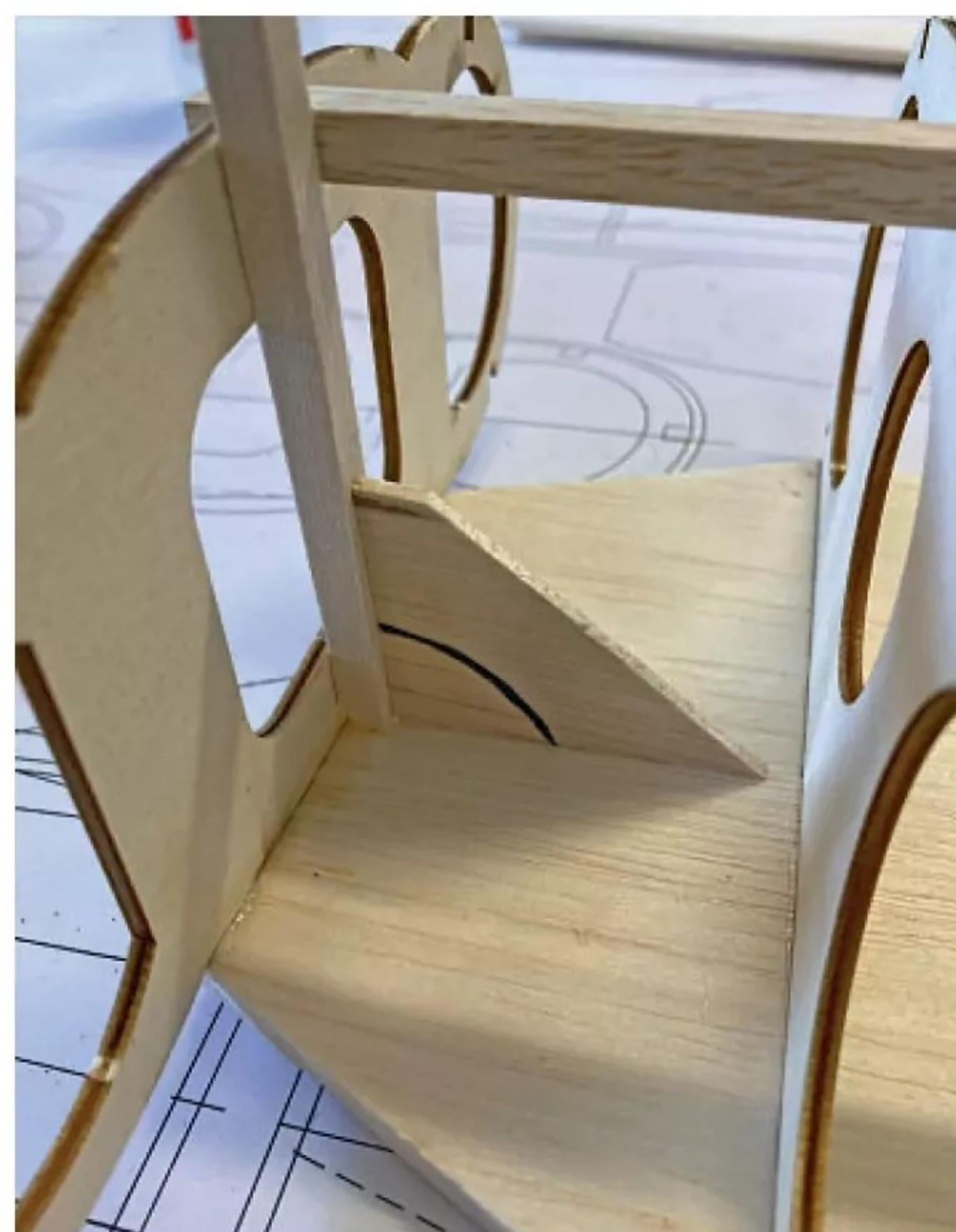
Use the templates shown on the plan to align the formers at their correct angles.
