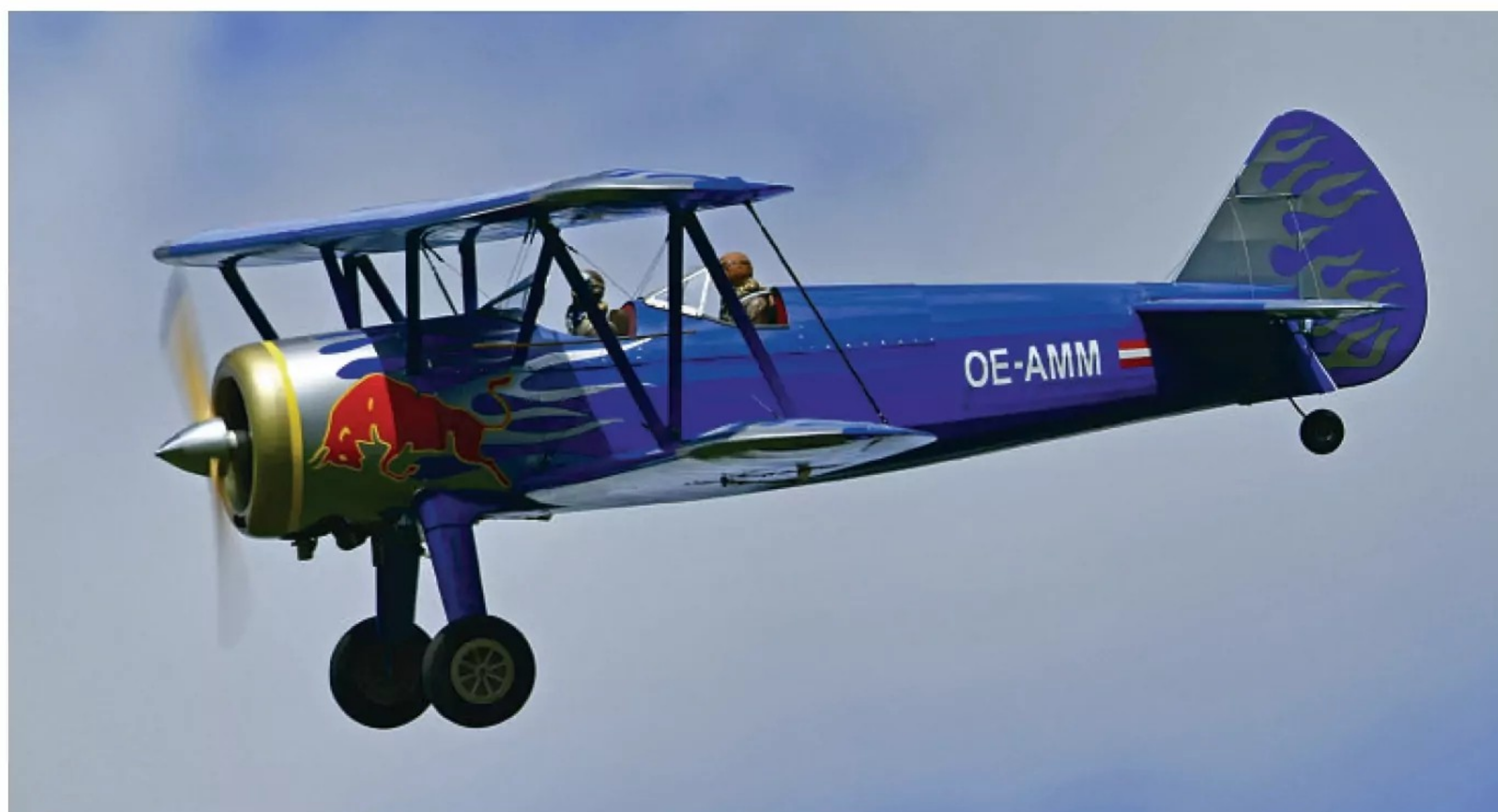
Colin's model is based on the Flair Products kit and is 1:4.3 scale with a wingspan of 89 inches.
