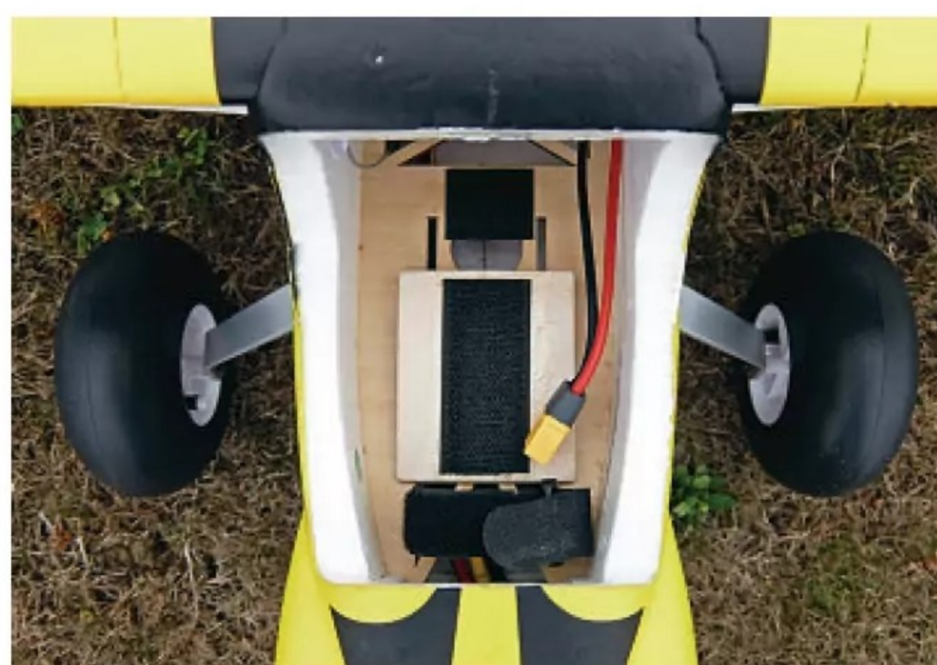
With Radiant's 4S 2200 mAh LiPo relocated as far forward as possible a new battery seat was glued in for extra support. The LiPo strap was brought forward too.
