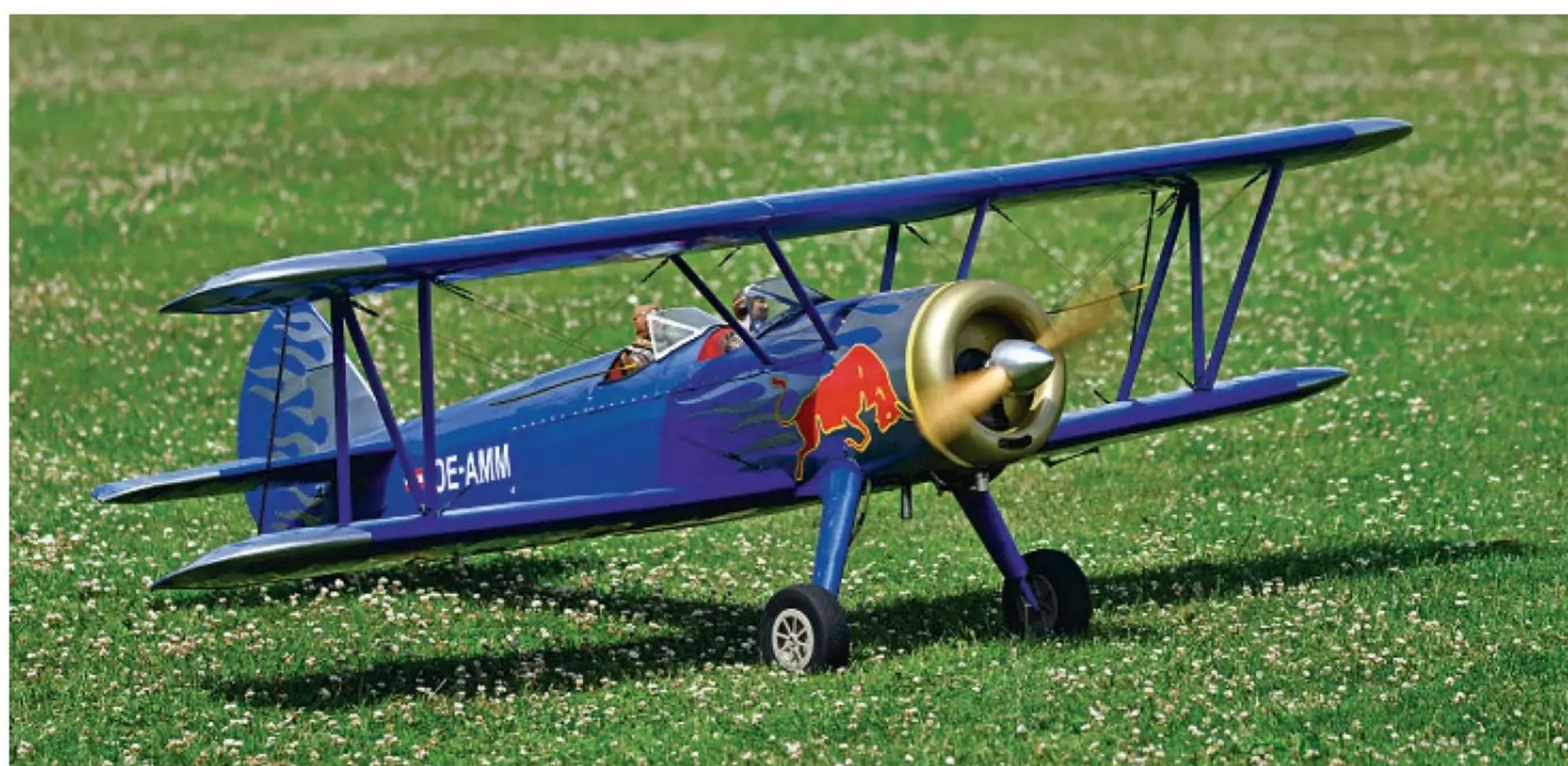
Performance was lacking with the original four stroke, so a ZDZ 70 engine was fitted turning a Punctilio 22 x12 wood prop.
