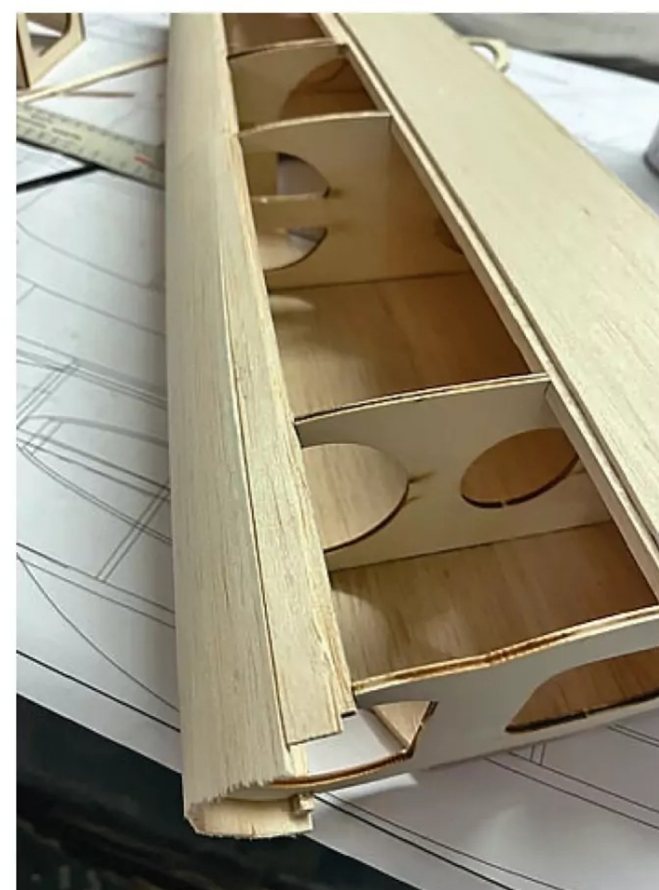
Use soft 2.4 mm sheet balsa to sheet the fuselage sides. Wet the outside surface to aid bending.
