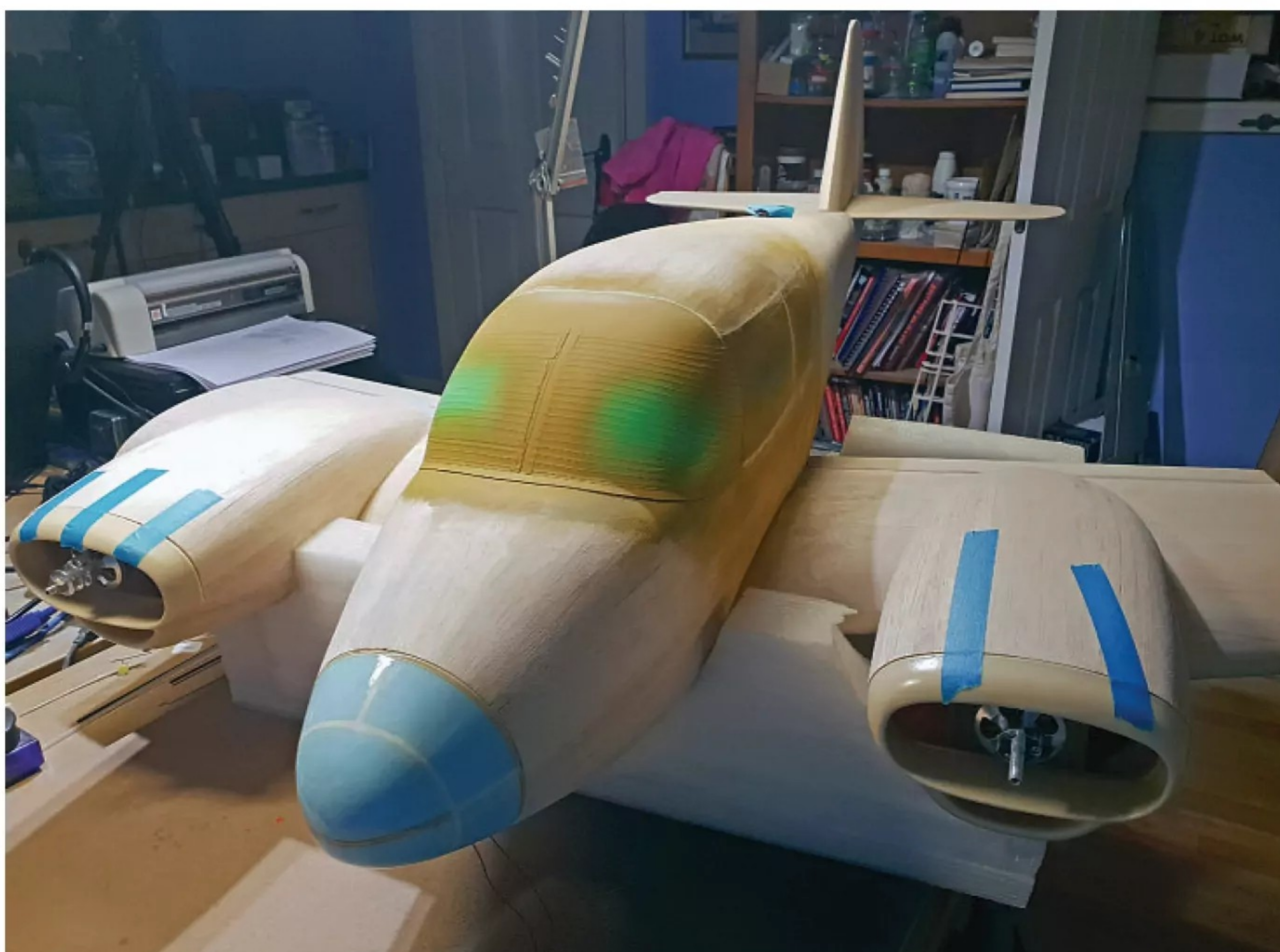
The nose piece simply mounts on screw heads in slots and a slight twist secures it.
