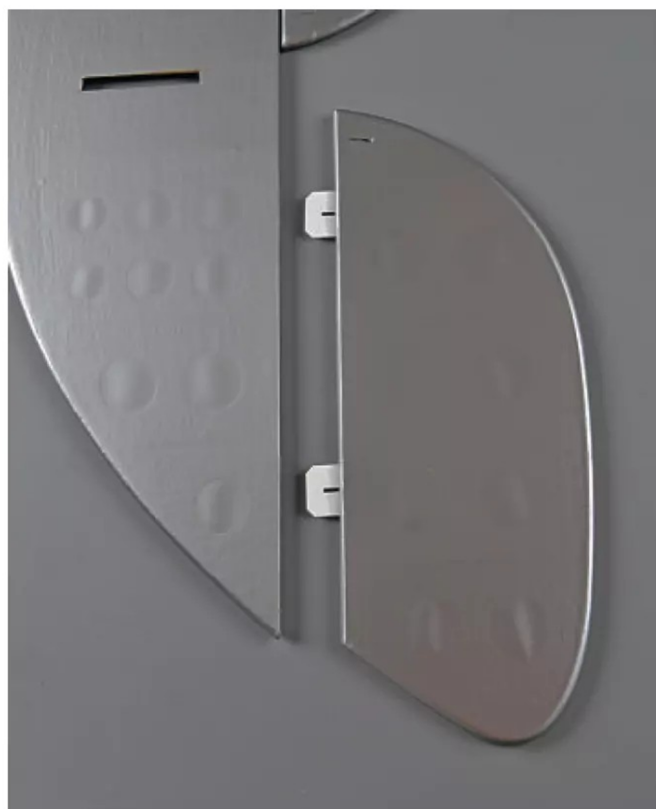
Hinges are dry fitted so will need gluing in place, with cyano carefully wicked into the central slots.
