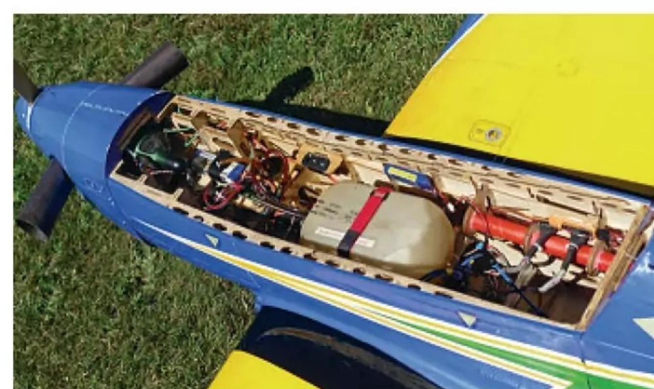
Underneath the canopy of Steve Kilbon's ARTF Tucano showing all the paraphernalia required for the Wren 44N Turboprop turbine and radio control. That one litre fuel tank gives it around eight minutes of flight time.
