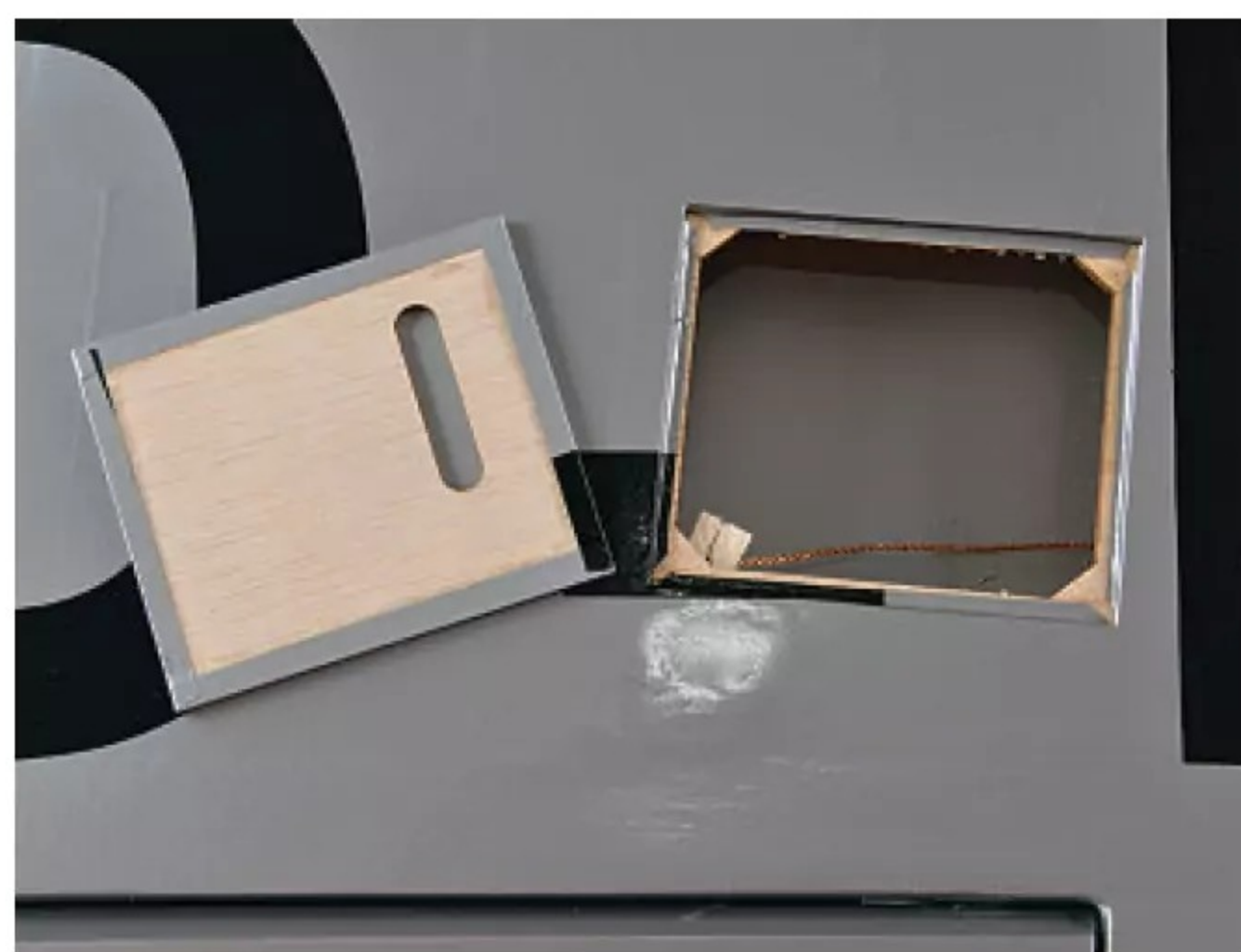
Aileron servos need to be mounted on the back of the servo hatches.
