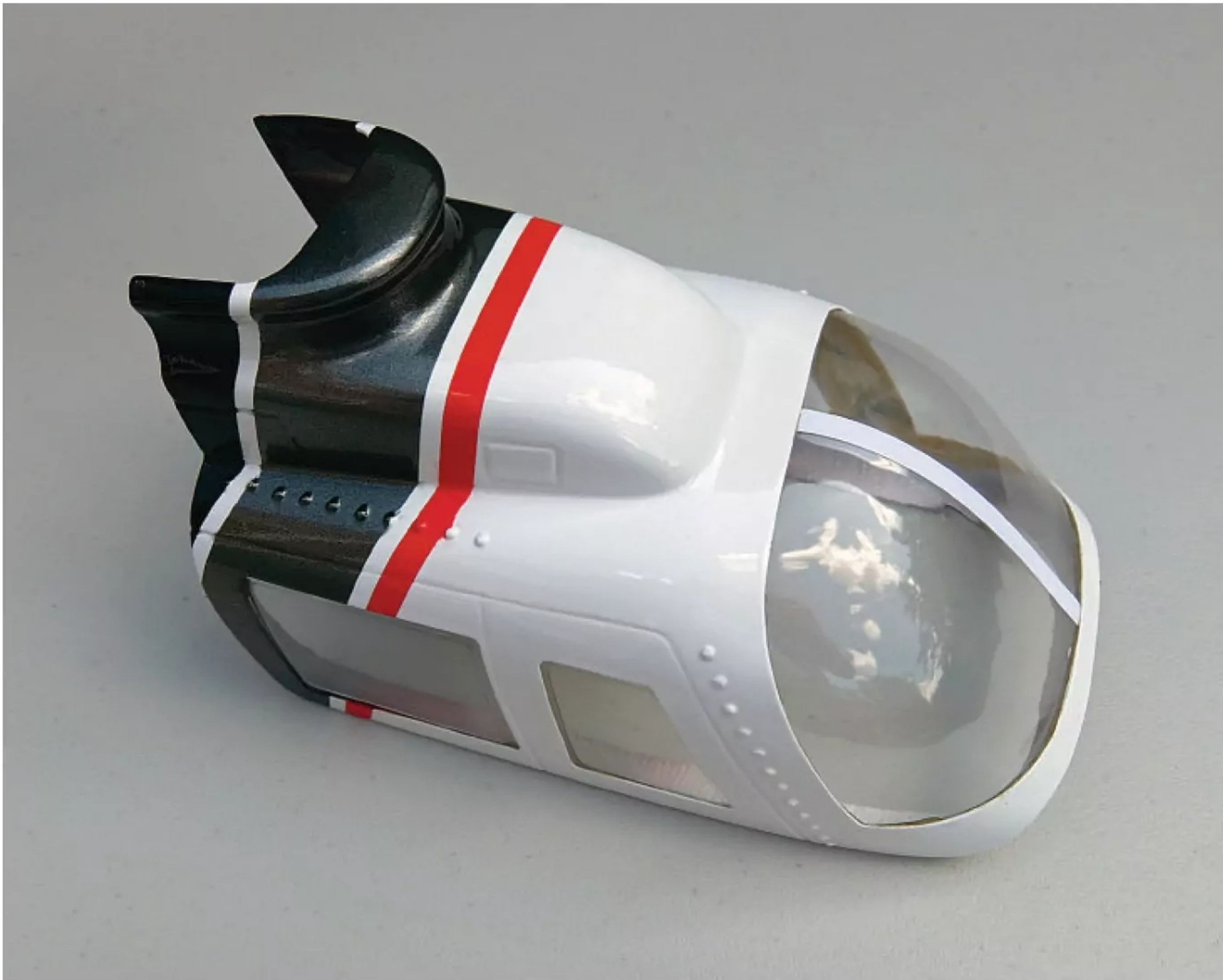
A spring latch allows for speedy removal of the canopy to give access for quick battery changes.
