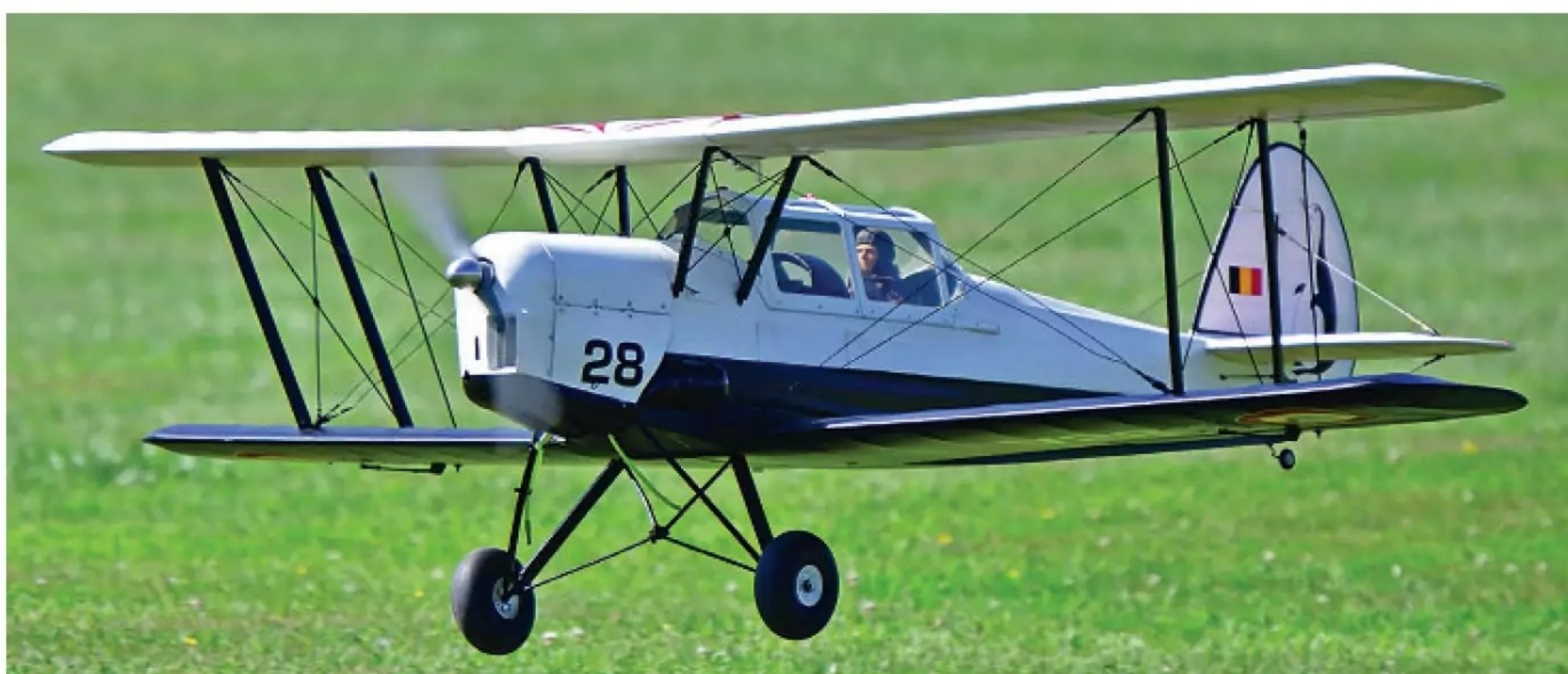
Simon Wood's Stampe SV-4B from the Svenson kit is finished in the livery of a Belgian aerobatic team called 'The Penguins'. Rigging wires are fully functional and it takes a while to assemble, but it's worth the effort as it looked great in the air.
