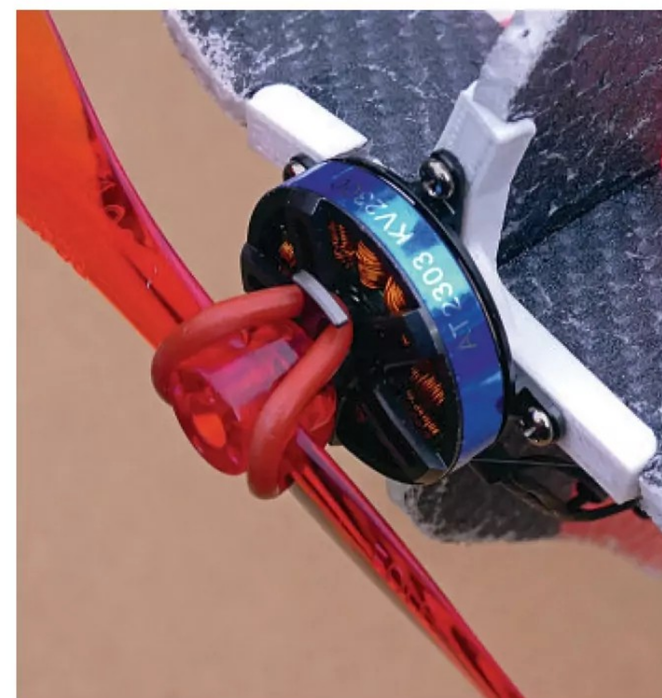
This low-cost motor proved to have plenty of power. Fitting higher quality ELO eight and nine-inch props have proved worthwhile.
