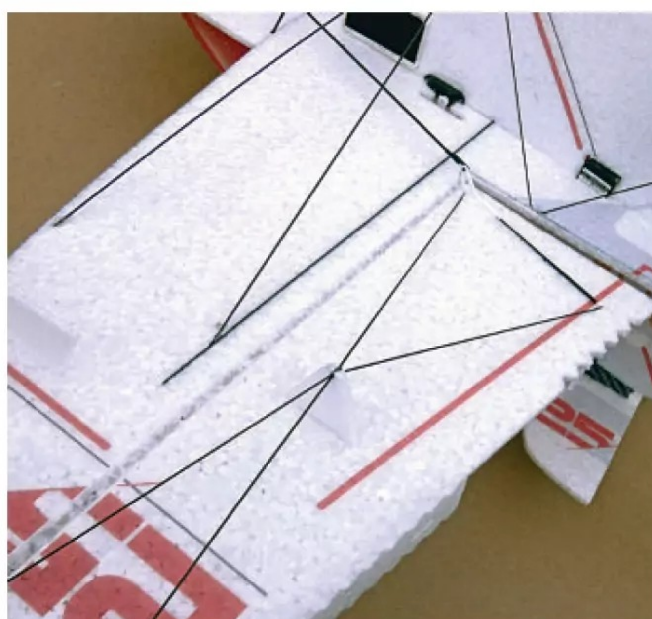
Lots of CF bracing gives the model its required rigidity.
