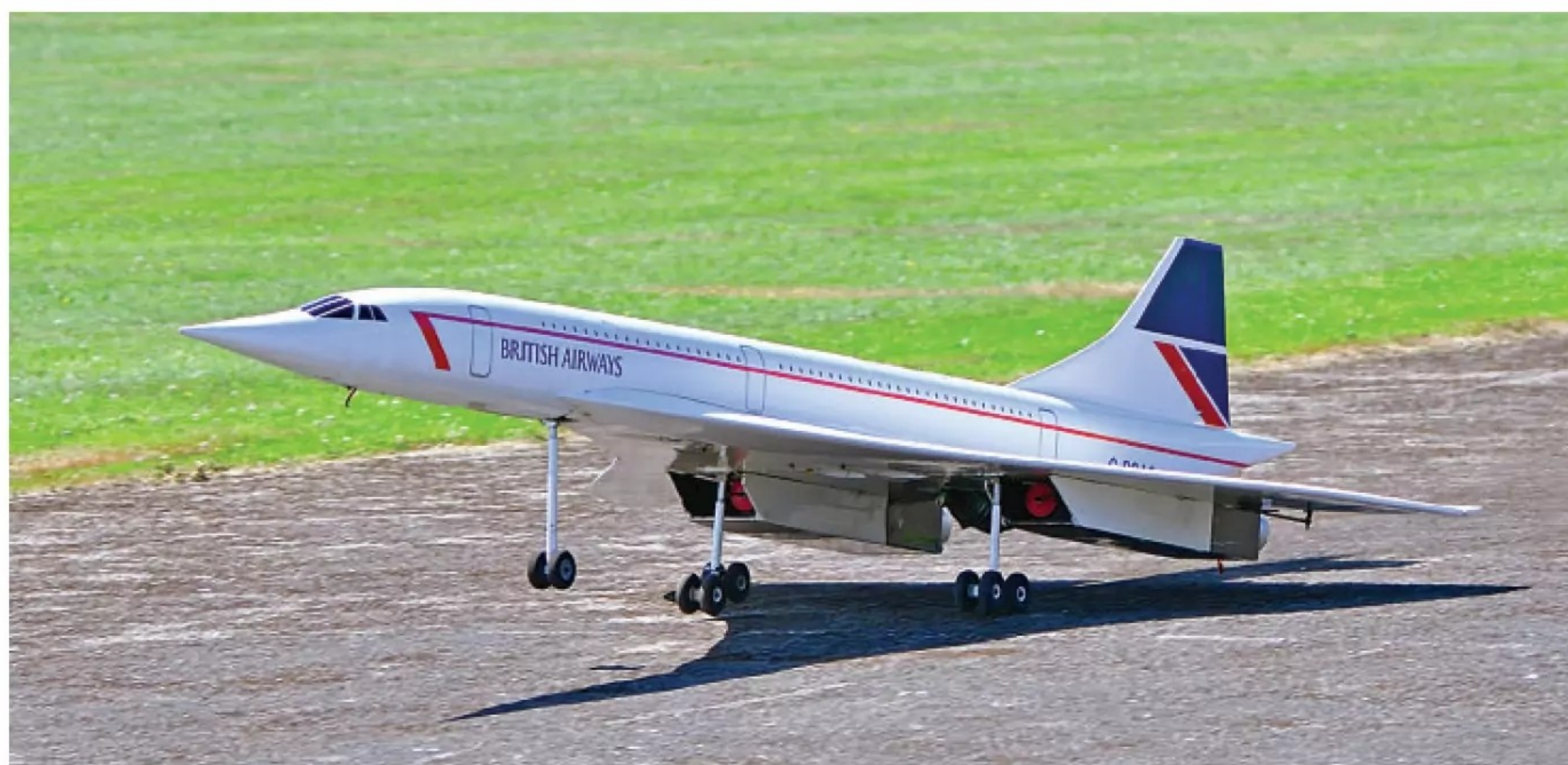
Concorde gets away easily thanks to its cleverly hidden single Wren 70N turbine. Those red cylinders in the intakes are two of the three one litre fuel tanks, giving around eight minutes of flight time.
