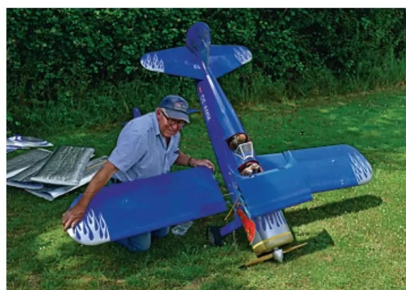
Top centre section is attached to the fuselage by cabane struts with the wing panels mounted via aluminium spars located into corresponding sockets.
