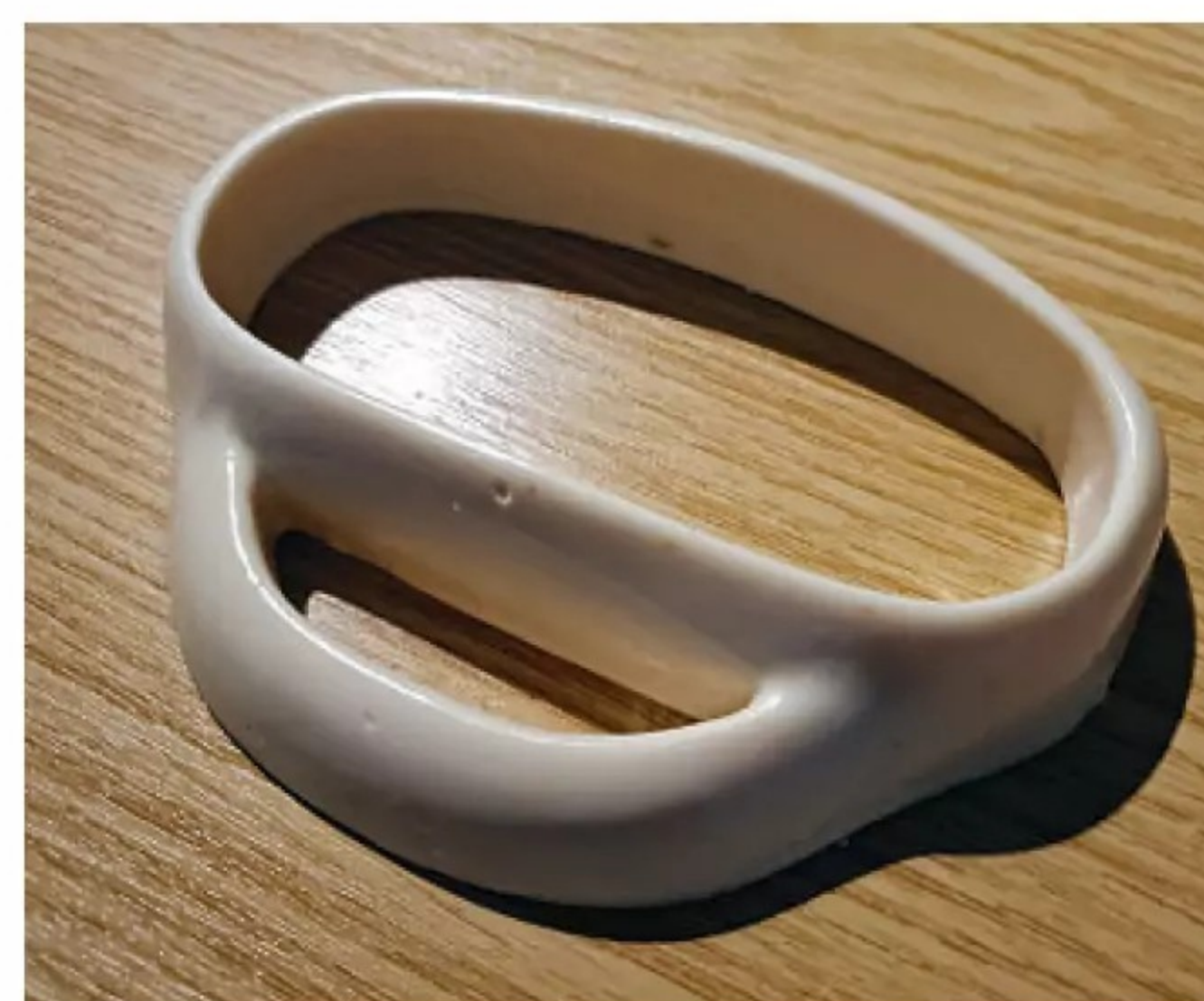
Cowl nose bowls were made in blue foam, then silicone moulds were made to create the final pair. It turns out the shape is slightly wrong so I will have to add some material.
