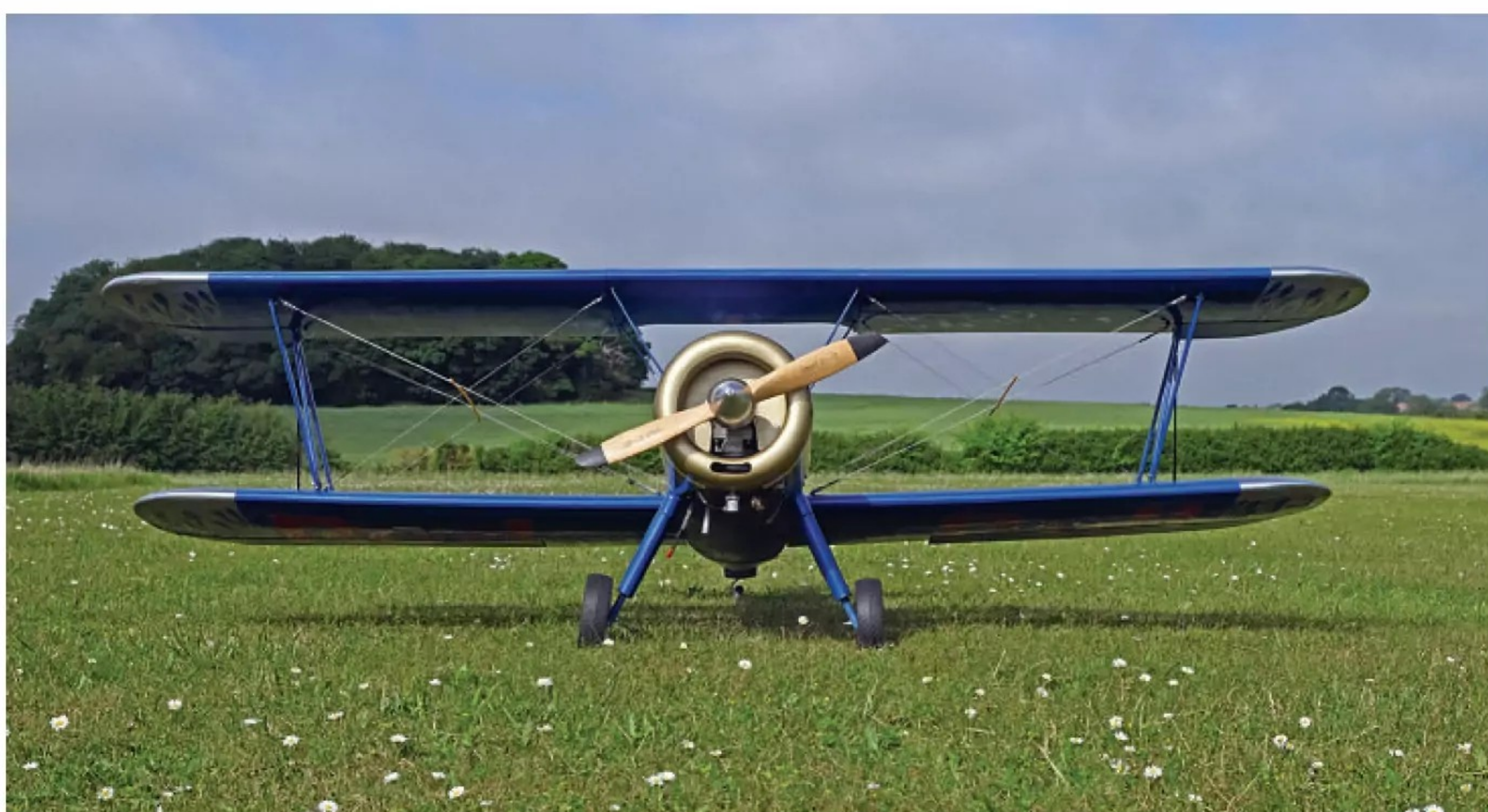
Front view showing the rigging which makes a whistling sound when the aircraft is on the glide.
