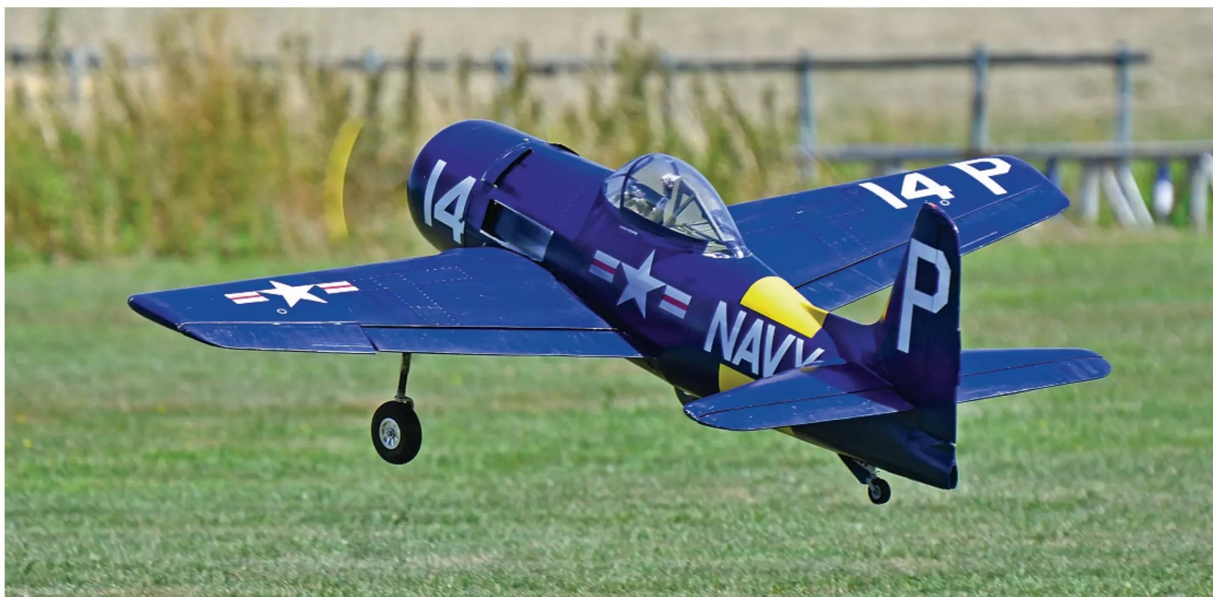
Henry Fray's 88" span, 1/5th scale Grumman F8F Bearcat was built from the Zirol plan and is powered by a 80 cc Zenoah twin. Henry says it is very docile to fly but lets his friend Keith Barnes fly the model at shows.
