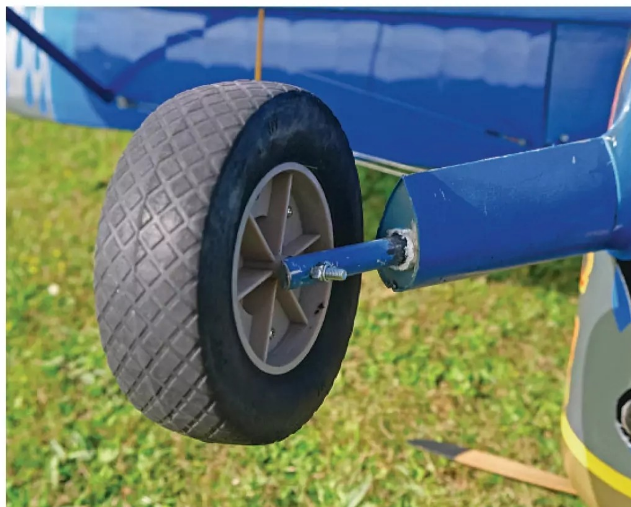
Faired and sprung main undercarriage detail.
