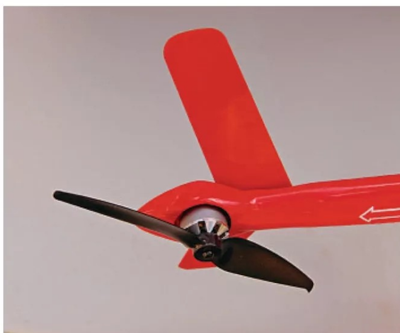
A one-piece, two-blade prop serves as the tail rotor.
