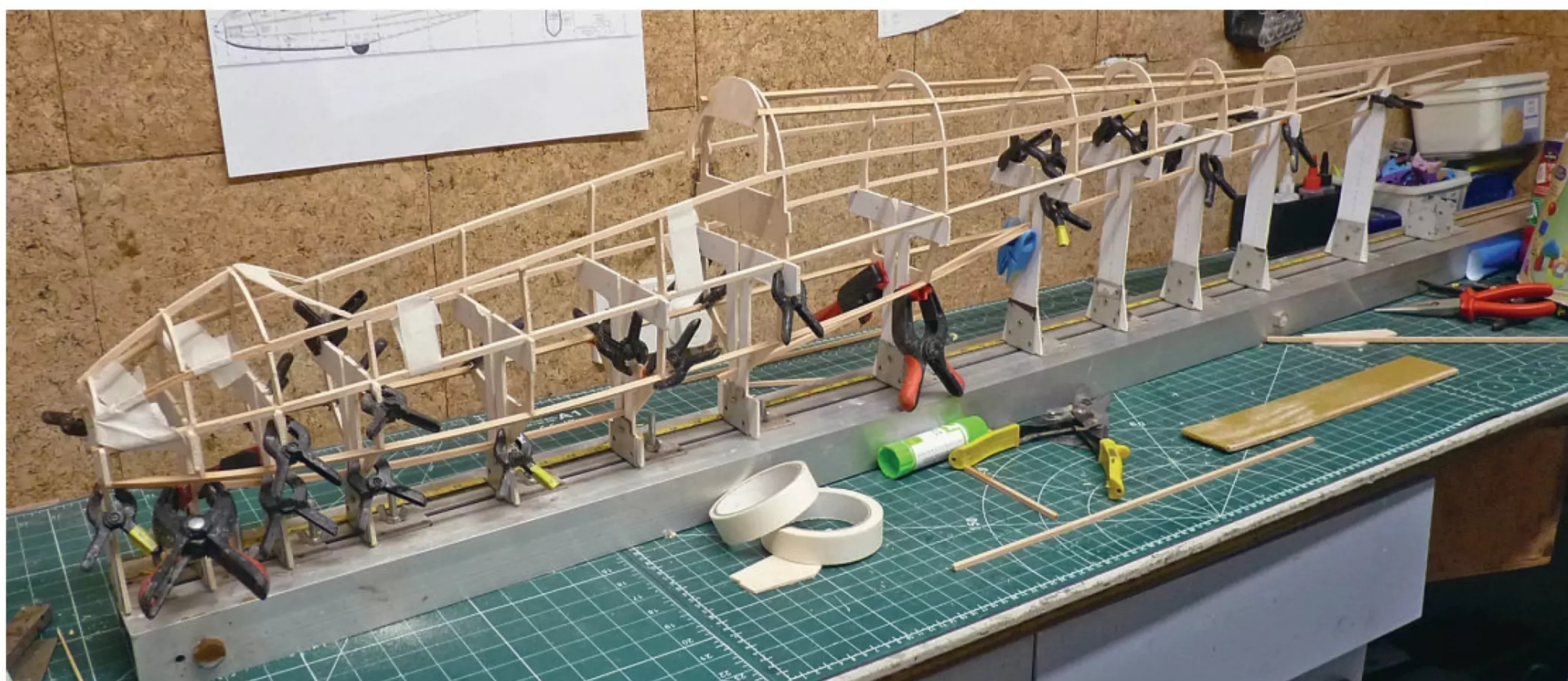
Initial fuselage construction on the 'Bridson' jig. See Scale Soaring UK website for jig details.
