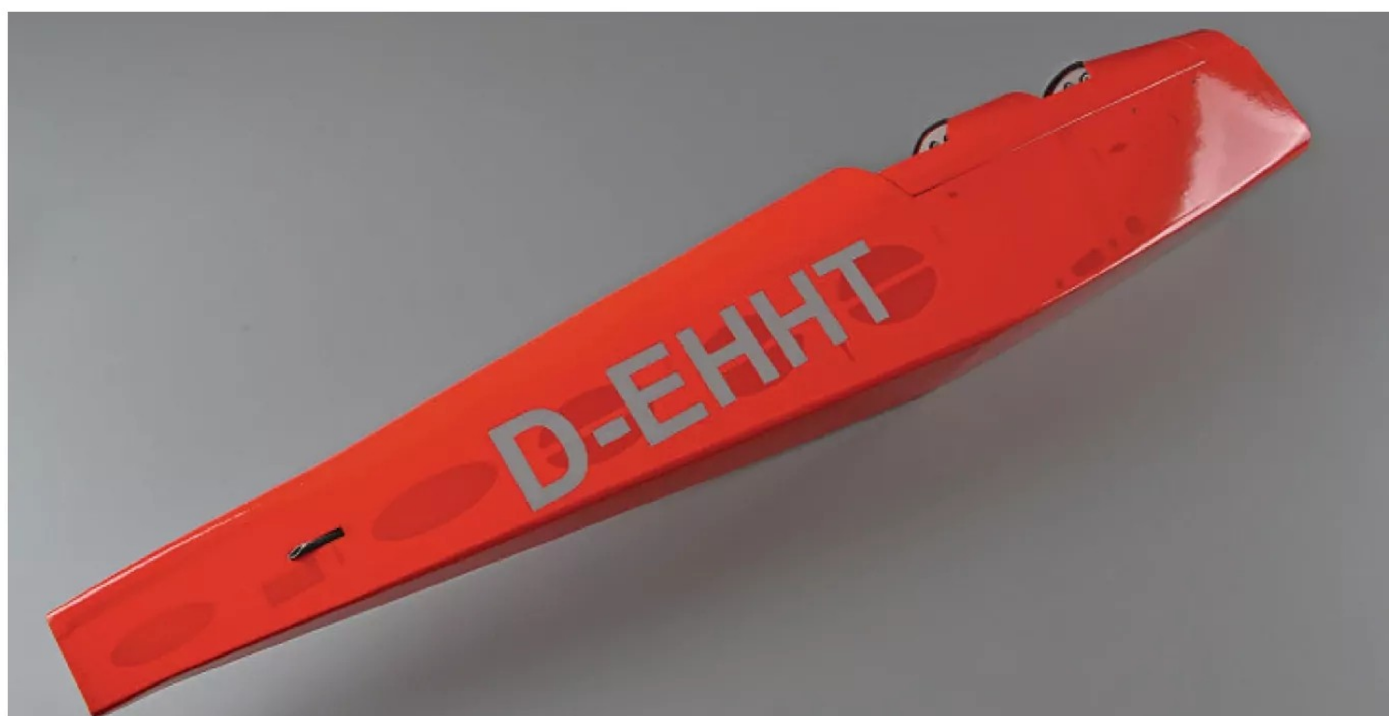
The fuselage's red covering is evenly attached and has the registration letters embedded in the film.
