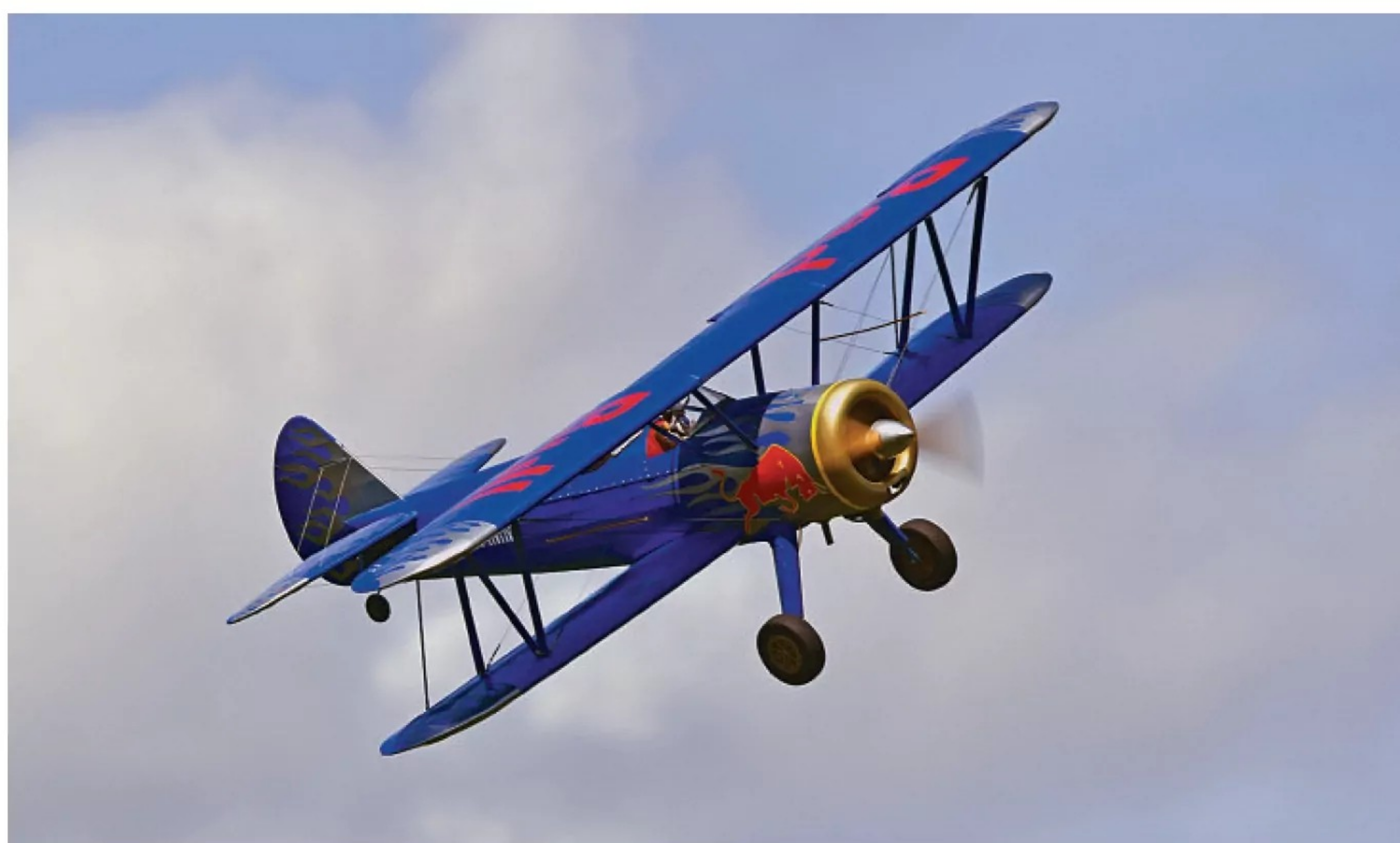
The original engine was an OS 40 cc four stroke, balanced using three pounds of lead!
