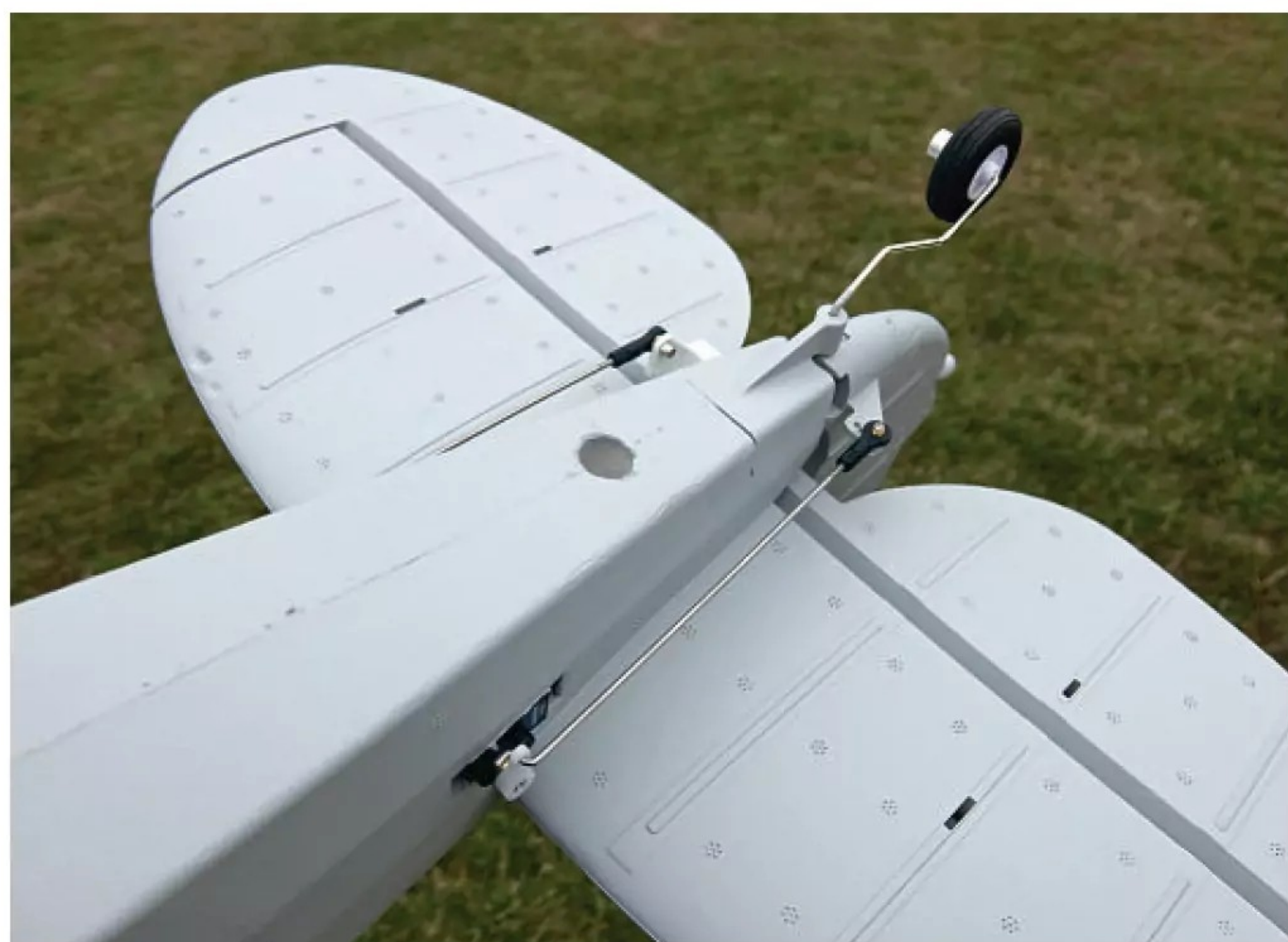
Tailplane is attached with a small screw dropped into the deep hole just forward of the tailwheel. Elevator and rudder pushrods are close to the correct length.
