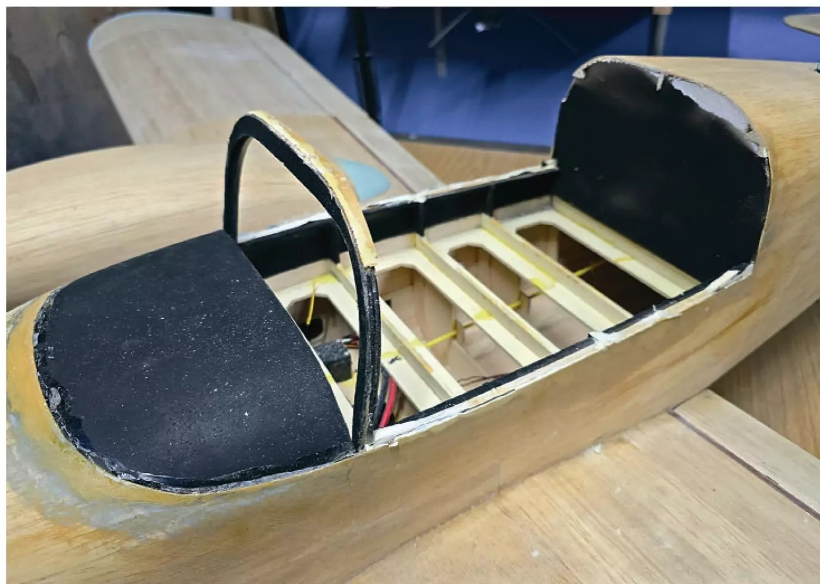
First, I hacked the roof and front canopy away. A painful thing to do.
