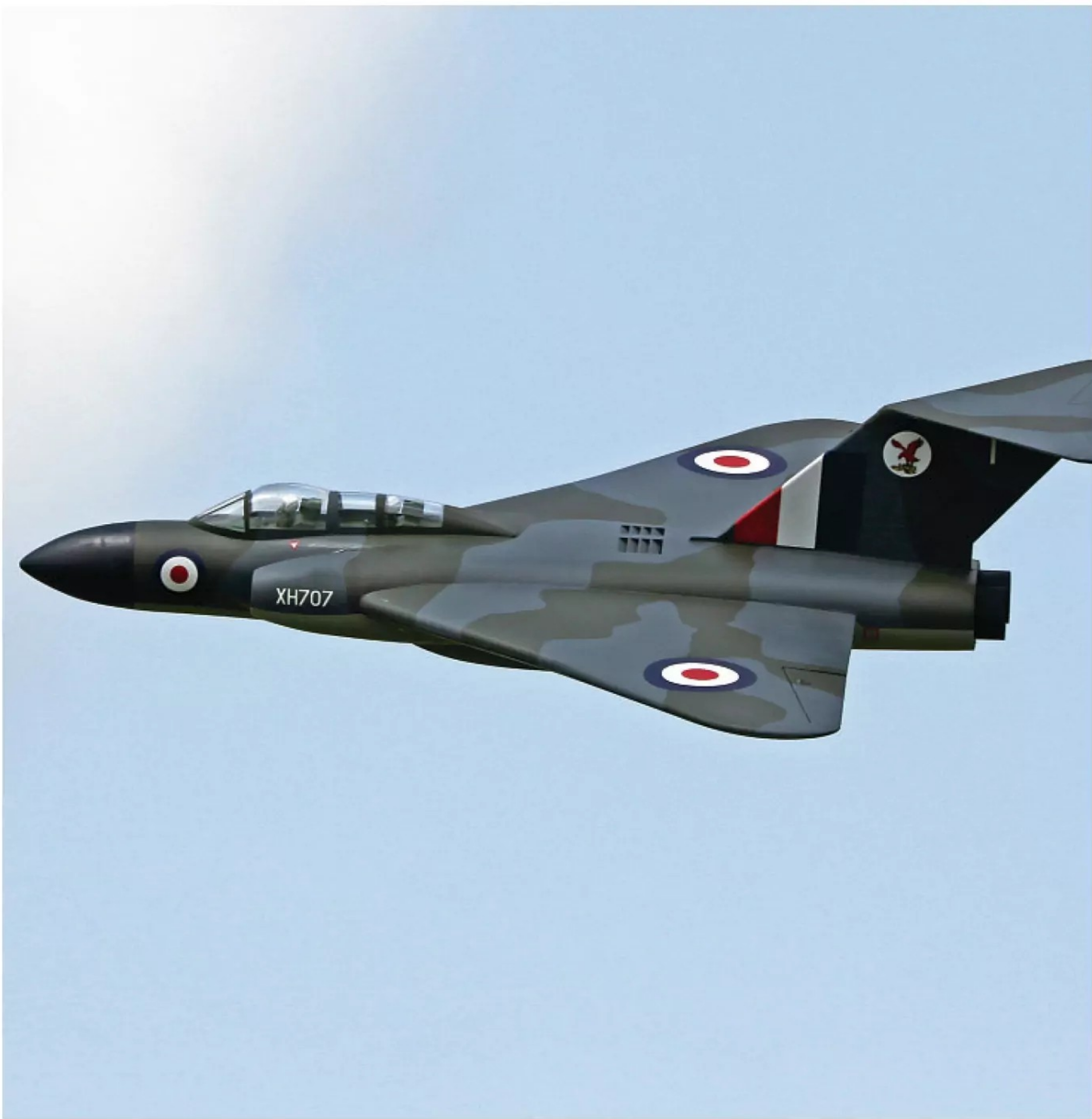
Powerfun's 4S 11 bladed EDF gives a lot of punch and flight times are surprisingly good. Expect a good five minutes depending on throttle use.
