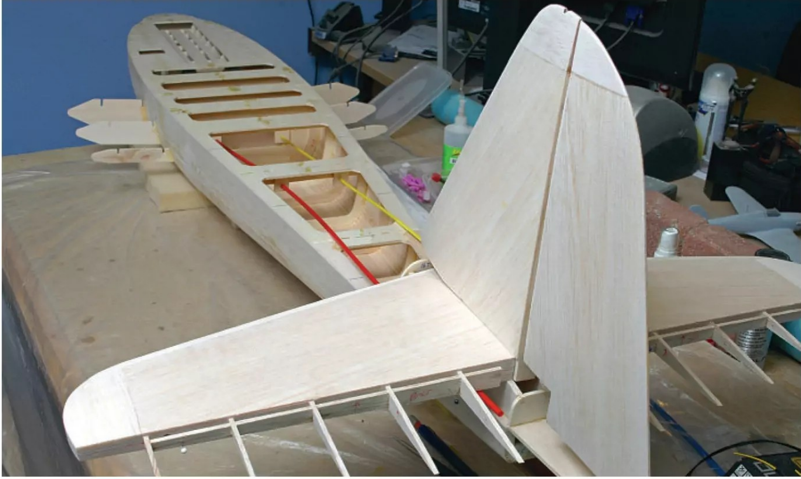
The lower fuselage was assembled first and sheeted up to the datum.
