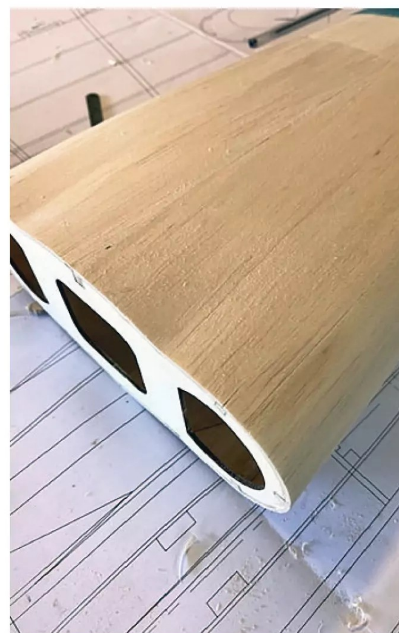
Use a razor plane and sanding block to shape the fuselage to a smooth profile.
