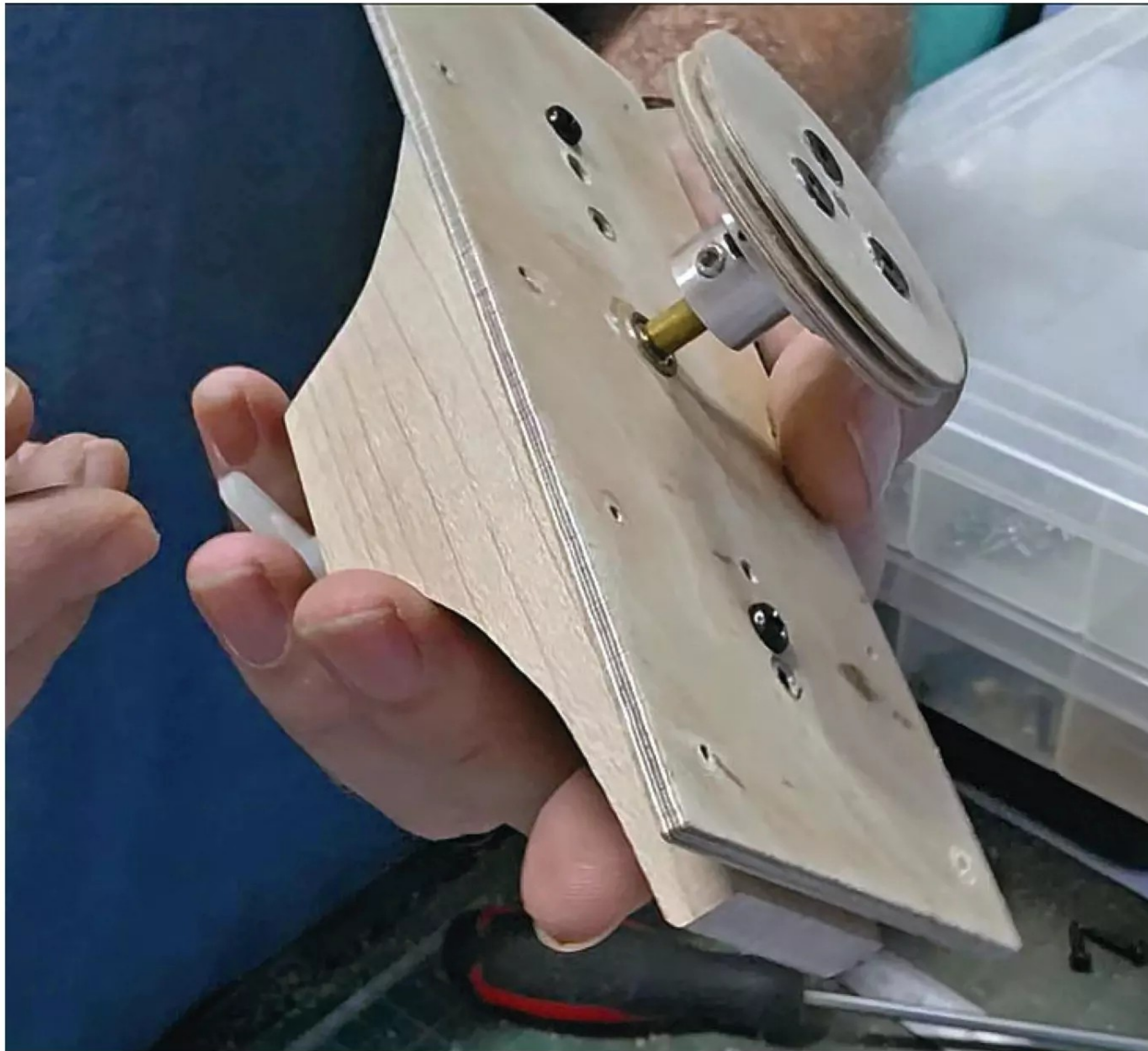
A maple block with a twin bearing 6 mm ground steel shaft running top to bottom, allowing the anulus bellcrank to transfer the torque to a nylon arm at the bottom.
