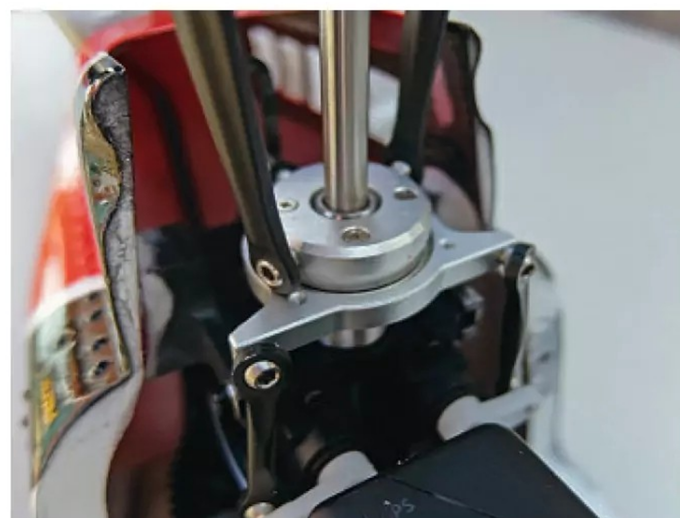
Three 4 kg metal geared high speed servos are used to control the swashplate.
