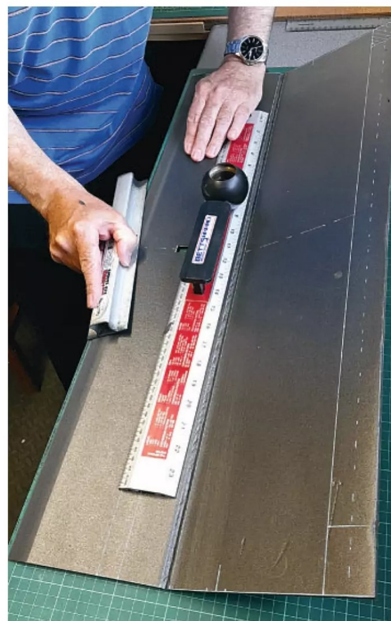
Sand or cut the bottom skin, inside the trailing edge, to a 20 mm wide taper. This blends the two skins together without a step. Clean dust off the parts with a damp cloth before you start to apply glue.
