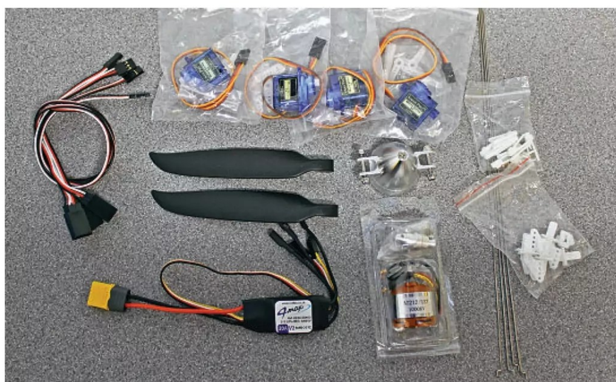
Electrics supplied by 4-Max include a 2212 1000 kV motor, a 20A ESC with brake, a 10 x 6 folding prop and four SG90 servos.
