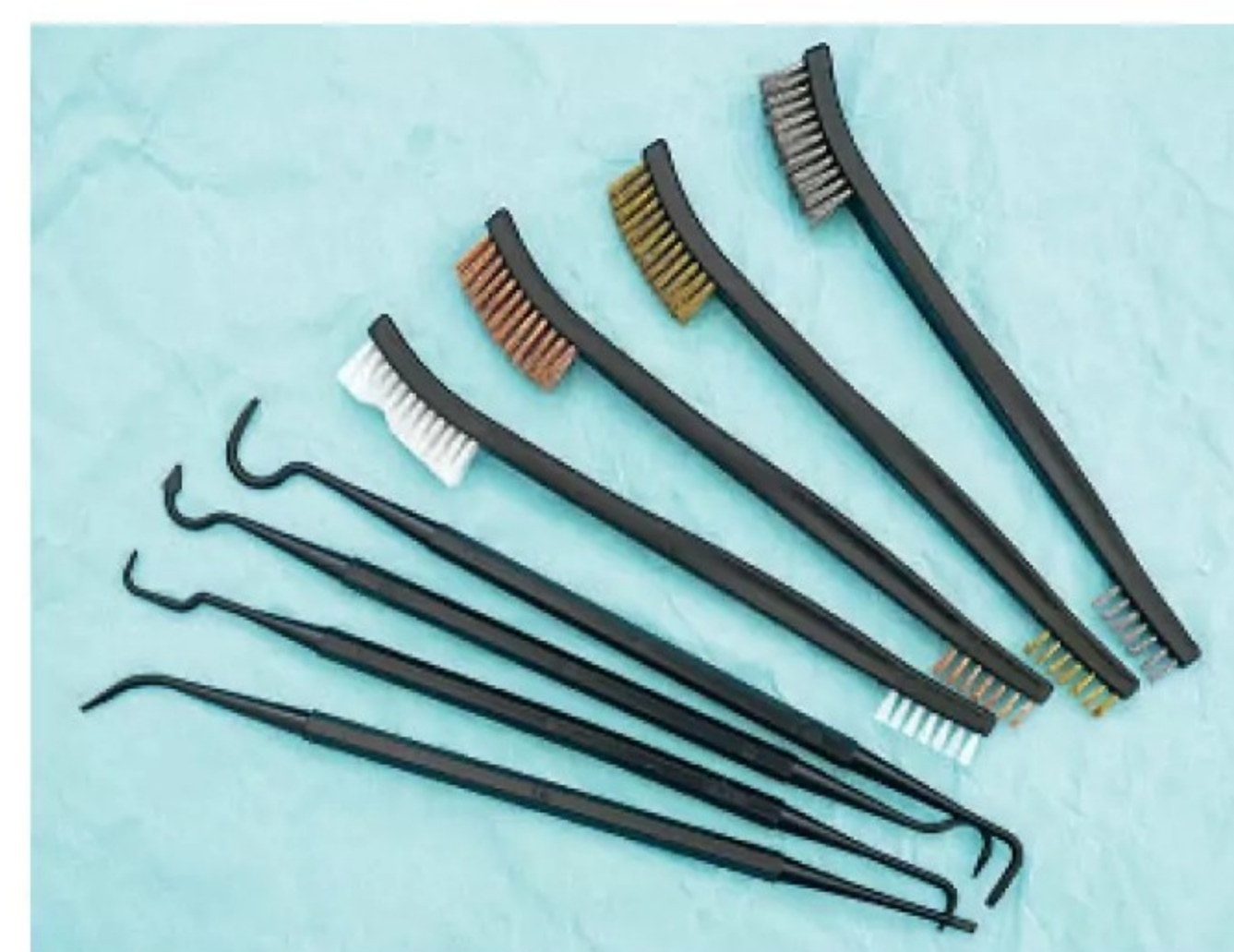
Each brush material has a specific task, whilst the plastic picks won't damage aluminium parts.
