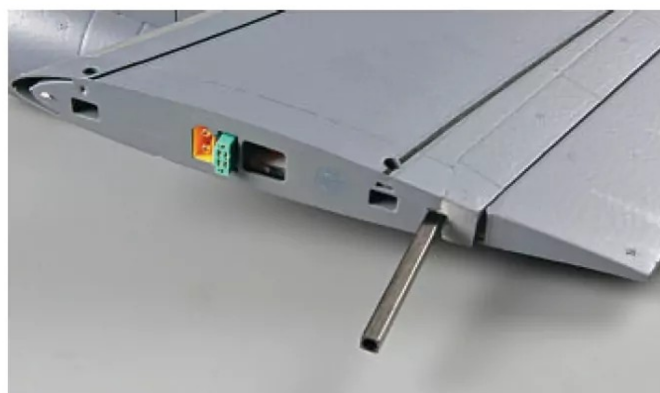
Close ups of a wing root and fuselage wing mount showing the XT60 power connectors and the green six-pin servo connectors. The connector block in each fuselage side needs pulling out slightly and pushing firmly in place at the wing root before pushing the wing into position.
