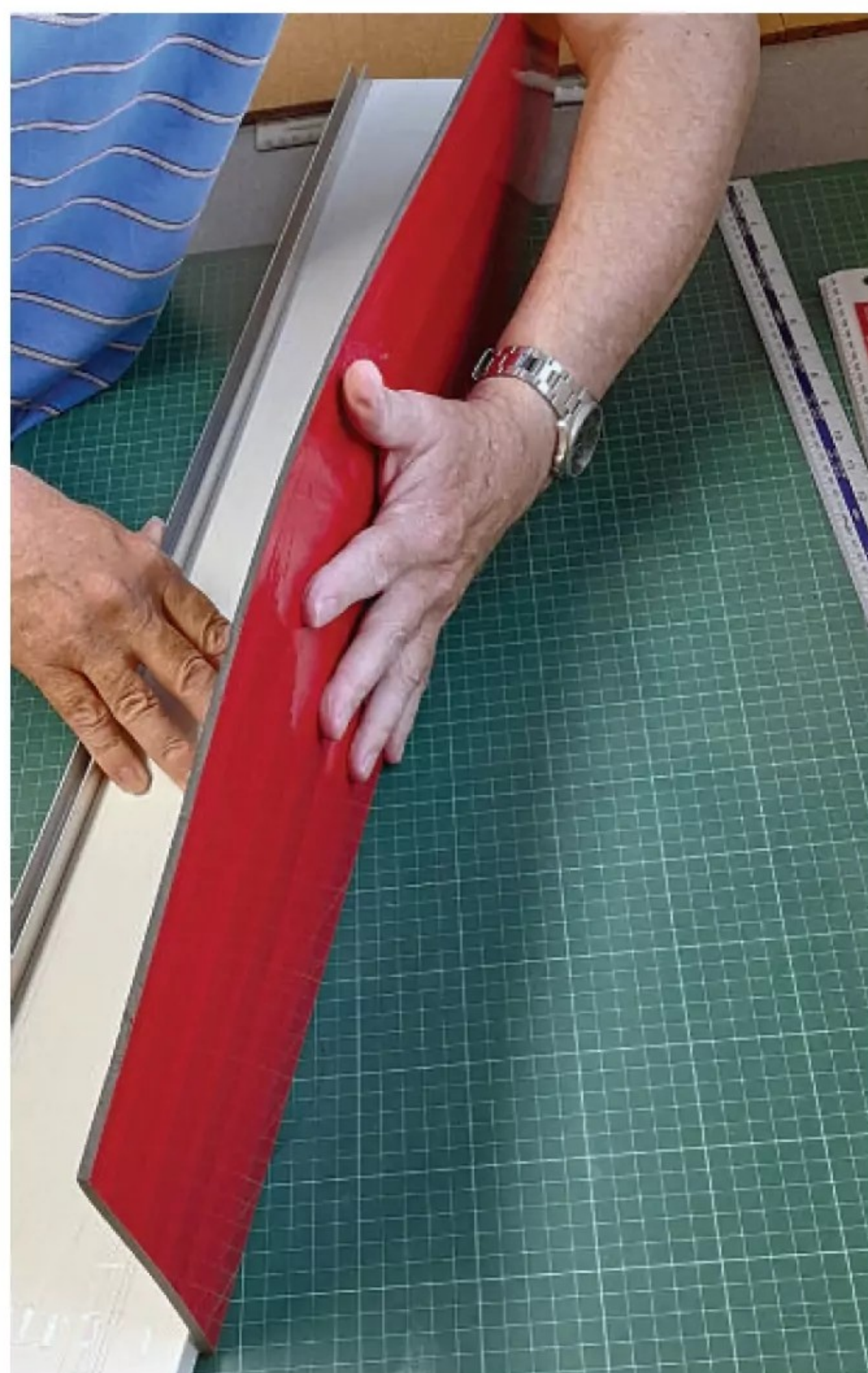
Hold a flat edge along the fold line, then carefully bend the sheet up to 90 degrees.
