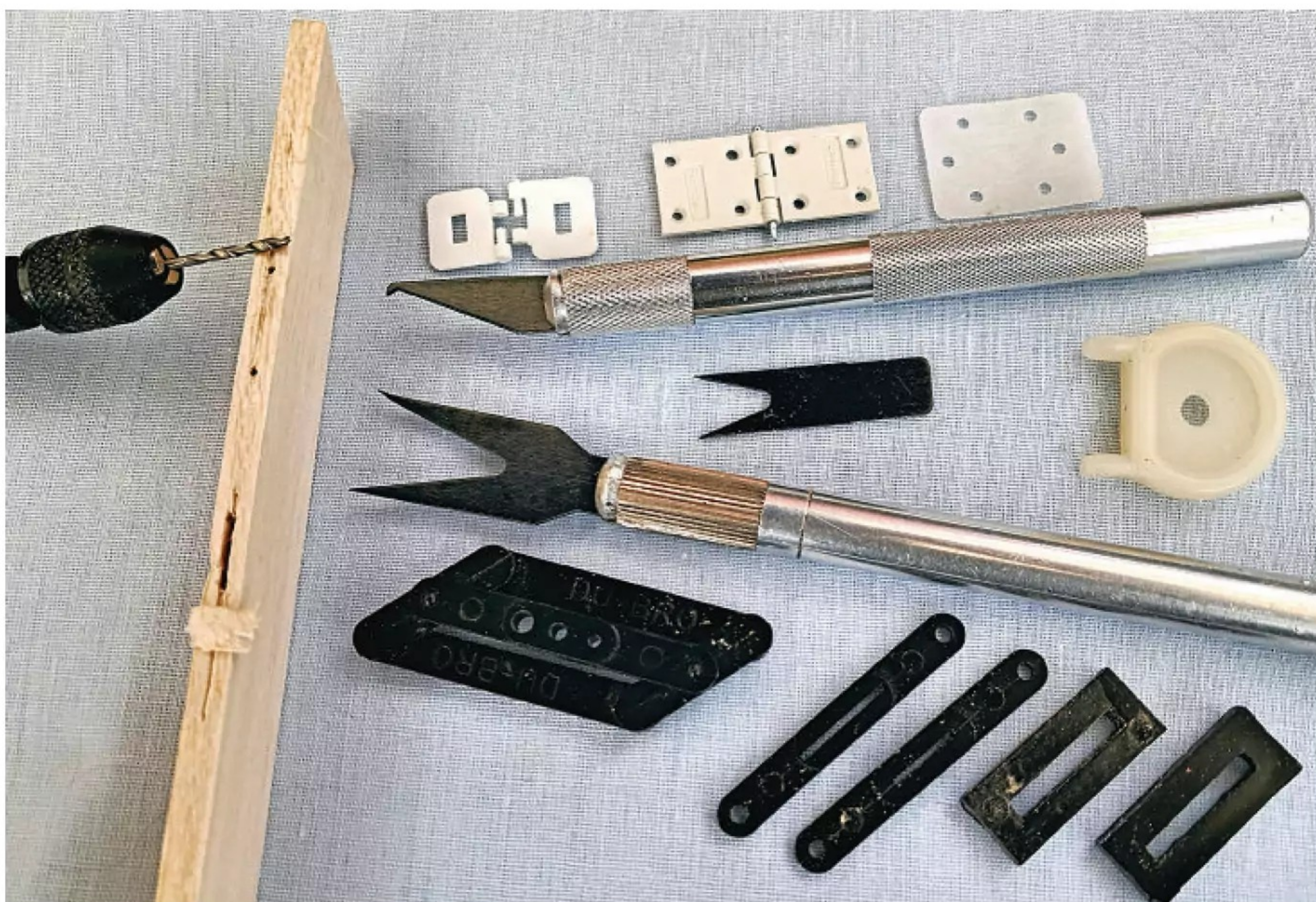
My Du-Bro hinge slotting kit can prepare two widths of slot in various thicknesses of wing trailing edge and aileron. Fixing strength of the hinge depends on a well-prepared recess and thorough gluing.
