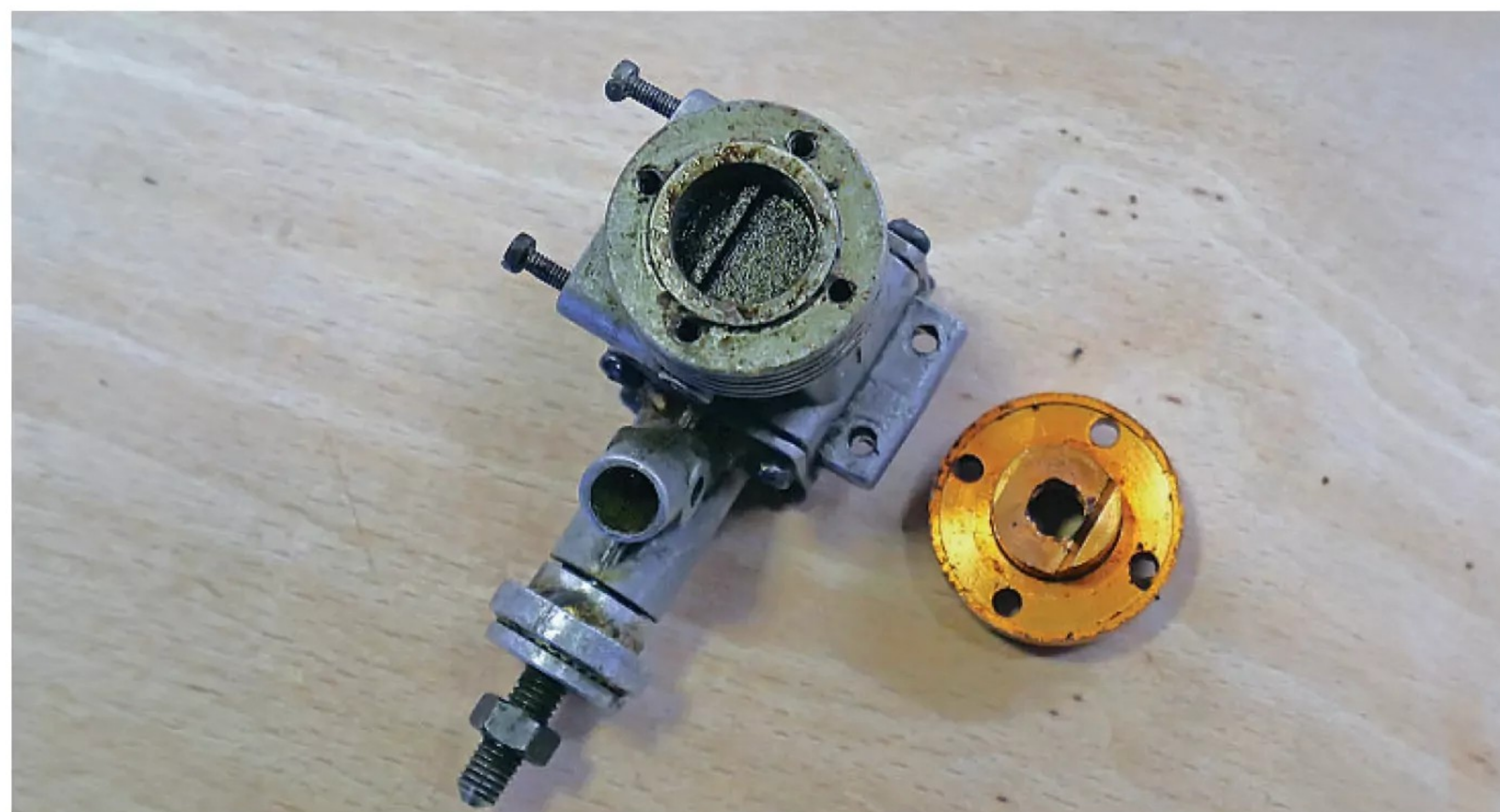
Oh, dear! The piston baffle is on the wrong side. No wonder the piston has a large carbon deposit on it.
