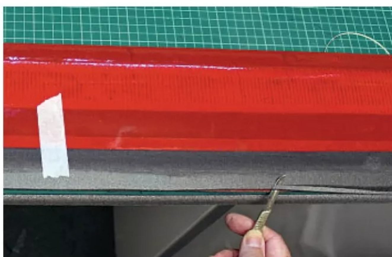
Lay the aileron flat on the top surface and cut or sand the hinge angle.
