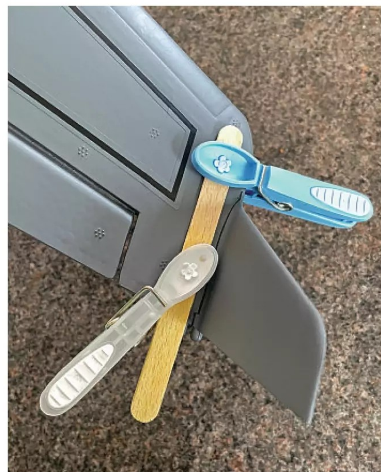
Gluing a winglet in place using a lolly stick to spread the pressure applied by the clothes pegs.
