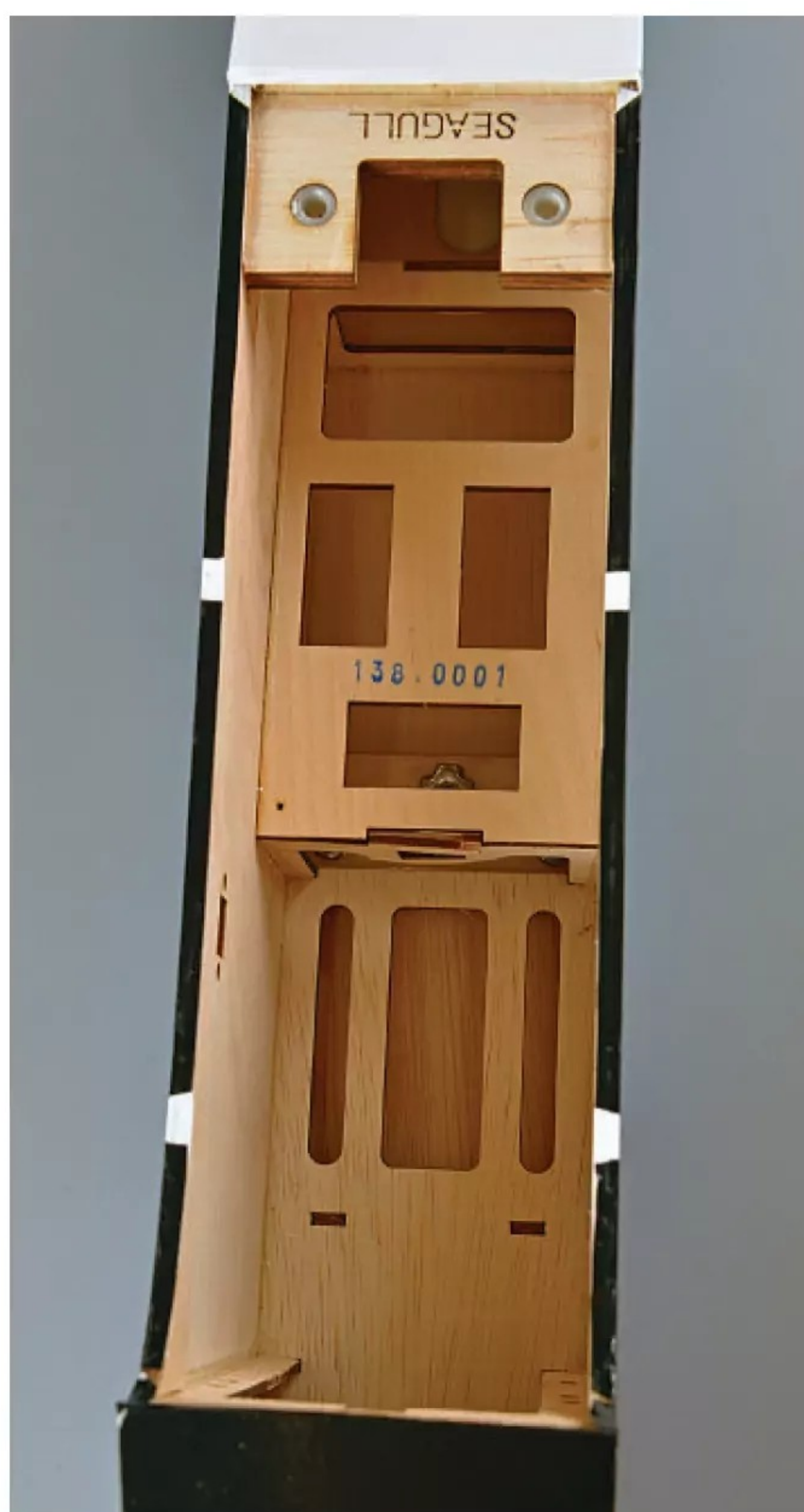
Servo tray has plenty of room for two standard rudder and elevator servos side by side, with the throttle servo mounted transversely in front.
