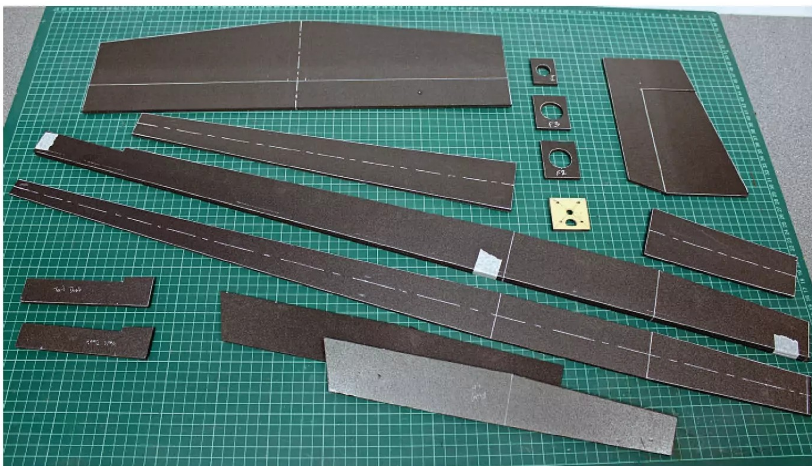
Start the fuselage and tail by cutting a kit of parts from Vitrex premium foam underlay sheet.
