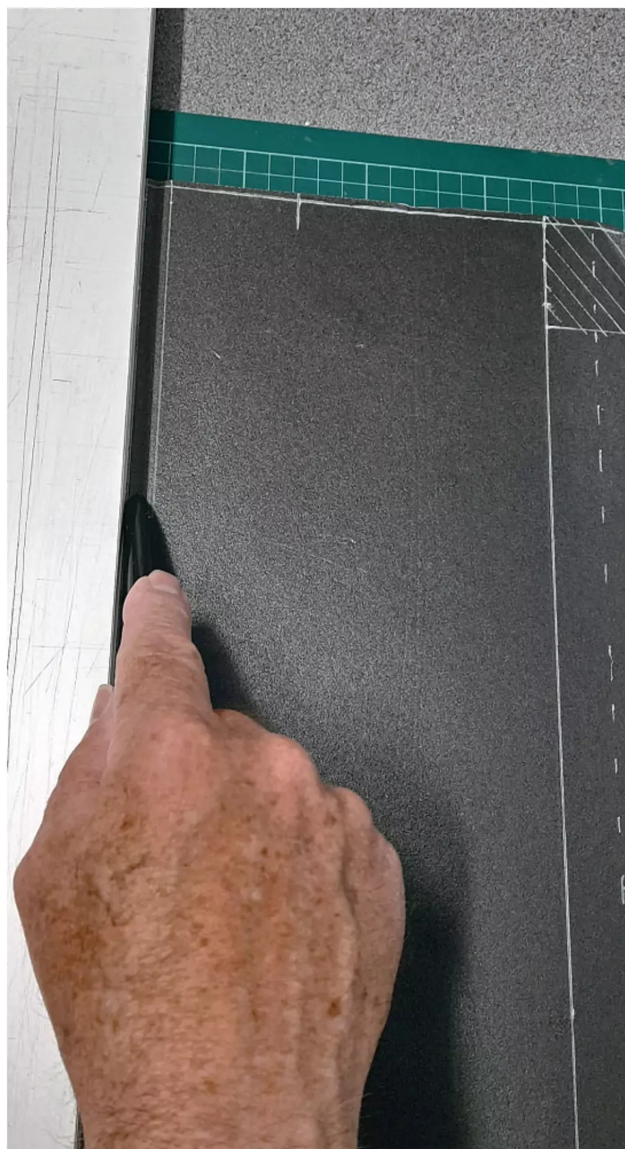
Scoring a fold line to crush the foam. Try not to split the foam surface.
