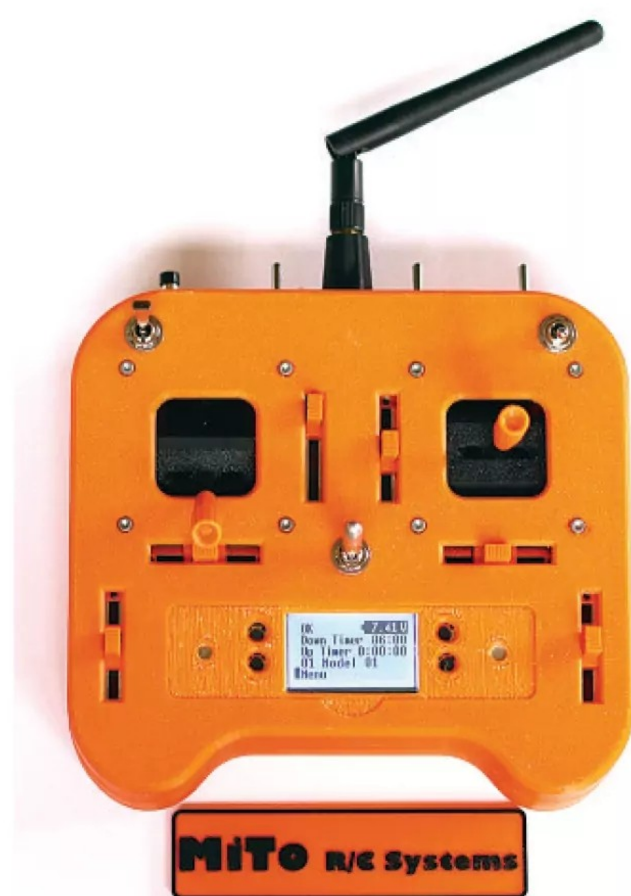
Tobe Kallner's latest 3D masterpiece. Totally home designed, including stick units, servos, PCBs etc and built in his shed.
