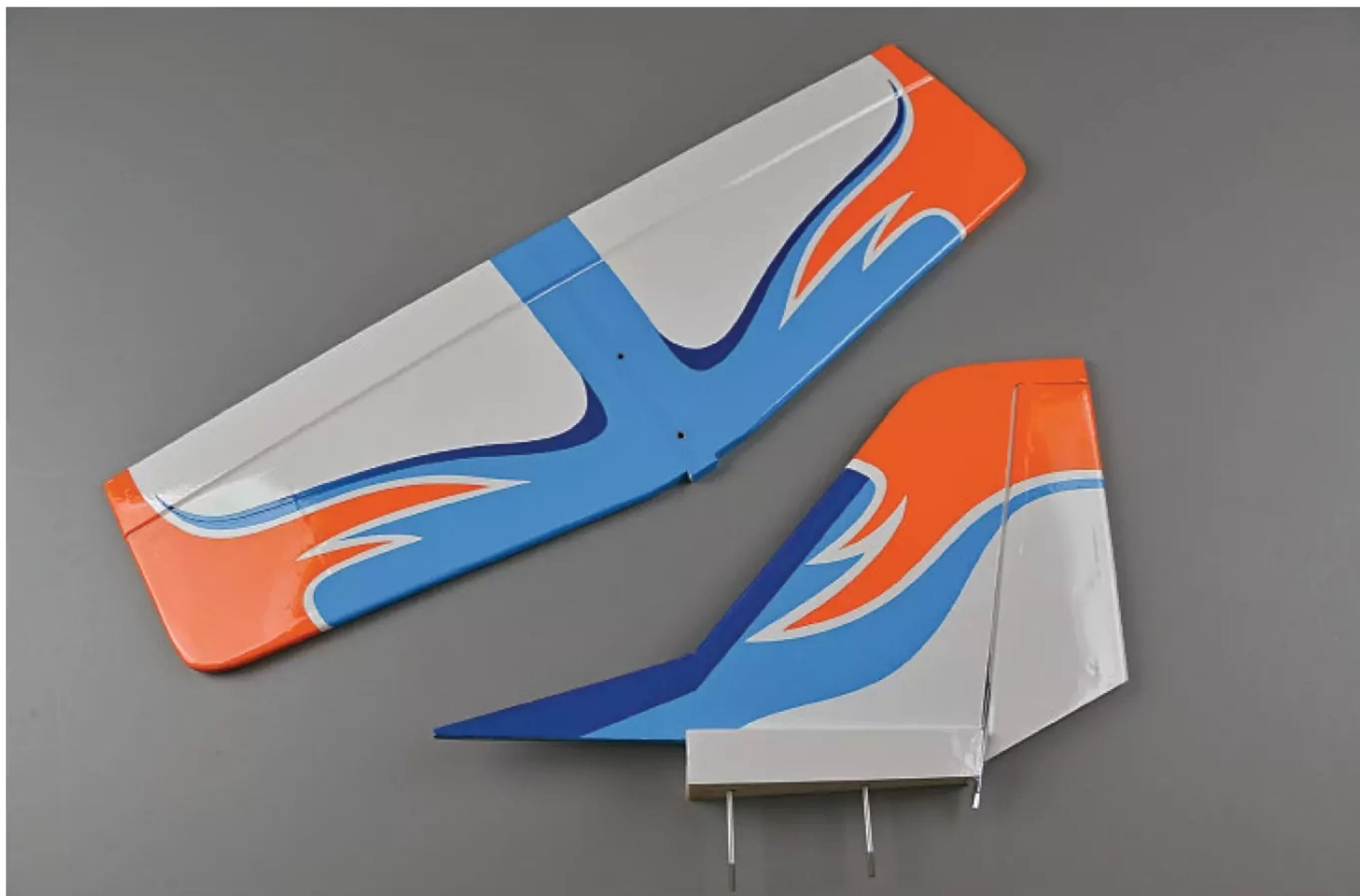
The tailplane is sandwiched between the base of the fin and the rear fuselage, pinned in place by two long studs.
