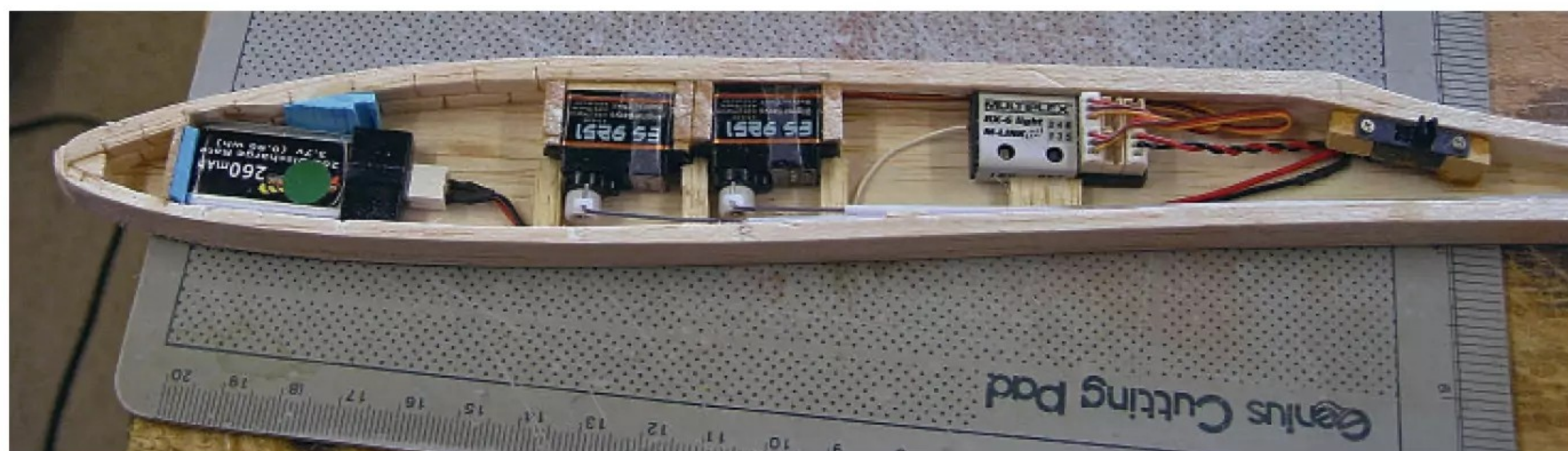
Front fuselage of the original Comet of 22" span. Single LiPo cell, Emax 9251 servos, Multiplex five channel receiver and a small switch. Available internal depth is only about 7 mm.
