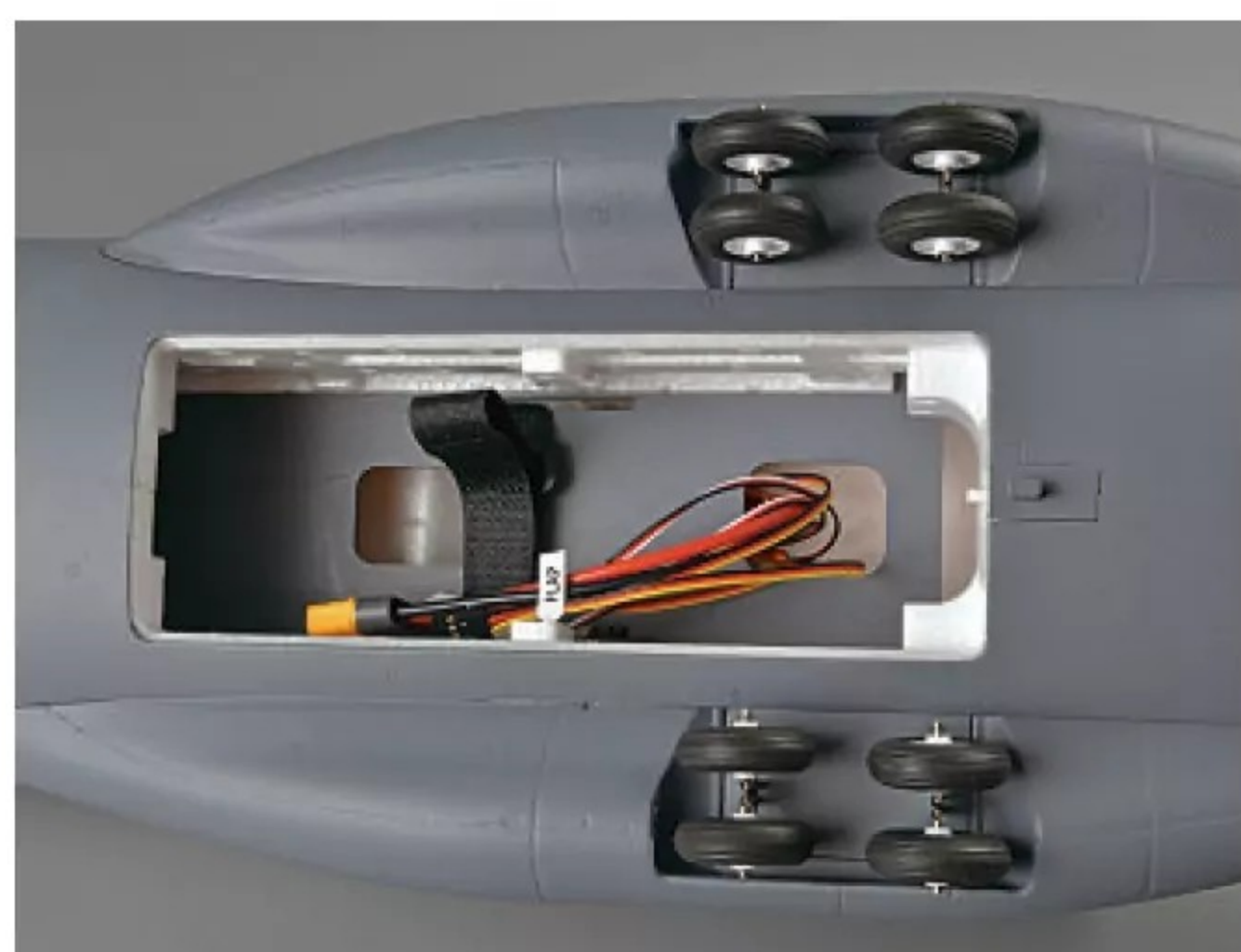
There's oodles of space in the battery bay for a large 4S LiPo, with a receiver mounted at the rear. Servo leads are all neatly labelled according to their functions.
