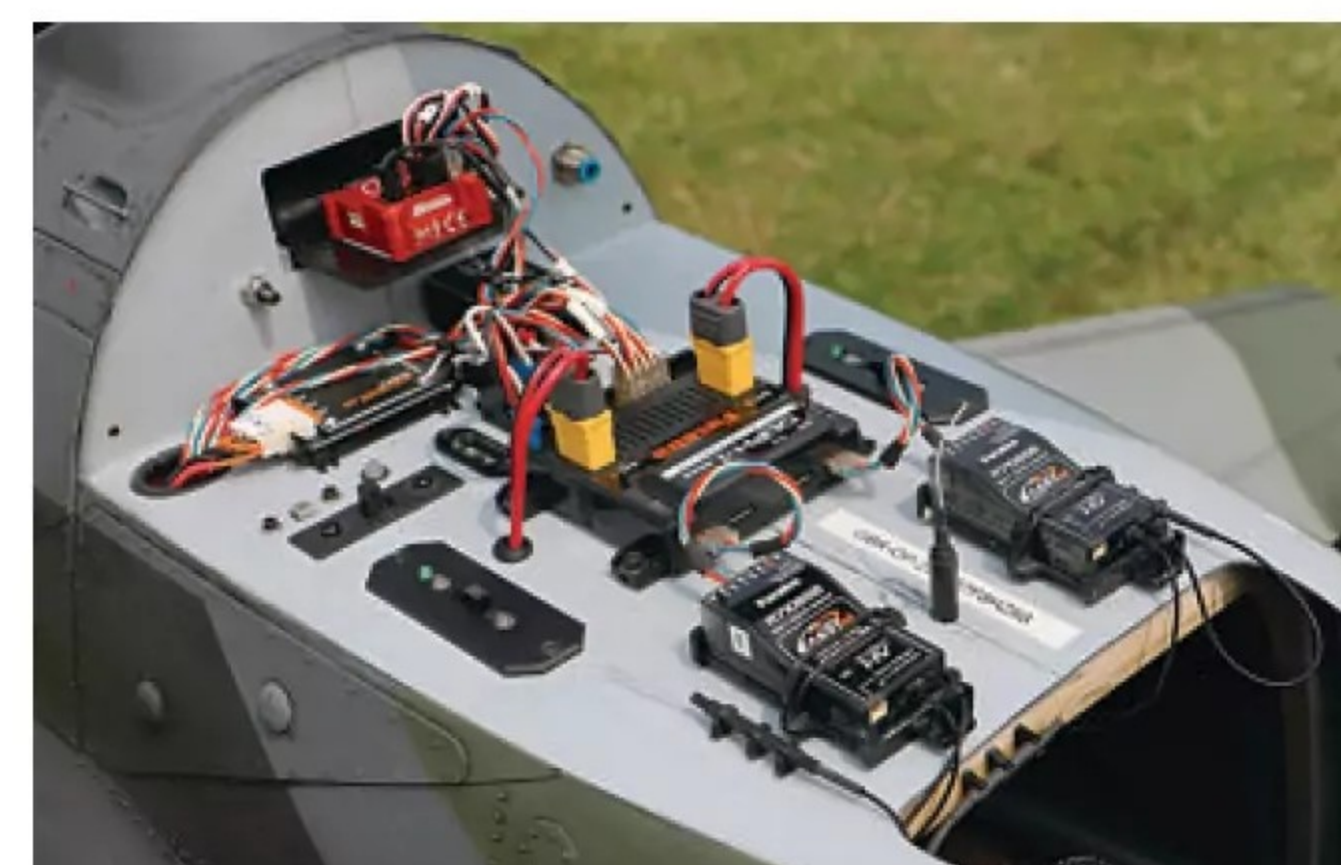
At the heart of Lee's Mil-24 is a Futaba DLPH-1 Intelligent Power Hub and twin R7108SB receivers. Oh, and a Pahl Taurus 12KW turbine.
