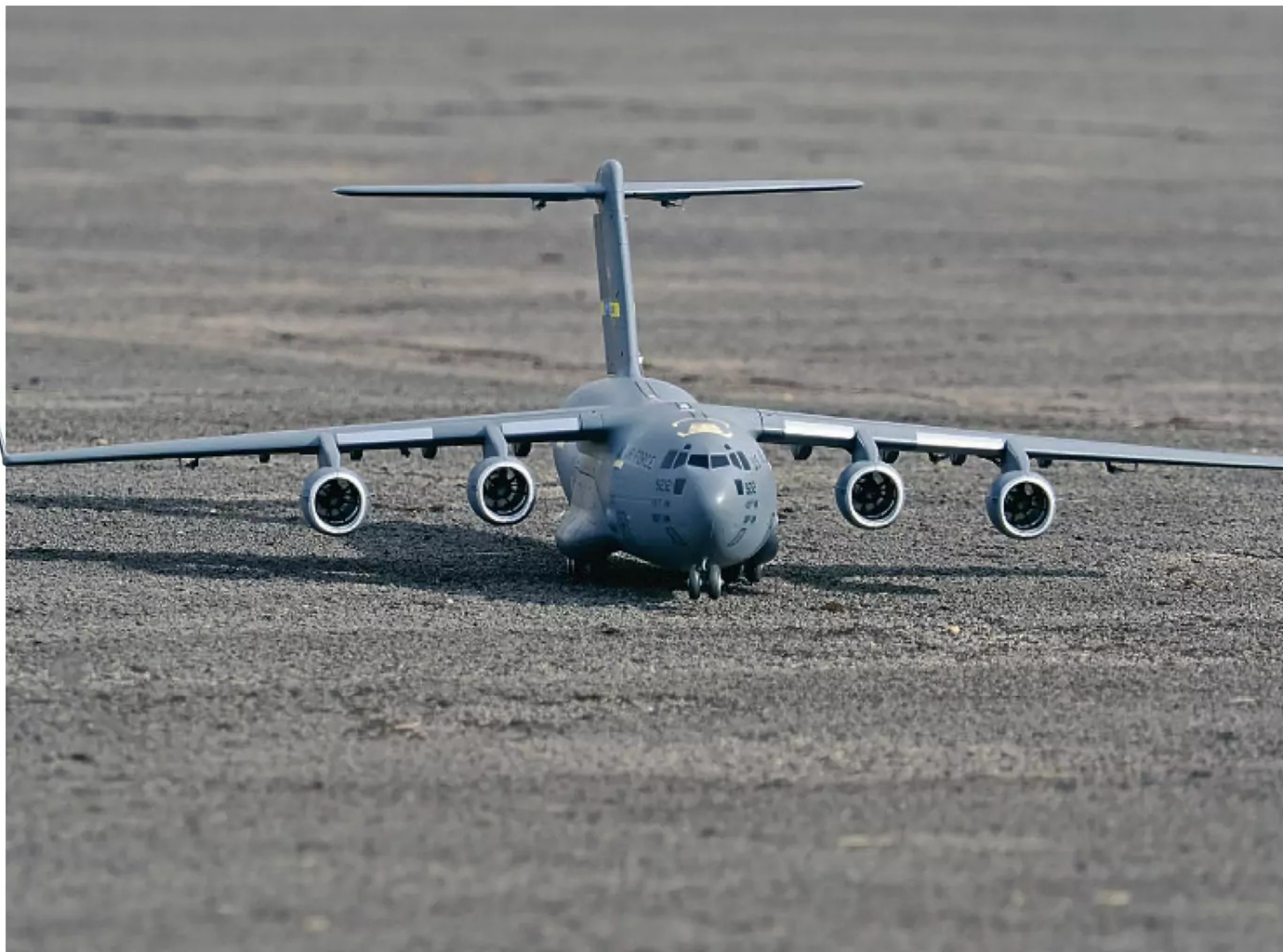
Globemaster shows off its distinctive anhedral on the main wings.
