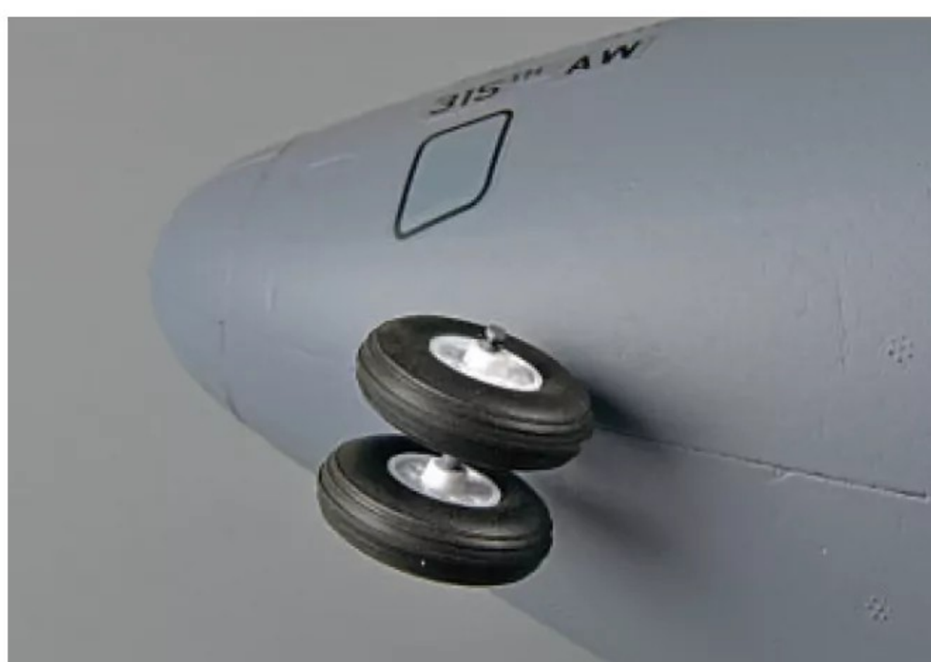
Twin nose wheels are linked to the rudder servo for steering.
