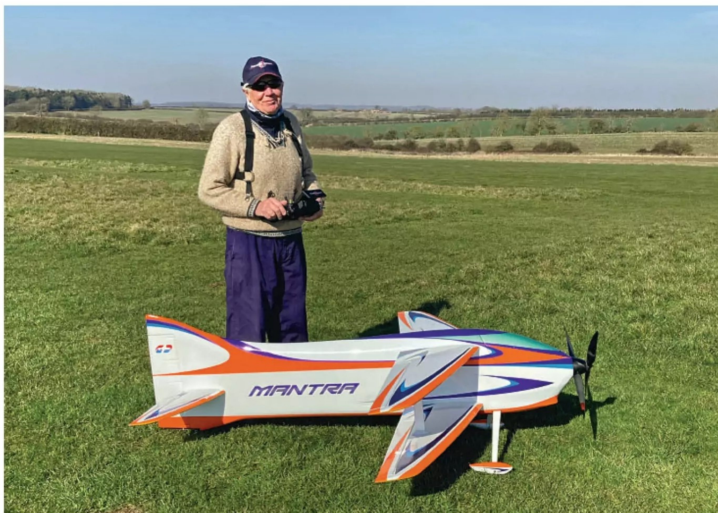
UKF3A Chiefjudge Alan Williams with his contra powered Mantra biplane. It is fitted out with a VLV contra and a VLV governor ESC, along with Futaba servos all round.
