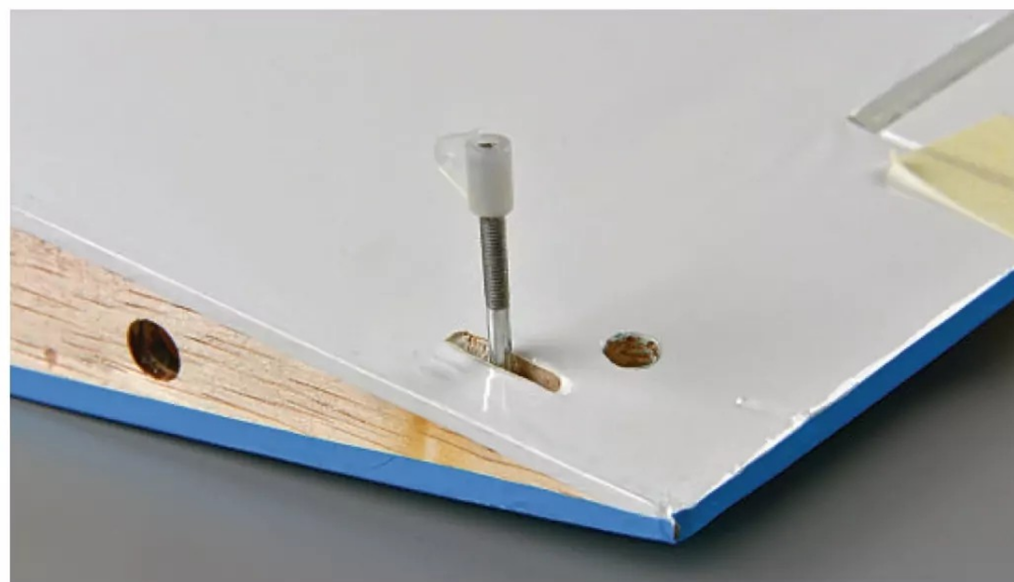
Remember these? Ailerons are moved via torque rods controlled by a centrally mounted servo.
