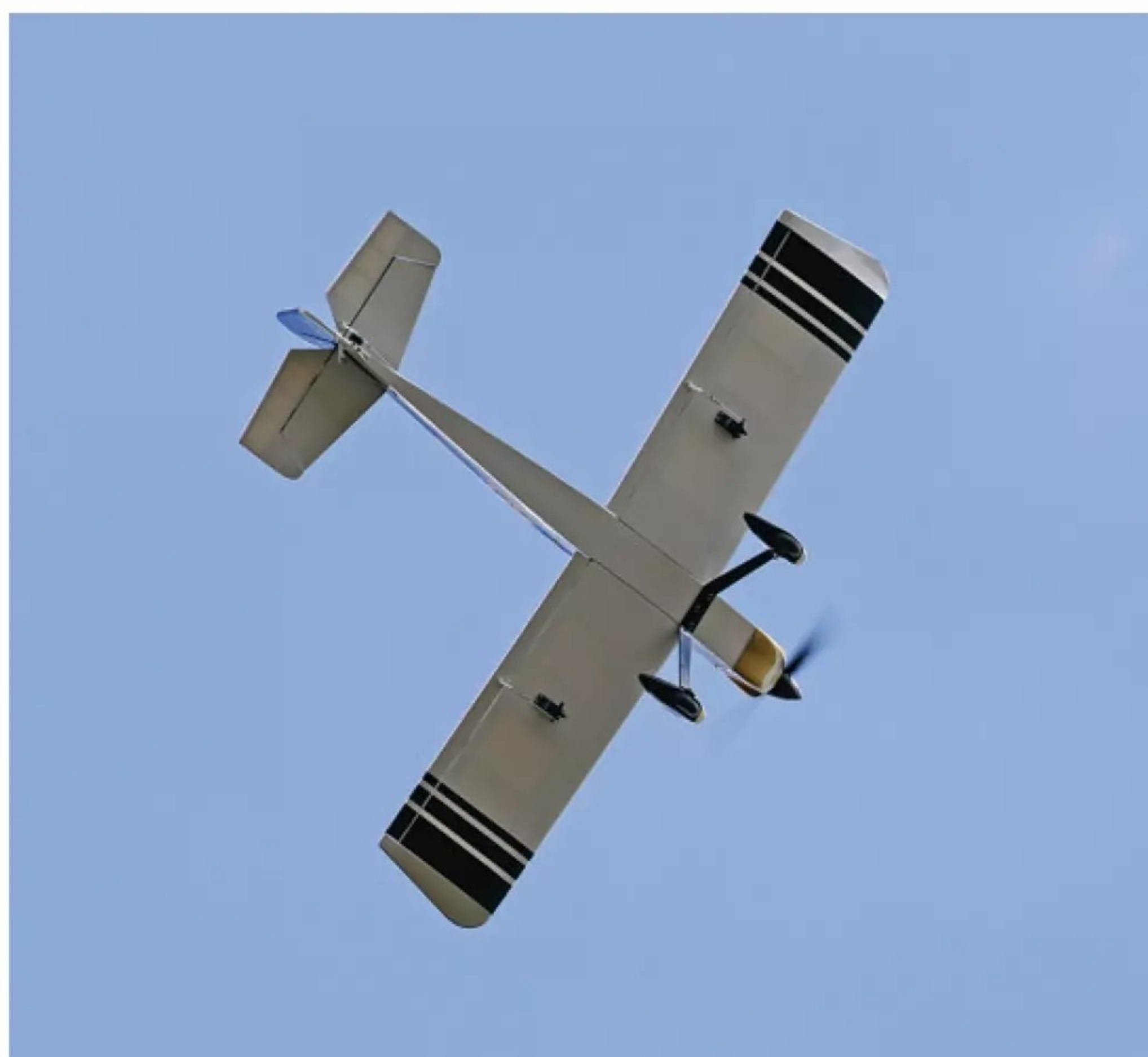
Simple underwing stripes aid orientation.
