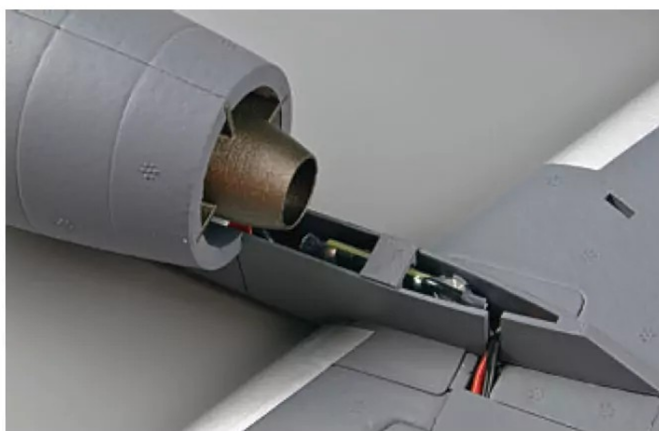
A 20-amp ESC snuggles neatly inside each of the four EDF pylons.
