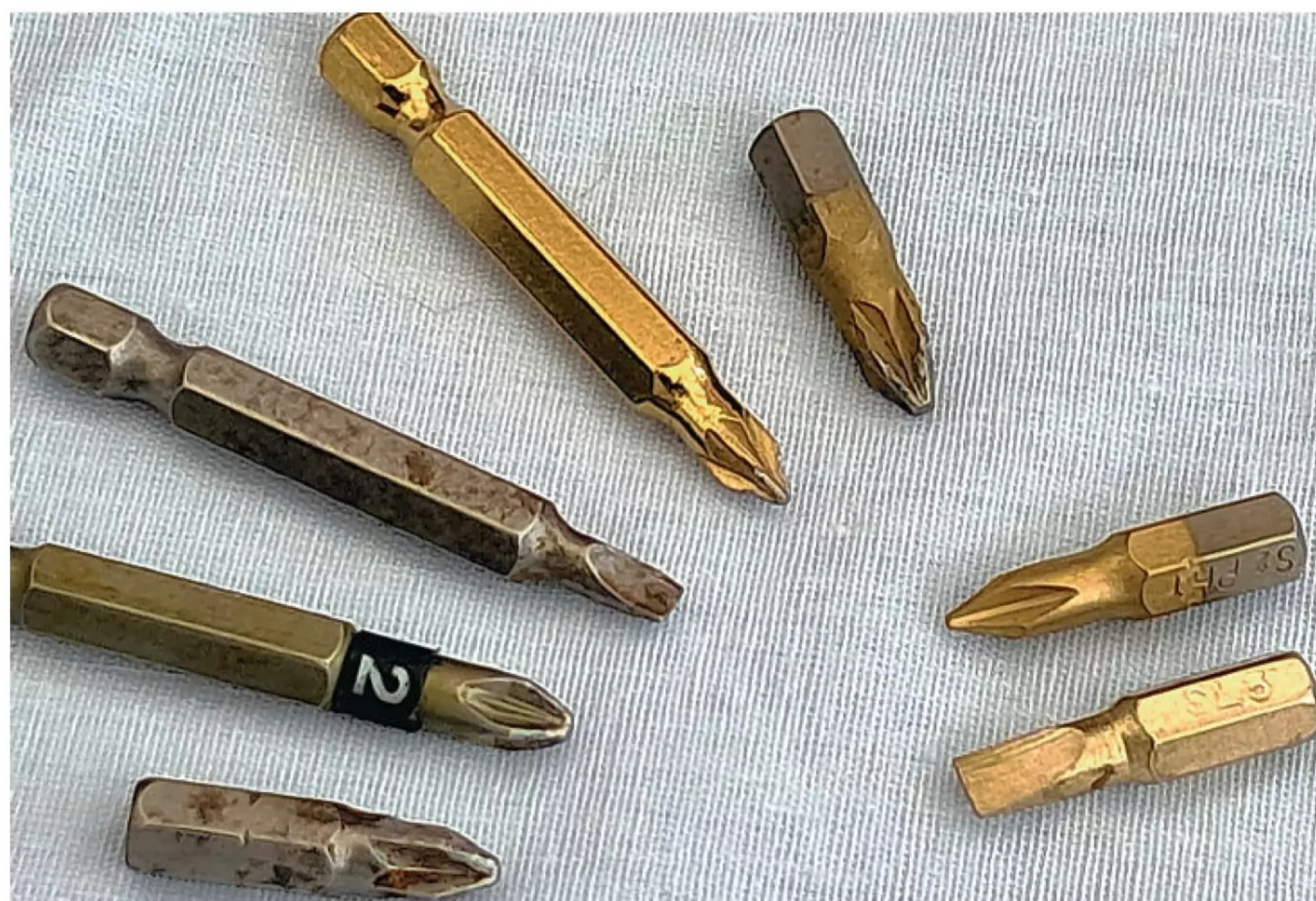
All five tips (left) are worn beyond reasonable use. Don't keep struggling and making do. New tips are cheap and won't slip if used correctly.
