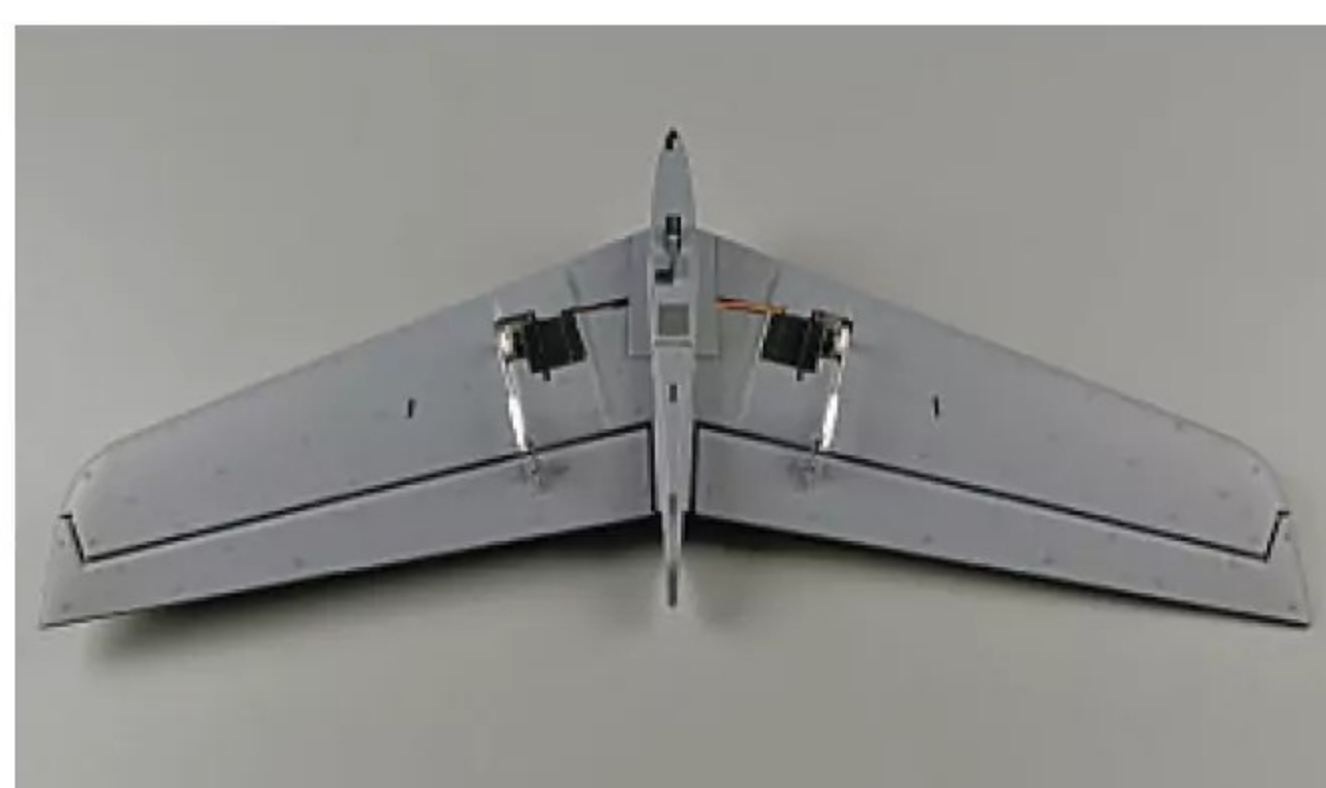
Elevators are controlled by a pair of 9 g servos.
