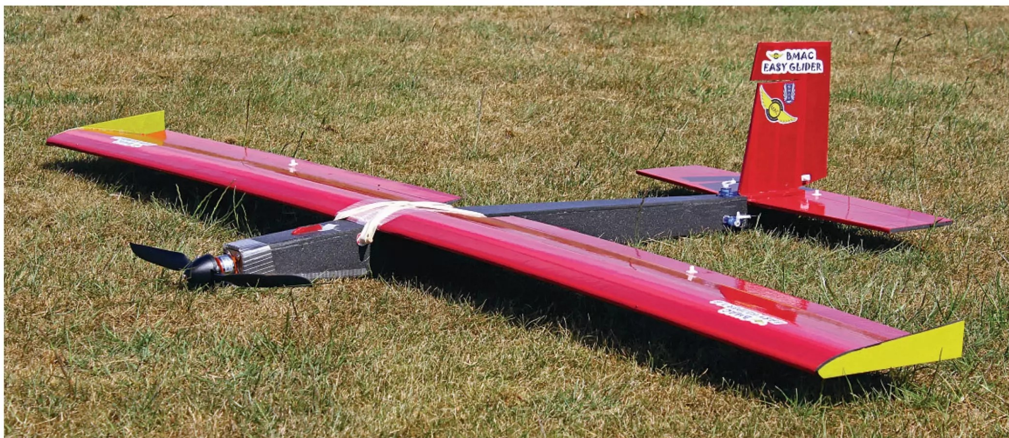
Easy Glider prototype had no dihedral and flew well, but on the ground there was noticeable anhedral. This corrected itself once airborne. Adding 25 mm under each wing tip will stop the wings drooping whilst on the ground.
