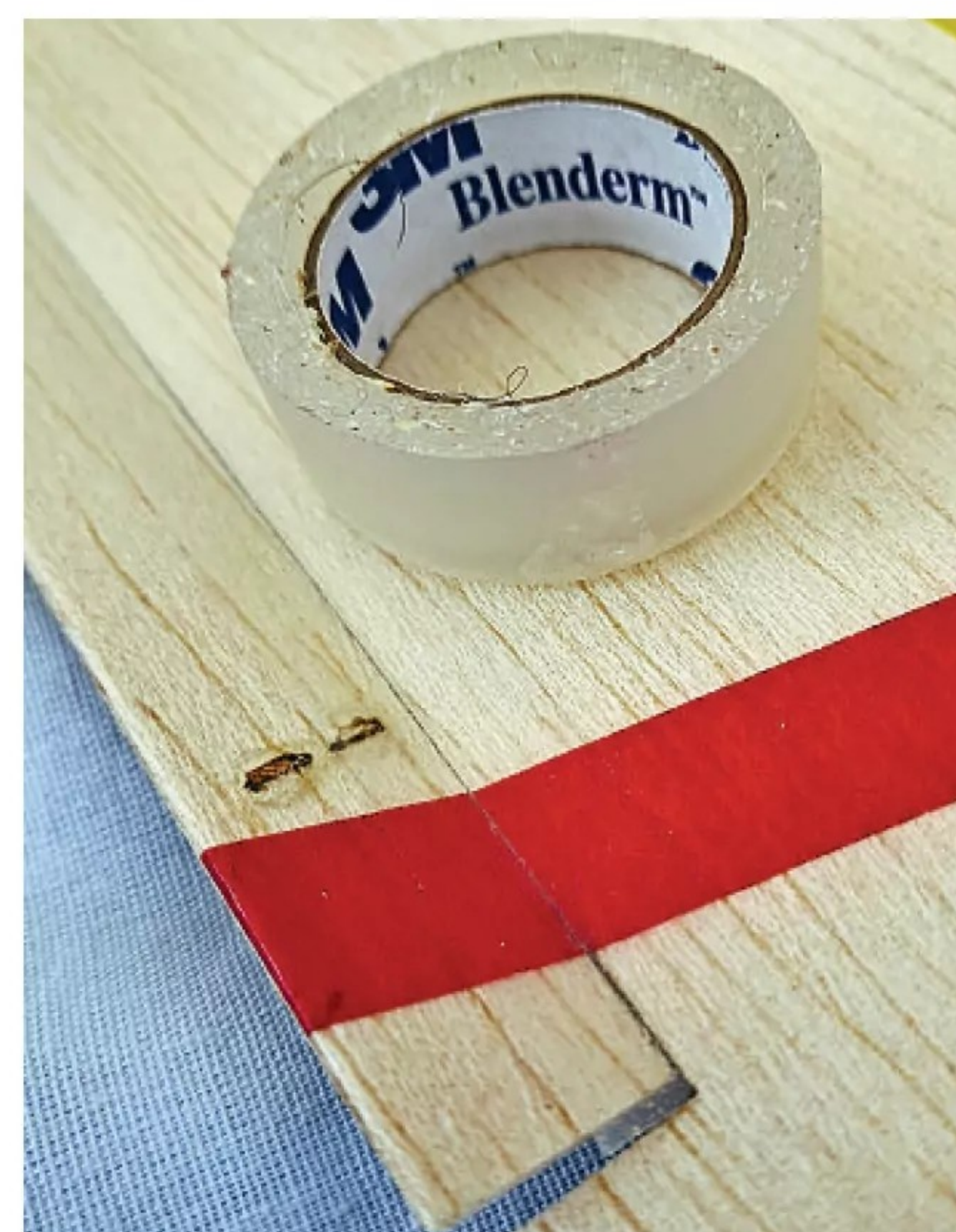
The simplest hinge material for thin wing trailing edges in small models is Blenderm tape. Almost invisible in use, can you see it? This is a 2 mm thick Jedelsky wing/aileron. See 'Top Hinging' overleaf.
