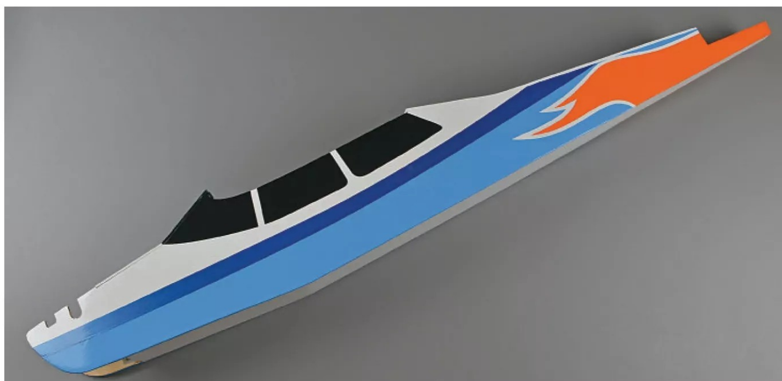
The fuselage is neatly covered in the same style. It's even more important to fuel proof the covering here, especially at the front and also any exposed wood inside the fuselage.
