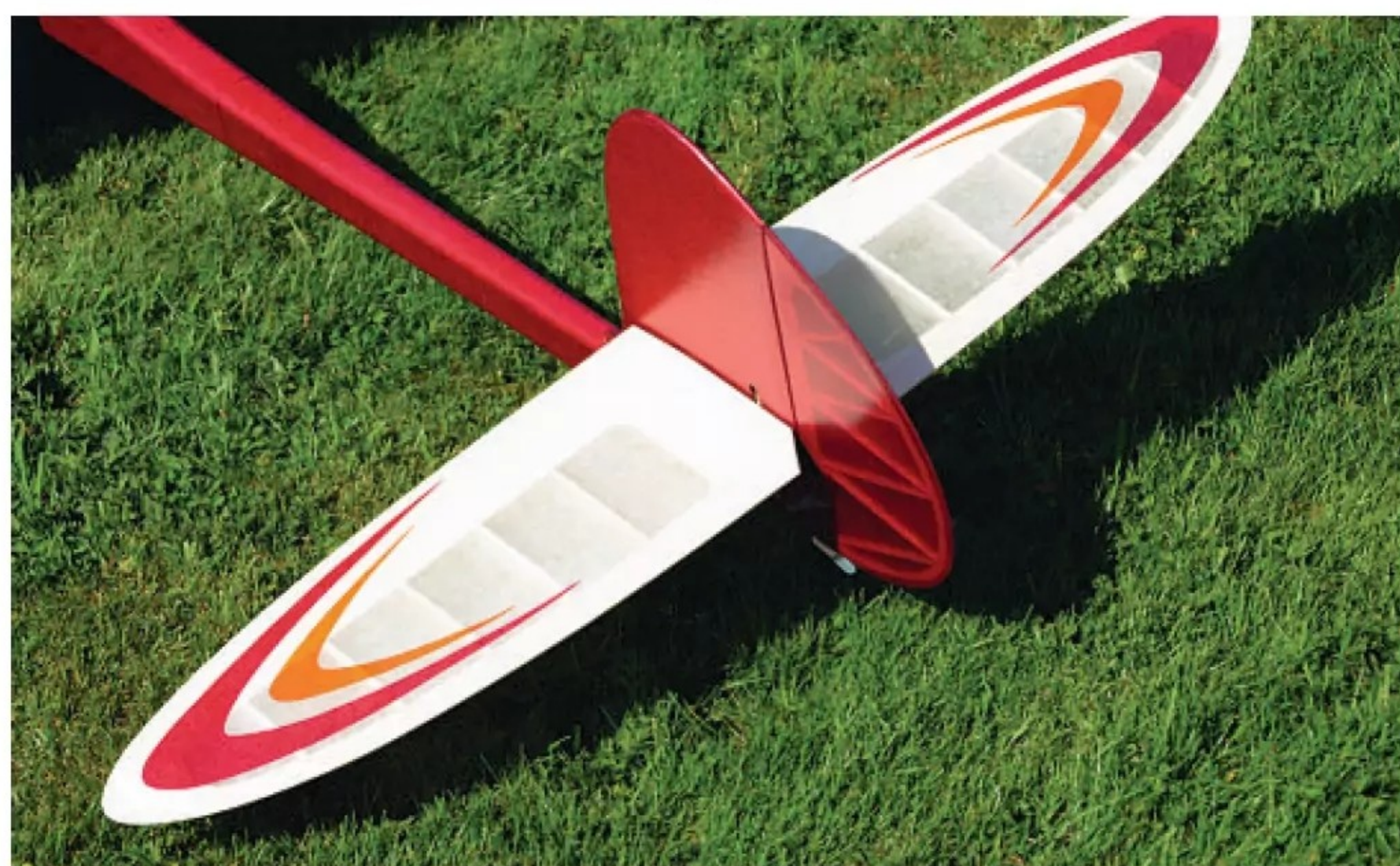
Tail end of the Comtesse. Covering is burgundy tissue on the fuselage and vertical tail, cream tissue over Doculam on the tailplane, with doped-on tissue decoration.
