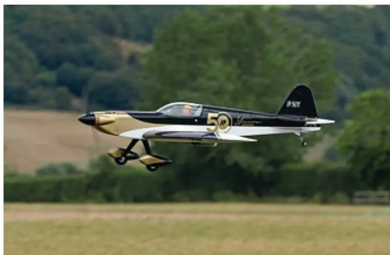
Challenger is fitted with a sturdy undercarriage with painted spats. Keep a check on the wheel retaining bolts. One of mine came loose and the spat came off.
