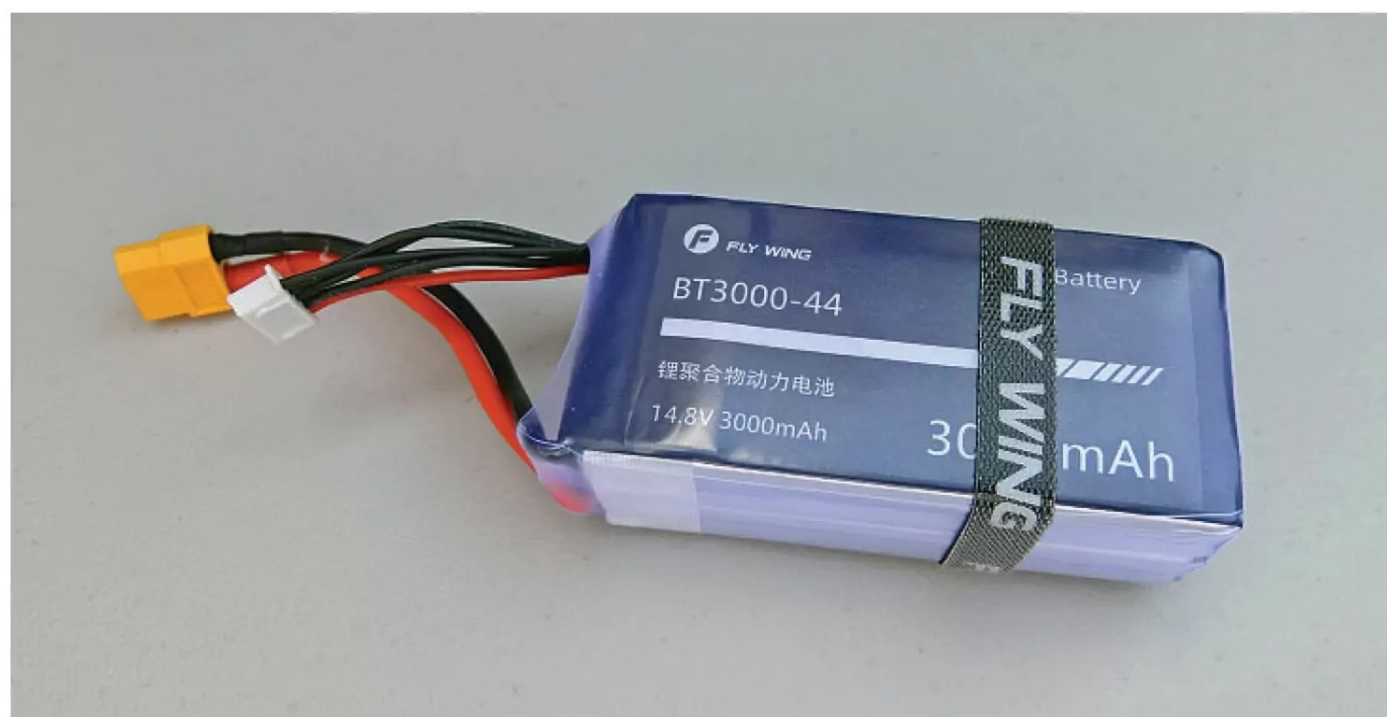
A 4S 3000mAh brick style LiPo is supplied, complete with a hook and loop hold down strap.
