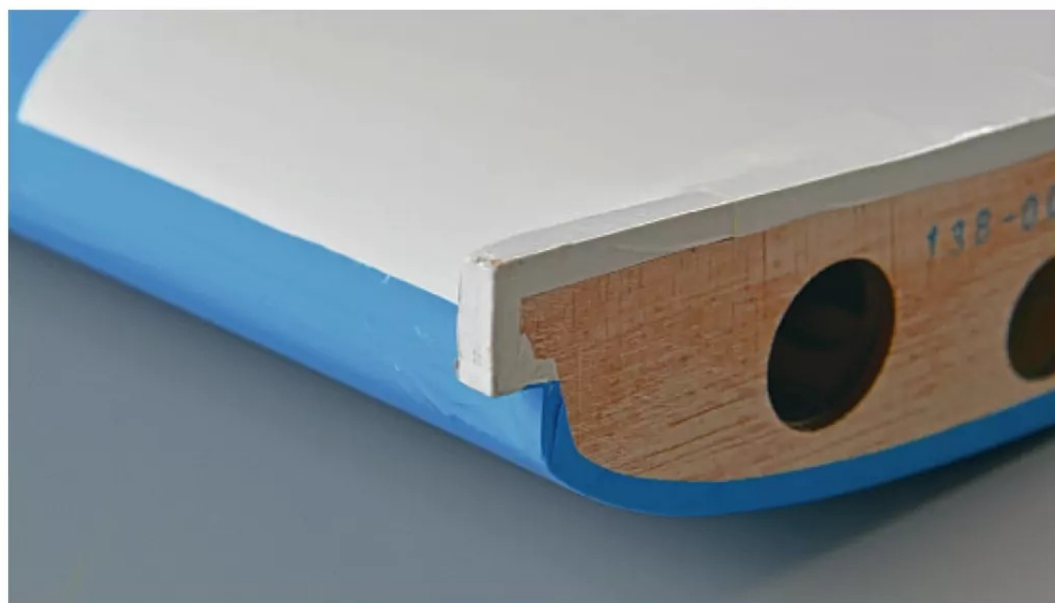
Front wing retaining lug. When paired up with the other wing this makes for a robust wing fixing. Two plastic bolts are used to secure the back of the wing.
