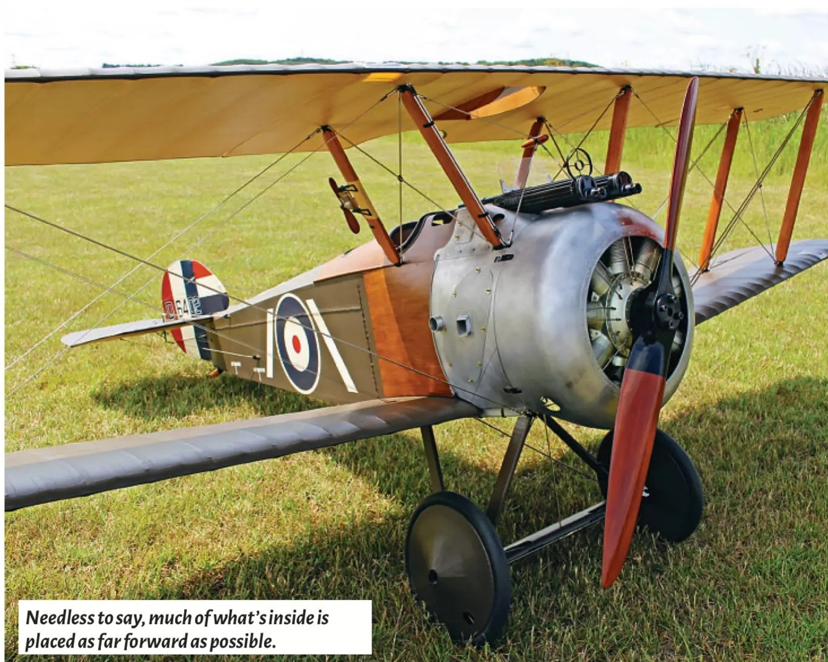
Sprayed 'Guild Materials' paint no. PC10 provided the main colour, sealed with a semi-matt coat of polyurethane varnish.
