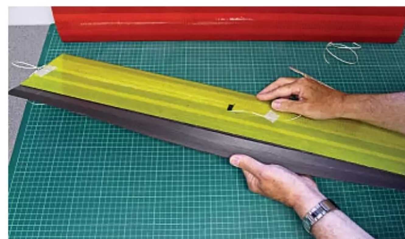
Cut the foam along the aileron hinge line part way through and the foam should snap cleanly along the fold line.
