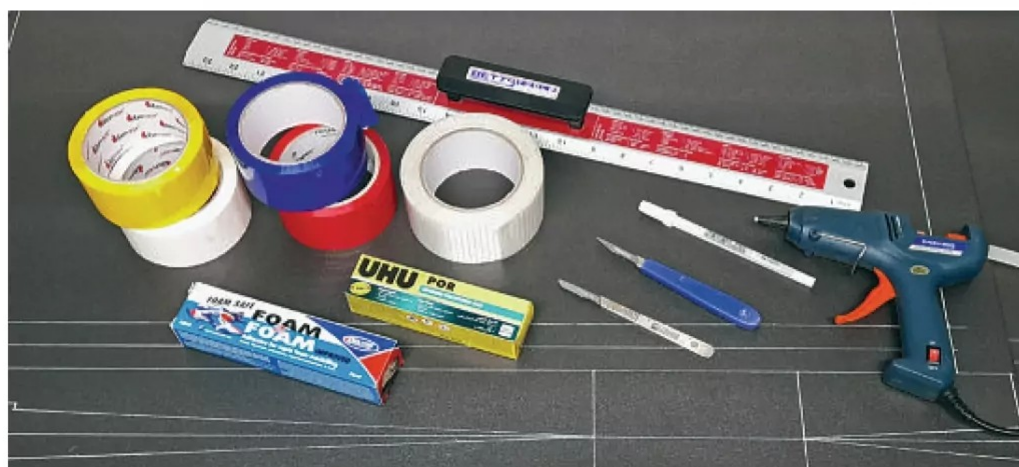
Main material is 5 mm Vitrex foam underlay, with fibreglass cross-weave tape and packing tape added for strength and colour. Fresh knife blades are a must! Mark out with a white gel pen.
