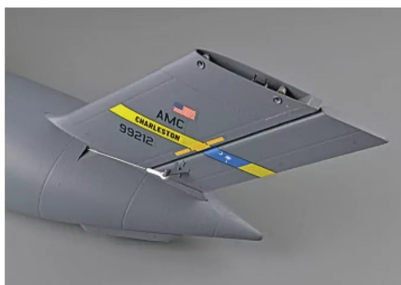
The elevator servo connector is mounted inside the tail mount on top of the fin.
