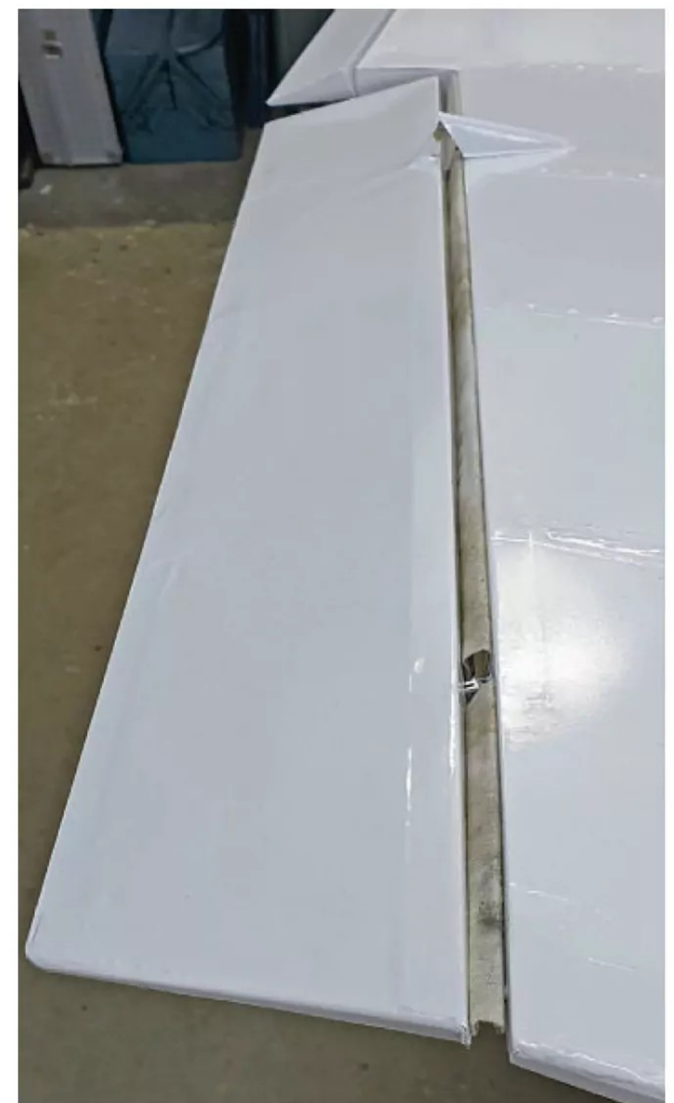
Leather sealing strip between an aileron and wing.
