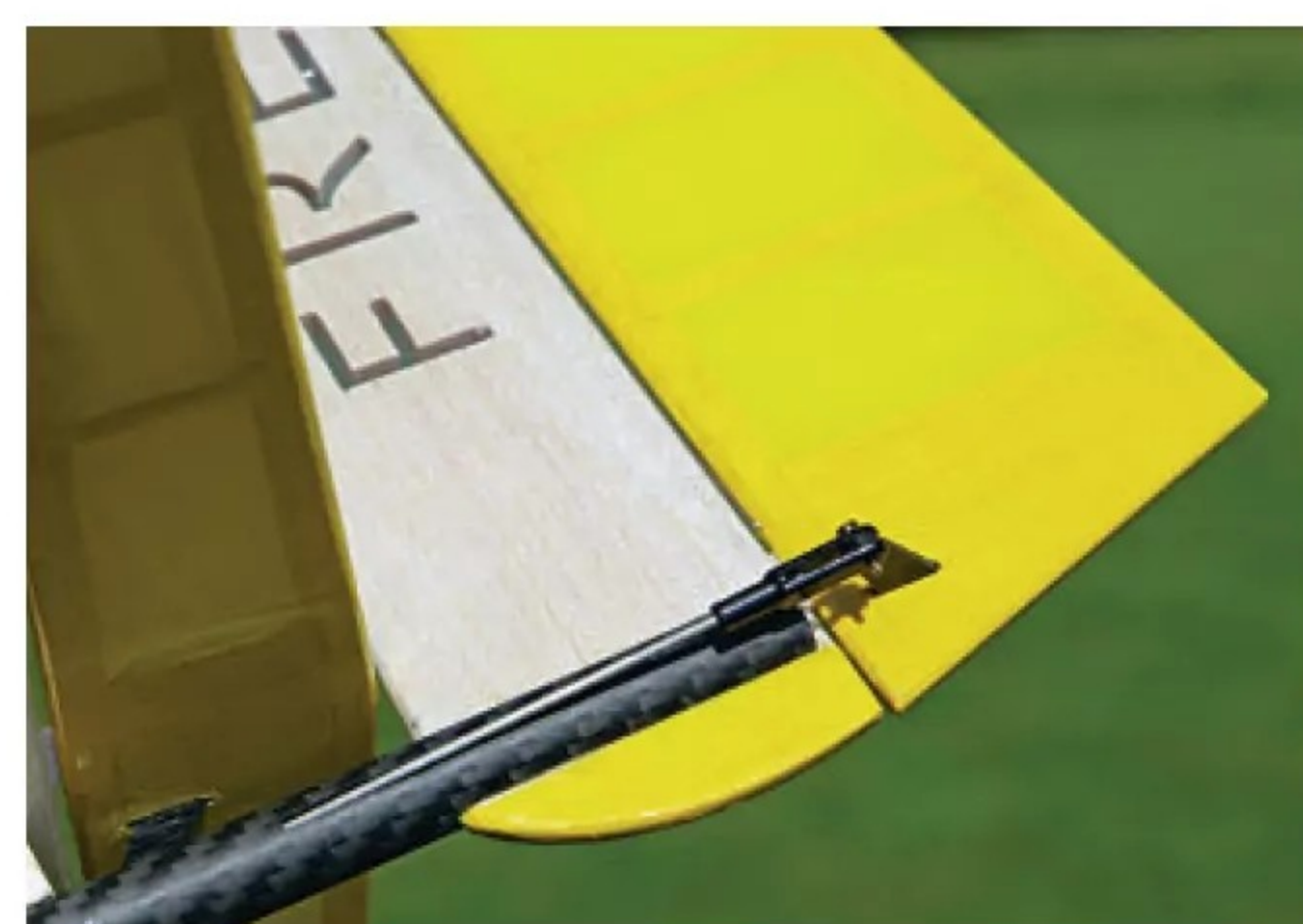
Everyone replaces the sprung tail control surface pull cords with carbon push rods.
