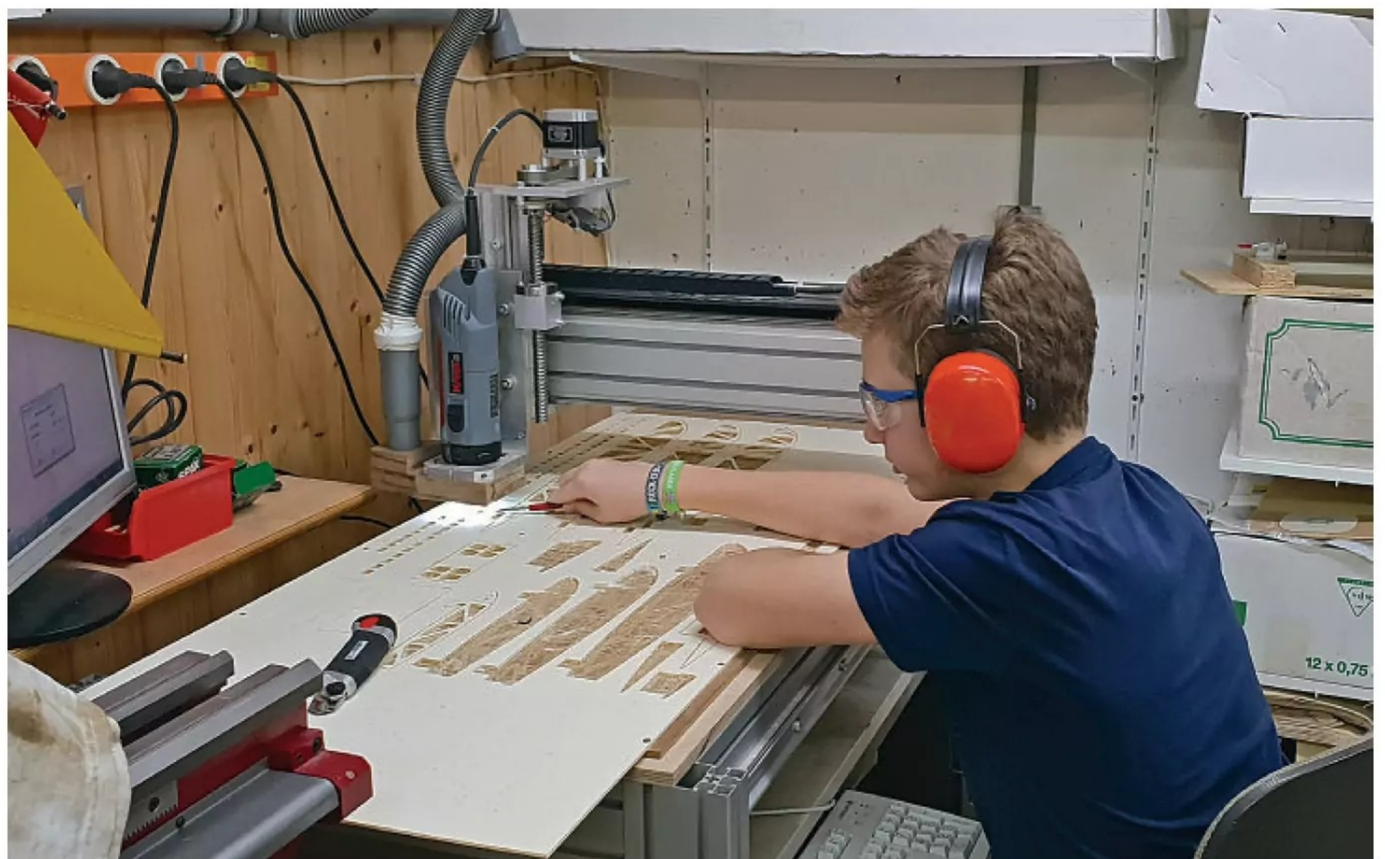
Cutting all the parts with the CNC milling machine.
