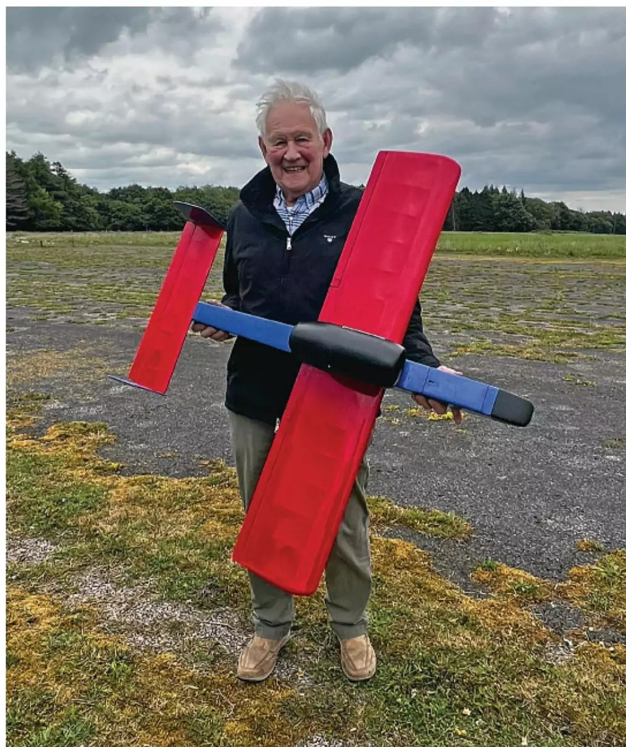
ACT's model with the pod on top is a Tresster, his version of Dick Sarpoulius' Jester which was used as a power unit test bed. Again, built in the 80s, the Tresster originally had a pod fitted with a Cox TD .051 and various .09 ducted fan units and pylon mounted prop units to compare performances. More recently, Alec has been testing XFly ducted fan units and has conclusive proof of their efficiency over the EDF units he previously used. Always looking to progress, ACT has recently fitted an airspeed indicator to the Tresster to further validate his findings. At 86, Alec is still very active and keeping his test pilot Jamie Cuff very busy!
