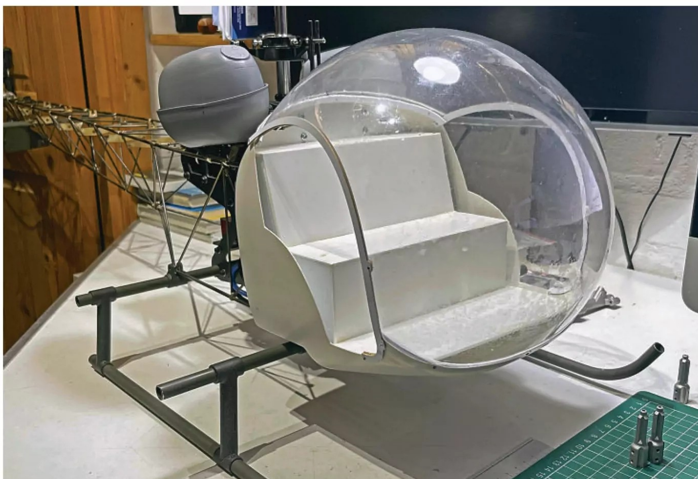
Finished cockpit moulding and bubble canopy. It took a lot of fettling to get a good fit.
