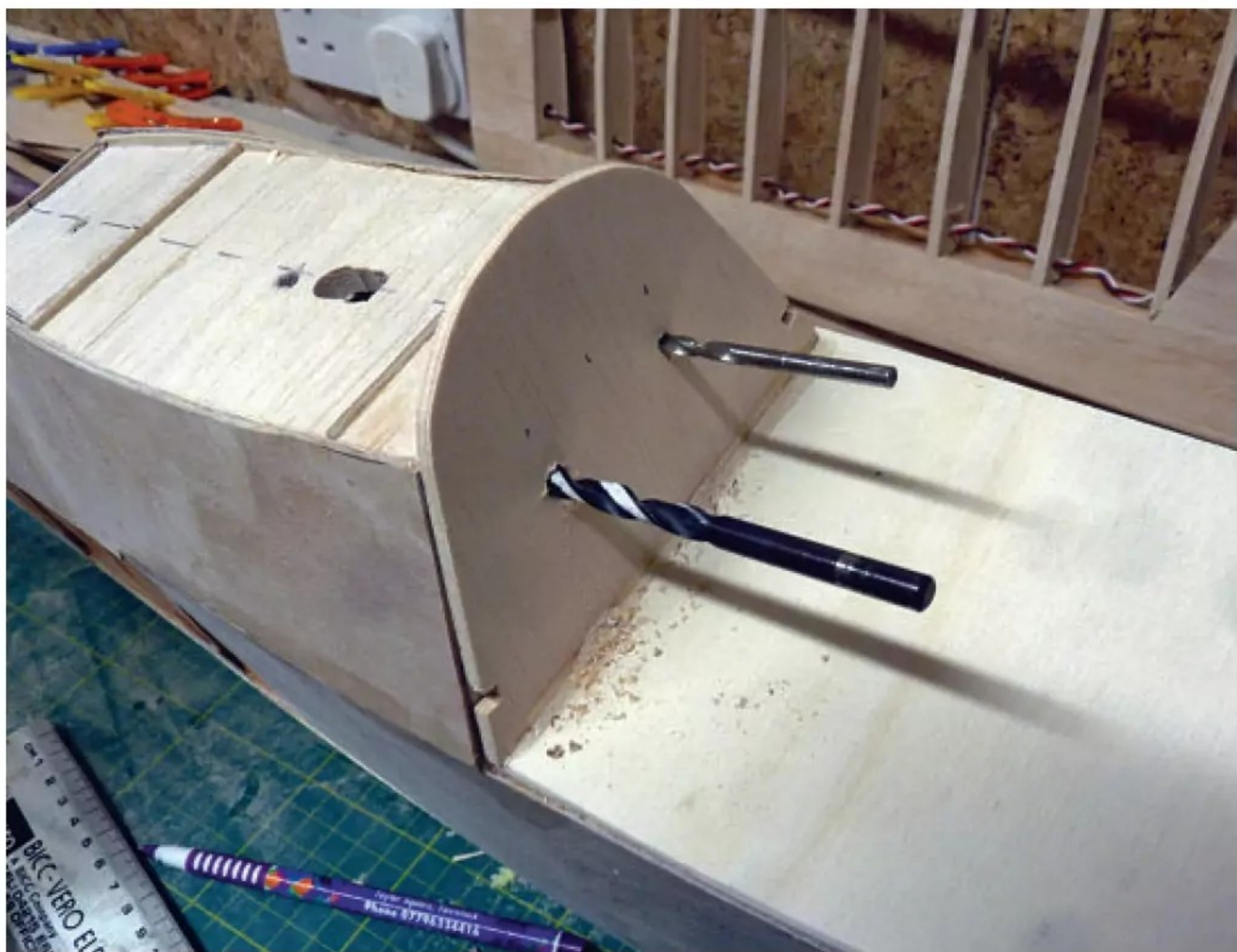
Drilling out for the retention magnets.
