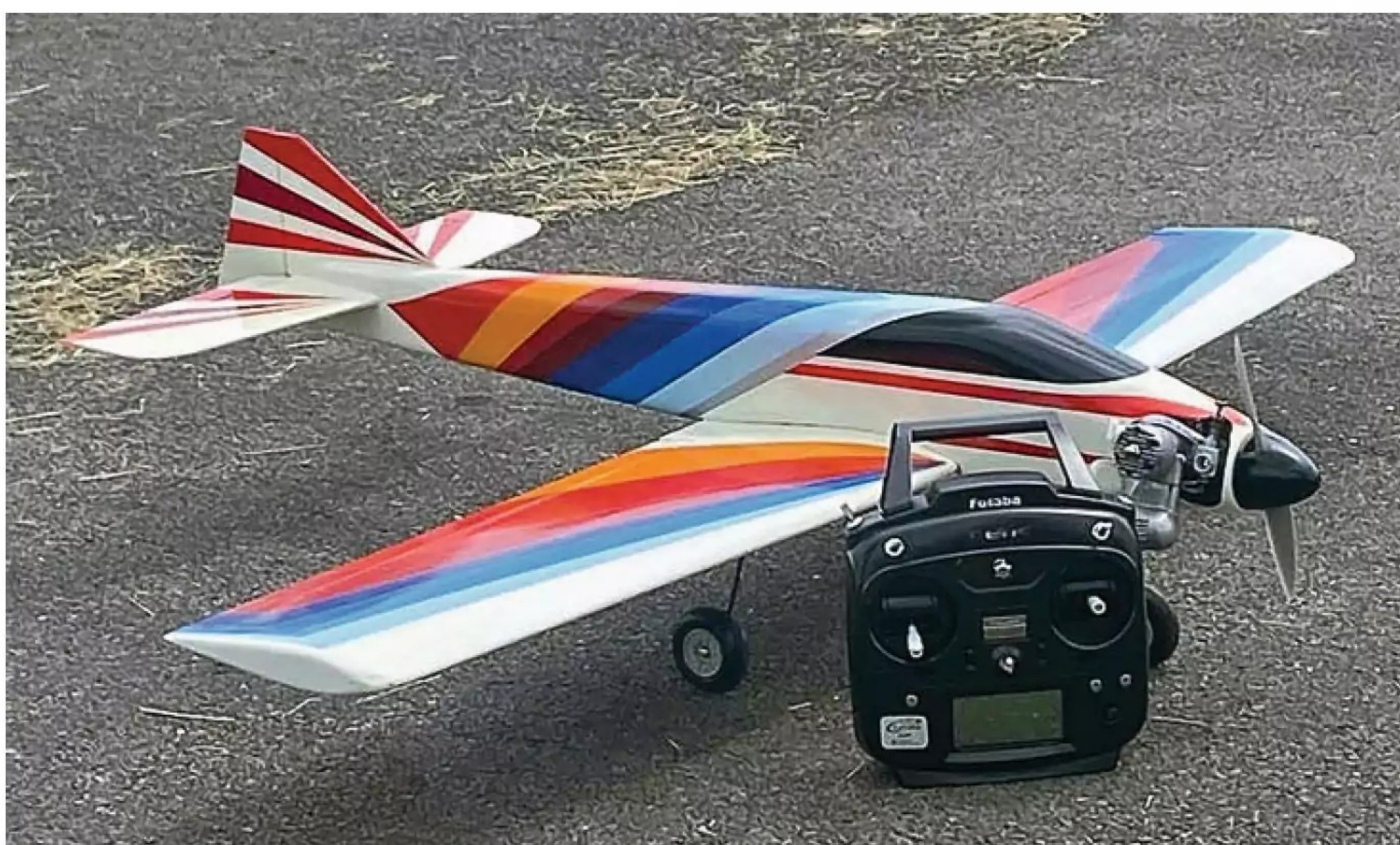
Jamie Cuff's very pretty 42" span Micro Mold Starlet that is O.S. MAX-25FSR powered. All his models are excellent fliers.
