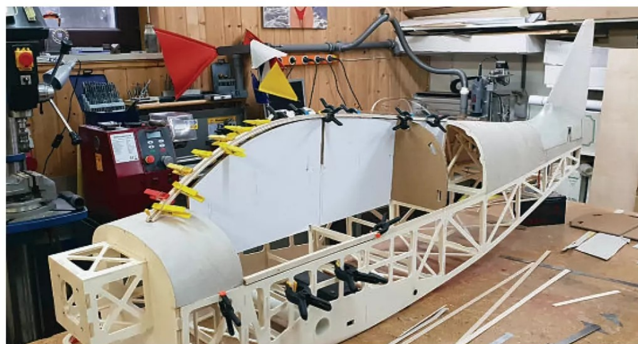
Building the canopy frame.
