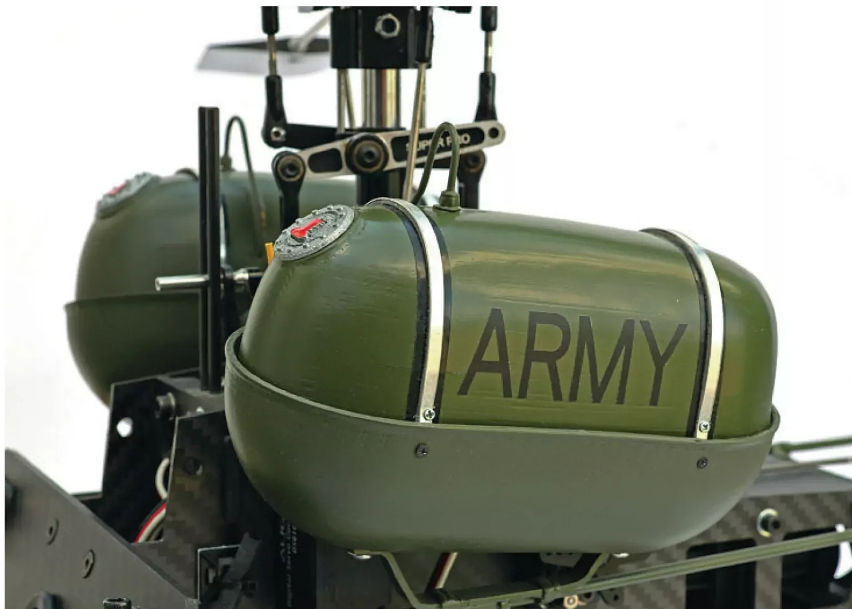
The 3D printed dummy fuel tanks required a lot of sanding and filling!
