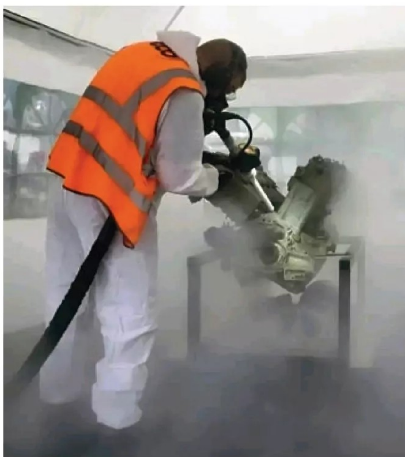
Steven McCreadie, Head of Eco Dry Ice at Eco Group, cleaning the engine with the company's dry ice solution.
