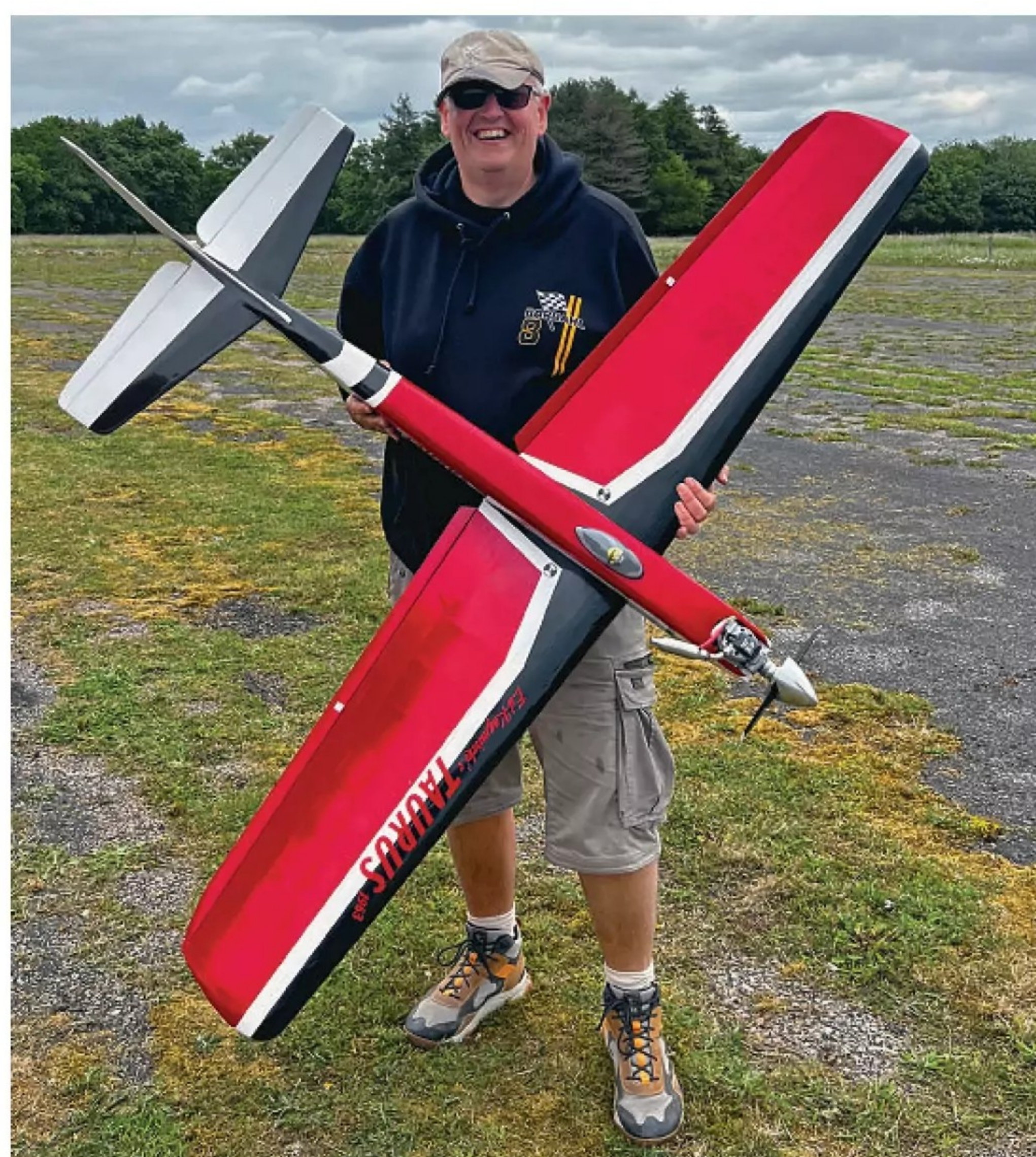
Another classic shape in the form of an Ed Kazmirski designed Taurus. Owned by Jason Hyland, this gorgeous looking model was built by Simon Claydon and is perfectly powered by an O.S. FS-70 four stroke. Looks beautiful in the air!
