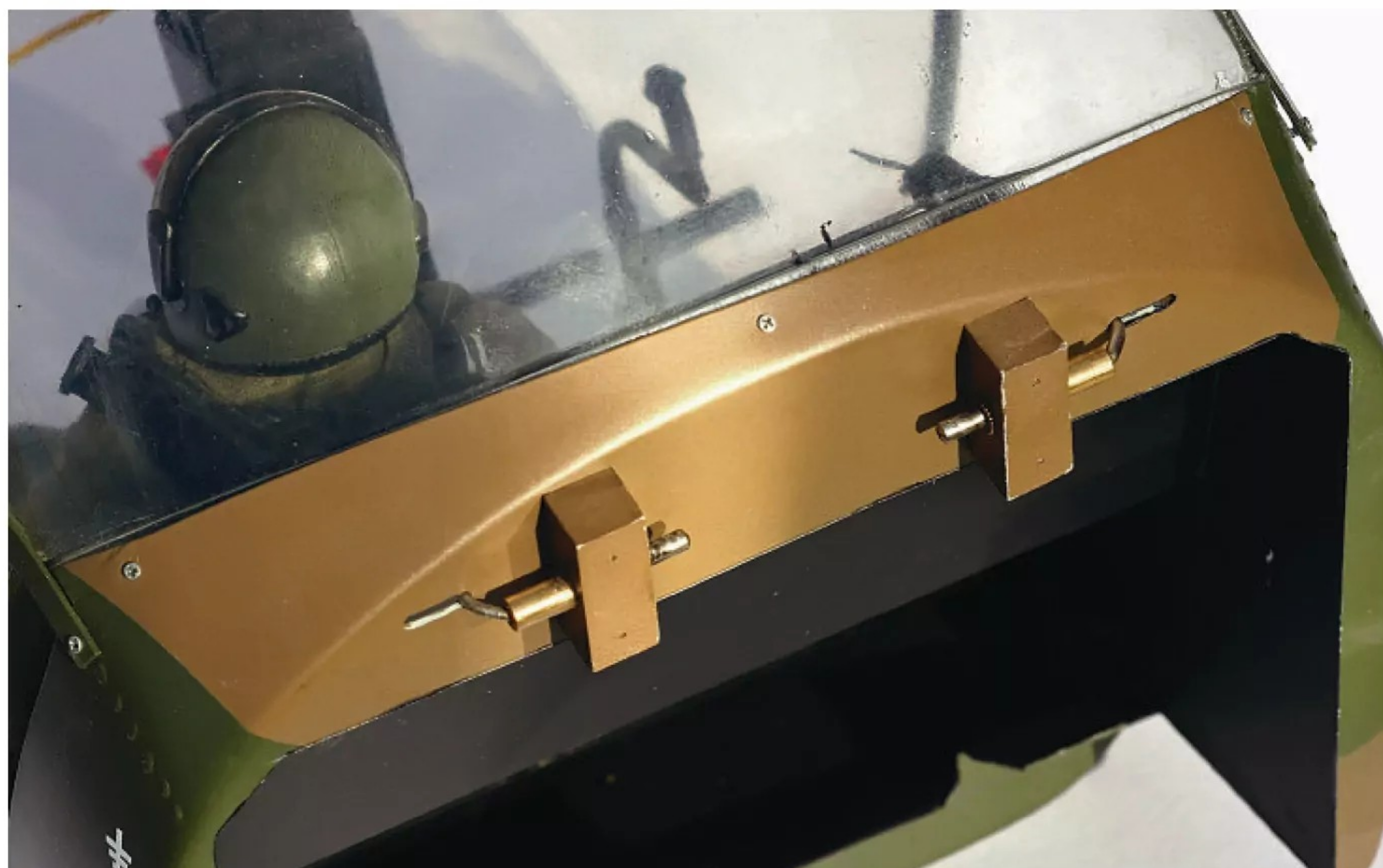
I used a pair of sprung canopy latches to hold the cockpit in place on the chassis.
