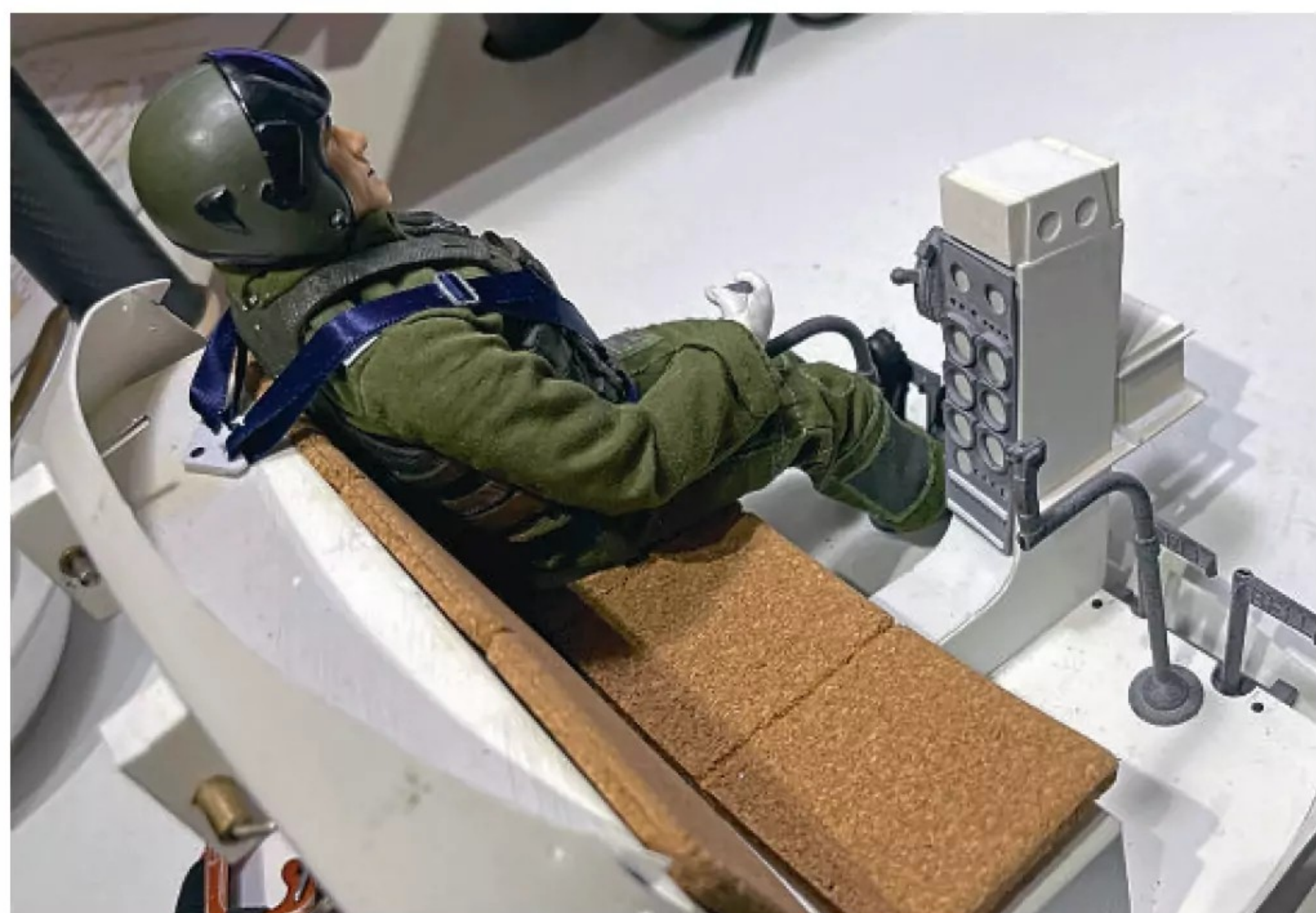
Most of the cockpit is made from styrene sheet, with a few 3D printed details.
