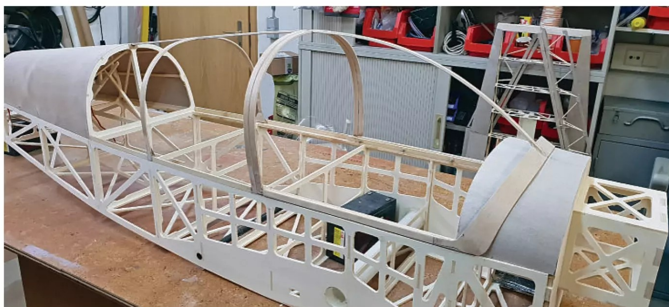
Finished canopy frame fitted to the fuselage.
