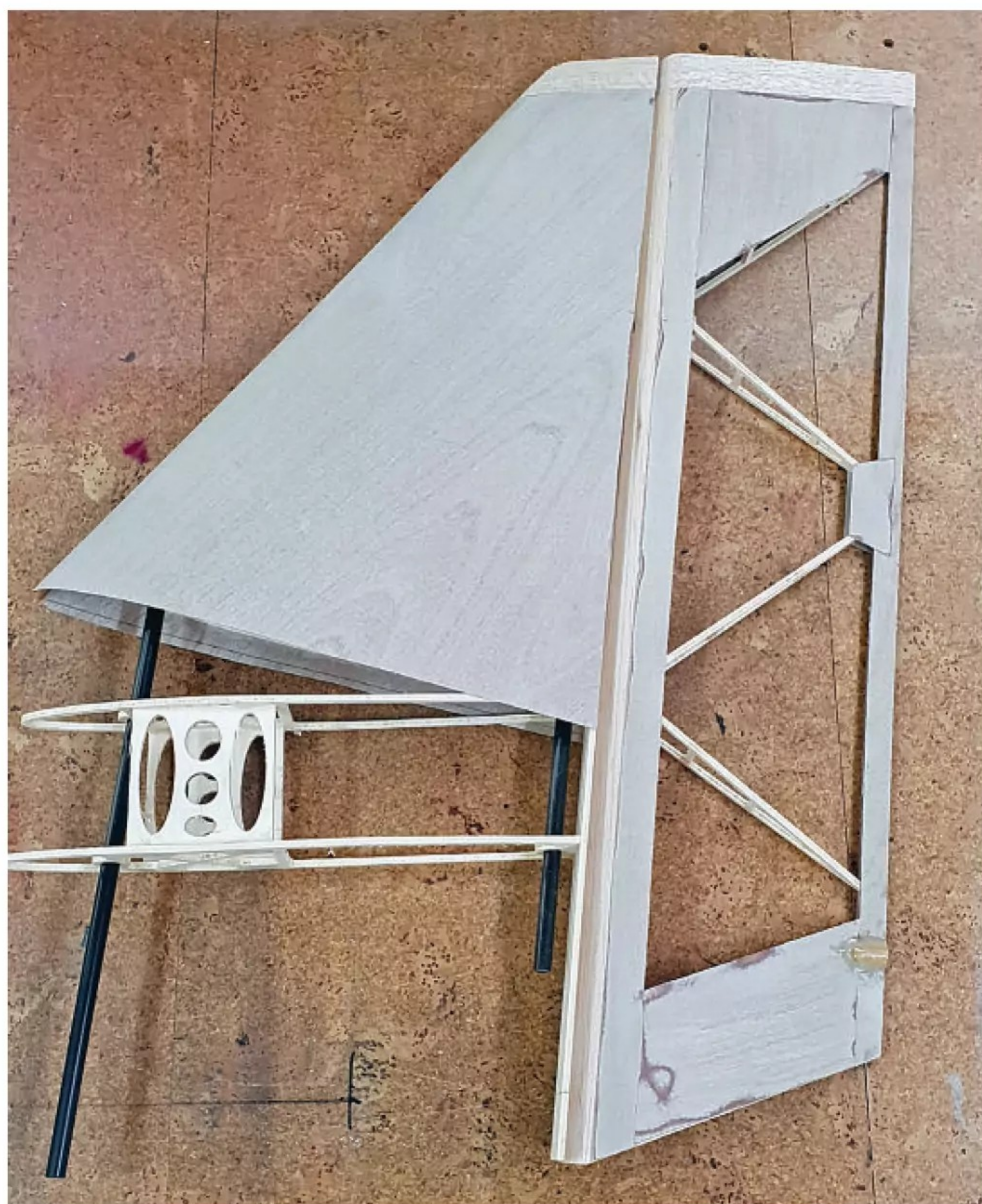
The same ply sheeting is used for the vertical stabiliser.
