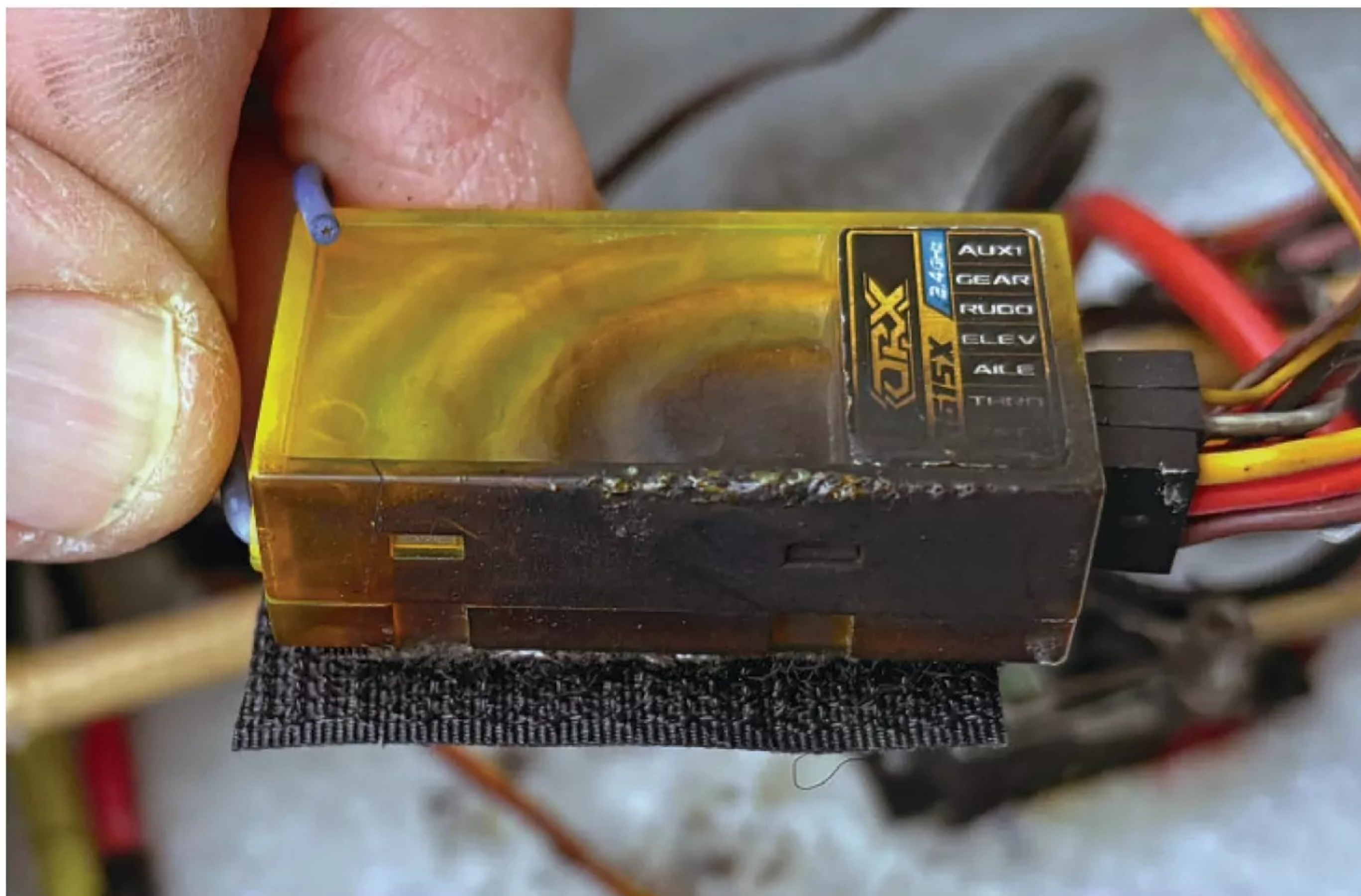
The receiver's hard case protected it from internal damage.
