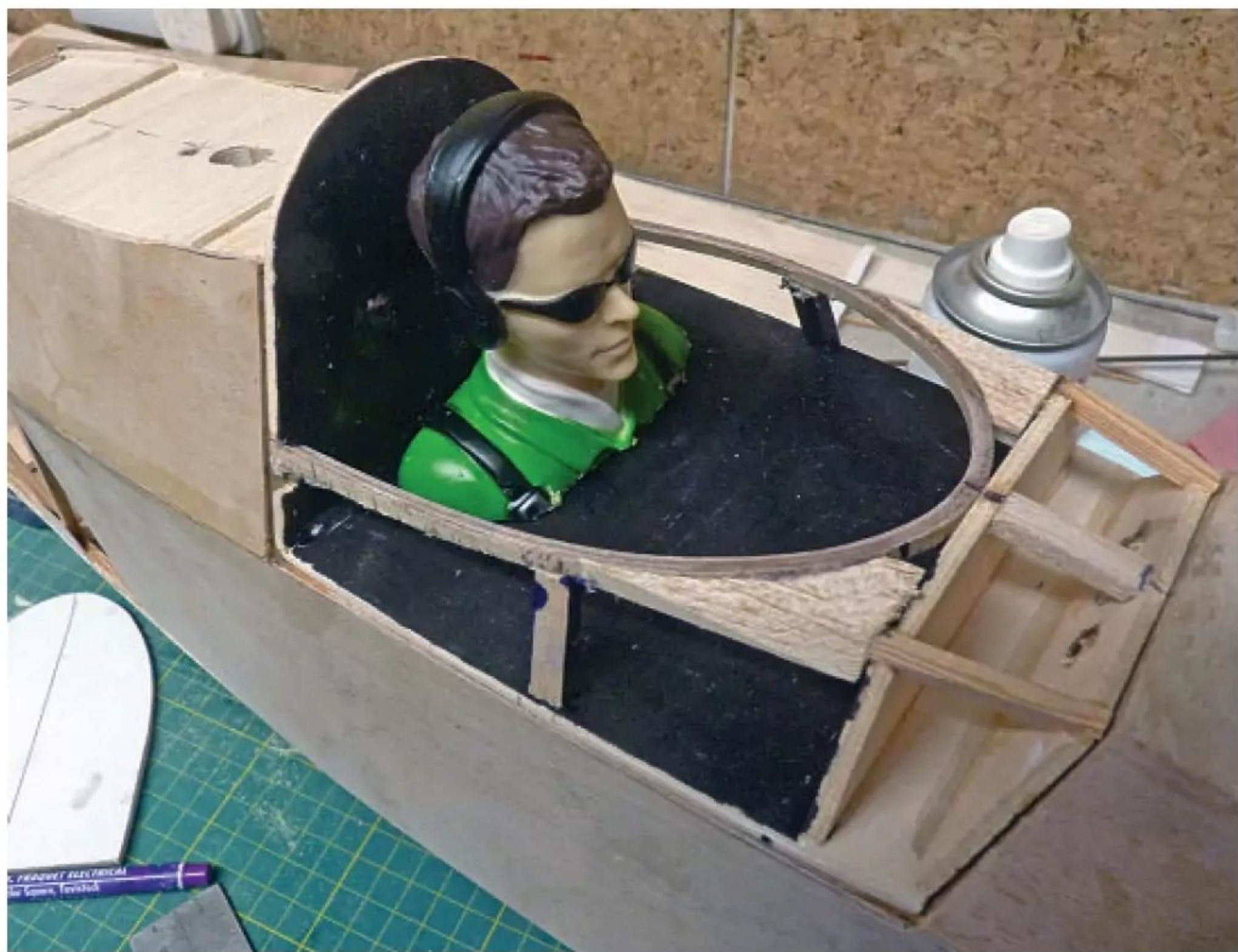
Basic framework of the canopy/hatch.
