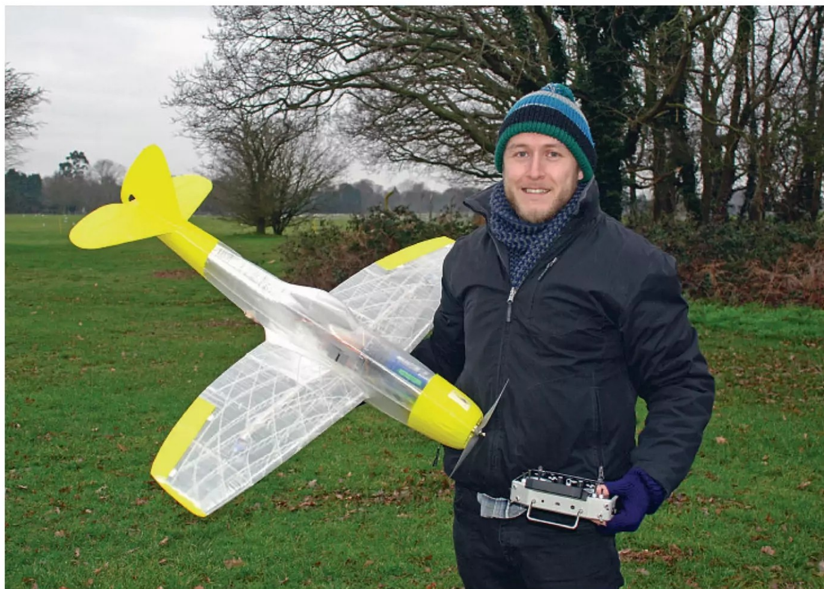
Jack looks pleased with his printed plastic P-47. It flew well after reinforcing the butt joints.
