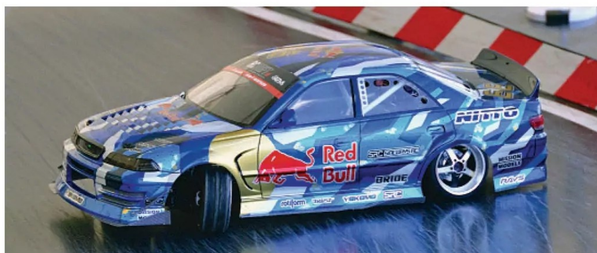
The giant marquee at the show housed lots of interesting activities including a Drift Car circuit. Drift cars have an impressive lock on the front wheels and adverse camber on the rear to help them travel sideways around the track
