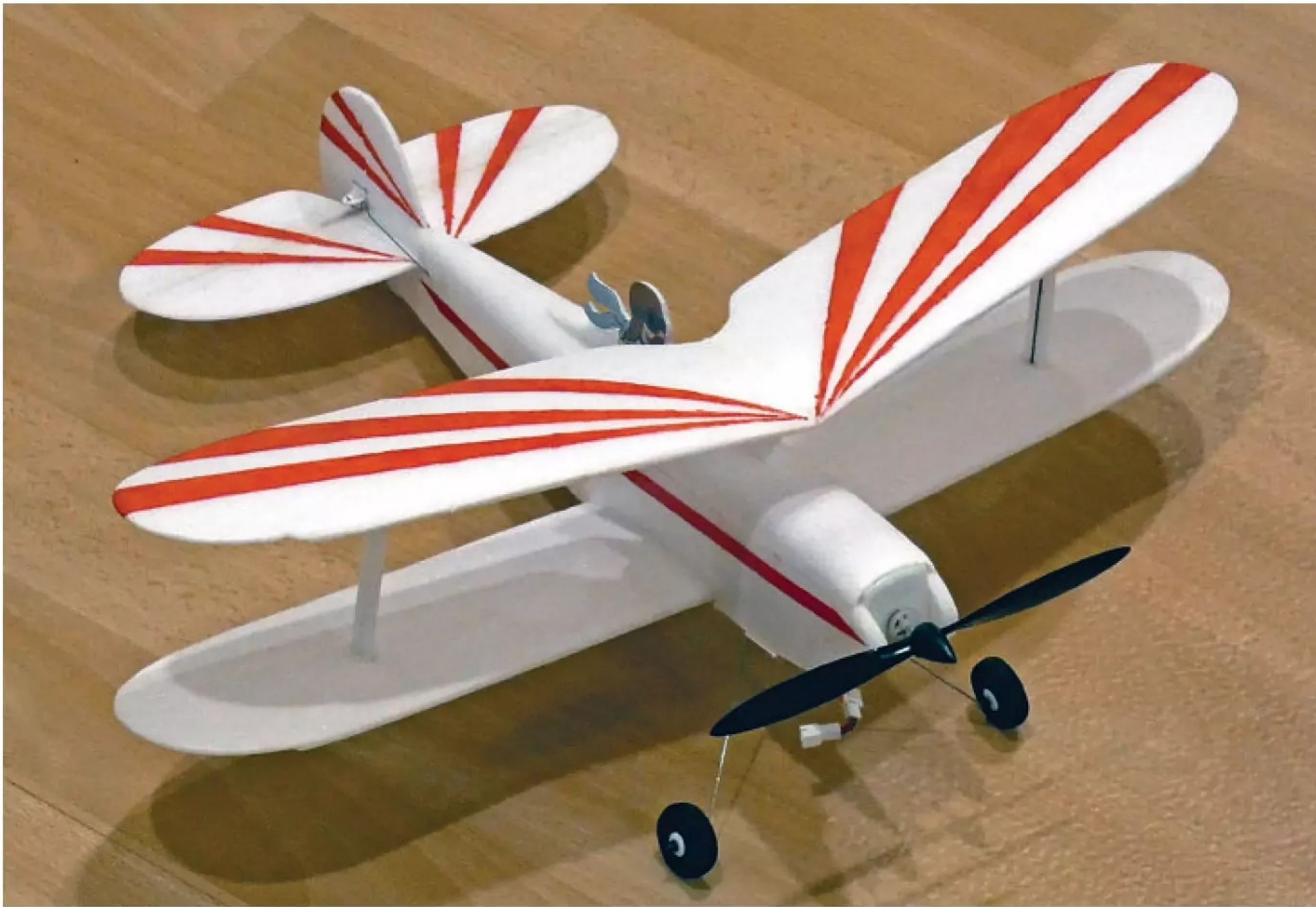
John's Prairie-E-Duster biplane uses a standard 1S LiPo and a coreless geared motor unit
