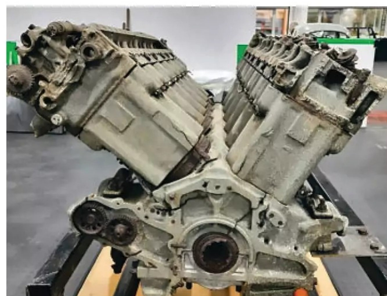
Rolls-Royce Merlin engine after being cleaned by Eco Dry Ice.
