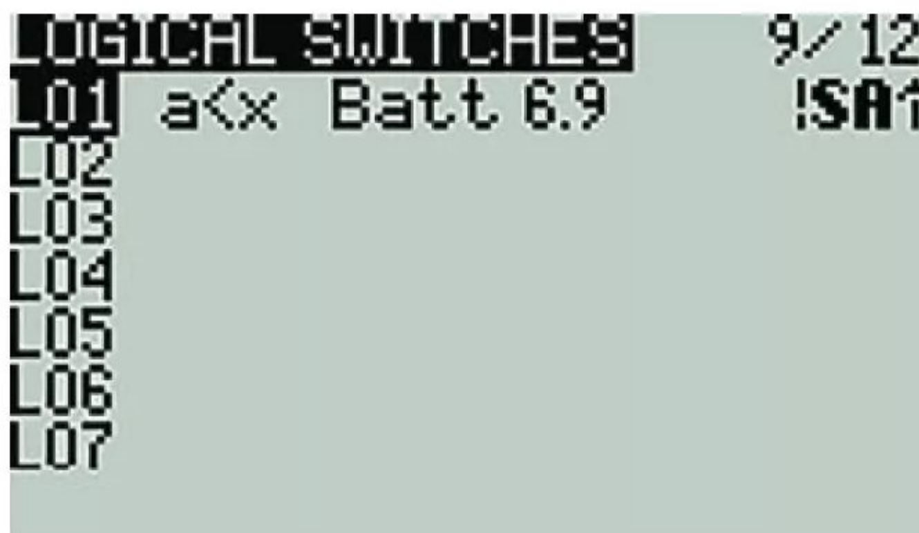
Logical Switch monitoring Battery Voltage.
