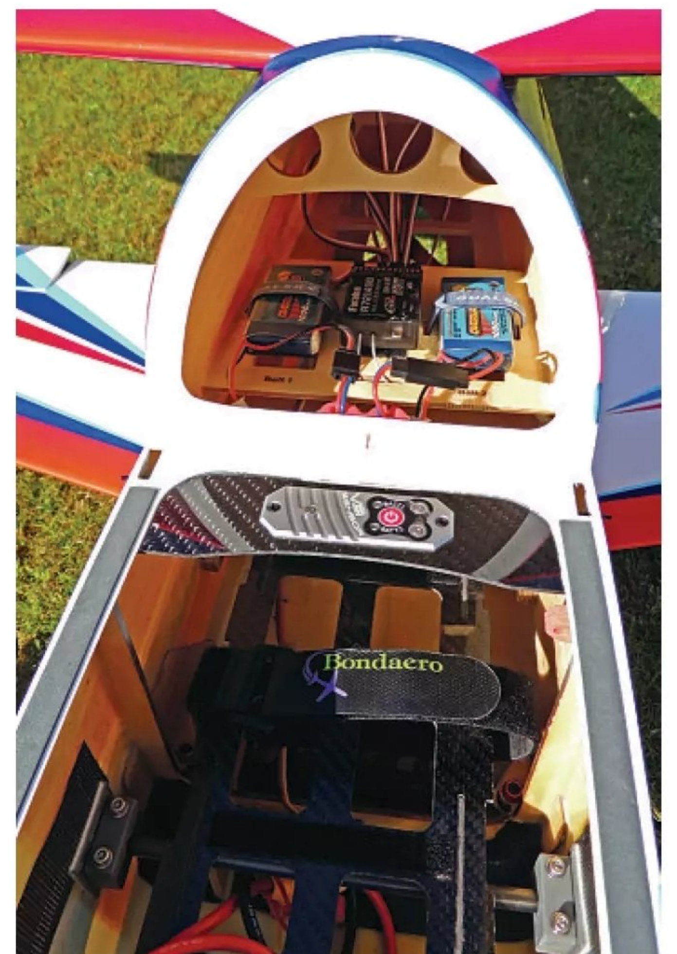
Receiver location rearwards of carbon components to prevent RF shielding. Powerbox Digiswitch V3 with twin LiPos for power.
