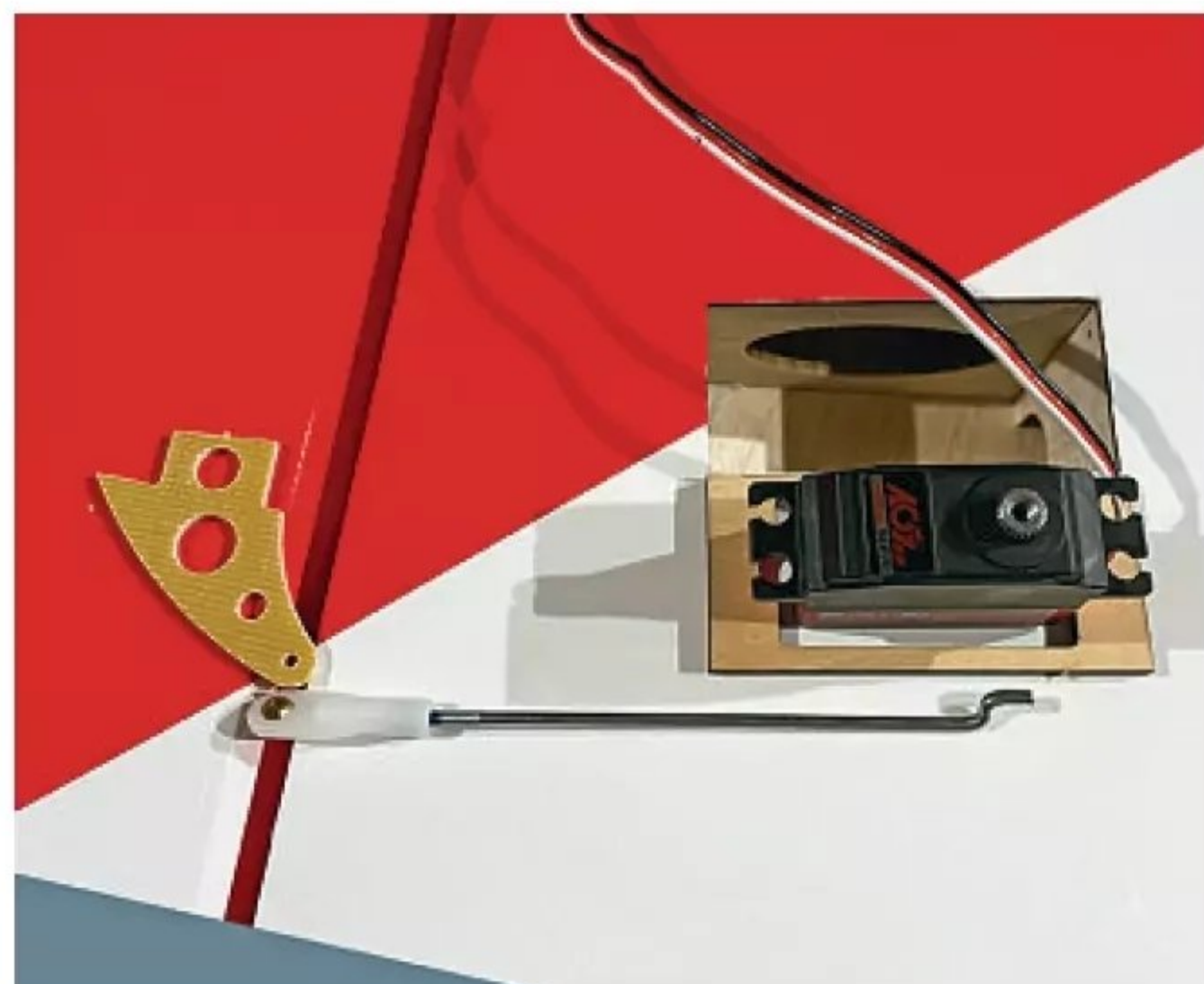
One of the wing servos sits astride its laser cut mounting plate. You can see that screws dropped through the mounting holes will not all bite into wood if left like this.
