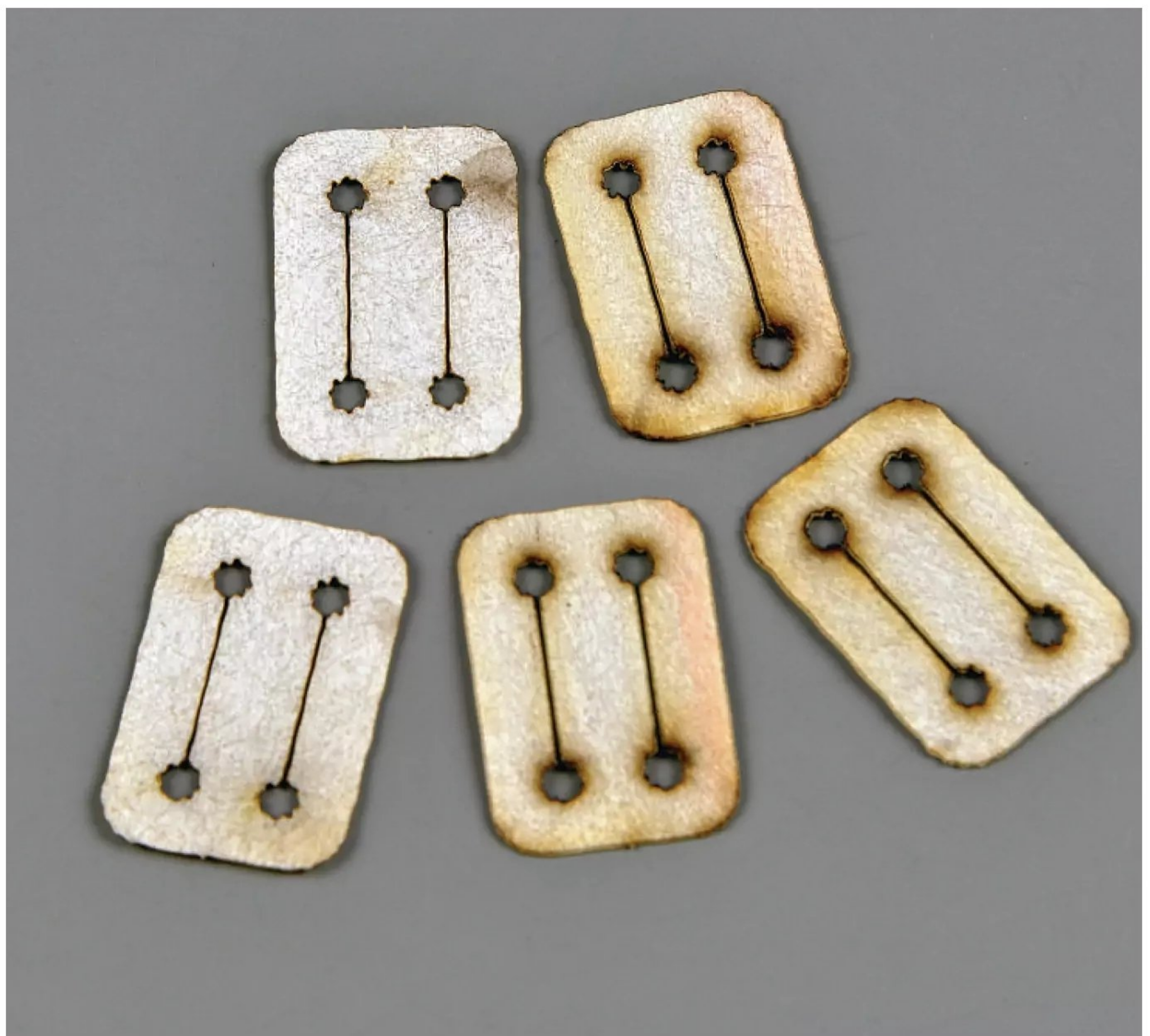
Laser cut furry Mylar hinges. Note the slits which provide an effective way of wicking cyano into the wood when inserted into the panels and control surfaces.
