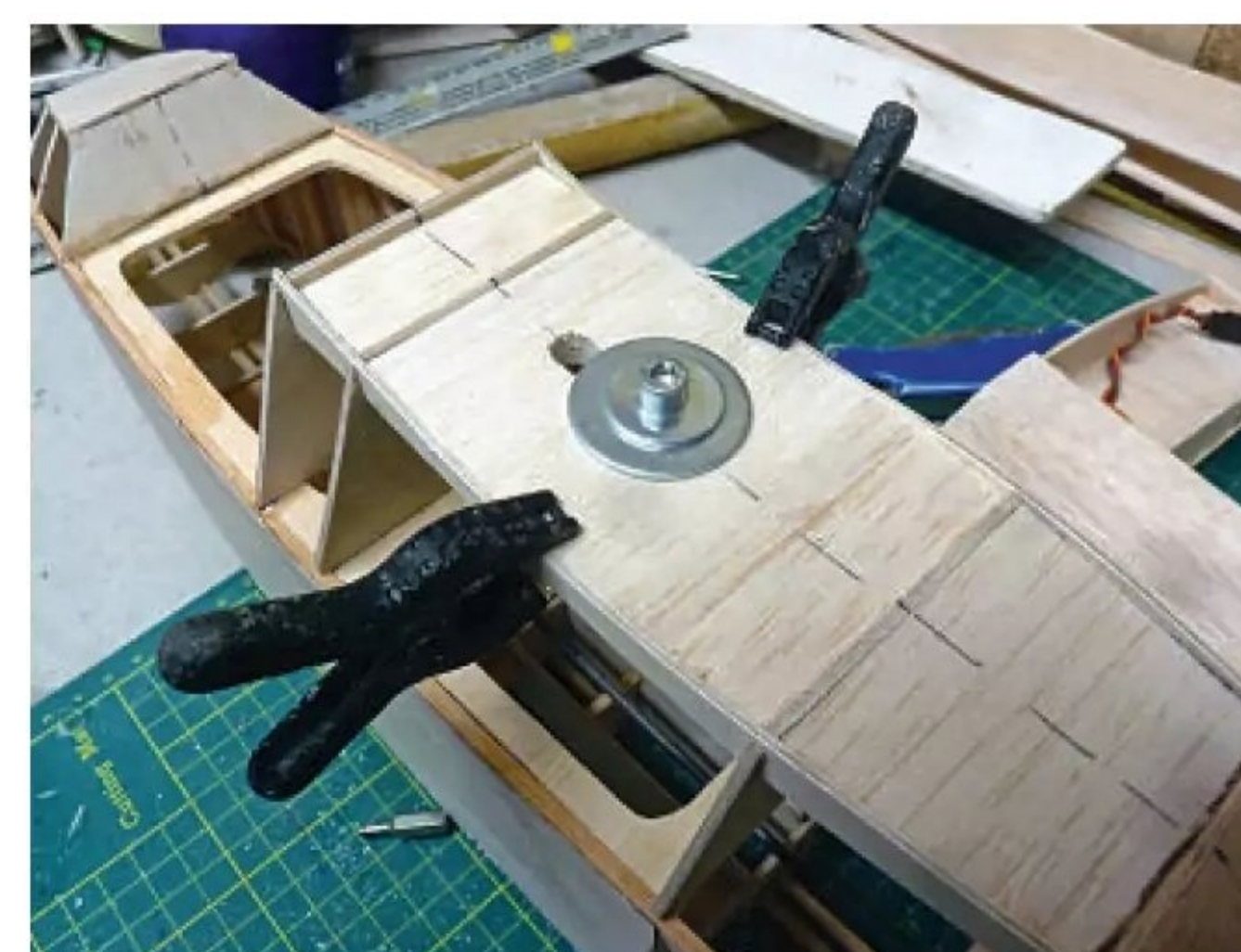
Fixing one of the captive nuts for wing retention.
