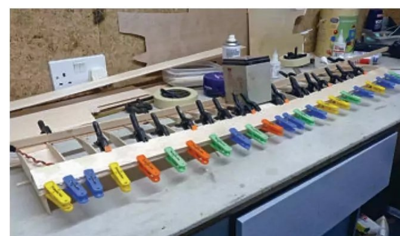
Adding the top sheeting with the wing jiggged up.
