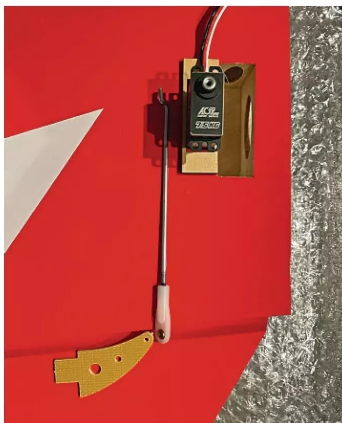
Ditto the elevator servos. Note the use of longer control horns at the tail to reduce control movements compared to the shorter horns used for the ailerons.
