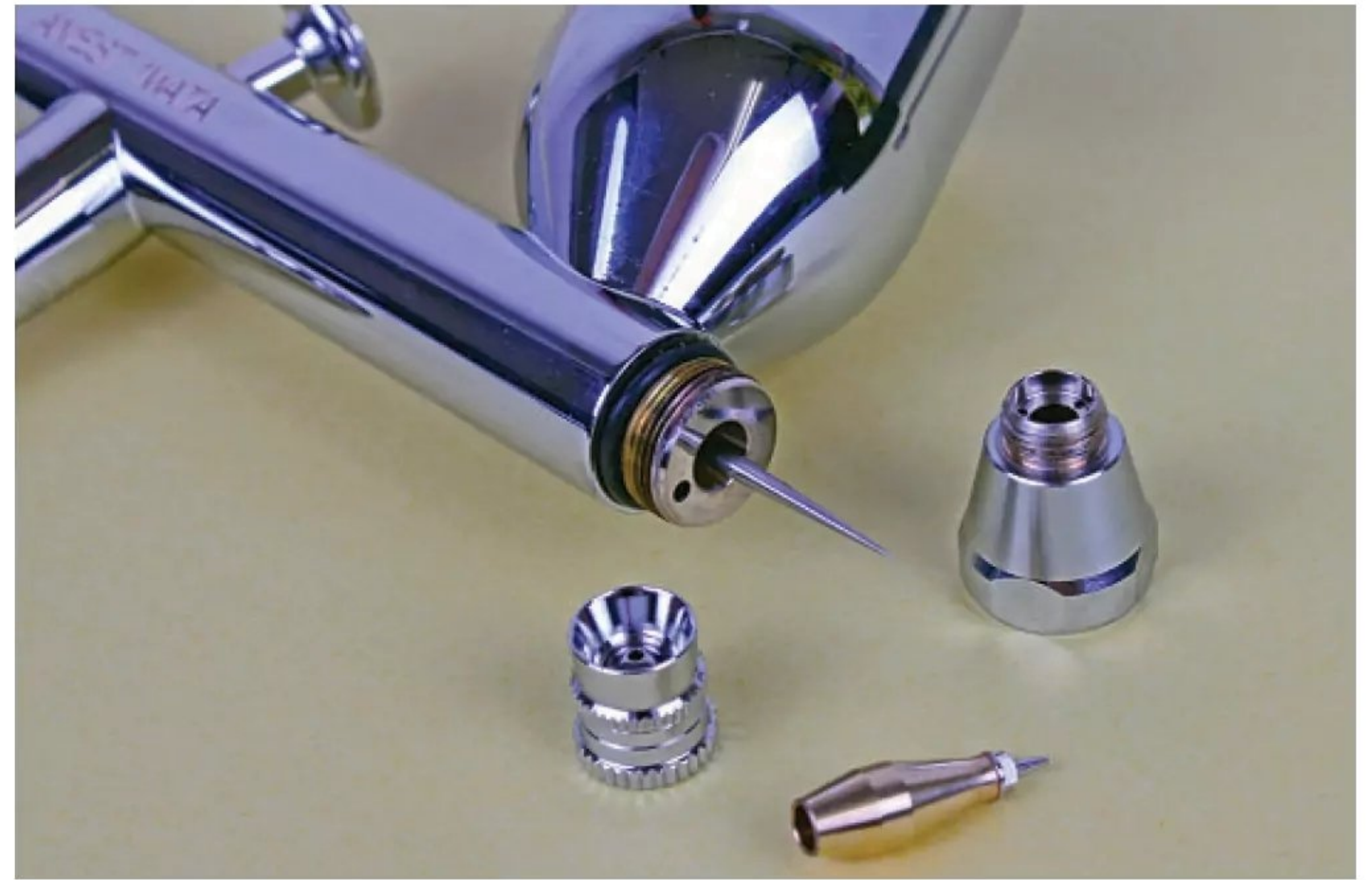
Spray head parts. All should be removed and cleaned after every session.
