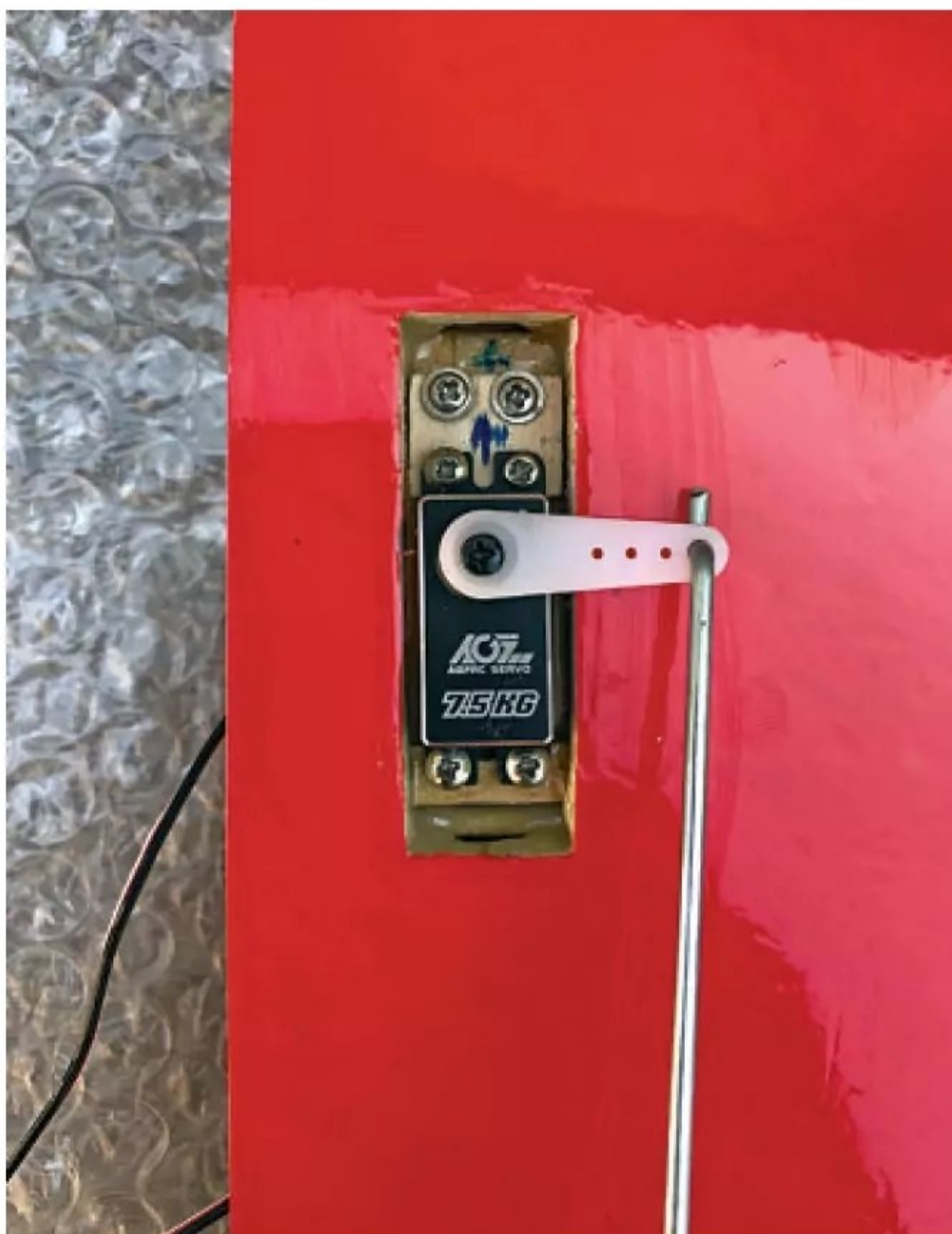
It might only be a small elevator servo, but I still used all four mounting screws. Six if you include the two screws used to fix the additional plate to the original servo mount.
