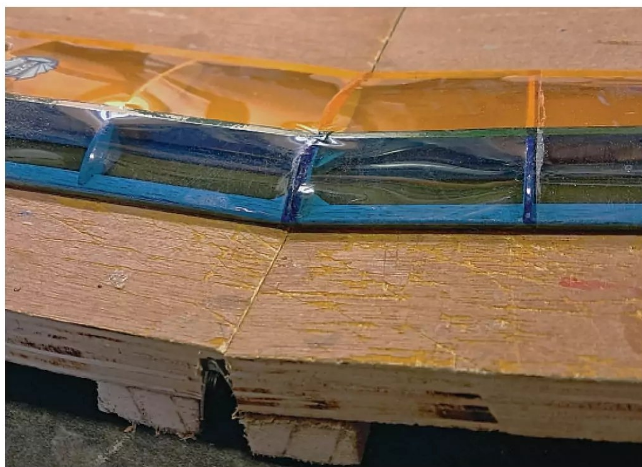
It's as rough as a Bear's chuff but my old building board serves one last duty. Hinged in the middle it allows dihedral to be built-in direct on the board.
