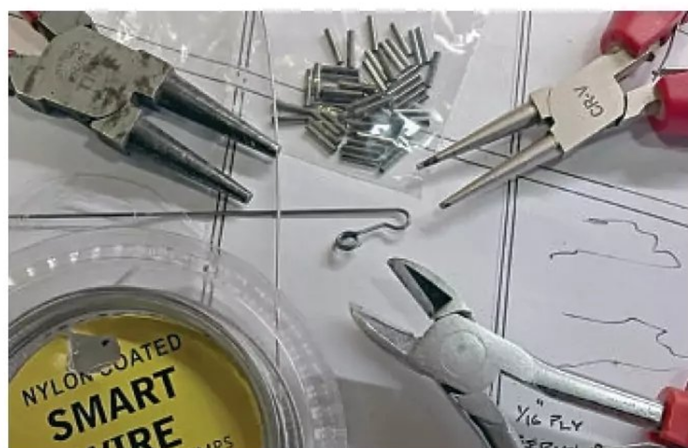
All you need to form your own hook and loop ends, then attach them. The coated wire and crimp ferrules are cheap fishing equipment.
