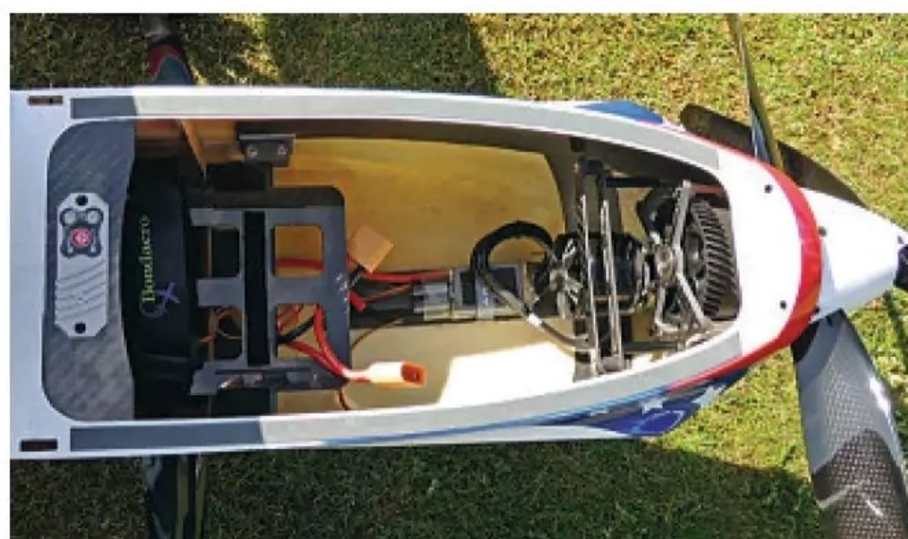
Internals of the Skyleaf Leader biplane showing the CRS3000 contra drive and D3 ESC.
