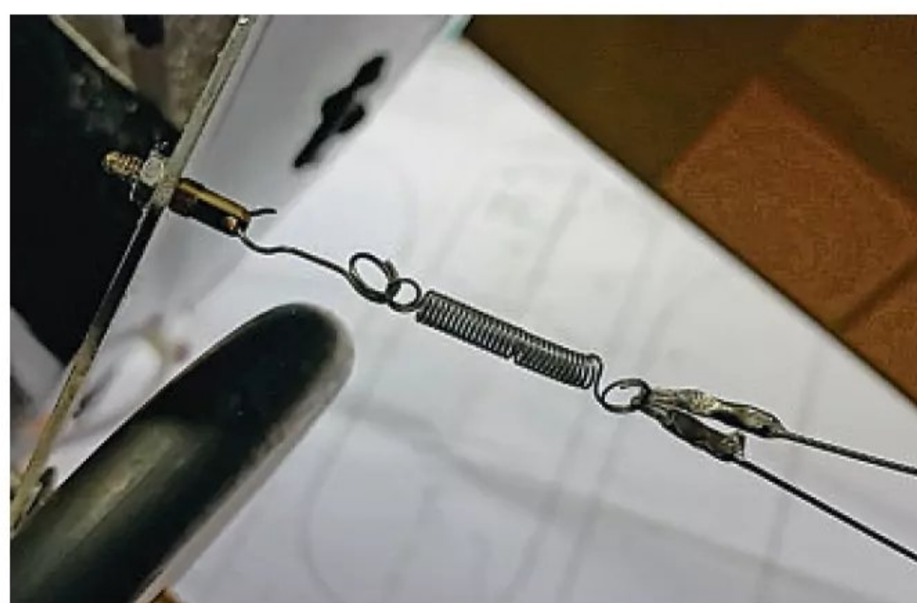
Moustique lower rigging attachment. Steel fishing trace, crimps, spare spring, brass closed loop end fitting and a handmade hook/loop - simples!
