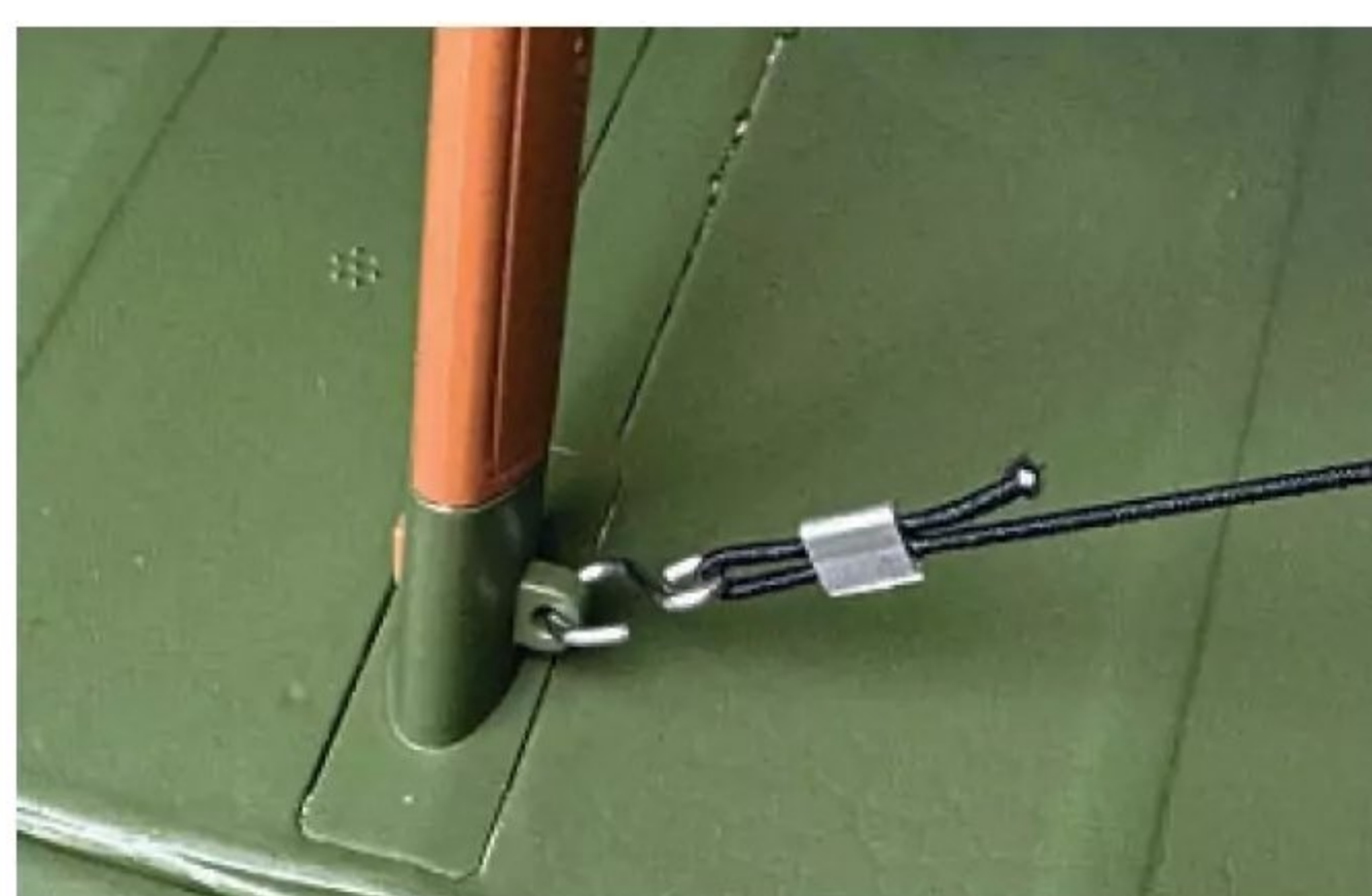
Elastic flying wires hook on to moulded loops on the struts.
