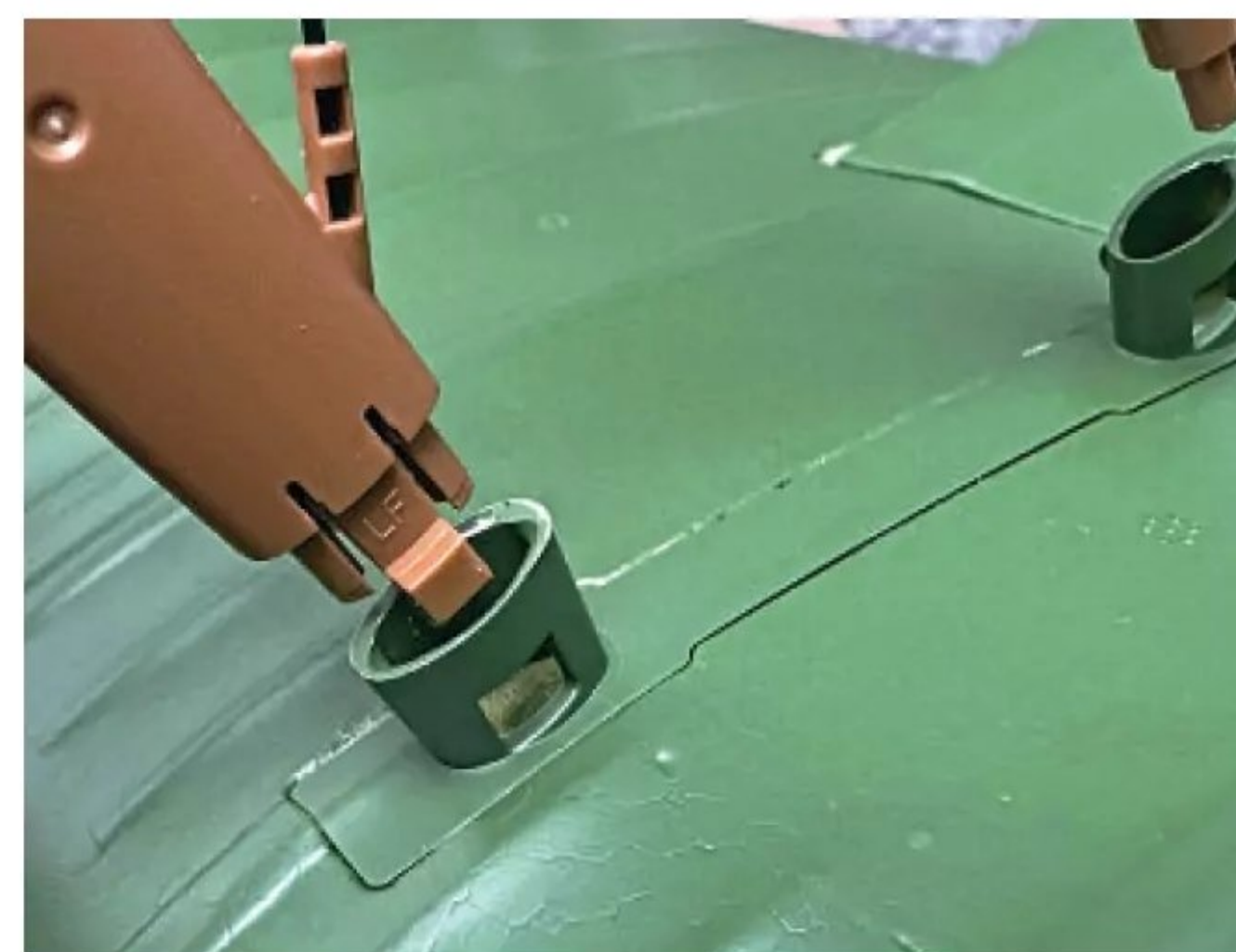
Wing struts have clever clips to hold them in place.
