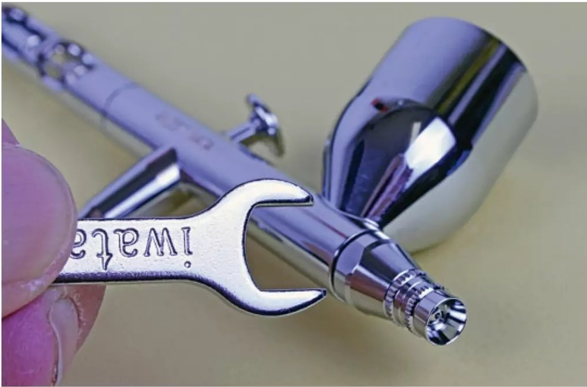
A small spanner helps secure and release the head cap.
