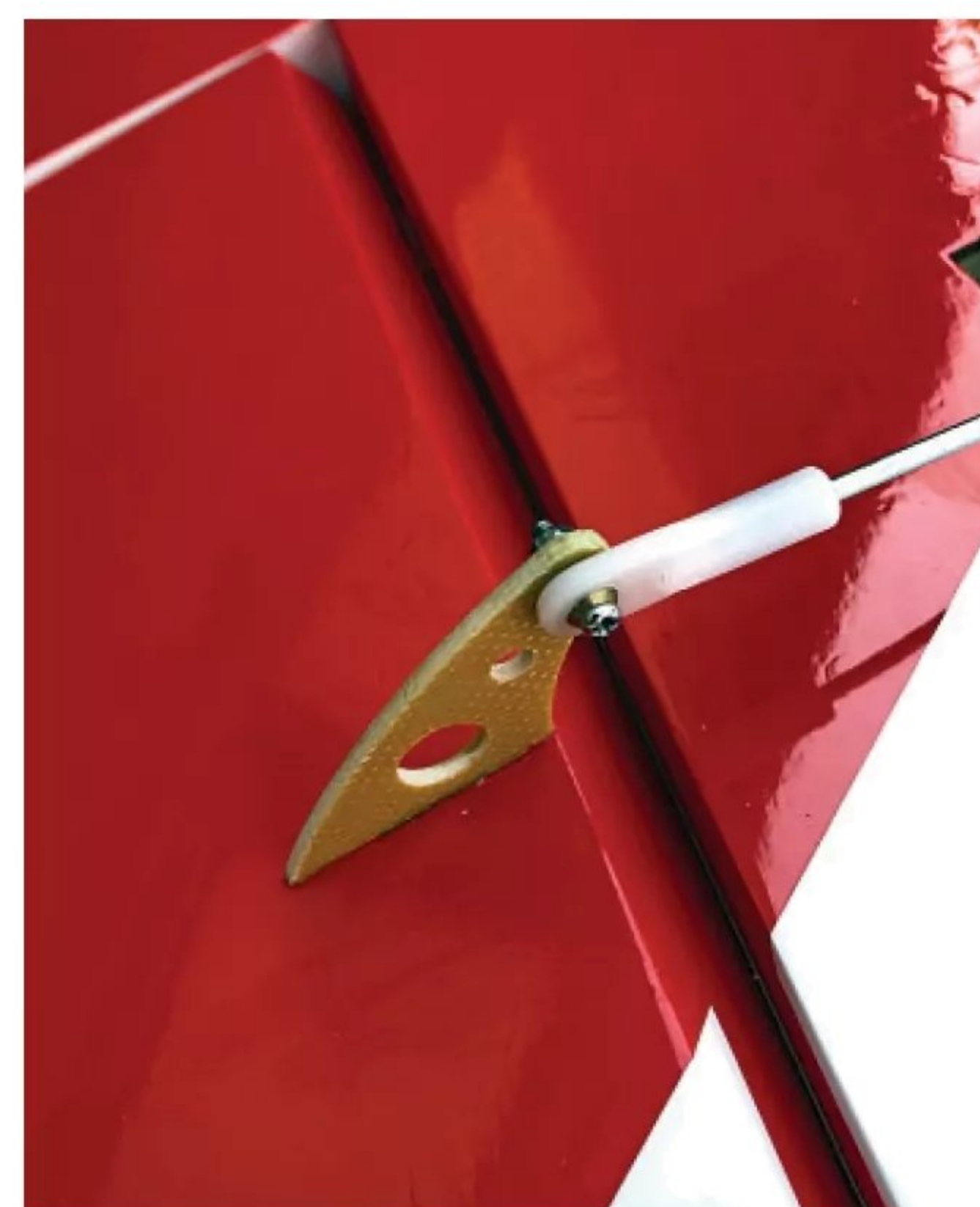
One of the aileron horns fitted neatly in its slot in a control surface.
