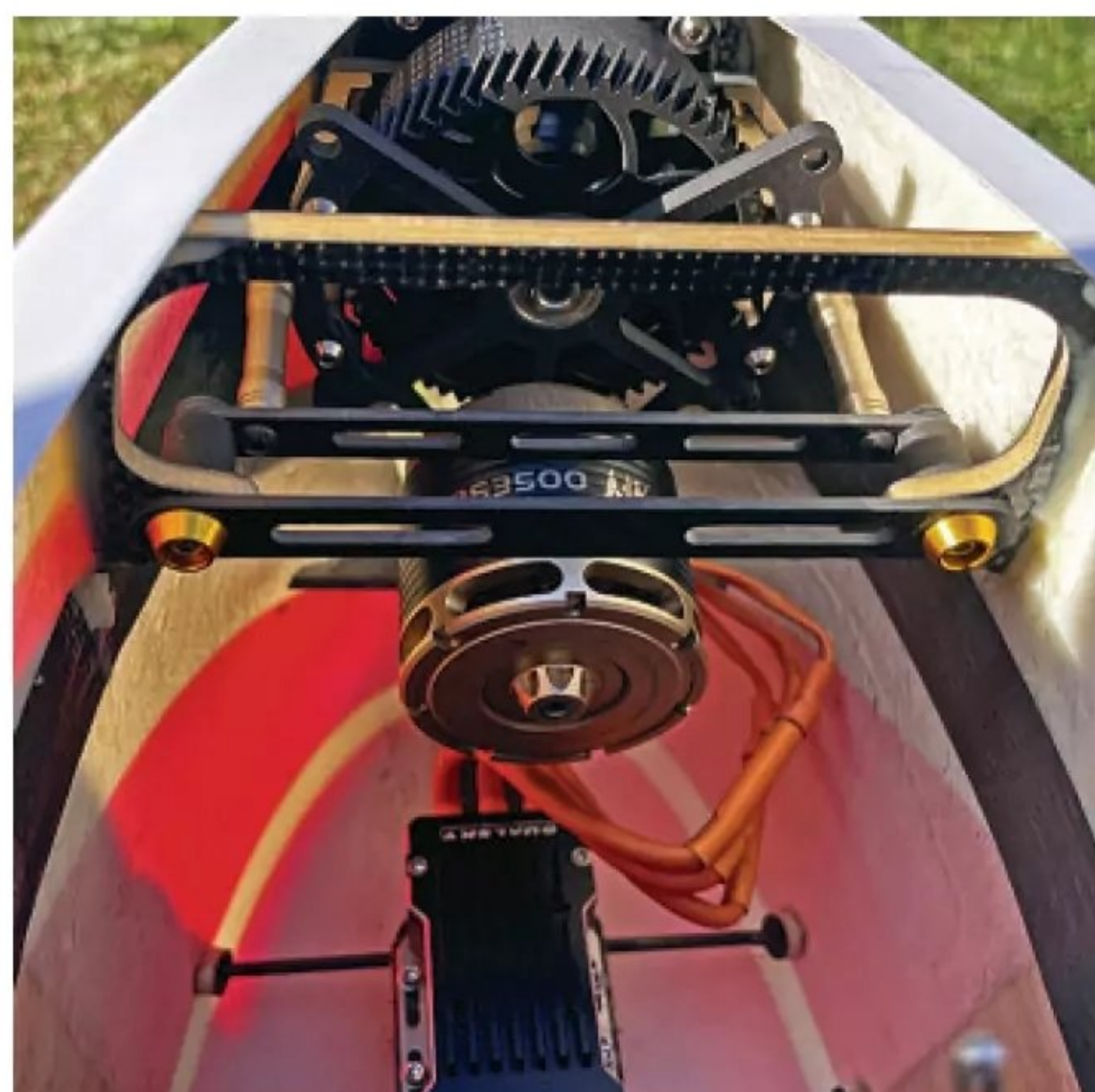
Interior of the Muscle Cloud showing the Dualsky CRS 3500 contra drive installation.
