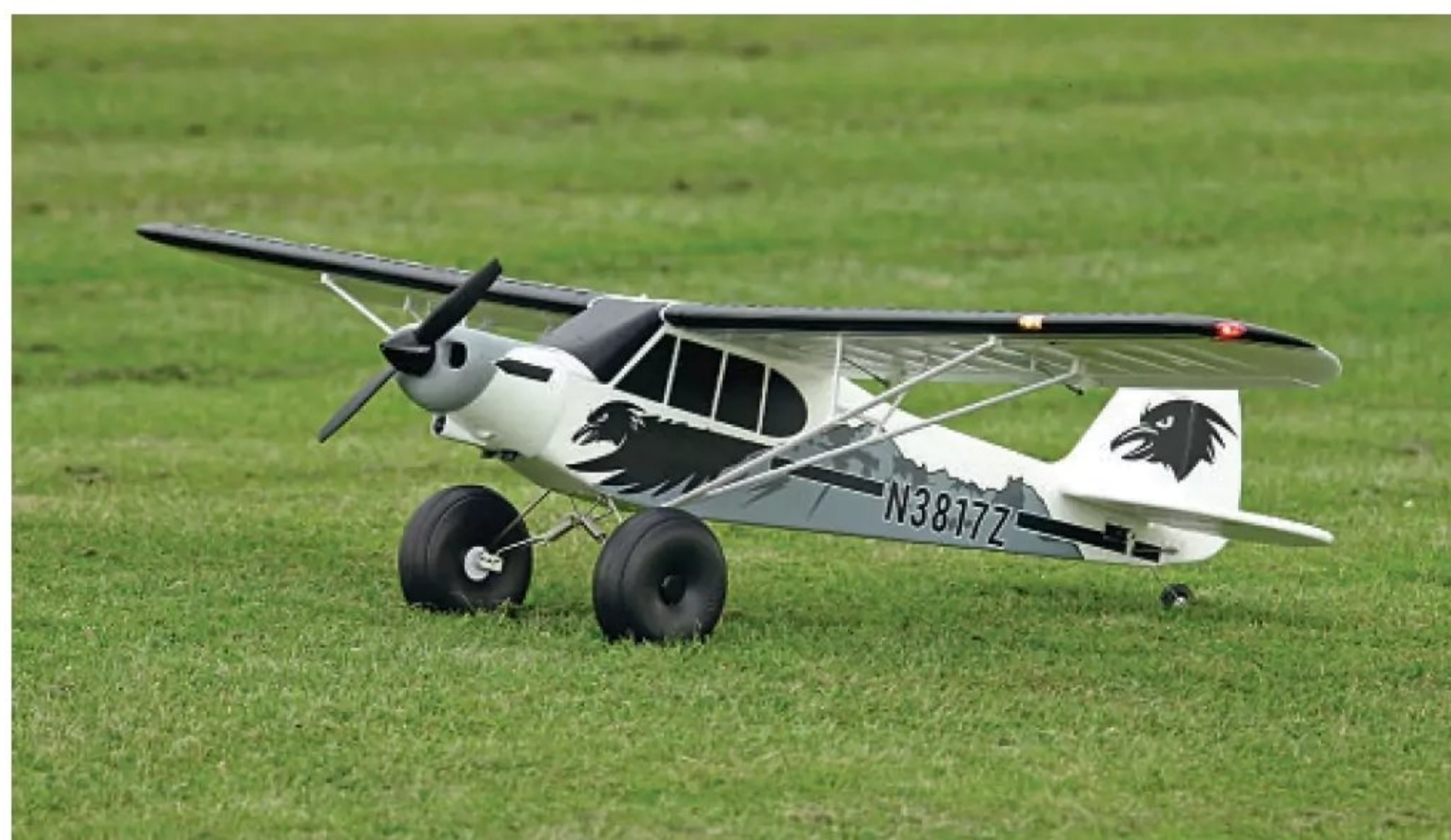
The ideal trainer should be as big as you can fit in your car and be fitted with a robust undercarriage with wheels as big as is practical.
