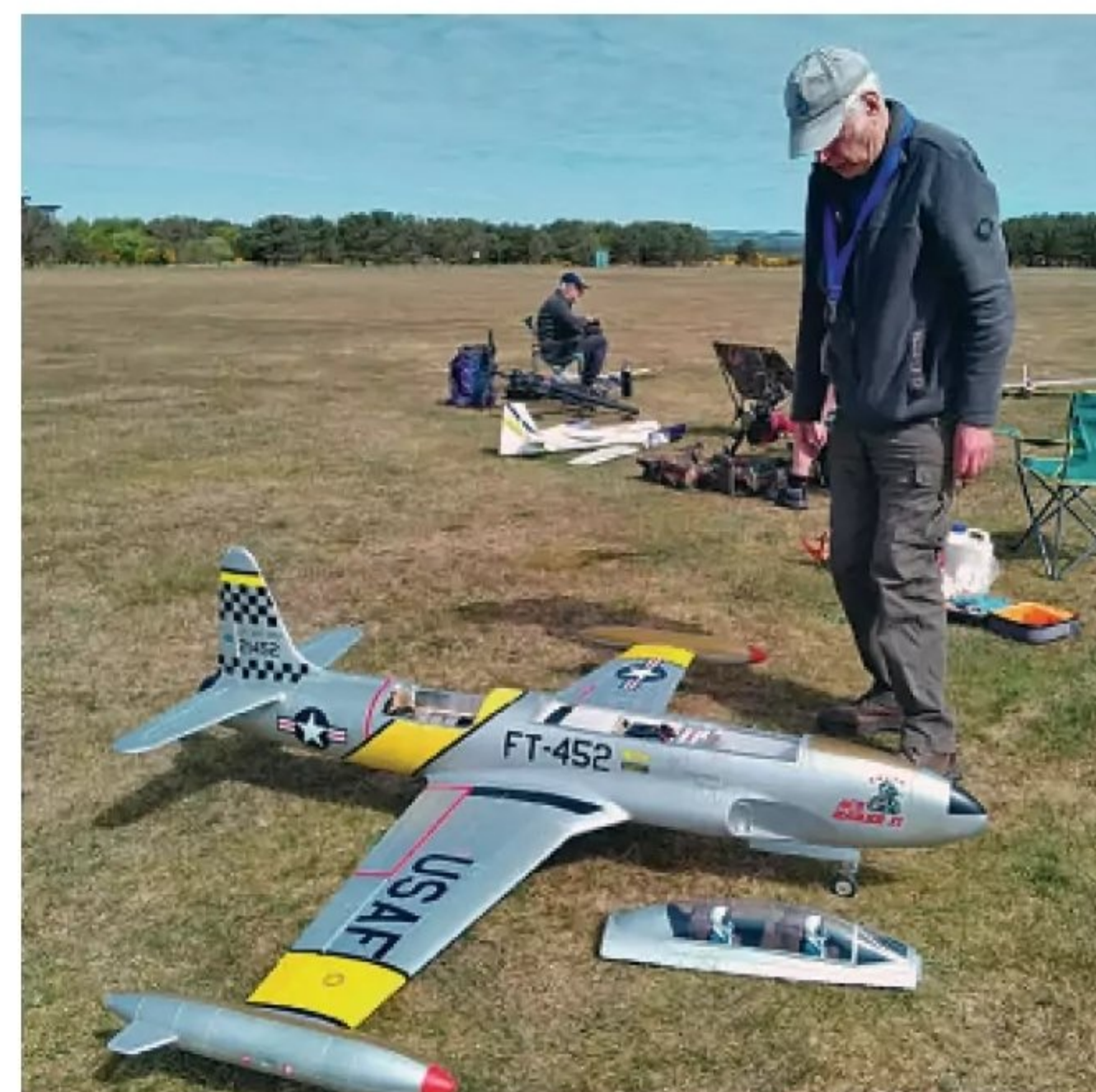
Here's Dave Socha with his turbine powered T-33. The Shooting Star is by HSD Jets using Futaba S-bus radio. Turbine is a Swiwin 60 converted from brushed starter to brushless at the factory - bit different from Graham's old Jetex 50!
