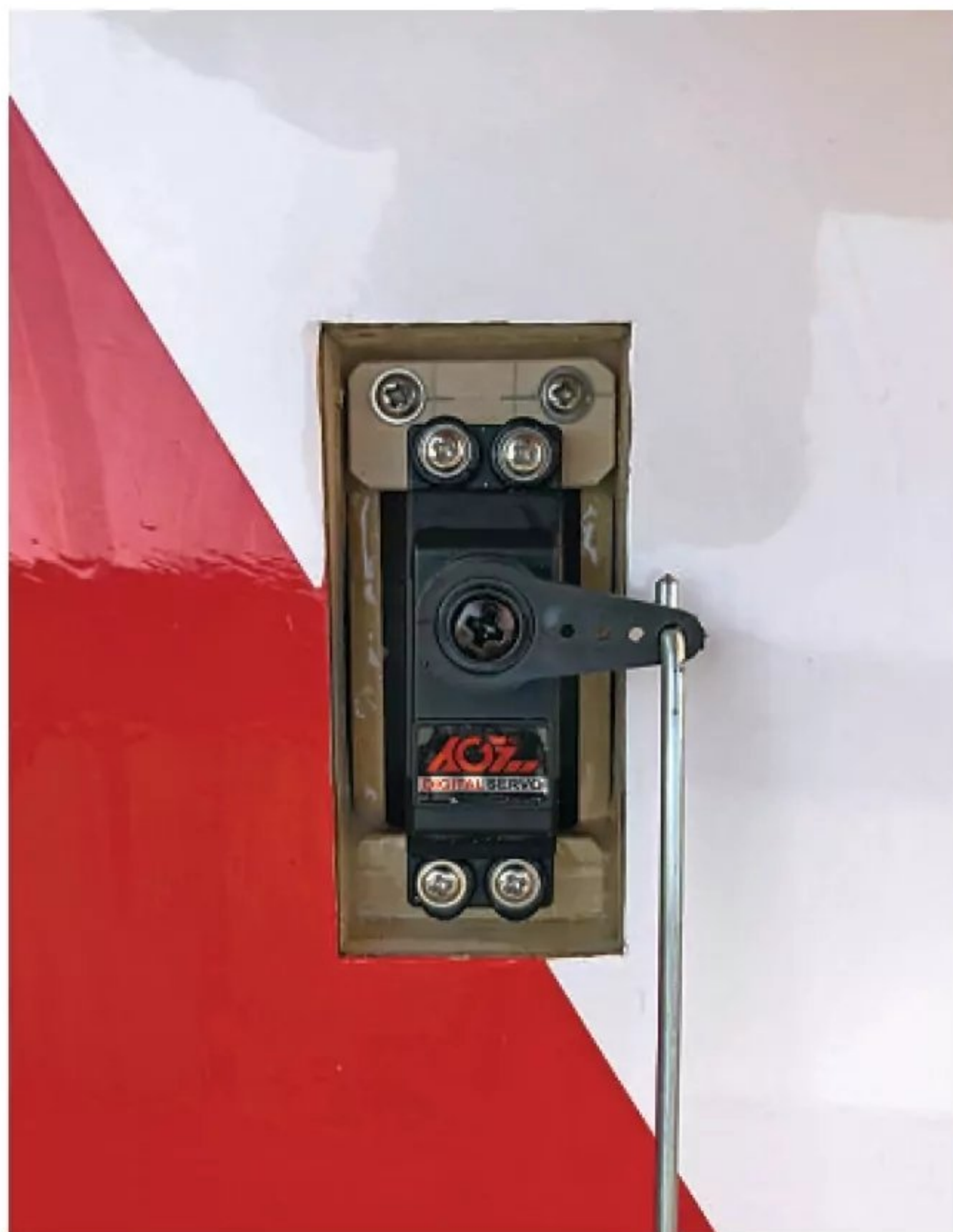
Final aileron servo installation showing the extra mounting plates. A side benefit is that a notch is not required to make way for the cable when inserting the servo.
