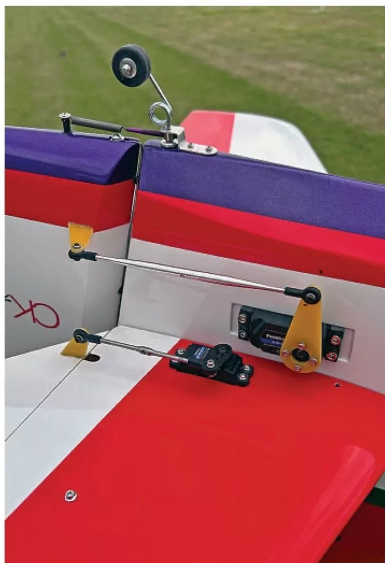
Tail group installation is entirely conventional on the Skywalker.
