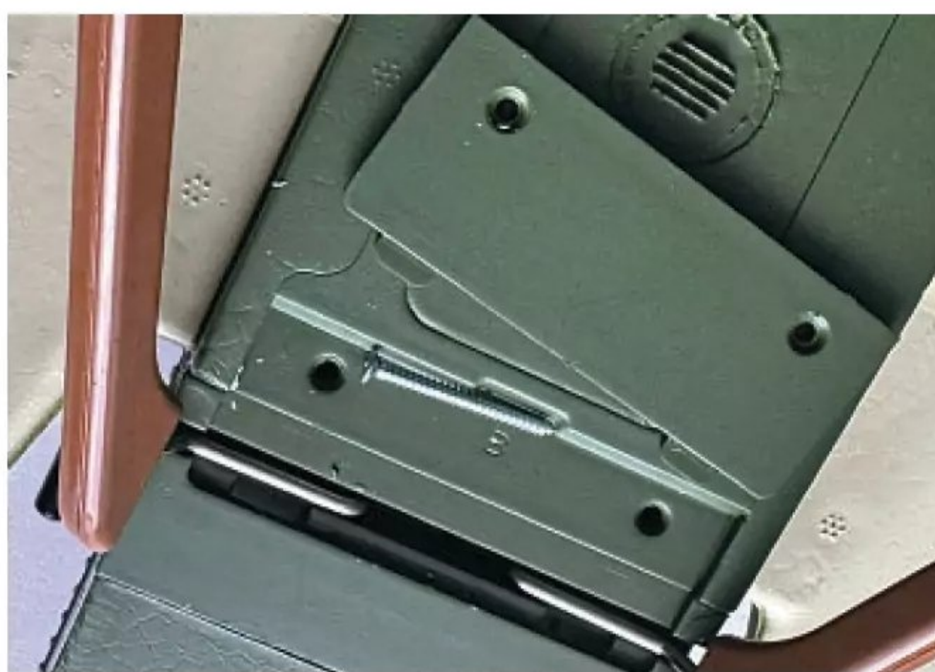
Lower wing and undercarriage are retained with a pair of screwed on plates.
