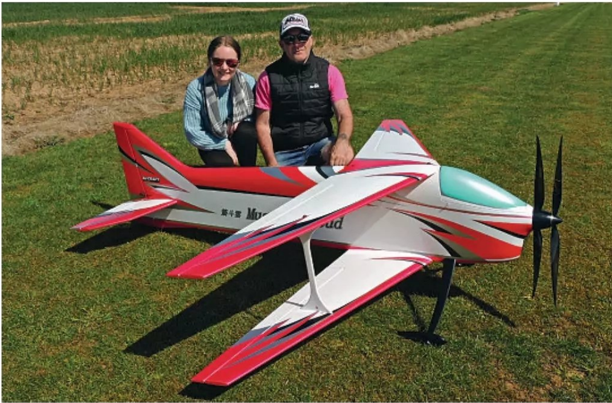
Peter Madden with helper Yazz flew this Muscle Cloud biplane kitted by BJ Craft. Huge 24" propellers are now becoming the norm driven by the Dualsky CRS3500 contra drive system.
