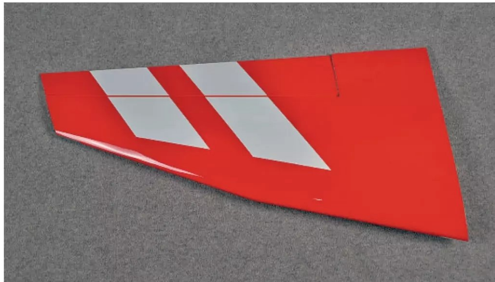
One of the Epilogue 1900's immaculate wing panels. Of all wood construction, with sheet balsa skins, the servo well awaits cutting out.
