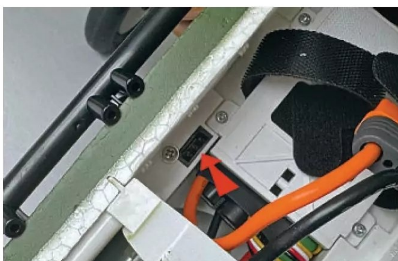
There's a bind plug socket mounted behind the motor in the battery bay.
