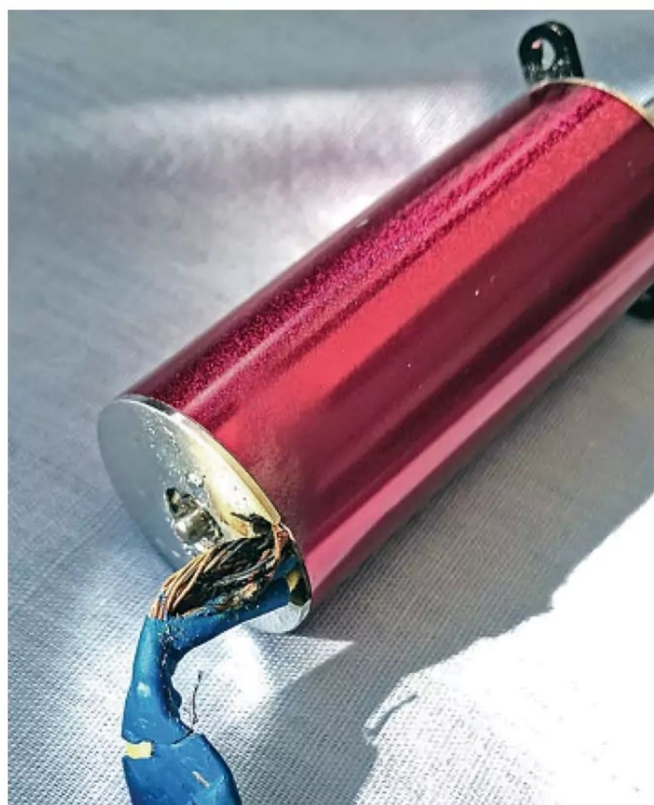
The cause of my KK 'Topper' x 2 crash. A sudden internal short and blowout through the motor end cap. Note the solder spatter and burn deposition.
