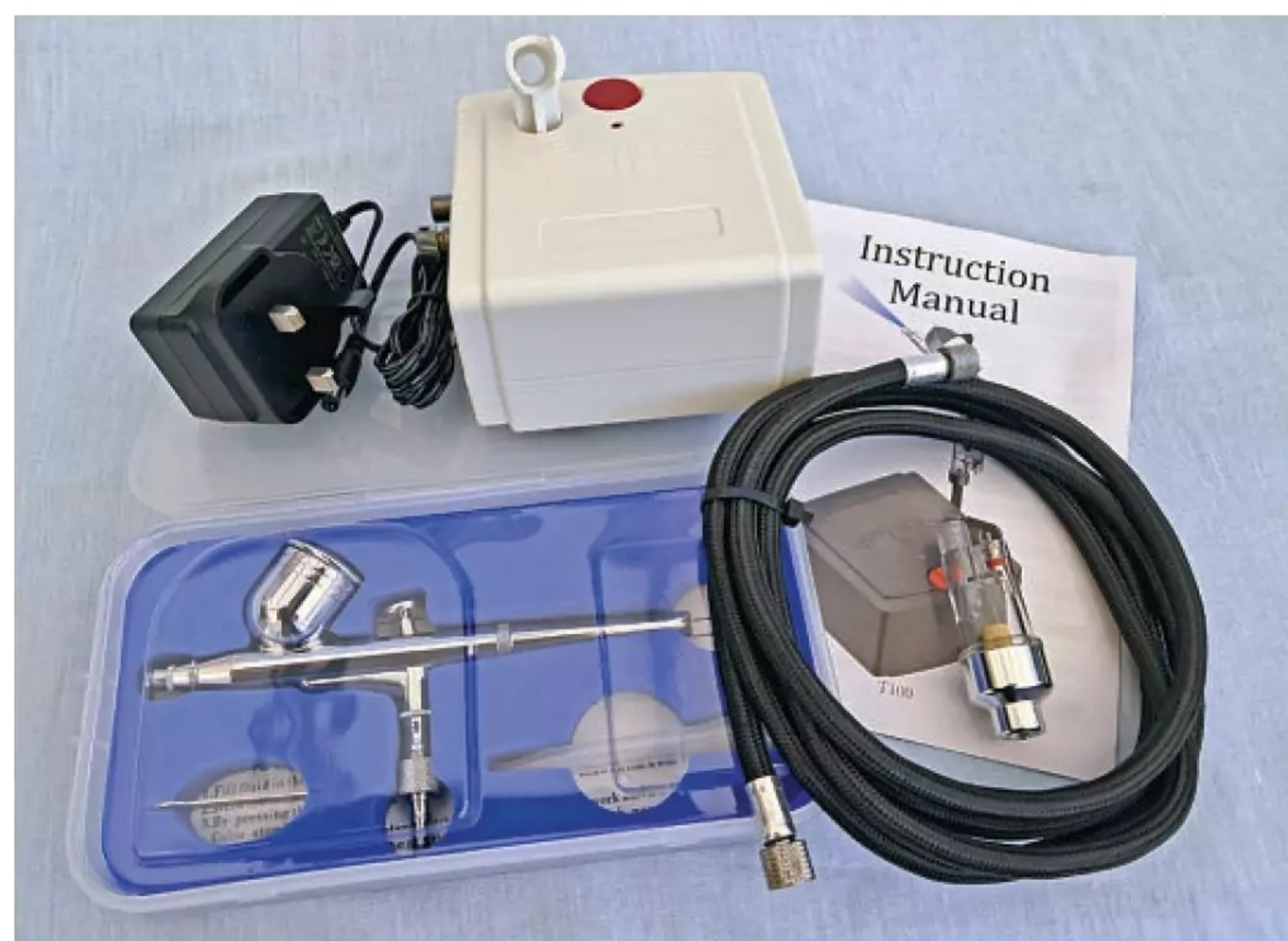
My cheapo new airbrush set. The white box is the neat and adequate compressor and the small unit within the flexible hose loop is the moisture trap.
