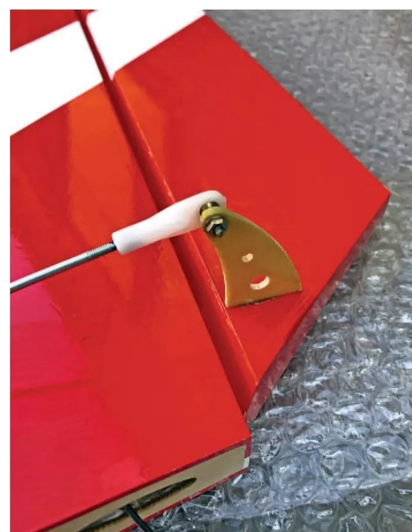
And here's one of the elevator horns. Slotted-in horns work really well but be sure to rough up the tabs at their base to give a firm grip for the adhesive used.
