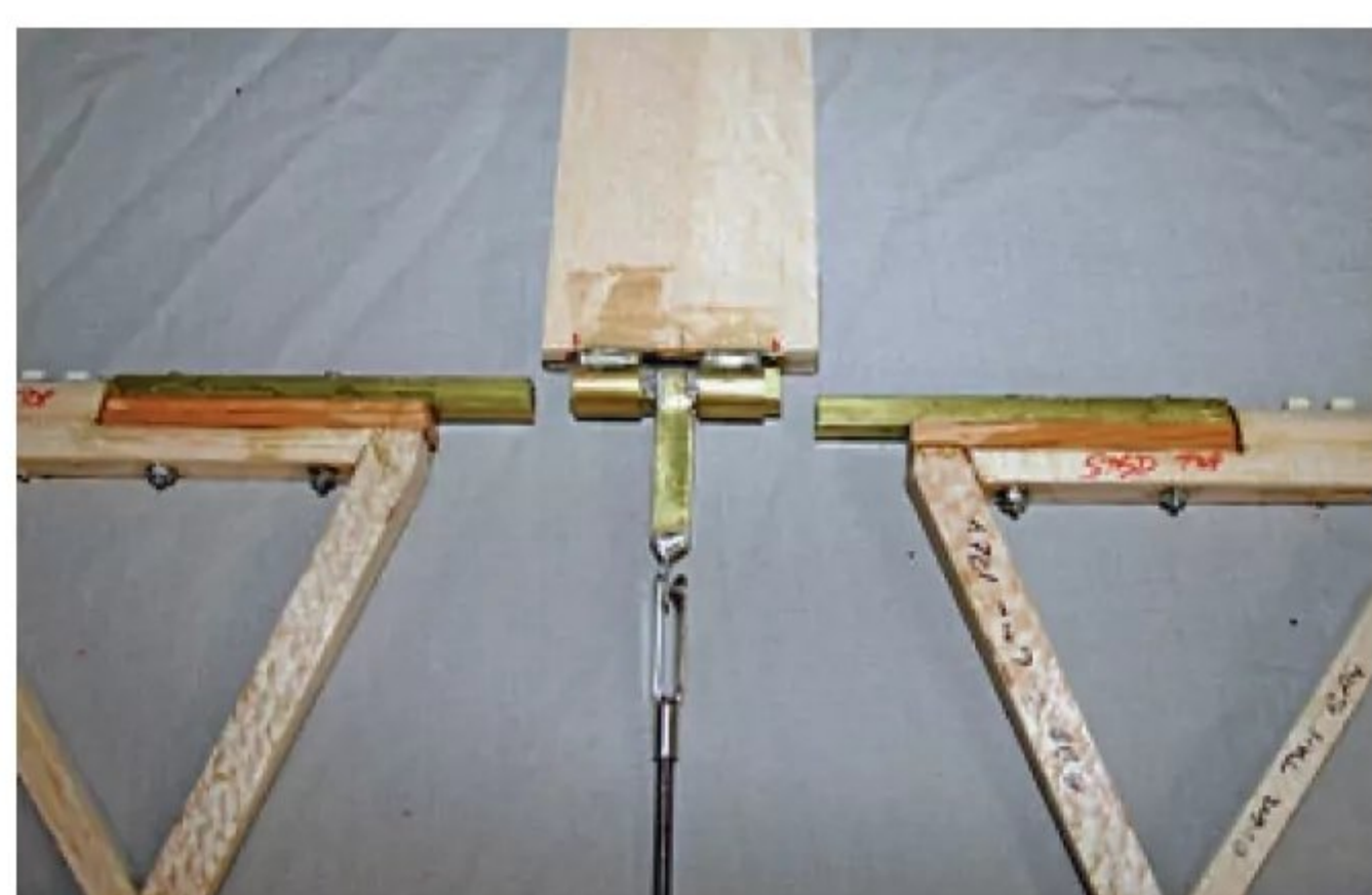
Elevator connections to the central operating lever.
