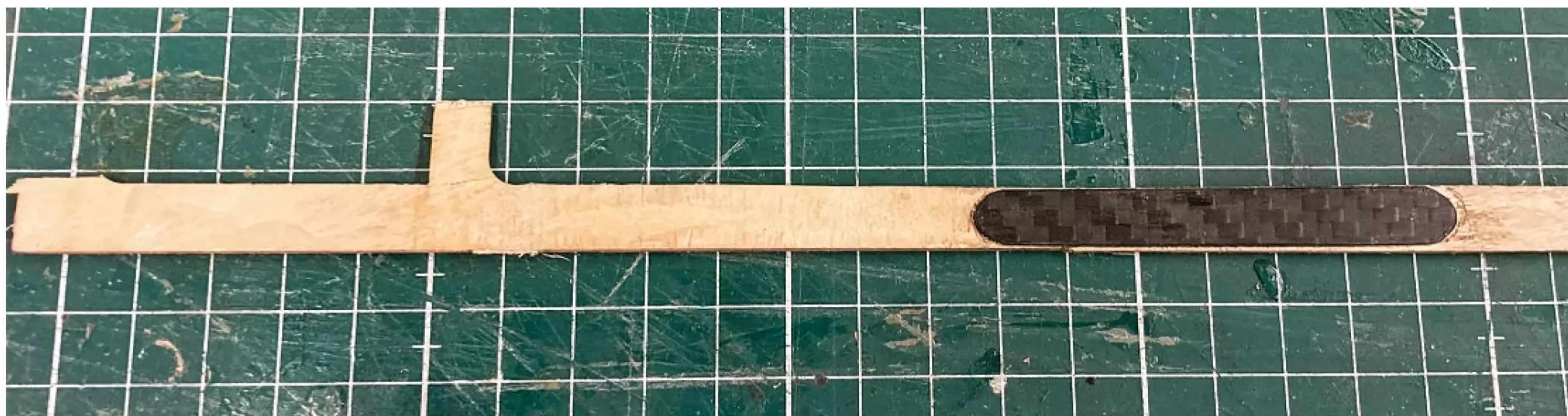
First, the doubler was repaired by splicing it and reinforcing the joint with a strip of thin carbon sheet, glued with slow-curing epoxy. Note the rounded ends of the carbon to ensure a gradual distribution of forces acting on this part. It was then glued back in place.
