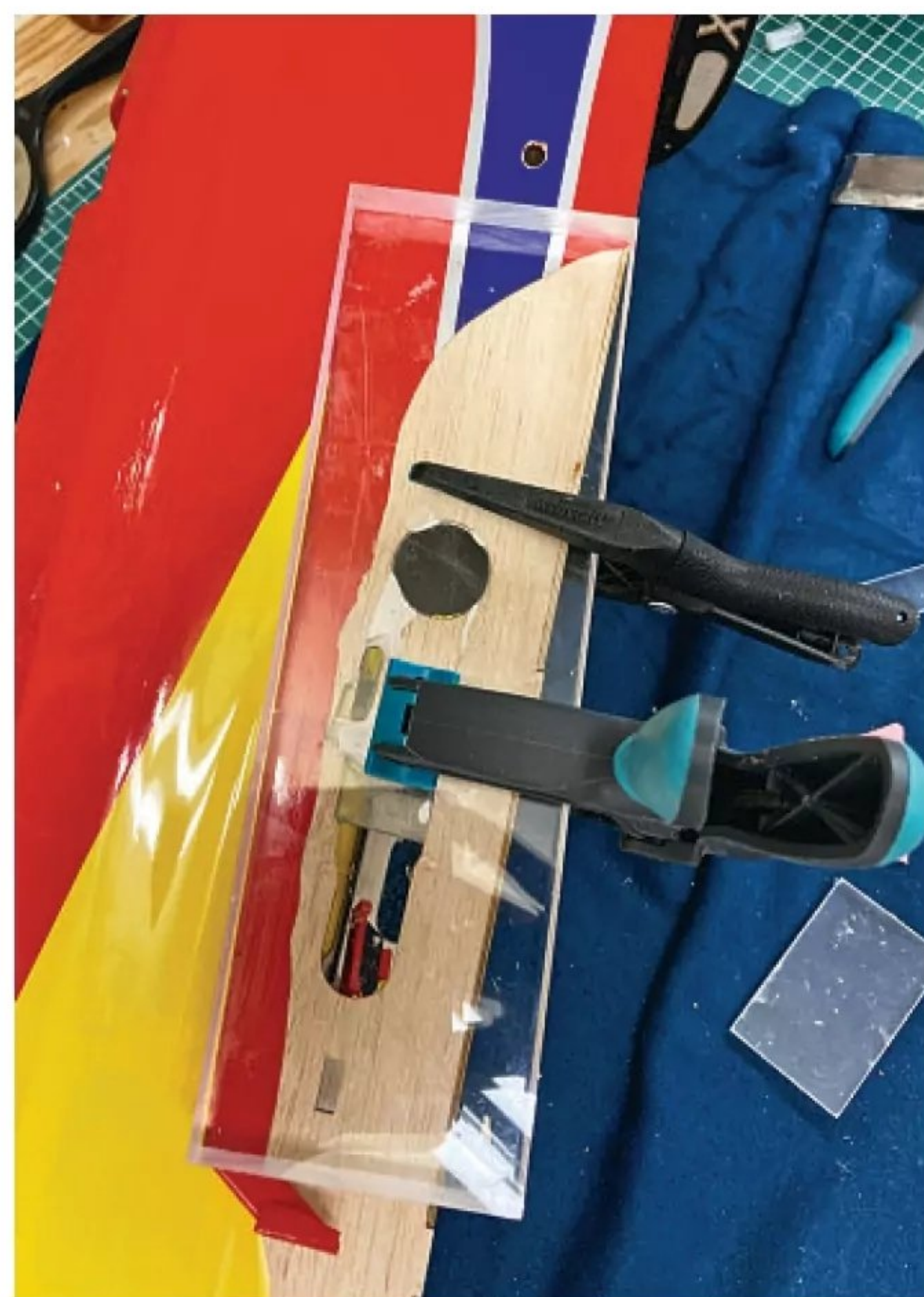
As the wing had taken most of the impact the port fuselage only suffered minor damage. After carefully removing as little of the covering as possible the sides were glued back using PVA and a piece of thick acetate (Plexiglas) on each side of the repair, acting as a jig. To enable the water to evaporate from the PVA leave it in place for at least 24 hours.
