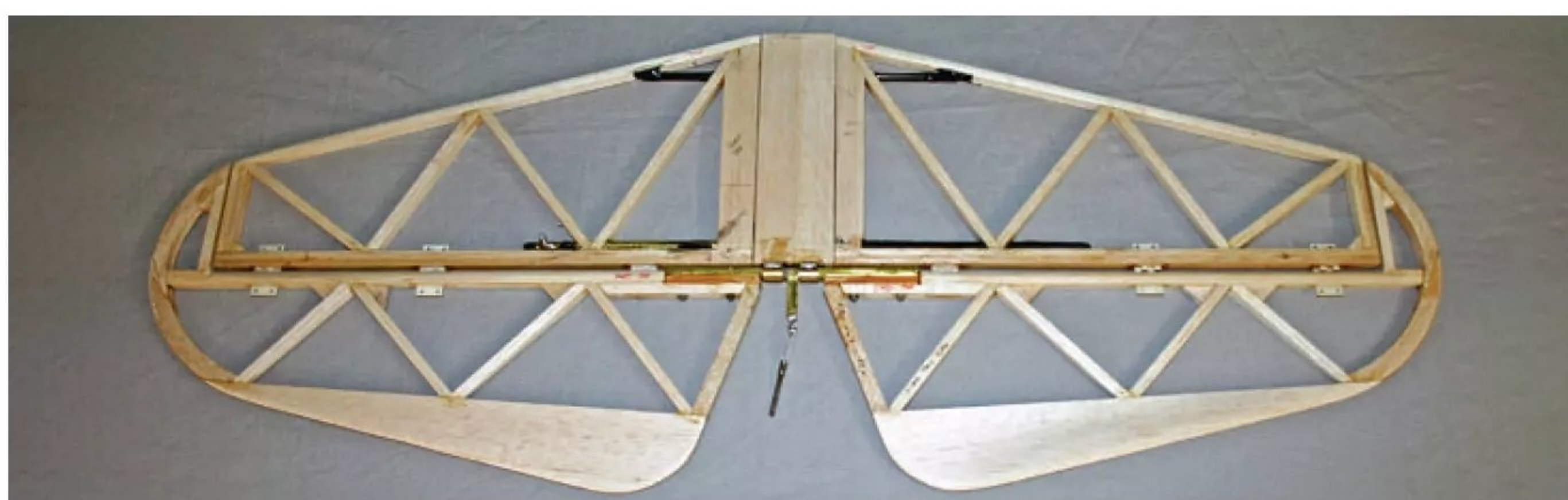
Tailplane fully assembled.
