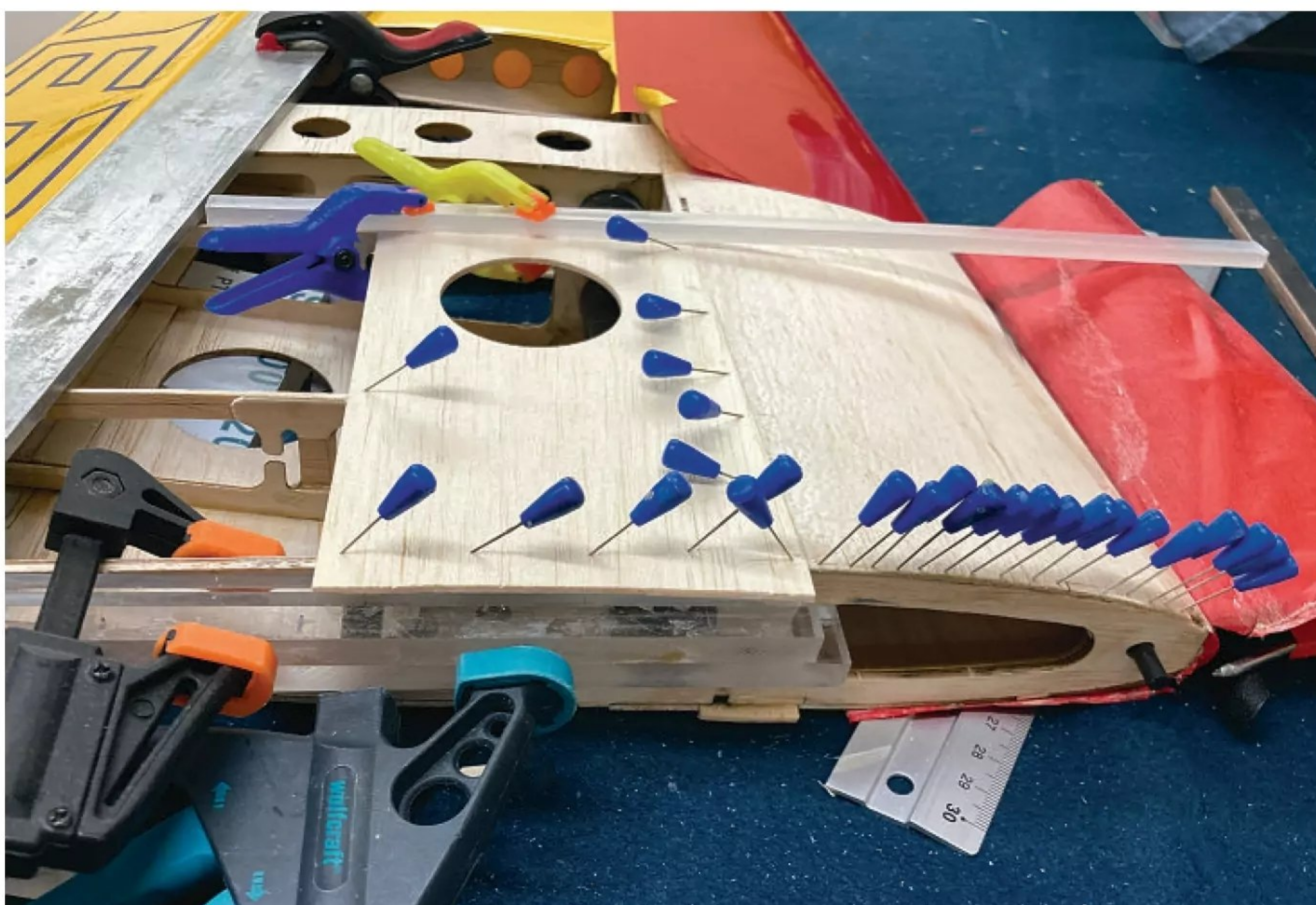
New sheeting was applied using slow-setting PVA and plenty of pins.
