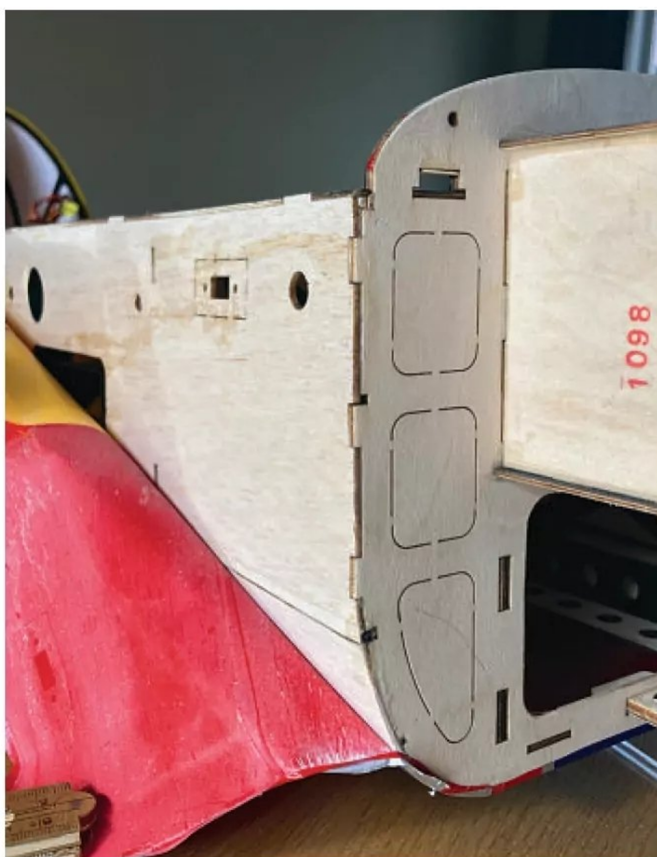
At first sight the starboard side of the fuselage did not seem to have suffered much. But removing the covering showed several cracks. These can be fixed with sparingly applied thin cyano and sanded smooth afterwards. Here as well, do not be tempted to 'strengthen' the area of repair.
