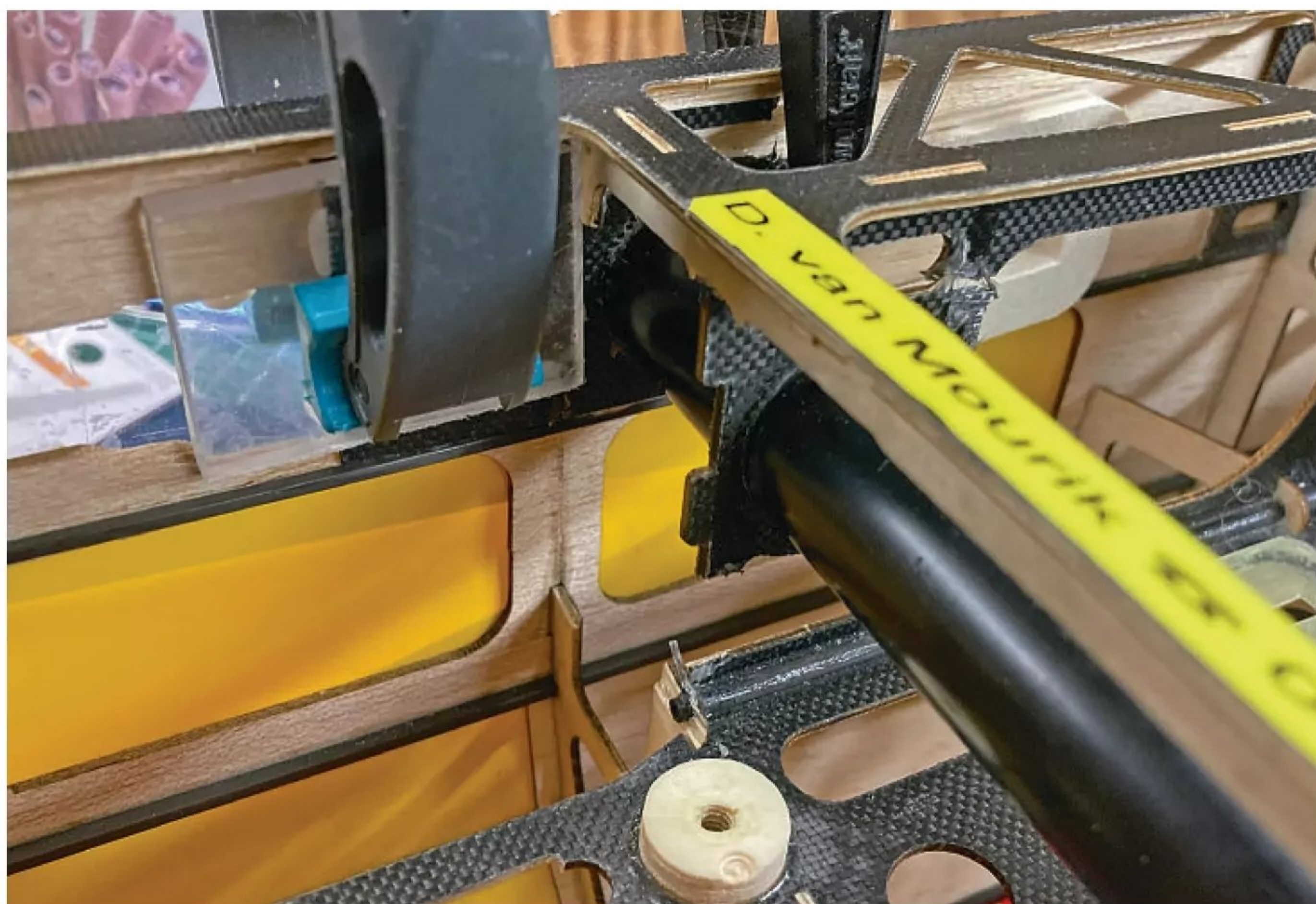
As the wing had taken most of the impact the port fuselage only suffered minor damage. After carefully removing as little of the covering as possible the sides were glued back using PVA and a piece of thick acetate (Plexiglas) on each side of the repair, acting as a jig. To enable the water to evaporate from the PVA leave it in place for at least 24 hours.
