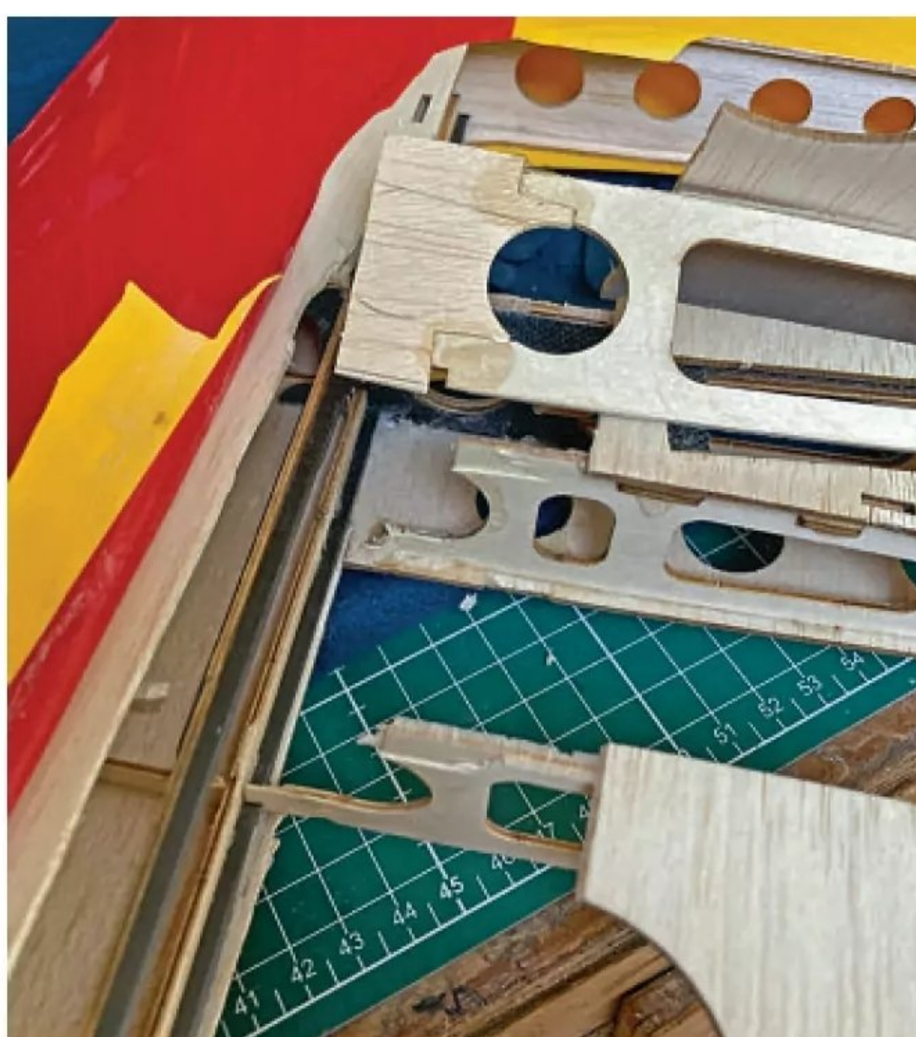
As only the front part of the ribs, where they hold the wing tube were damaged, there was no need to replace entire ribs. Simply add a new front piece and all will be fine. In this case, the cut out for the wing tube was undamaged. If you need to make adjustments it makes sense to enlarge the circular cut out for the wing tube slightly (about half a millimetre or around 1/64" larger than the required diameter) and use a thin plywood washer to secure the tube to the wing ribs.
