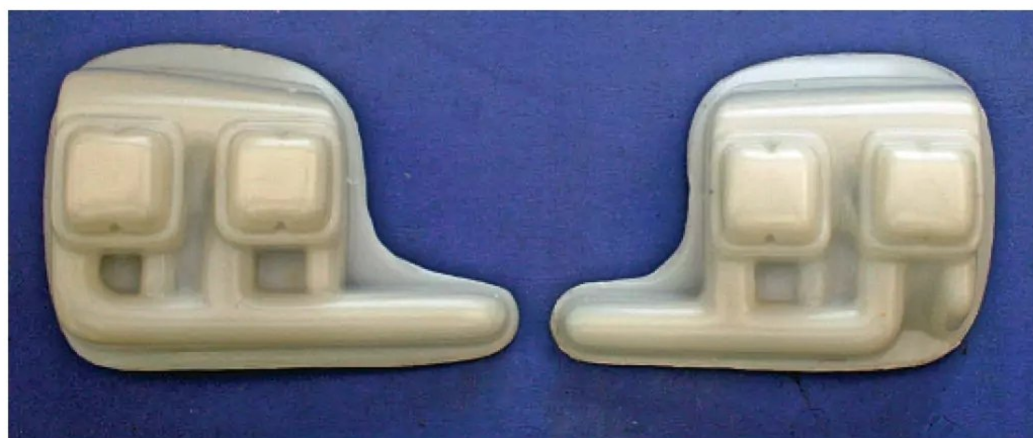
Cylinder head mouldings after trimming.
