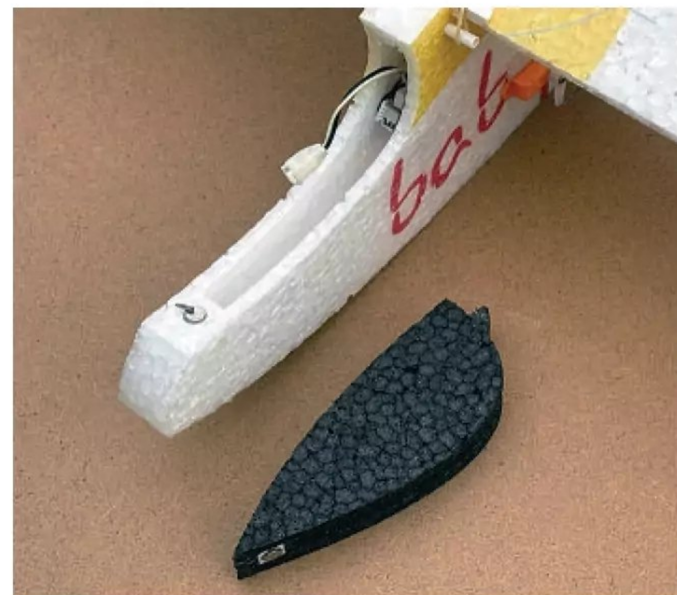
Micro-Rx is in the rear of the cockpit space. The rest is used for the 1S 380 mAh LiPo.
