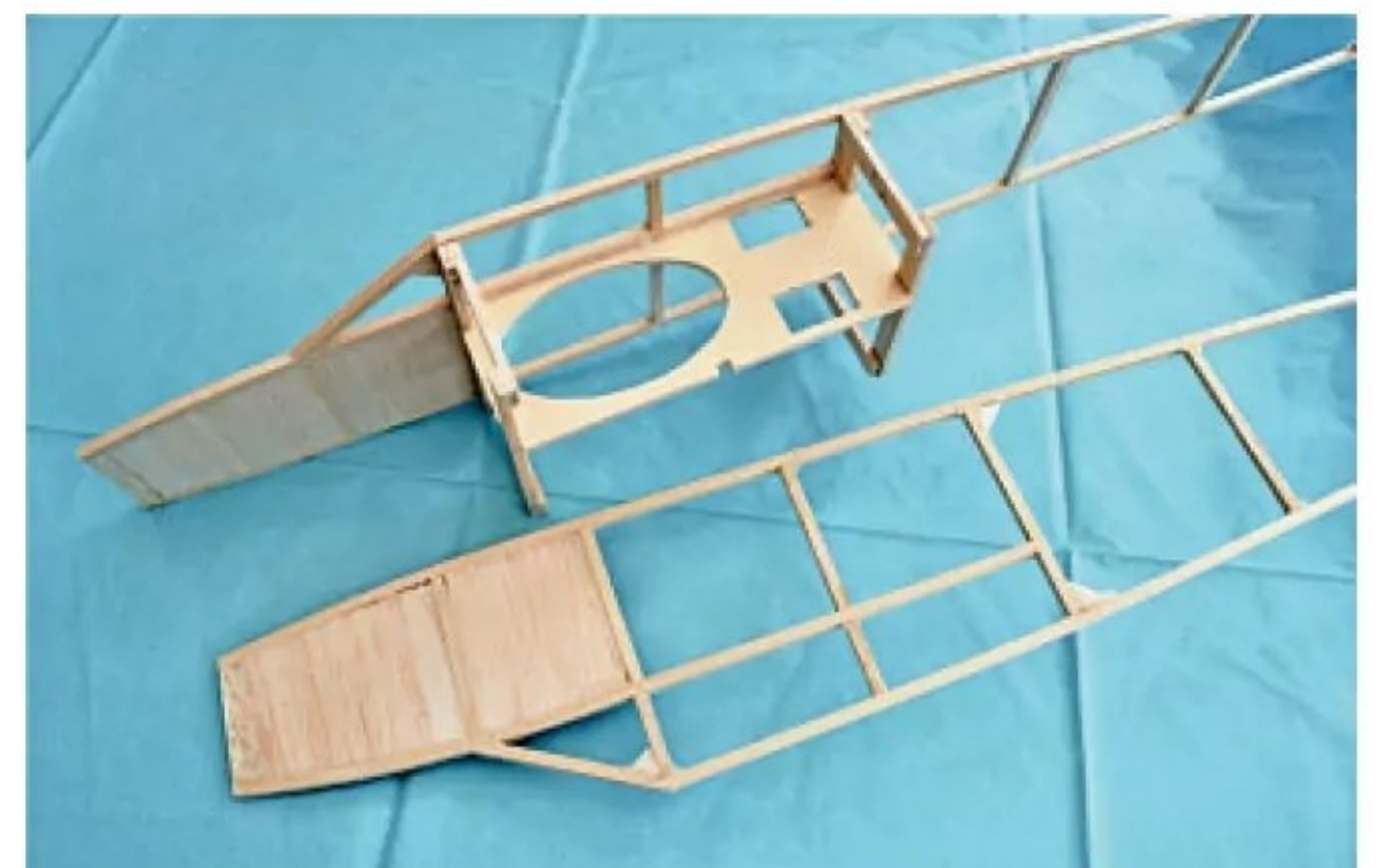
The two fuselage formers and servo tray act as a jig to keep the sides square during assembly.
