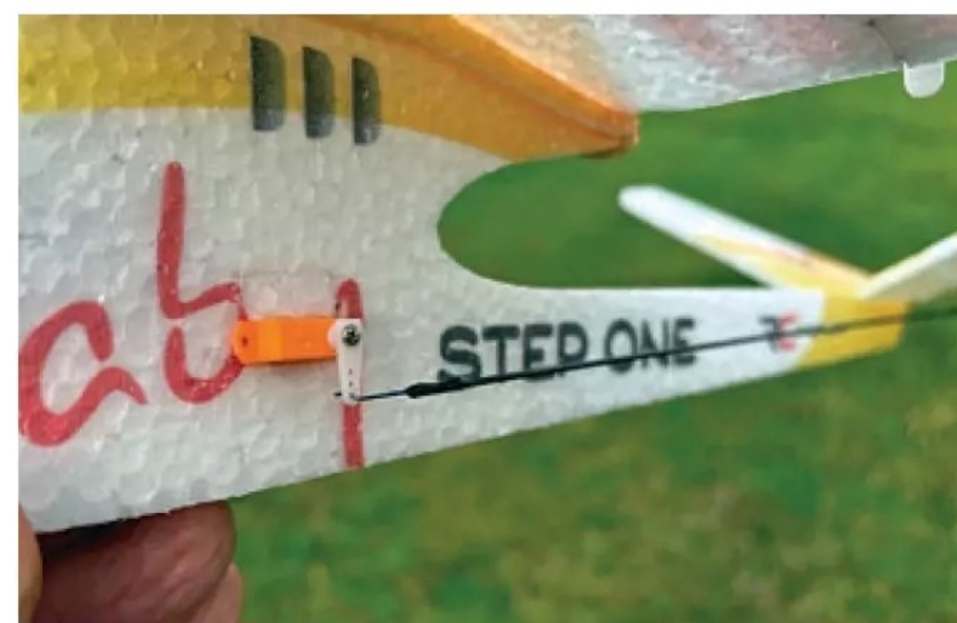
My adaptation showing one of the two 1.7g servos. I used pushrods to operate V-tailerons rather than the intended proportional motor system.
