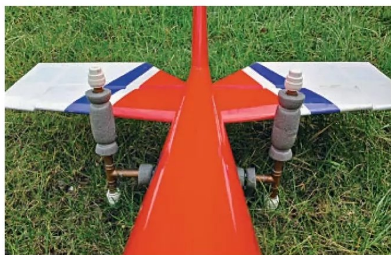
A reliable model restraint can be easily made up using plumbing pipes and fittings. Pipe lagging protects the tail surfaces of the model.
