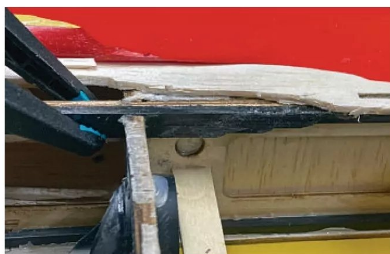
The split carbon spar was soaked with thin cyano and after this had set the spar was carefully sanded. Always wear PPE as carbon dust is unpleasant stuff! Next, three layers of 2 x 4 mm carbon were added with epoxy and the lot clamped to the already repaired plywood doubler, using thickened epoxy resin. The chamfered shape of the reinforcement aids load distribution. After curing the result is a solid construction which will never break again in flight with only a marginal increase in weight.
