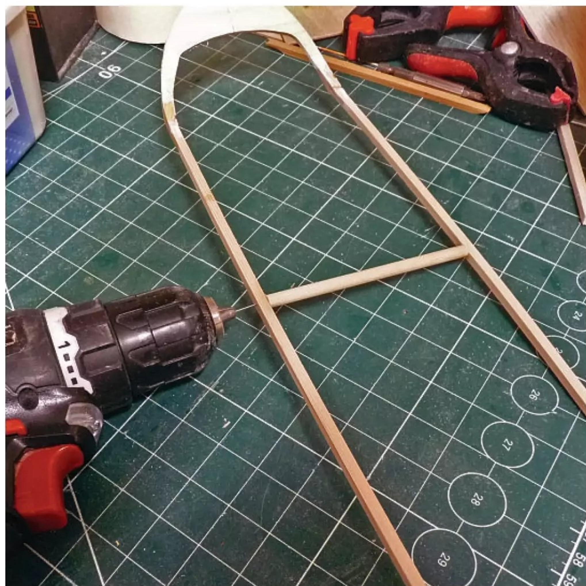
Withdrawing the drill slightly allows the pin to be knocked back flush after cutting.
