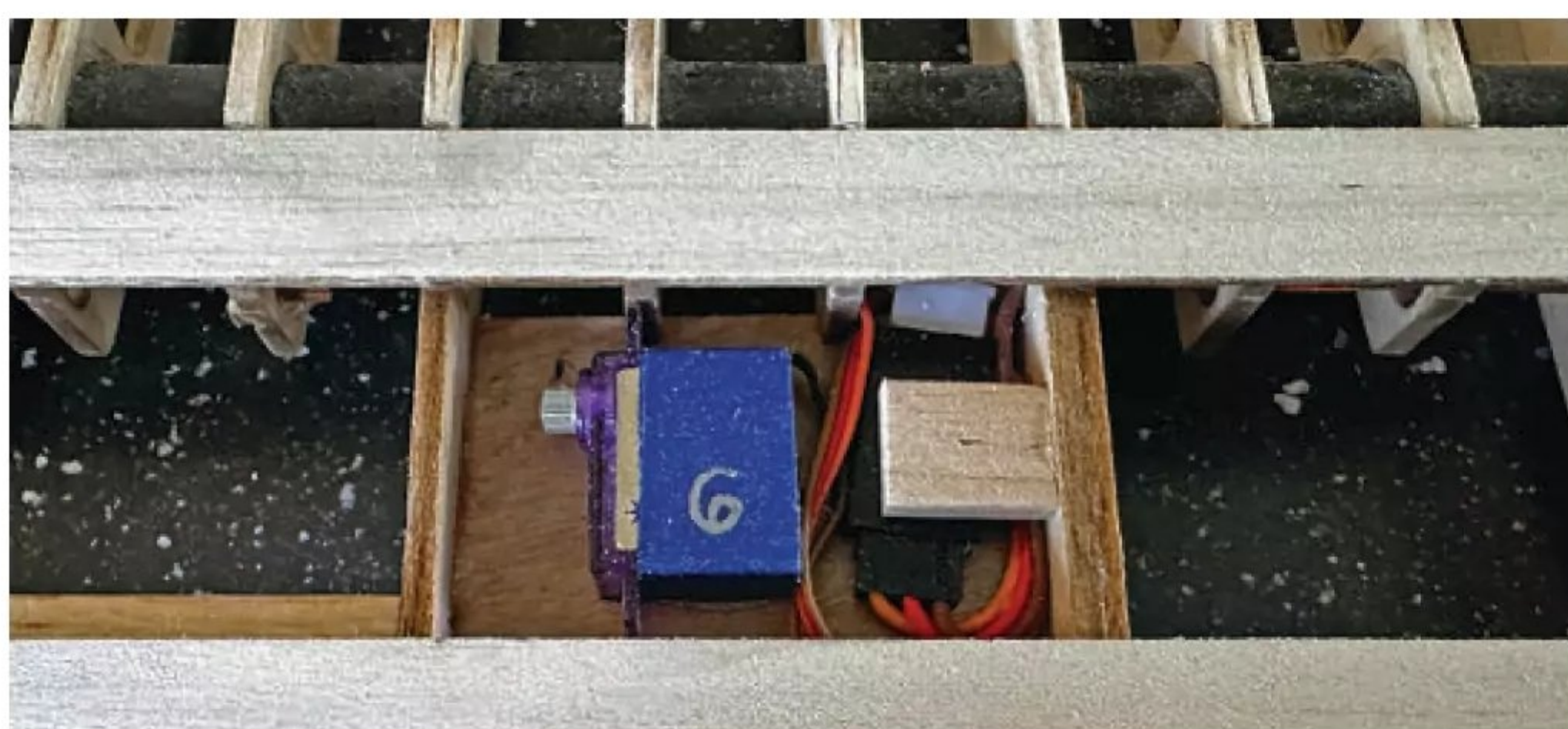
Wrapping the spoiler servo cases in masking tape allows for easy removal if they ever need to be replaced.
