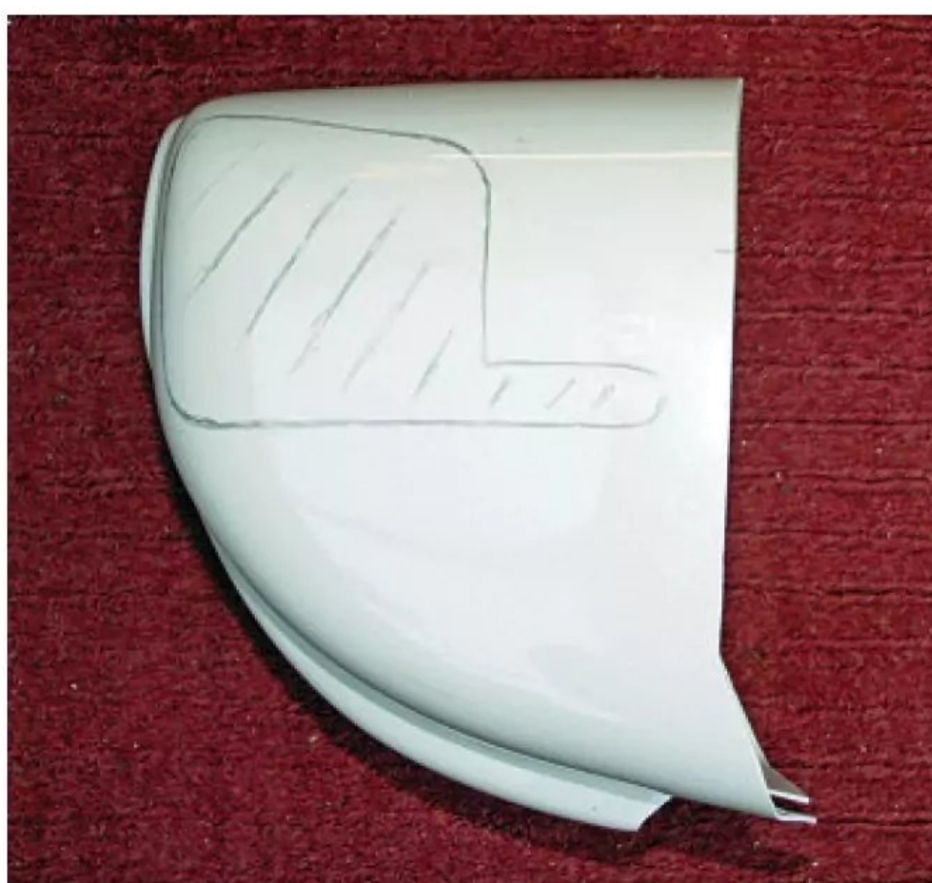
Resulting cut line on the cowl.
