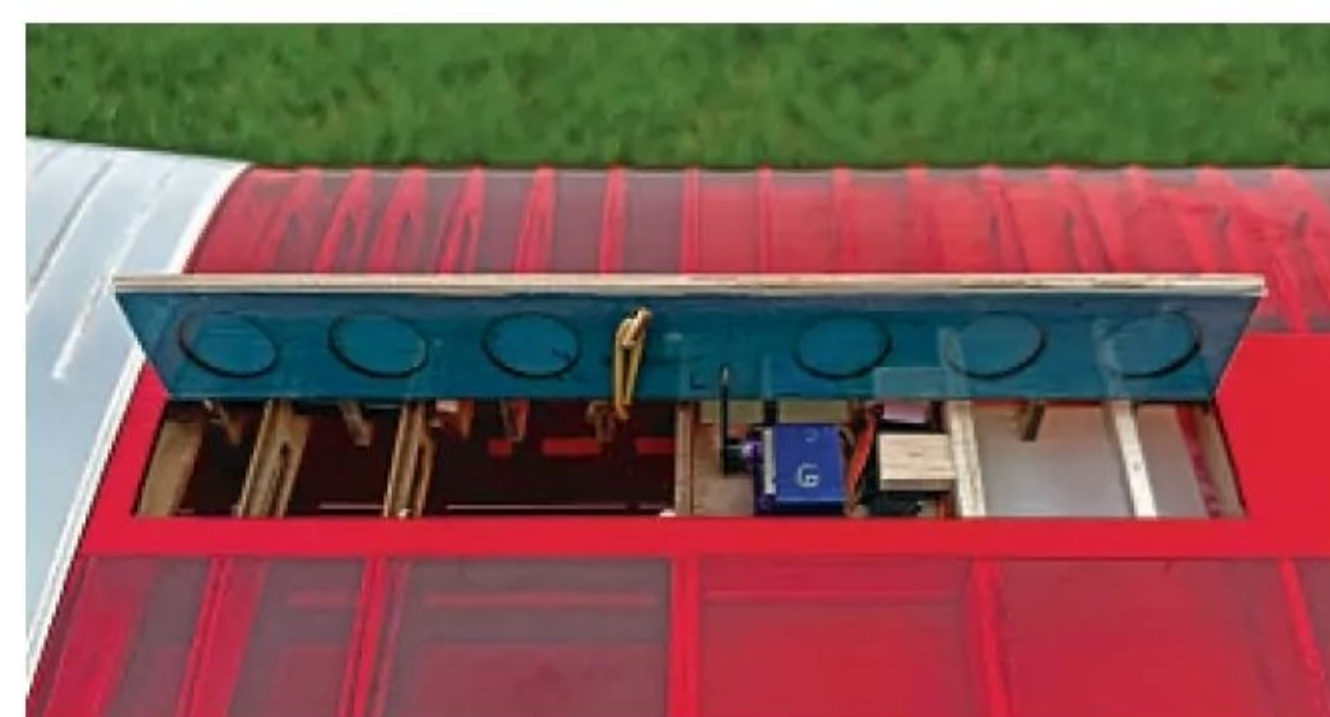
Spoiler detail showing the servo holding it fully extended. Note also the small rubber band that ensures that it snaps fully closed during climb and glide.
