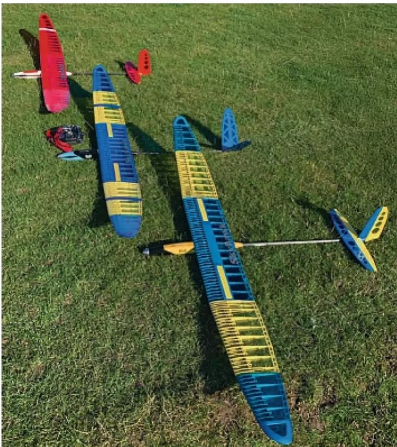
Steve's Skyhawk fleet showing the X-tail and V-tail (middle) options.
