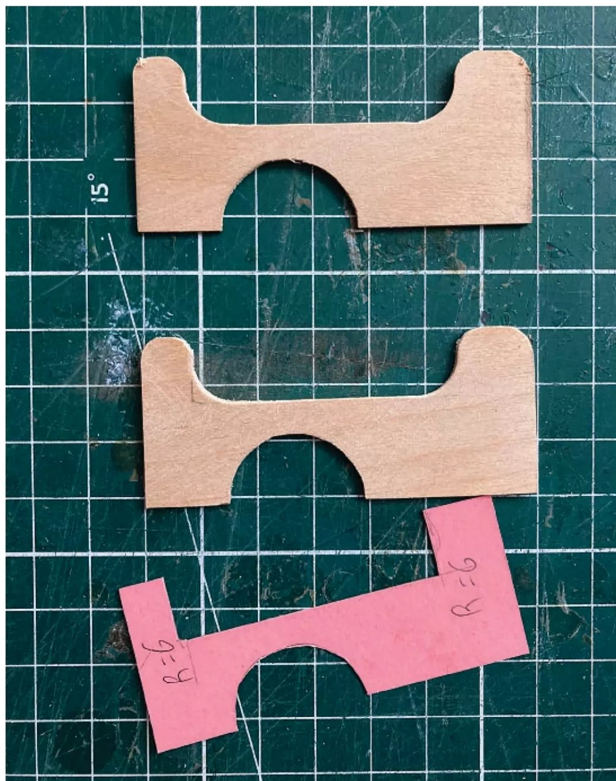
A simple template was made out of a piece of scrap cardboard. The new side plates were made from 1.5 mm (1/16") aircraft grade plywood. To enable gluing without too much surgery the new plate is split lengthwise. This image shows the rear halves of the former
