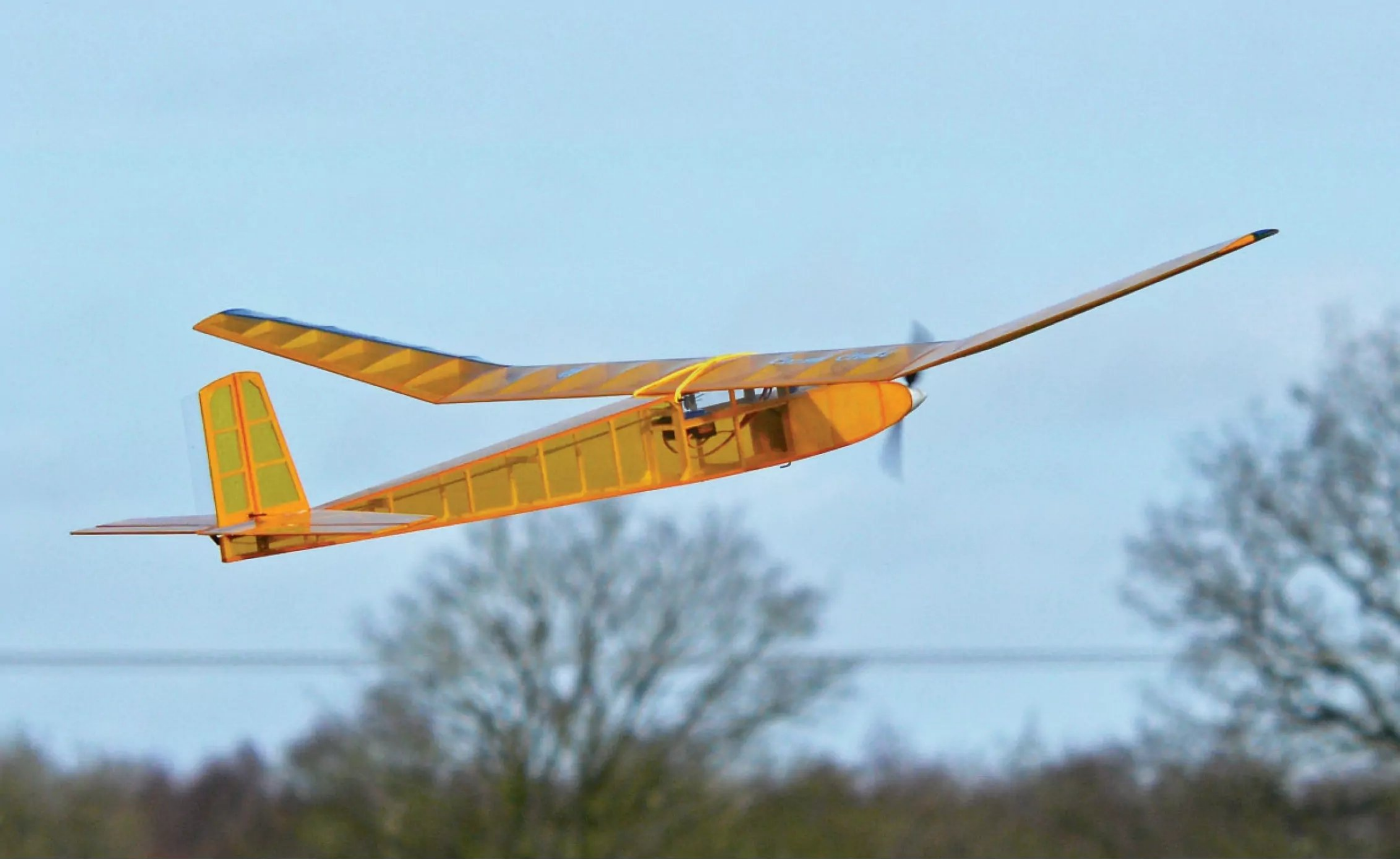
At the second test session a transparent rudder extension was attached to give more positive directional control.
