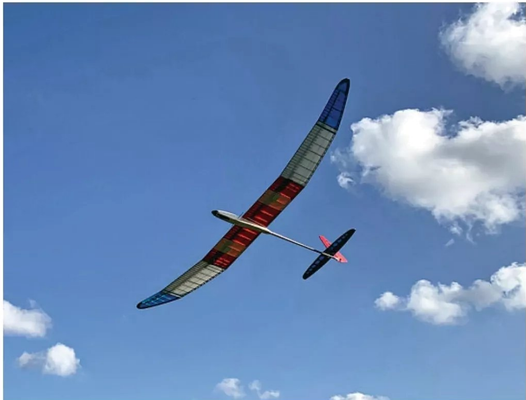
Alex started at a CG position at the forward end of the recommended range and then slowly moved it rearwards until the model behaved how he likes it.
