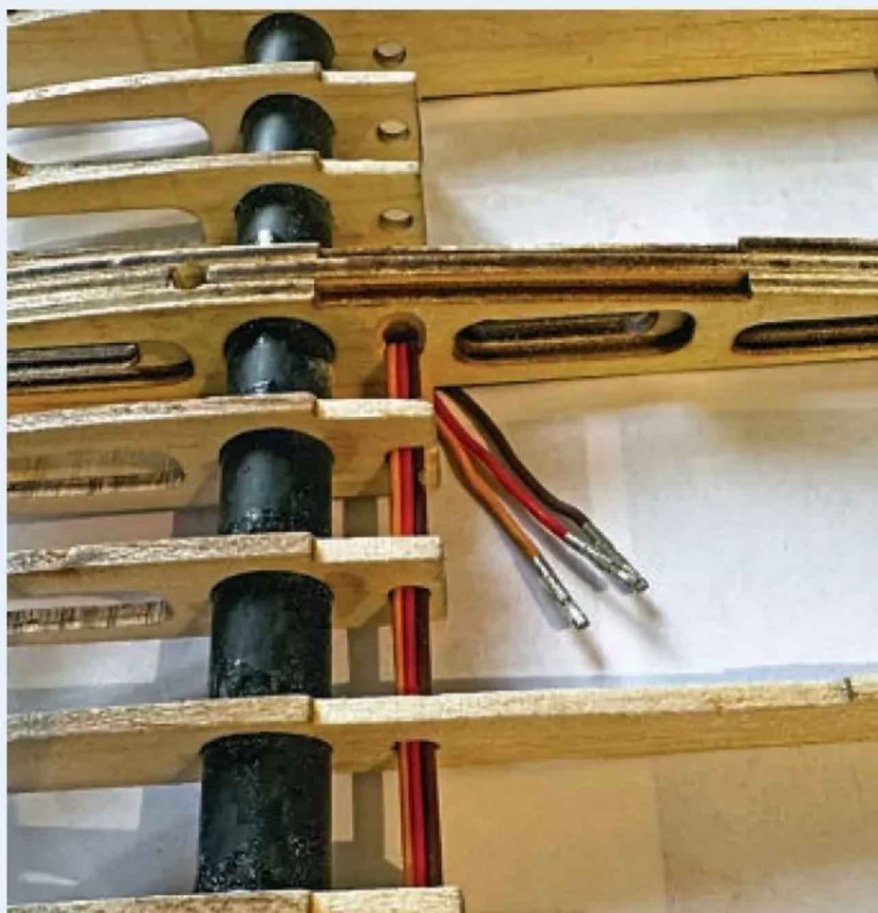
Spoiler servo plug casings are removed and the extension leads threaded through, leaving the crimps in place. The cases can be refitted afterwards, making sure to get the wires in the correct order.
