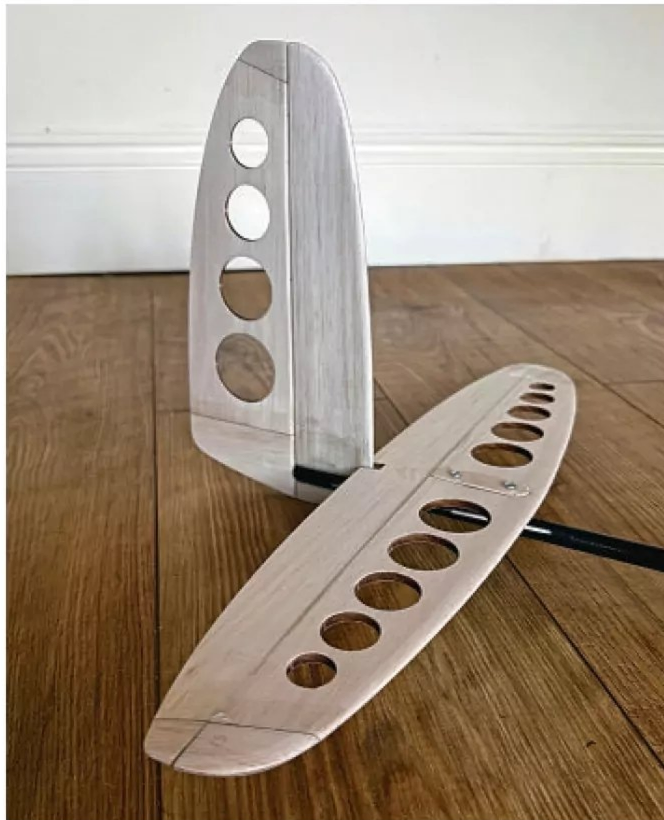
Finished cross-tail (aka X-tail) ready for covering.
