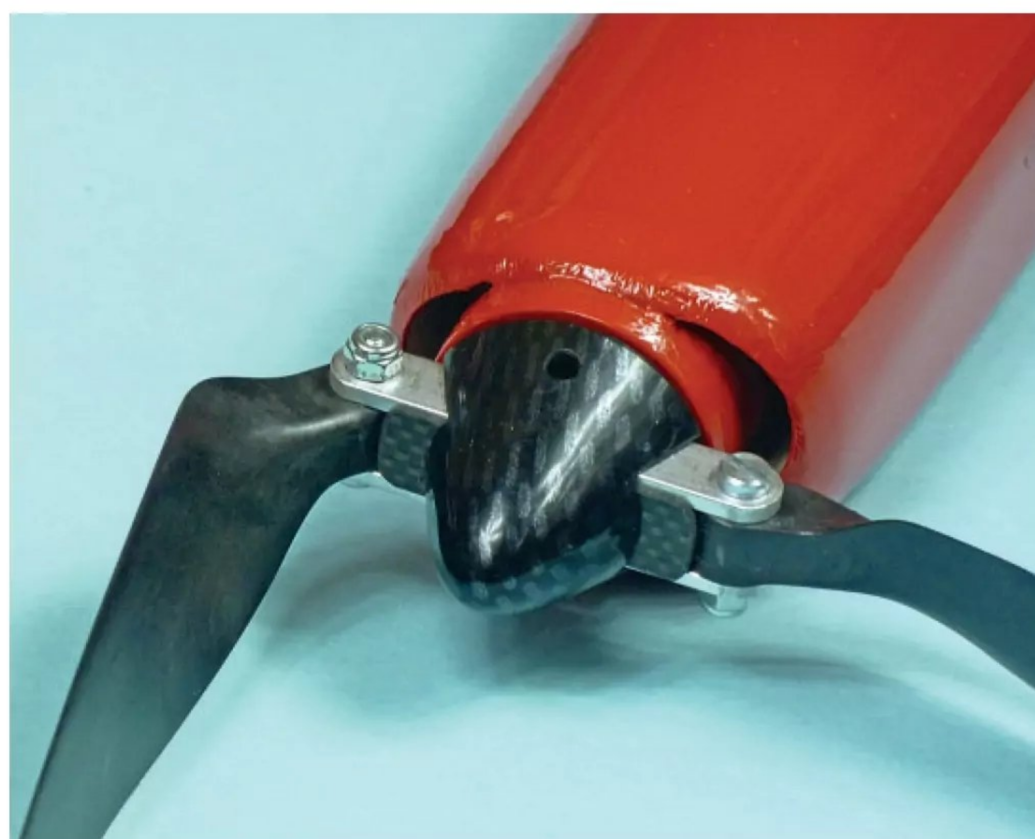
Once fitted the thin carbon fibre strips look unobtrusive but do an essential job.
