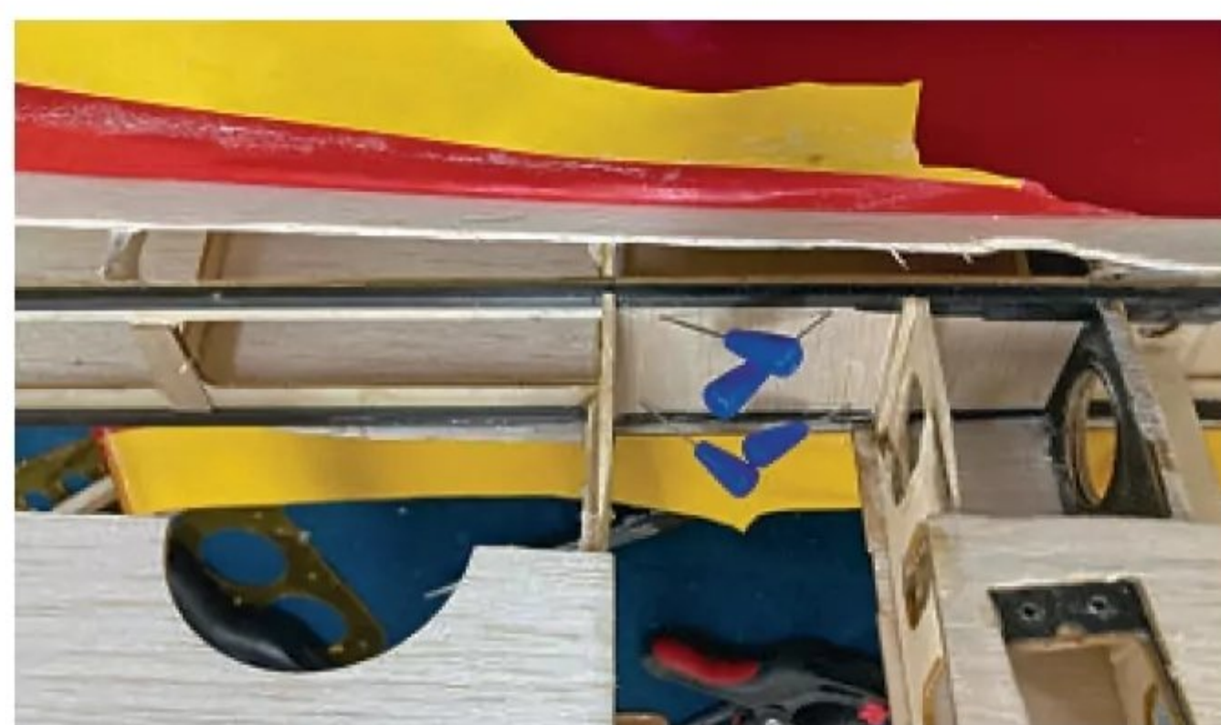
New webbing was added to the damaged area to strengthen the repair. When in contact with carbon always use slow-drying epoxy, never cyano or PVA.
