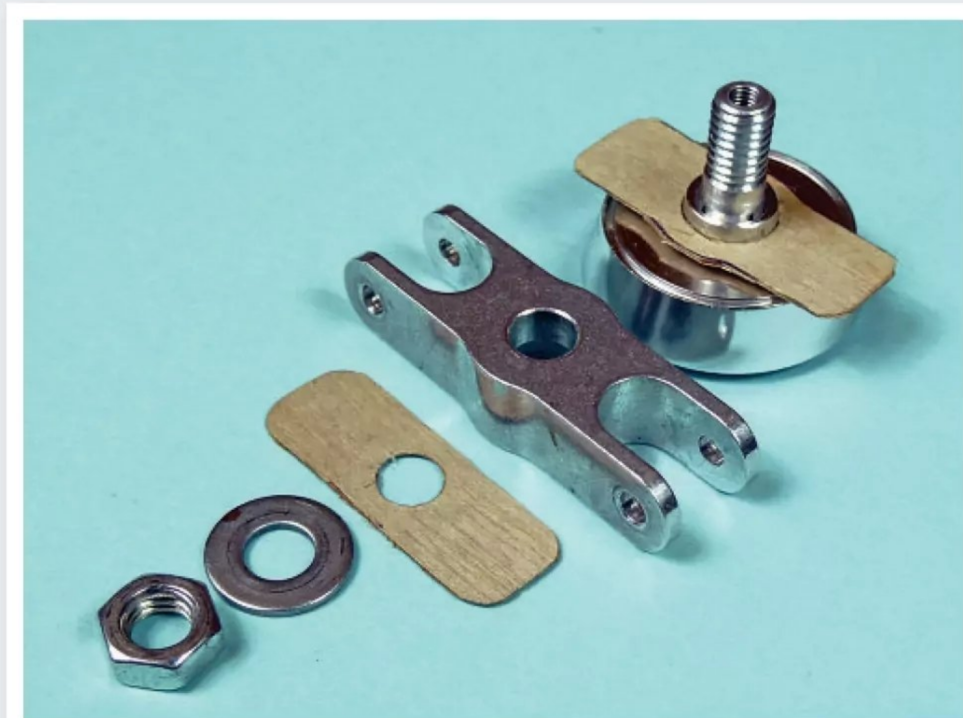
Thin ply could be used instead of carbon fibre strips.
