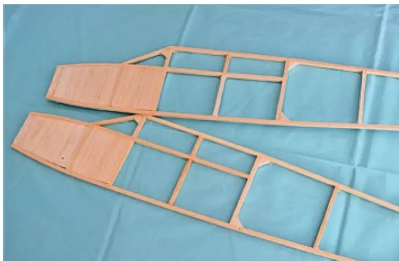
Very simple fuselage sides. Use aliphatic glue for preference as it's more resistant in a prang.
