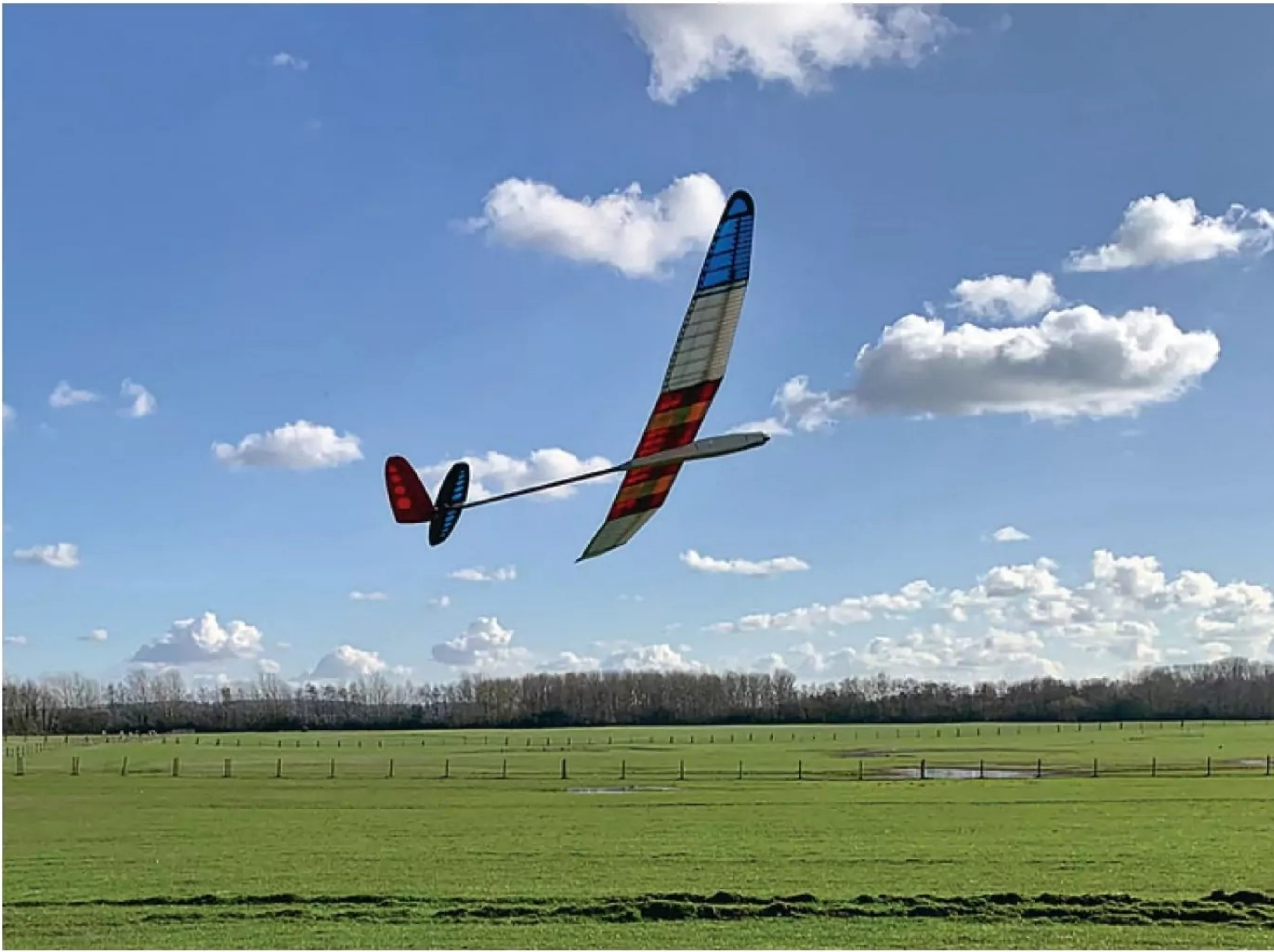
F5L class allows for a mainly wooden 2M thermal soarer using an electric motor for launching.
