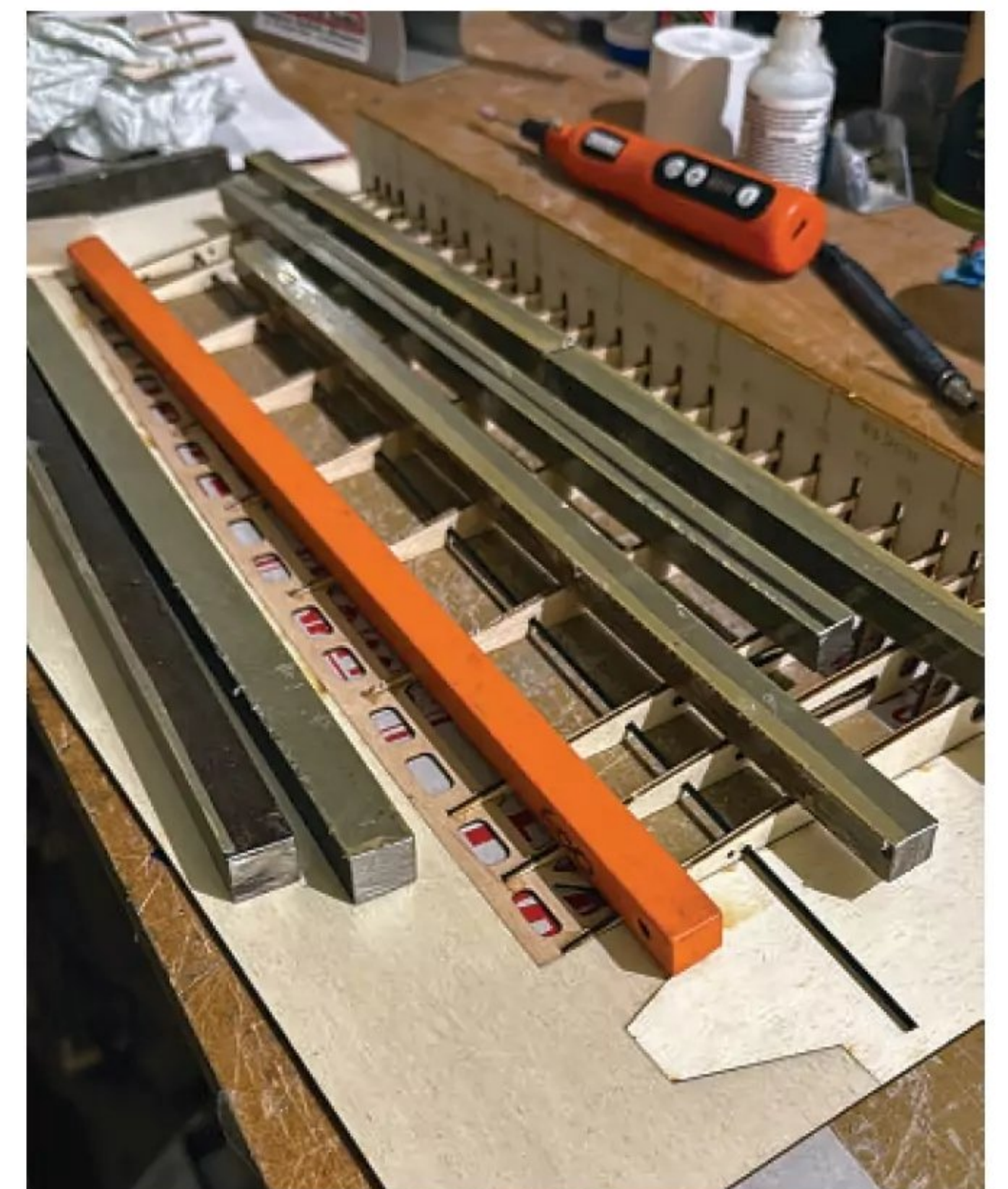
No plan required. The wing slots together, with the ribs spaced evenly using a ply jig. Spanwise weights hold it flat while the glue sets.
