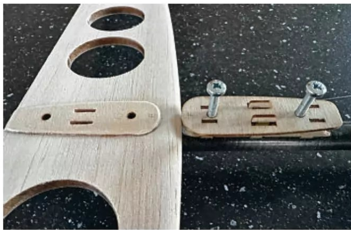
Horizontal stabiliser is screwed to a ply mount.
