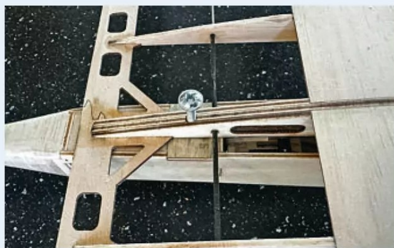
Single screws, front and rear, hold the wing to the fuselage.
