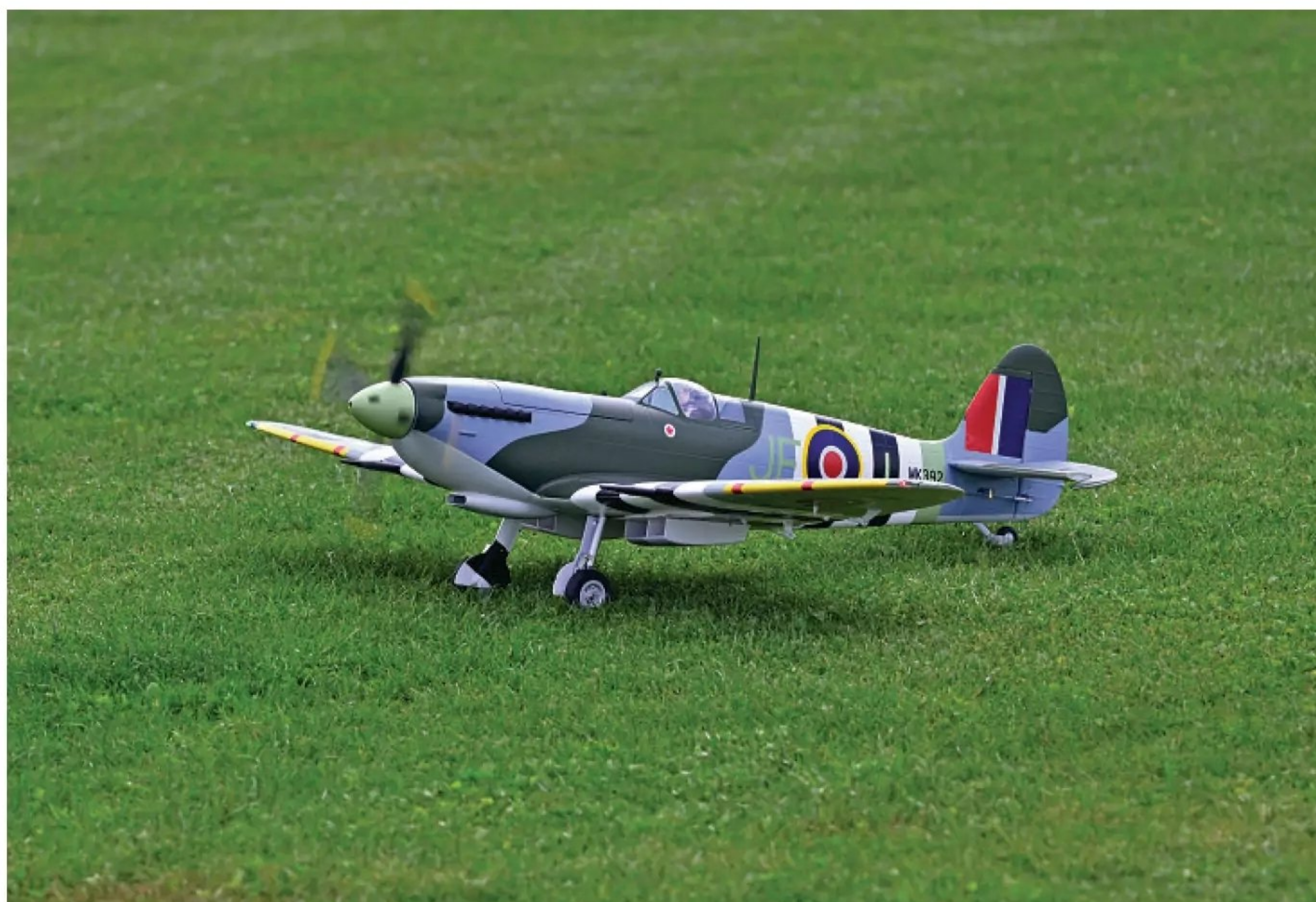
Due to the narrow track undercarriage and small wheels the XFly Spitfire is best flown from short grass or tarmac. Even this well-manicured turf is starting to get a little long for safe take-offs
