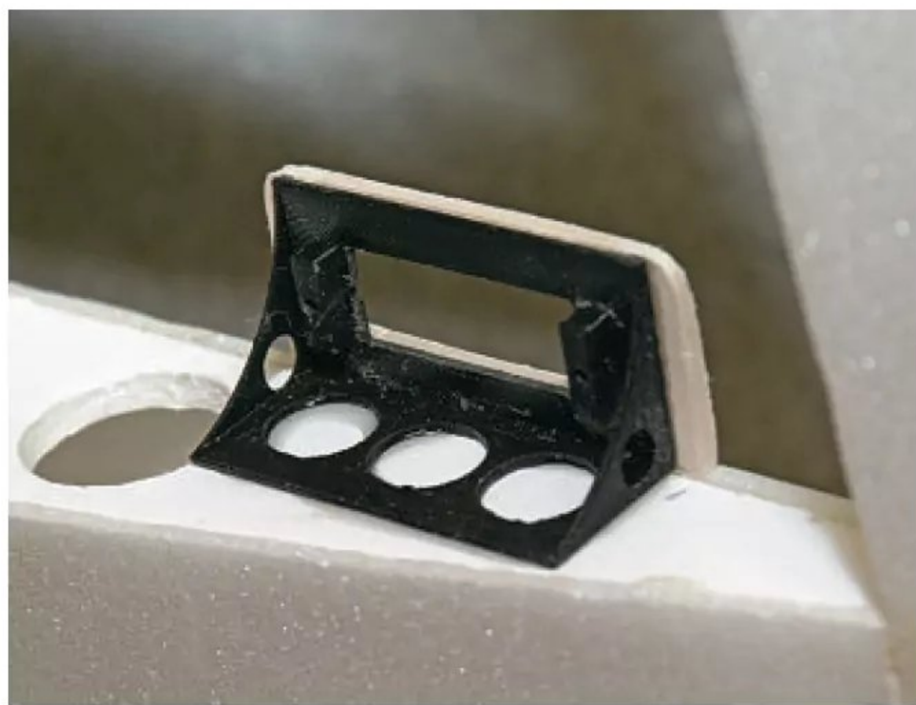
Aileron servo mount glued to W2.
