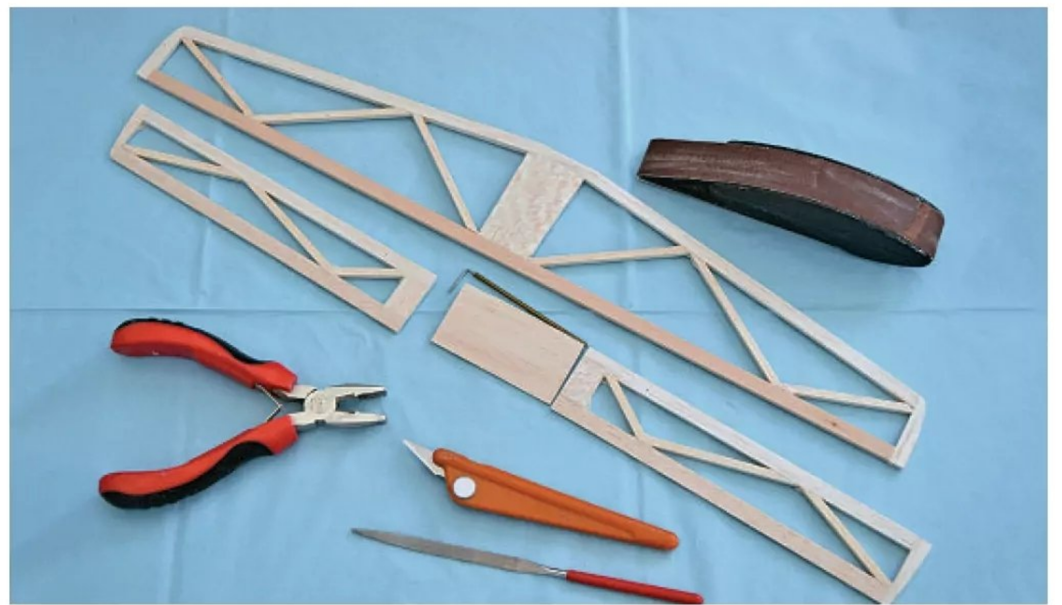
Tailplane is dead simple. I've found that you only need one elevator half for adequate control.
