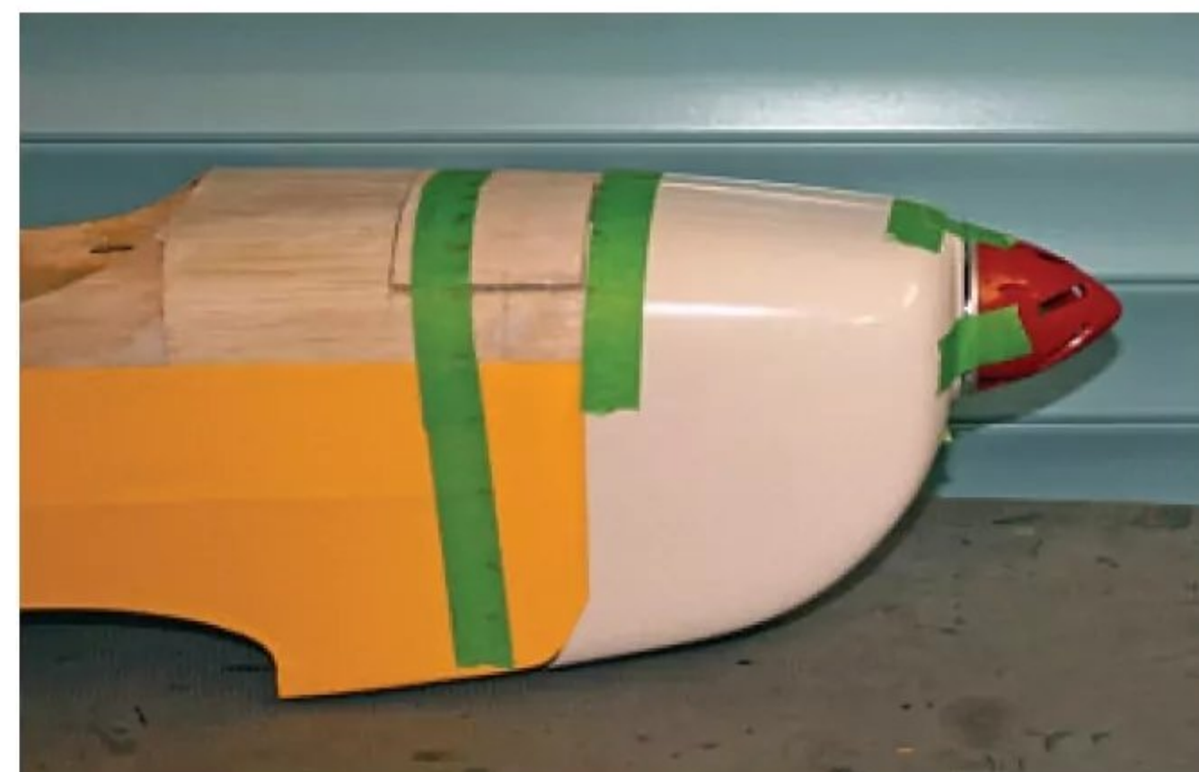
Shaped cowl showing measurements and cut line.
