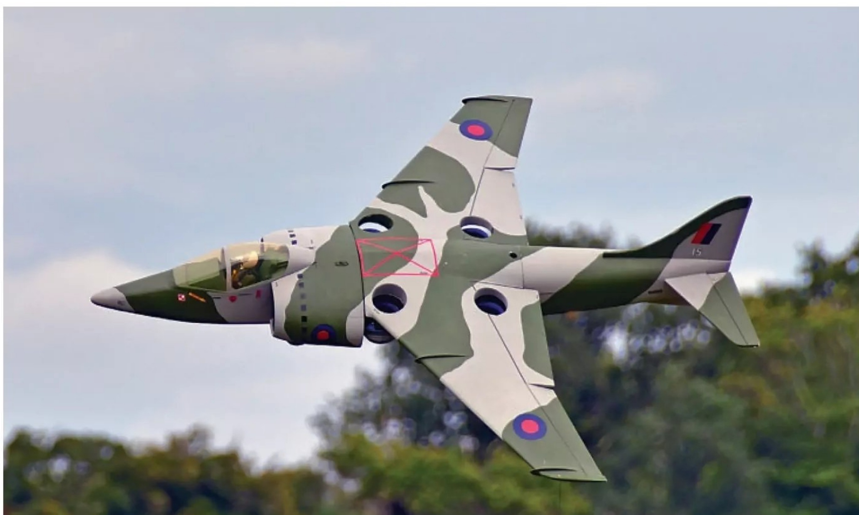
Tony Nijhuis' epic VTOL Harrier project with four vectored EDFs. Note the cheat holes in the wings to allow air into the fans for hovering.
