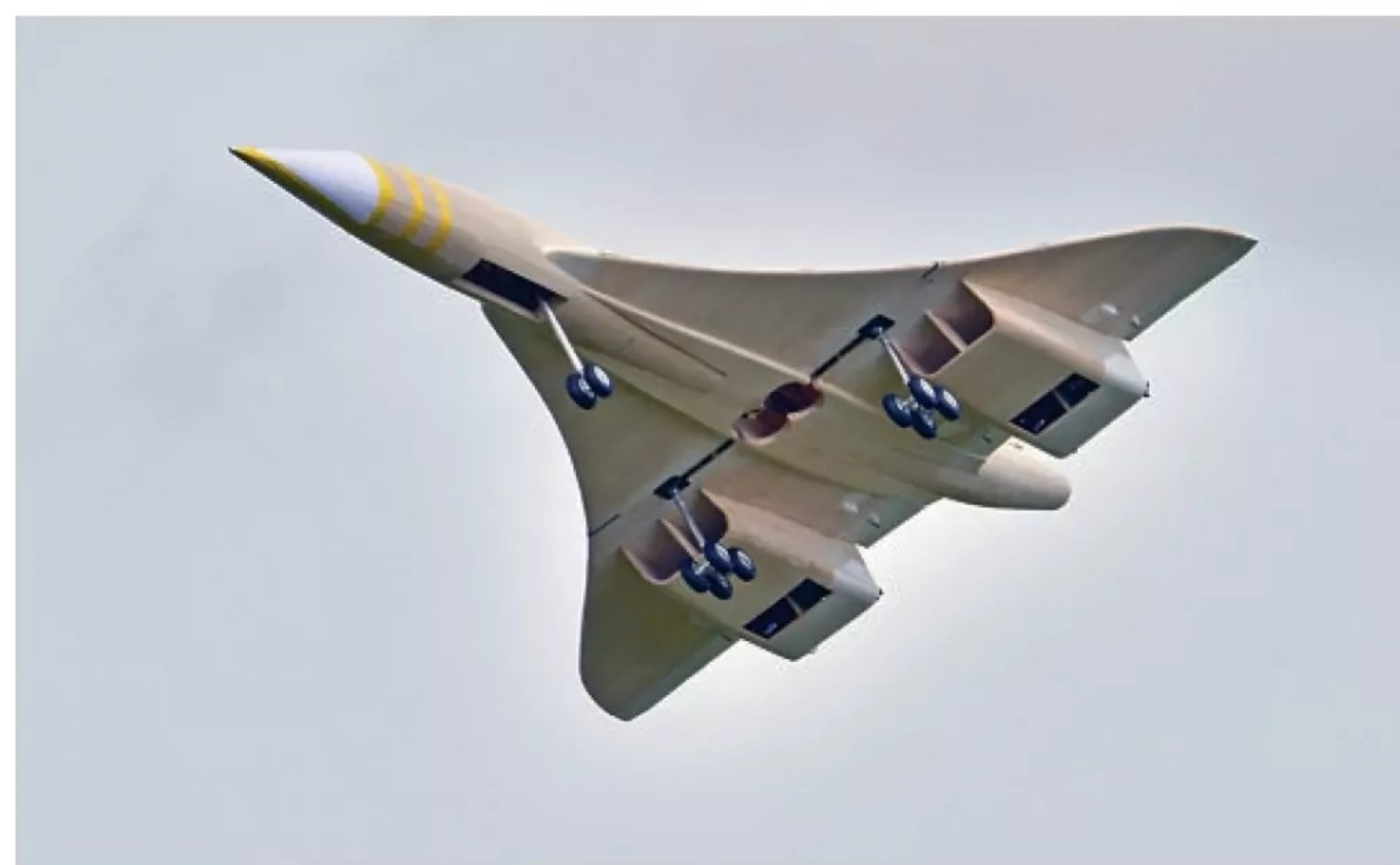
Unmistakable shape of the iconic Concorde in the air. Tony Nijhuis' 2.7M long prototype looked awesome with its four 70 mm EDFs on full chat!
