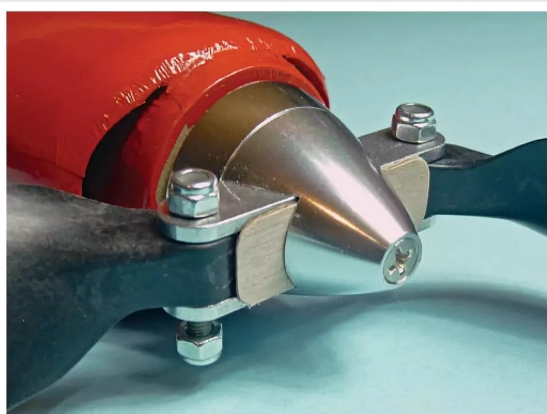
Once fitted the thin carbon fibre strips look unobtrusive but do an essential job.
