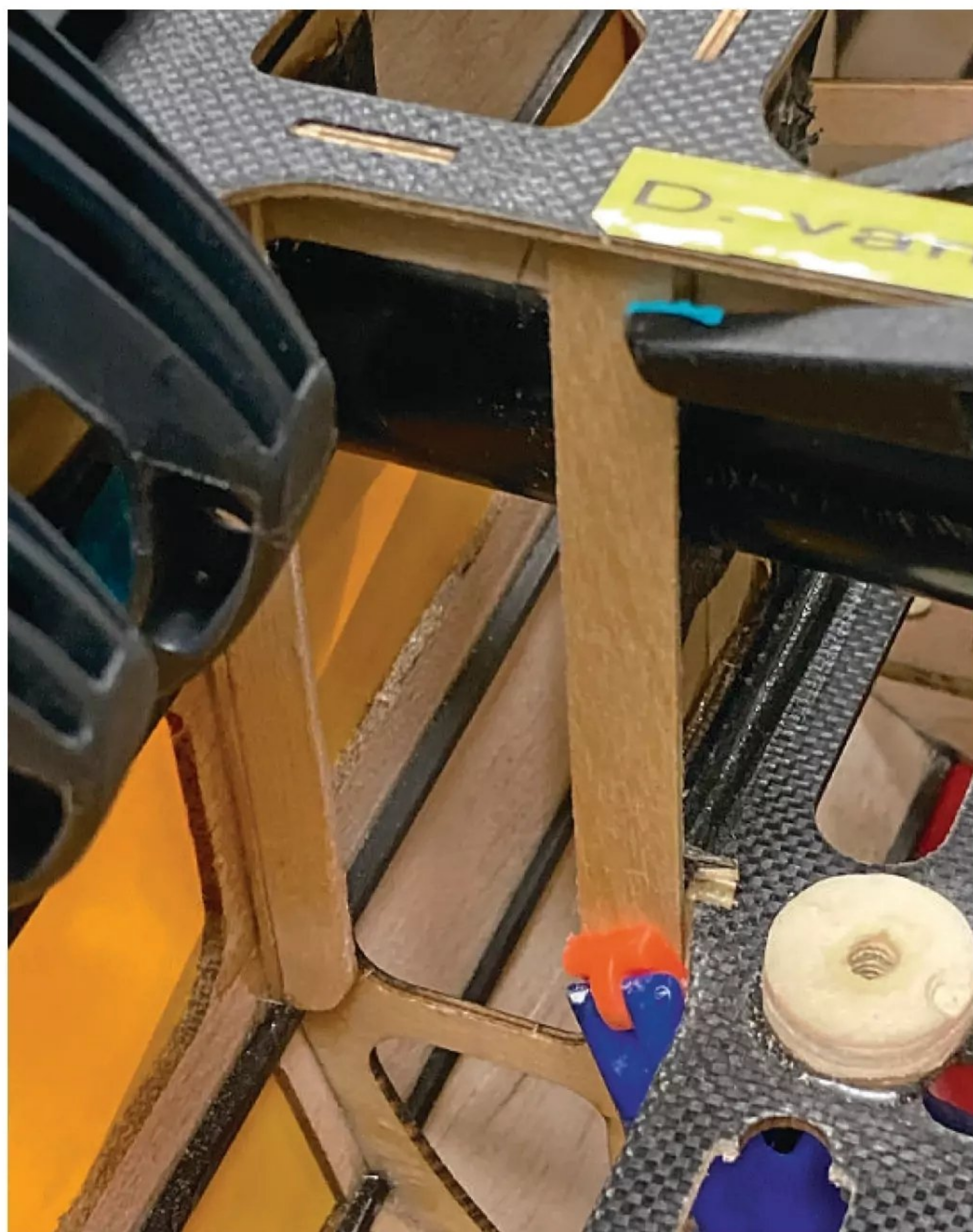
The former holding the wing tube had been damaged on both sides of the fuselage, which was easily repaired. The first step was to install a strip of 1.5 mm (1/16") aircraft grade plywood to act as a support for the fuselage side, which also required repair. There is no need to beef up the original structure.
