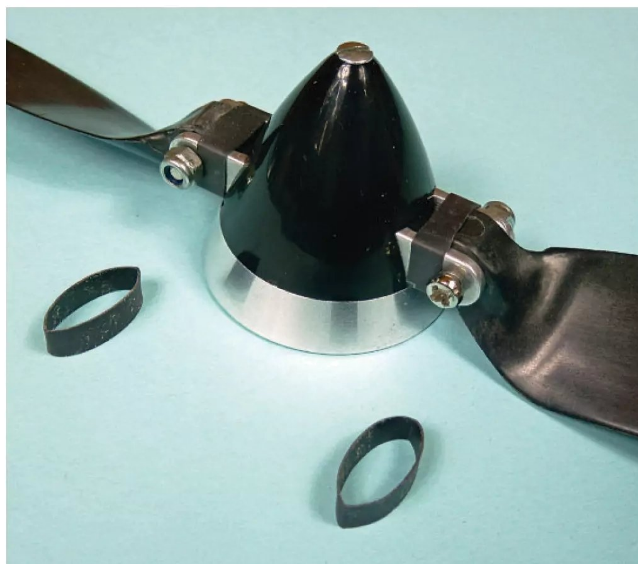
My preferred solution is to use shrink wrap tubing which is cheap and easy to fit. This is the method I use on my Hi8us flying wing.
