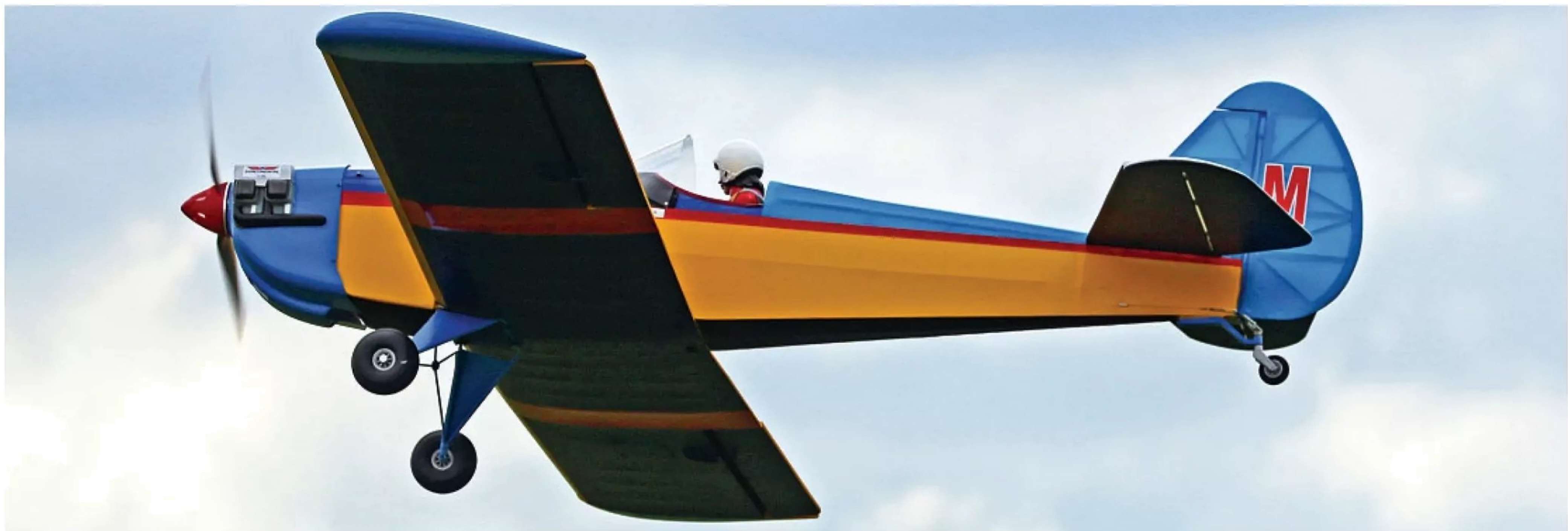
Wings and fuselage were covered in Oratex, with bright colours selected for good visibility in poor light conditions.
