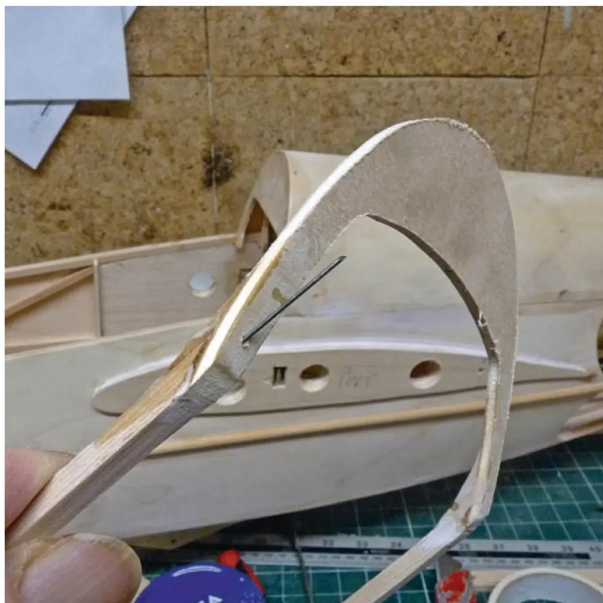
Gain extra security and peace of mind by pinning the canopy frame together.
