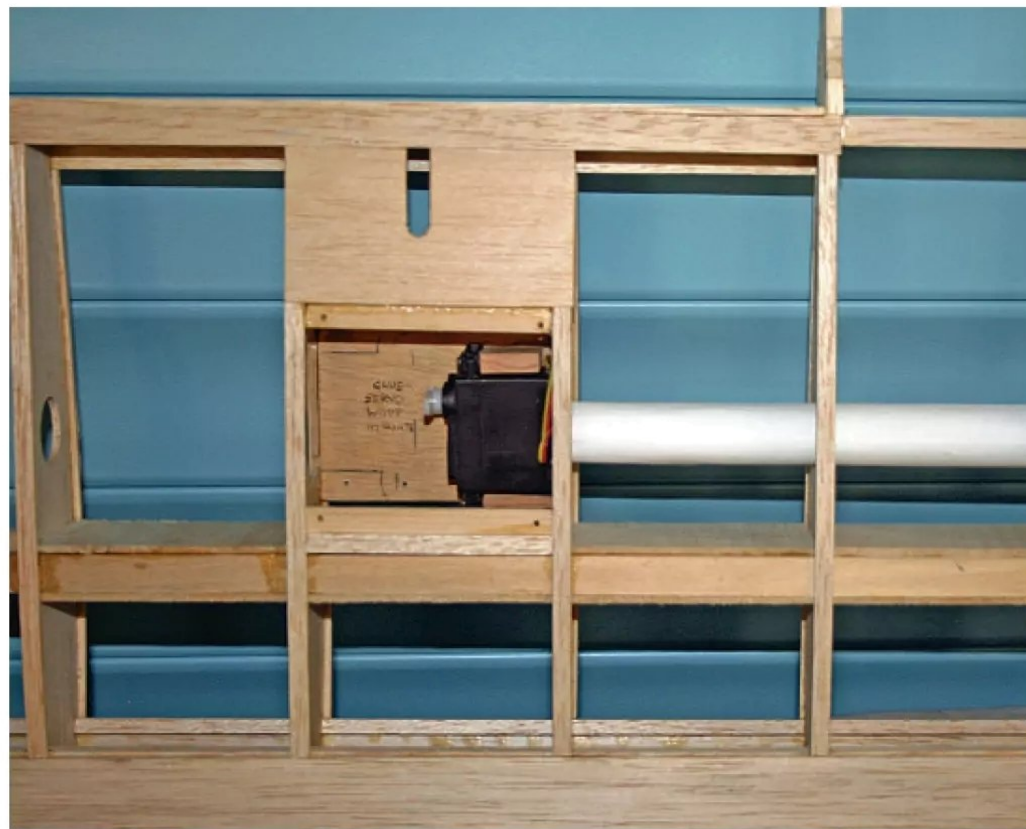
Aileron servo fitted, with wiring passing through the tube to the fuselage.
