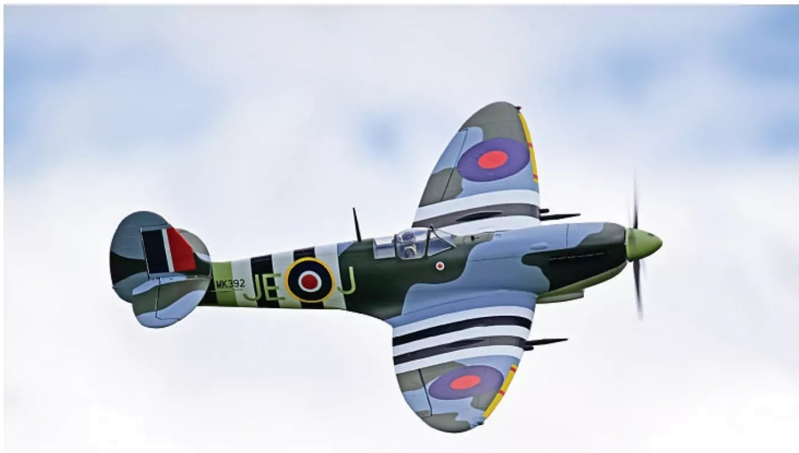
I used a Voltz 4S 4200 mAh LiPo when test flying the new Spitfire. It's the perfect weight to avoid needing to add any lead in the nose.
