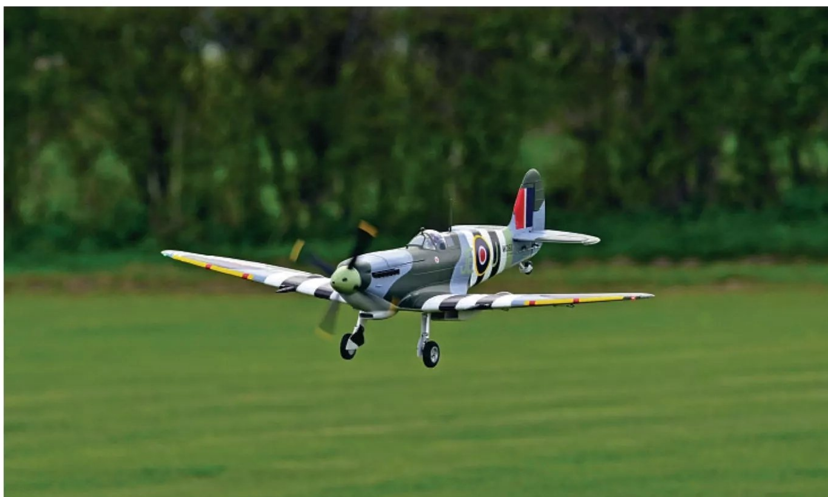
Half flap is all that's needed for a well-controlled approach.
