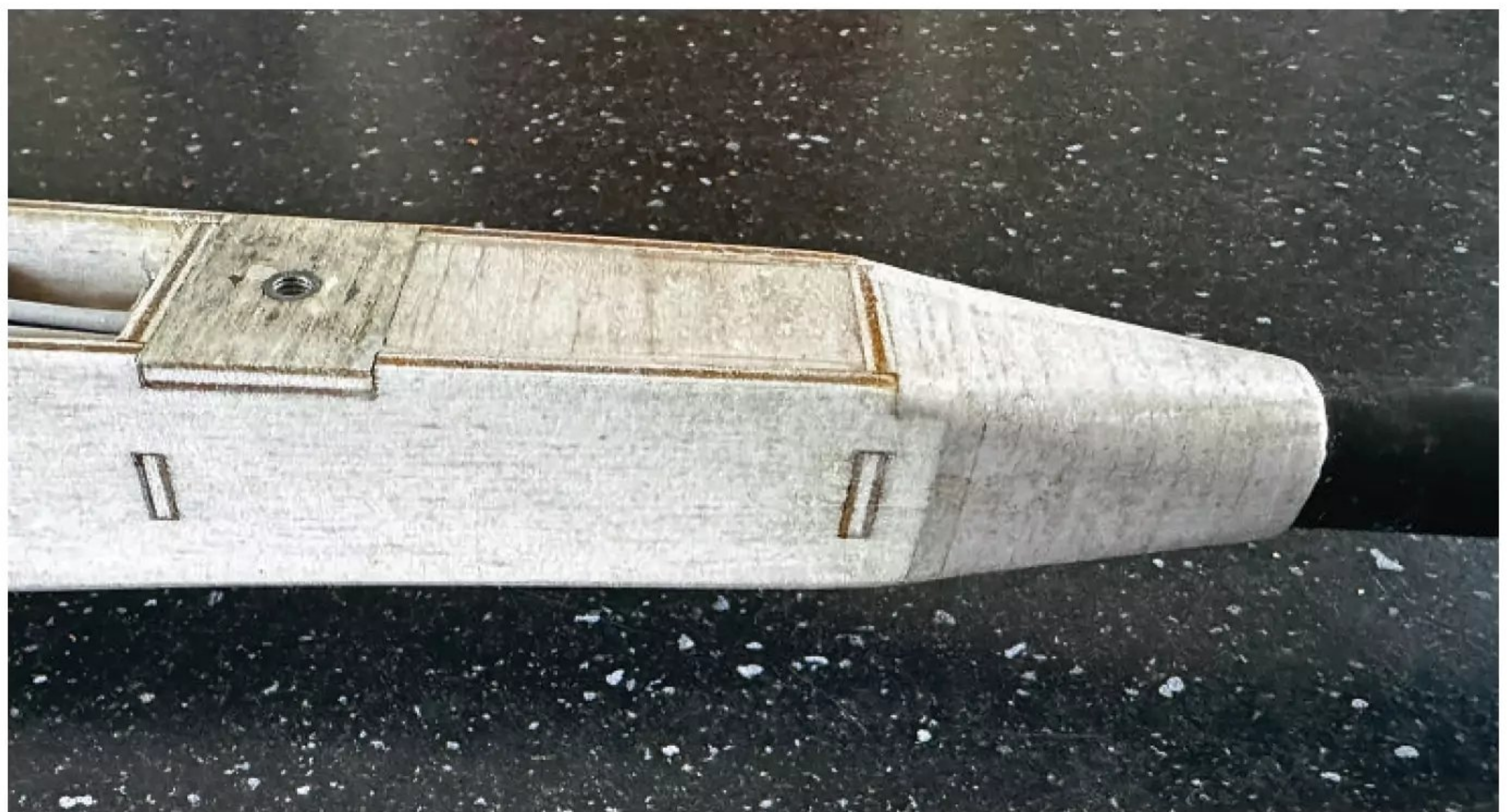
Another view of the back of the pod, this time showing the laminated boom support.
