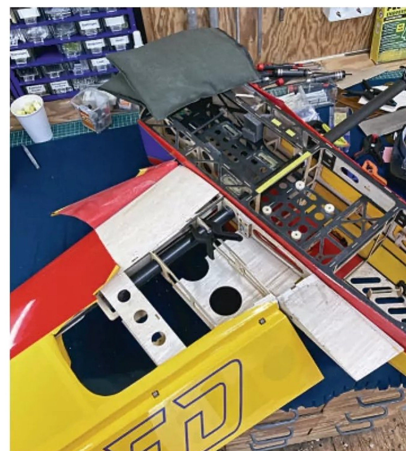
With the spar repaired and the ribs back in place the wing tube can be glued in place again. It is vital to check the position of the wing panel carefully. Not only does it need to fit flush against the fuselage but also the incidence of both panels needs to be equal. The next step is to repair and/or replace the ribs and glue them back in place, making sure to keep them in line with the undamaged ribs still in the wing.
