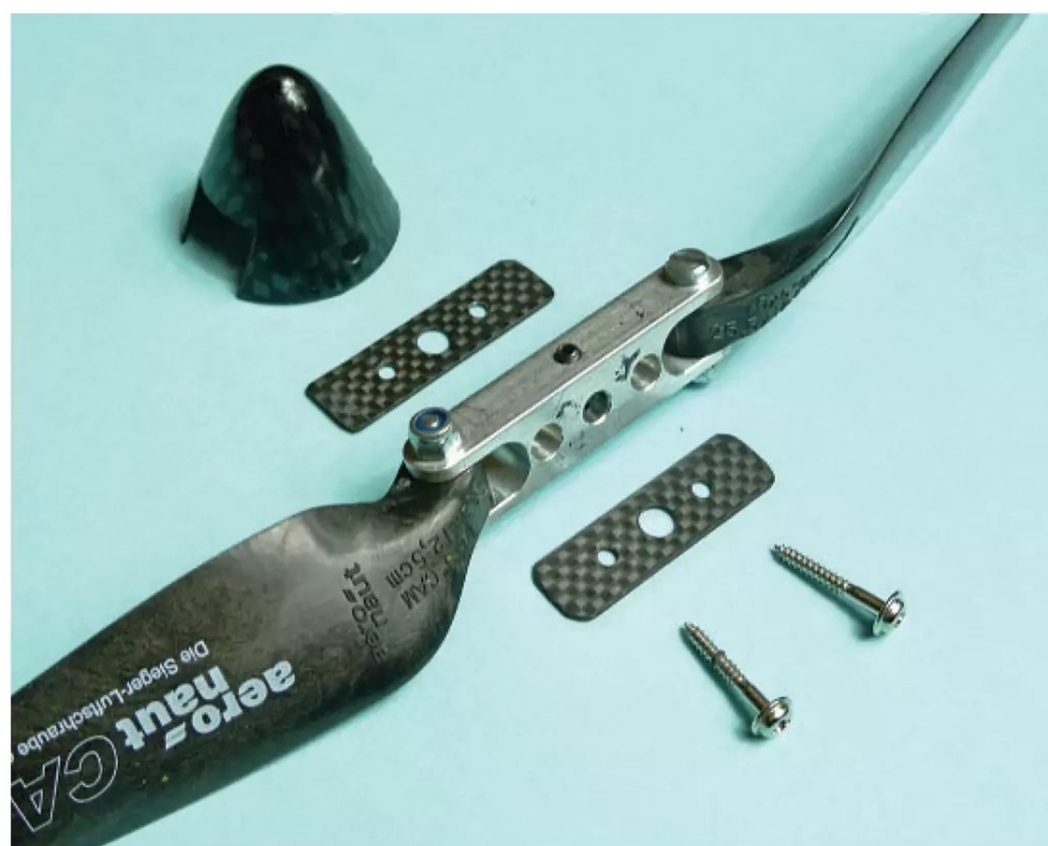
Thin carbon fibre strips added to either side of the yoke limit the blades movement.
