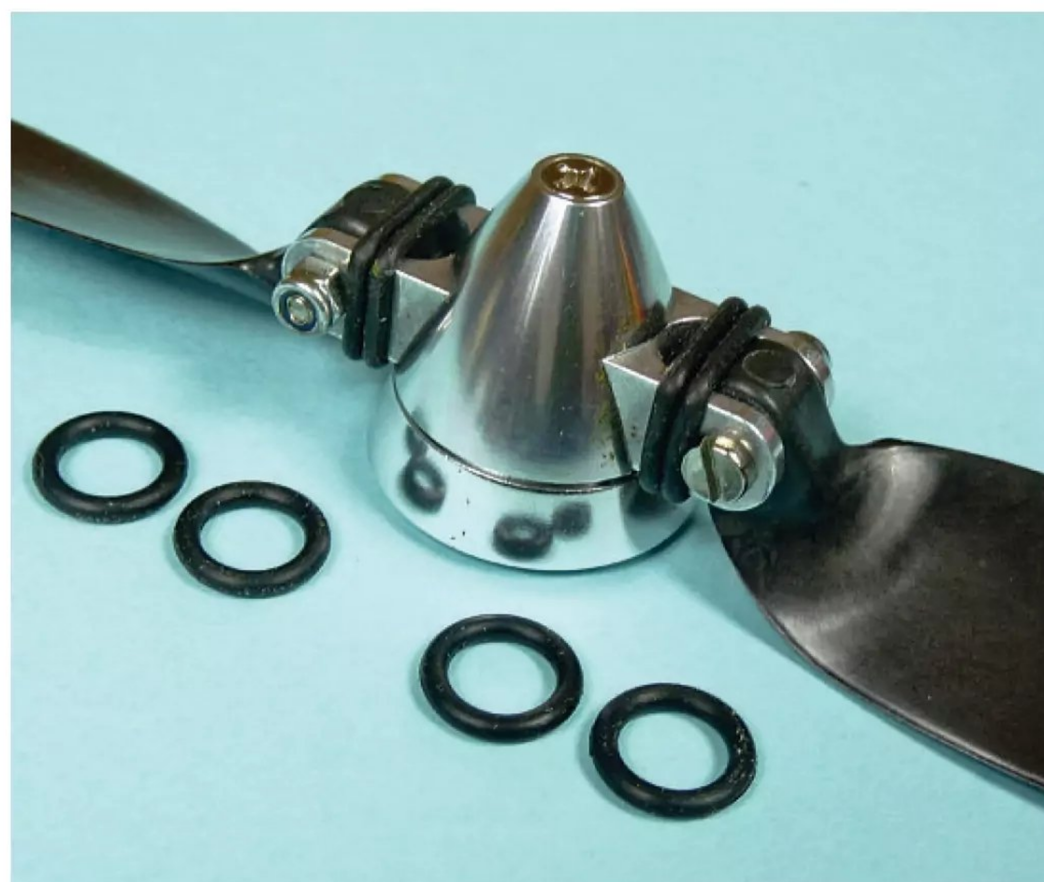
O-rings slipped onto the yoke before the blades are fitted limit the blades movement, but the diameter and thickness of the O-rings needs careful selection to achieve the desired result.
