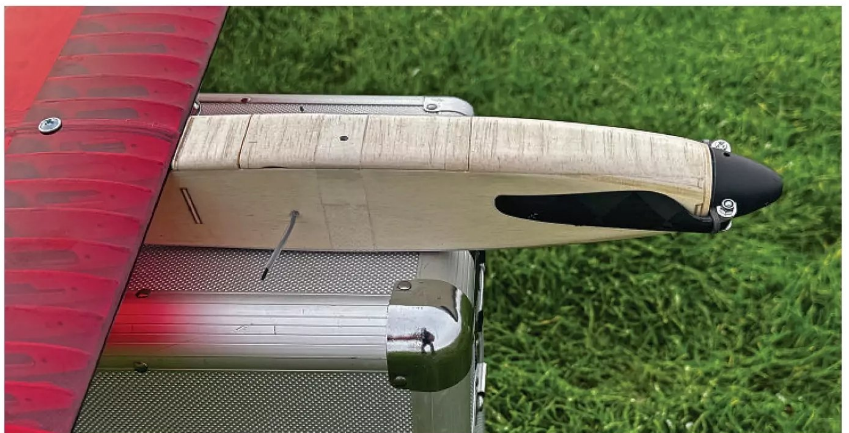
Careful shaping of the nose is needed to blend the ply and balsa parts, allowing the corners to be rounded so that the folding propeller fits snugly along the fuselage to reduce drag.
