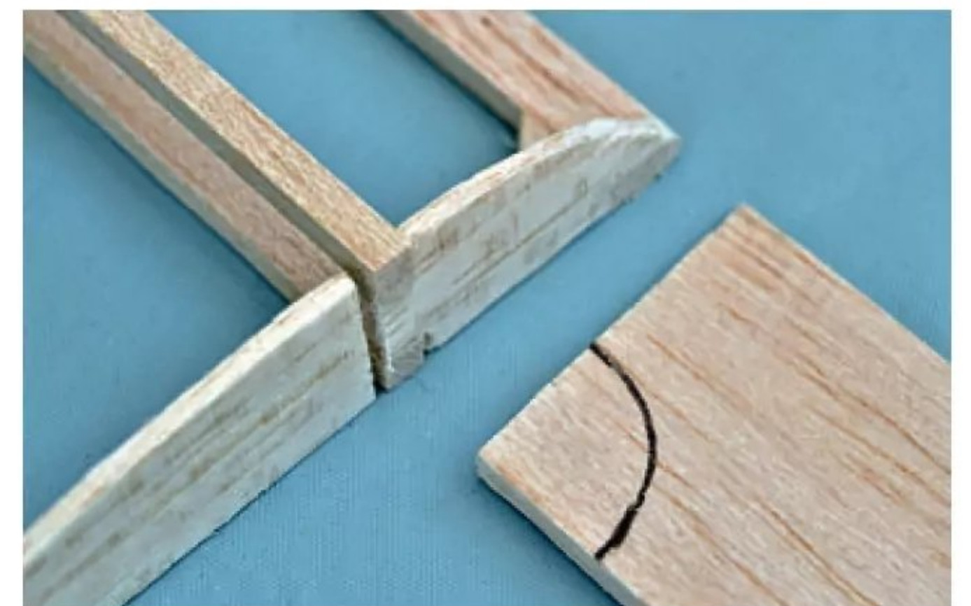
Don't forget to give the outer panel root ribs the correct tilt.
