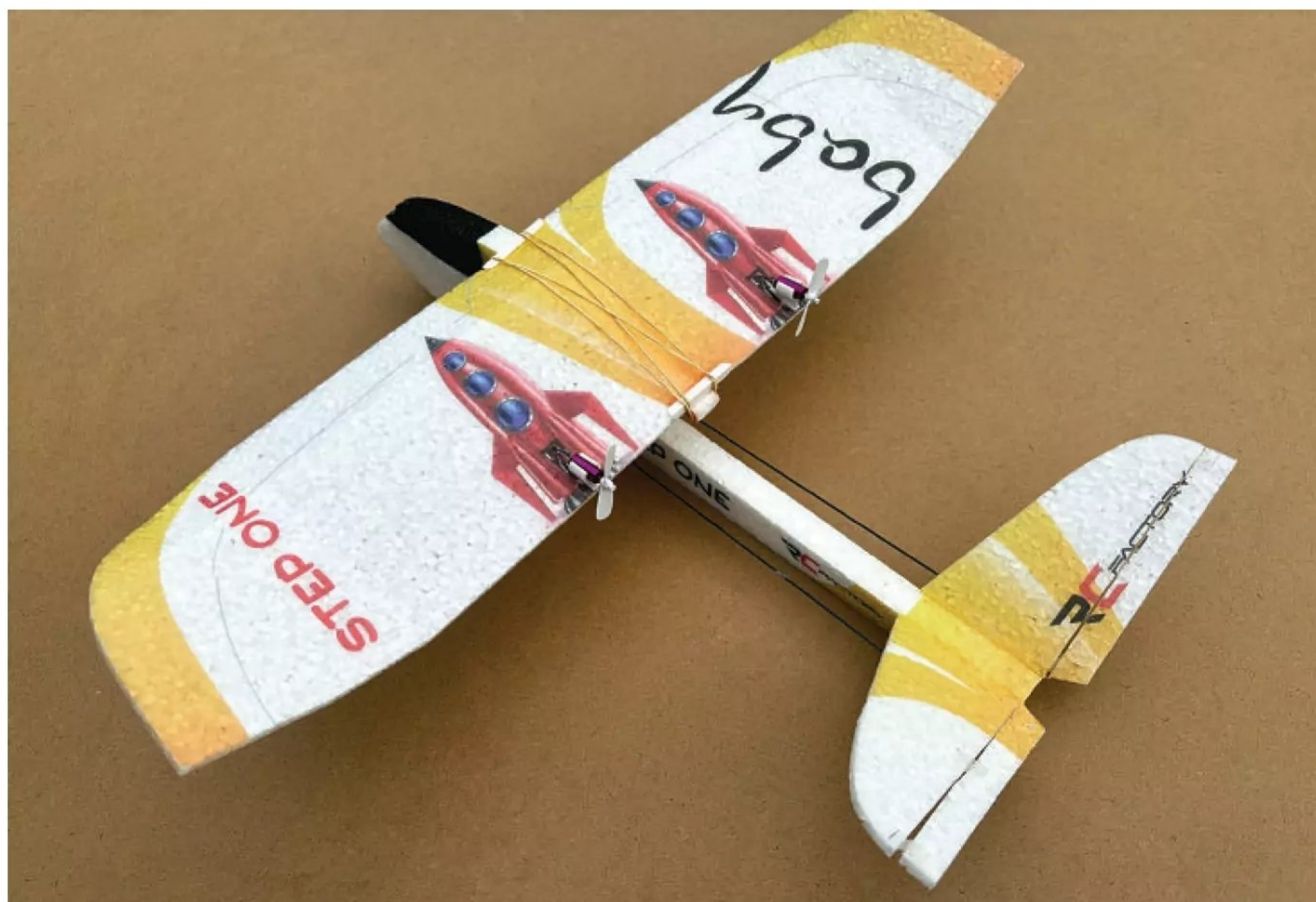
Twin trailing edge 6 mm coreless motors are the Baby's special feature, fitted with 30 mm handed props.
