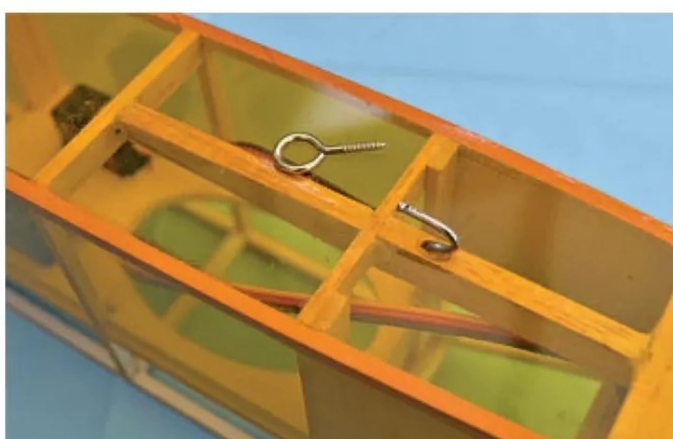
Tow hook is simply a tiny screw eye straightened out. Use a dab of epoxy glue to prevent it loosening.
