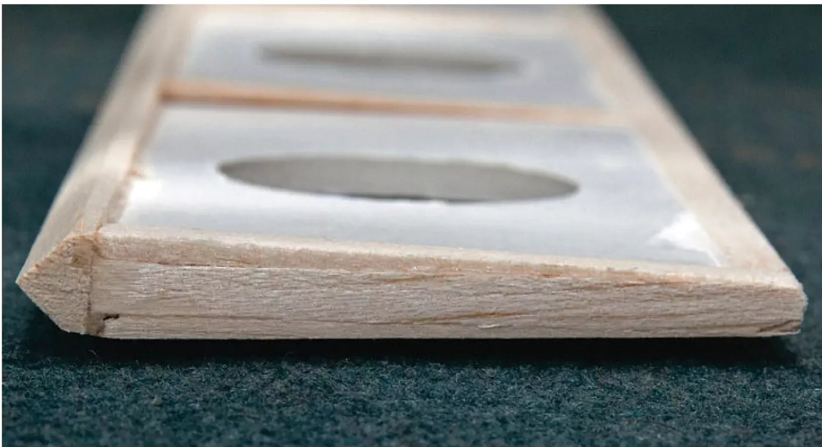
Aileron cross section.
