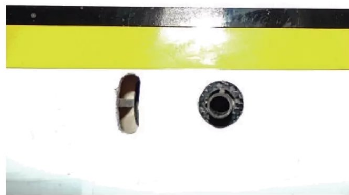
Chain drilling one side of the fuselage. A cocktail stick was used as packing to lift the tube by the required amount.
