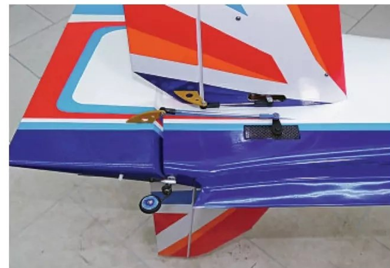
Servo cover made from carbon sheet and bonded into place.
