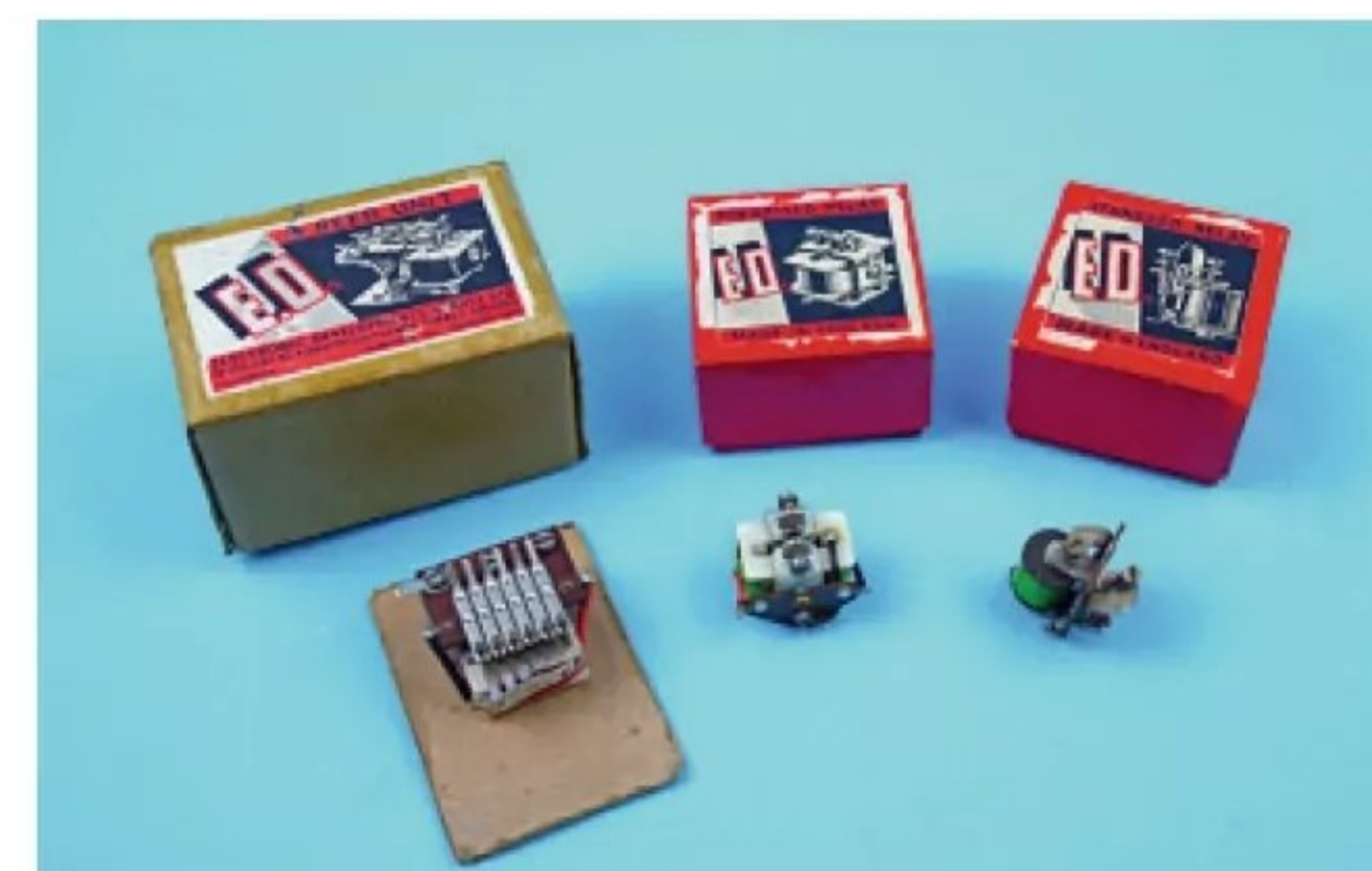
ED sold several parts for the home builder. From the left: a six-channel reed bank (comb), polarised relay and standard relay.
