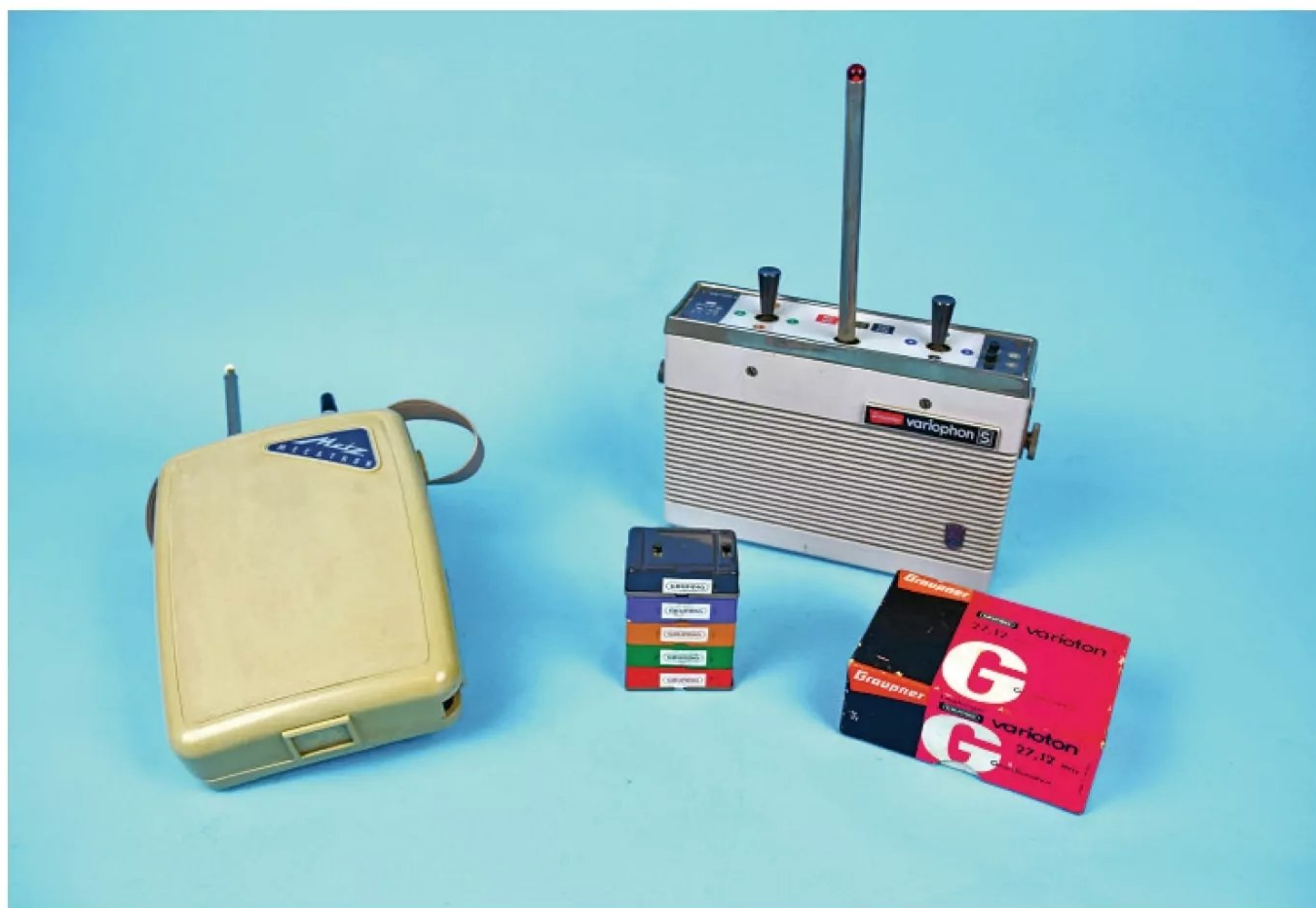
Examples of the Graupner and Metz tuned filter sets, plus the Graupner plug together receiver allowing easy expansion of channels.
