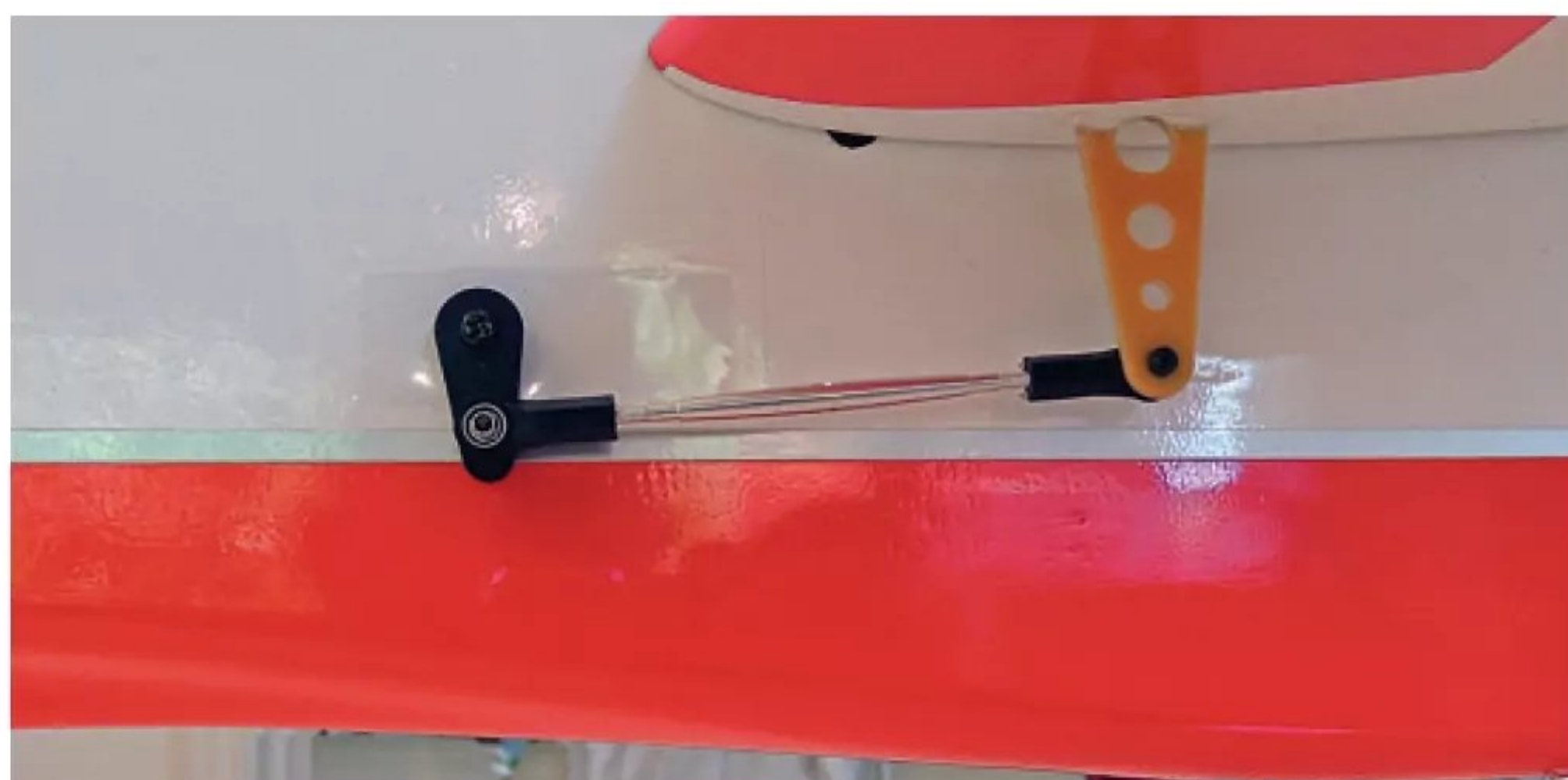
All Moving Tailplane (AMT) arrangement in the Fantasista.
