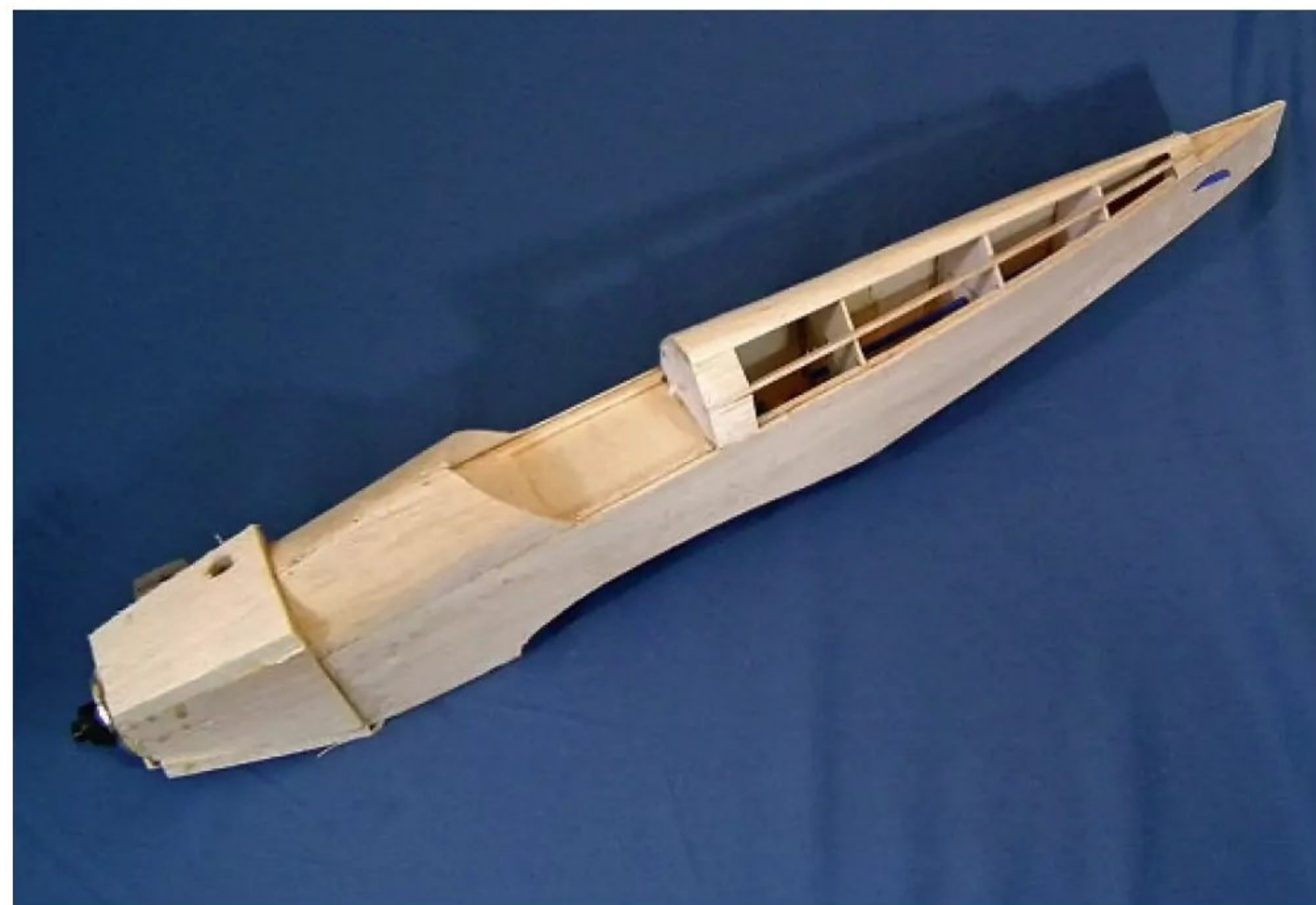
A sheeted fuselage. Note the thick sheet cowl and spine on top of the rear deck. The odd stringers could be cut from sheet in this case.
