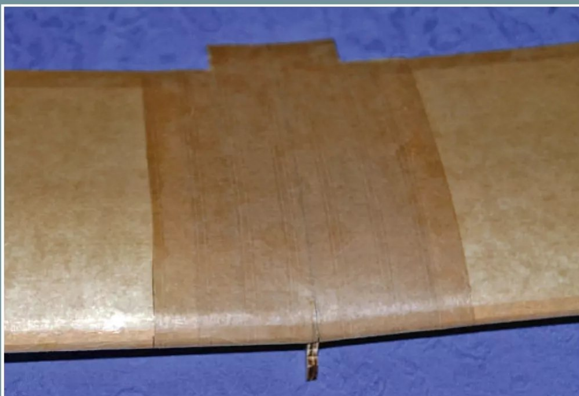
Some extra wraps of brown paper help to reinforce the centre section.
