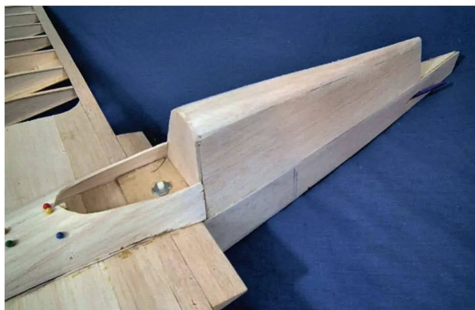
Slab sides on a rear turtle deck with a thick sheet top. Note the plywood on the cockpit floor and the blind nut for the wing bolt, both of which need to be on your list.
