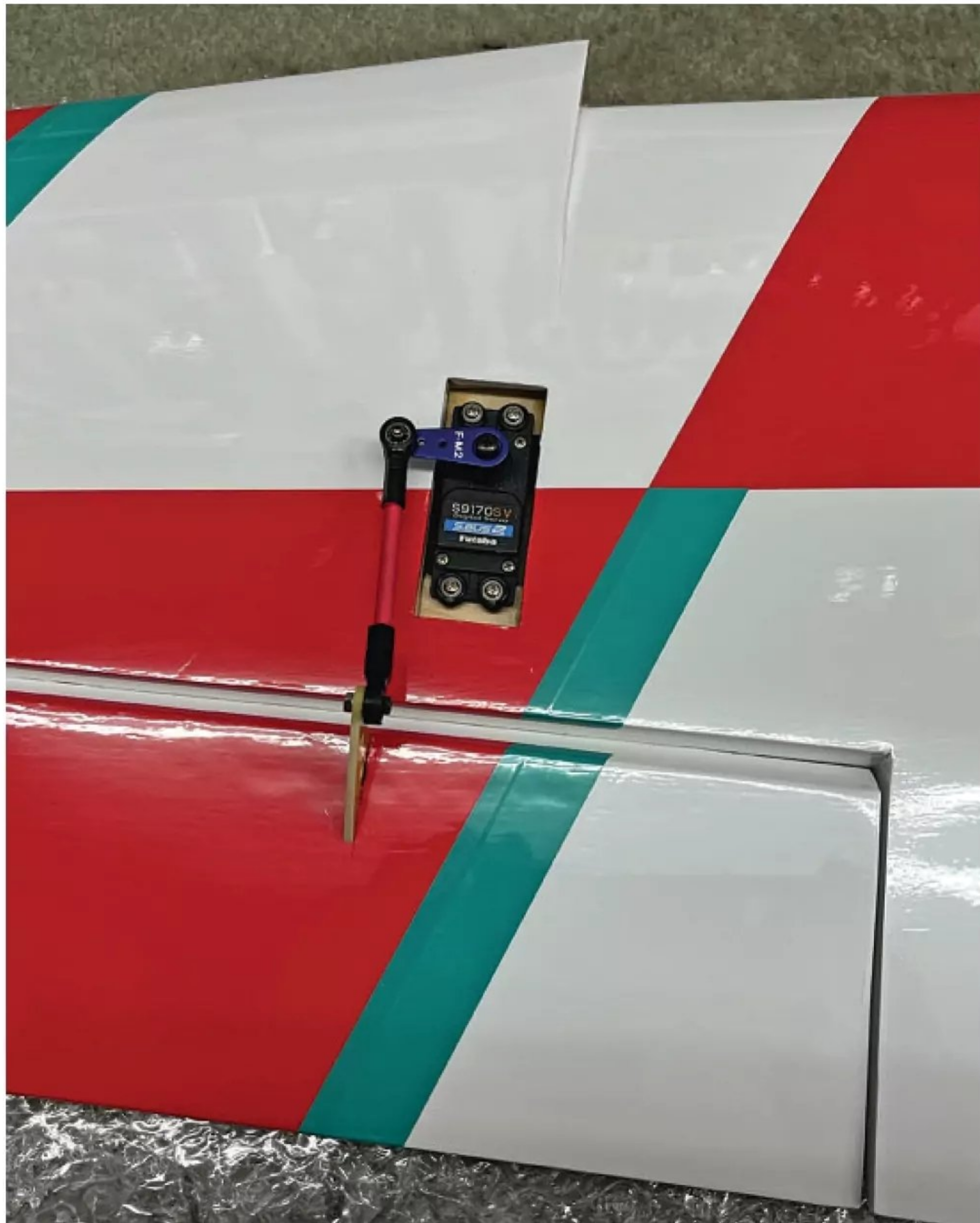
Typical servo aperture with two colours.
