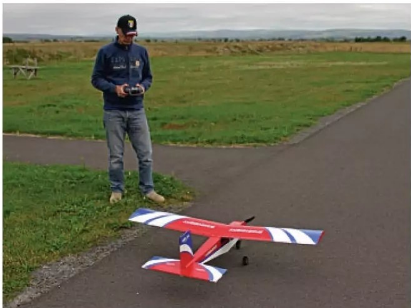
Bertrand performs a control check before flying Ambisagrus. This should be done before each and every flight, whether a beginner or experienced pilot. Tyro pilots may prefer to do this from behind the model.
