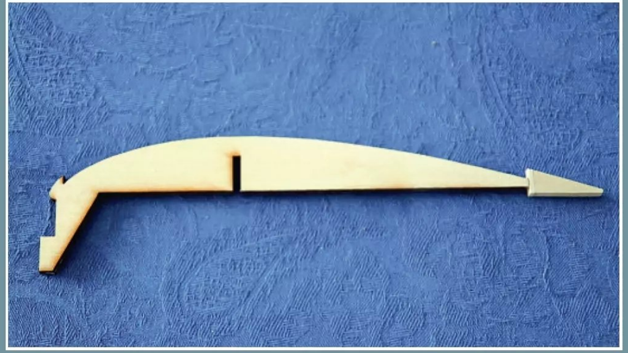
Central ply rib has a forward retaining 'hook' built in.
