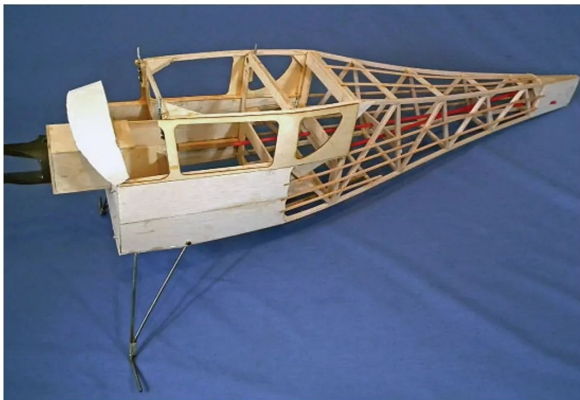
This built-up fuselage will need to be measured up on the plan. Also, all the stringers will be needed, plus assorted pieces of sheet. Inside there are hardwood servo rails which should be shown on any plan.
