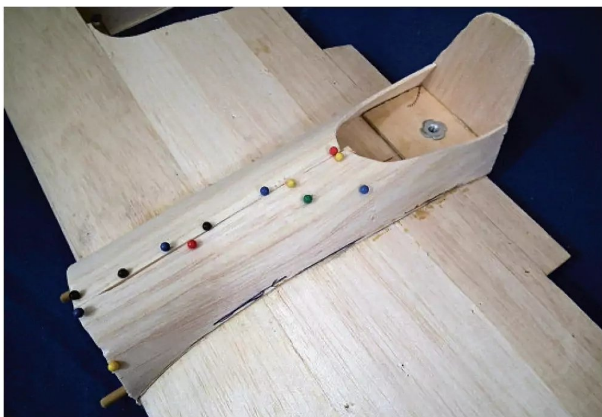
Rolled sheet turtle decks can use up quite a lot from a sheet.
