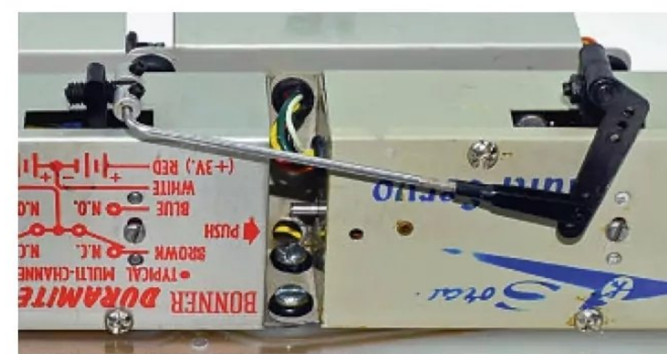
A ready-made linkage was commercially available for Bonner servos.
