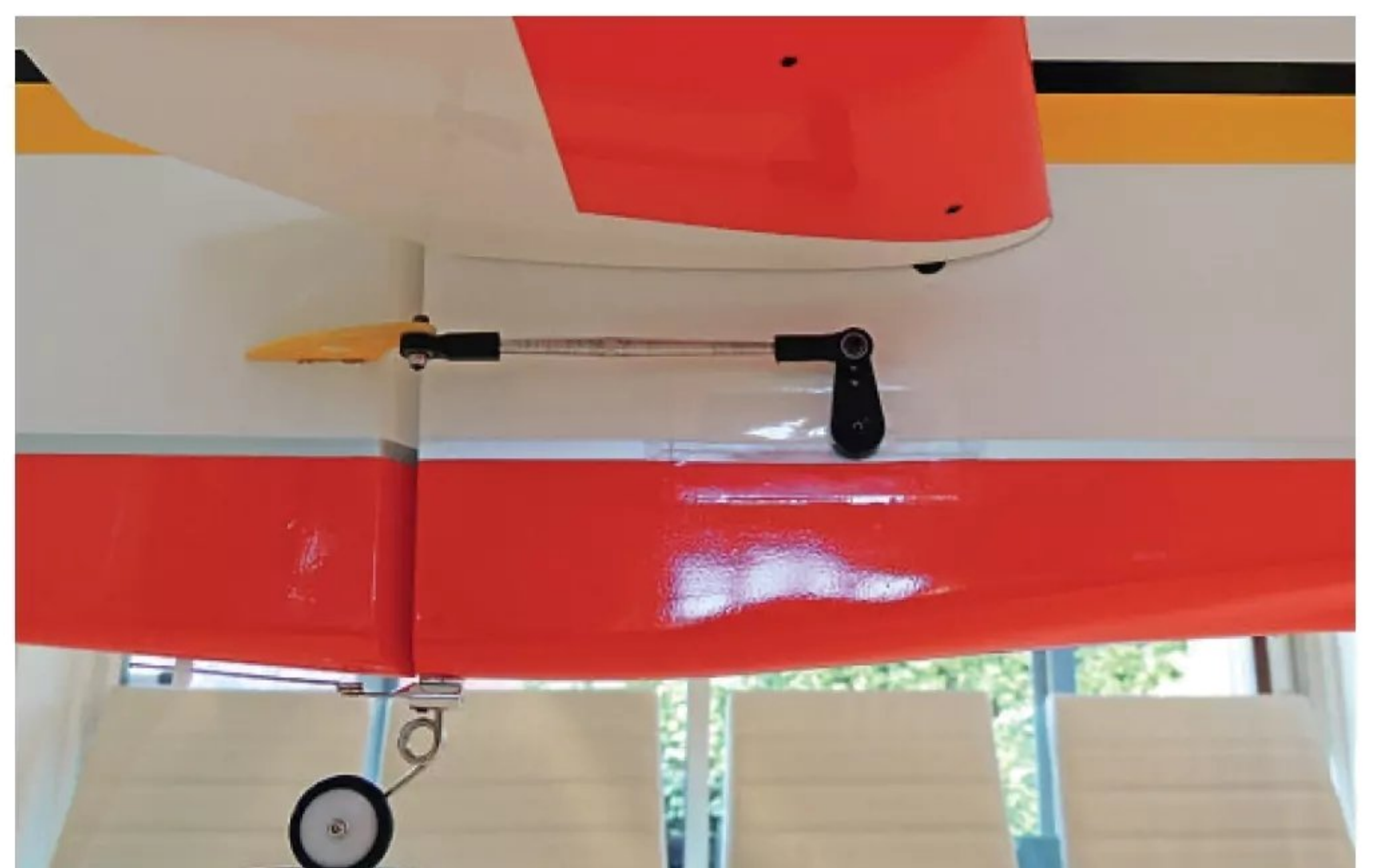
Three-layer servo cover is reasonably invisible.
