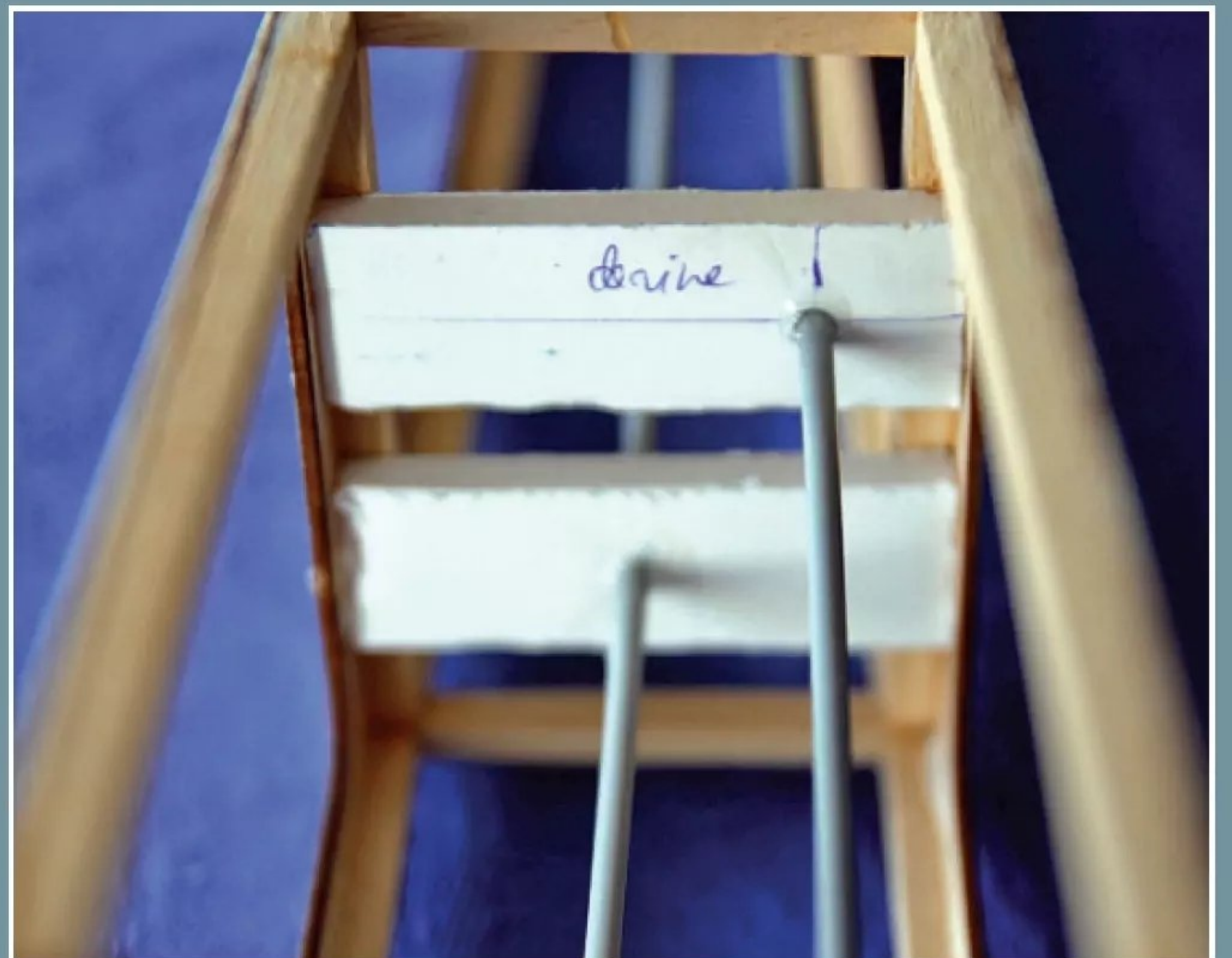
The tail servos are hooked up with a snake to the rudder and a wooden pushrod to the elevator. You could also use two snakes if you prefer but make sure to brace the runs along the fuselage to prevent them moving and introducing slop in the controls.
