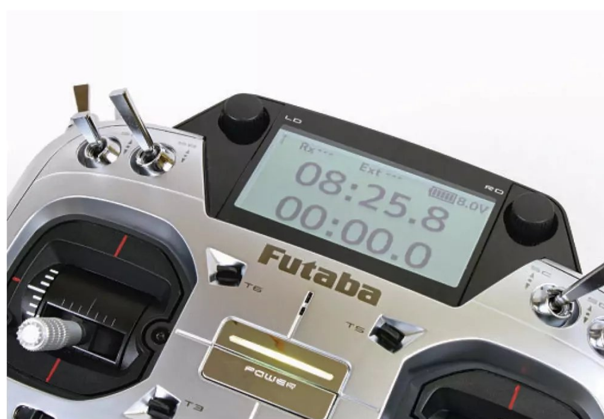
A sub-display shows timers or telemetry info but not both at the same time.
