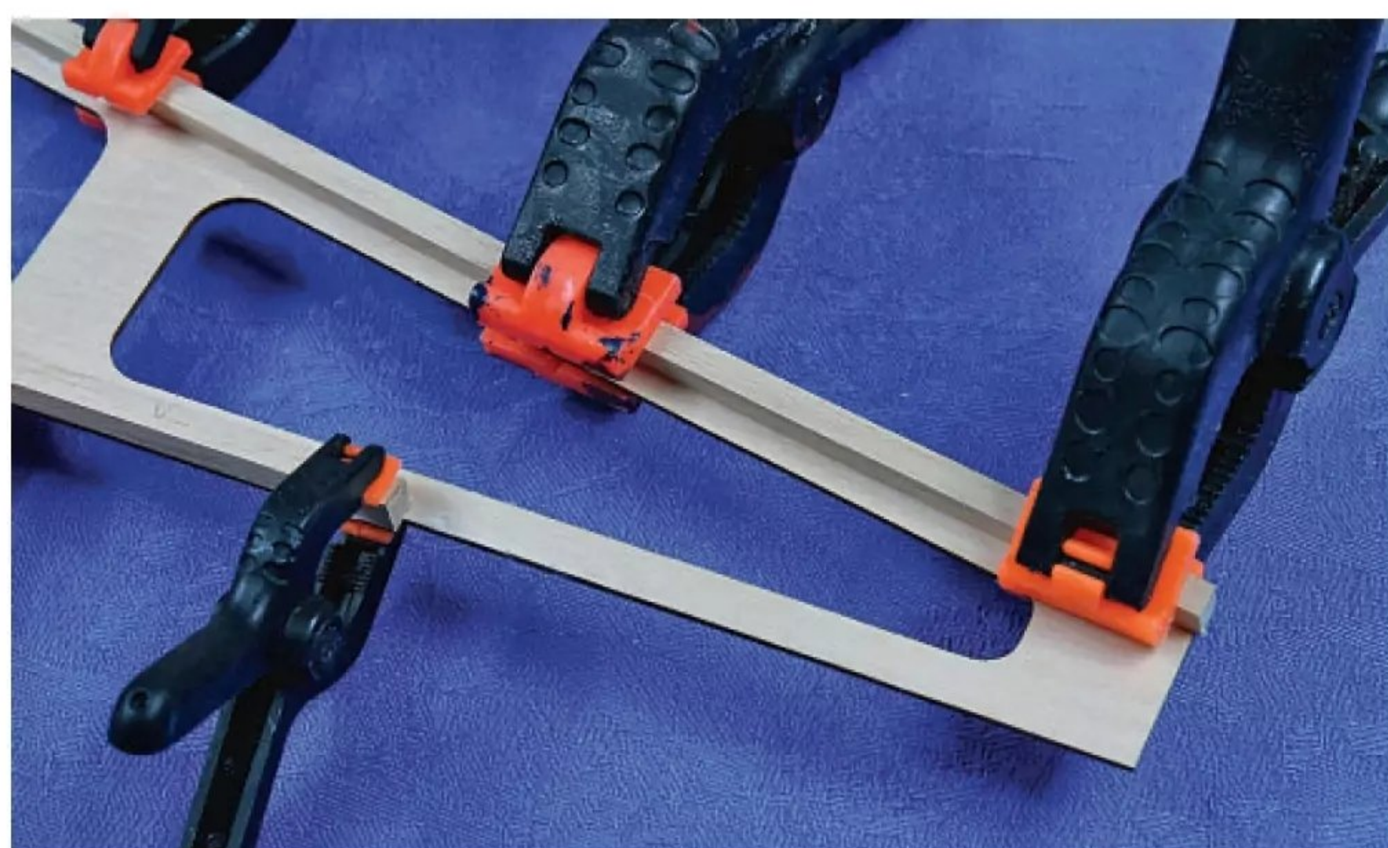
Each side piece is edged with square sticks.
