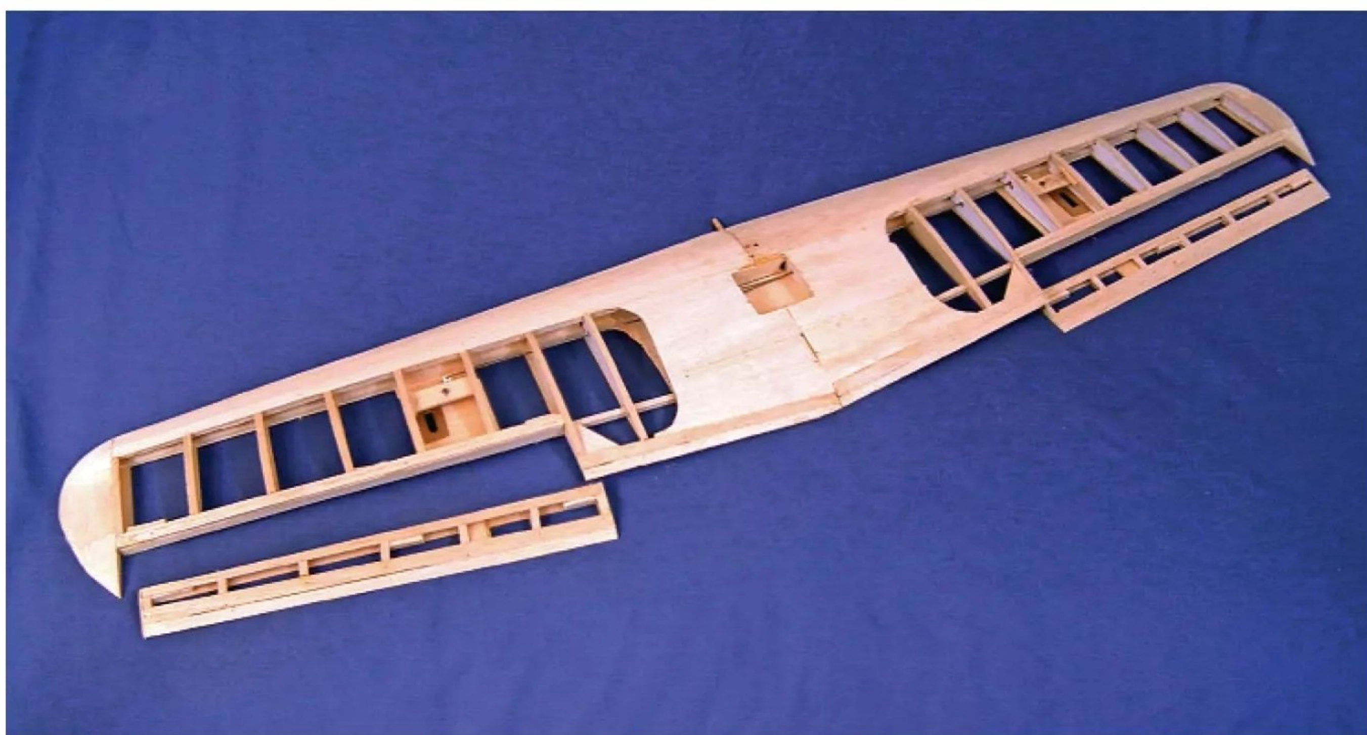
A complete sheeted wing. Again, compare it with your own plan. Note the built-up ailerons in this example.
