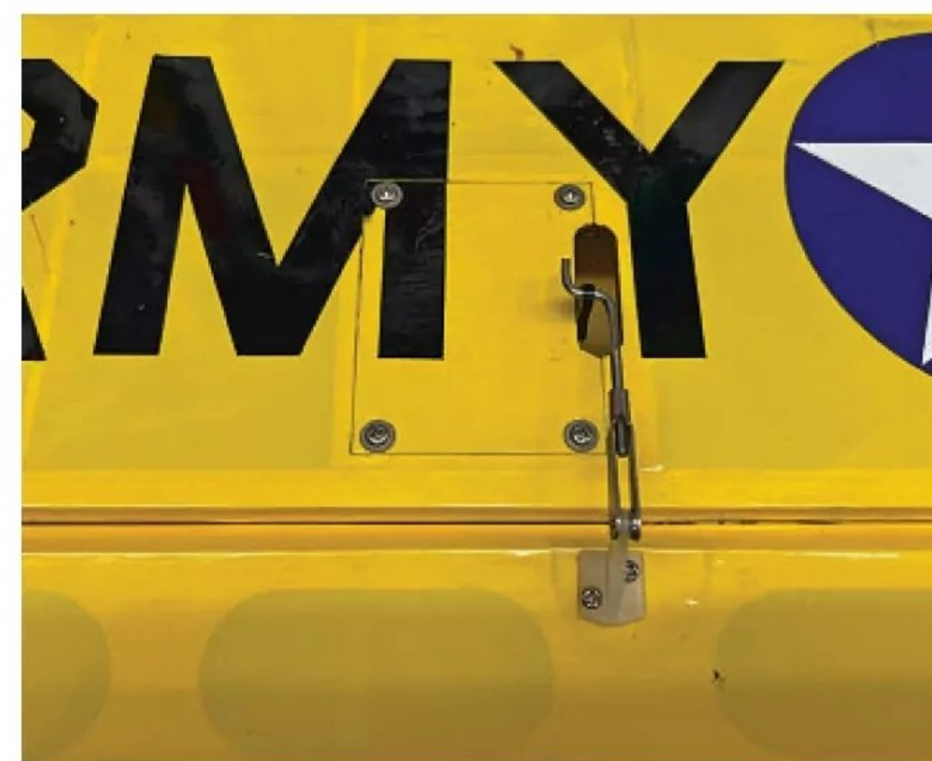
Traditional servo cover using plywood and screws.
