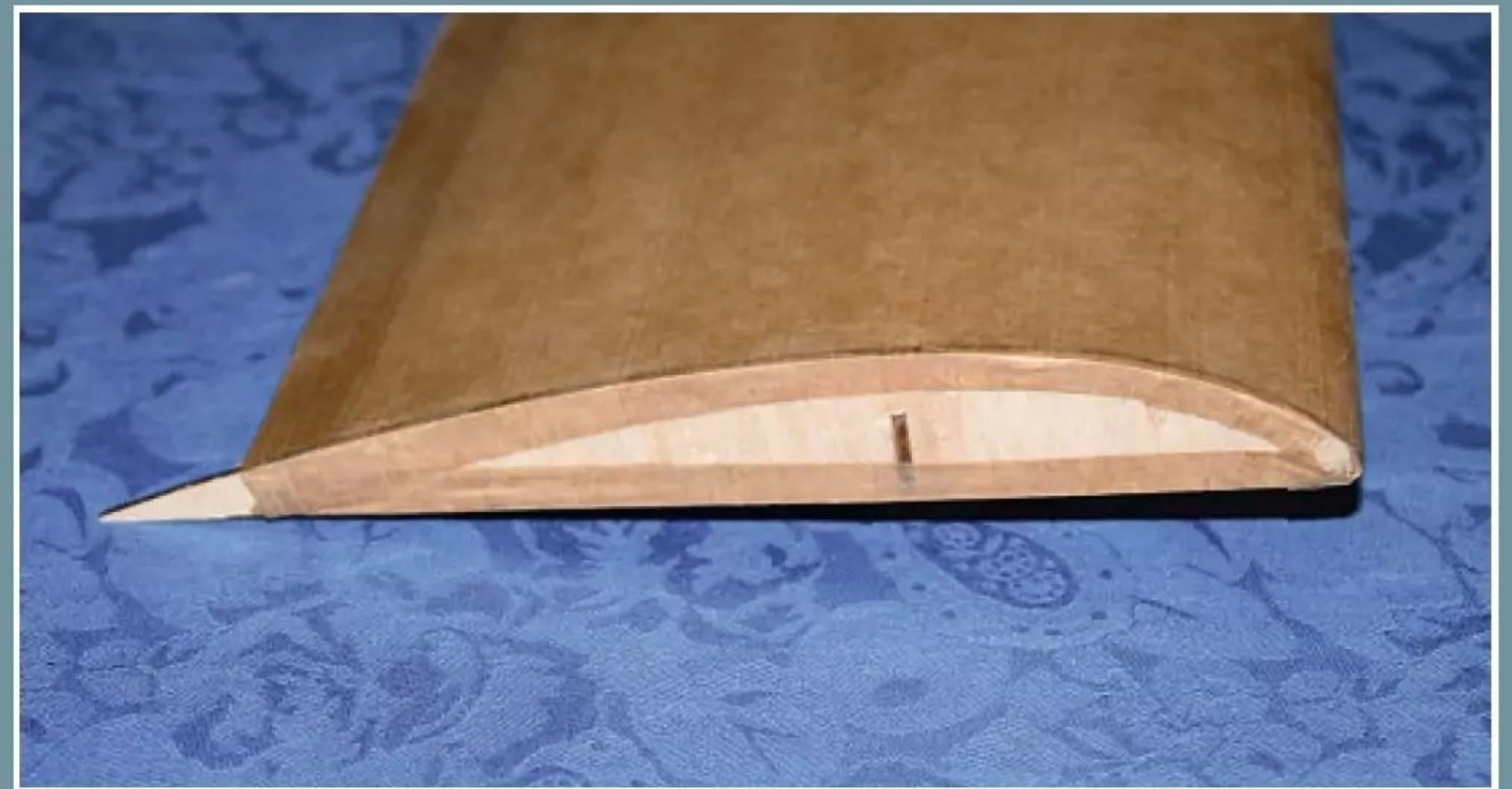
Tip rib added, showing how the brown paper covering wraps over the ends.
