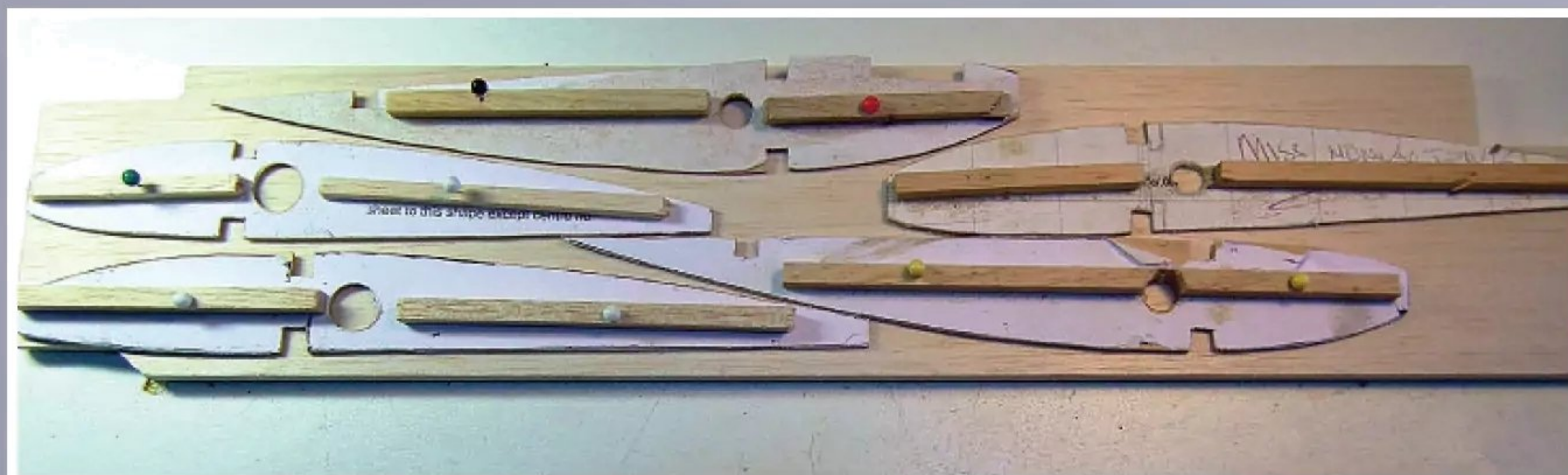
If you can interweave the ribs, you can get more out of each sheet.
