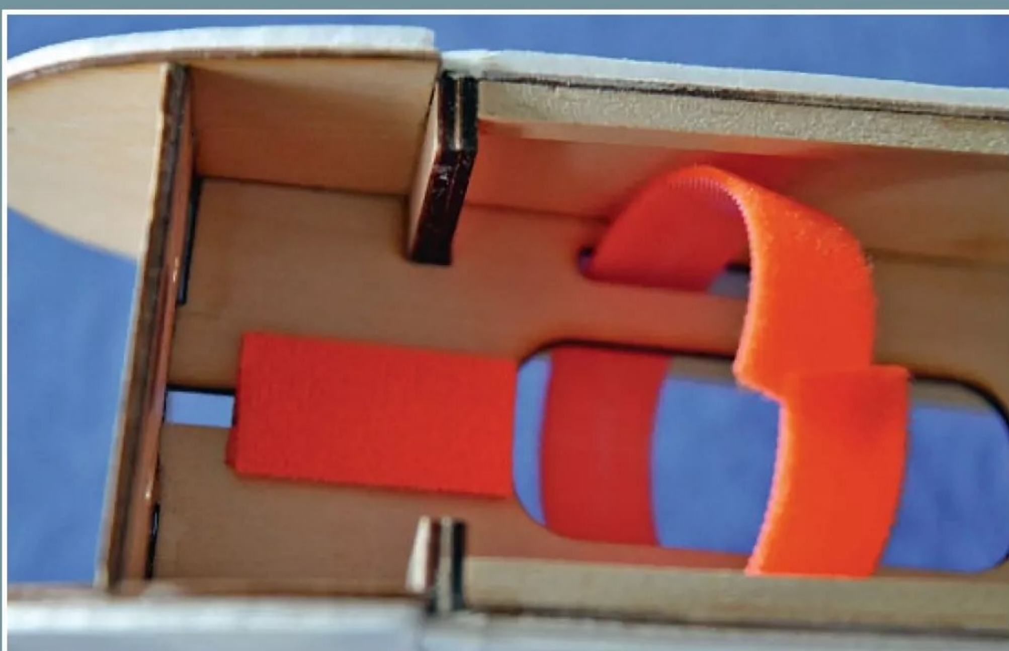
Ensure your LiPo is well retained by using a hook & loop strap and additional pieces glued to the battery bay floor.
