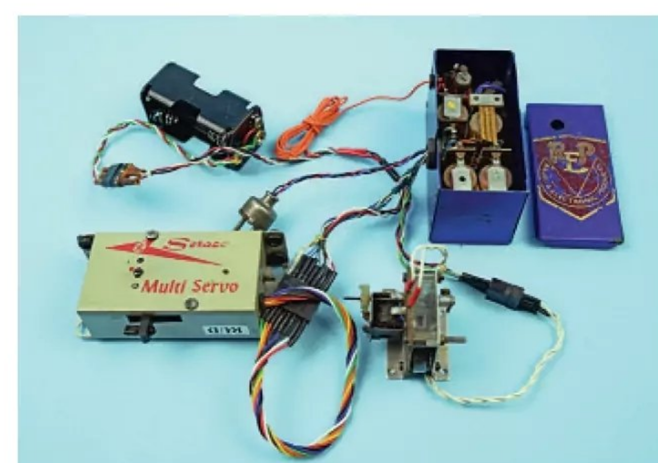
REP 3 channel receiver. Rudder control is via a Soraco servo, (basically a re-badged Bonner) and, for throttle, a Fred Rising sequential clockwork actuator.
