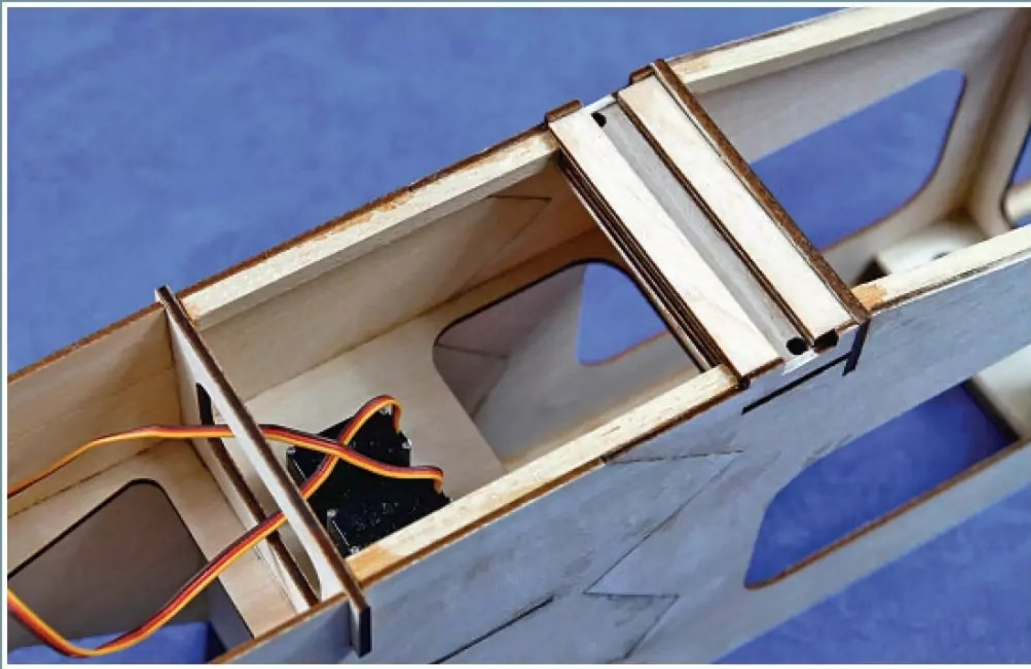
Main undercarriage mounting block detail.
