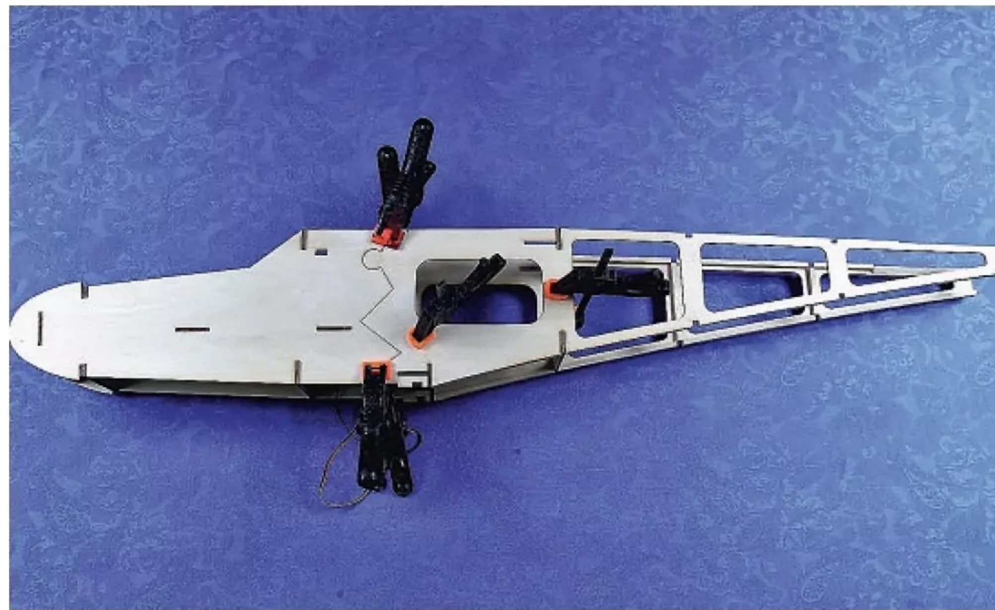
Clamp the fuselage assembly together while the glue sets.
