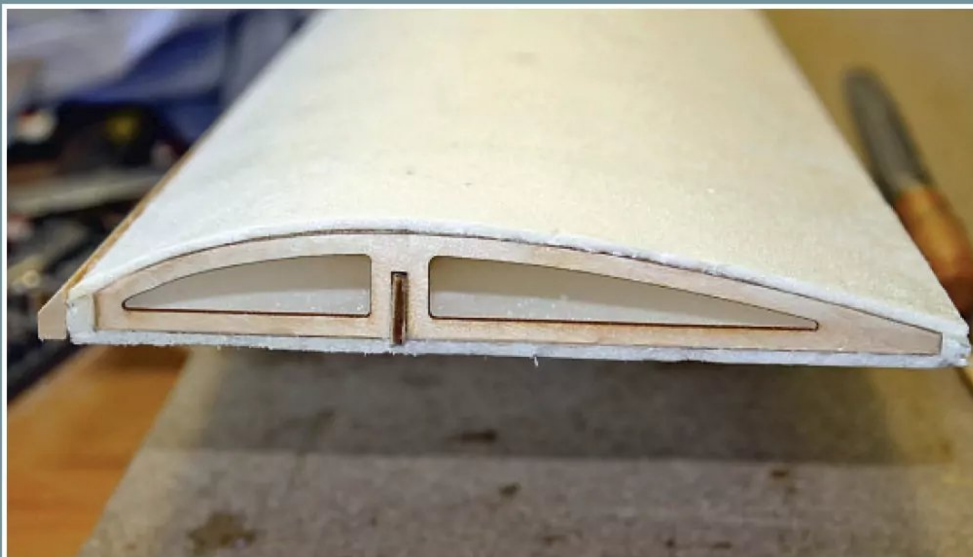
End view showing the wing construction around each rib. Leading edge is ready for shaping.
