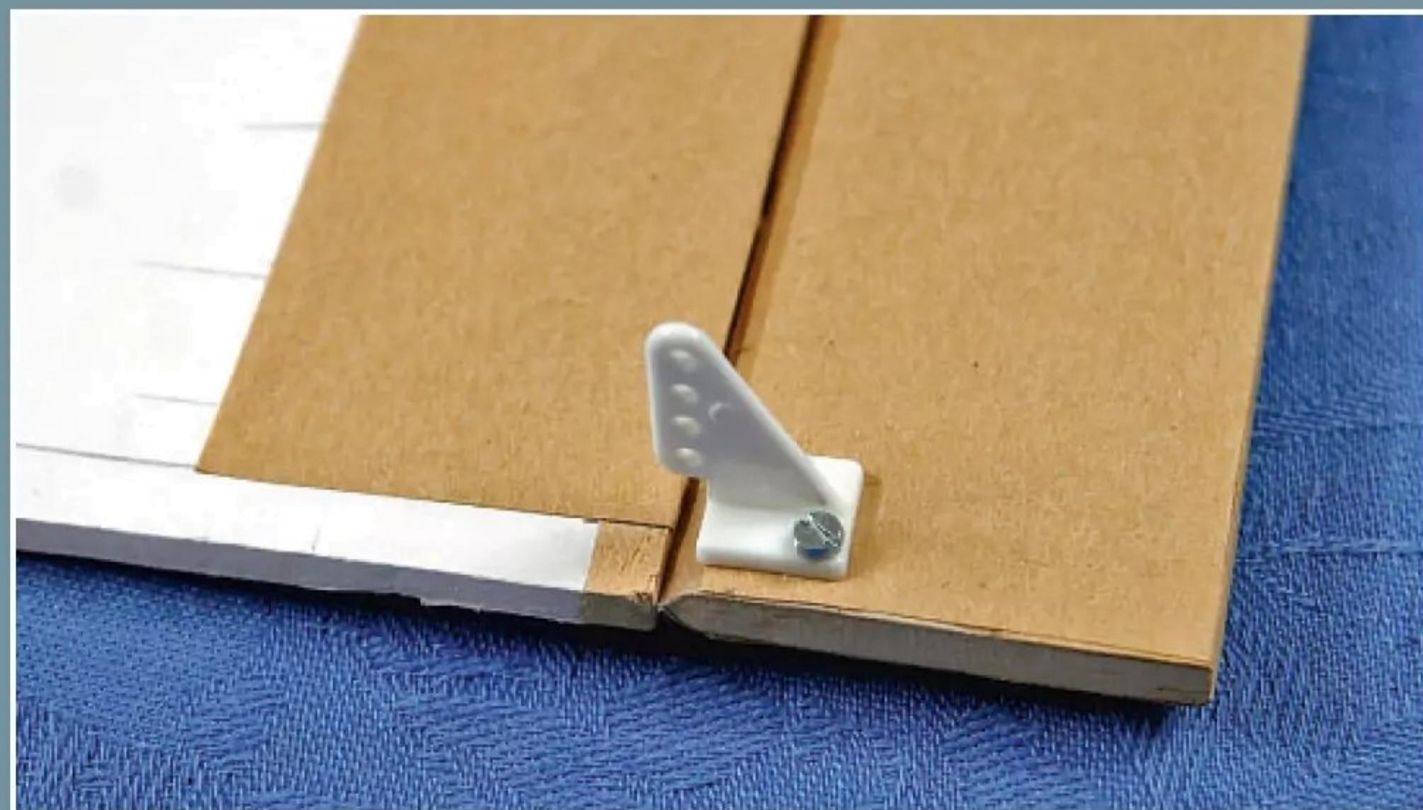
Both the elevator and rudder are bevelled ready for hinging. Standard nylon controls horns provide easy hook ups to the tail servos.
