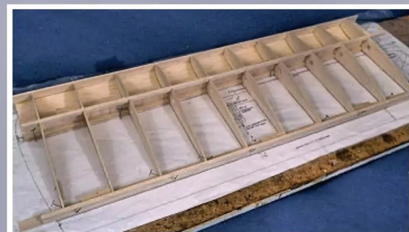
A basic wing. Note the spars, leading edge and trailing edge. Compare it with your own plan.
