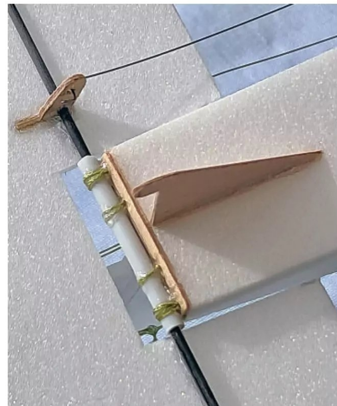
The simple tube and pivot spar assembly is light and works very well. I've used it on several other models.
