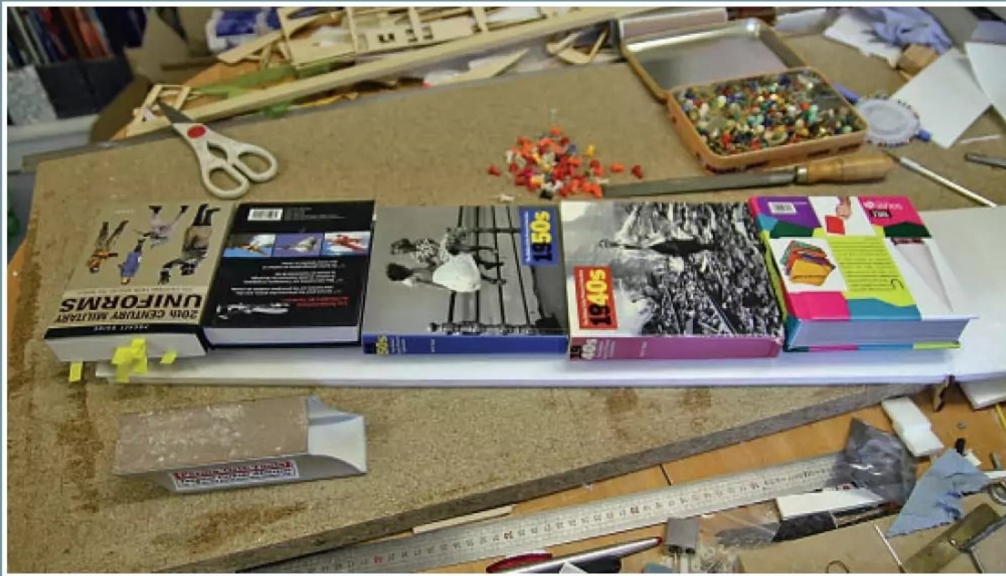
After attaching the top wing sheets weigh each of the panels down in turn to keep them warp free whilst the glue fully sets.
