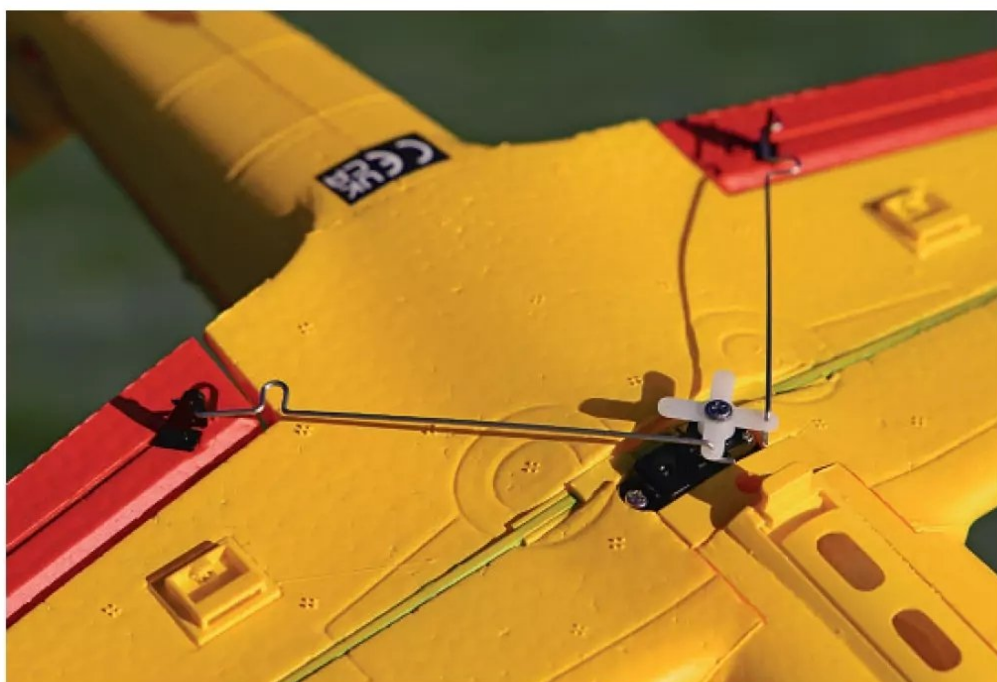
I wondered whether the exposed aileron servo would suffer when landing but that hasn't been the case.
