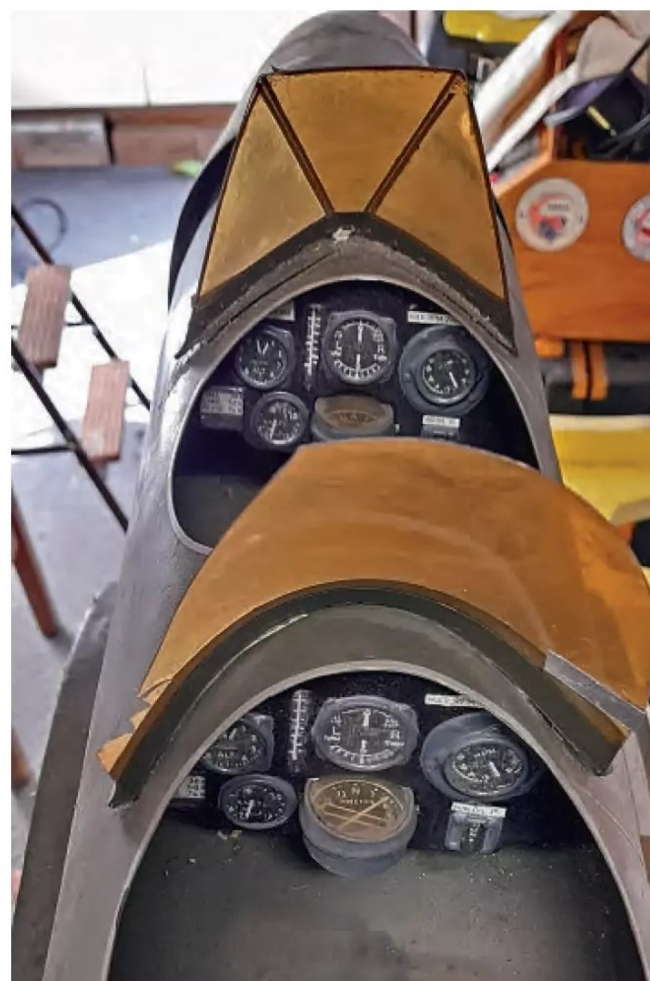
Cockpit instruments were found to be Tiger Moth panels.
