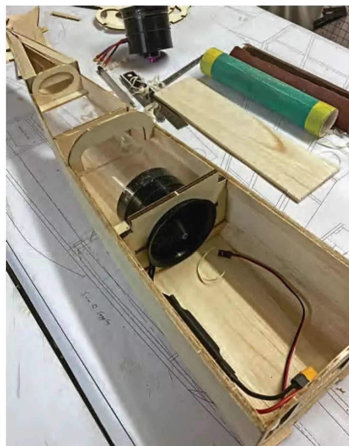
Installing the thrust tube.
