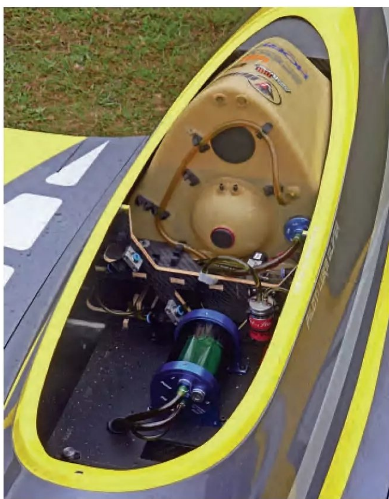
A look under the canopy of Luke Oliver's Tomahawk Integral showing the large three chamber fuel tank and the other on-board paraphernalia that jet turbines need.
