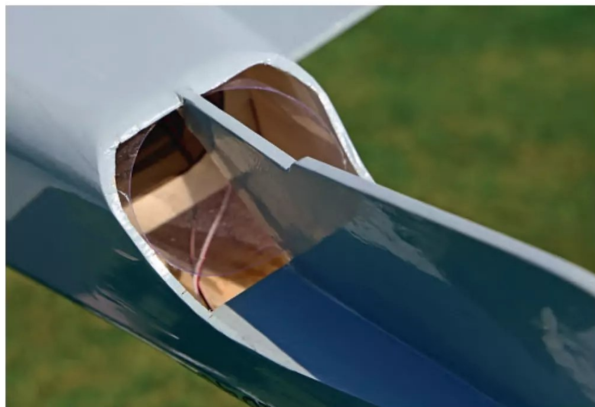
Rear end view showing the end of the thrust tube.
