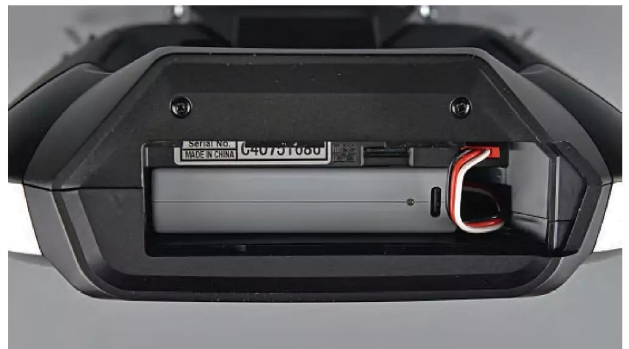
Battery compartment is at the bottom of the case. Next to the label is the microSD card slot.
