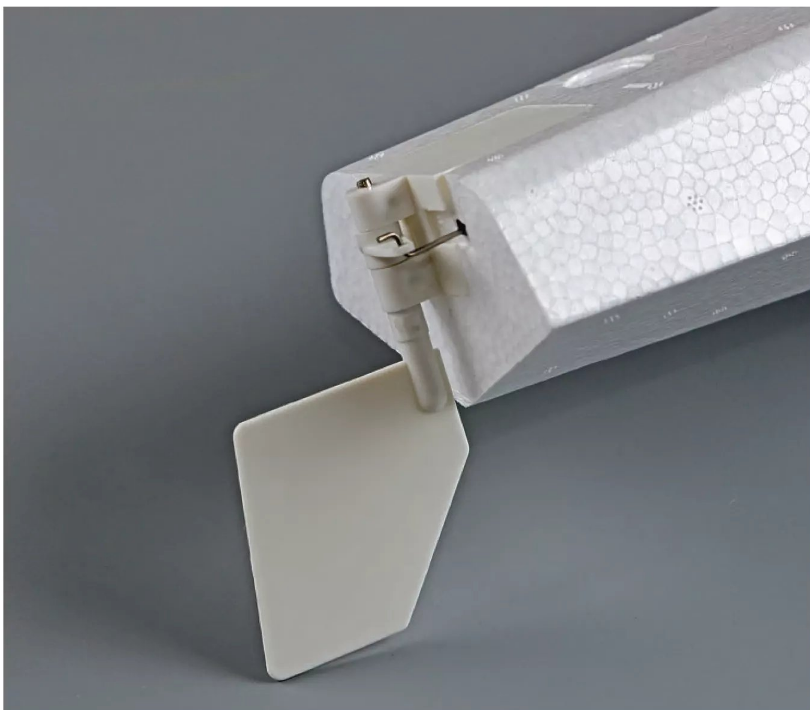
Port float features a large water rudder attached to an integral servo.
