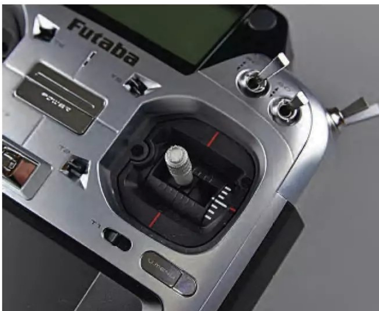
Smooth operation of the main sticks is helped by the use of hall effect non-contact potentiometers.
