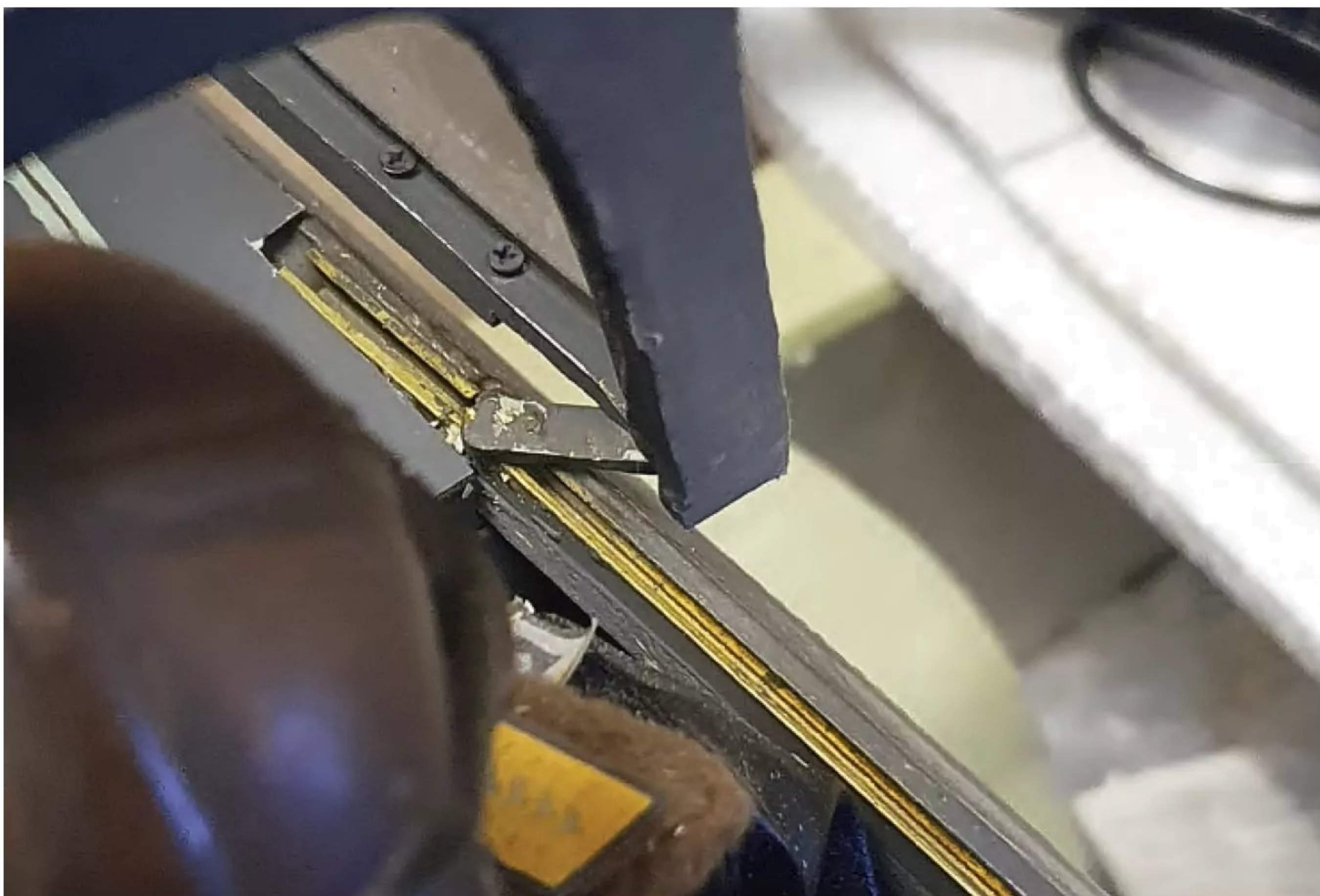
Close up on a canopy slider with its pivoting guide.
