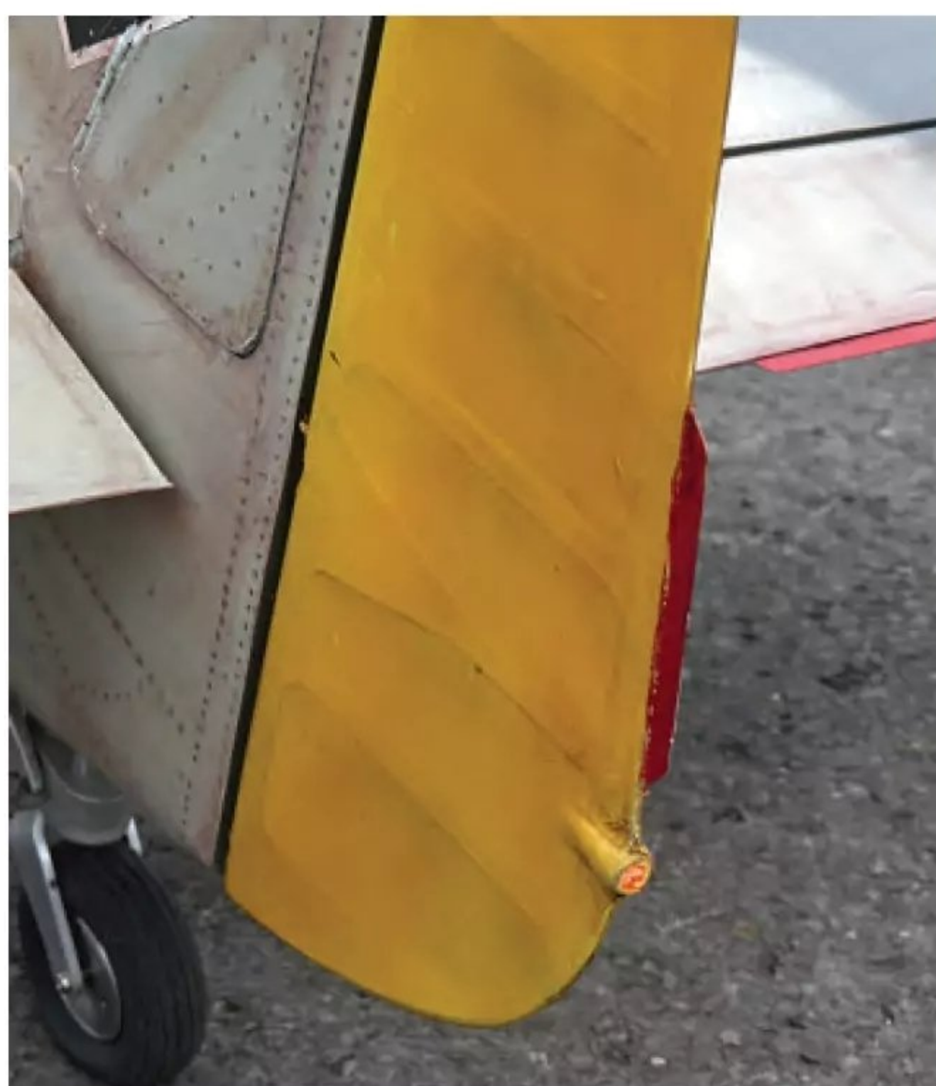
Rudder incorporates a working navigation light.
