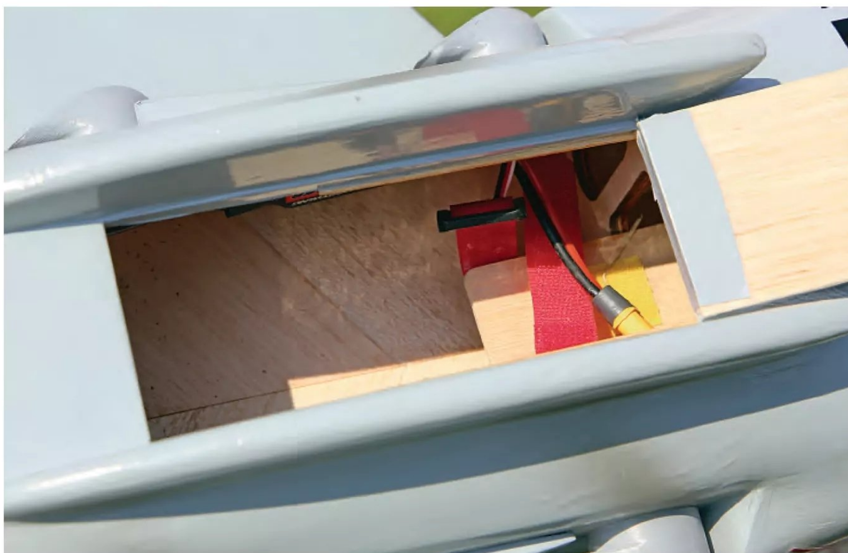
A peek inside the battery bay.
