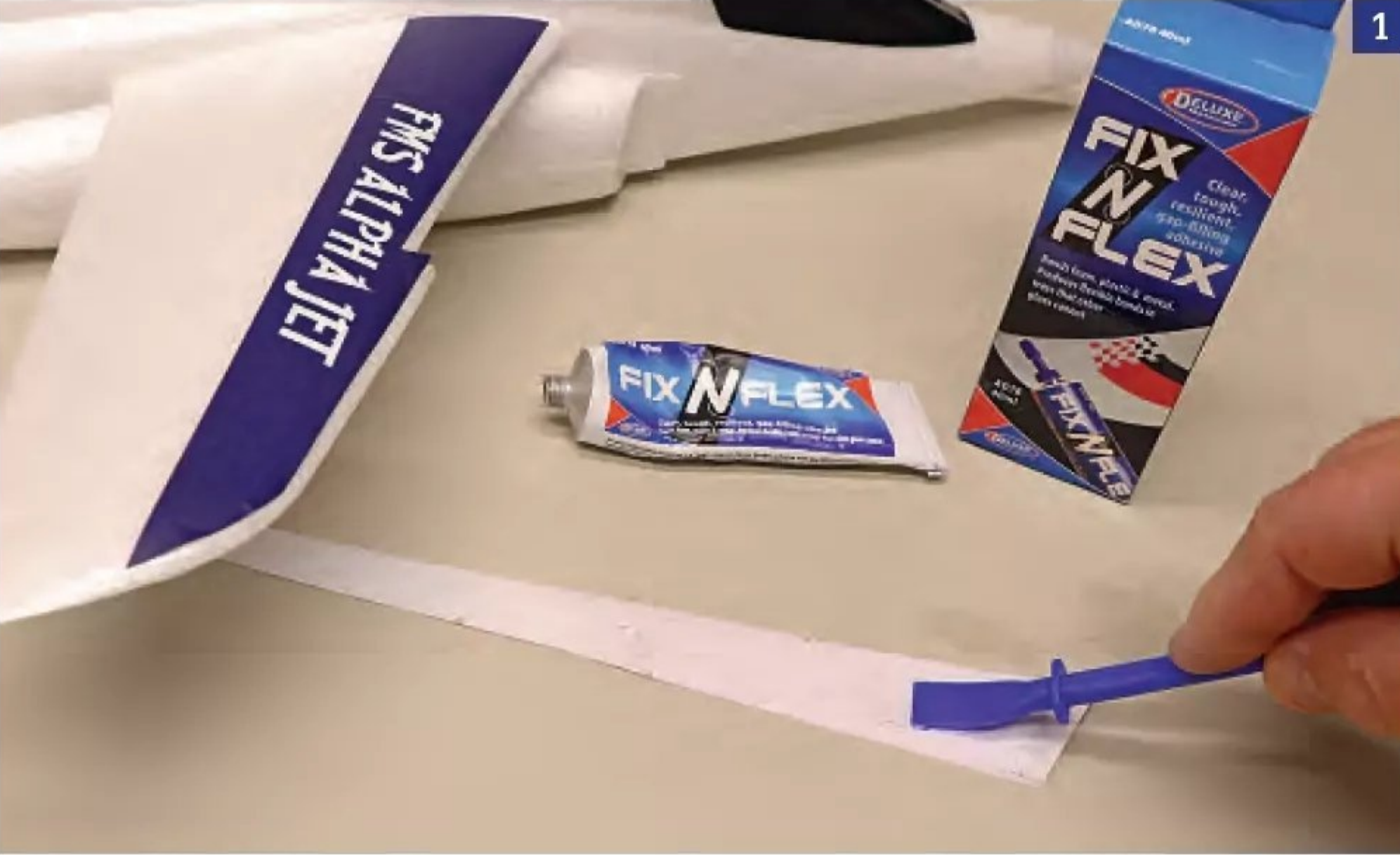
Remove the decal and spread FIX 'N' FLEX on the underside using a spatula.
