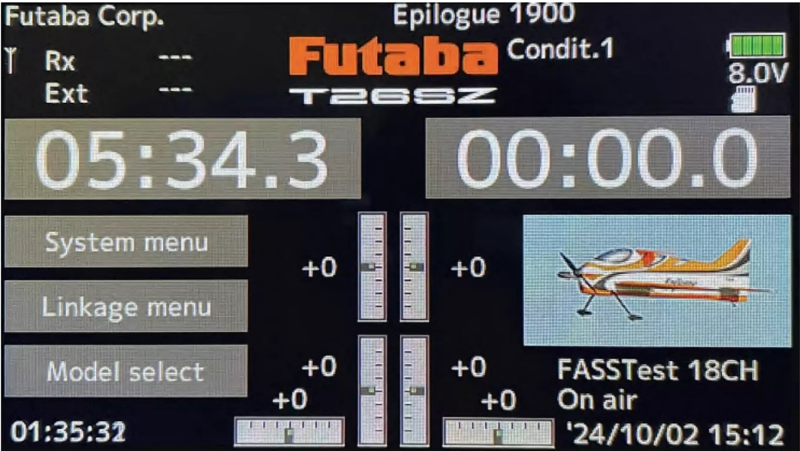
Home screen shows a wealth of information, plus a neat little image of your model using a bitmap file stored on a microSD card.
