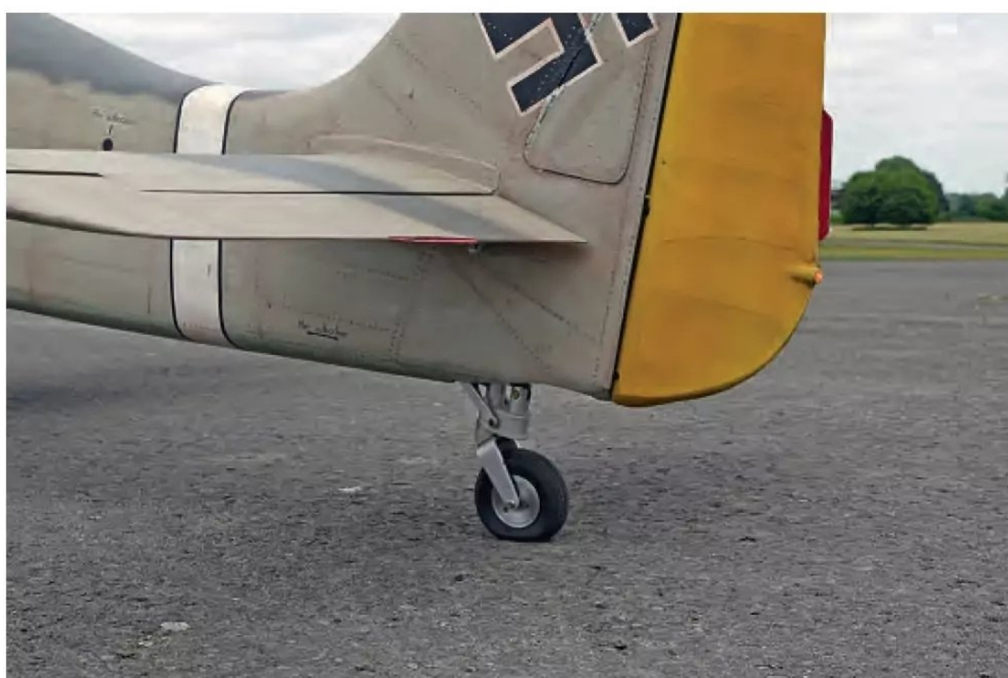
As with the main retracts the retractable tailwheel is from Giant Sierra in the USA.
