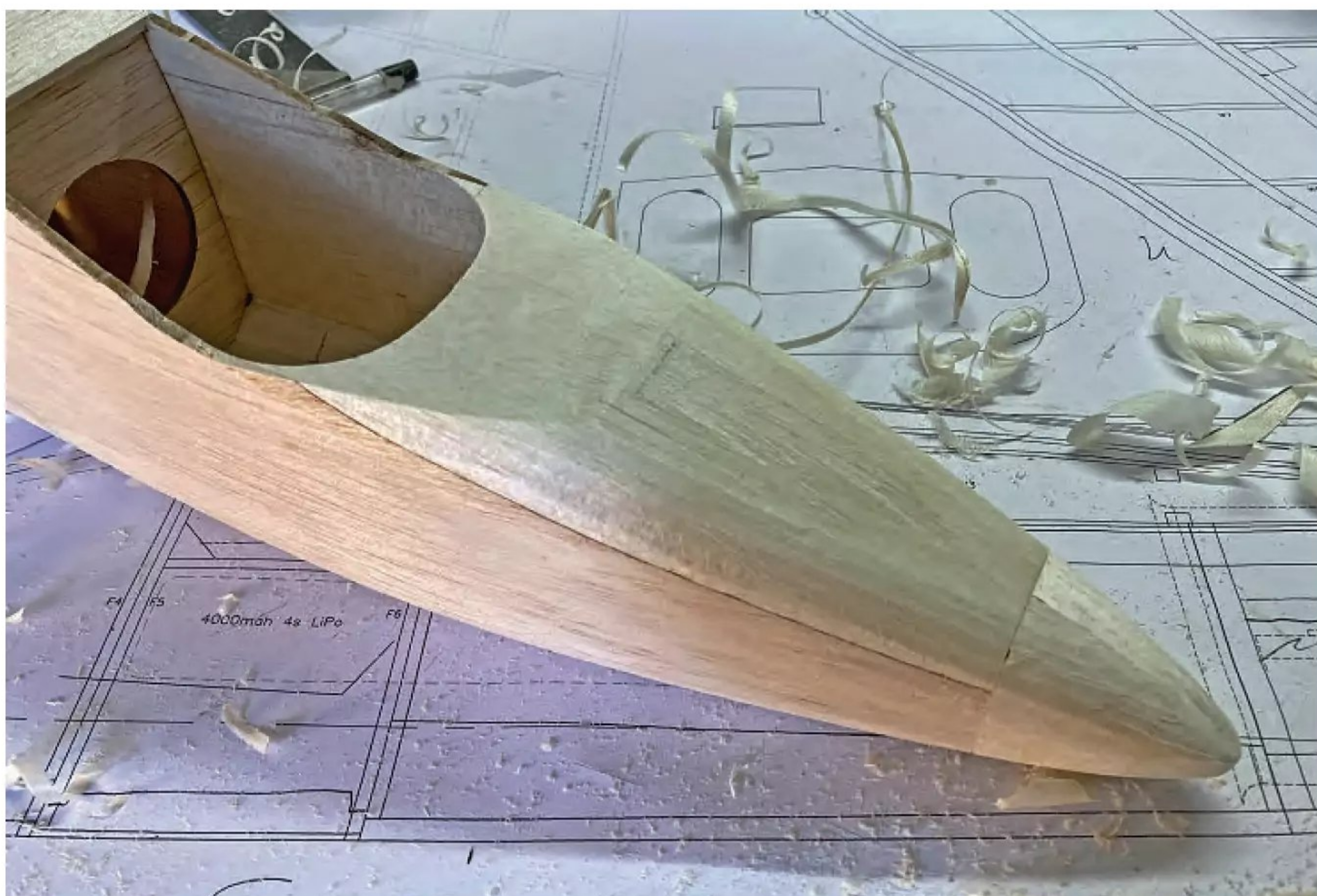
Use a razor plane and sanding block to profile the front fuselage to its finished shape.
