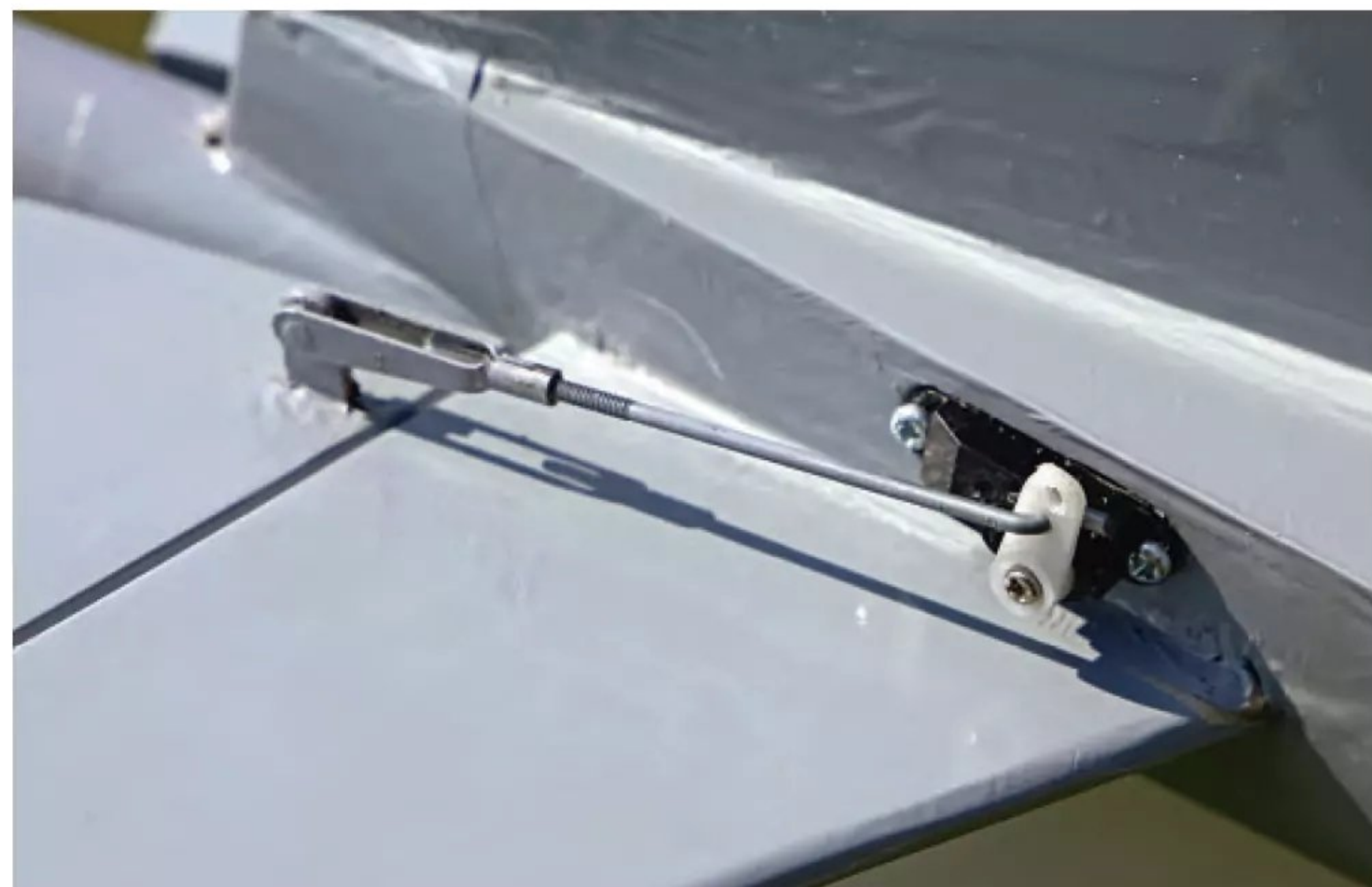
Elevator linkage connected to one of the control horns made from 2 mm birch ply.
