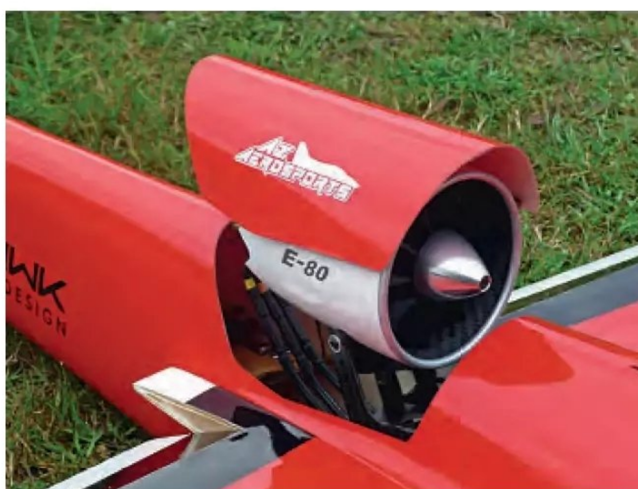
Close up of the Swift's 80 mm retractable EDF unit which produces a phenomenal 4.5 kg thrust from a 12S LiPo pack. It sounded just like a turbine on full chat.
