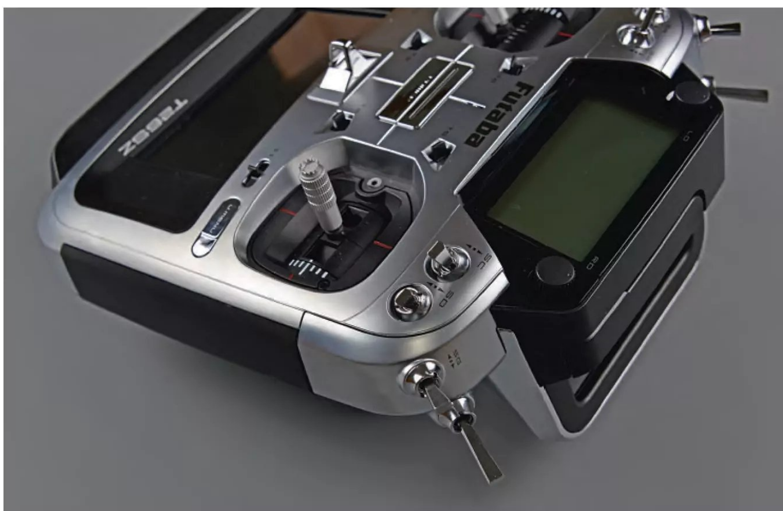
Shoulder switches can be swapped around or replaced with alternative types to suit personal preference.
