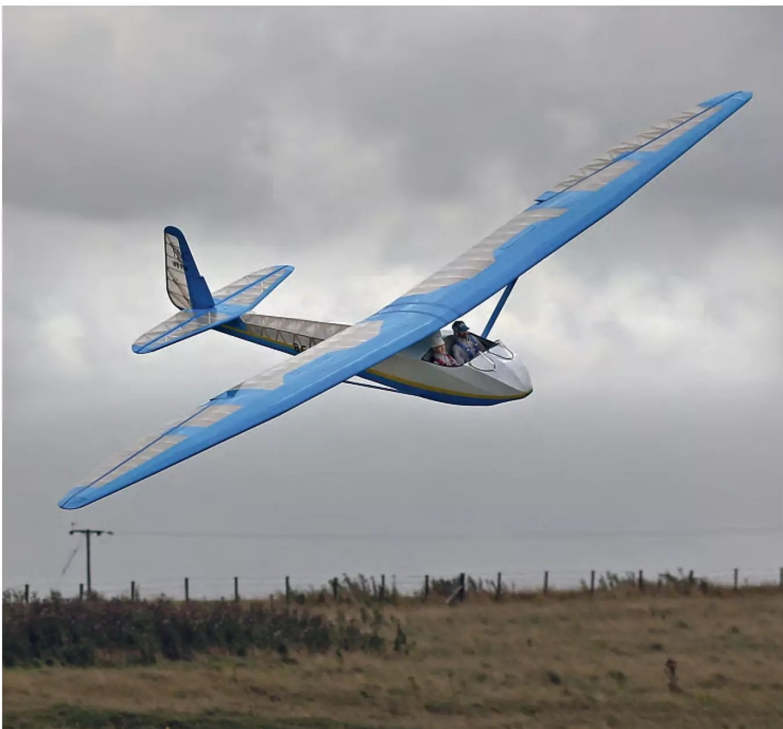
At 1/4 scale the Barge spans 4.1 metres and weighs in at around 12 lbs.
