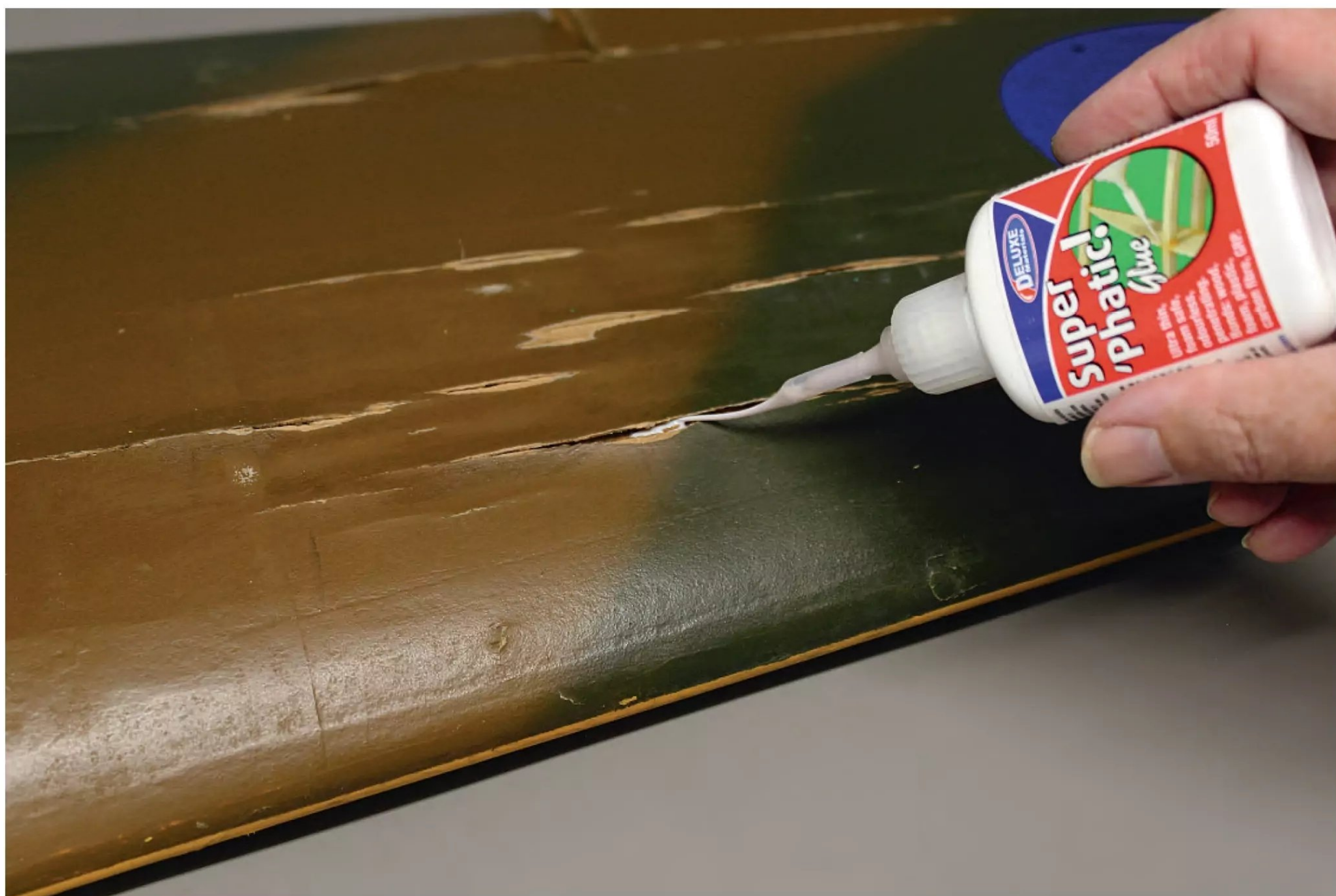
Super 'Phatic! glue was carefully applied directly into each split.
