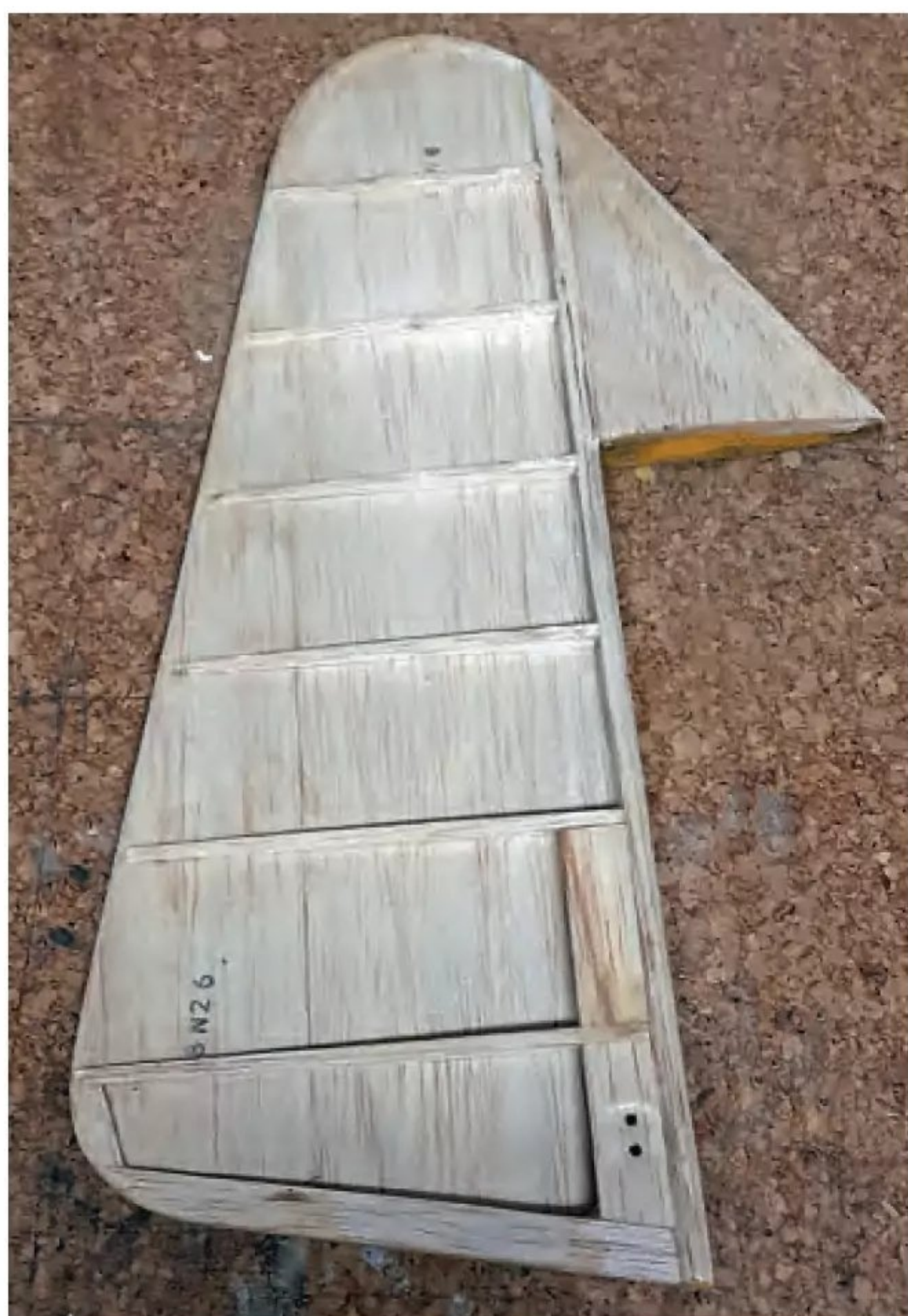
The rudder was controlled by a closed loop in a scale like manner and is seen here stripped back and ready to recover.
