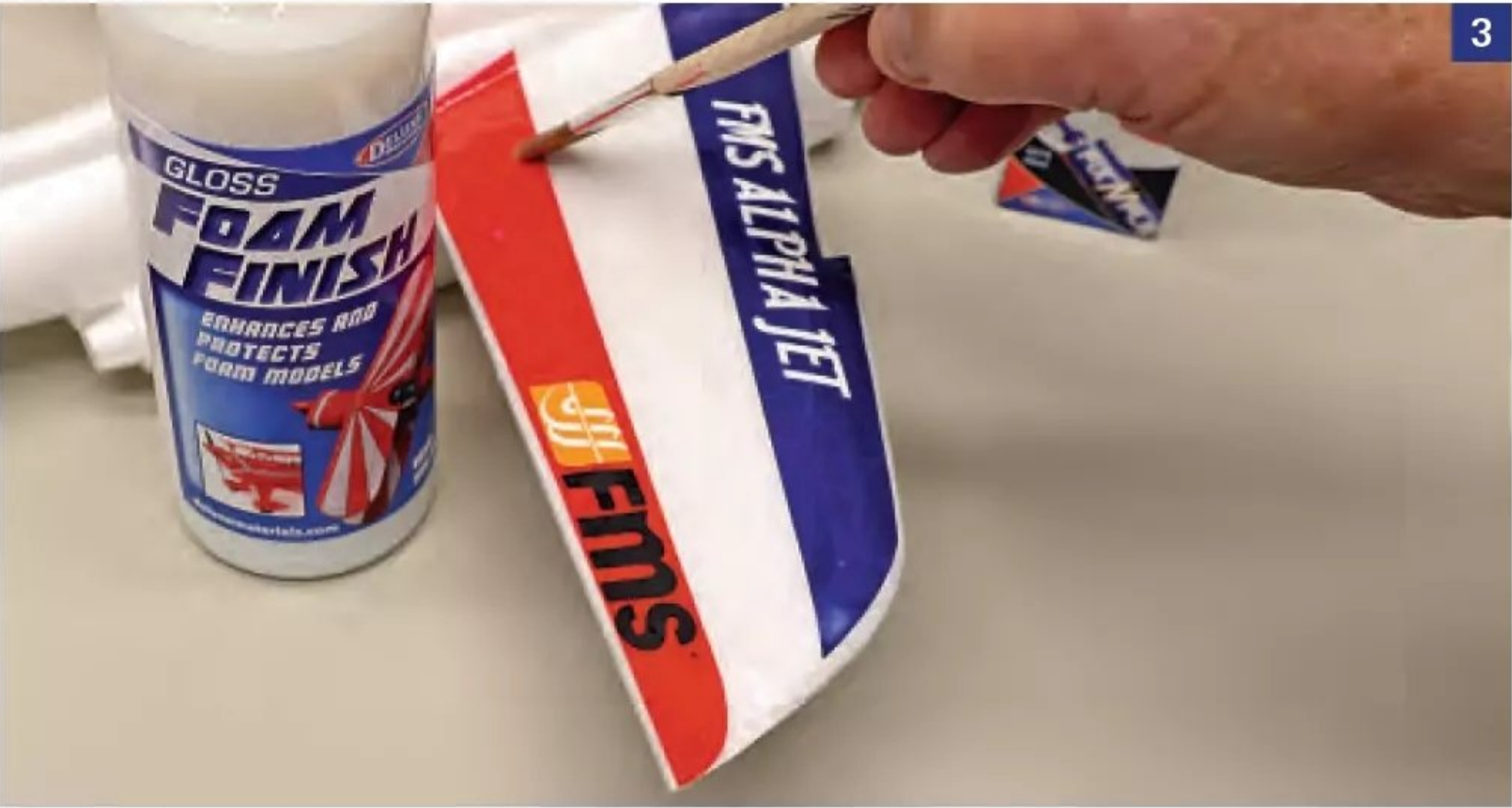
Allow to dry and then use FOAM FINISH GLOSS or MATTE on top to seal the edges. Allow to dry. Job done, go fly!
