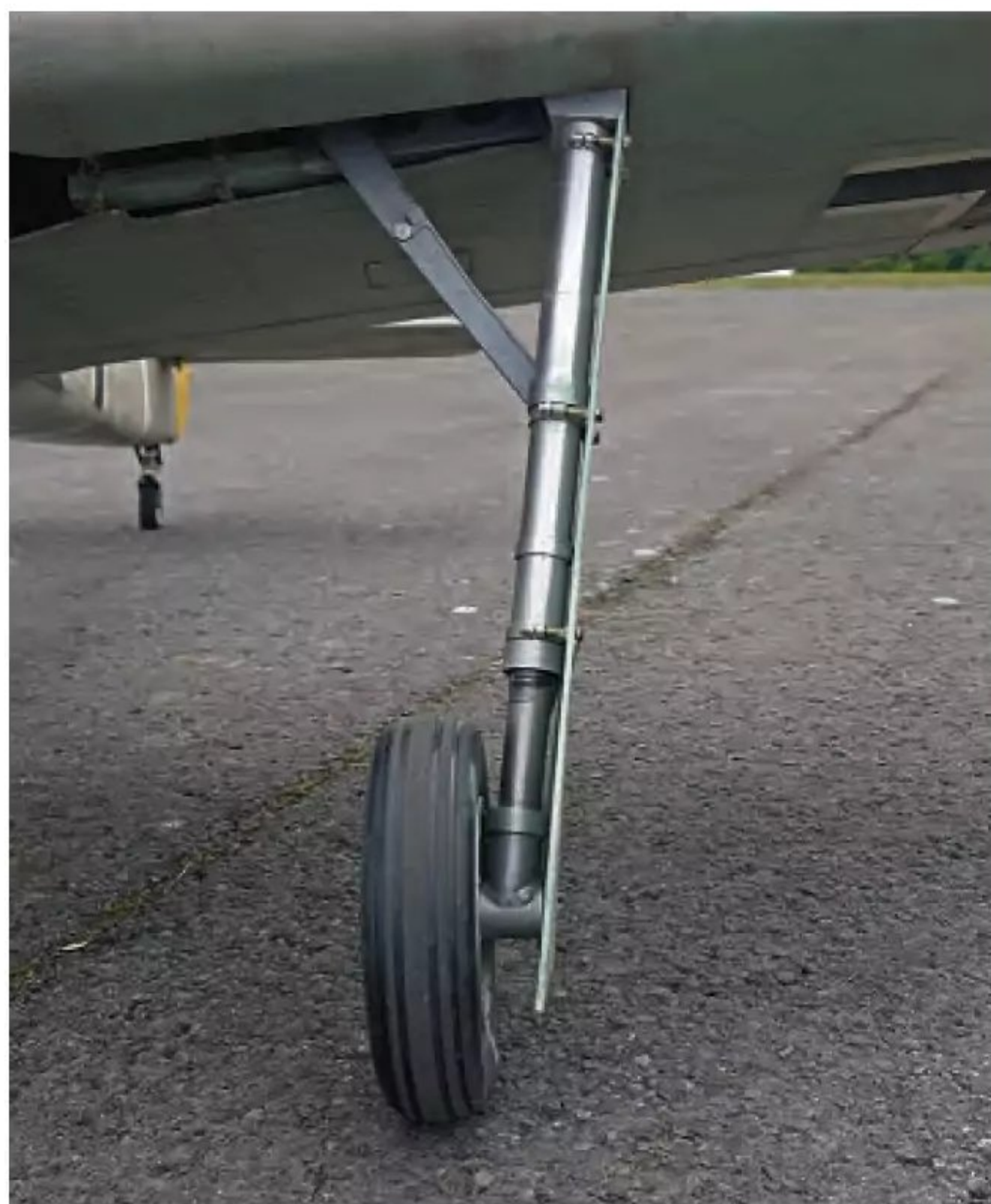
Scale sprung retracts are robust enough for the 30 kg model.
