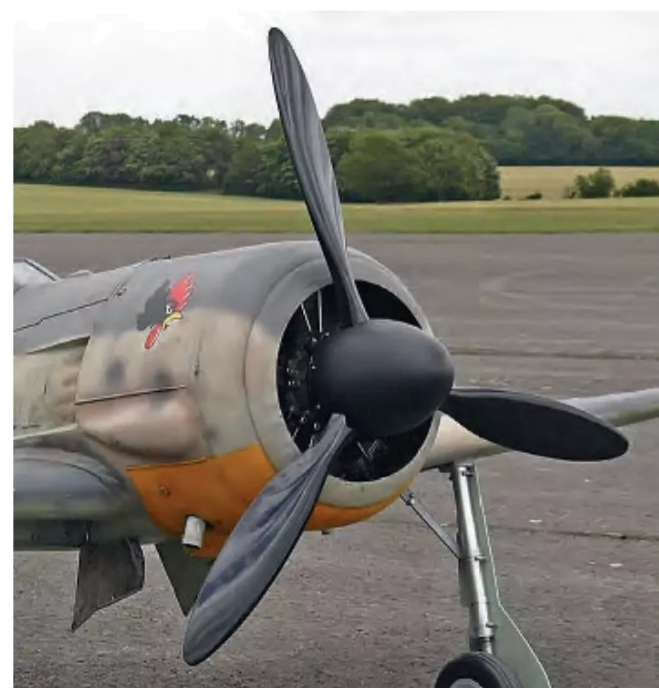
The Moki is tightly cowled and baffled to ensure that cooling air flows over the cylinders.
