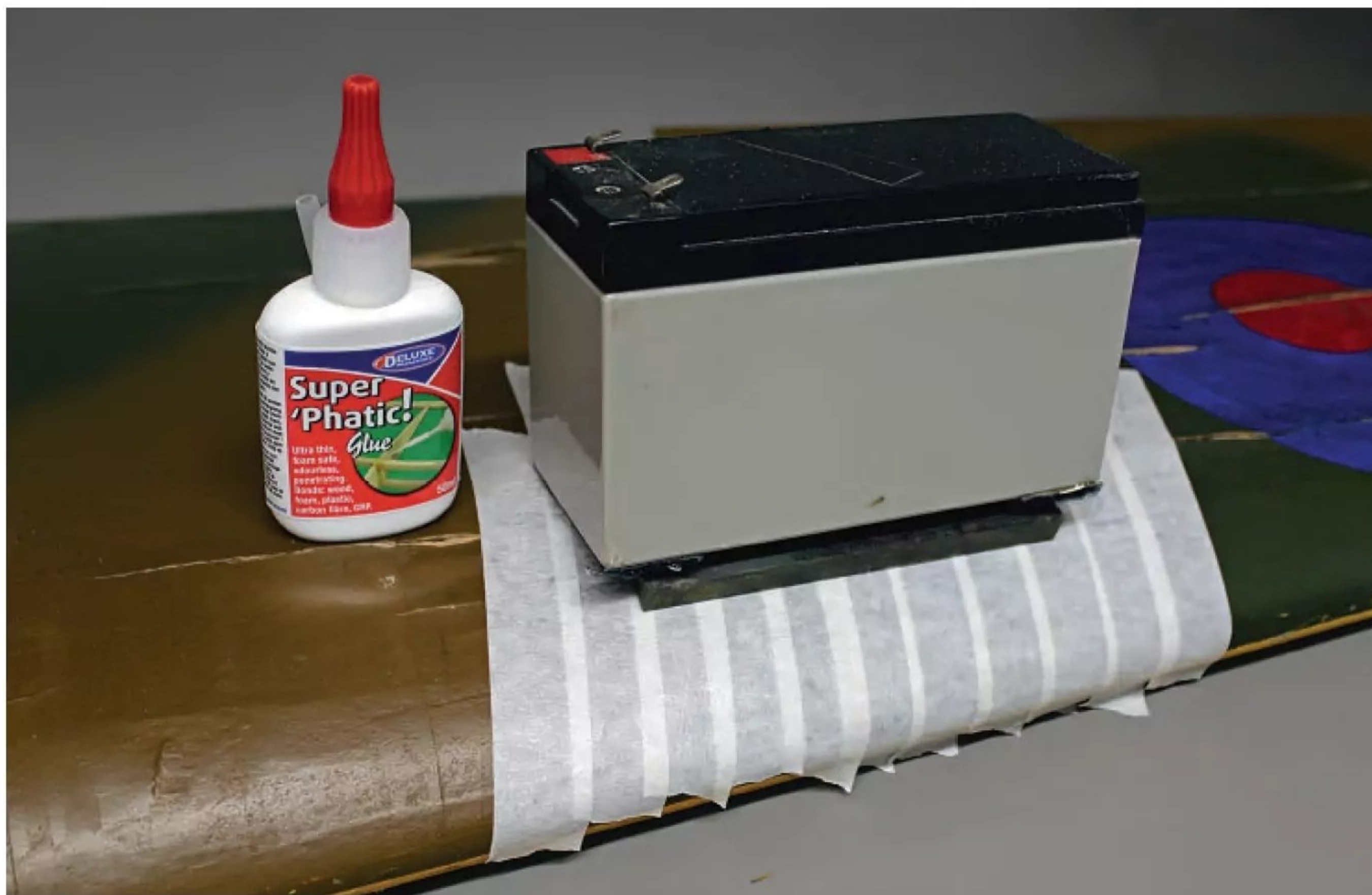
Each repaired area was taped up and left to dry out overnight with a hefty weight on top!
