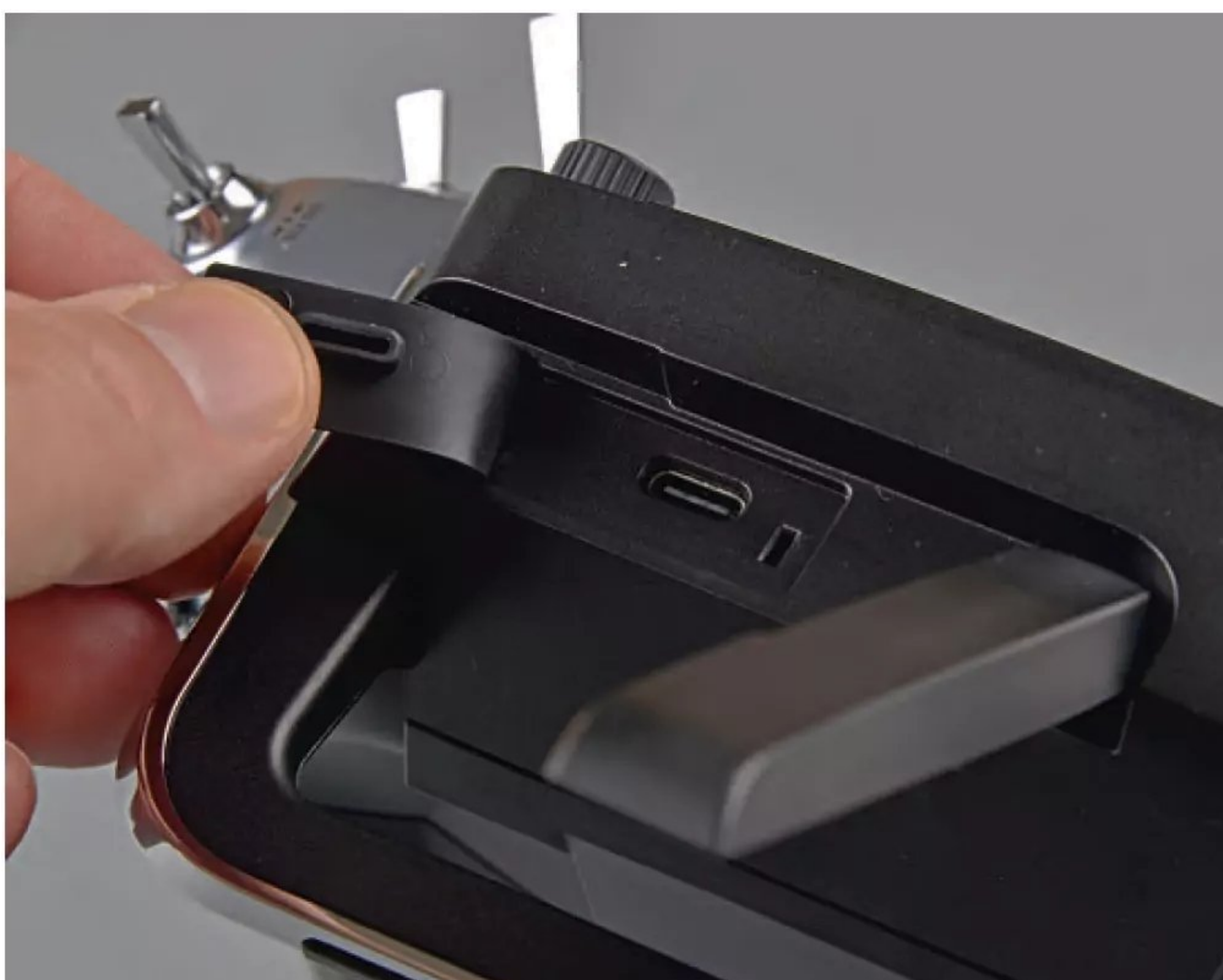
Underneath the antenna you will find the USB-C charging port. Best not pull it back this far though!
