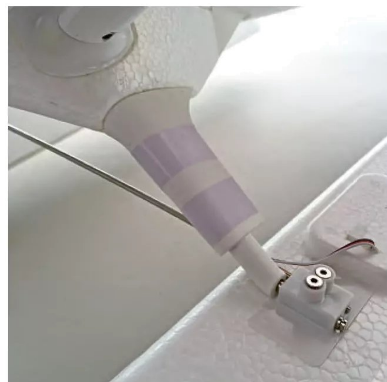
Additional leg fairings are not supplied which is a shame as the float set looks too spindly without them. But you can pop the fairings off the main wheel set and tape them in place.
