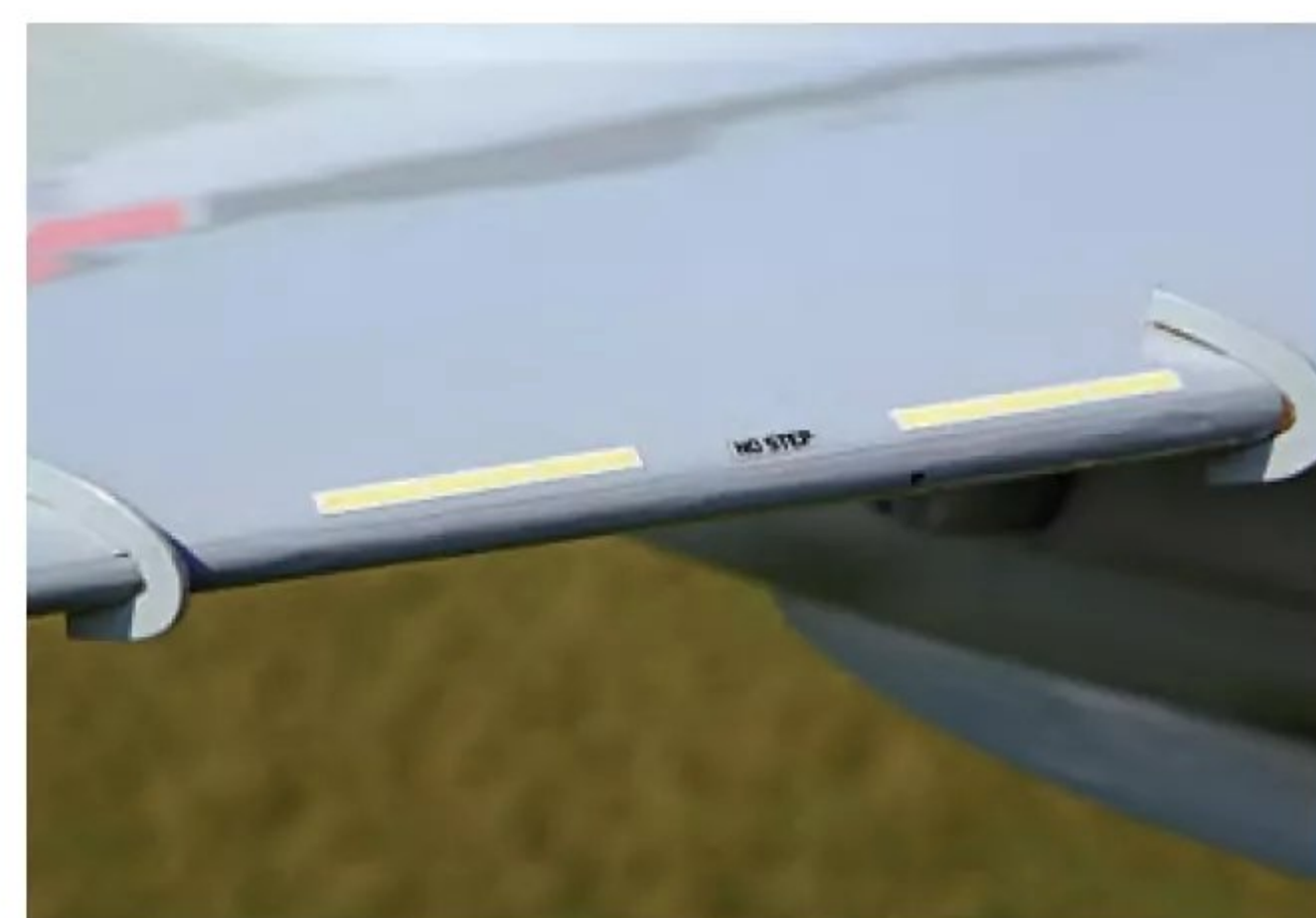
The wing fences and straight leading edges are key to making this model Harrier fly so well.
