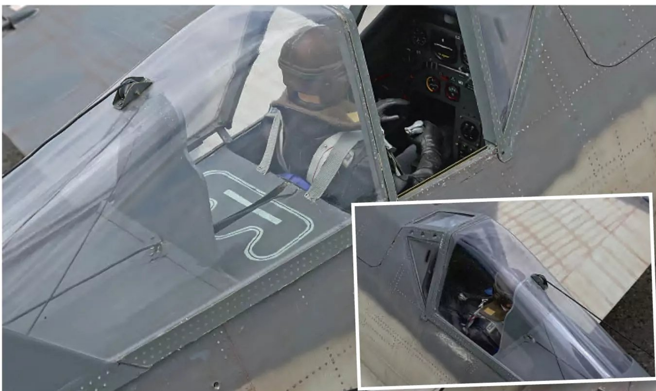
Open and shut case! A powered sliding canopy really adds to the scale effect. Note the antenna pulley system.
