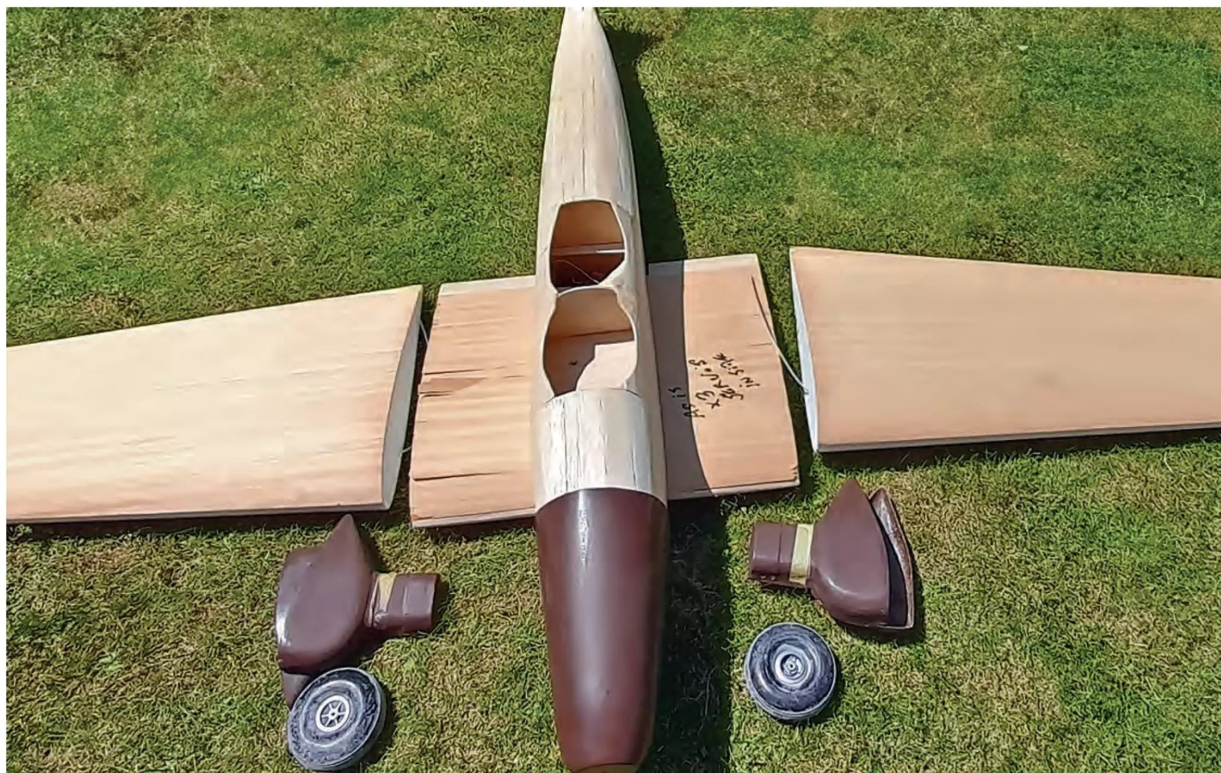
Model number two offered several unused parts but the wing centre section was badly split.
