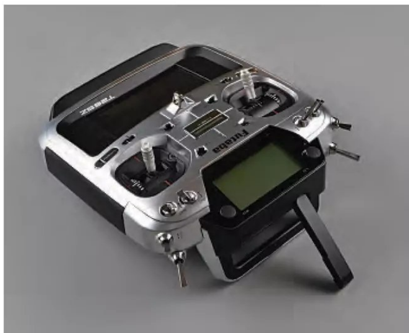
Antenna must be swung out and swivelled downwards before use to maximise signal strength.
