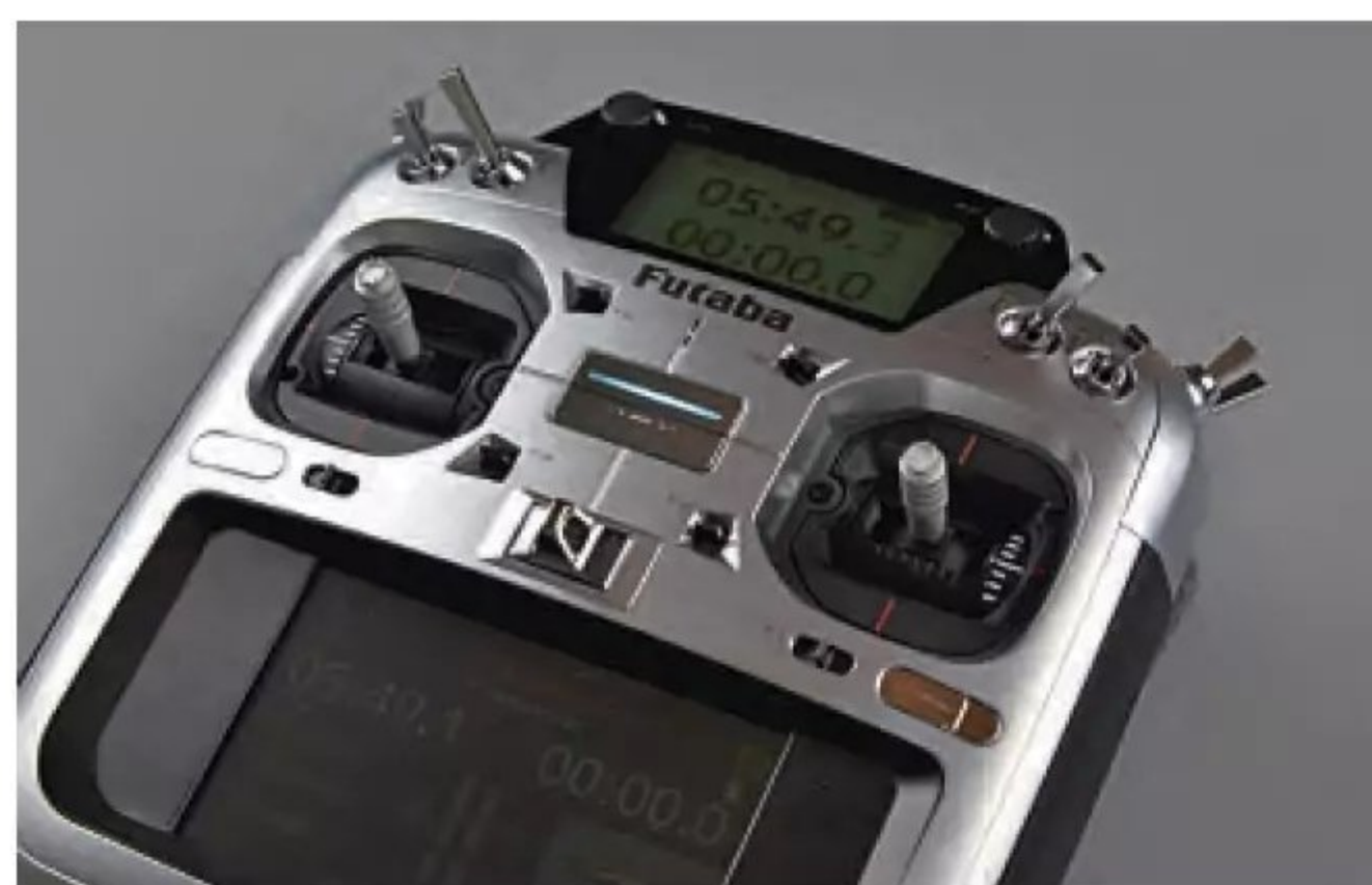
A last look at the Futaba T26SZ showing the switch lit up blue. This gives a clear indication that RF is switched on. If it's pink, then RF is off.
