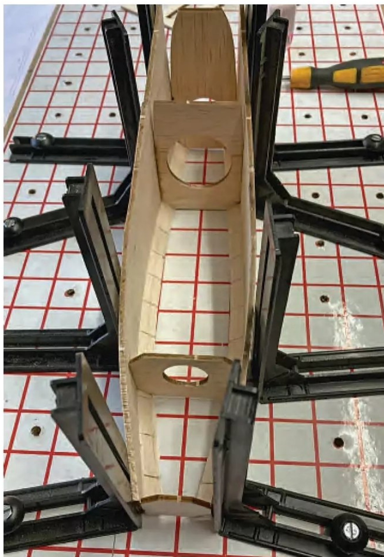
Building jig back in action, this time being used to assemble the front fuselage.
