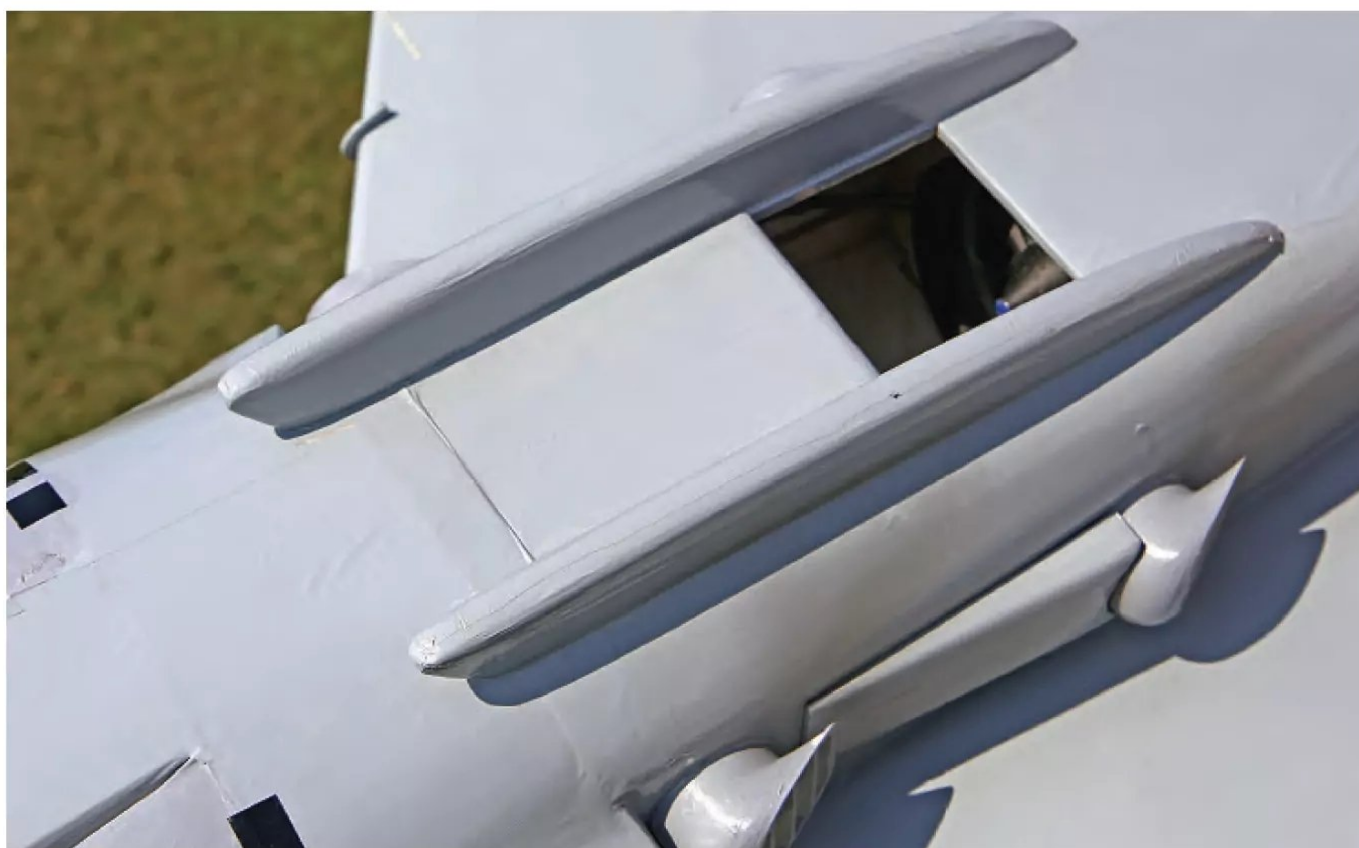
Two dummy rocket launching pods on either side of the battery hatch give a good grip when hand launching.
