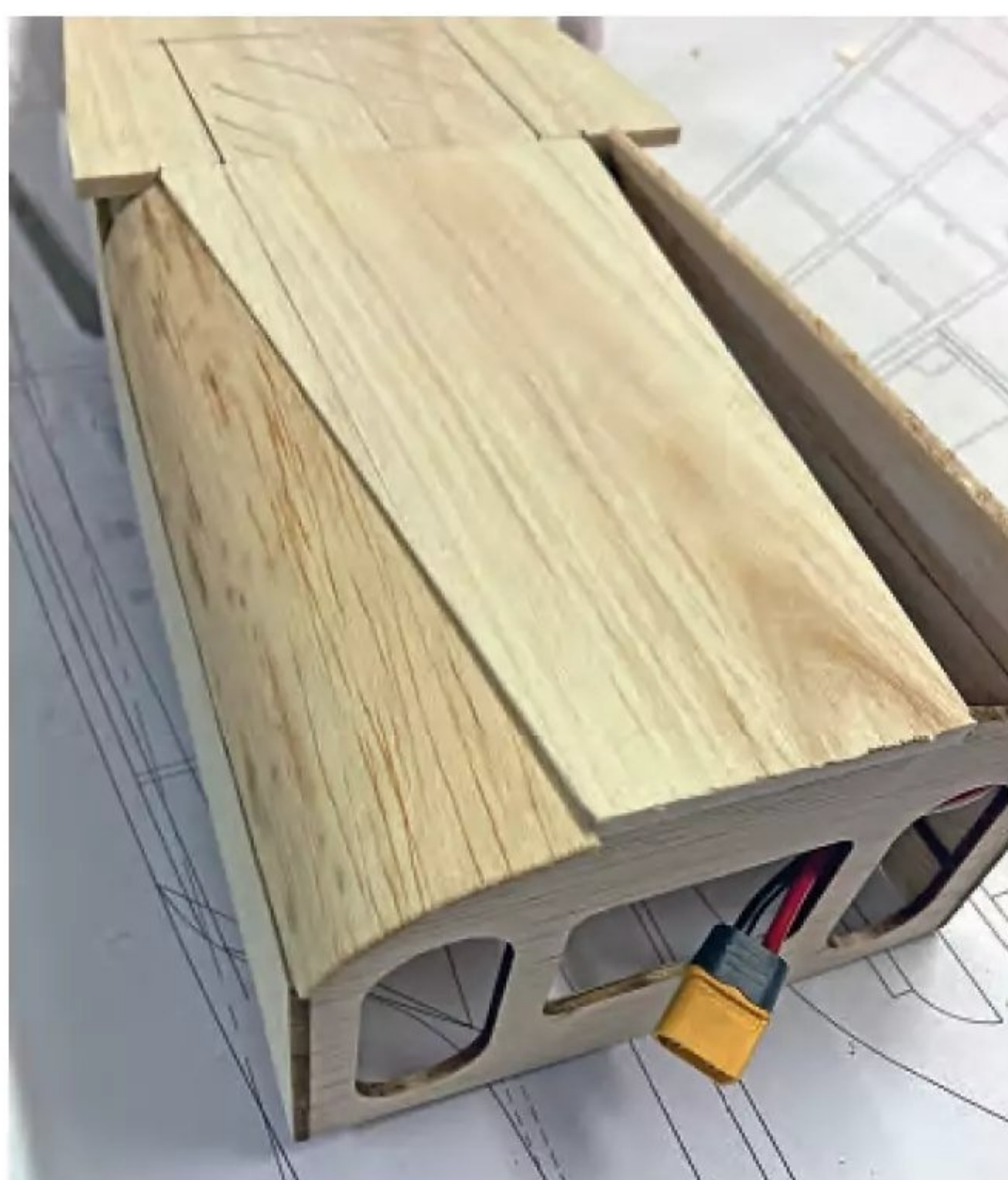
When making the rolled bottom fuselage sides you may need to wet the wood's surface to assist bending it around the corner of F9.
