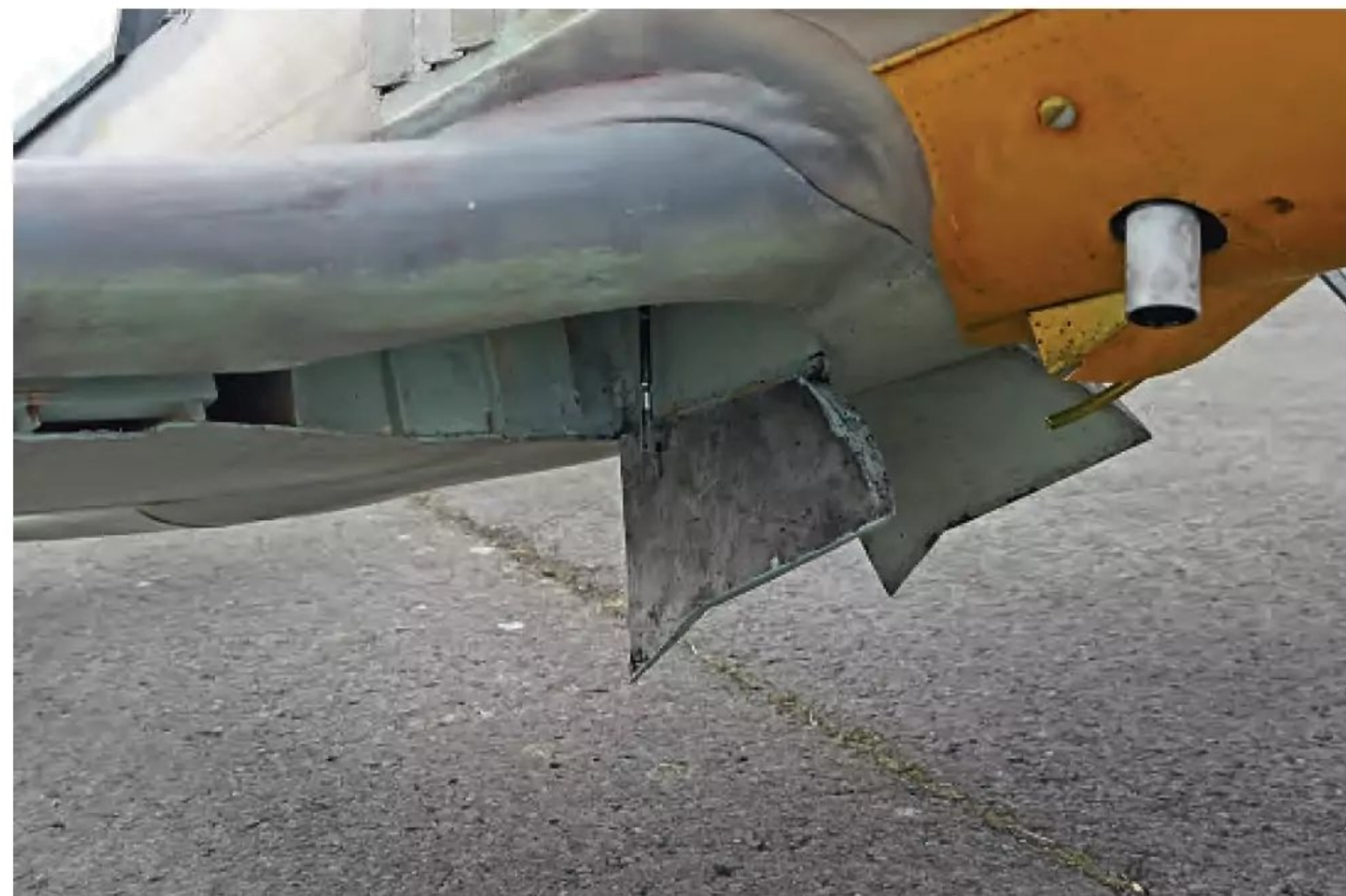
Inner wheel doors operate using separate servos and are sequenced to the retracts on the transmitter.
