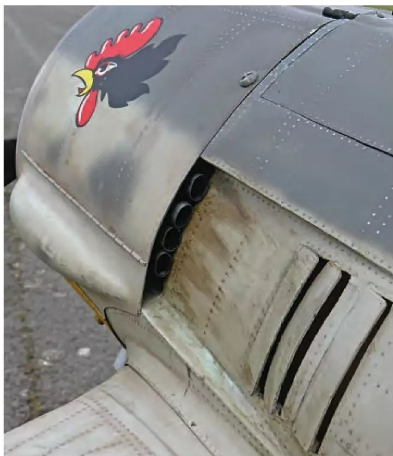
Dummy exhaust outlets and louvres are both used to vent hot air from the Moki.
