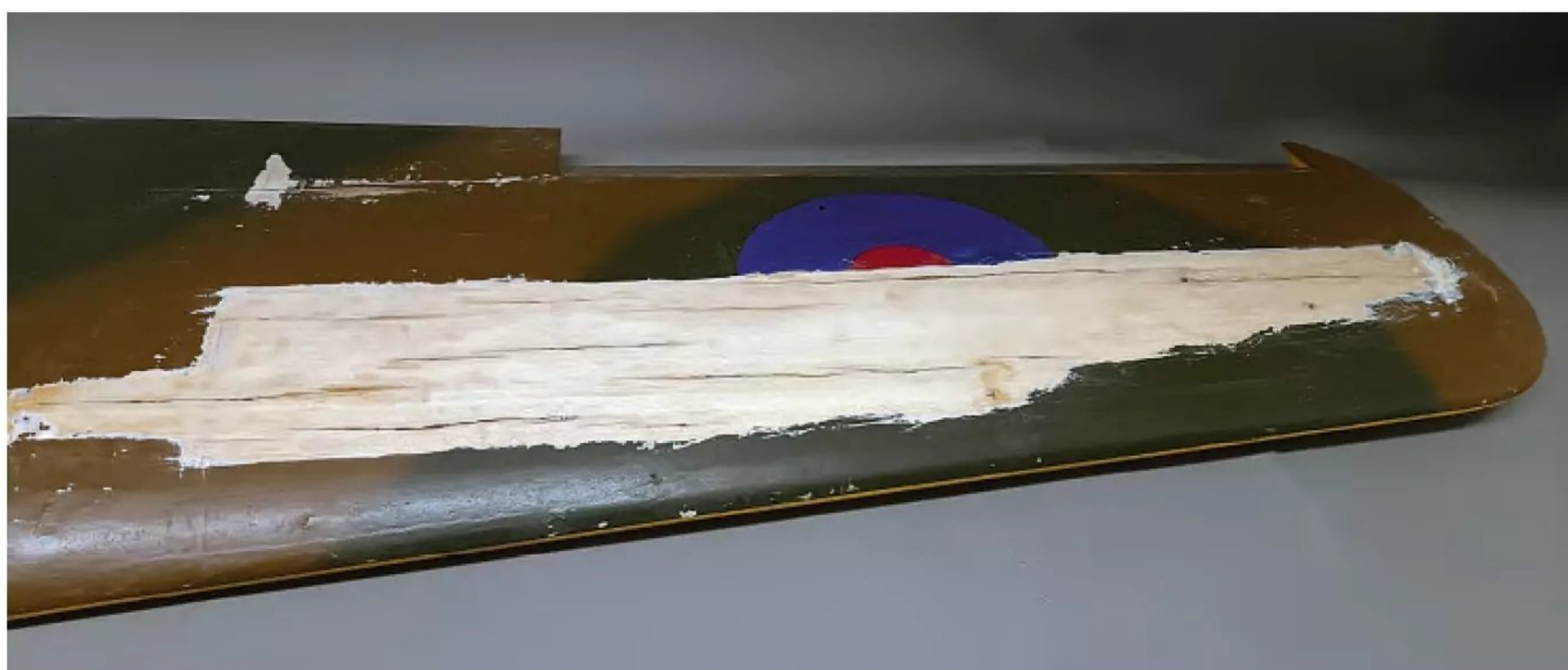
The finished veneer repairs rubbed back and ready for covering and painting.
