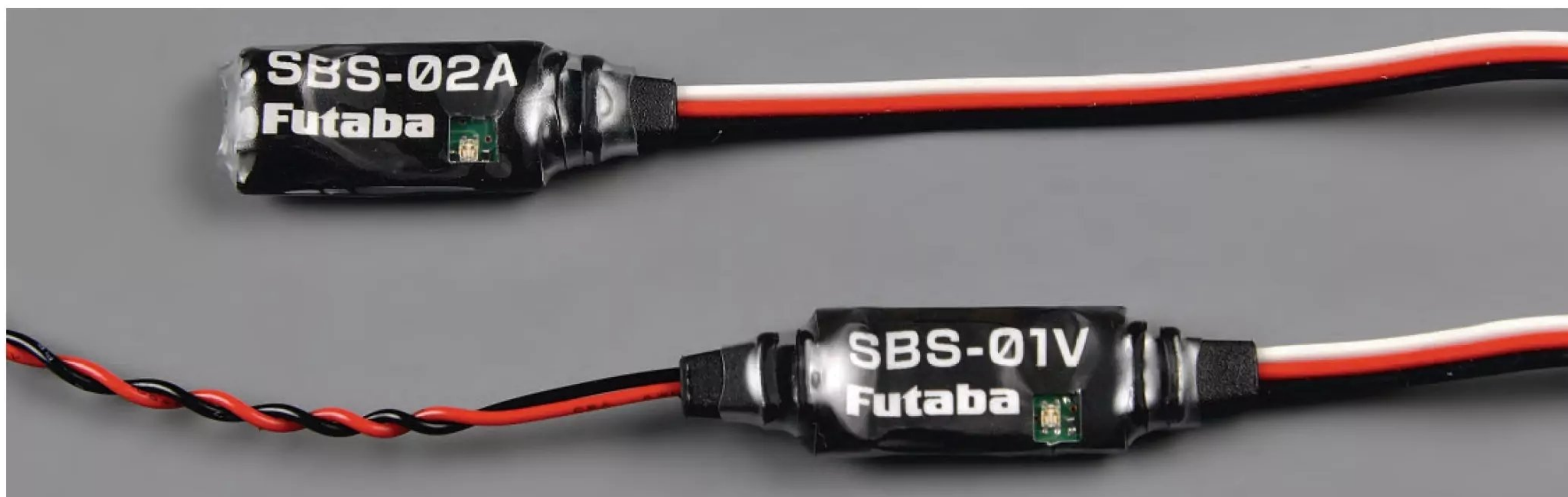
Examples of Futaba telemetry sensors, with a Vario on top and a Voltage sensor below. Telemetry data can be fed back either on screen or by voice announcements.
