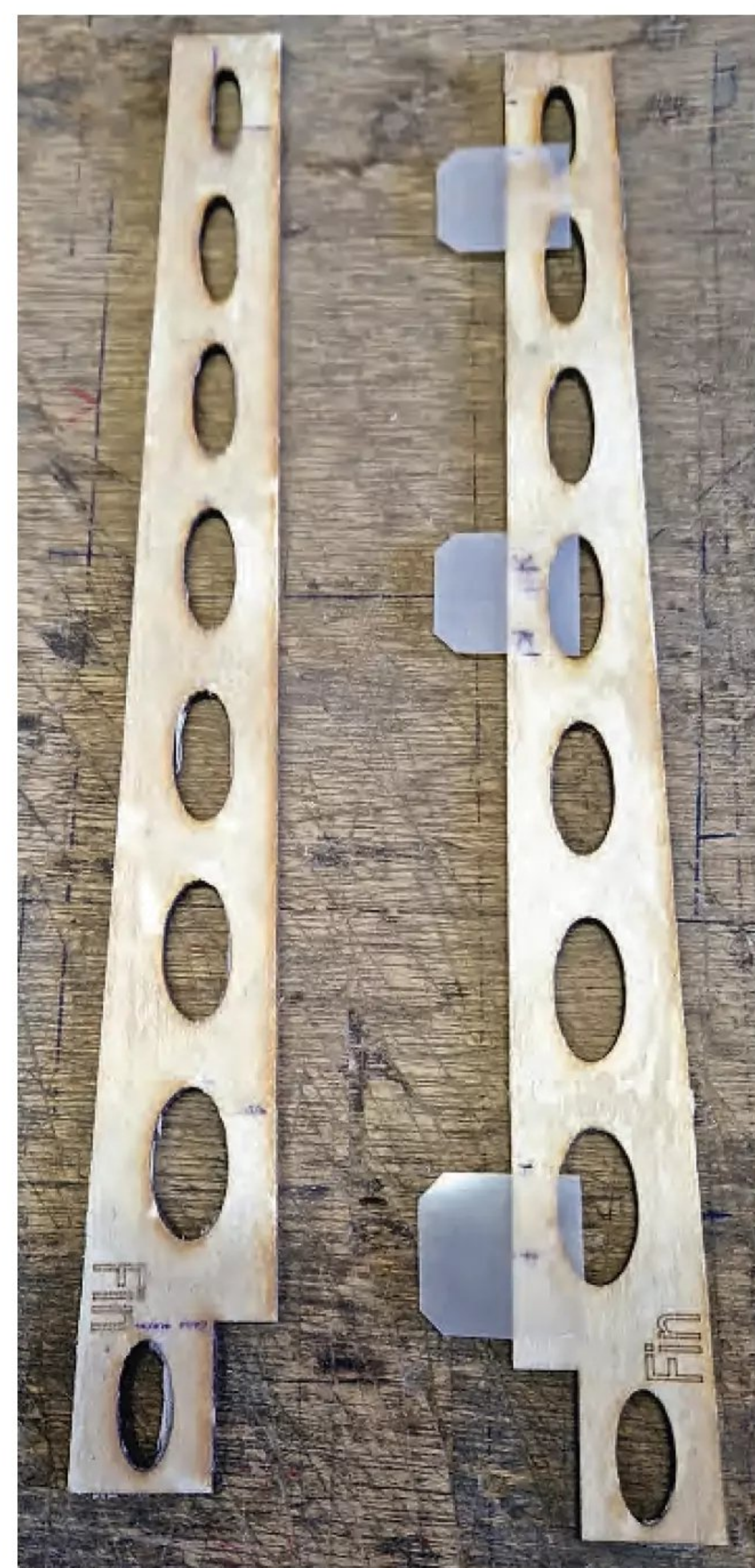
Mylar hinges are sandwiched between the two fin post halves.
