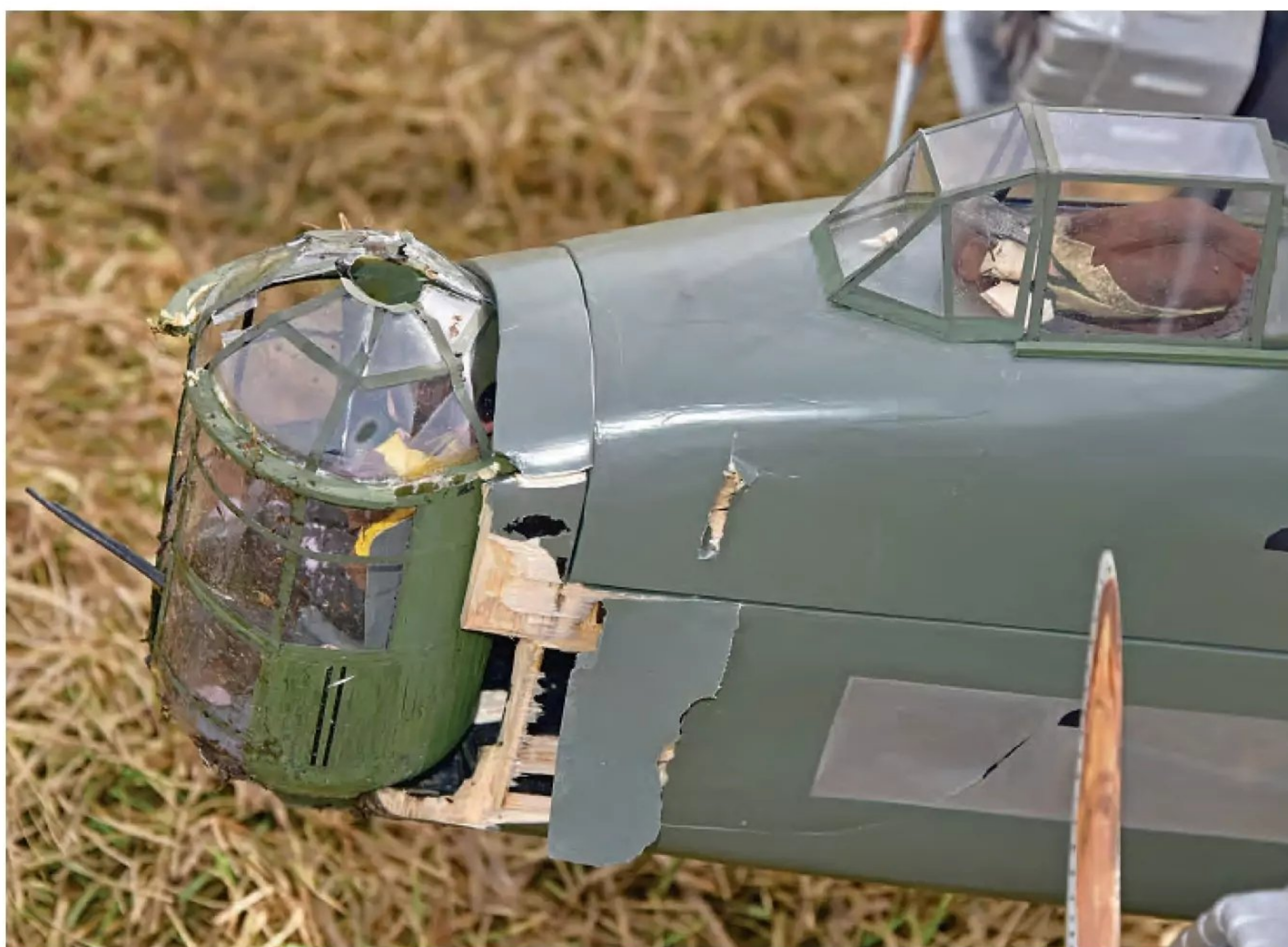
Nose structure after the test flight crash. Note the compressed turret which made a great crumple zone.
