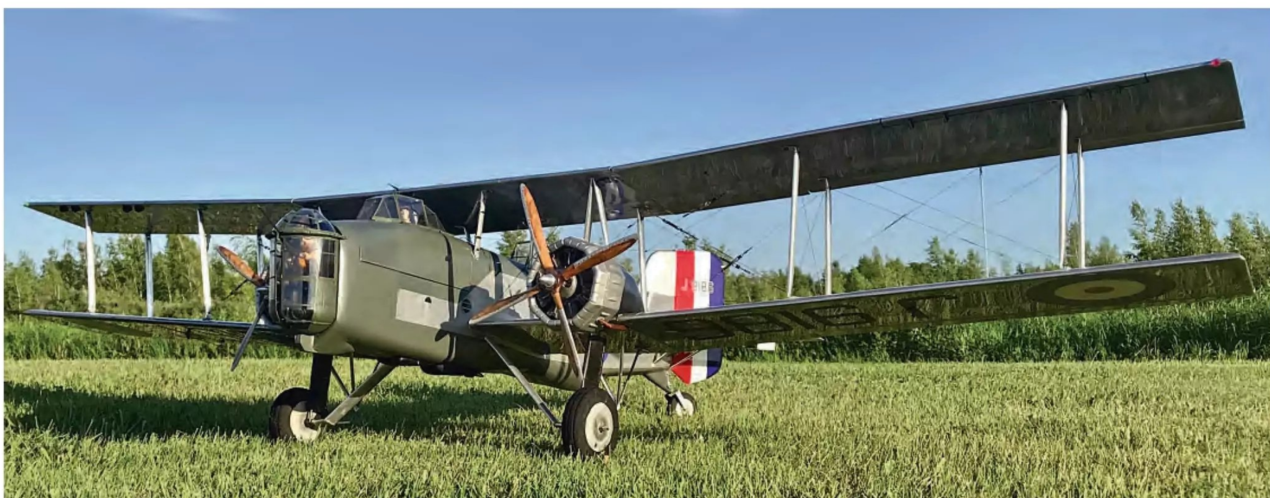
A good illustration of the plethora of scale flying wires.
