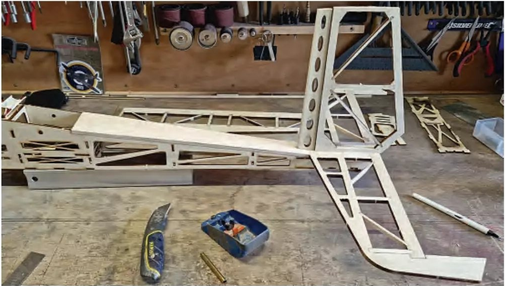
Rear decking in place after planing and sanding it to follow the fuselage sides. Just needs rounding off.
