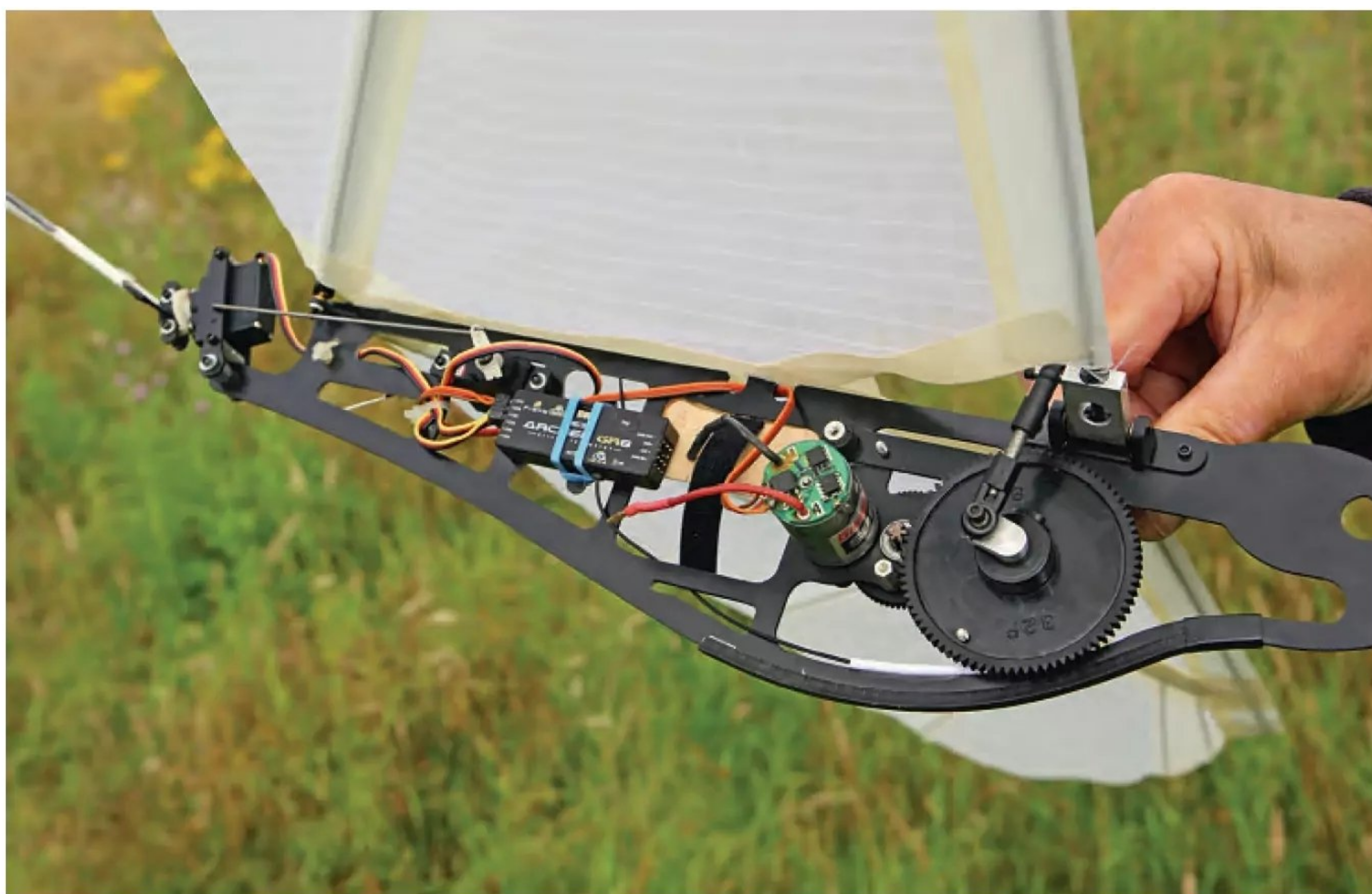
It's about 20 years old and came from the USA. Note the brushed motor.
