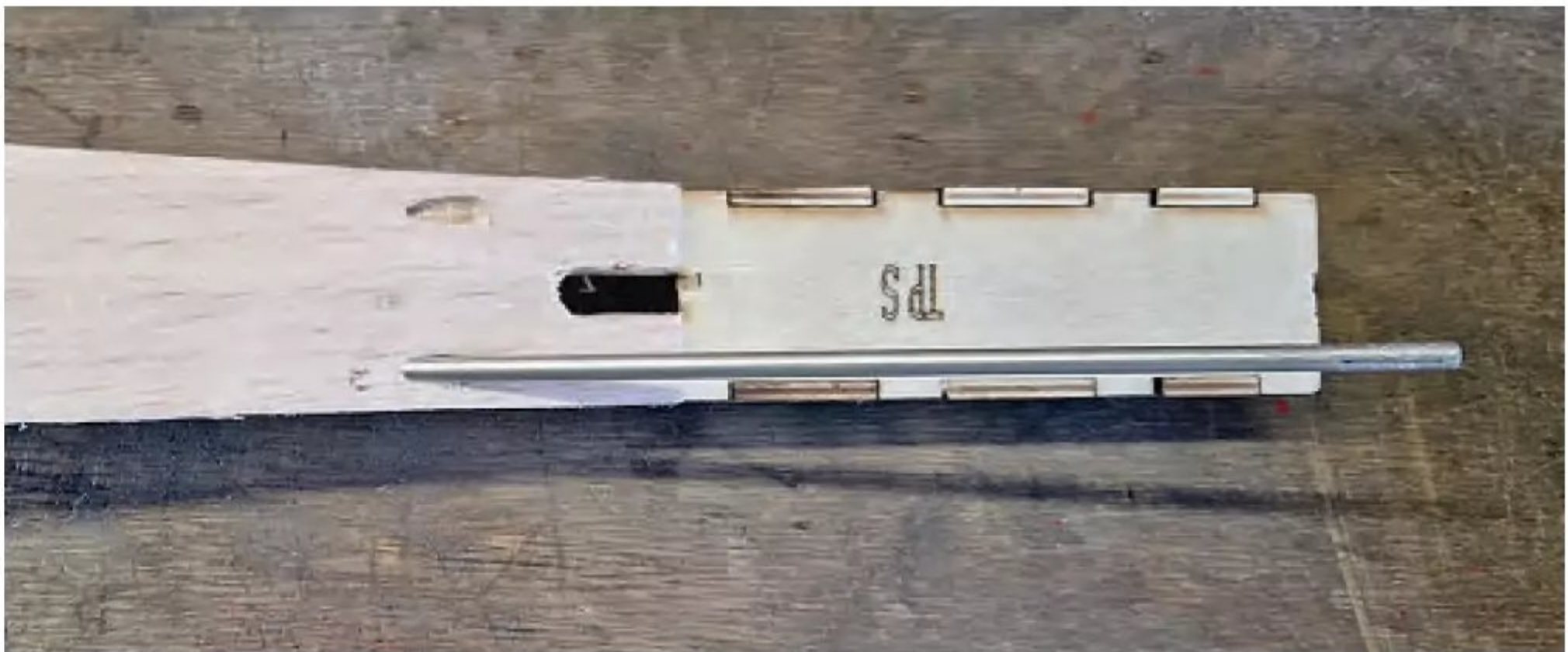
A sharpened ali tube was used to ream out holes for the rudder closed loop guides.
