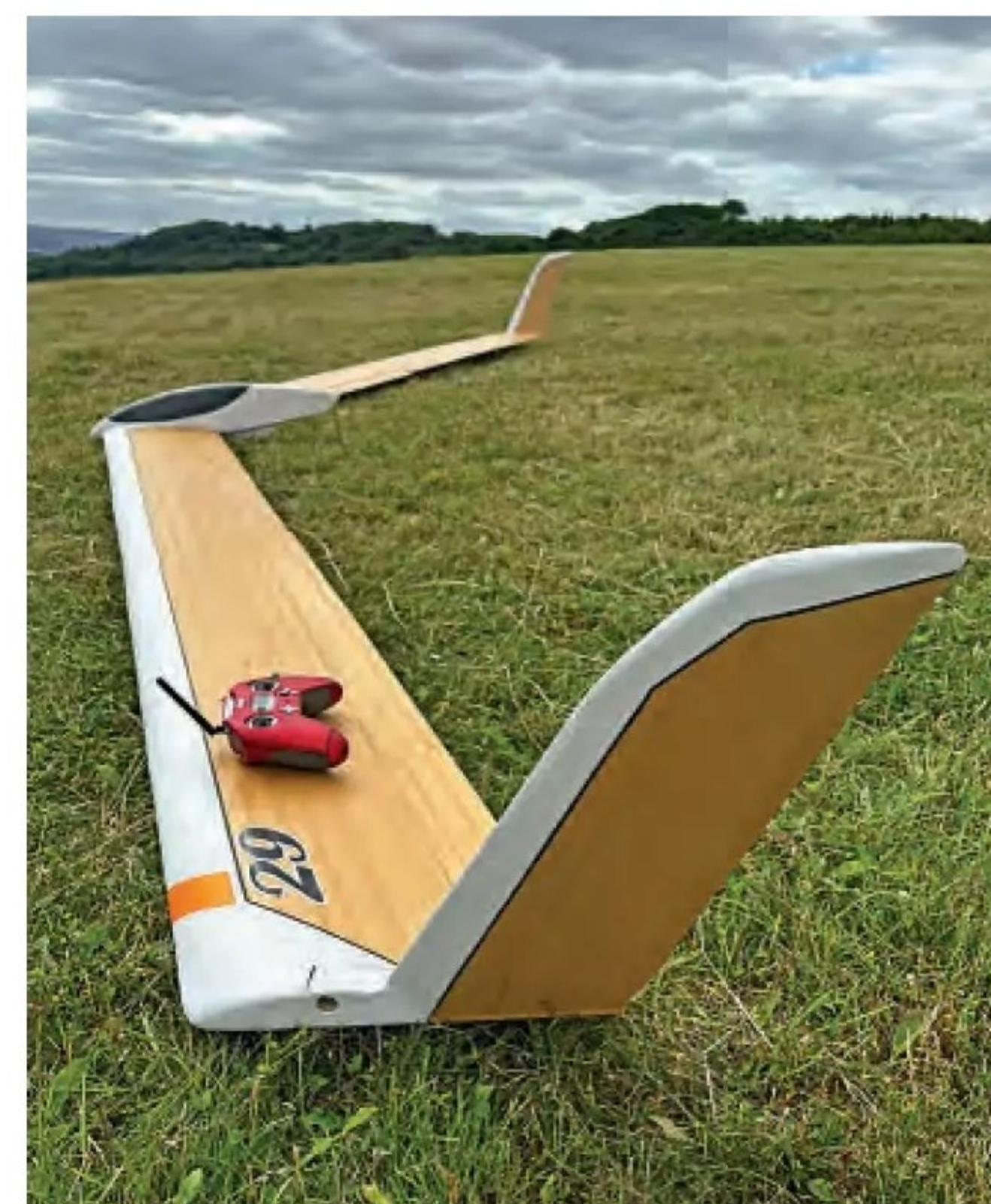
Foam core and glass skinned construction is a common feature.
