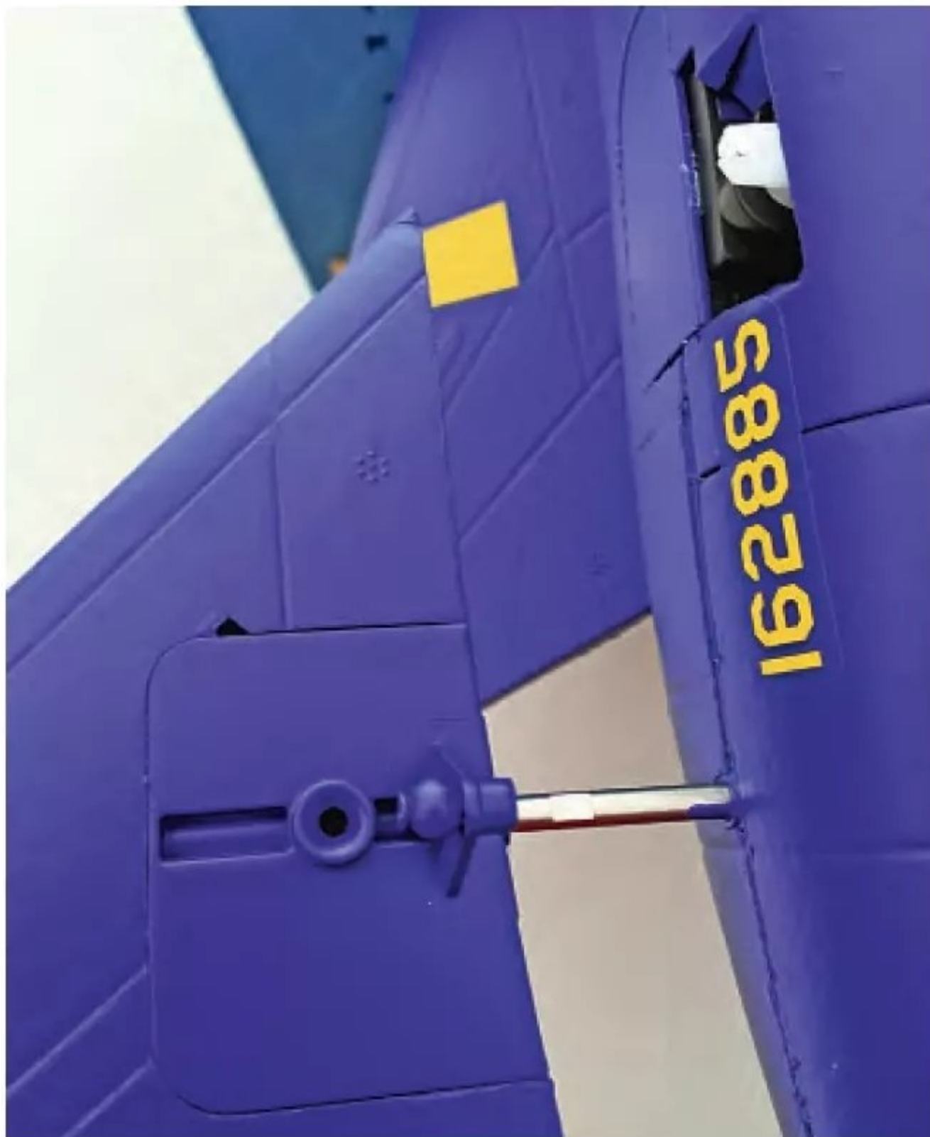
Make sure to align the stab locking screws with the flats on the pivot shafts.
