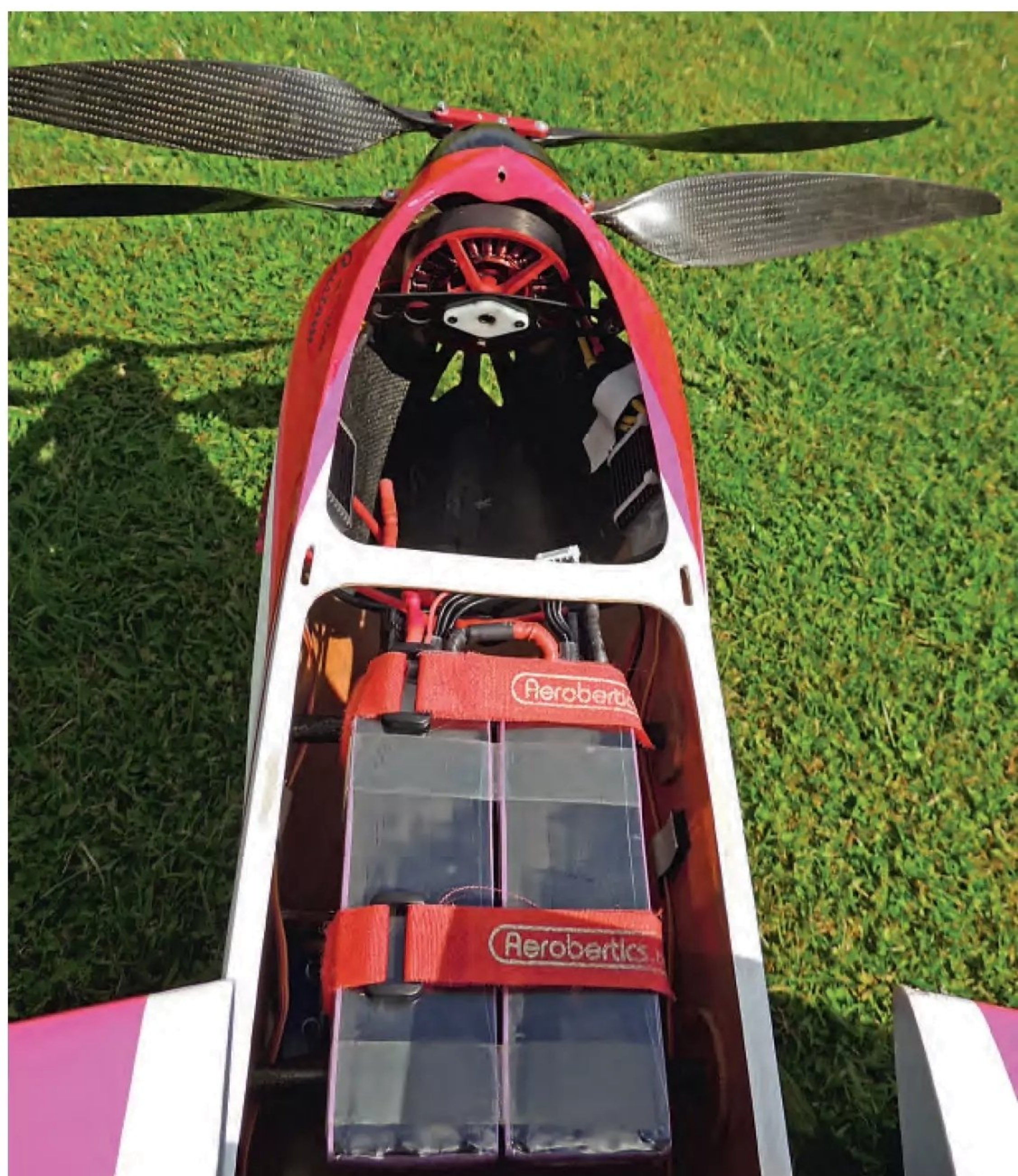
Derk's Hui Yang Ascent biplane was powered by the unique D3 contra drive system from Adam Dubowski.
