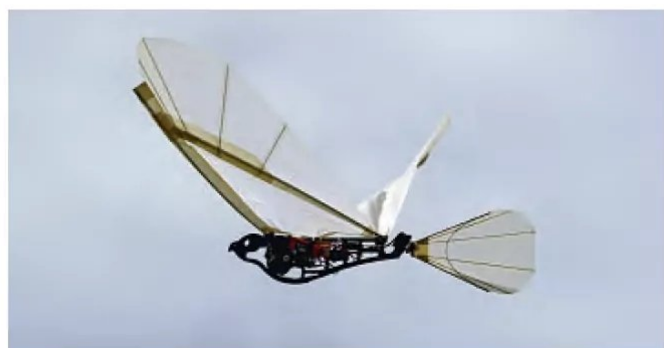
The flight characteristics were initially 'interesting'. Note the crazy amount of tail deflection required to guide it.
