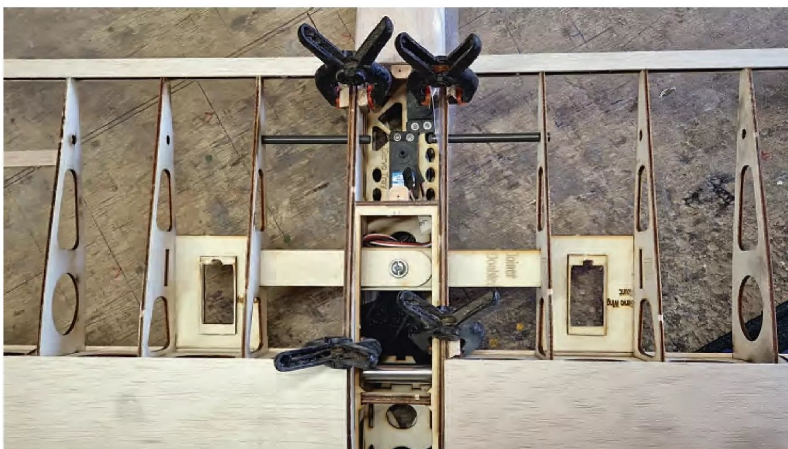
Trial fit of the wing panels to the fuselage.
