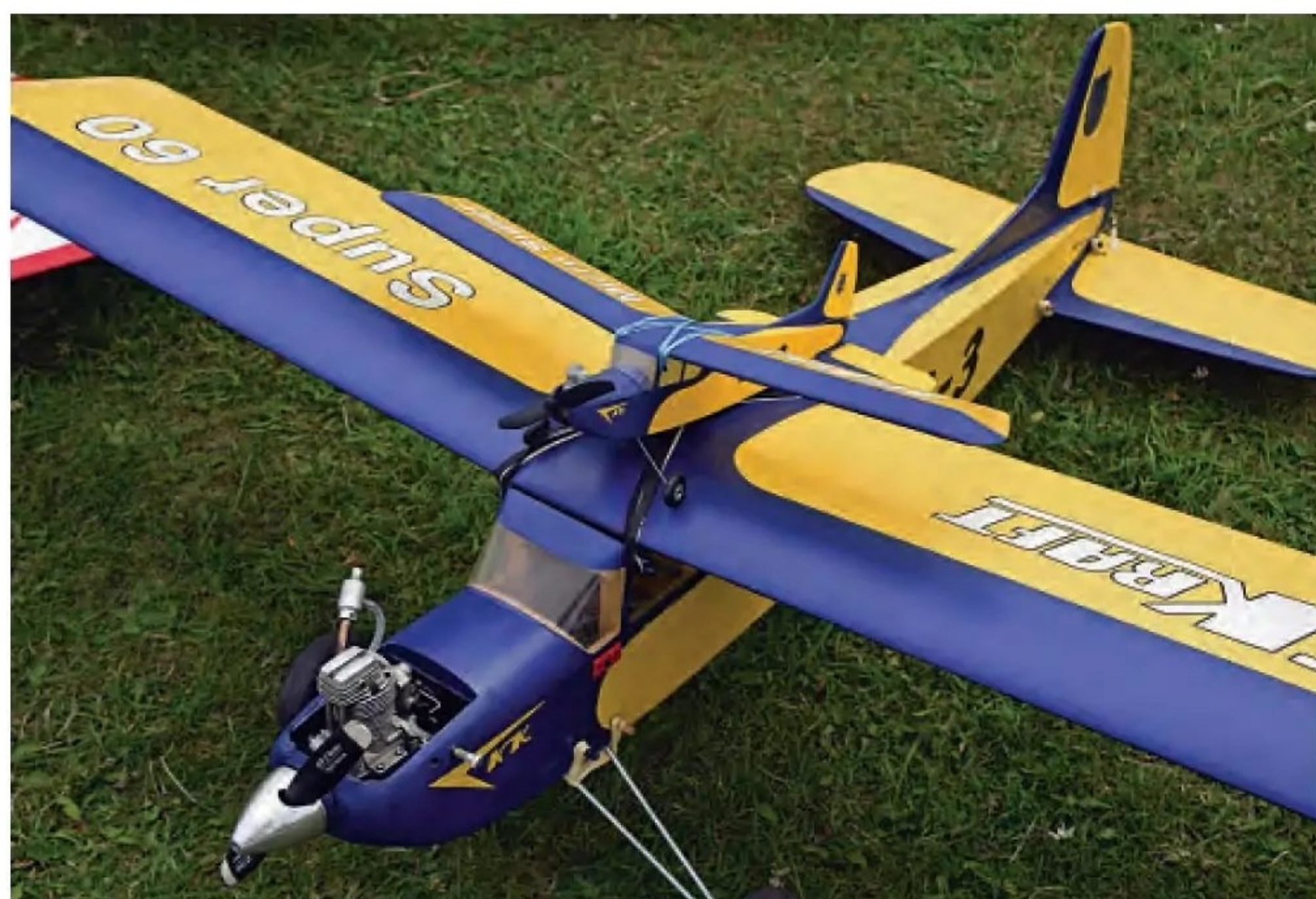
Just have a look at the 3D printed four stroke on the micro Super 60.
