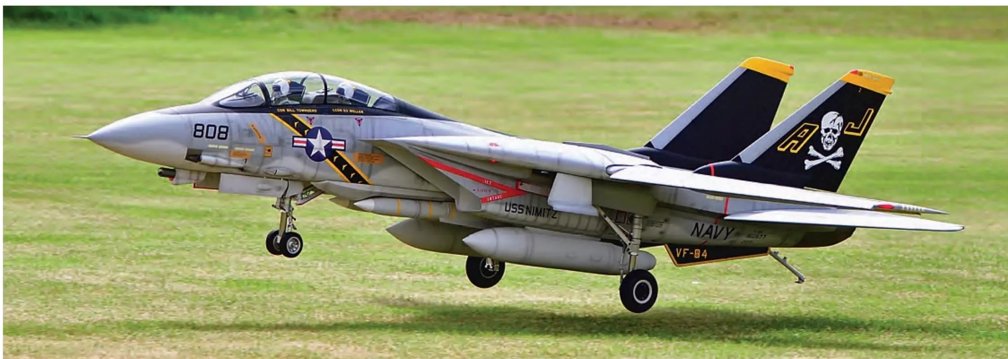
Tomcat makes a safe return. Note the working LE slats and the drooping arrestor hook.
