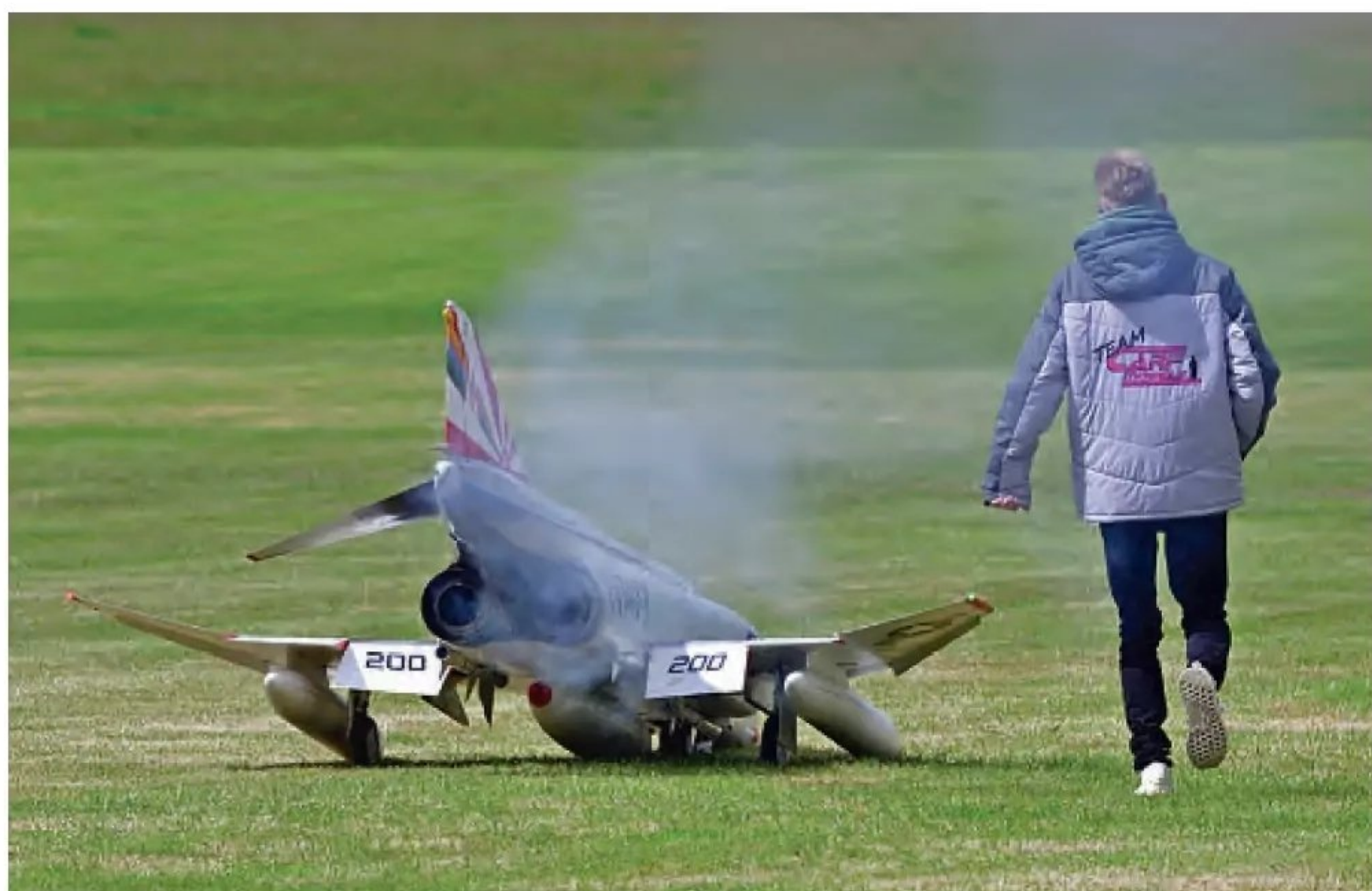
Sadly, the F4's nose leg came a cropper a few minutes later. CARF have already beefed up the leg's design ready for production.
