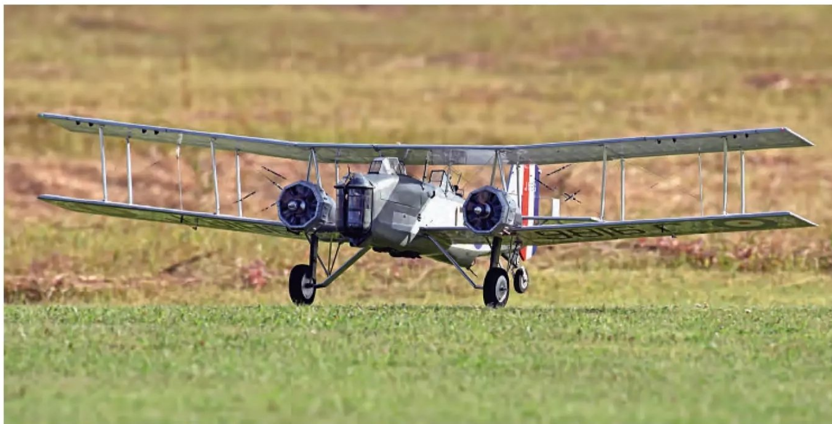
Take off roll requires a large amount of right rudder to counteract the propeller gyro effect. I would highly recommend using counter rotating props to dumb this down.
