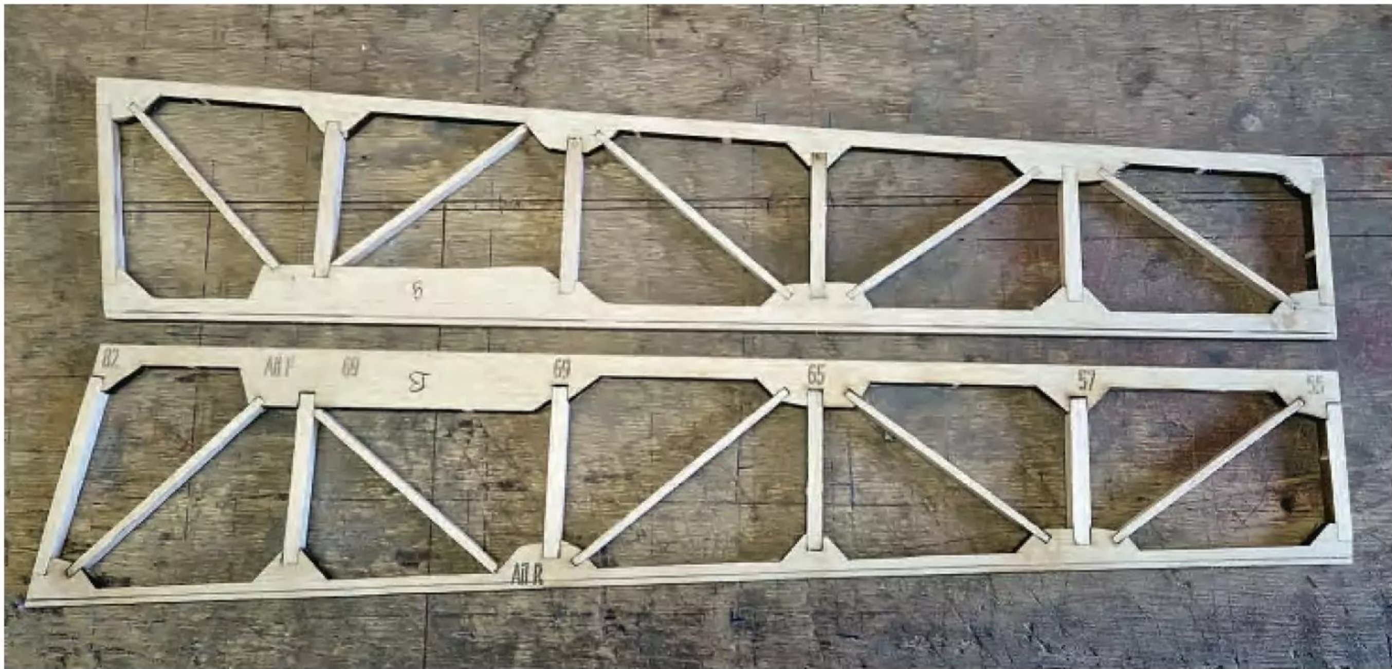
Well braced ailerons use plenty of gussets.
