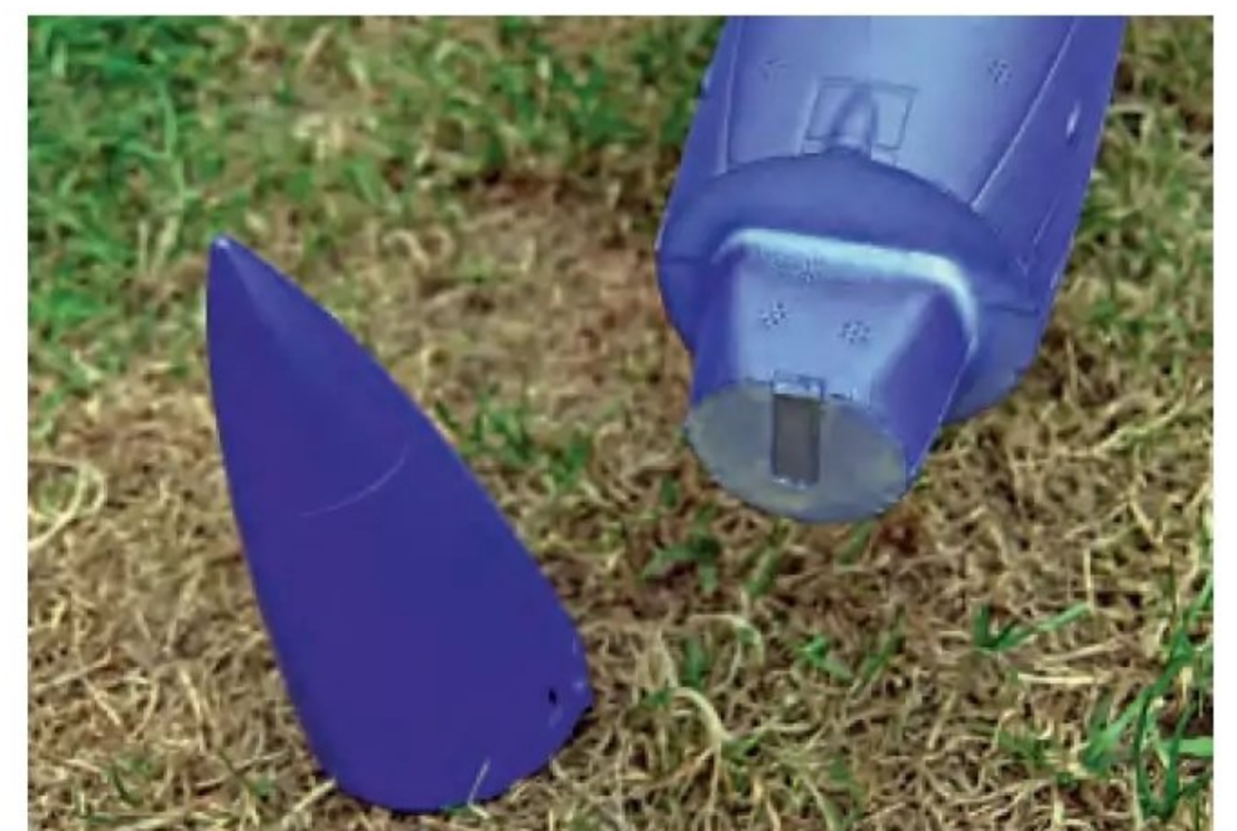
Nose cone is held in place with a strong magnet, allowing it to pop off if it makes contact with the ground when landing.
