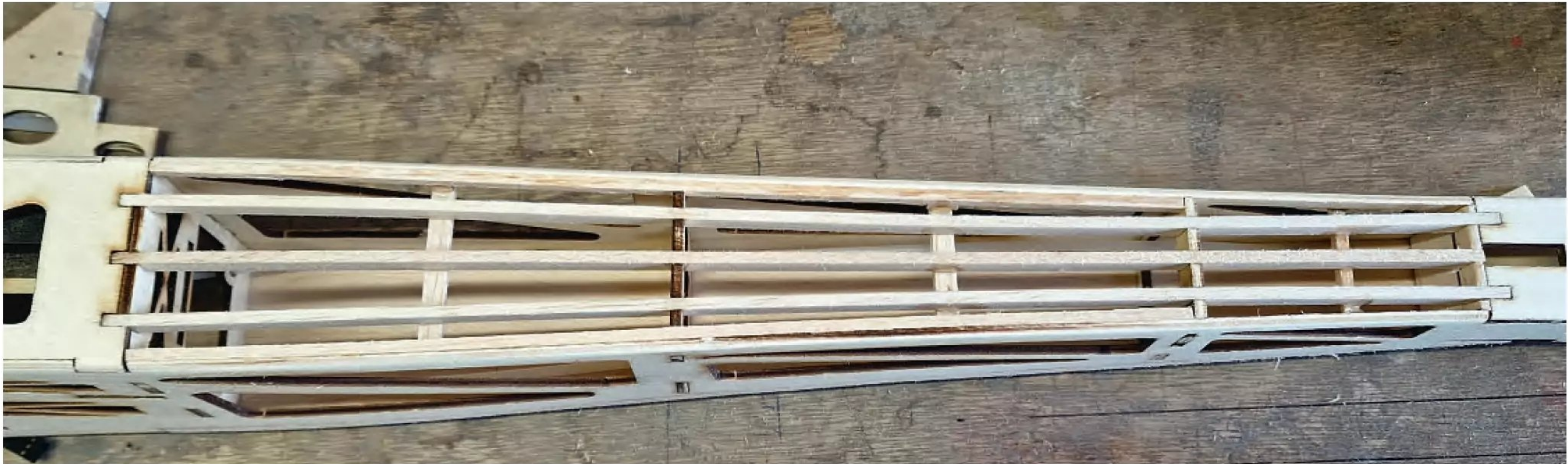
Stringers are used to fill in the underside of the fuselage.
