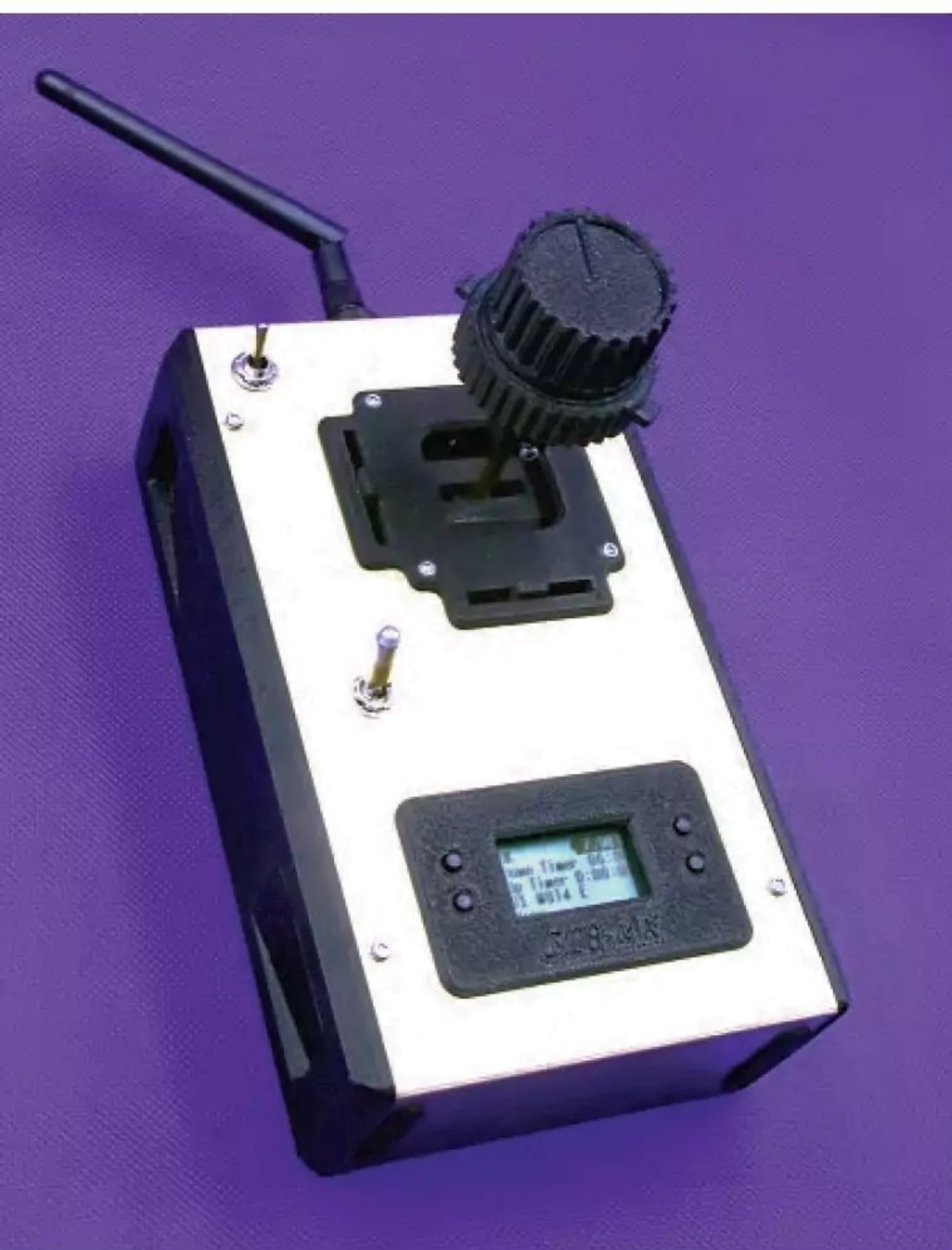
Tobe's unique four function single stick set as mentioned in the article.
