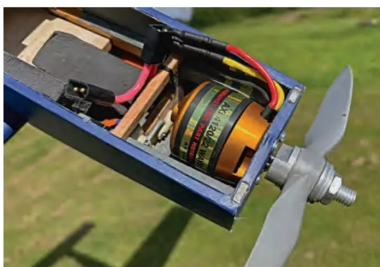
Recently updated, an outrunner and six LiPo cells now provide the urge.
