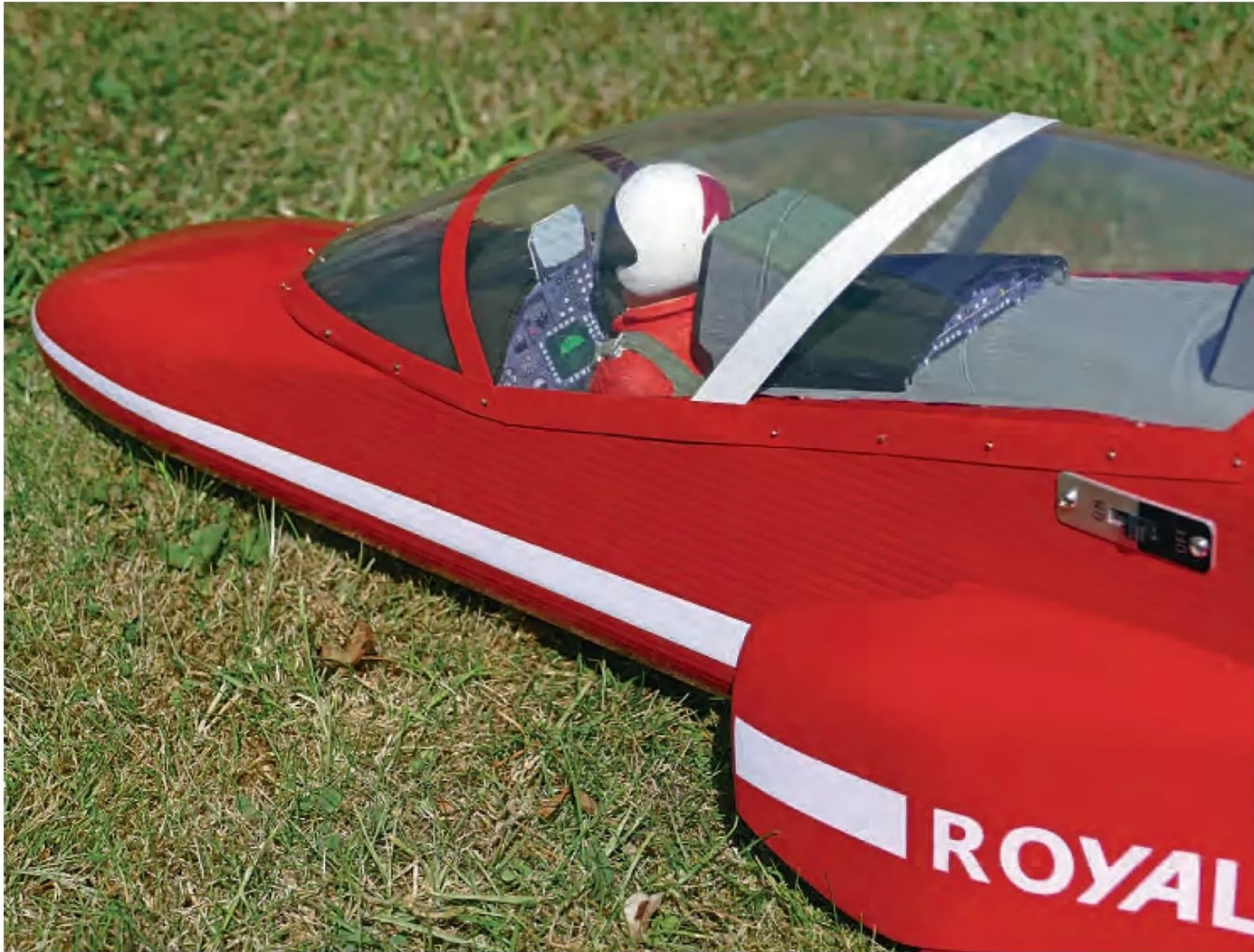
The long Hawk canopy can be made from two 2 litre soft drink bottles moulded over a wooden former.
