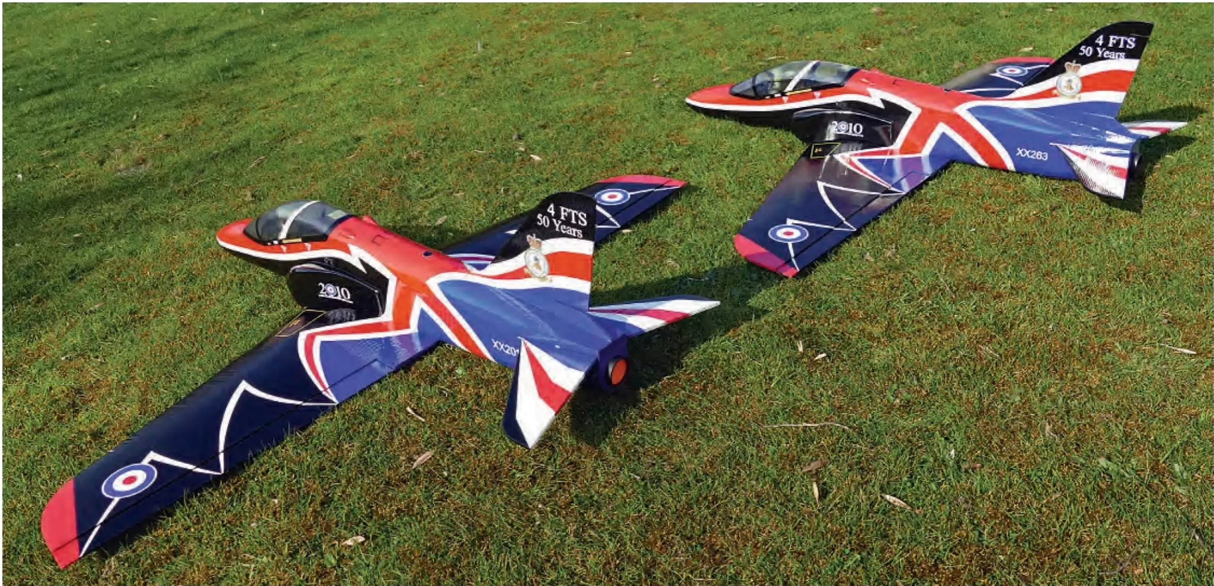
The Union Jack Hawks were one of the most time-consuming schemes to recreate. The four main colours were spray-painted, with graphics made from self-adhesive vinyl and paper prints covered with clear tape.
