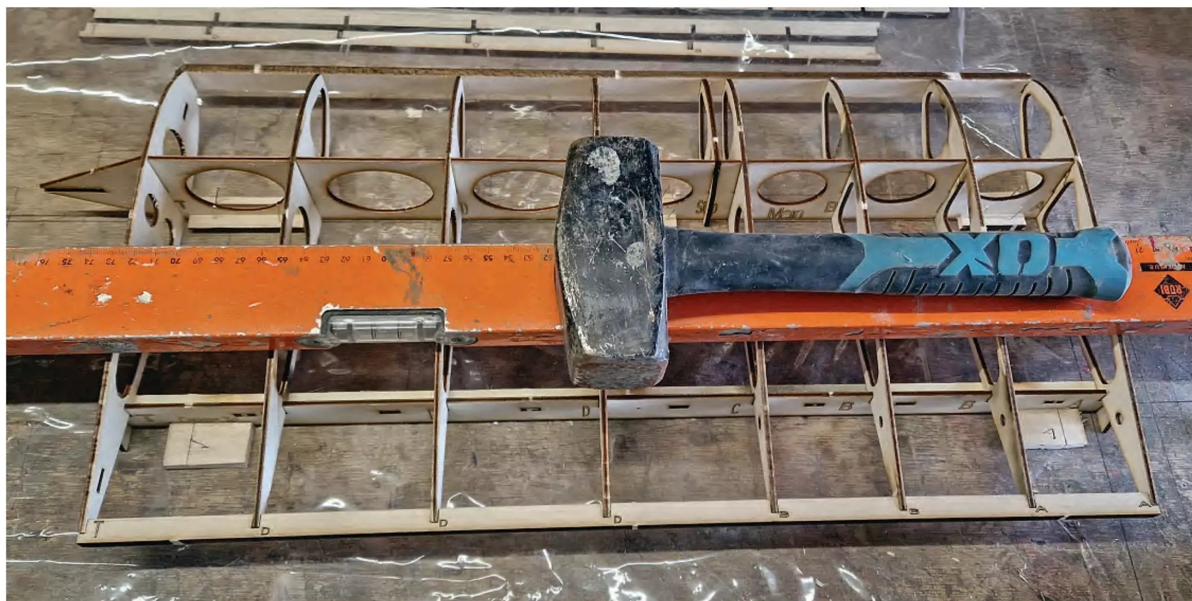
Use a weighted bar to hold the wing structure straight while the glue sets. A spirit level and club hammer do a good job here.
