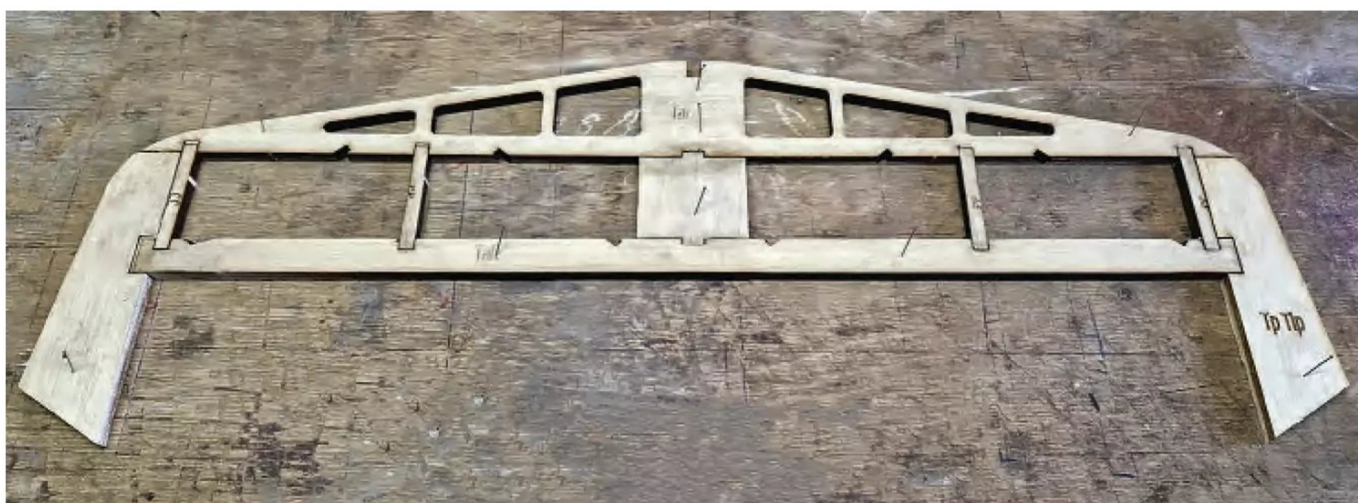
The tailplane slots together very quickly.
