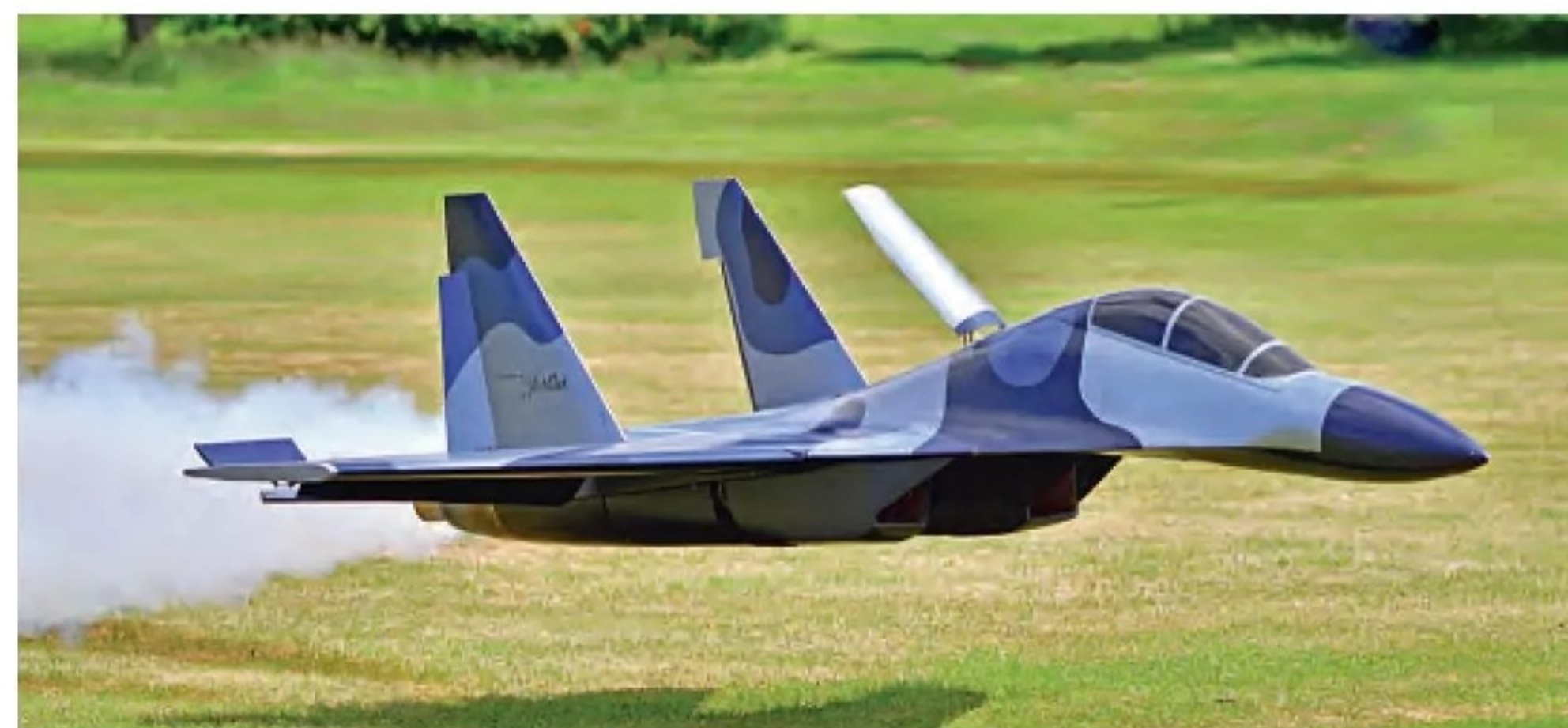
Ralph put his SU-30 into a vertical dive with its air brakes deployed and pulled out into a low level fully braked pass. Note the twin rudders in opposition and raised wing TE air brakes as well as the obvious hatch brake.
