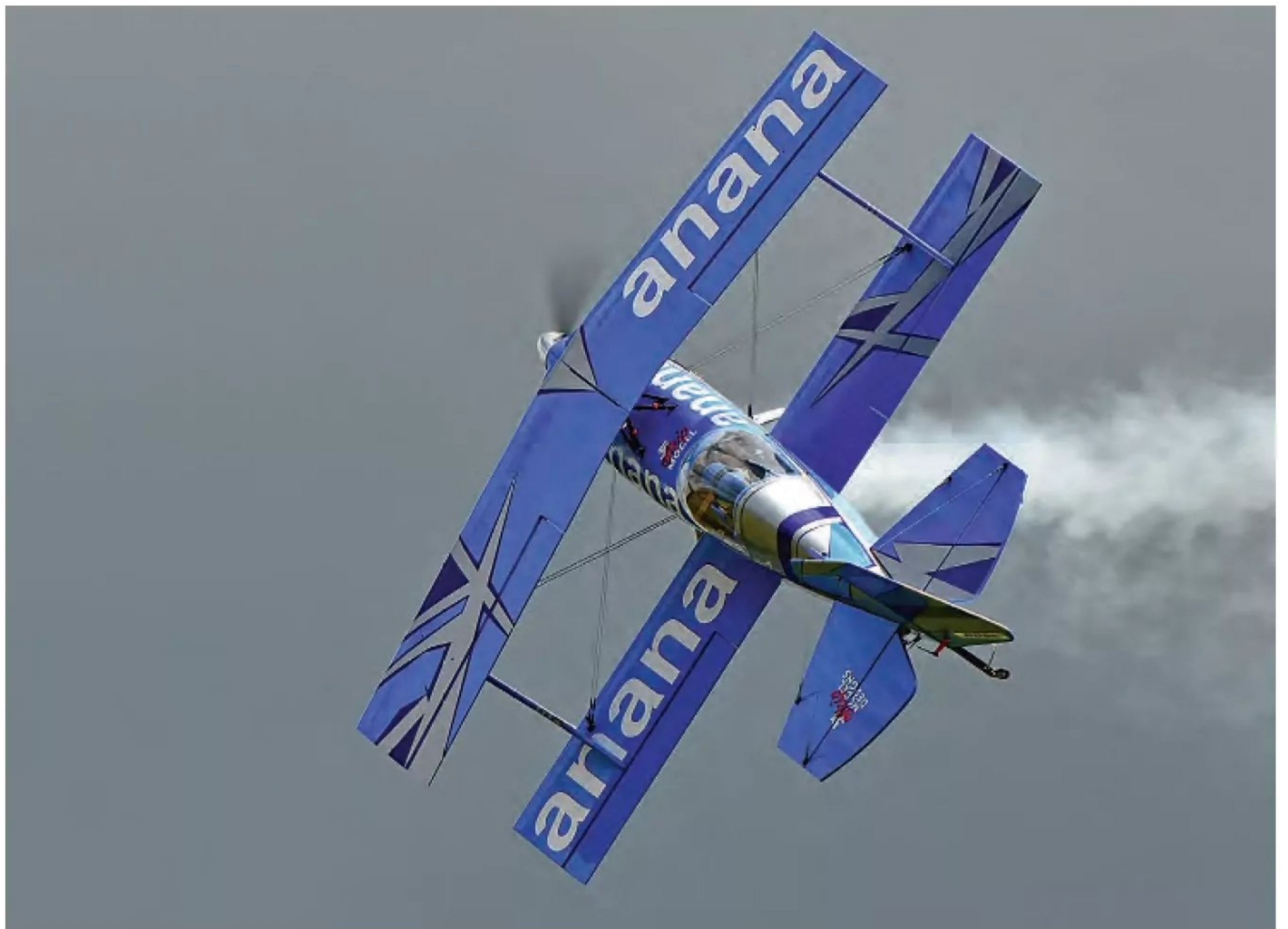
Adam Broomhead's 44% Pitts Challenger V1 on a Farnborough Pass. It's a built-up kit from Skip Models and has a DLE120 up front.
