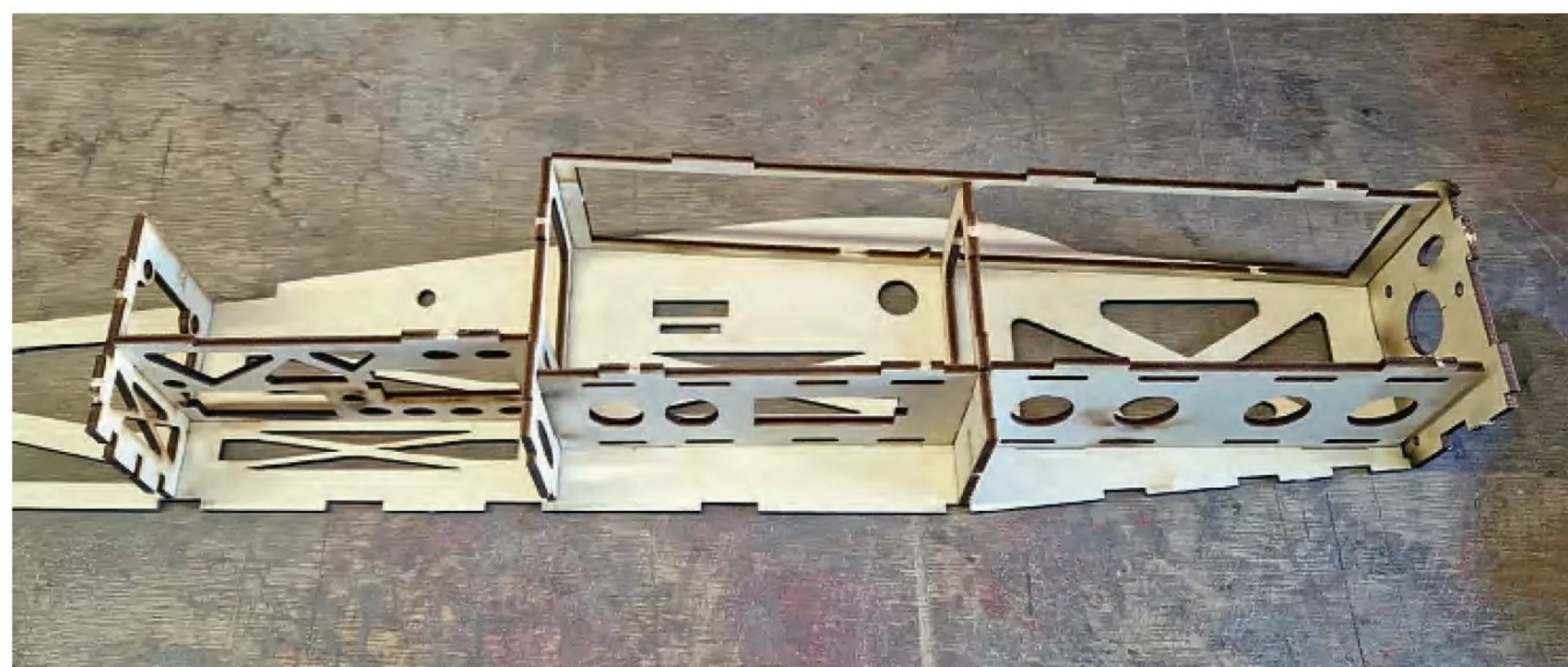
Initial stage of fuselage construction.
