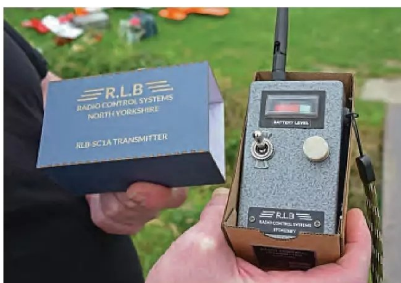
Ron Buckwell's skill at making one-off transmitters is astounding. He uses a laser to make the labels and cut logos on the cardboard outer case. The nRf transmitter and encoder electronics are also home constructed by Ron using Phil Green's code and circuit design.
