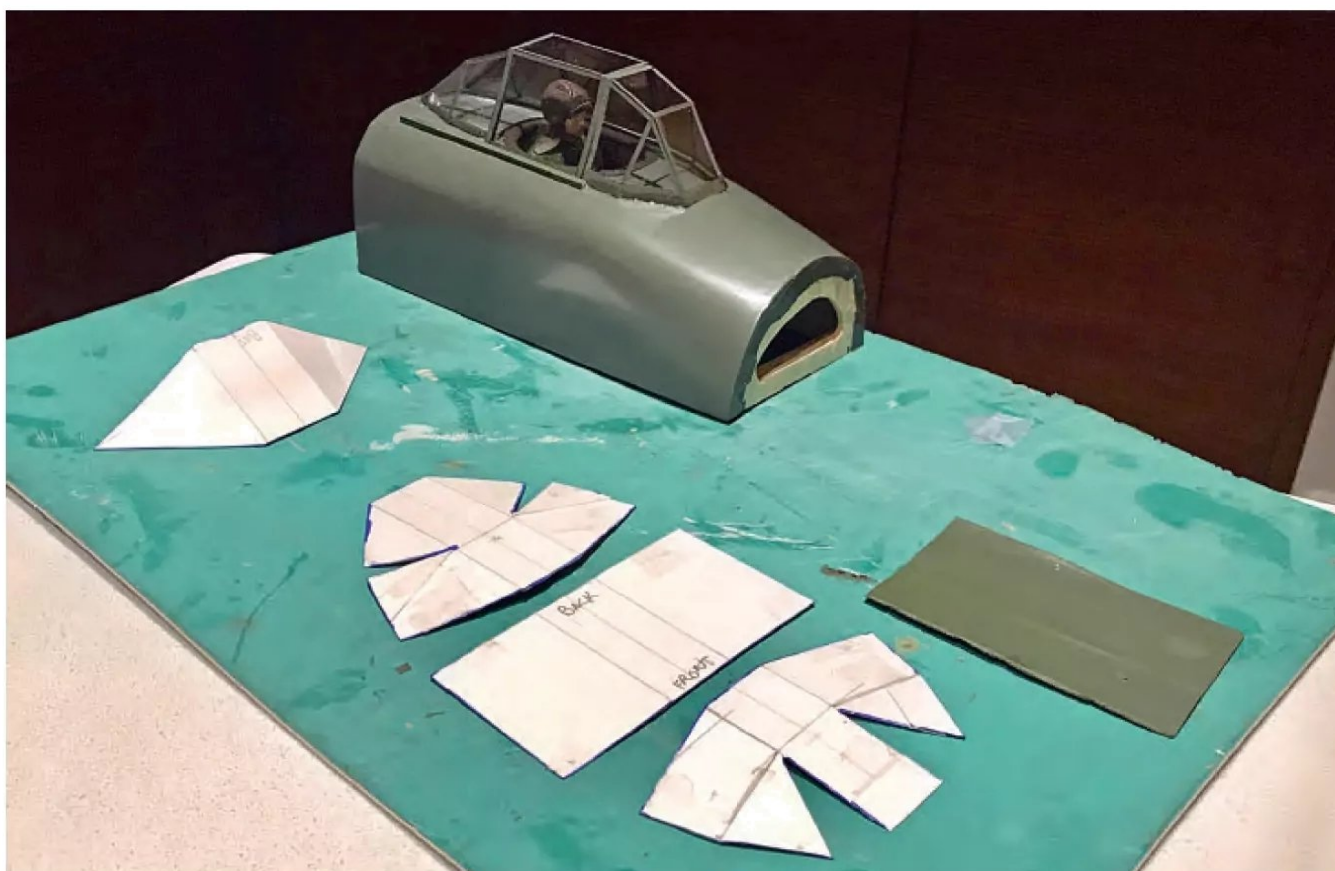
Cardboard canopy templates were used to confirm the shapes prior to cutting the final parts from acetate sheet.
