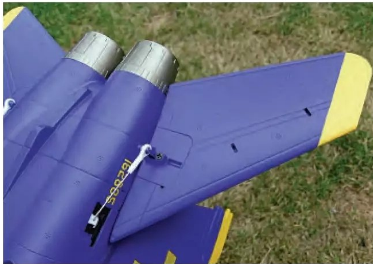
Each all-flying stabiliser is operated by its own servo.
