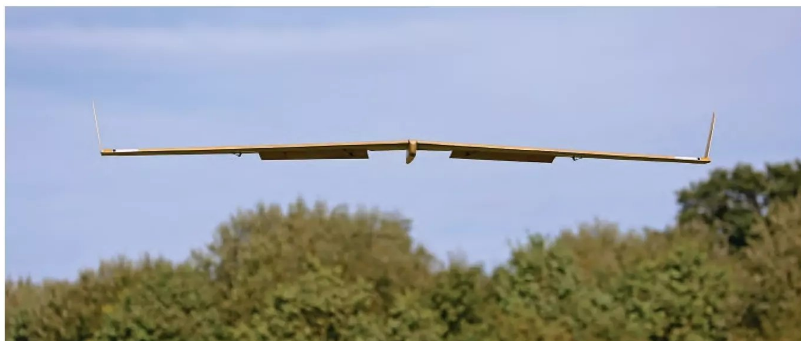
No. 27 weighs 2430 g and uses a 23-degree sweep.
