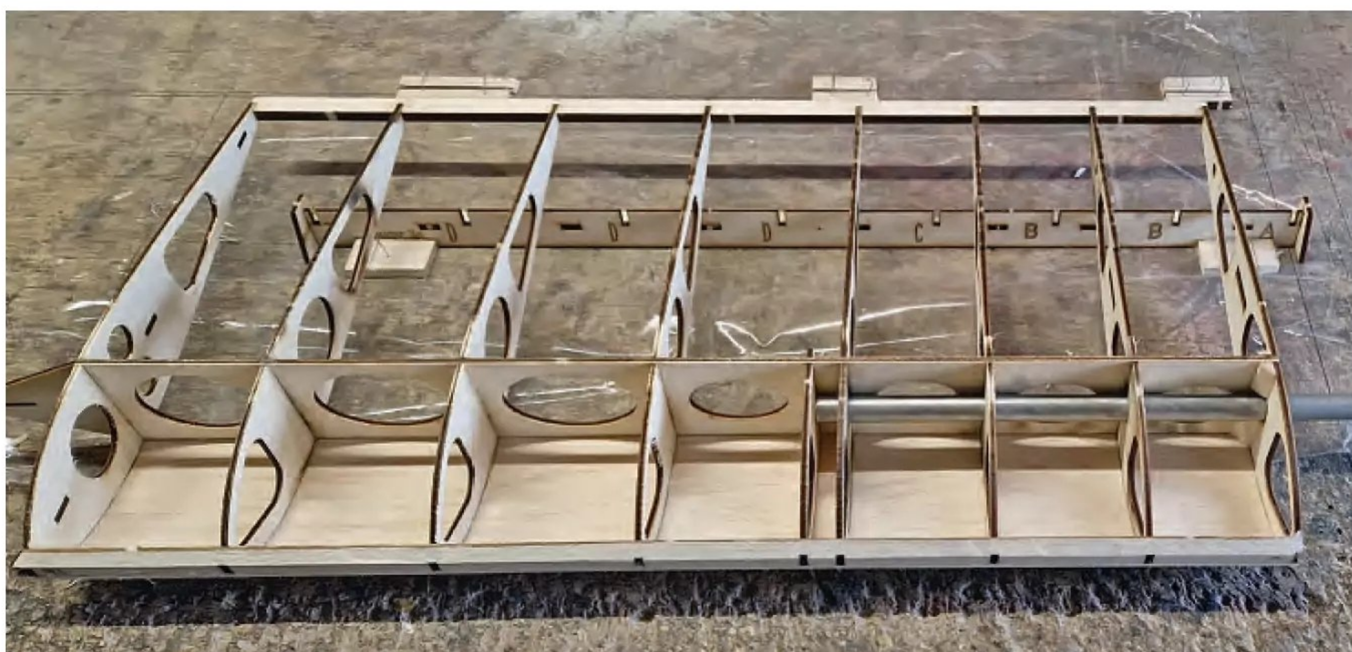
Starting to add the wing sheeting. Note the wing jig supporting the structure at the rear.
