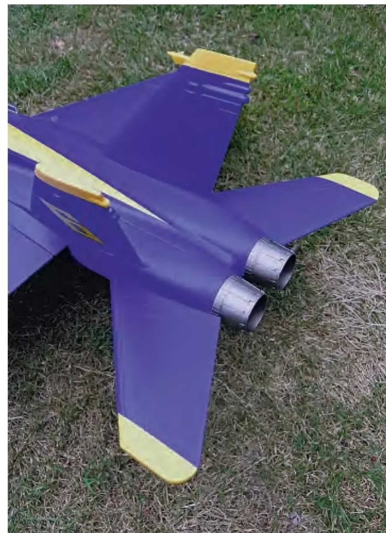
Back end of the Hornet showing its distinctive twin fins, large all-moving stabilisers and the well-detailed mock afterburners
