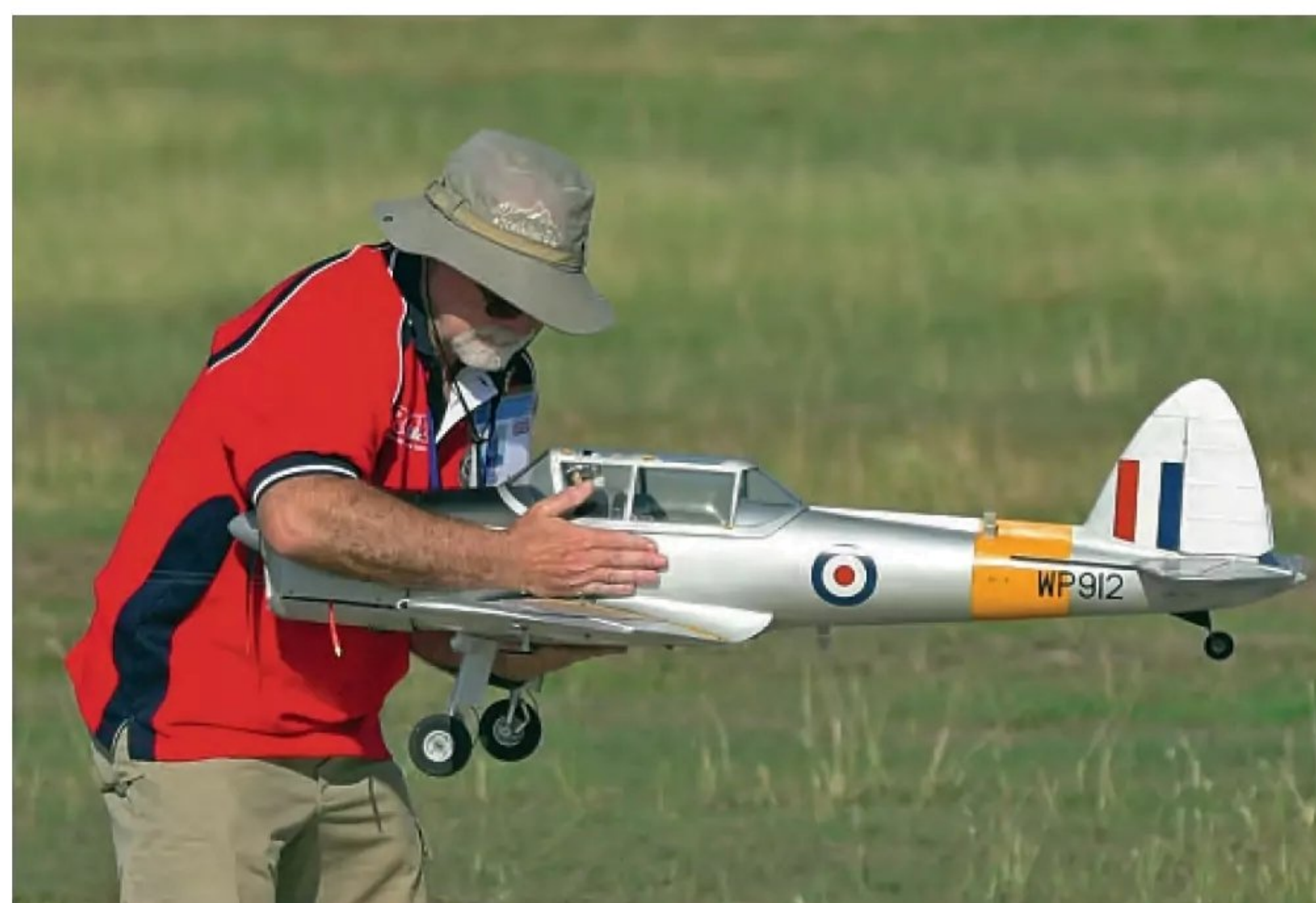
One of the scariest bits is the pull test. Before every flight a spring balance is attached to the handle and the modeller holds his plane while a pull of five times the model's weight is exerted on the handle, lines and bell crank. You can see I am doing my best to spread the load across the fuselage. Failure here and you are going home. My model had to pass a pull test of 12.2 kg.
