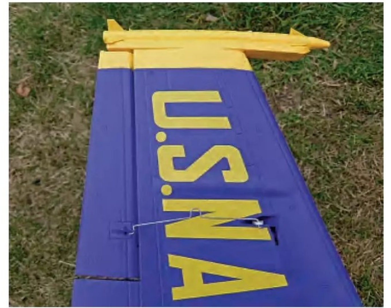
Aileron neutrals are easily adjusted by tweaking the U bends in the wire pushrods.
