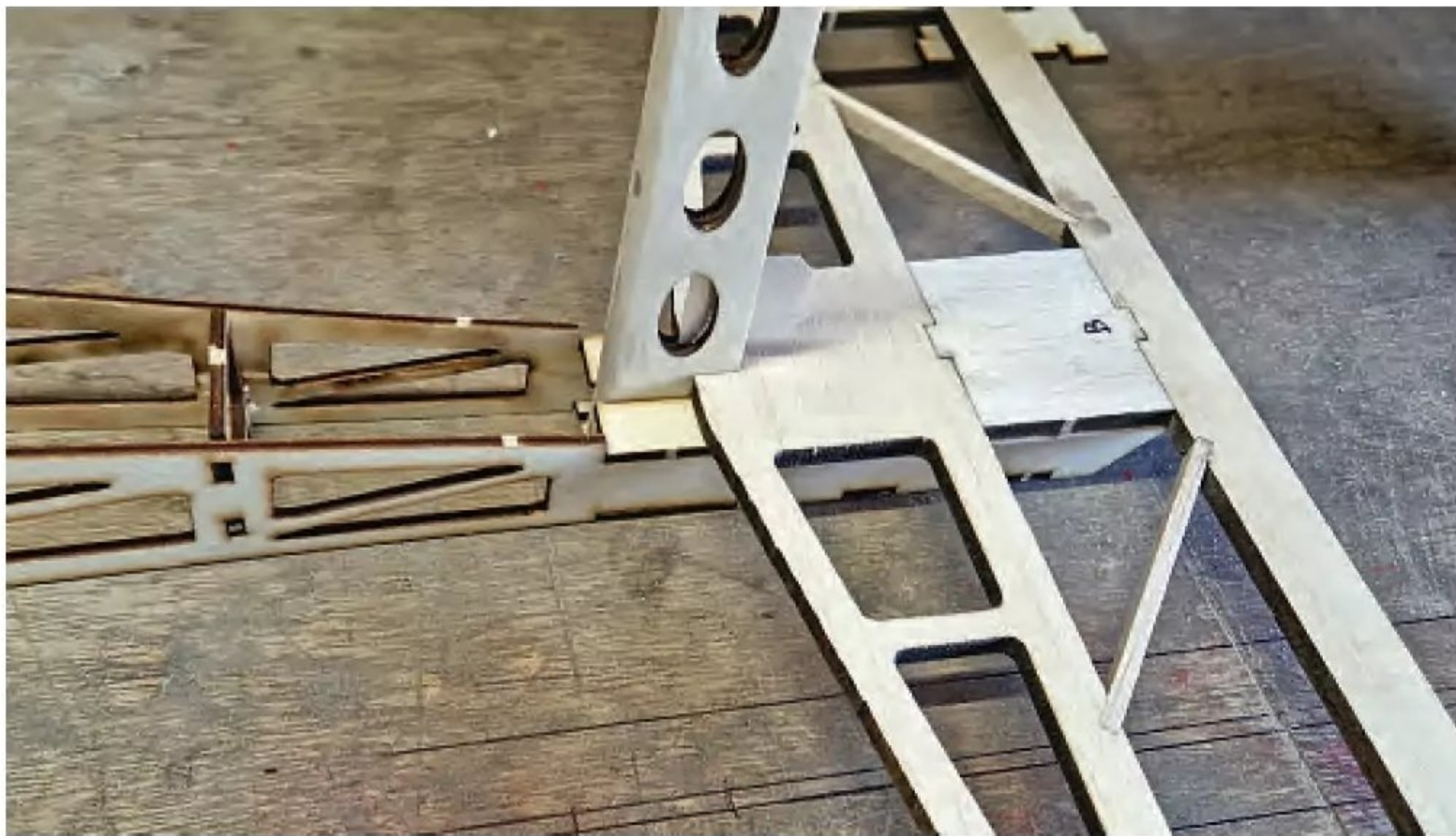
Lining up the tailplane and fin on the rear fuselage.
