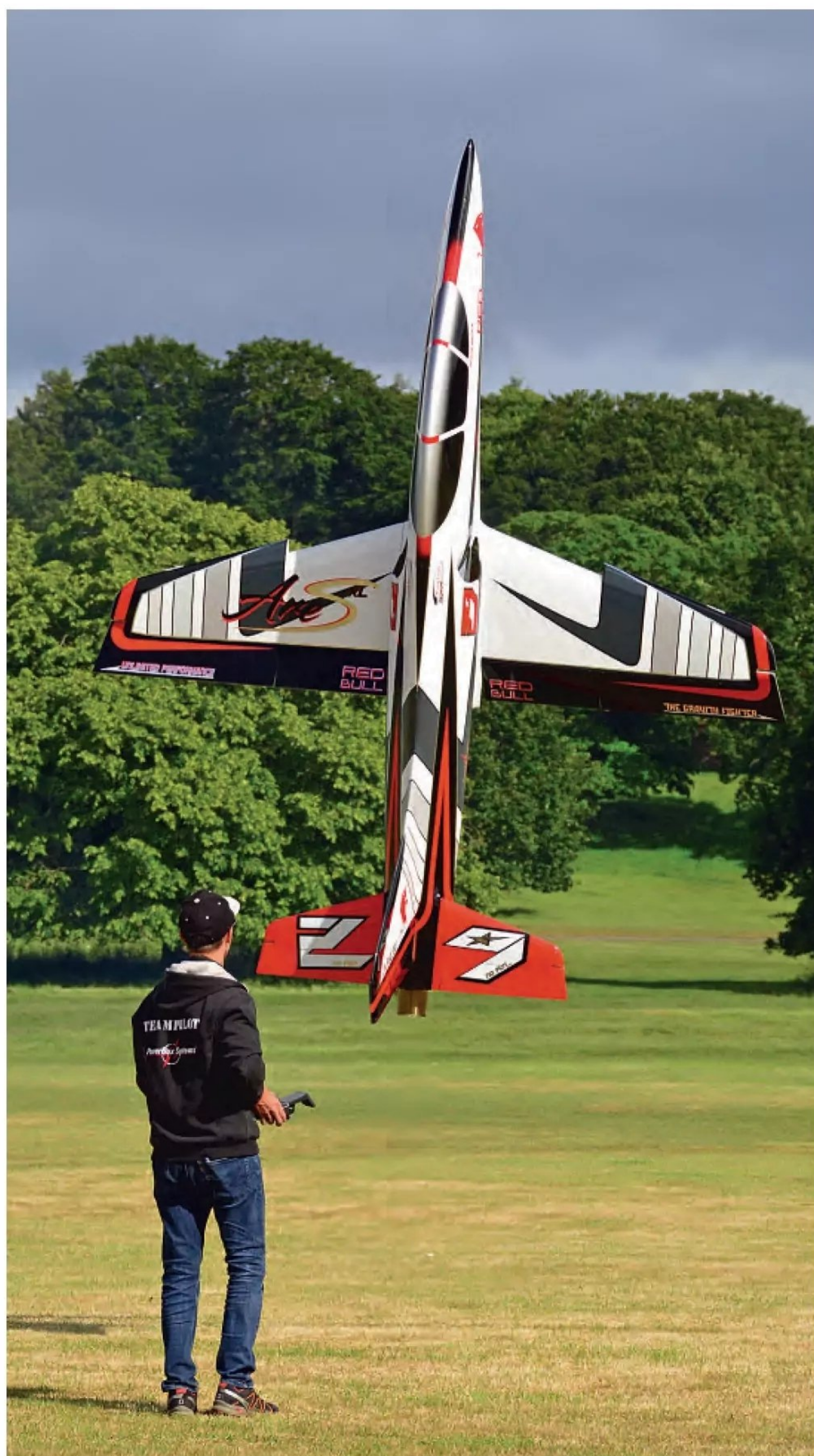
Nicolas Gastaldi gave us a masterclass in 3D jet routines with his Ares XL which is powered by a Kingtech 320 turbine with vectored thrust.
