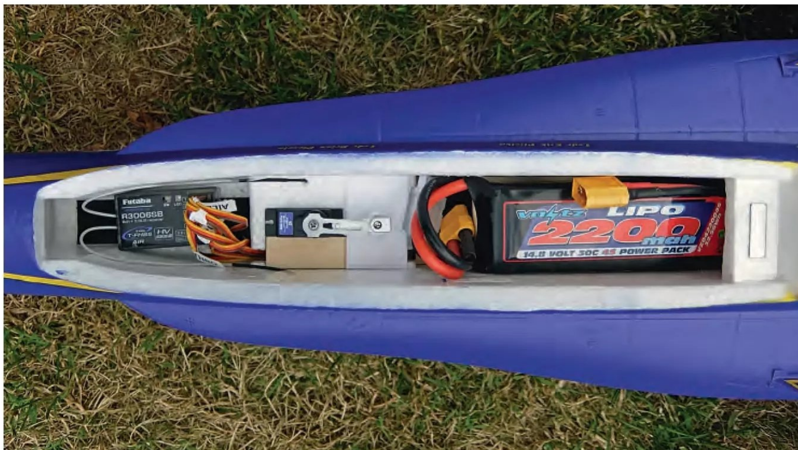
Inside the battery bay, also showing the Rx and steering servo locations.
