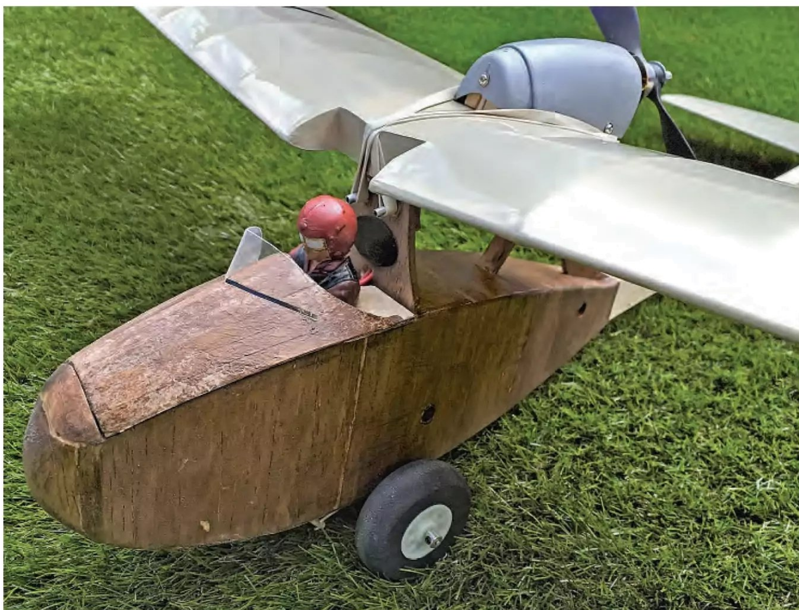
Dark varnish over untreated balsa doesn’t look quite right. Not the effect I was looking for, unfortunately.
