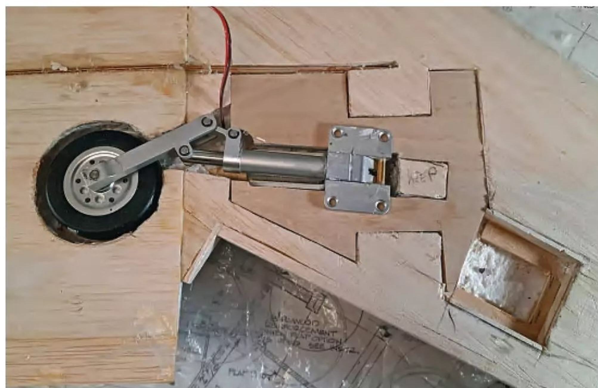
Main retract unit being test fitted to the wing.
