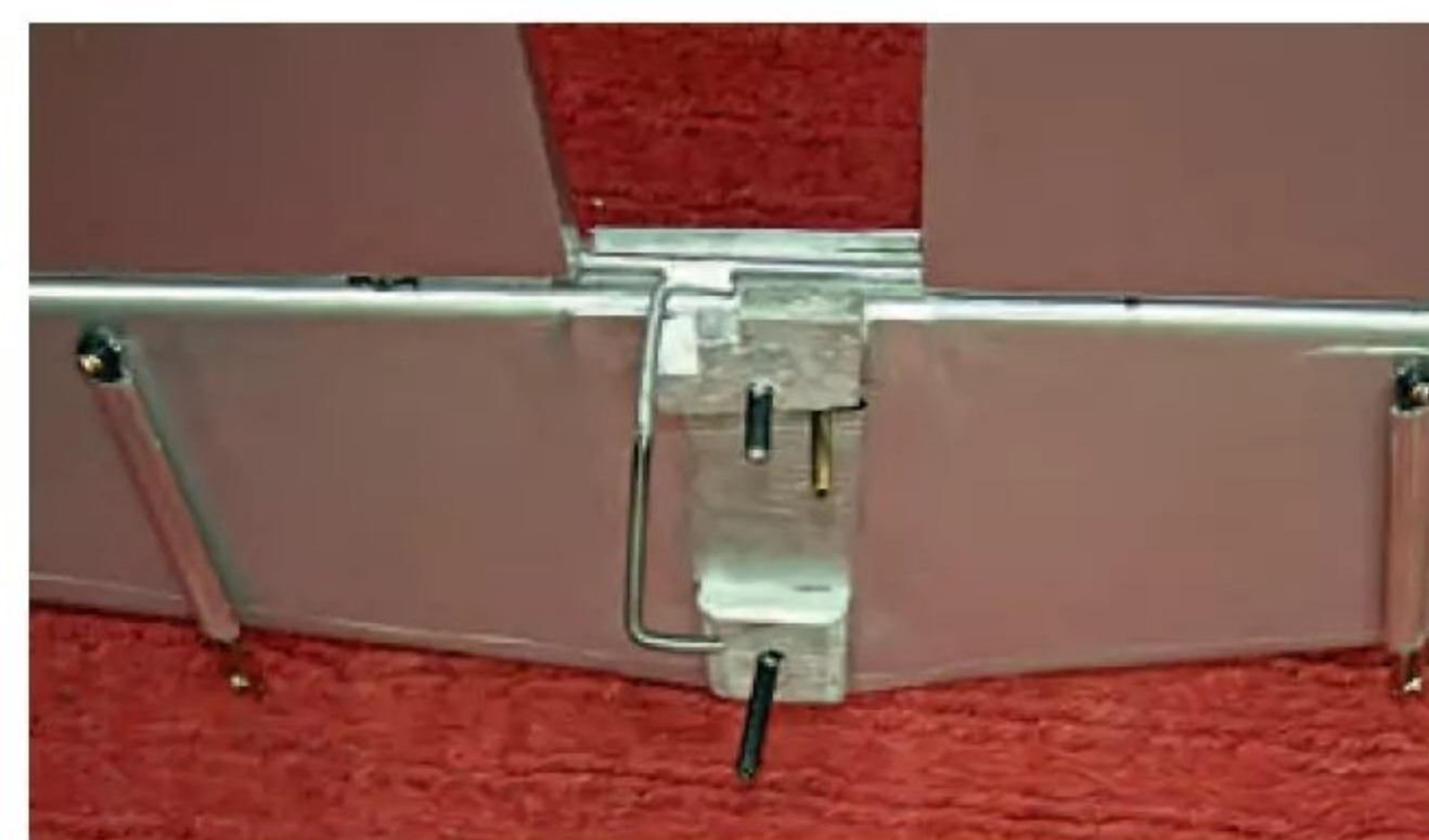
Fuselage to tailplane control linkages. This connection method has been in use for some time now on my Beverley model and has proved easy to use and reliable.
