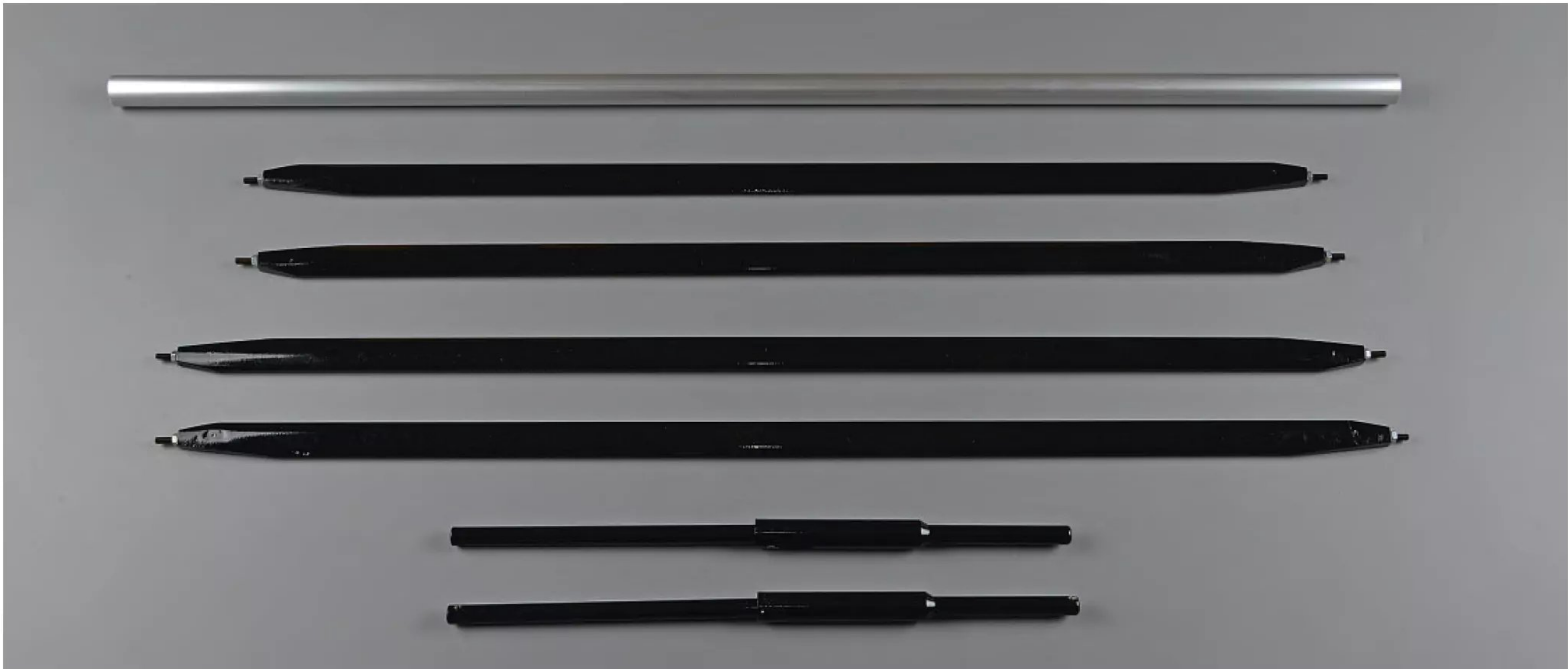
All the long bits laid out, including the ali wing tube, aerofoil shaped wing struts and the uber long shock absorbers.
