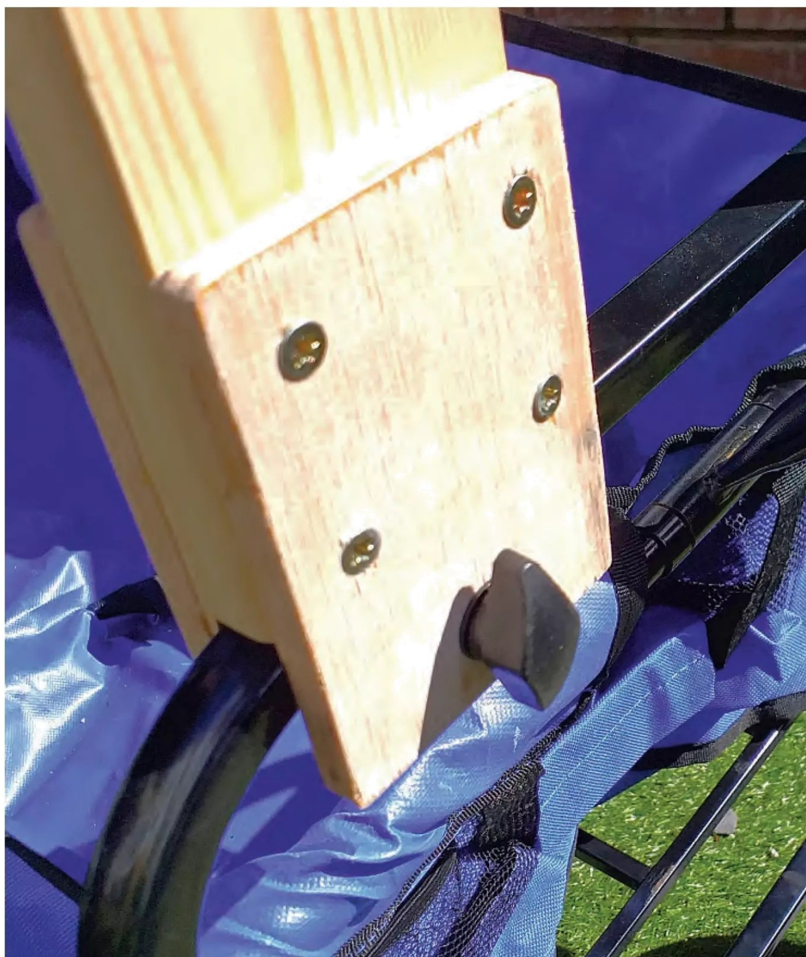
The 'Aircraft Carrier' flat top rests on the truck's upper frame and is clamped by long thumb screws.
