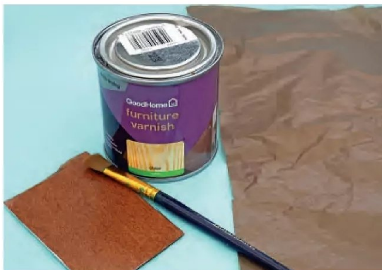
When coloured varnish didn’t work too well on balsa, I tried a test piece of brown tissue ‘doped’ on with acrylic varnish. Well, I think it works okay.
