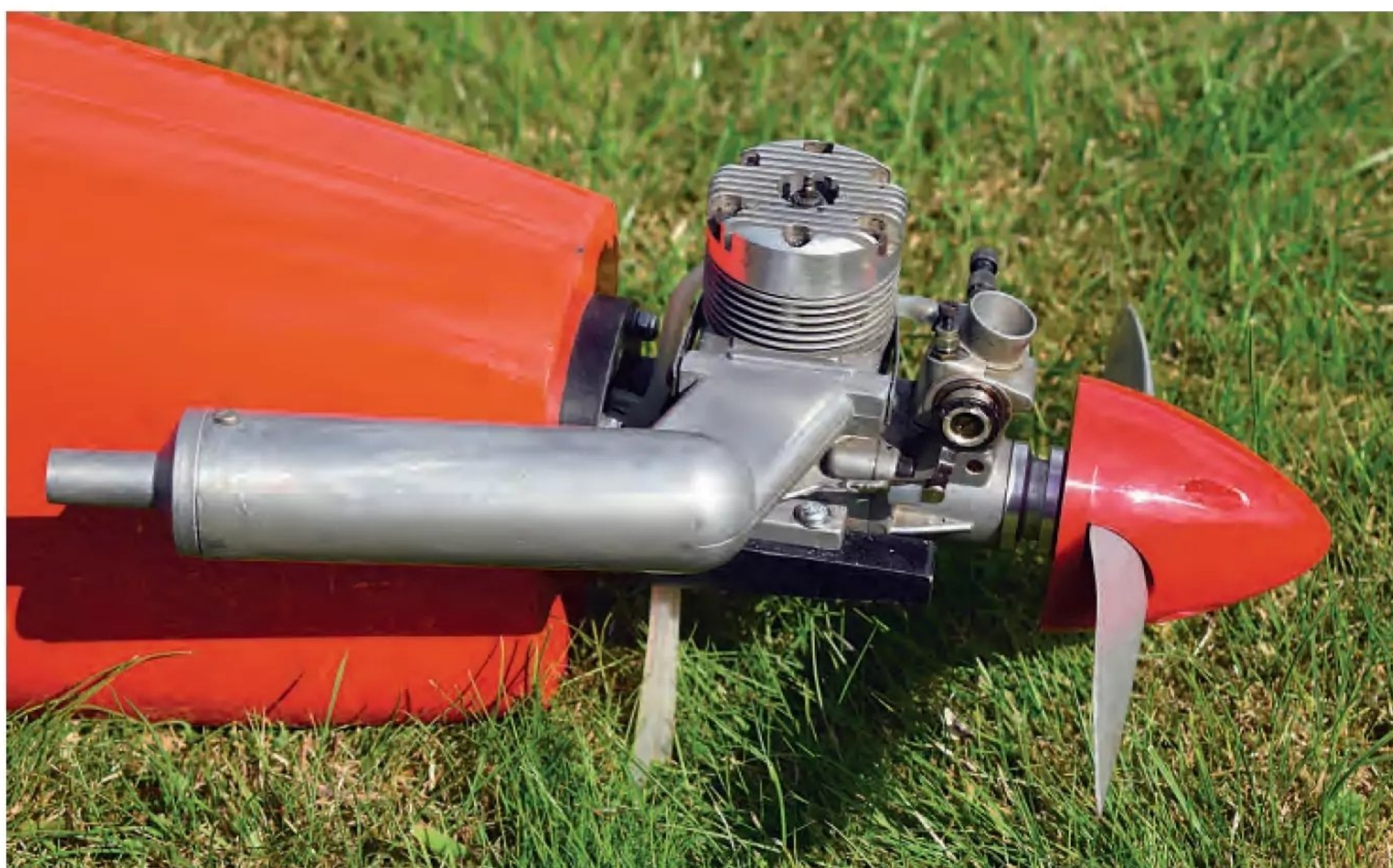
There's no problems servicing, cleaning or changing motors when they are mounted like this - and definitely no overheating issues.
