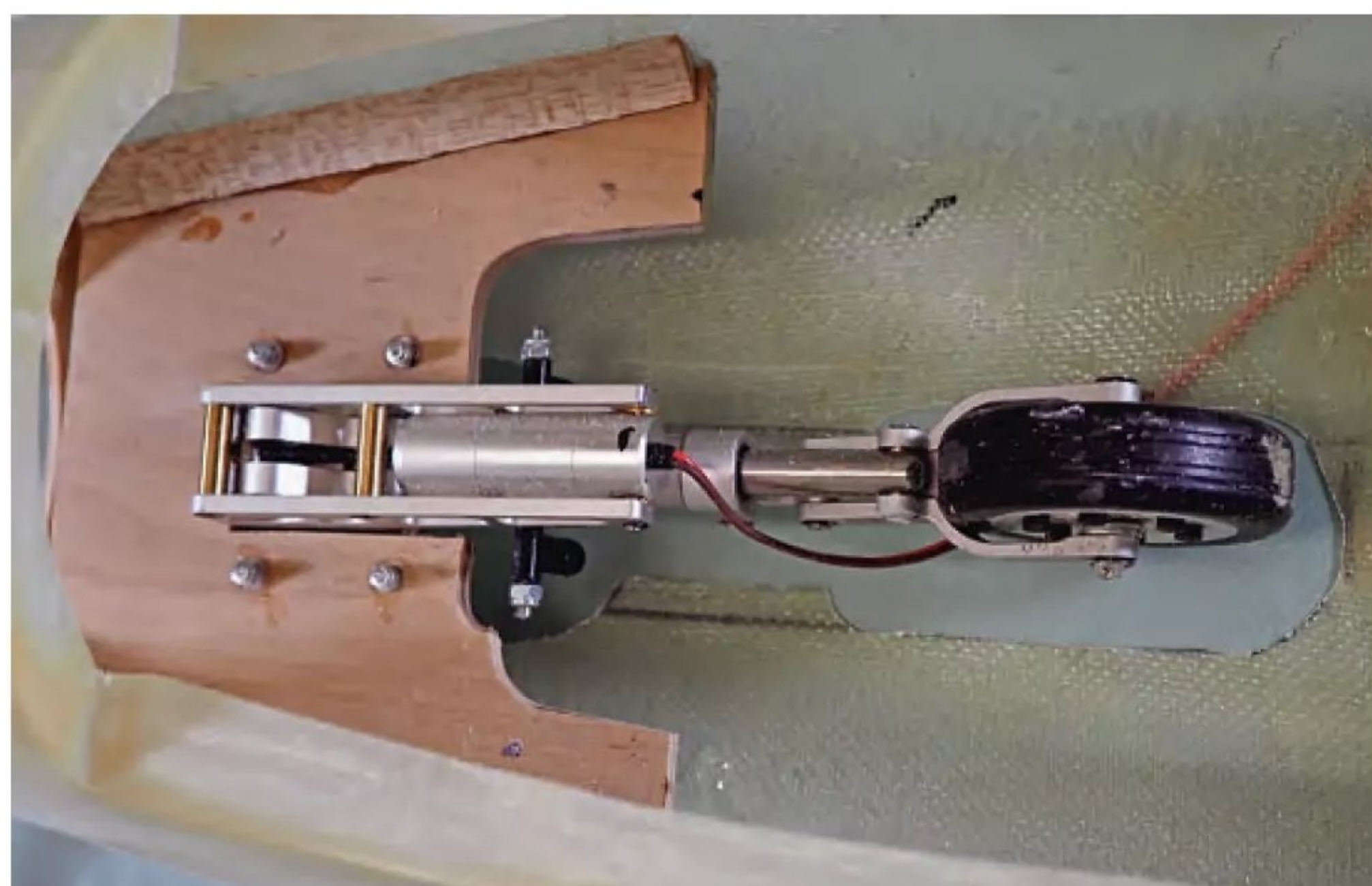
Nose retract unit mounted on its ply mount.
