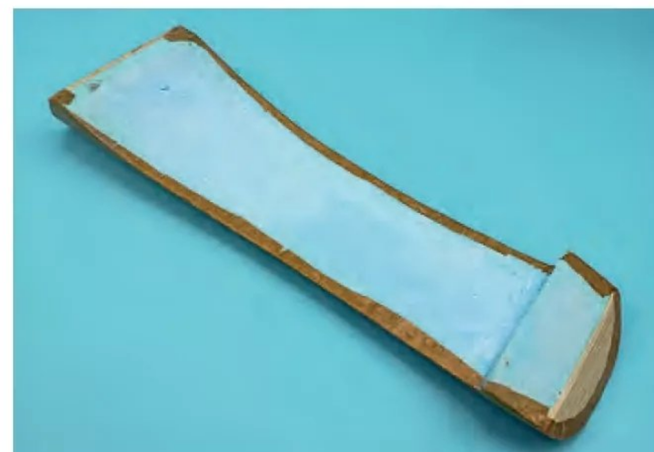
The fibreglass moulding that housed the parachute recovery system was missing on my model, so I used brown paper covered blue foam to replicate it. No need to hollow it out as I wasn't going to have that facility.
