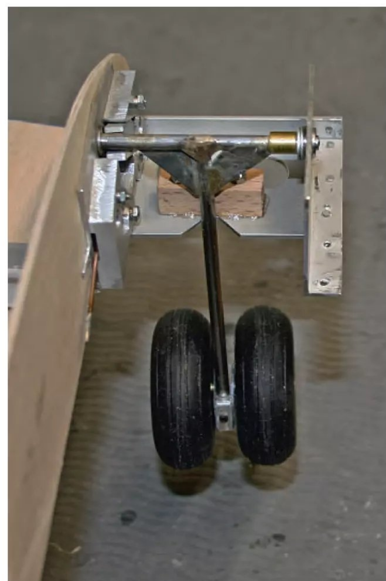
Test fit of the main retract unit.
