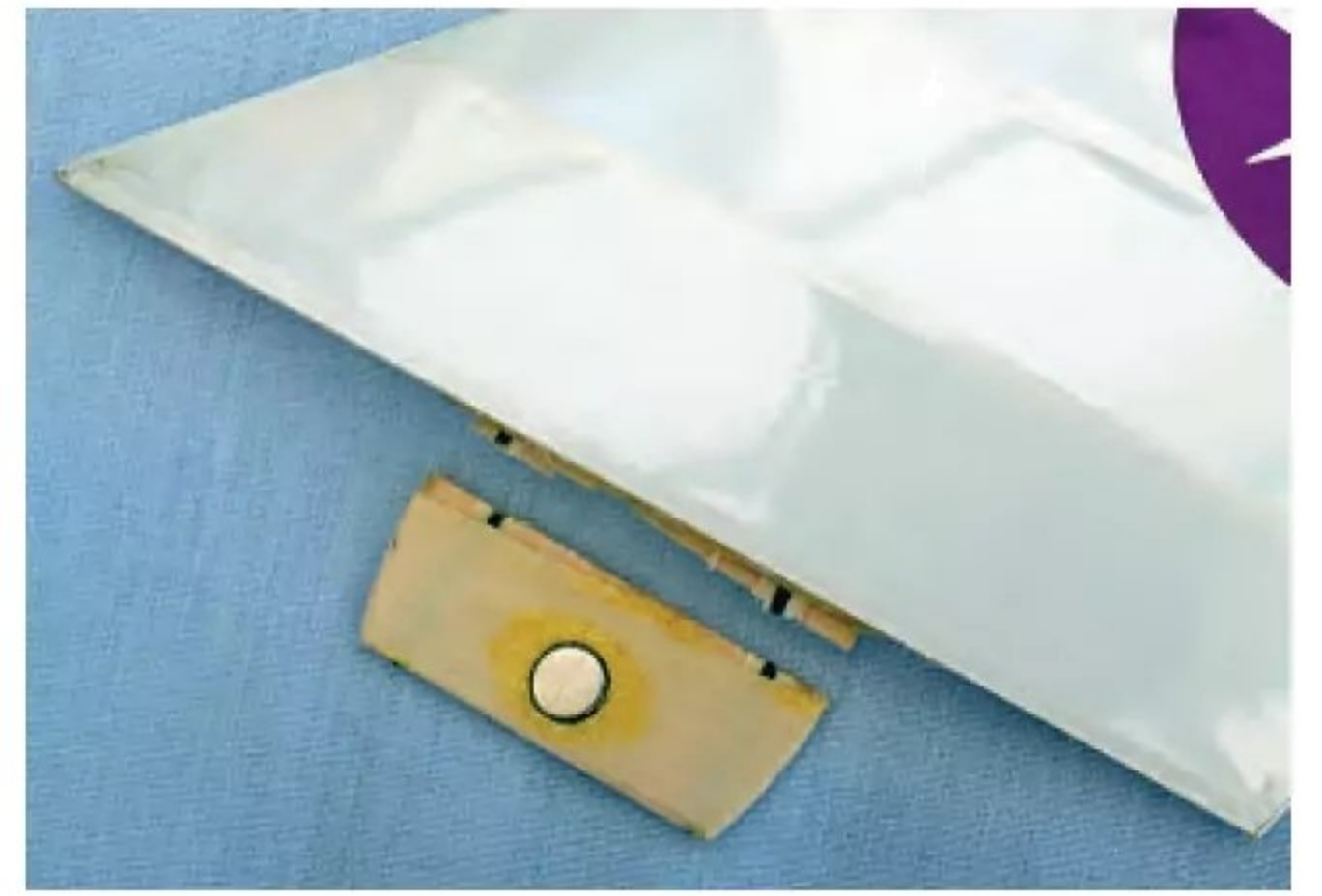
A problem since testing began. The fin locating tongue kept snapping off in bumpy landings.
