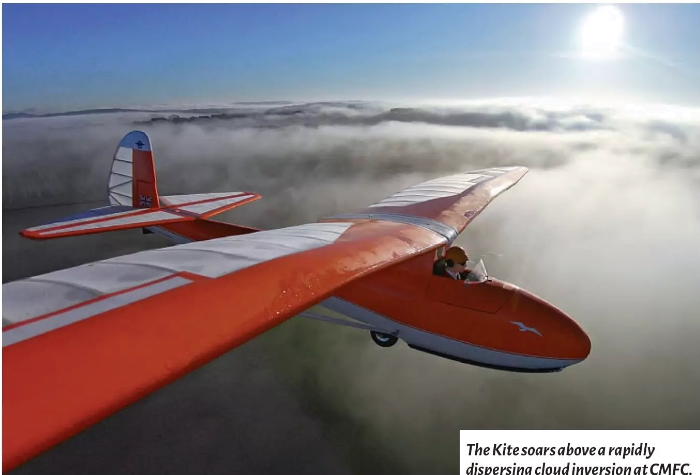
This shot shows the up-going ailerons deployed for glide path control.
