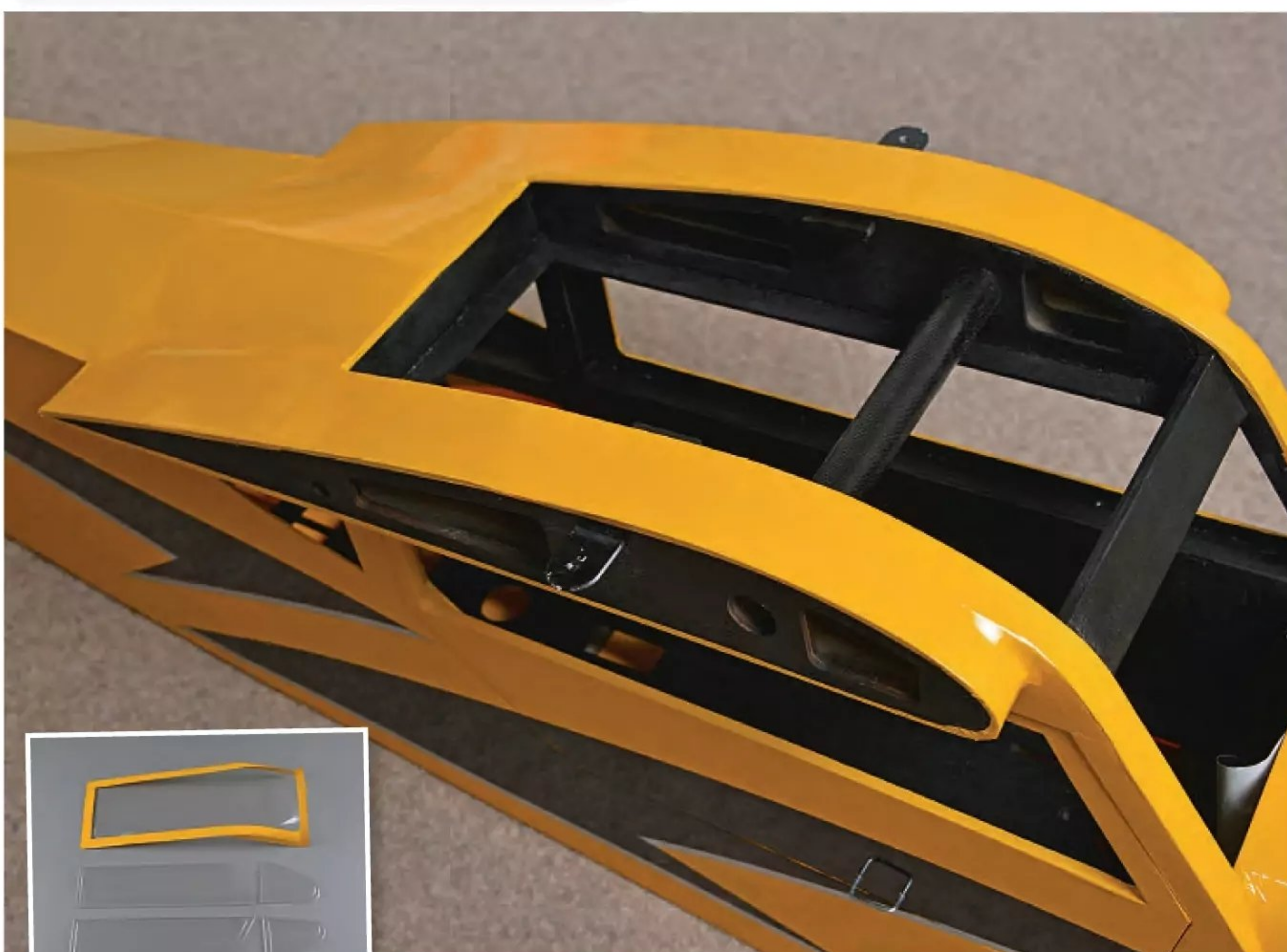
Clear mouldings are supplied for the cockpit windows and windscreen.
