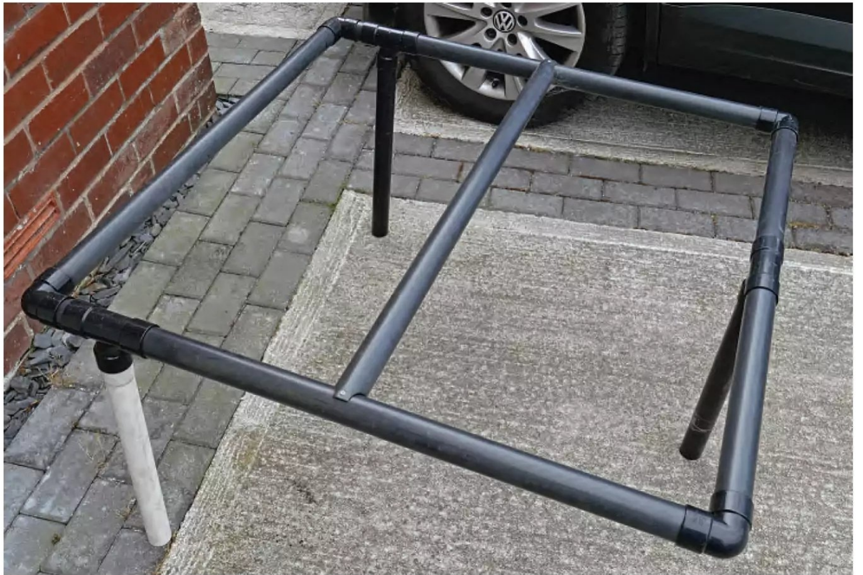
Yes, I agree, it's total bodgeneering! This is the demountable model carrying frame that I use in my car. My support gear sits underneath, with all the models resting/bungeed on top. All made from bits of left-over 40 mm plastic plumbing.
