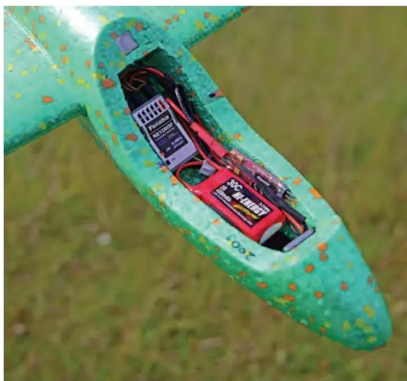
Scoop out the interior and there's plenty of room for a receiver and battery.
