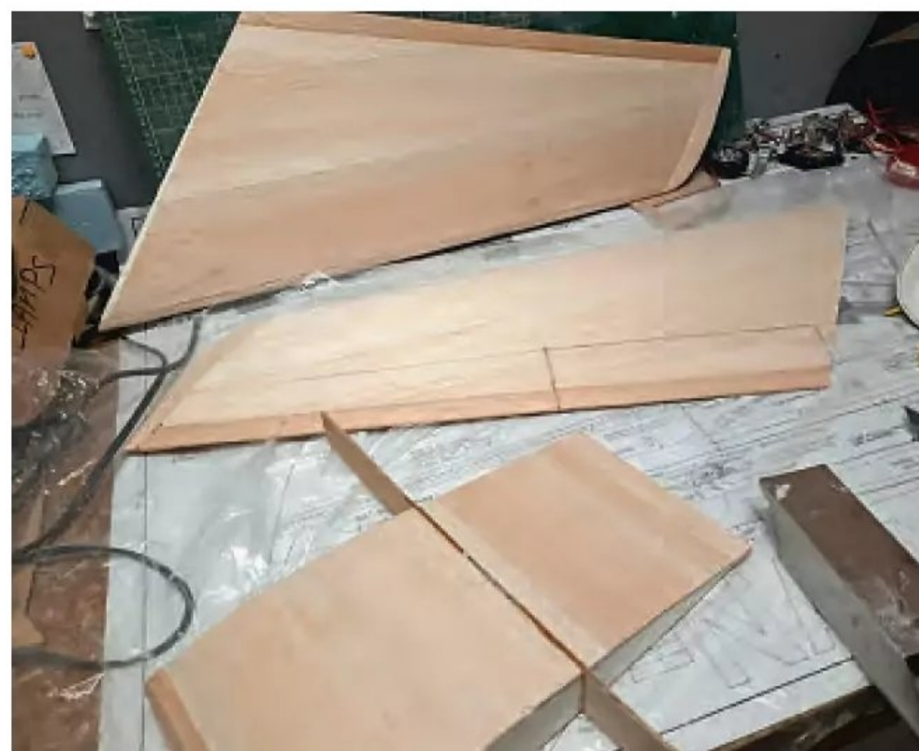
Wing cores laminated with 1.5 mm soft balsa and with the controls marked up, ready to cut out.
