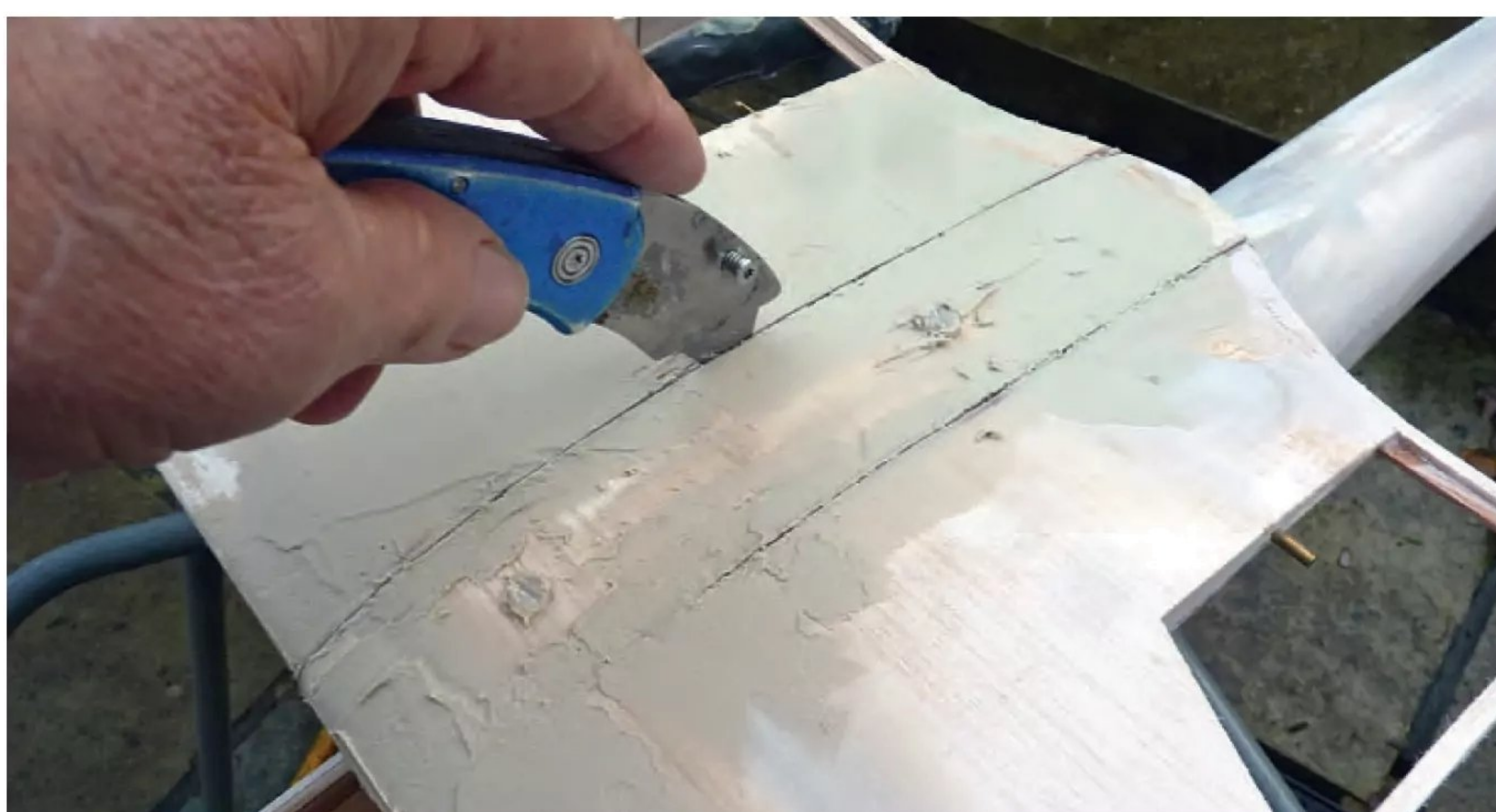
Score the filler applied to the centre section before it dries hard!
