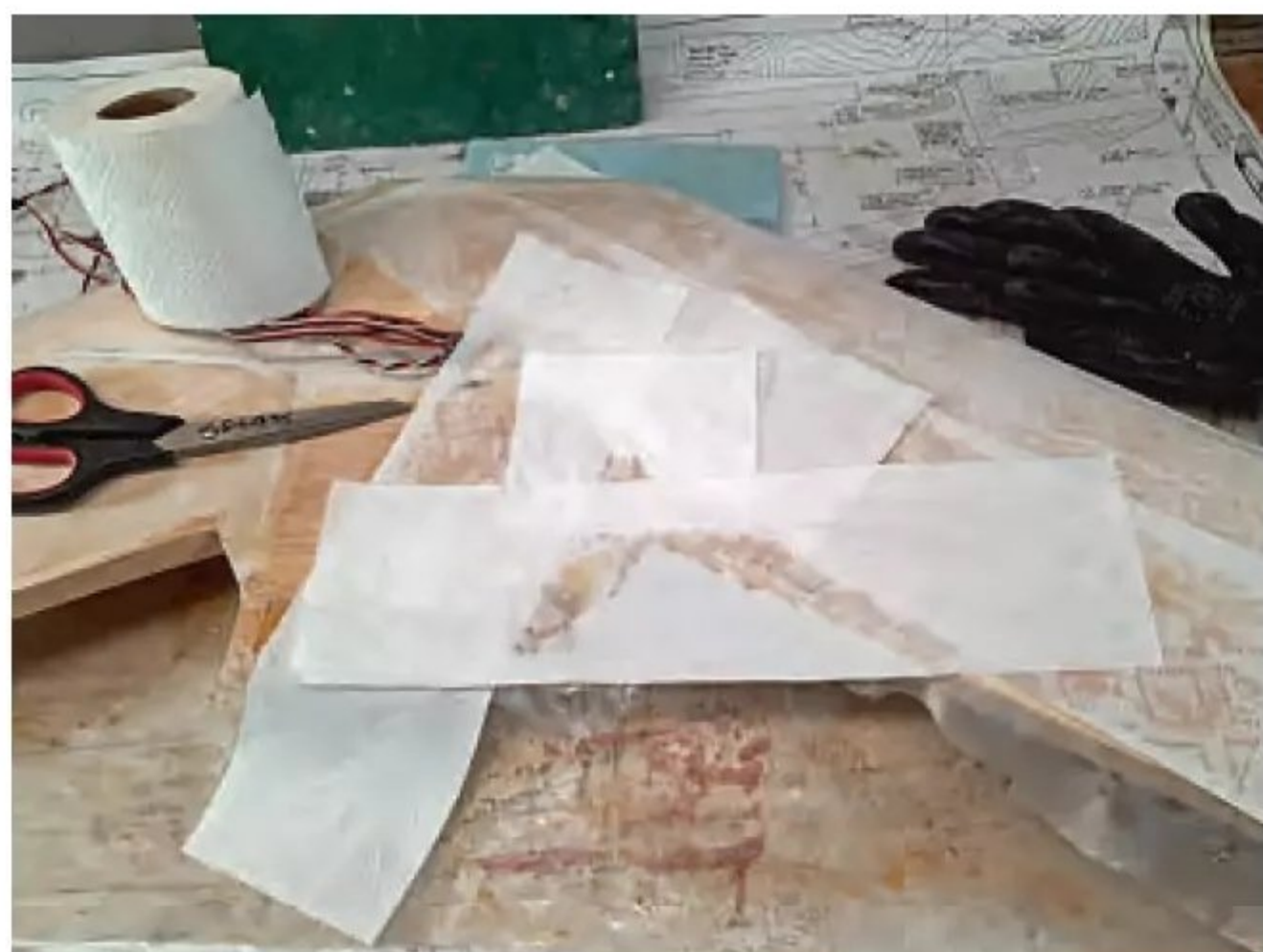
Lamination process underway, with toilet roll being used to soak up excess resin. The paper was rolled from the wing tip to the centre, absorbing resin along the way.
