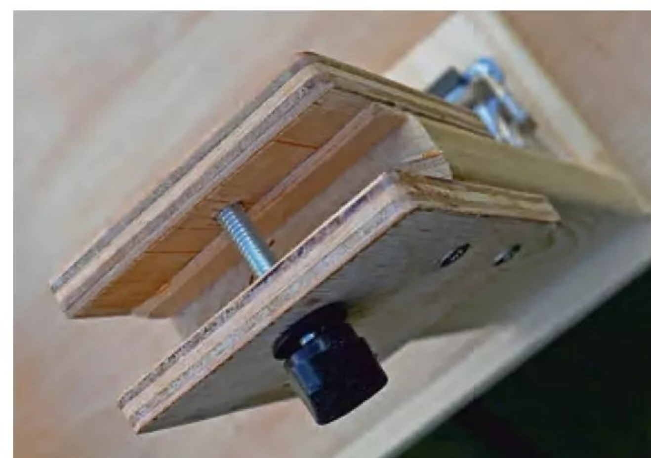
Detail of the clamp that secures the 'deck' to the truck frame. Easy and quick to make, solid in use.
