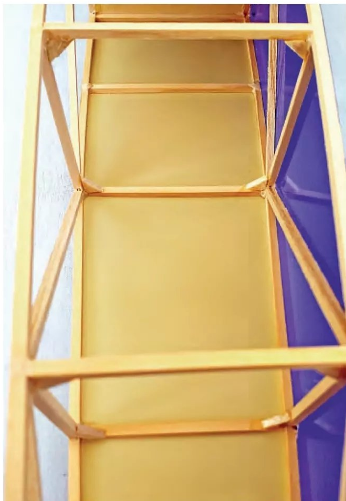
After self-imposed damage the Allen A-4 sports reinforcing gussets where they won't show through the covering.
