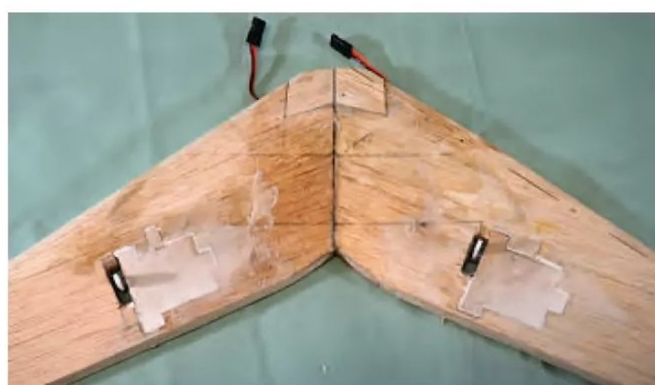
Holes were cut full depth of the tail for the elevator servos to sit in. They are hidden by a combination of light weight filler and thin balsa sheet.
