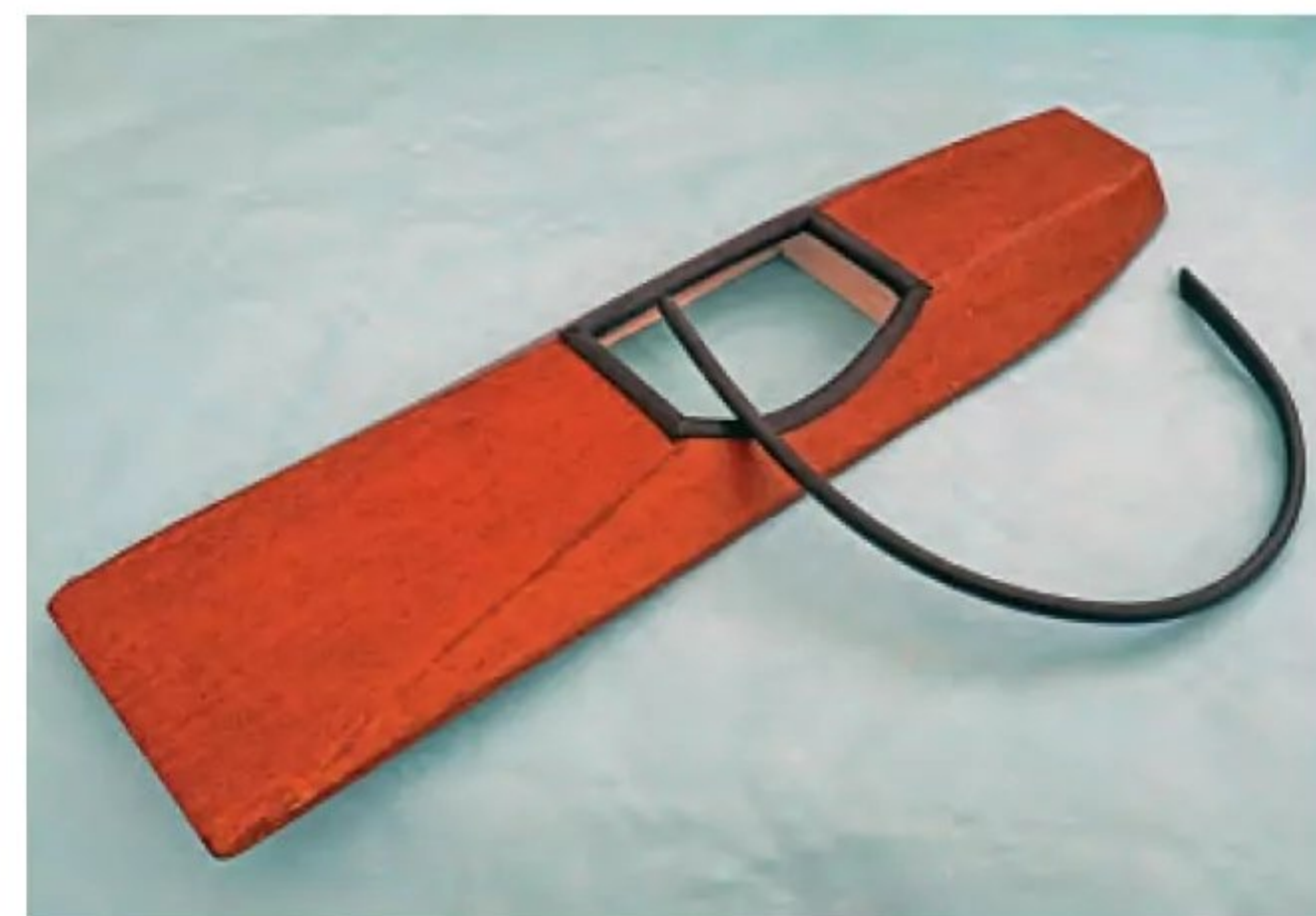
The Allen A-4 top deck after finishing with doped brown tissue. It looks like varnished ply, doesn’t it?
