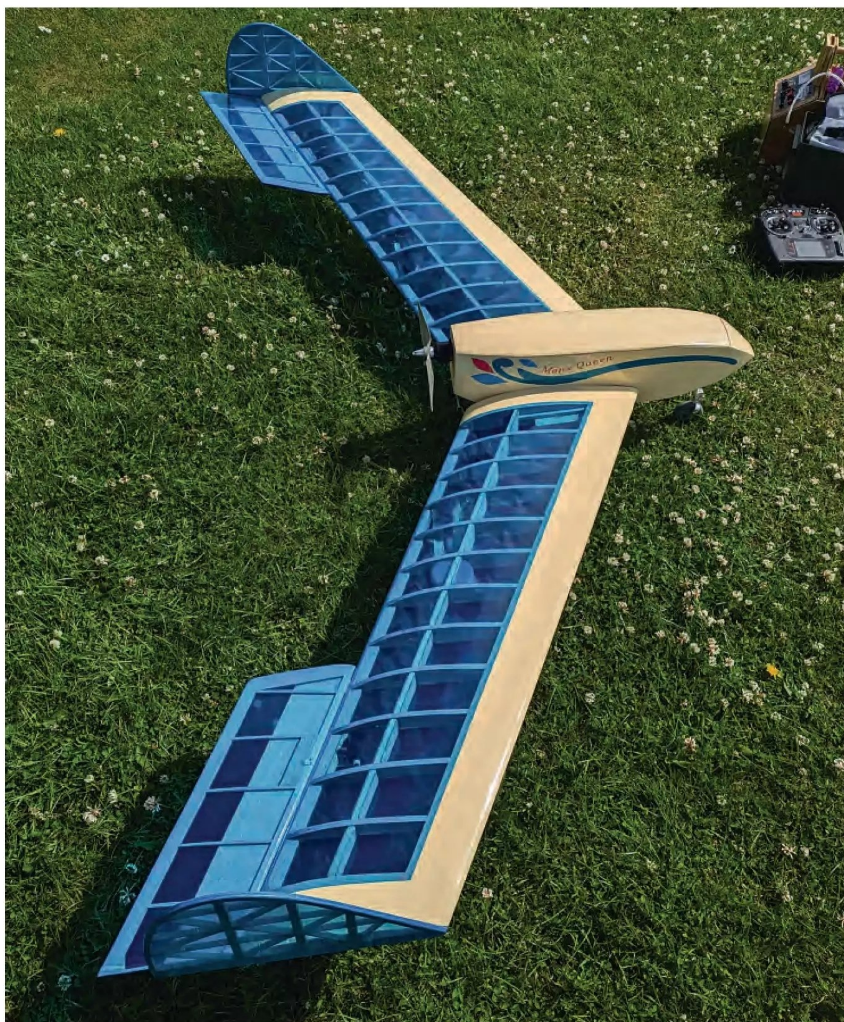
Another Manx Queen by Stuart Houston has modified wing tips and a retracting undercarriage.
