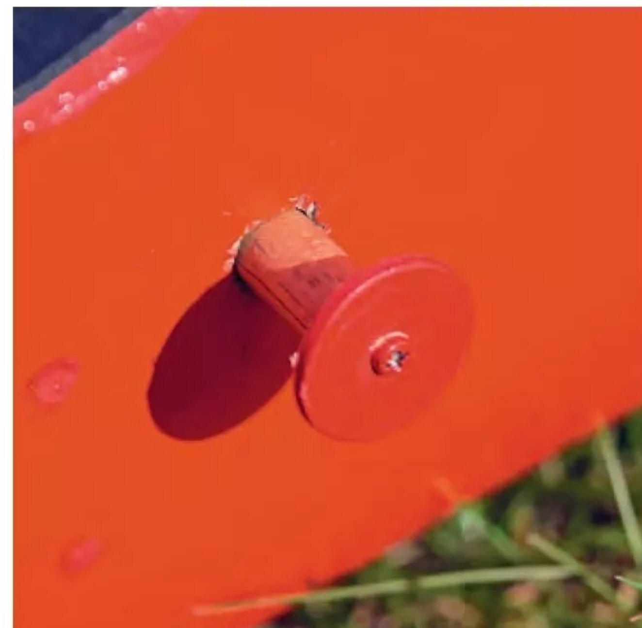
This is a little mod my old pal Phil Smith of Veron used on his models, especially ones with swept back leading edges. The ply discs stop the wing bands slipping off oily wing dowels.
