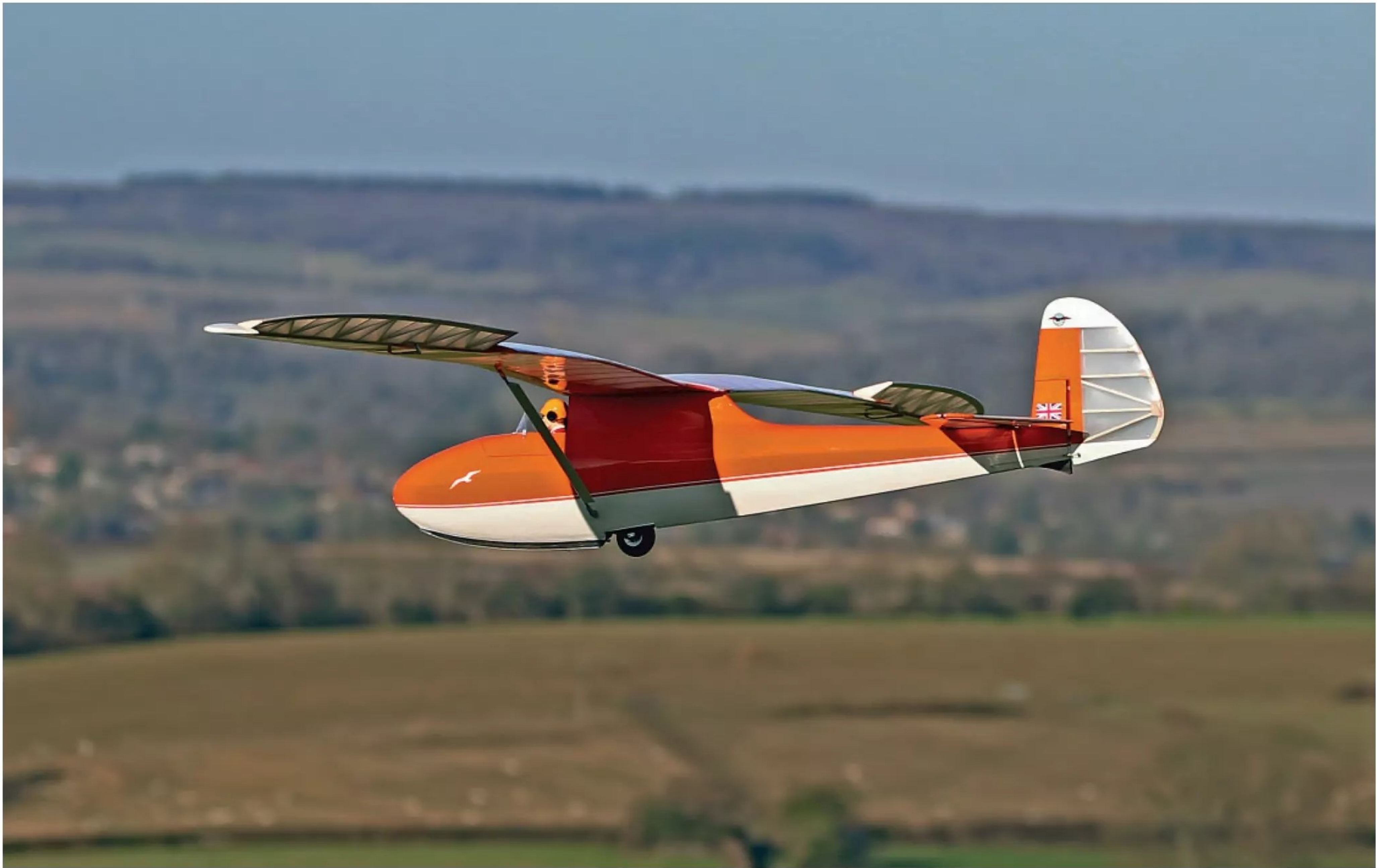
This shot shows the up-going ailerons deployed for glide path control.
