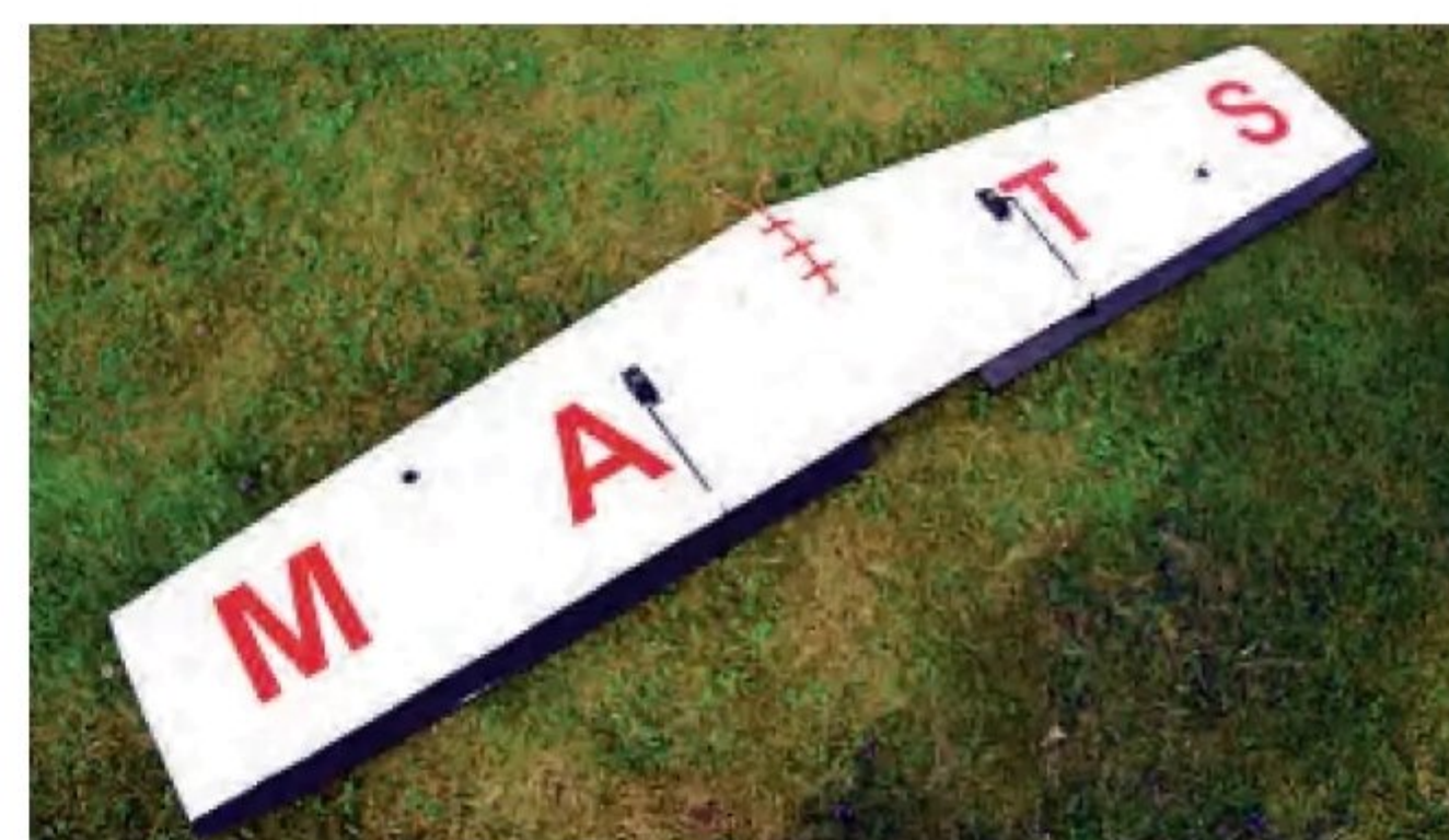
This was the only other mod I made. As new wings were required, two servos were utilised for the ailerons rather than the original's single centrally mounted set-up.
