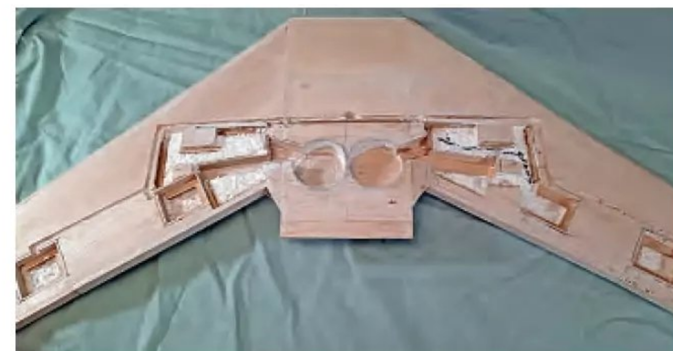
A busy wing underside with slots cut for retract units, wheel wells, and flap and aileron servos. Reinforcement was made with wing spars and glass-fibre laminations.
