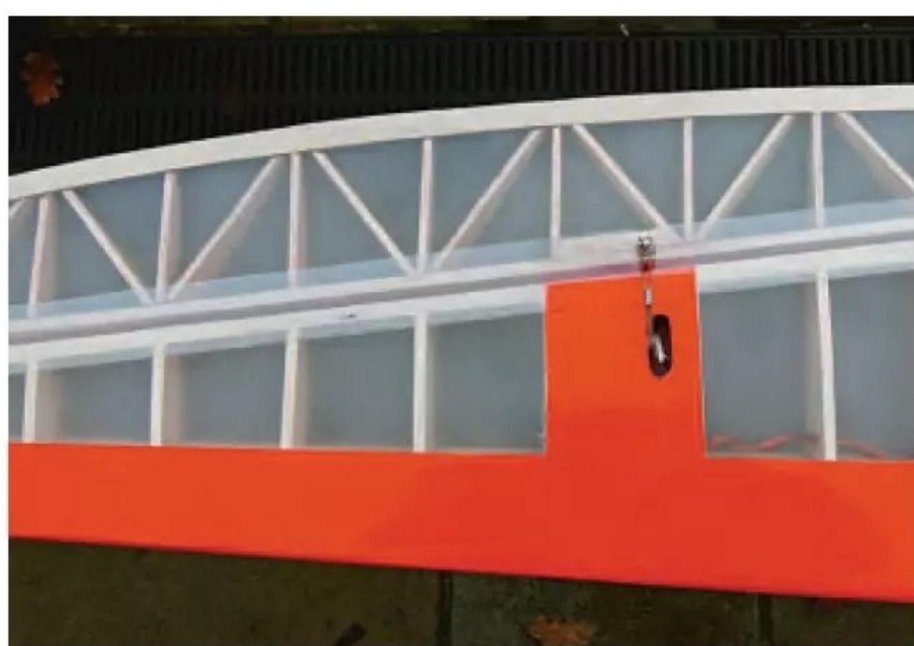
View of one of the aileron servo installations.
