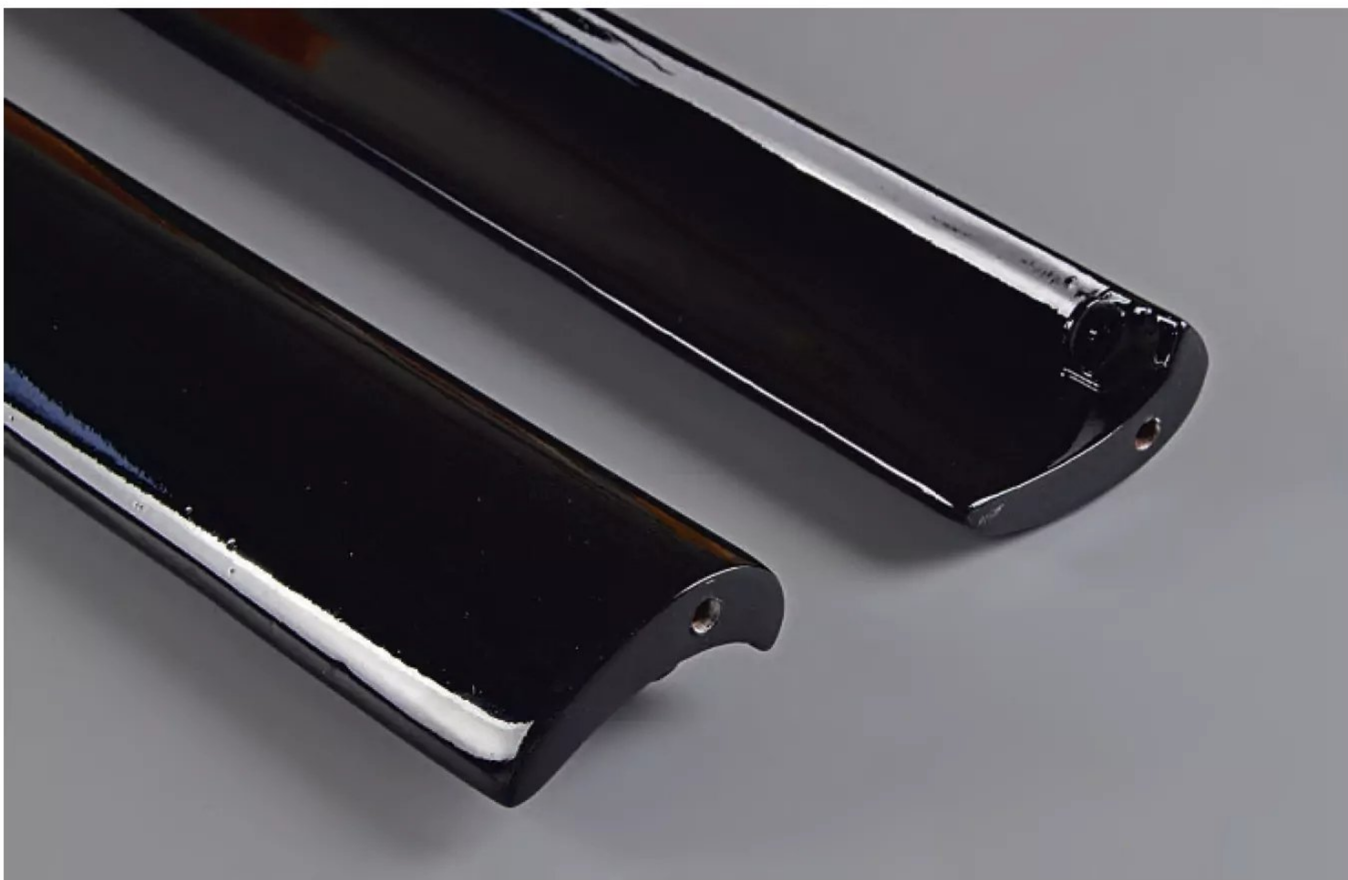
End detail of the full-length slats.
