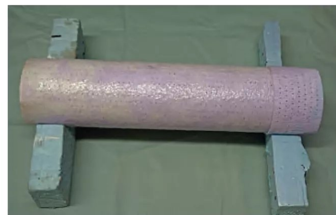
Final rear jet tube. The diameter reduces to 85% along the length of the pipe.
