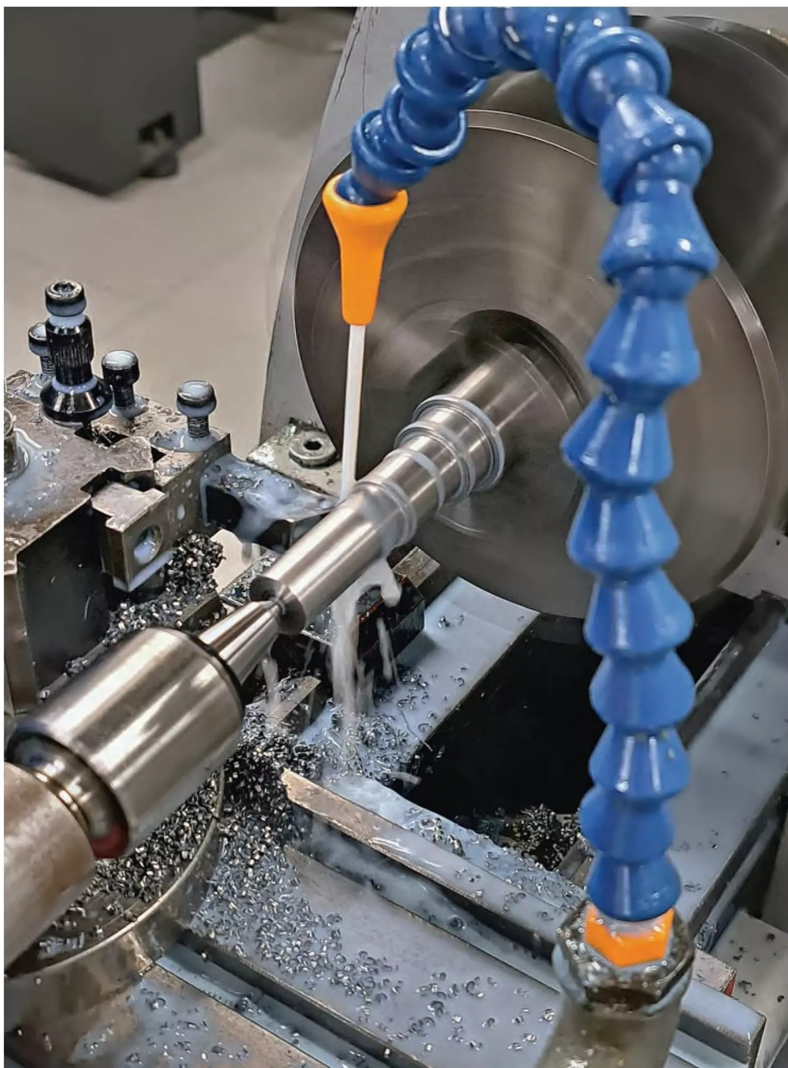
Turning the crankcase on the lathe.
