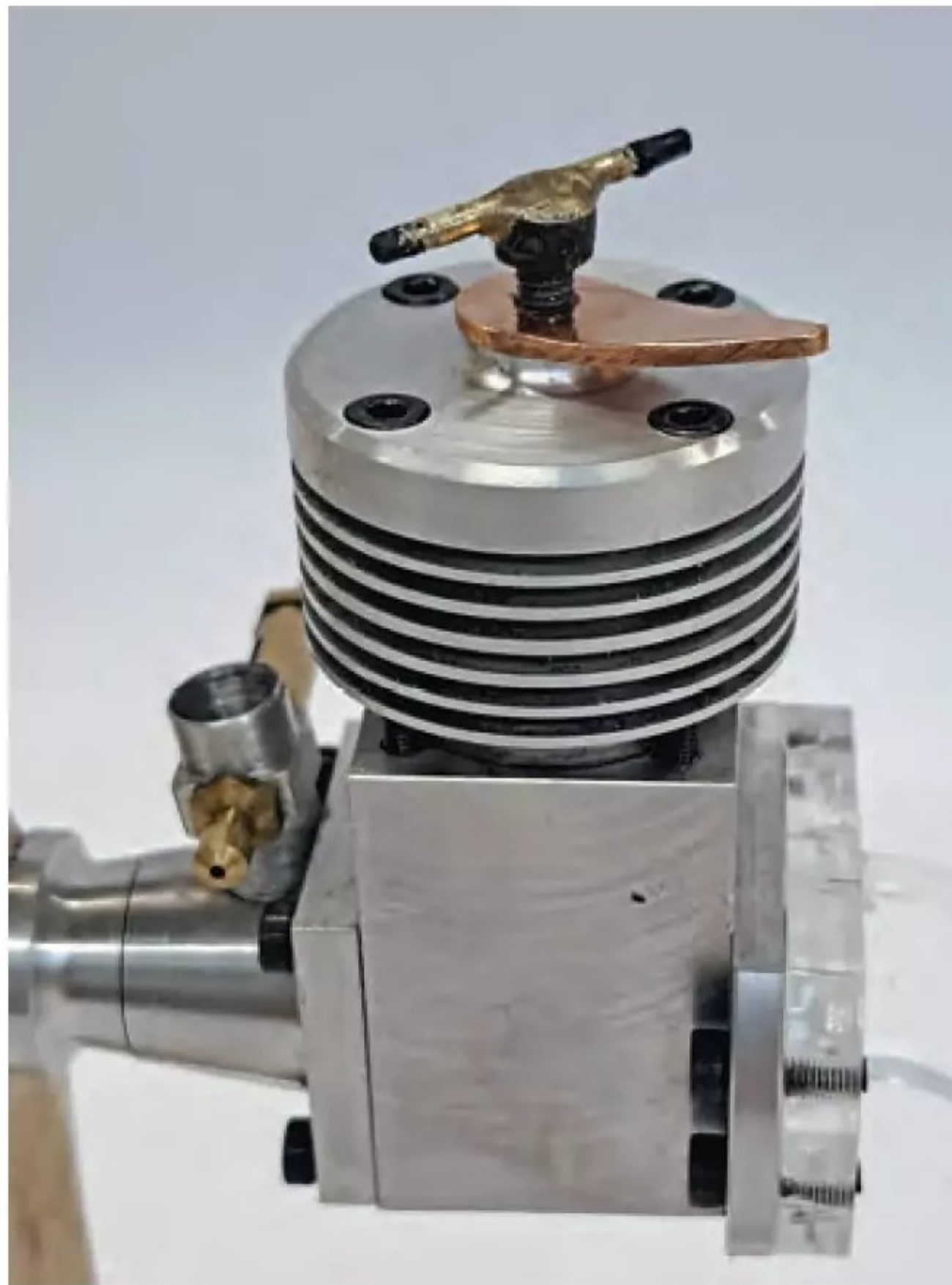
The engine runs well but is very sensitive to the compression screw setting. A locking lever made from 2 mm copper sheet keeps it in the desired position.
