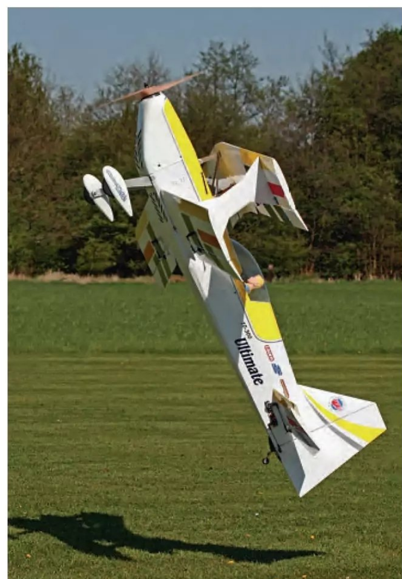
3D hover. Not truly vertical, it is reliant on thrust rather than lift and is definitely outside the envelope.
