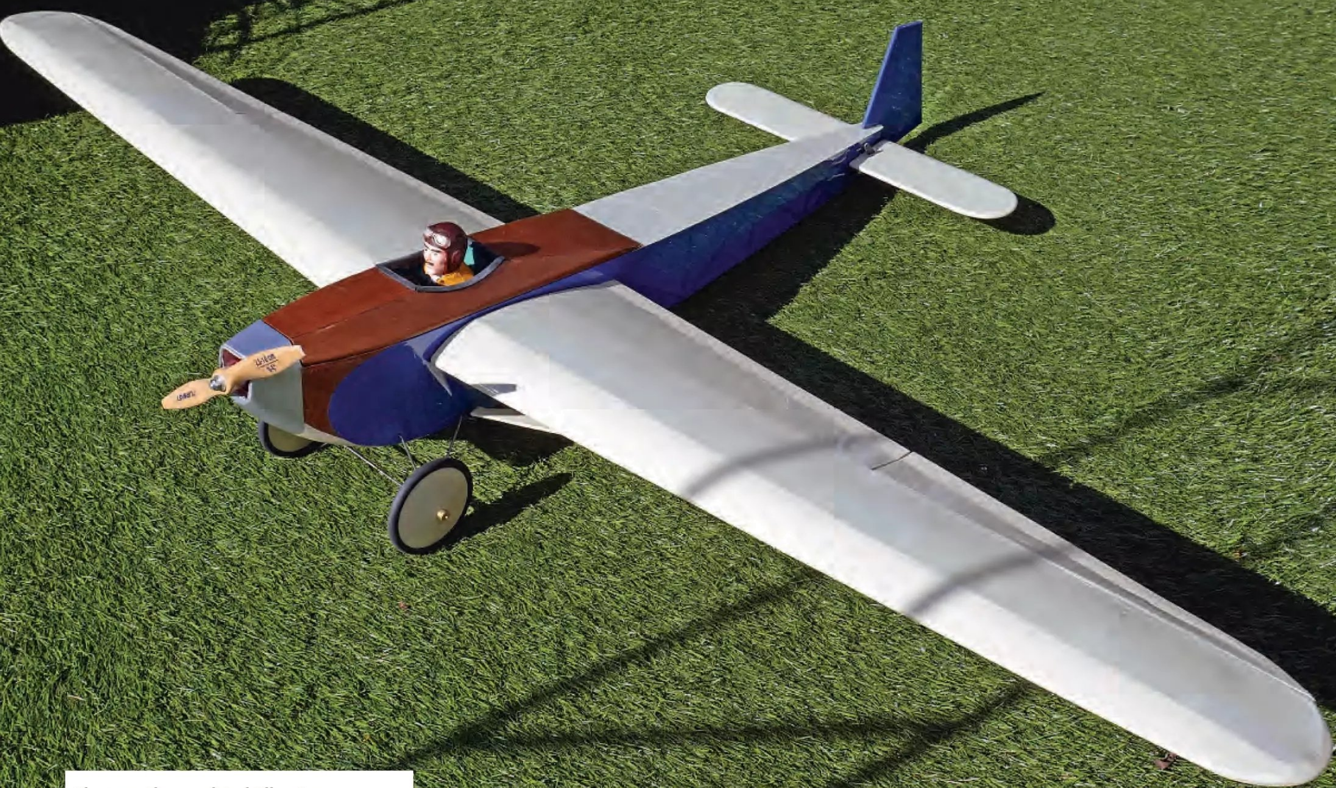
The recently completed Allen A-4 resplendent with a top deck finished with doped brown tissue. See 'Wood is Good?'
