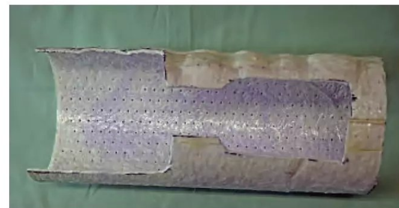
Homemade nose inlet tube cut to fit the nose-leg retract unit.
