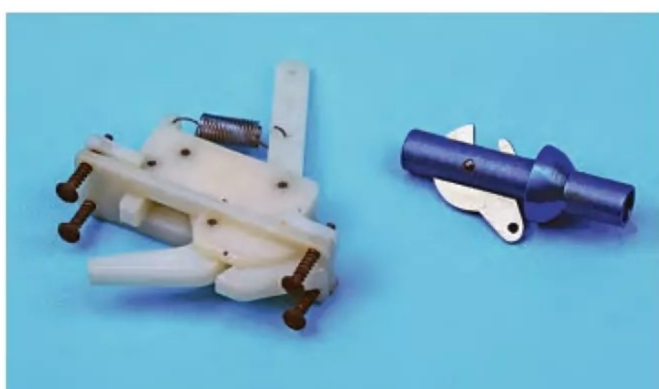
Servo operated tow hook and aero tow release mechanisms will be fitted after the test flights. That's assuming the front of the model doesn't need oodles of lead to get it balanced up.
