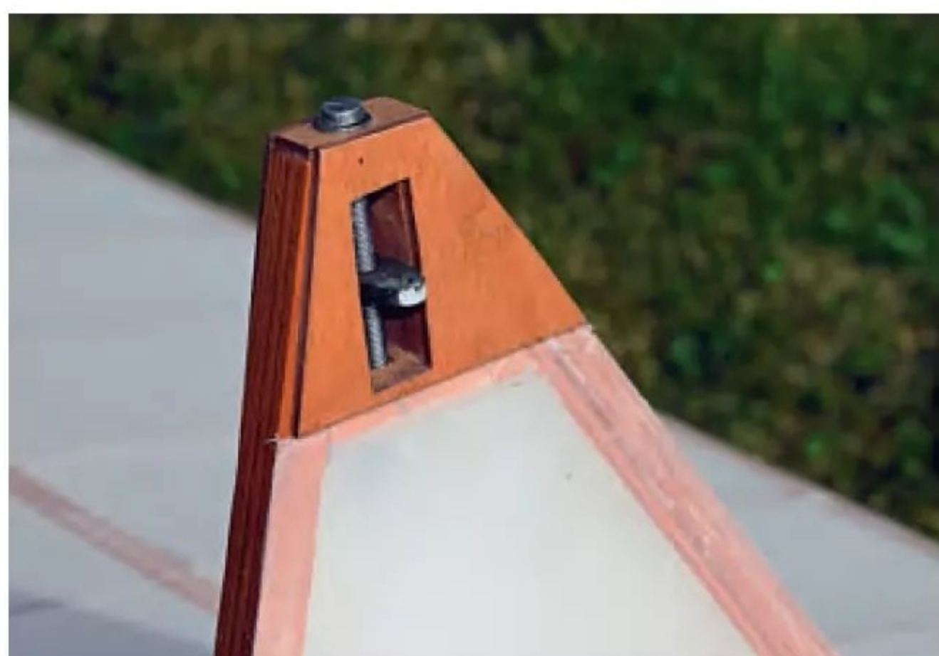
The pylon on top of the fuselage has an adjuster to tension the functional flying / landing wires.
