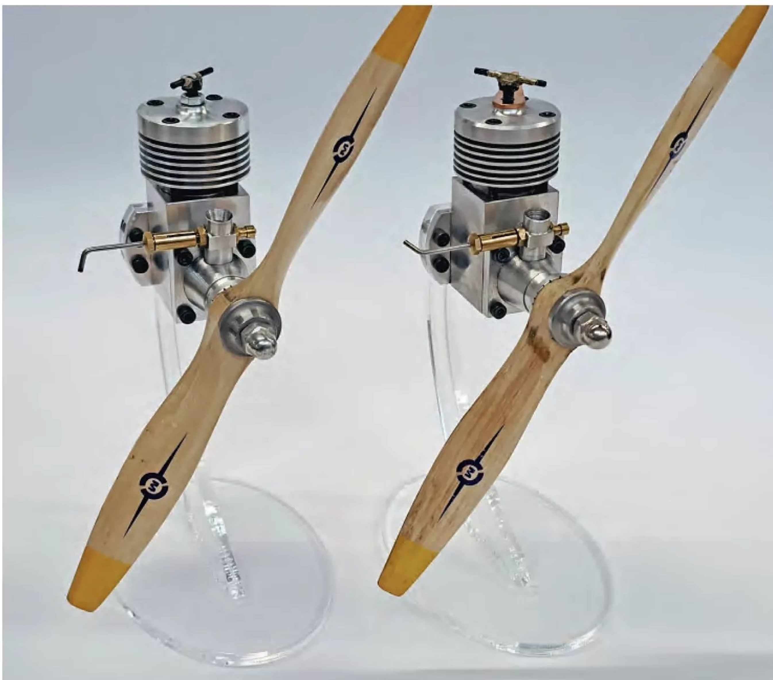
Peter teamed up with a work colleague so that they could both make a Holly Buddy engine. The pair of 2.5 cc diesels are seen here, looking dapper on their display stands.
