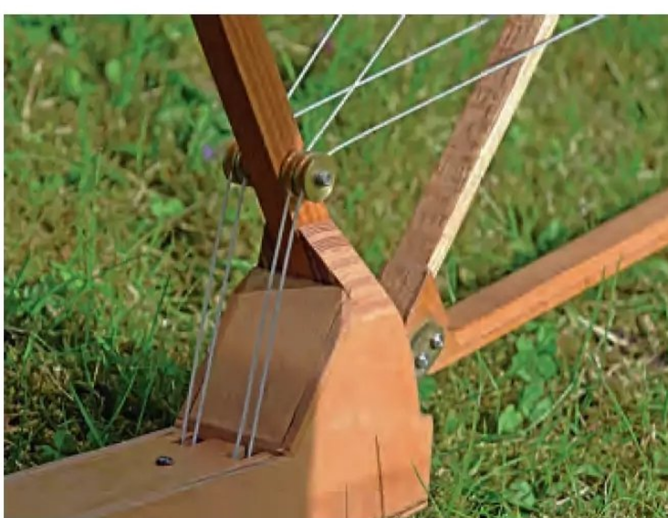
Working pulleys guide the rudder and elevator cables, just like the full-size.
