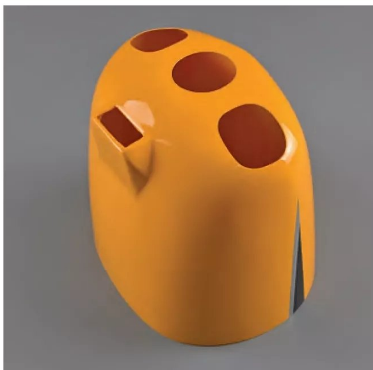
Front end is topped off by a nicely moulded and painted epoxy glass cowl.
